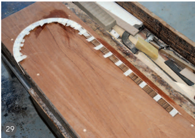
25 The zebrano strips were cut for yet more crossband effect 26 Small segments of zebrano kept safely while cutting and laying out the circles 27 Straight zebrano banding with light coloured lines glued to each edge 28 One of the circles laboriously cut on an electric scrollsaw with great care 29 Creating part of the 'overlap' marquetry for the drawer fronts 30 The square shape before the 'overlap' circle is added. Note the contrast between aged and new zebrano
