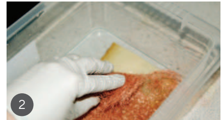
The holly veneer was placed in a sealed container under a layer of copper wire wool with distilled vinegar poured on top
