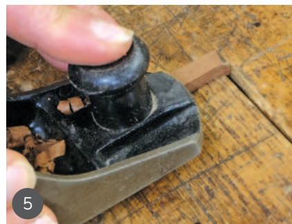
1 The drawer front with the broken section of handle 2 Positioning the broken section to assess what was missing 3 A template cut to shape for the back infill piece 4 Cutting the ends to form the joint on the drawer front 5 A block plane cutting the angled side of the infill piece 6 Using a chisel to shape the angled ends on the infill section of timber
