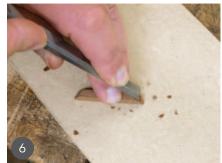
1 The drawer front with the broken section of handle 2 Positioning the broken section to assess what was missing 3 A template cut to shape for the back infill piece 4 Cutting the ends to form the joint on the drawer front 5 A block plane cutting the angled side of the infill piece 6 Using a chisel to shape the angled ends on the infill section of timber
