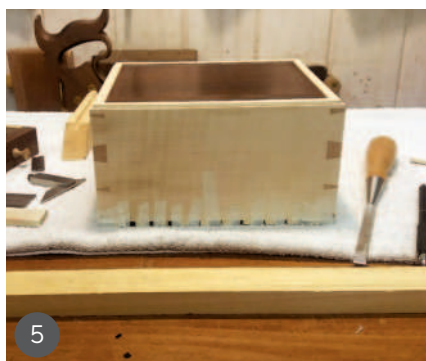
1 Making the through dovetails 2 The box ready for the inlays 3 The carcass sawn in two 4 Gluing the inlays in the bottom 5 Gluing the inlays in the top 6 The inlays done and planed flush with the carcass
