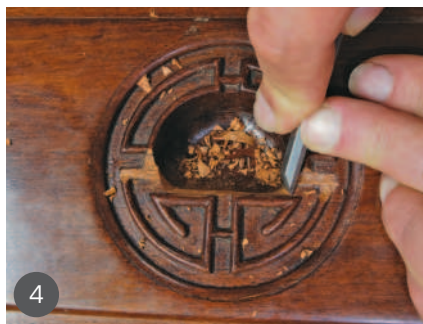
1 The drawer front with the broken section of handle 2 Positioning the broken section to assess what was missing 3 A template cut to shape for the back infill piece 4 Cutting the ends to form the joint on the drawer front 5 A block plane cutting the angled side of the infill piece 6 Using a chisel to shape the angled ends on the infill section of timber
