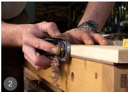
1 2mm-thick American walnut veneer with distinctive grain 2 Trimming the thin solid sections of walnut for the legs and carcass edges 3 Bonding the walnut veneer to the pre-sized blockboard cores 4 A Mafell Duo-Doweller used to join the carcass sections together 5 The basic carcass dry assembled for checking and marking out 6 Thick walnut veneer over spruce cores for the leg material 7 Trying out the fit of a projecting handgrip on a curved door edge section
