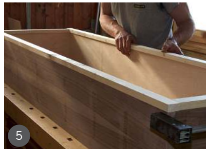
1 2mm-thick American walnut veneer with distinctive grain 2 Trimming the thin solid sections of walnut for the legs and carcass edges 3 Bonding the walnut veneer to the pre-sized blockboard cores 4 A Mafell Duo-Doweller used to join the carcass sections together 5 The basic carcass dry assembled for checking and marking out 6 Thick walnut veneer over spruce cores for the leg material 7 Trying out the fit of a projecting handgrip on a curved door edge section
