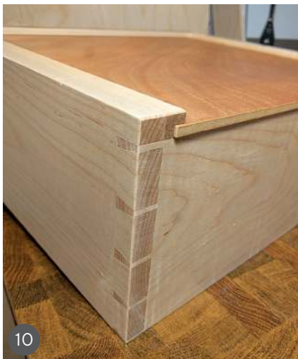
7 The cutaway to accommodate the rear of the drawer where the drawer bottom will be inserted 8 Plenty of clamps are needed to hold the slips precisely in place during glue-up 9 The result is a very neat, pleasing appearance ready for the drawer bottom 10 A very tidy result showing the layout of the dovetails relative to the drawer bottom 11 An equally tidy appearance in the internal corner of the drawer
