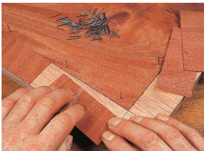
The central panel is held in place with veneer pins while fitting the cross-banding
