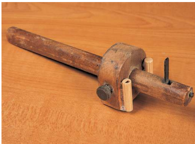
A modified cutting gauge for working with curved groundwork
