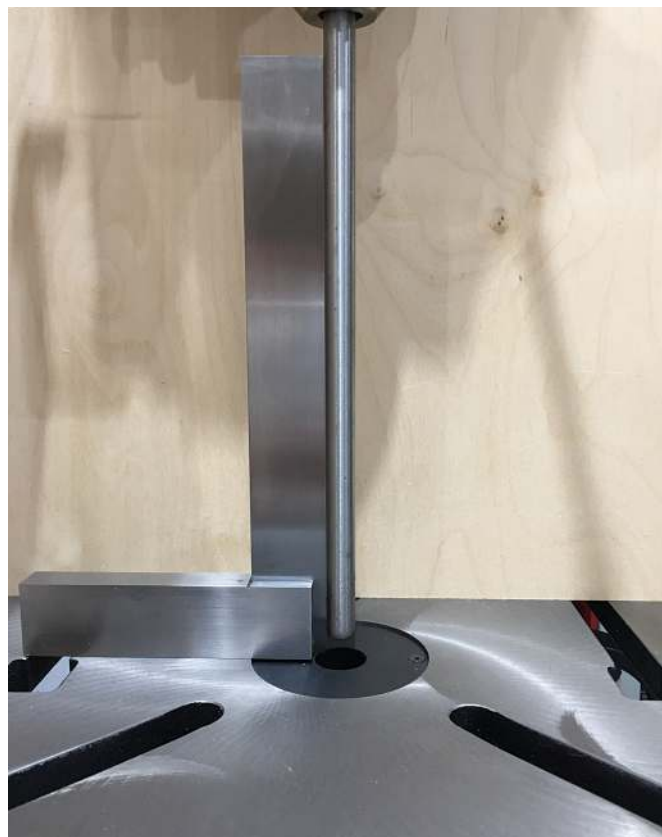
You need to use an accurate square and the longer the more accurate
