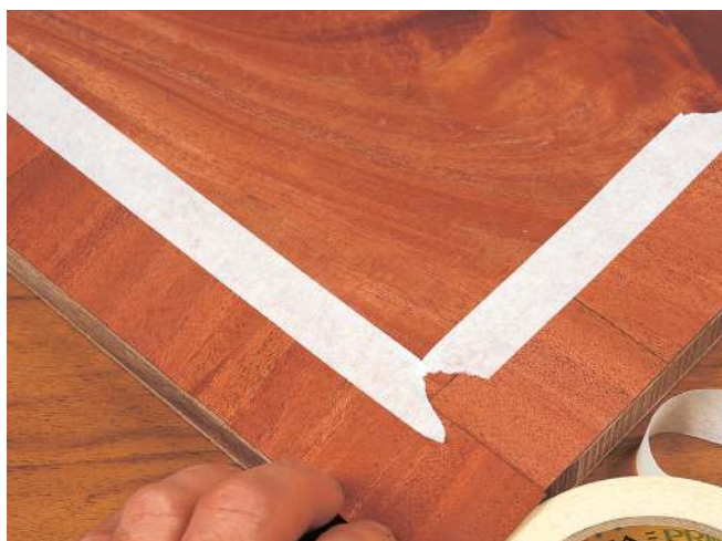
The cross-banding fitted and taped to the central panel. The overlap at the corners is suitable for a butt joint
