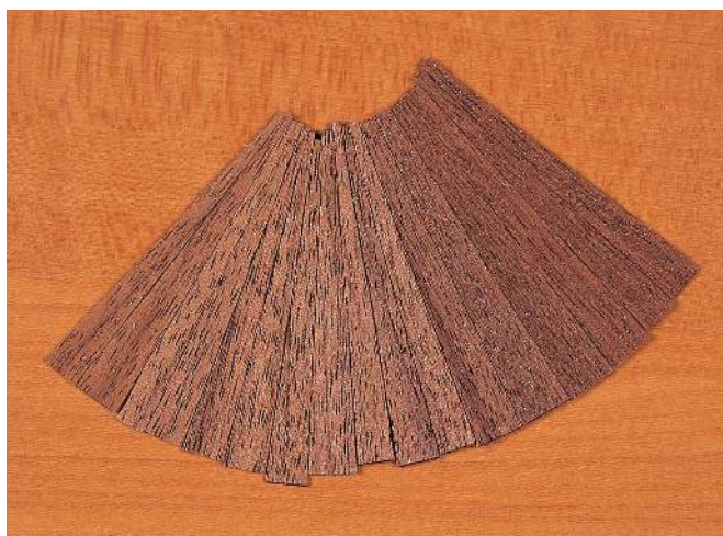
Prefabricate the veneer for the corner: it is a lot easier than trying to lay several small sections of veneer with accurate joints
