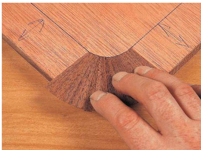
Rubbing the prefabricated corner into place. This is done by sliding the veneer into position. The natural grab of pearl glue will hold it in place
