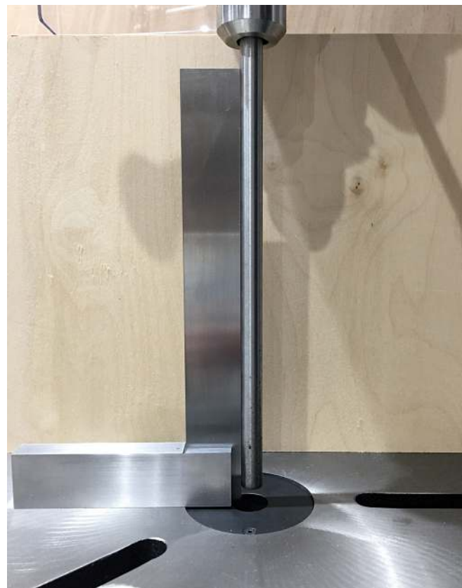
You can just see the gap at the top and rotating the bar 180^\circ the gap was at the bottom. The difference in the gaps equalled 0.01mm or 0.025^\circ – I'd say that was pretty accurate
