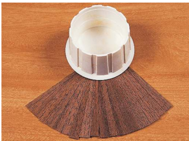
Use the template to make the inner curved edge to the corner cross-banding
