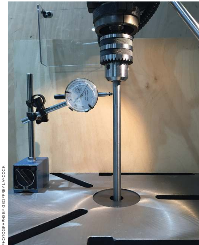
Using a good quality dial gauge and a magnetic stand makes it much easier
