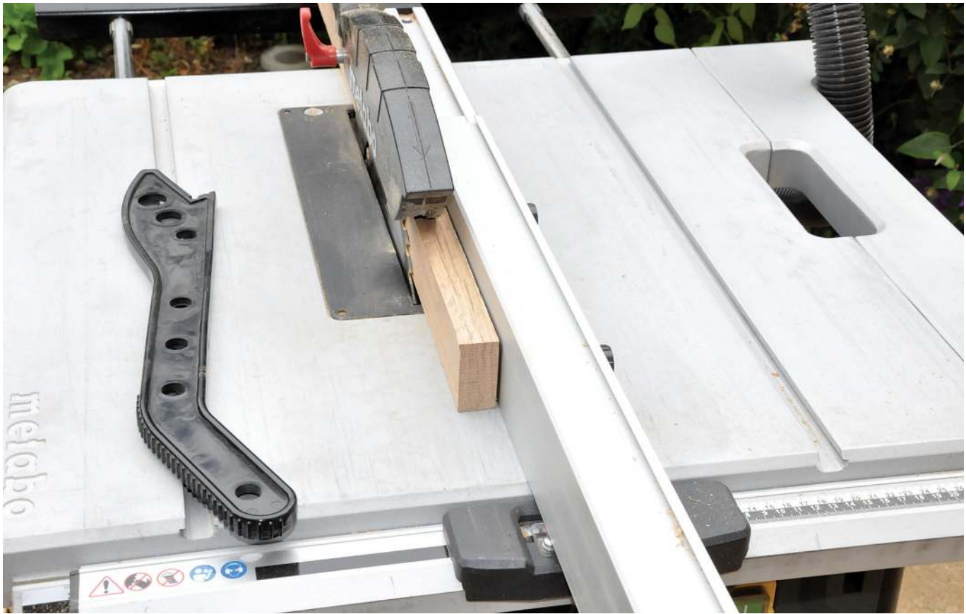
Set-up for typical rip sawing. The fence face is slid forwards, the blade has been adjusted so the teeth are just clear of the timber upper surface and the guard is as low as possible. The thin push stick allows passage to the side of the top guard
