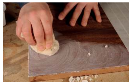
Using grain filler to level the surface of the wood before sealing and French polishing
