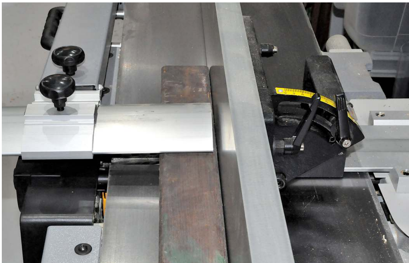
Planer/surfacers/jointer set up per European rules for surfacing, with the guard as low as possible to the timber surface to minimise risk of cutter contact. Note the guard attached to the rear of the fence automatically covers the cutter block behind the fence
