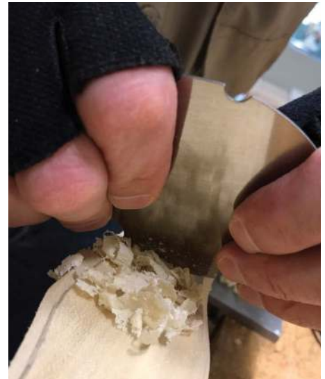
A convex scraper refines the surface
