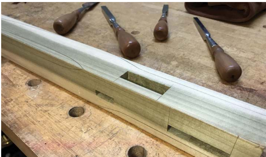
Be certain to lay out and excavate mortises before cutting to your pattern lines
