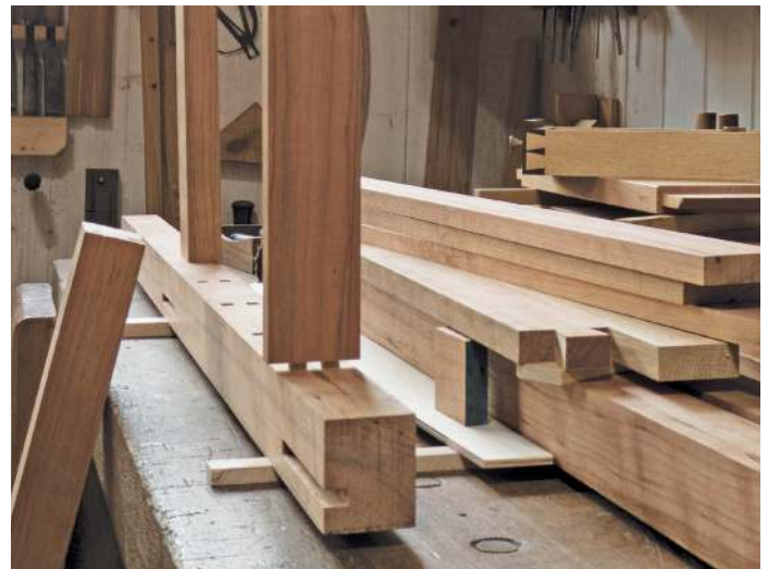
Twin mortises and tenons dry fit
