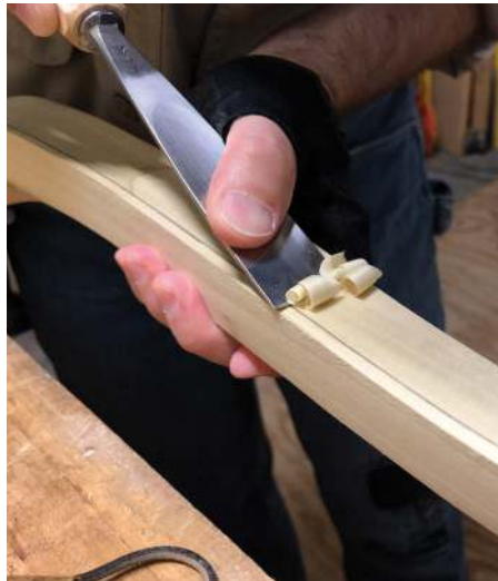
A #4 sweep 25mm wide carving gouge refines the concave profile
