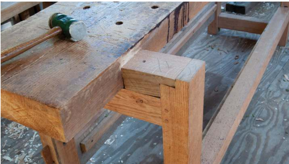
To support the thinner oak board that extends the benchtop, I needed to add some blocking on top of the short aprons. The blocking just friction-fits on top of the apron and nestles in a notch in the rear post. The thin top gets pegged down to the blocking
