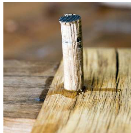
Glue the joint as usual, and coat the peg in glue before driving it home
