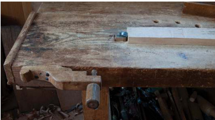
The iron toothed planing stop fitted in a wooden block driven through a mortise in the bench. Simple as can be. Jennie Alexander called this a 'toothy critter', which is descriptive enough. You can see the 'single bench screw' fixed to the front edge of the bench as well
