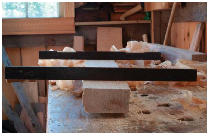
From the user's viewpoint, almost. The camera is higher here than the joiner should be. Remember, it's not level we're looking for, it's flat. Flat can be tilted, but not twisted
