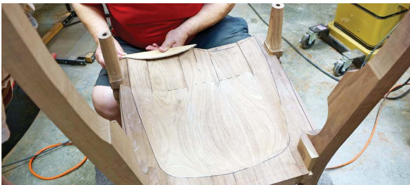
A student using Brock's templates to cut that signature profile on the front of the seat – giving the rocker its smiling face
