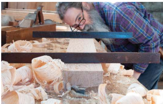
Winding sticks are indispensable in planing stock. On this piece the planing is underway, but it's good to start with the winding sticks, too. We all have a dominant eye, like our dominant hand. This is my left-eyed squint
