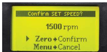
I am using a 25mm spade bit to drill a beech test piece. The setup sequence shows selecting the drill bit type, size, material being drilled and confirming that speed. I then set the self-start option, which is only two clicks
