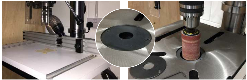
LEFT: A false table such as this can be easily made or bought for around a little more than the Nova fence INSET: The low insert plate is annoying when drilling at the end of a workpiece] RIGHT: Quill lock allows height setting on a sanding drum – maximum size 50mm
