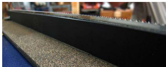
Clamp the saw plate into the flat iron plates and mount into the angle iron jaws
