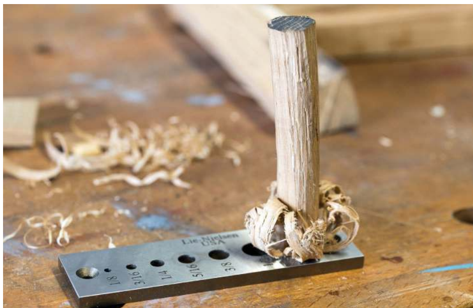
Cut the peg to final size using a dowel plate
