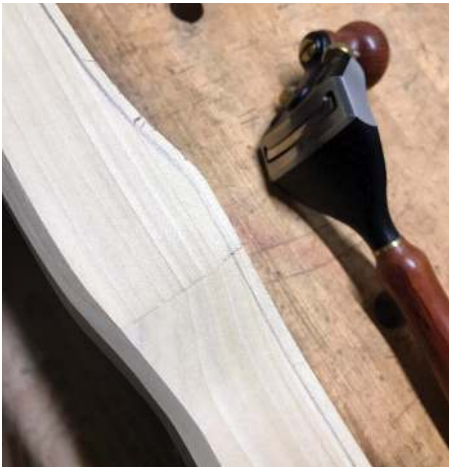
Pencil layout lines a few centimetres away from the rear arrises on the side faces of the leg. I use a Veritas pullshave to remove material quickly, but any convex sole spokeshave will work
