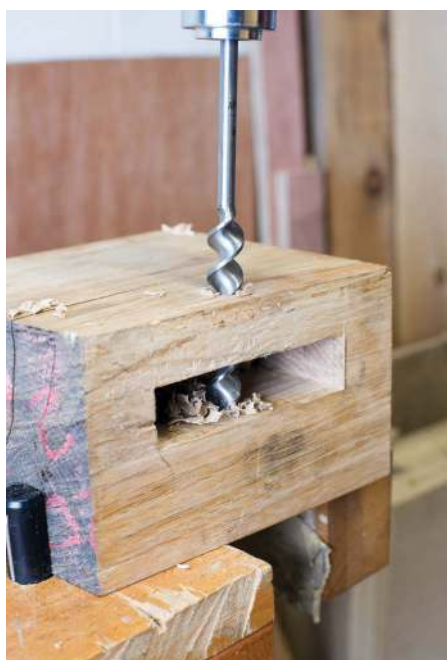
Once you are through the mortise, remove the scrap and keep drilling
