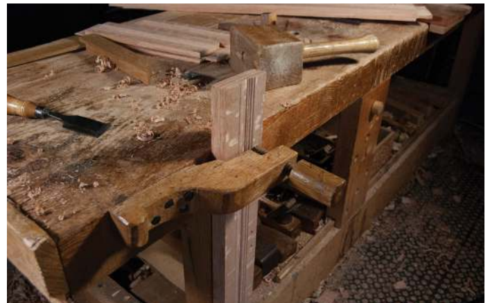
A long rail for a chest is pinned against the bench's front edge by the bench screw mentioned in both Moxon and Holme
