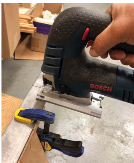
Fit your jigsaw with a metal blade
