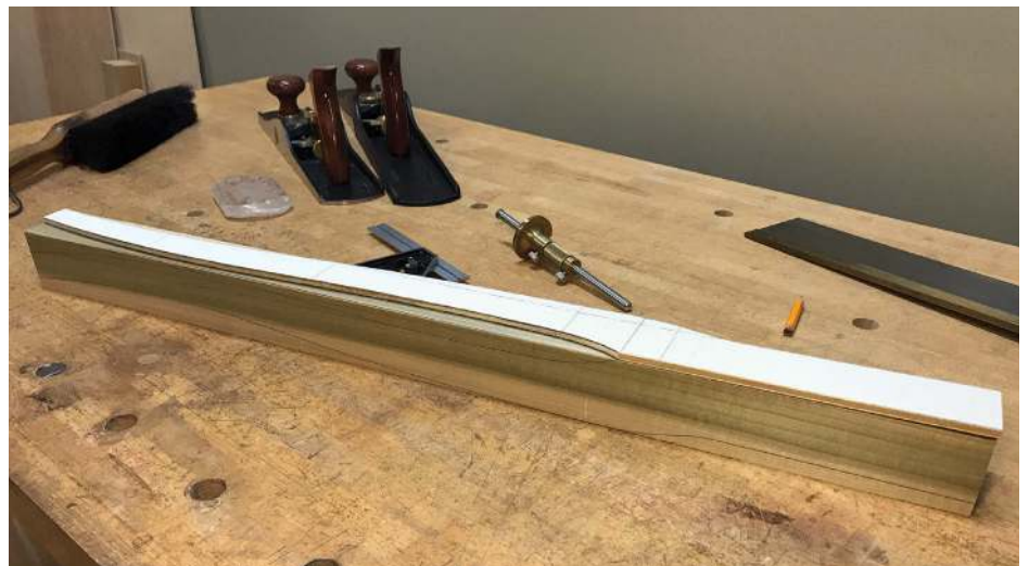
Carefully align and trace the side view drawing to the reference surfaces of the leg blank. Keep the 'rear' side of the template against the arris of the reference surfaces
