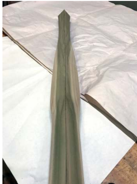
The centre arris should be straight when initial shaping is complete
