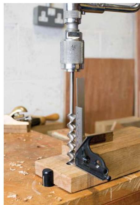
Drilling the peg hole in the tenon
