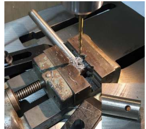
This shows my machine vice holding the round bar. The vice is secured on the table using parts from a universal clamping set. The inset shows the completed hole
