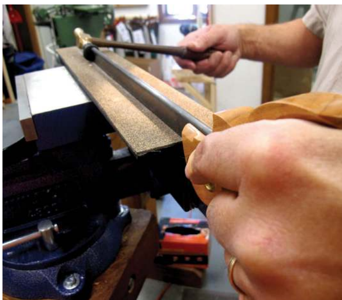
Gently tap the folded back towards the handle to close up any gaps
