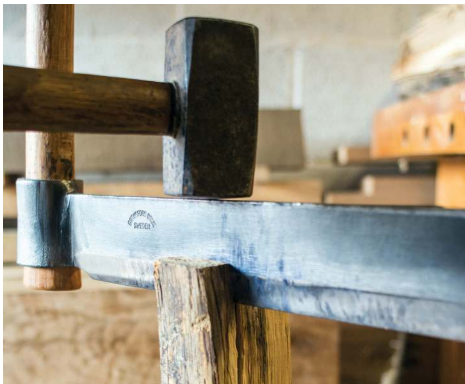
Splitting out the drawbore pegs ensures you have continuous grain the full length of the peg
