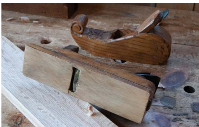
This plane was a smooth plane originally, but after grinding a generous curve in the cutting edge, it serves well in initial flattening of hewn boards. Behind it is a homemade plane with a similarly ground iron, based on some Dutch examples from the period
