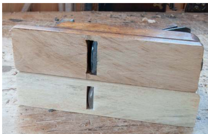
One of my everyday fore planes sitting on top of a typical narrow scrub plane. Either plane works just fine. I eyeball the curve when grinding.
