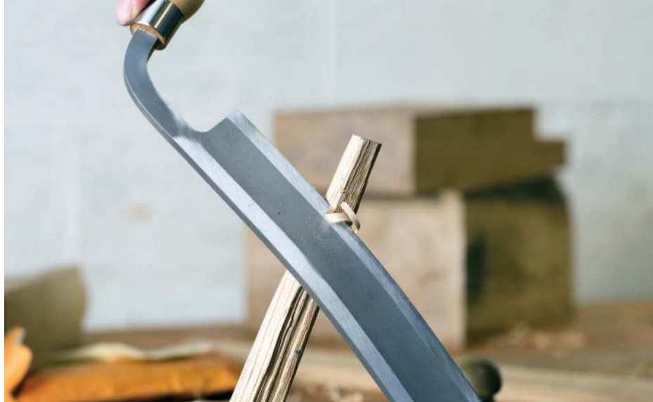
Roughly shape the peg with a drawknife or spokeshave
