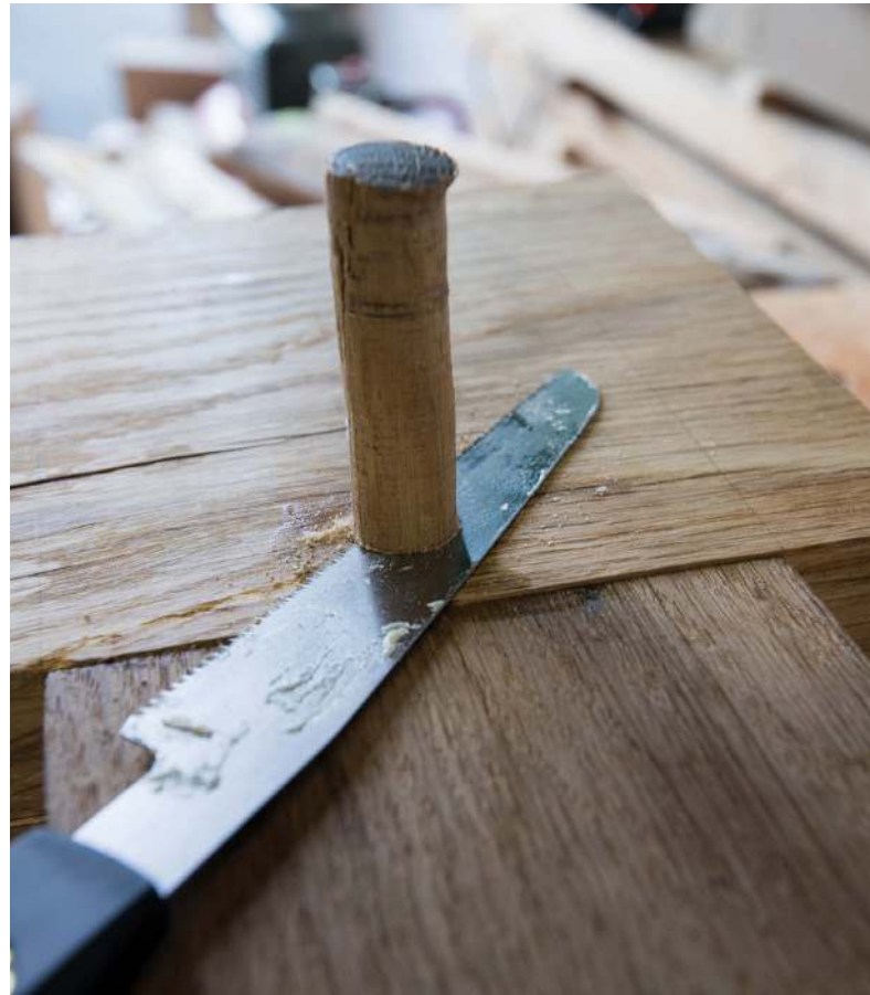
Cut the peg flush and clean up the surface with a sharp chisel
