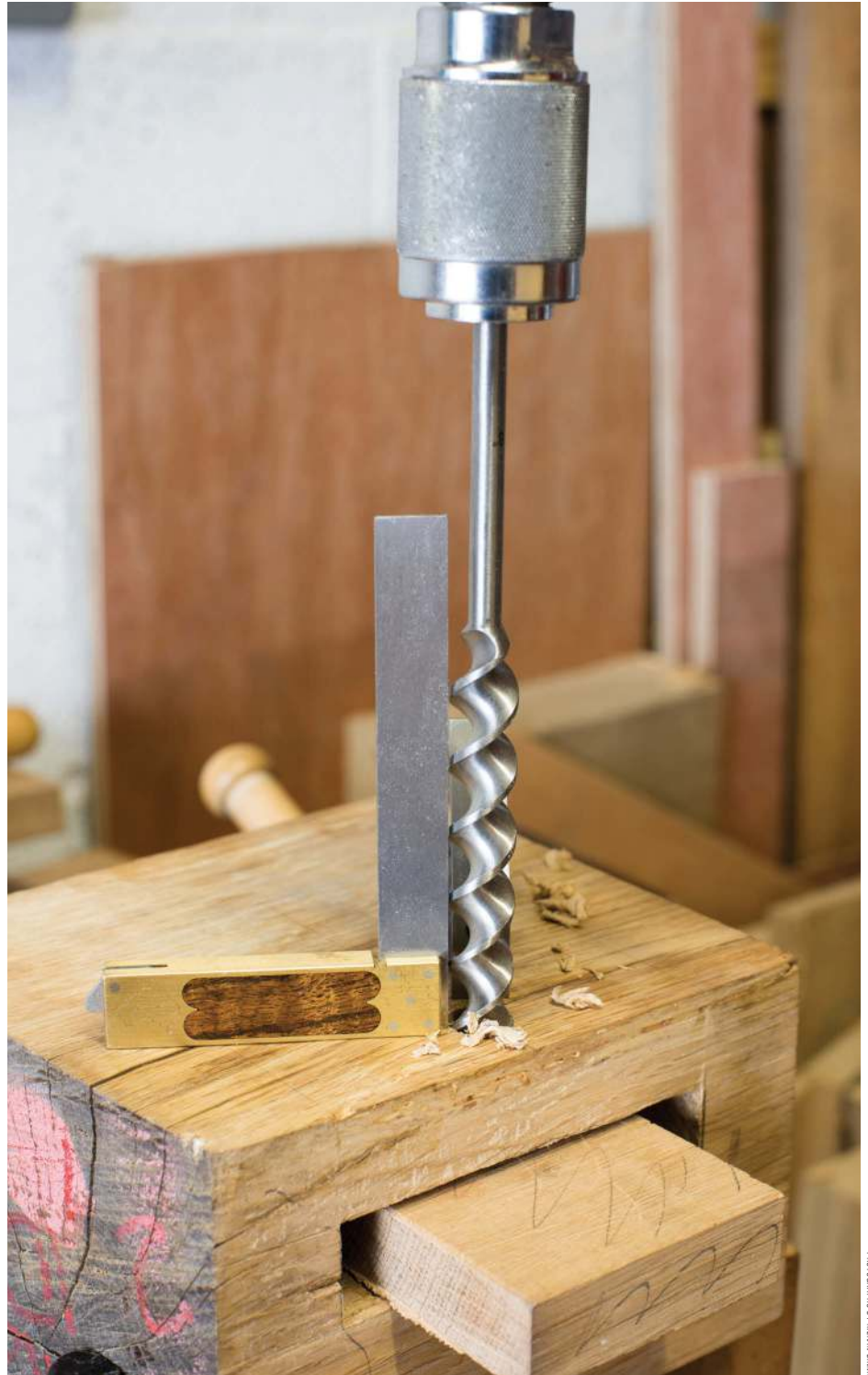
Drilling the peg hole in the mortise. Place a piece of scrap in the mortise to prevent blowing out the internal face of the mortise
