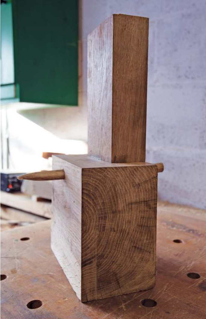
The test joint, with the peg proud on each side
