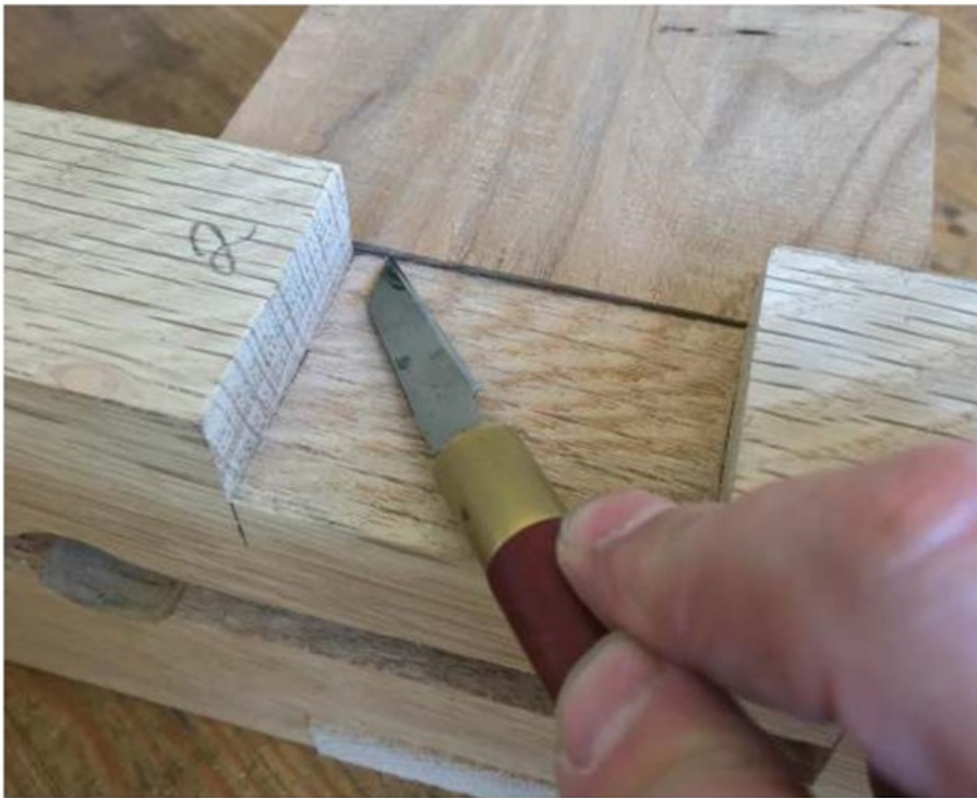
Scribe the thickness of the block directly from the back jaw when the dados are cut
