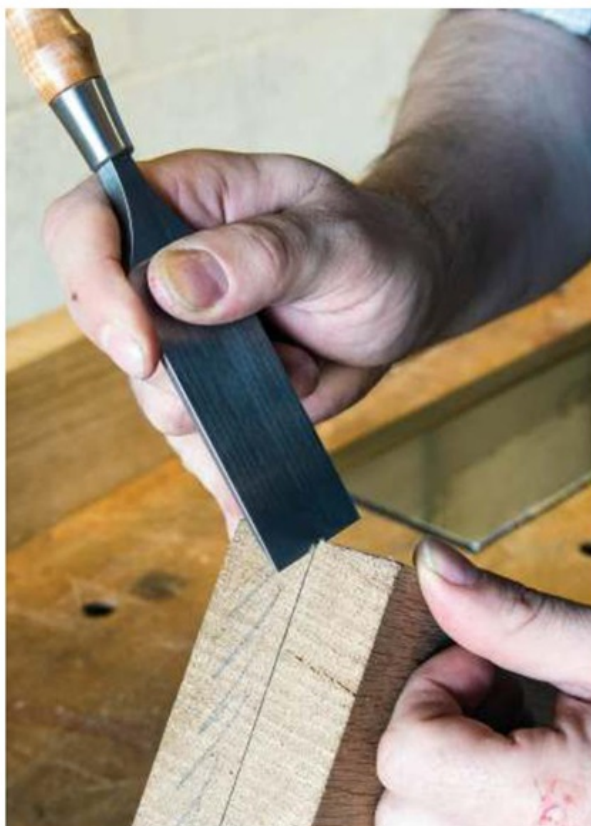
A notch provides a starting point for the saw
