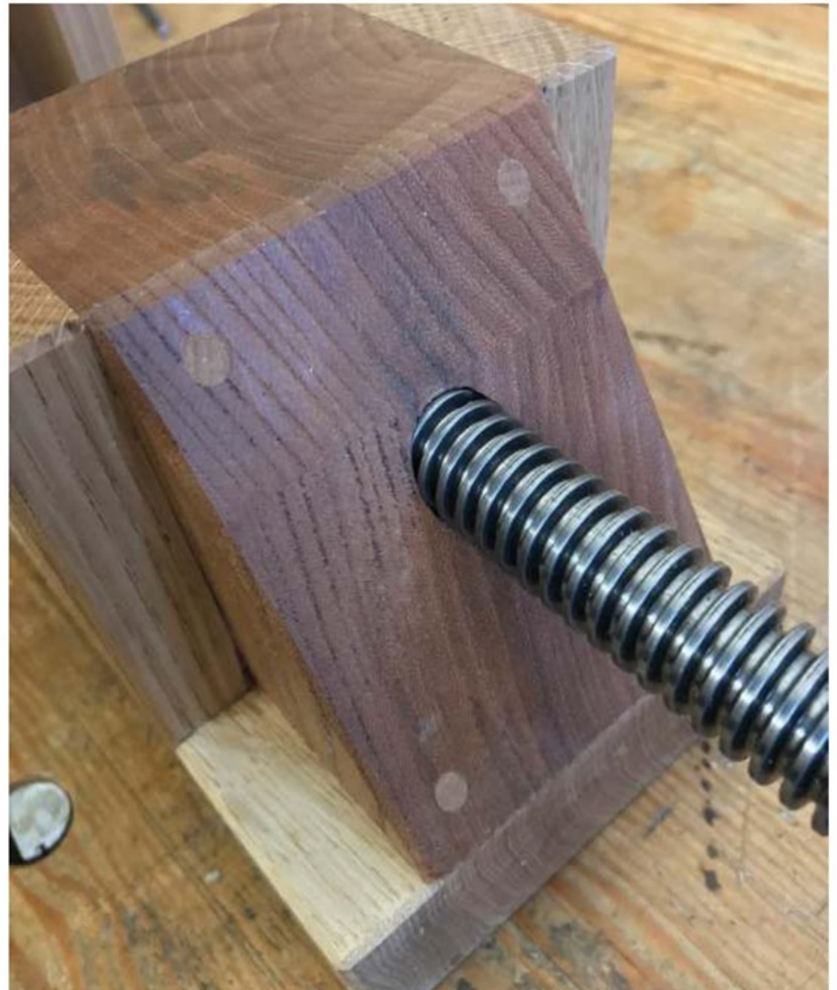
You can plane the block flush with its surrounding after assembly before fitting the screw
