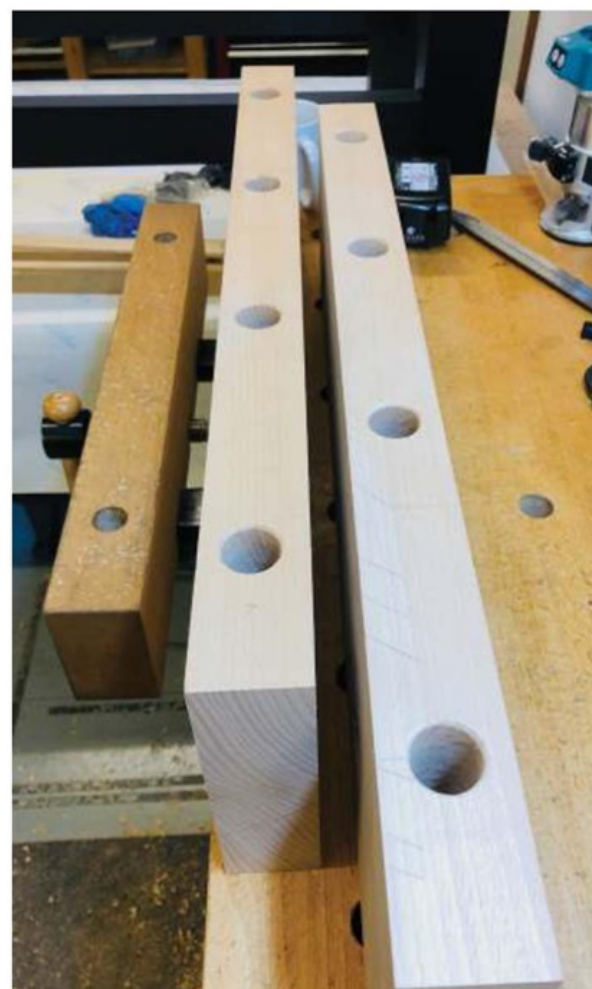
Extra dog holes in the vise jaw means greater versatility later
