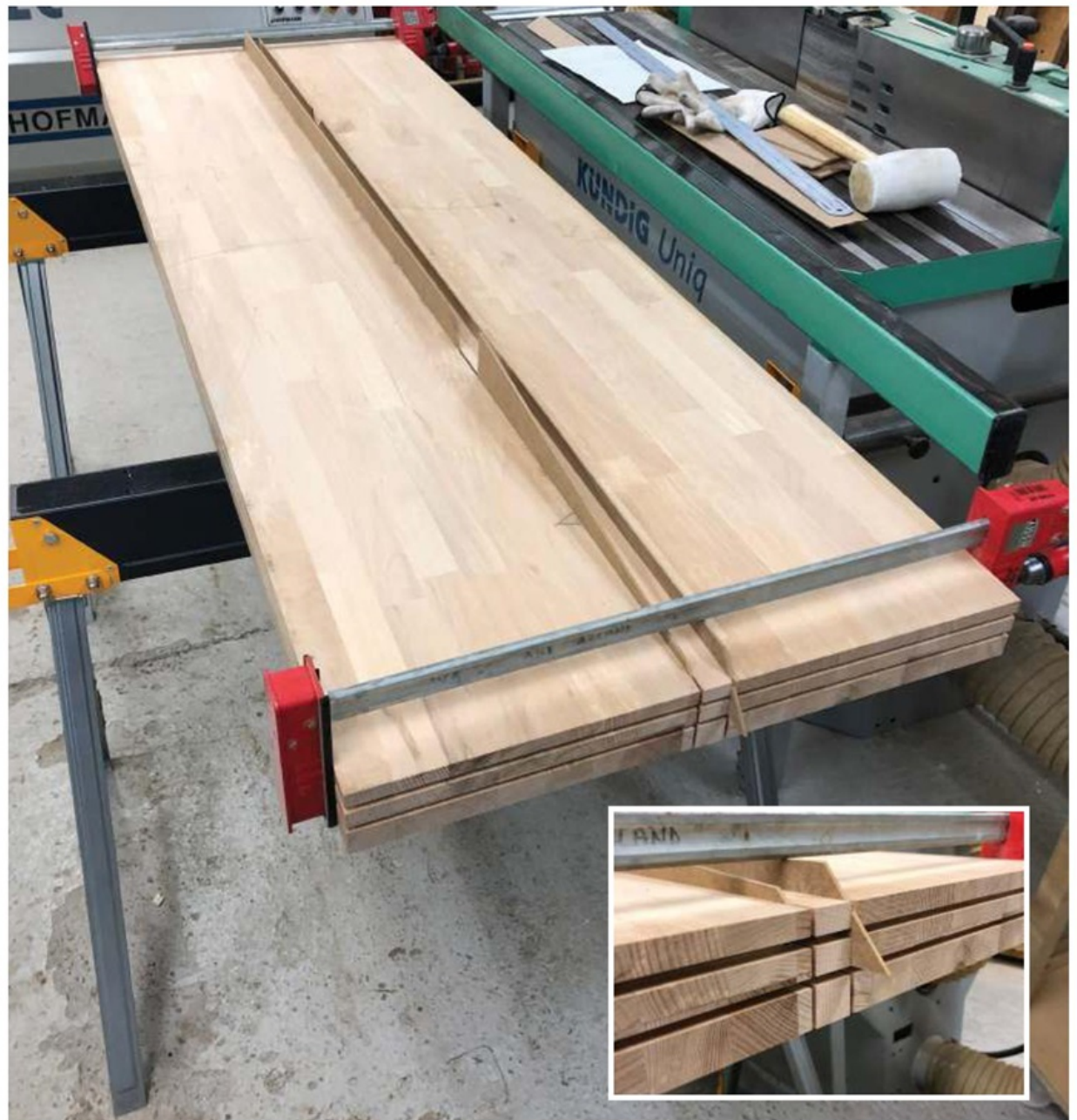
The two sheets of worktop have been laminated together and machined with grooves around the perimeter edges before separating to create the centre fillet
