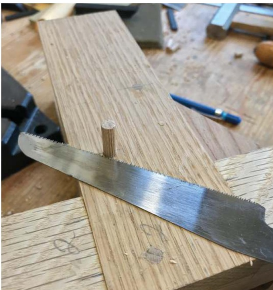
Dowels will add strength but also make gluing up easier
