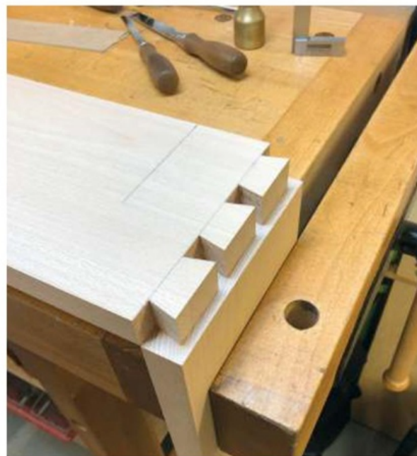
The tail and pin boards were alternated for their respective positions on the apron to avoid end grain exposure. This apron becomes the back jaw of the end
