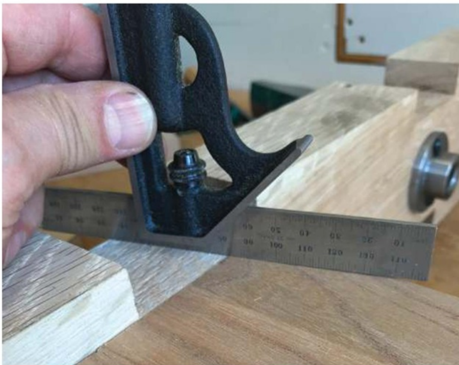
Make sure the block is flush
