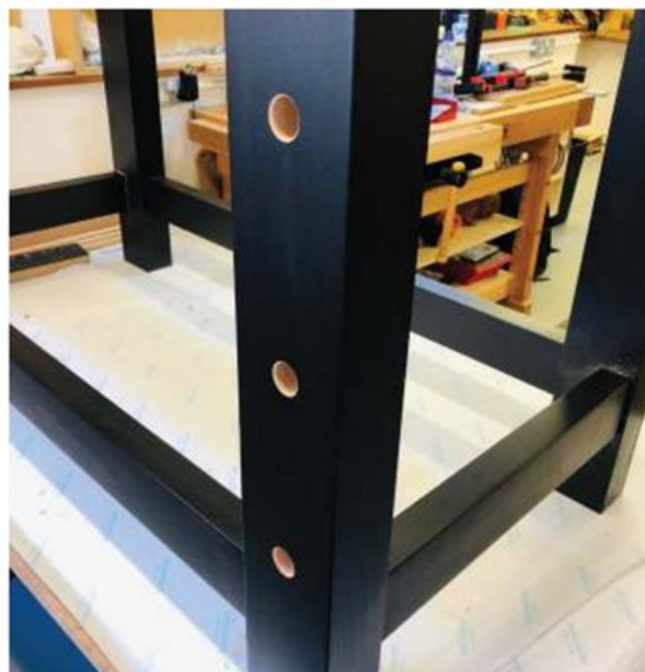
Two coats of Danish oil and the base was finished and ready for dog holes
