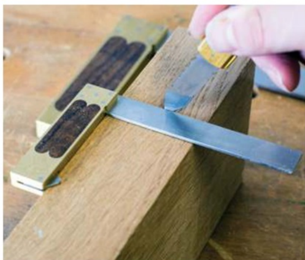
Laying out the tenon shoulders
