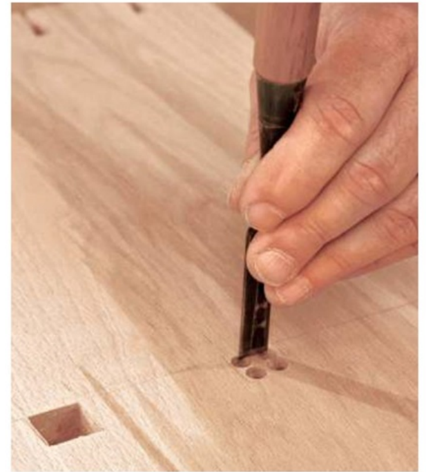
Drill and chop. Remove most of the waste on the drill press. Then use a chisel to chop out the rest, working back to the scribe lines gradually. Chop halfway down, undercutting slightly, then flip to complete the cut
