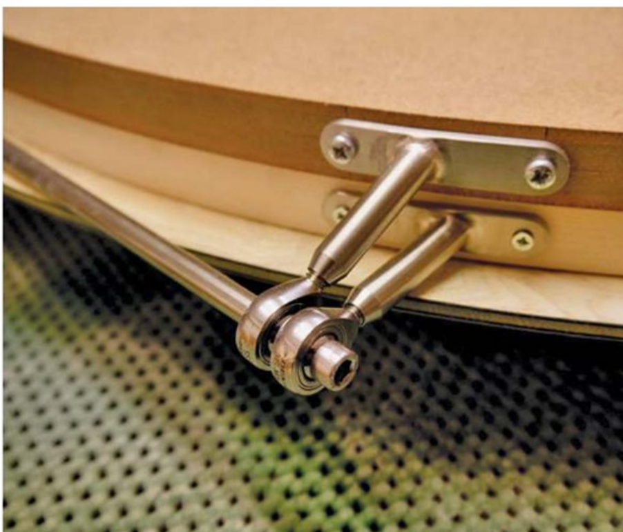
Custom hinges mounted on sample doors for testing
