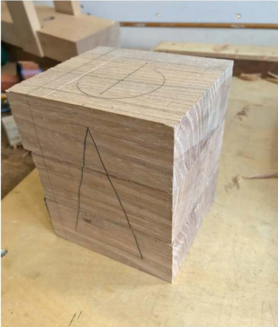
Three blocks marked up and planed to produce the clamp screw block
