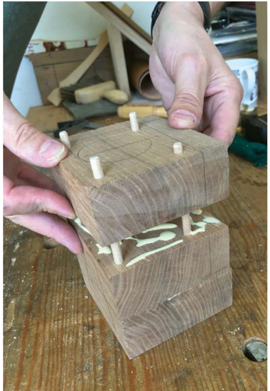
Dowels make alignment and gluing up much easier
