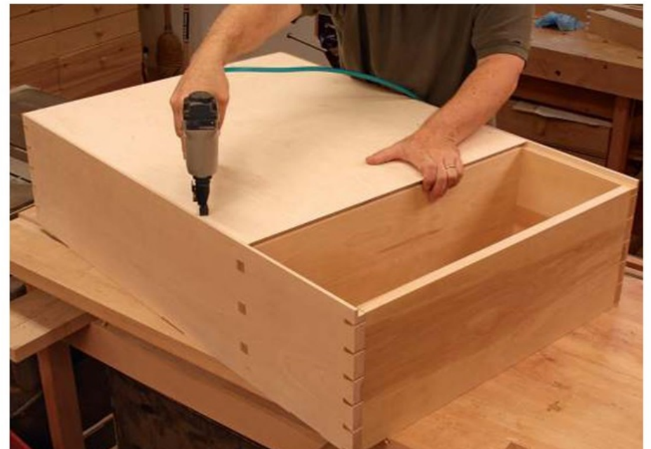
Big glue-up made easier. To provide clearance for the proud dovetails and the through-tenons, Pekovich elevates one side using wood strips (left). Then he assembles the main carcase, checking it for square. Once the case is dry, he attaches the back with glue and nails (above). Screws add a little extra security
