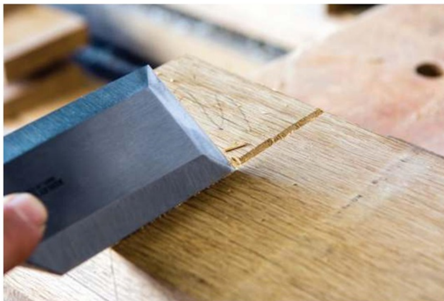
Paring a trench for a first class cut
