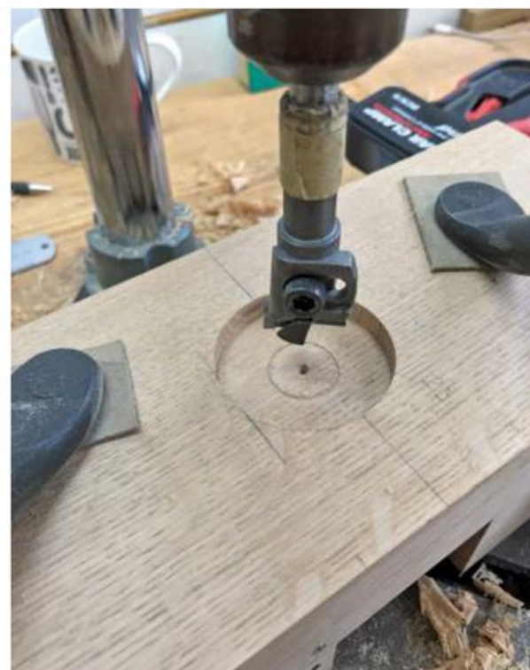
Start with the widest bore on a series of concentric holes
