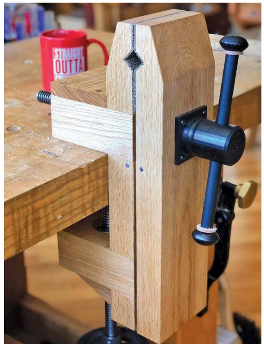
Brendan Gaffney's portable Hi-Vise complete with V channels and lined with rubber for holding round parts while conducting chairmaking demonstrations
