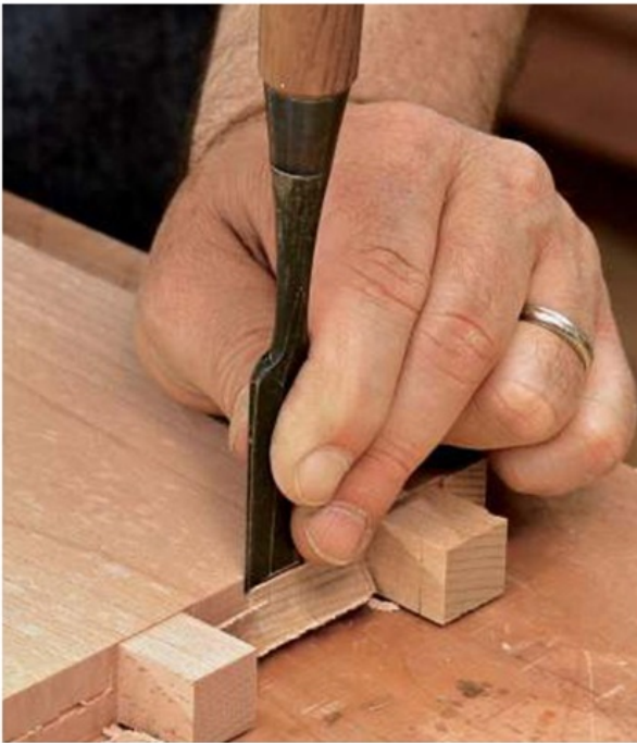
Clean up the waste. Bandsaw most of the waste and then chisel to the baseline. To ensure a tight fit, chop halfway down, undercutting the joint slightly, and then flip and work from the other side in the same way
