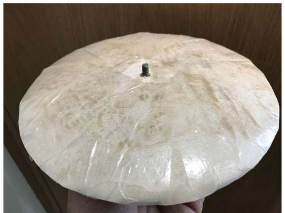
Testing the veneer's capacity for compound curves
