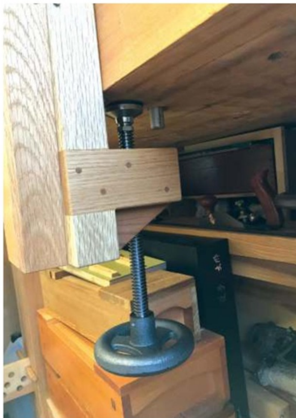
Allow plenty of clearance below the worktop to accommodate the clamping screw
