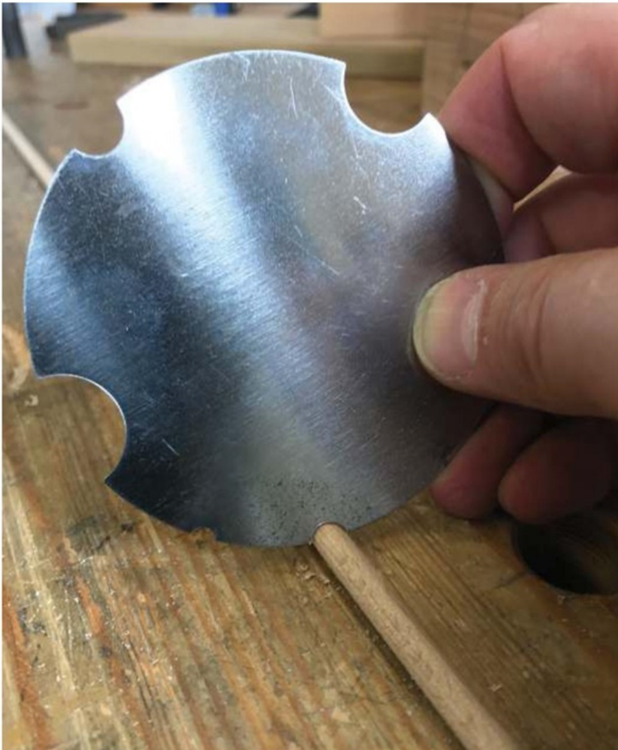
Reduce the size of the dowels with a scraper if they're tight
