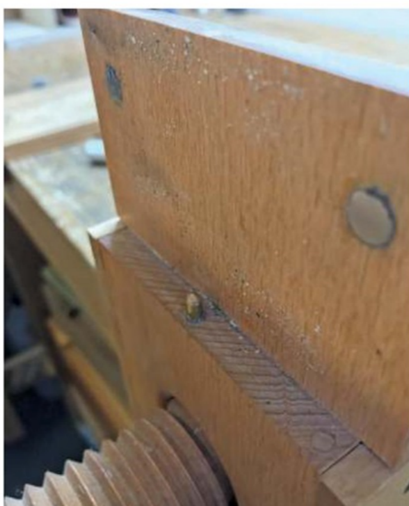
Magnets and dowel pins make it easier to swap inserts around
