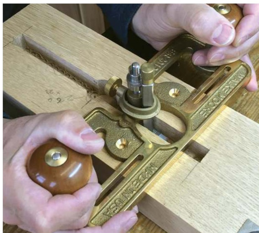
Clean the bottom of the mortise with a router plane
