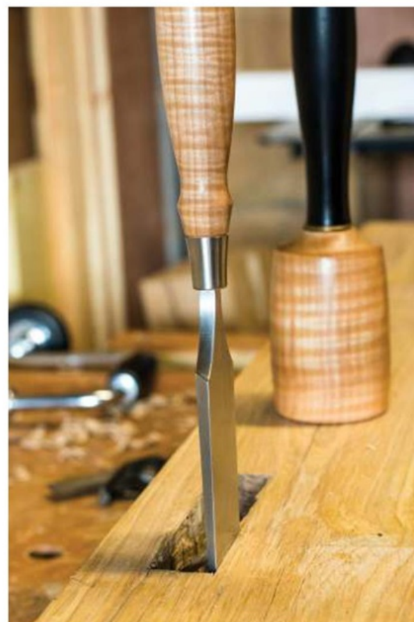
Paring the mortise walls
