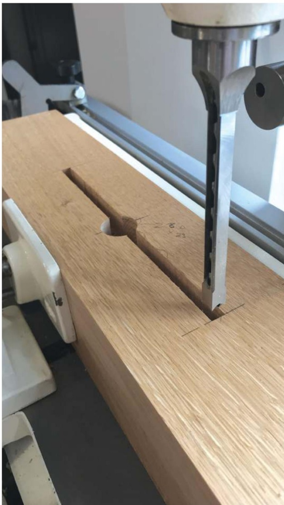
You may have to make two passes to complete the mortise with a hollow chisel mortise
