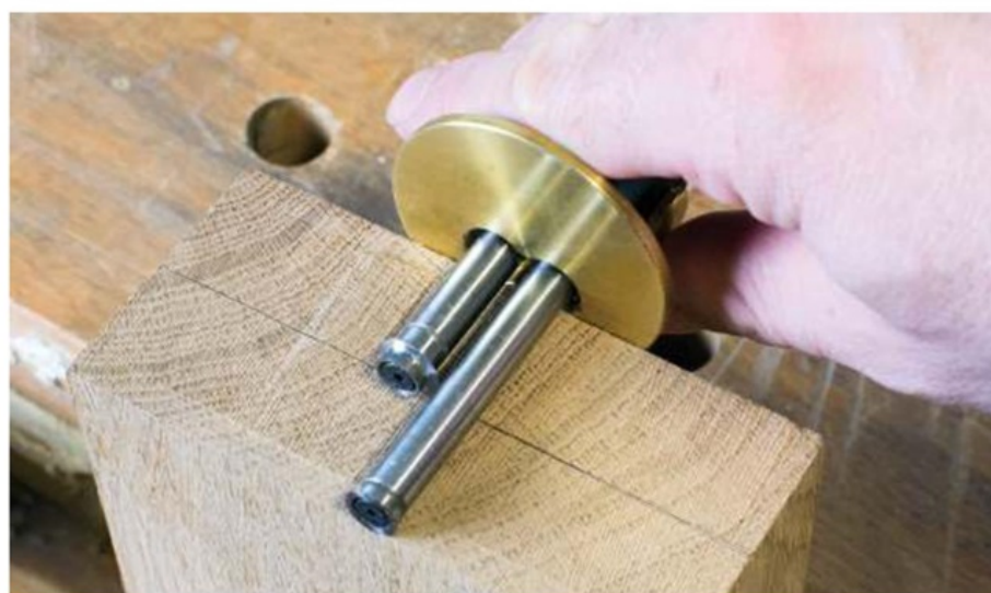
A mortise gauge is essential for laying out the tenons and mortises
