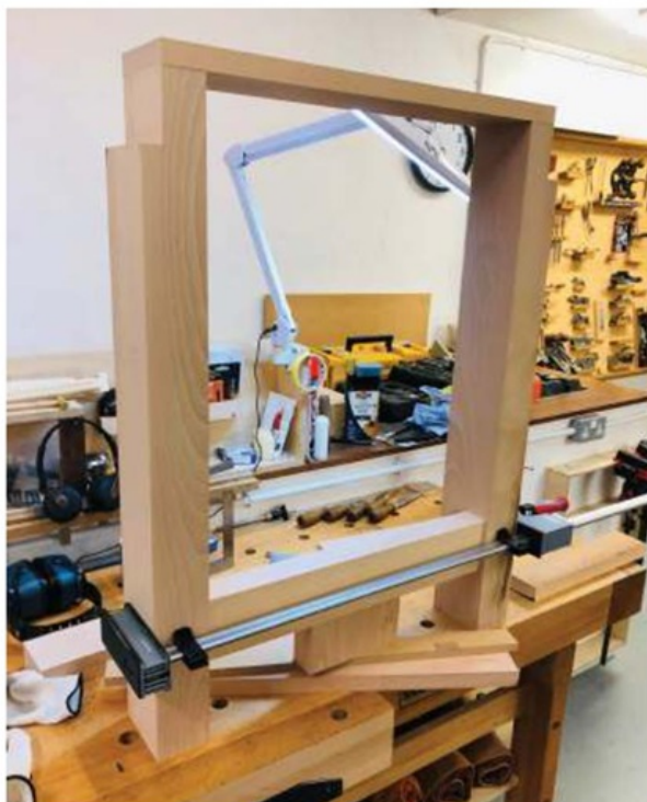
Cut-outs at the top of the base frame provide support
