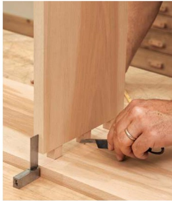
Scribe the mortise locations. Stand the shelf in place, using a square to align it flush with the back edge. Knife around each tenon and repeat on the opposite face of the case side
