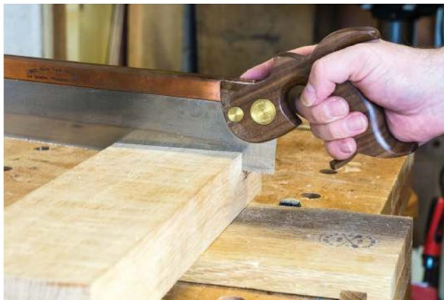
Cutting the tenon shoulder
