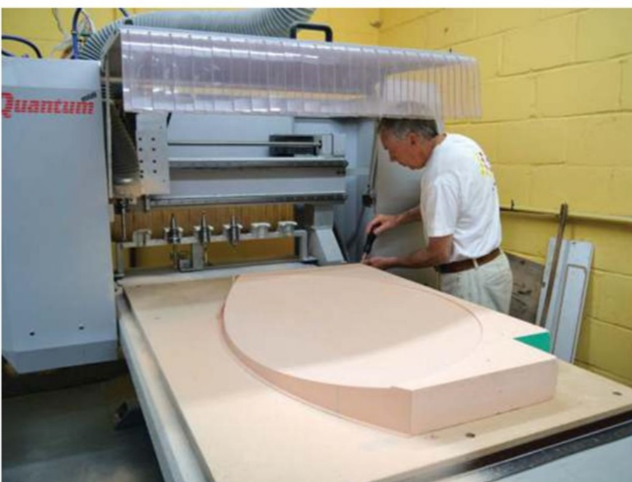
The former after milling on the CNC machine
