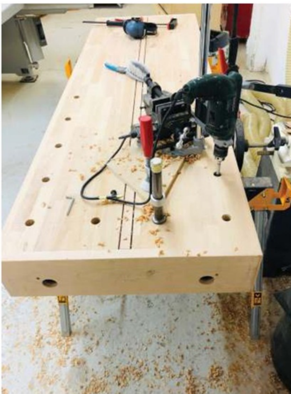
A mobile drill press with some extra ballast was used to drill the dog holes in the benchtop
