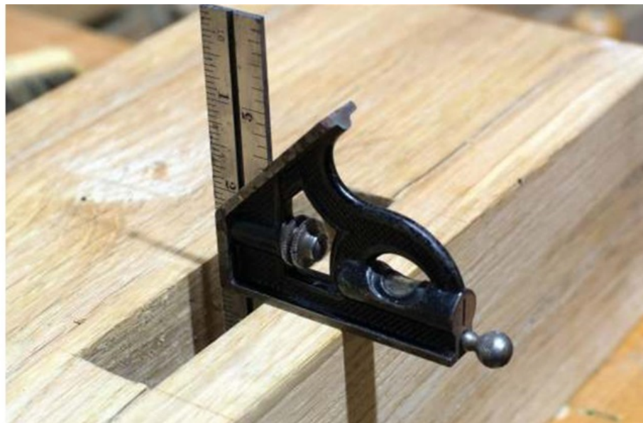
Checking that the mortise is plumb and to depth
