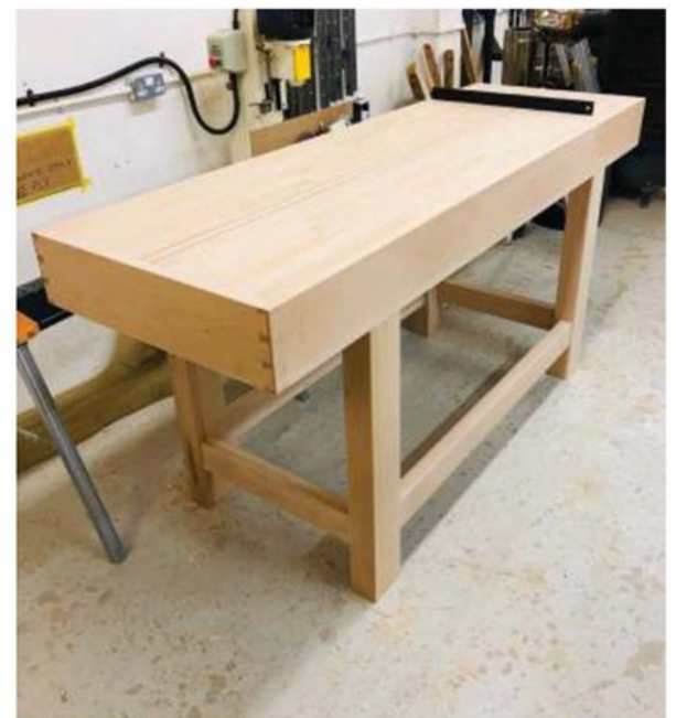
Bench top in position with the aprons flush with the front of the legs
