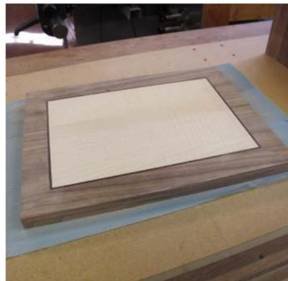
Flattening the box lid with a sanding board
