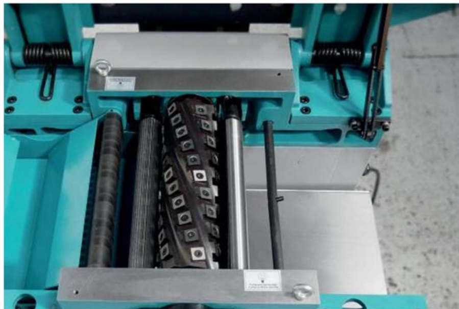
spiral planer block for lower noise, longer life and a superb finish
