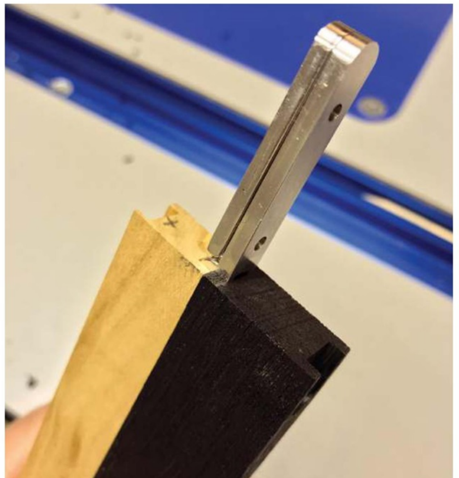
Check to make sure the hinge is held tightly between the two pieces and without a gap between them
