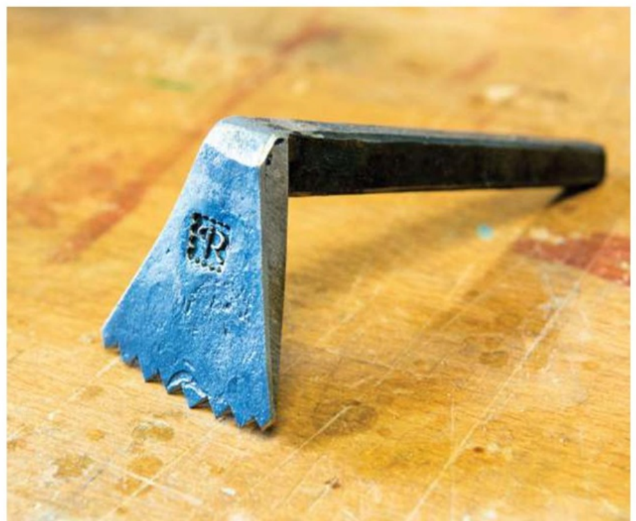
A planing stop is one of the key workholding solutions. This stop was forged by blacksmith Peter Ross
