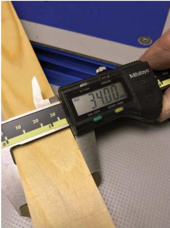
Make a spacer block to set a stop the correct distance from the edge of the cutter
