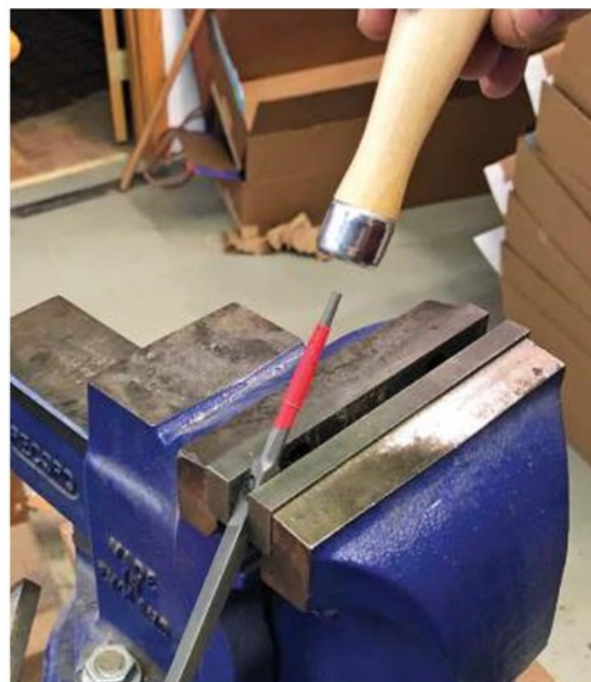
If the bore of your handle is too large, reduce fitting slop by applying a wrap or two of masking tape around the tang
