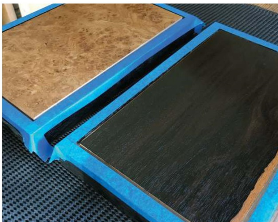
Epic fail; oil turns ziricote black (almost)
