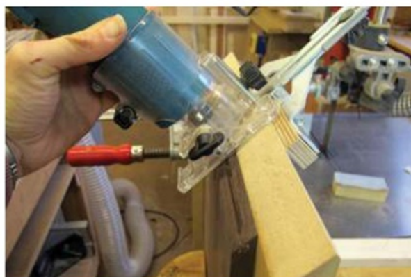
Routing channels for plywood mitre splines
