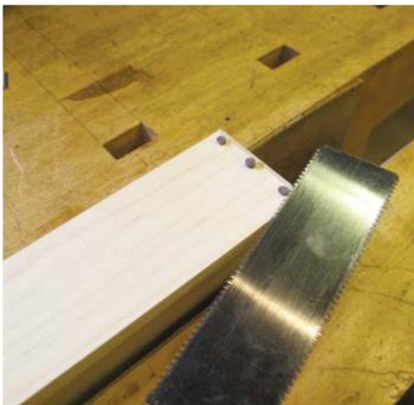
Walnut dowel pins being flushed off
