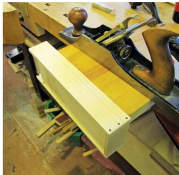
Fitting drawers to a piston fit
