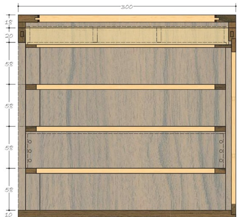
SECTION (Sample drawer and fronts shown dashed)
