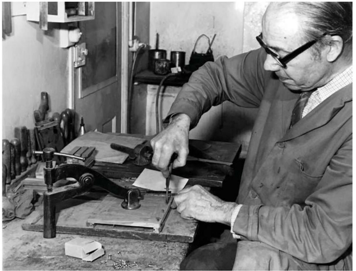
Fred Gandolfi using the 'hold-fast' as another hand while screwing baseboard components together
