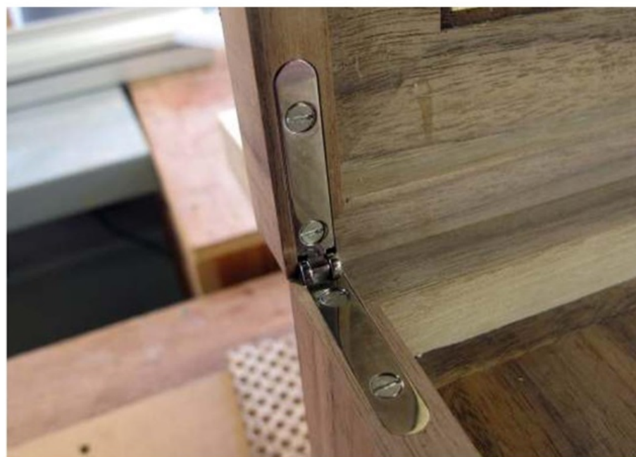
Fitting the smartHinges
