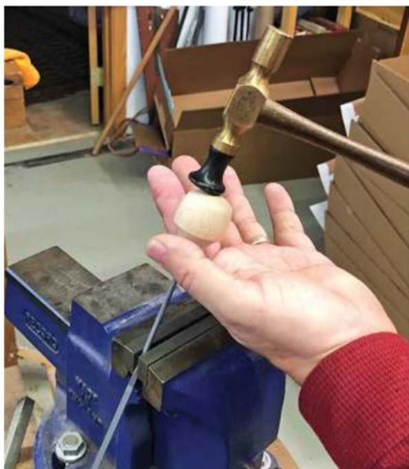
Secure your file in a vice when mounting handles. Note that needle files have cylindrical tangs, so handles are generally tapped on with a mallet
