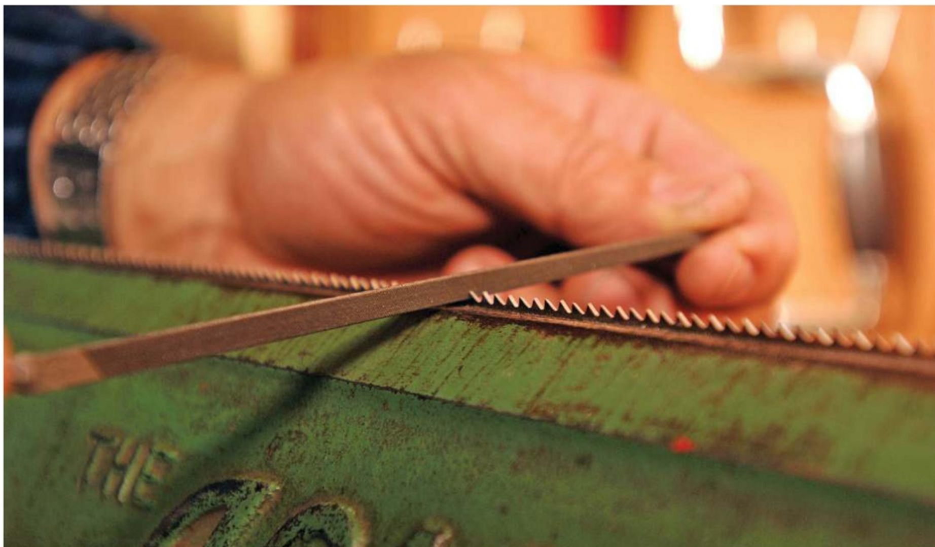
Secure your file in a vice when mounting handles. Note that needle files have cylindrical tangs, so handles are generally tapped on with a mallet
