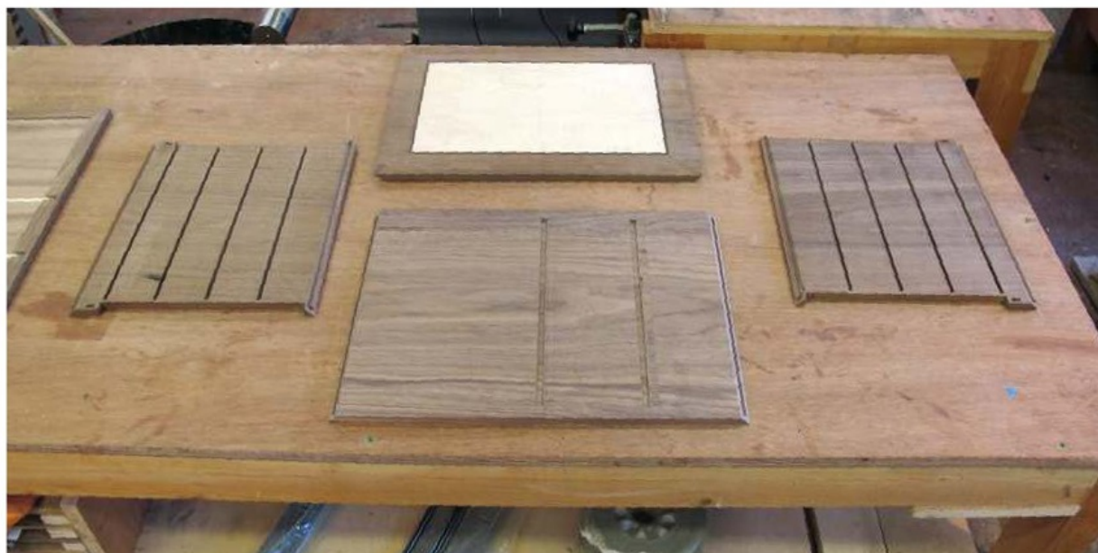
Carcase components ready for glue-up
