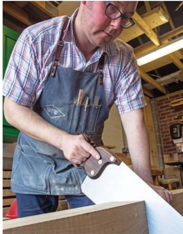
Breaking down the leg stock on the saw benches, using a cross-cut panel saw by Skelton Saws
