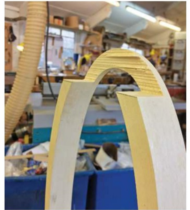
The ledges for the box were cut from the legs in numerous tablesaw passes
