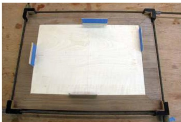
The box top being glued up
