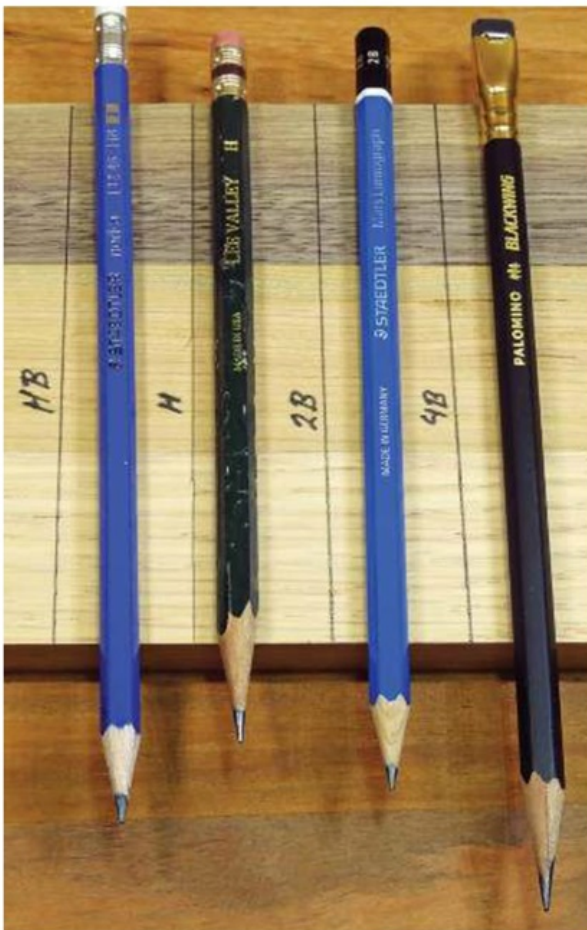
Various grades of pencils were used to enhance the knife line from a marking gauge
