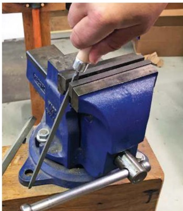
Some file handles, such as Skrooz-On handles, can be screwed onto a file's tang. Again, don't stab yourself with the tang and mount your file in a vice
