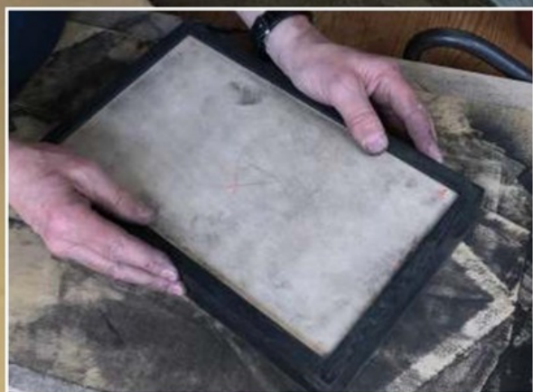
Cover a flat board with abrasive paper to make a sanding board to flatten the edges of the lid and box base
