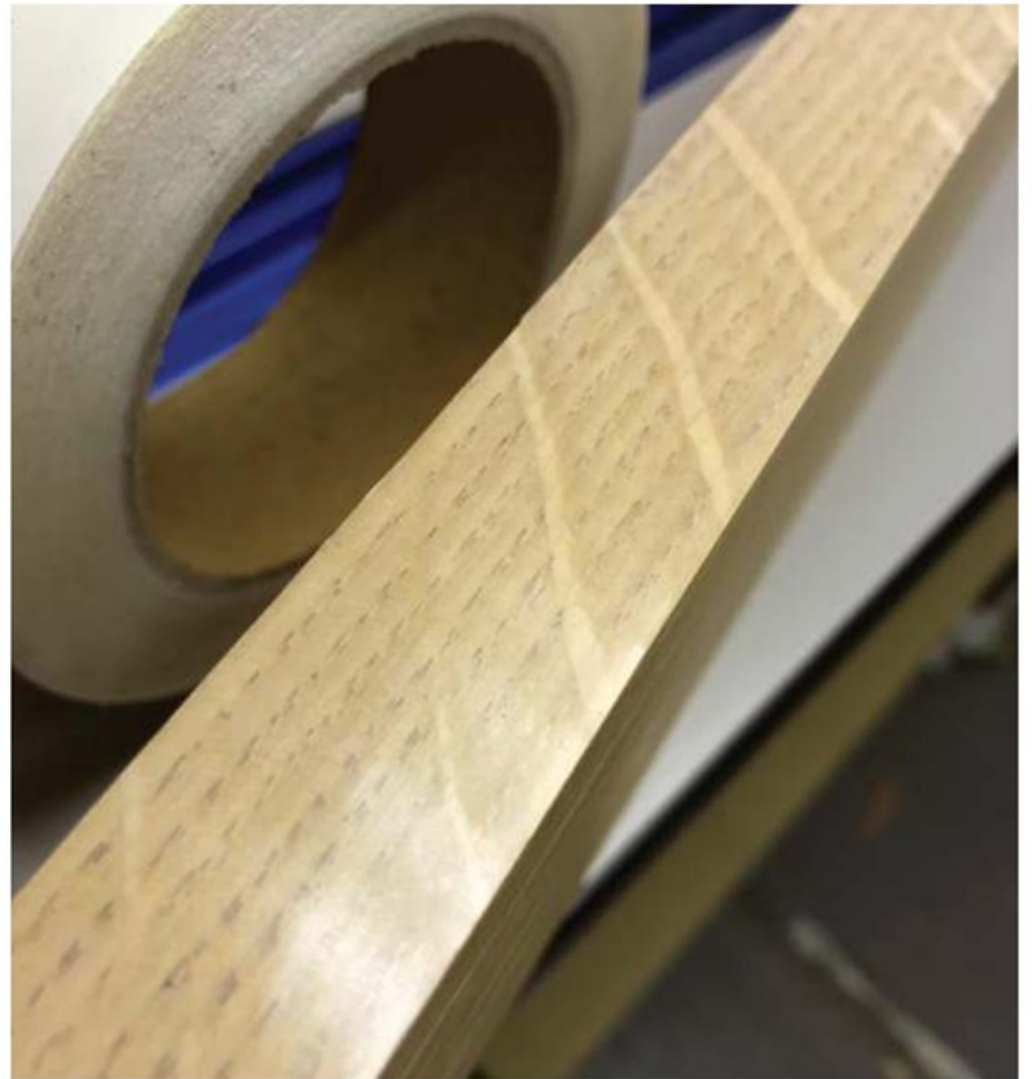
Apply low friction tape to the face of your router fence
