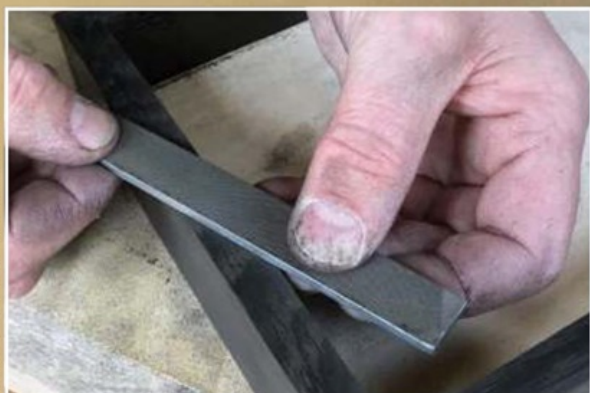
Use a fine metal file to remove the coarse sanding marks from the abrasive paper
