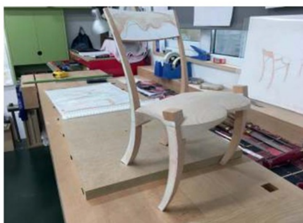
Sketching in the crest rail and propping up the back feet to change the seat angle
