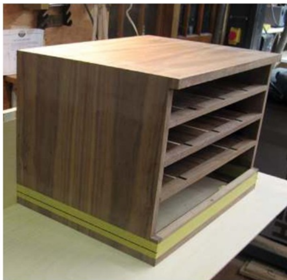
Lid separation at the router table
