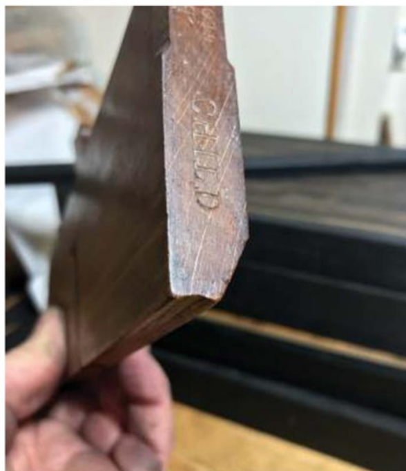
Use a moulding plane to take the corners off the square stock before using the scratch tool
