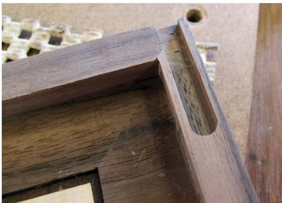
Fitting the smartHinges
