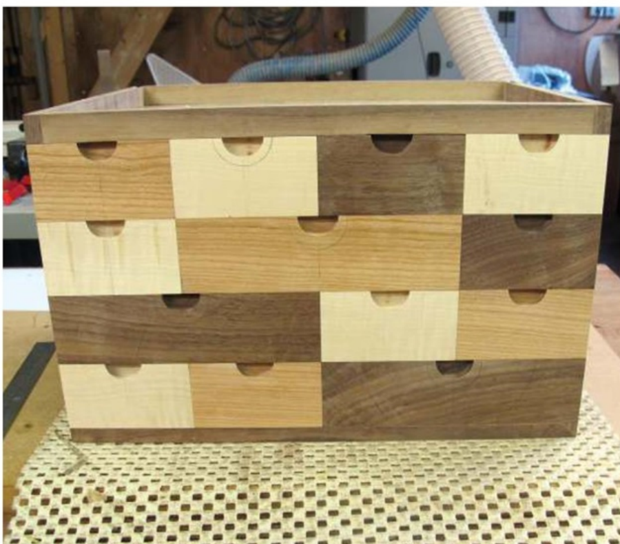
False drawer fronts attached with careful alignment
