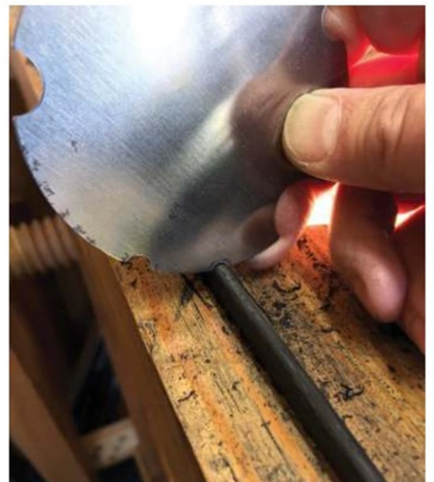
Clamp the moulding to the bench at one end and draw the scratch tool away from the clamp
