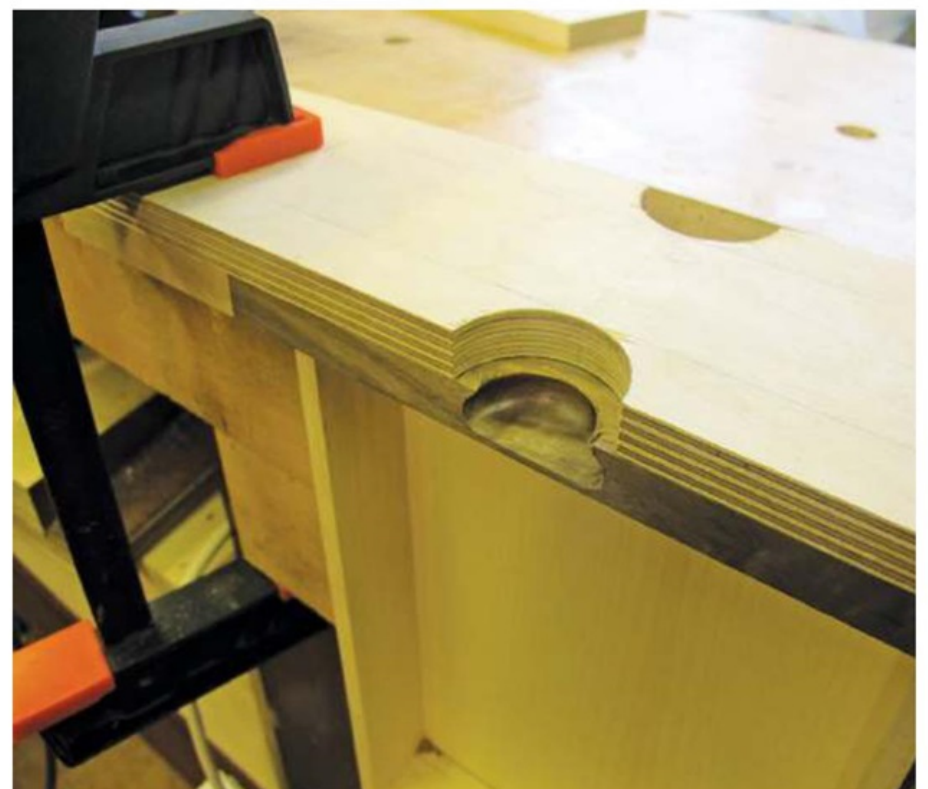
Template routing drawer finger pulls
