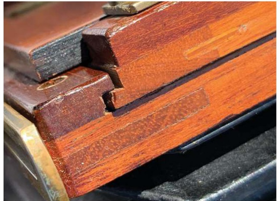
Mitred bridle joints to the rear focus screen, also showing the small end of the loose tongue 'biscuit' jointing used in bread boarding pieces together
