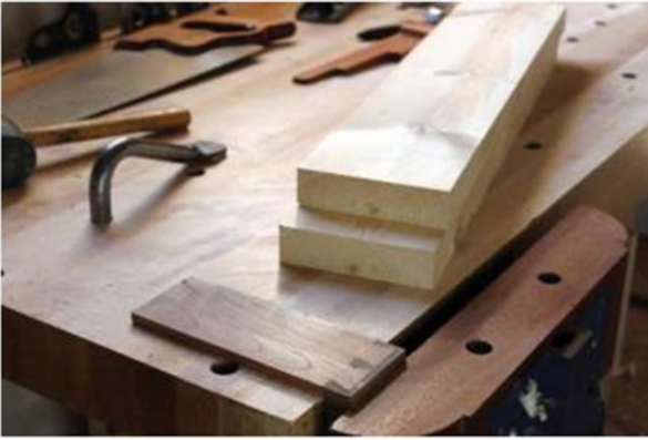
Prepare a couple of wide boards to the same thickness
