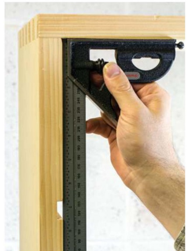
Checking the assembled case is square
