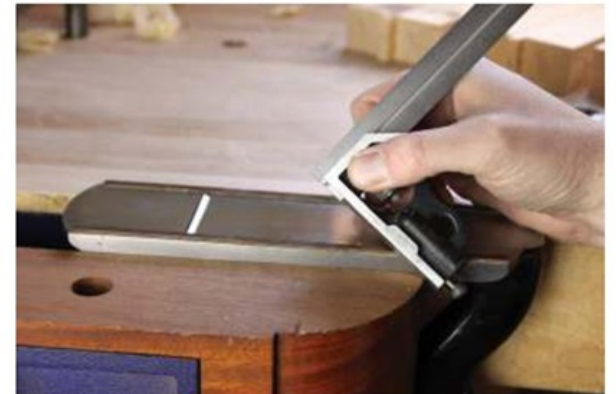
Use a multi square to measure the thickness of the strips
