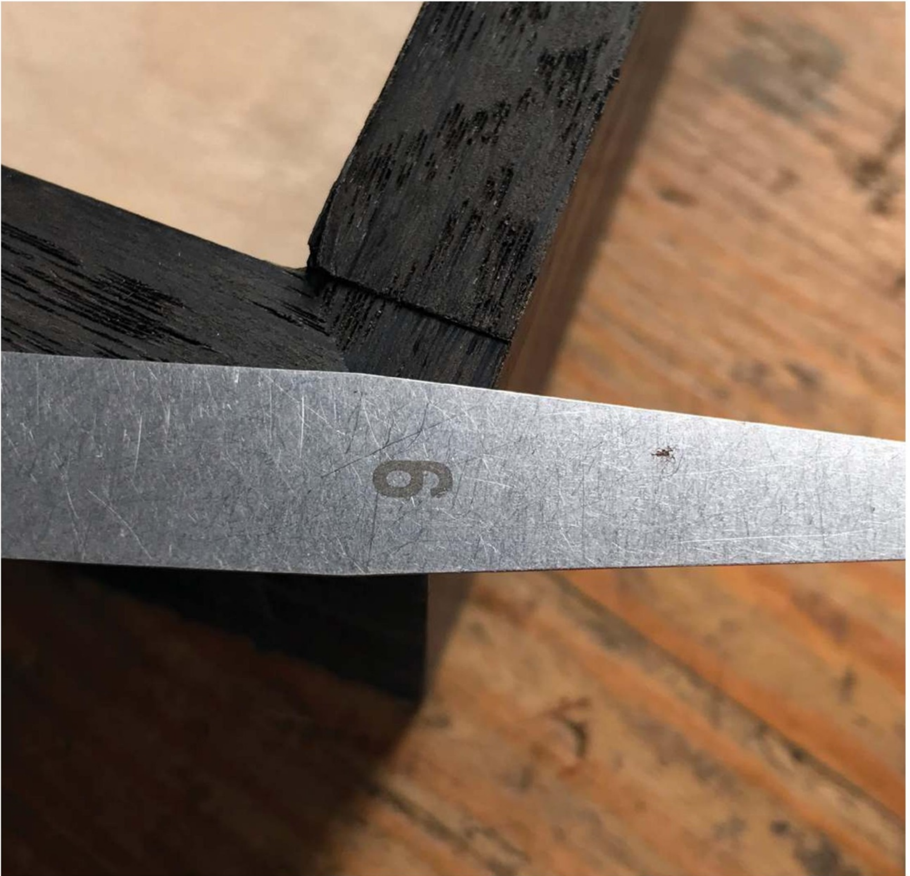
I had a discrepancy of 6 thou to clean up after separating the lid from the base
