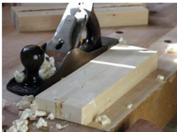
Plane the bottom of the jigs flat
