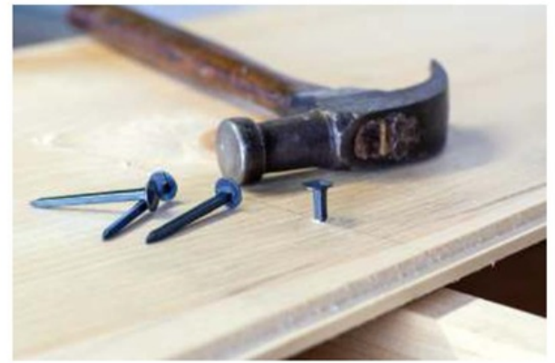
Nailing the back boards in place with 'Roman' style nails
