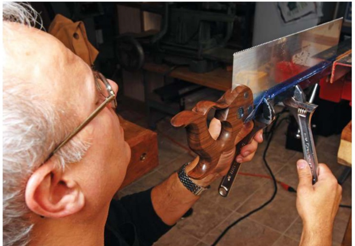
Clamping two adjustable spanners onto the back of a misshapen saw to correct any twist
