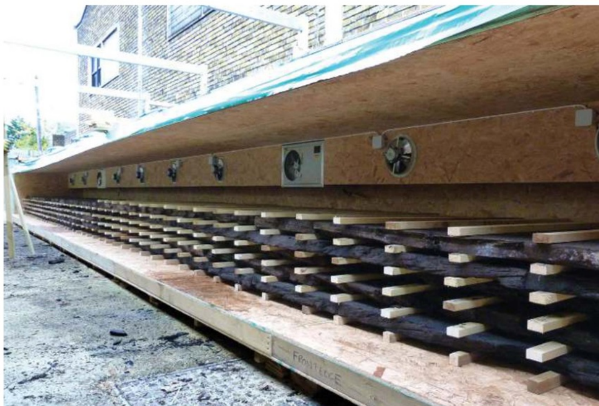
The bespoke drying kiln loaded with the 10 Jubilee Oak planks
