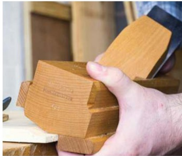
Raising the drawer bottom to fit the groove in the drawer sides
