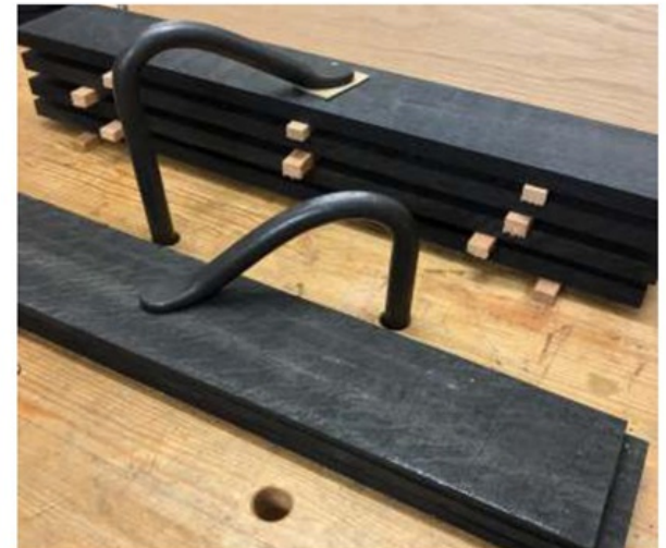
After resawing the boards developed a slight spring so were placed in stick and kept under pressure from a couple of holdfasts for a few days. After a week they straightened out and remained that way
