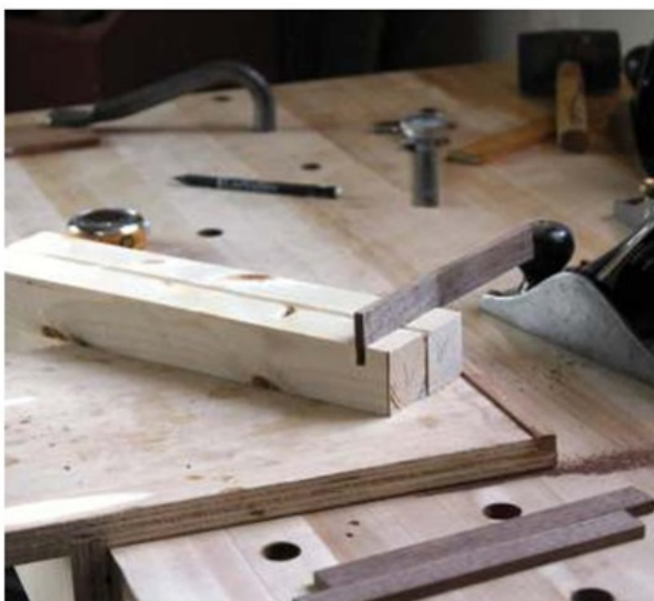
Cut grooves in the jigs for a bench hook and the stop
