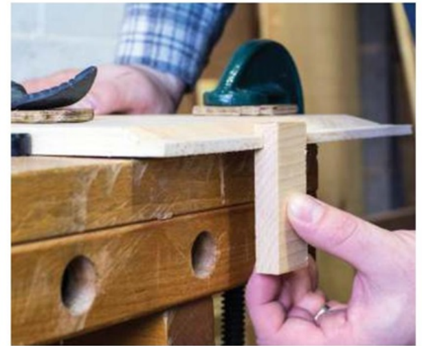
A muntin helps test fit the edge of the drawer bottom
