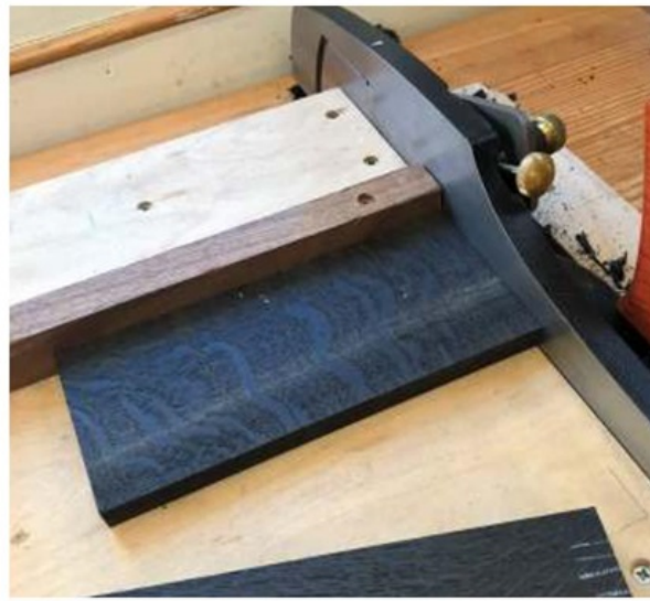
Shooting the ends of the box components by hand on a shooting board
