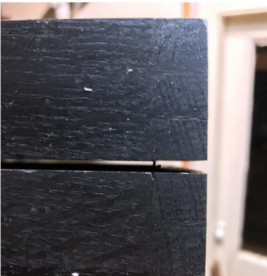
Leave a small slither at two opposite ends to hold the box together...
