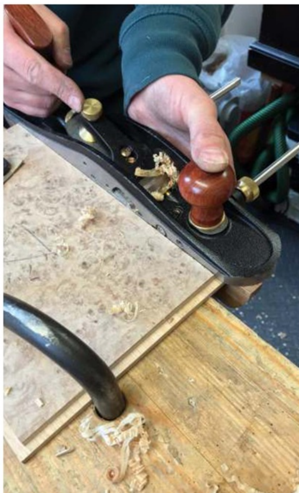
Rebating by hand is remarkably quick when you have a dedicated plane for the job
