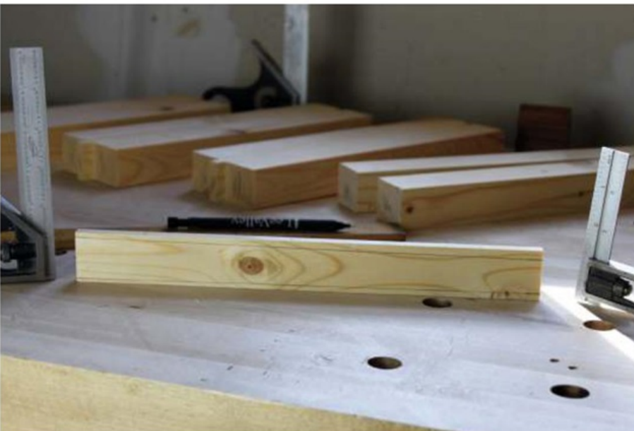
Mark out the tapers on a spare piece of timber to use as a depth guide later
