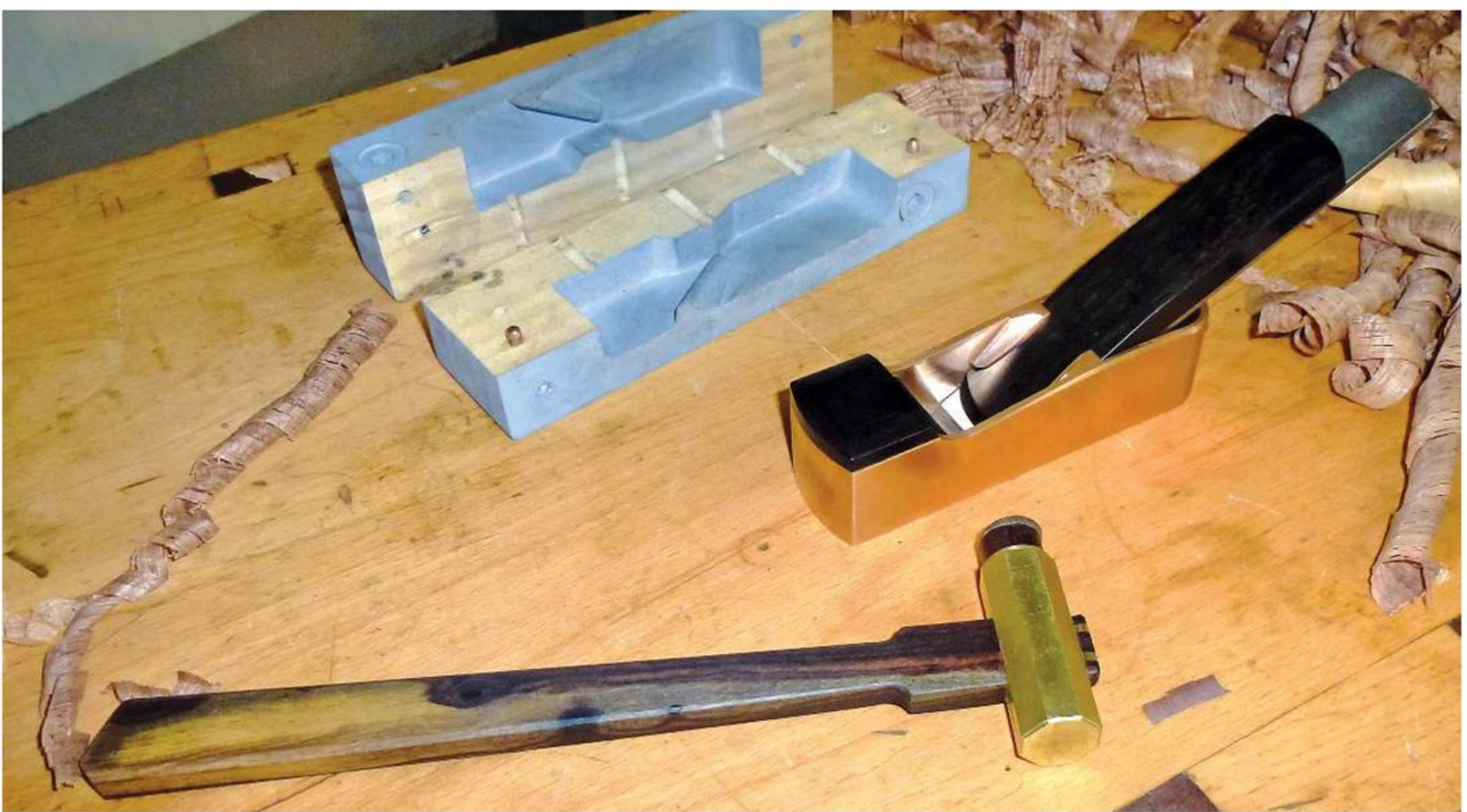
Ollie Sparks' stunning new lugged plane in phosphor bronze and ebony is inspired by the William G. Scott mitre plane of the last century
