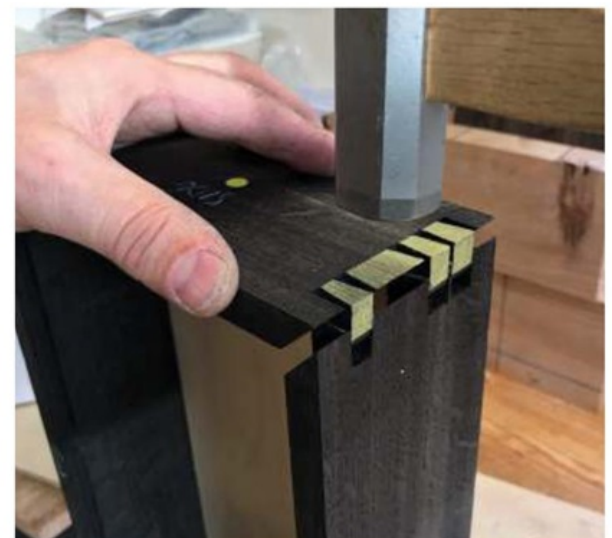
Carry out your test fit with either the lid panel or bottom board in place but not both. You'll struggle to get the box apart again!
