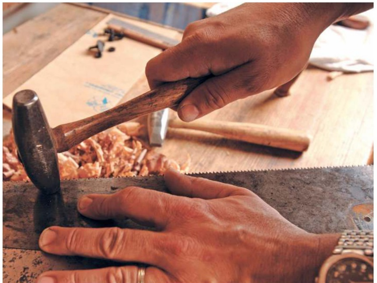
Tapping out kinks in the saw plate with a hammer
