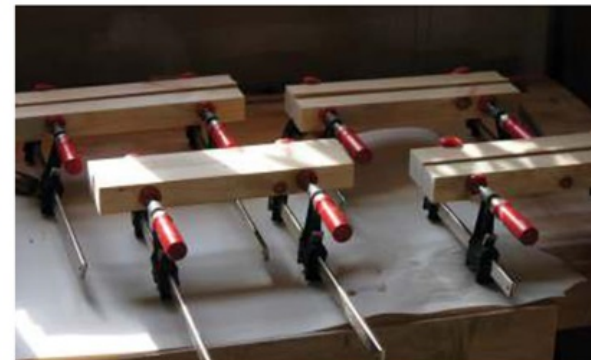
With the shoot strips set, tighten the clamps and leave to set
