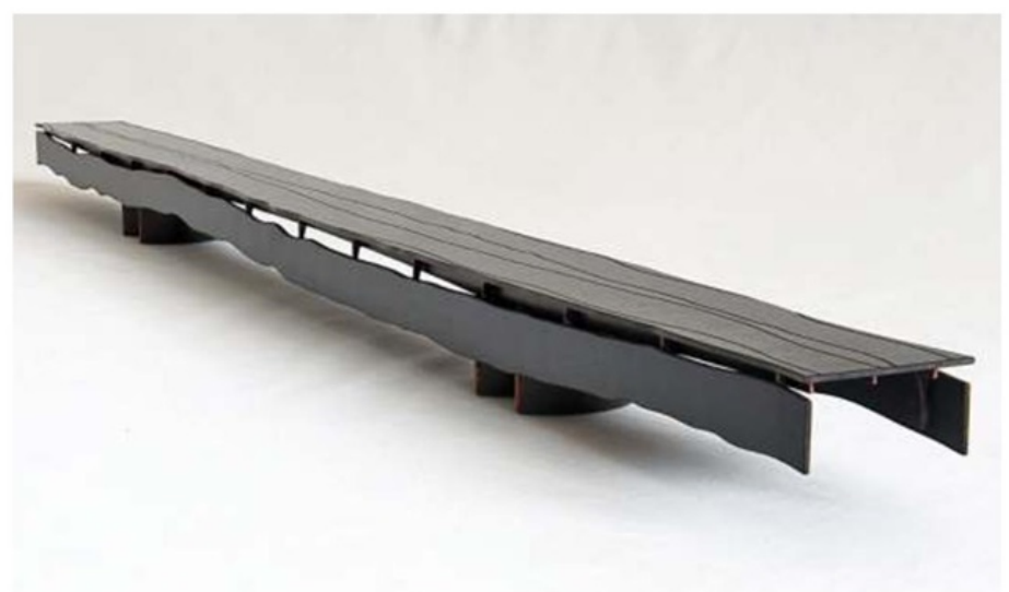
Photograph of a model. The two outer planks folded down reduce the table width to just 900mm and expose the river joints
