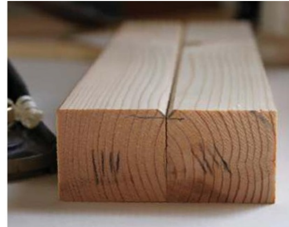
The v-groove jig has a chamfer applied to two corners
