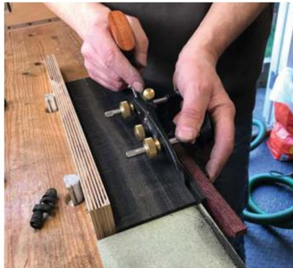
If you don't have access to a router try ploughing the groove for the lid panel and bottom by hand
