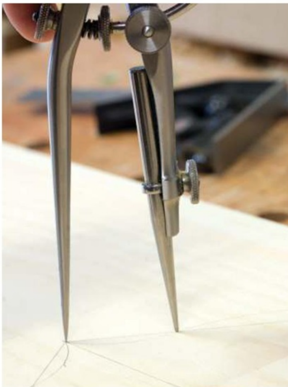
Laying out the foot detail with dividers
