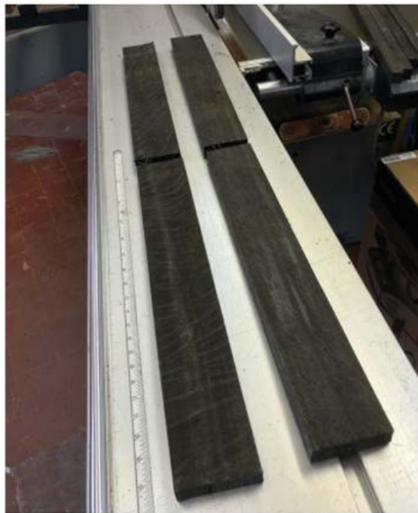
Planks of bog oak sawn into short lengths to preserve the thickness
