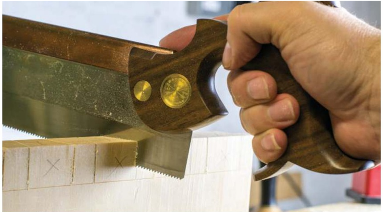
Cutting the dovetails which secure the top to the sides
