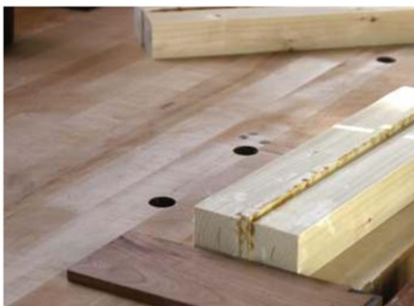
The underneath of the jigs will have the excess material from the shoot strip protruding
