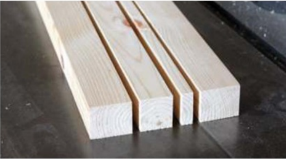
Harvest the separate components from the outside of the boards to avoid the pith
