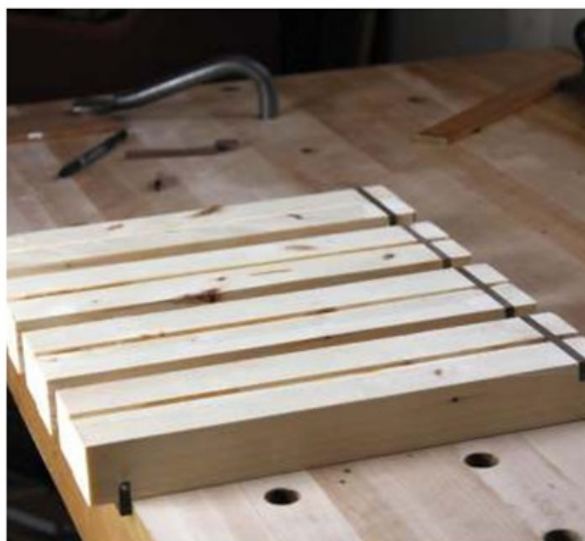
Plane the stops flush with the top surface of the jig
