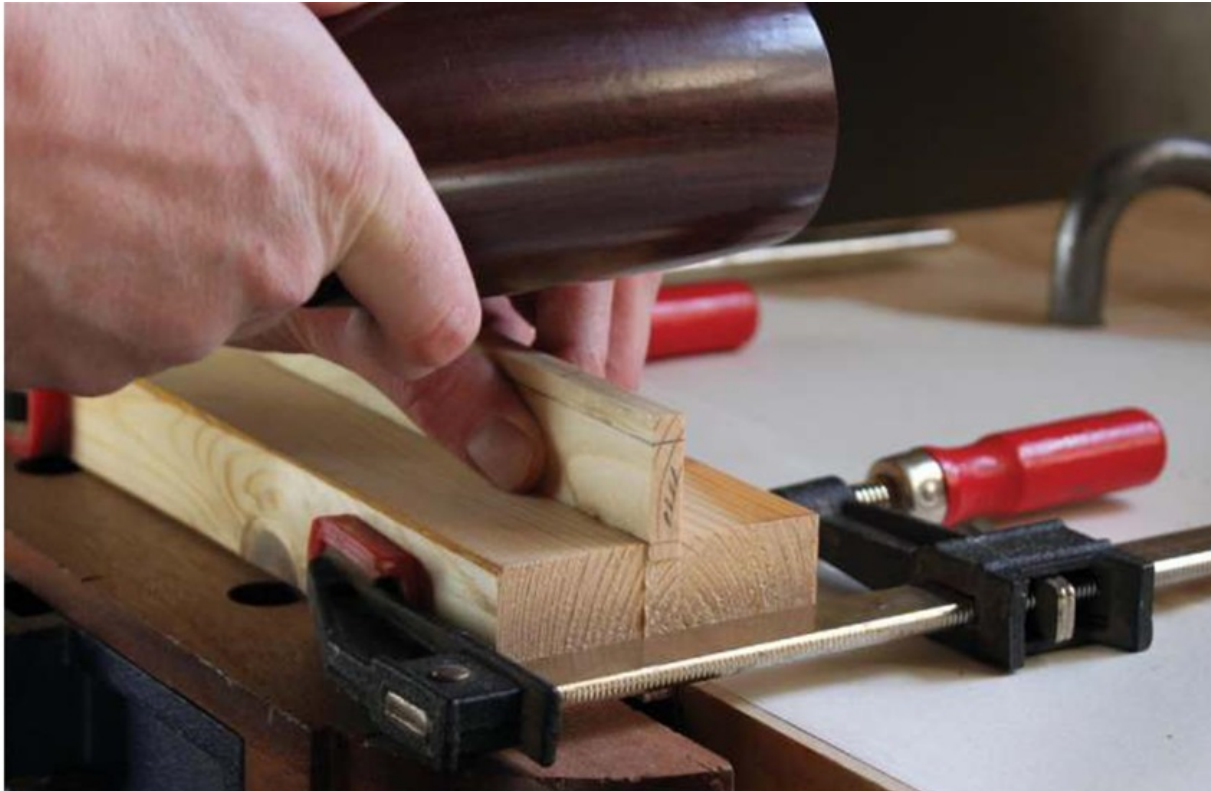
... and use the depth guide to set the shoot strip to the right depth
