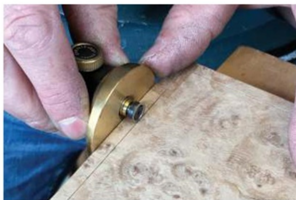
A wheel gauge was used to cut through the veneer before rebating to minimise the risk of splitting
