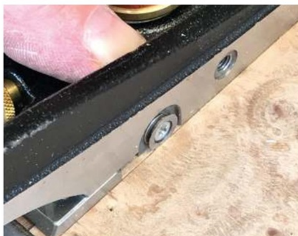
The gauge line is used to locate the knicker and set the fence position
