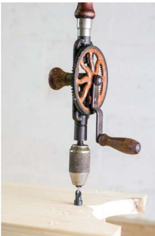
Drilling pilot holes for the Roman nails
