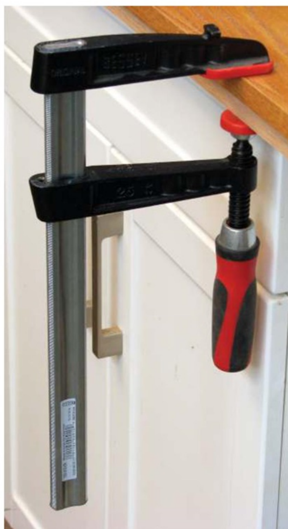
F-clamp handle too close to the cabinet front
