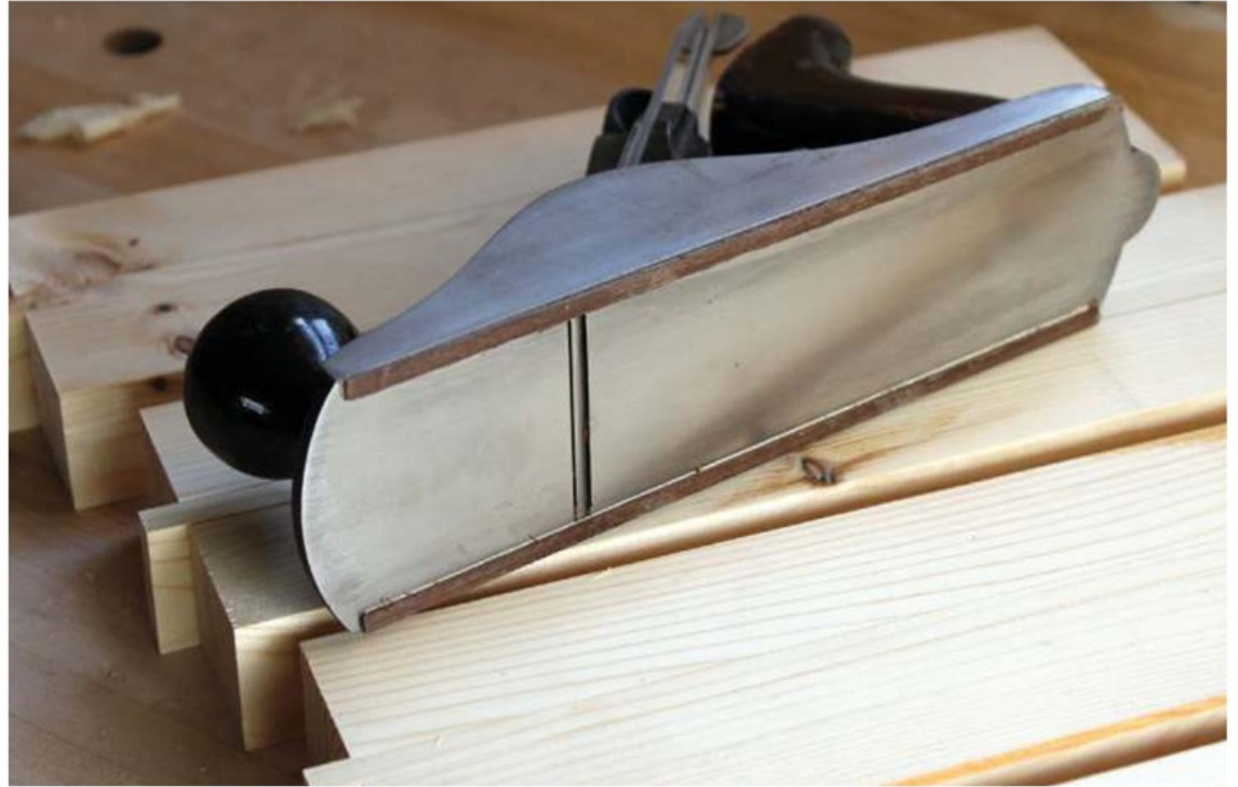
When reglued the jigs need to be wider than your bench plane, in this case a regular #4
