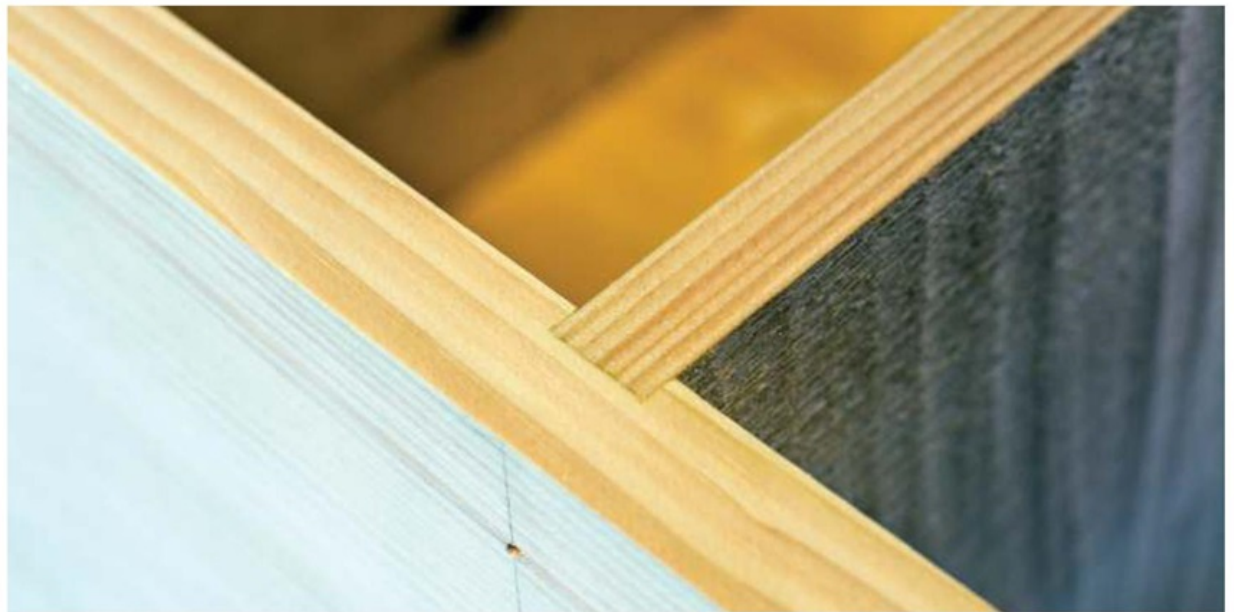
You can see several design elements here – dados securing the shelves, and the scalloped underside of the shelves from the scrub plane
