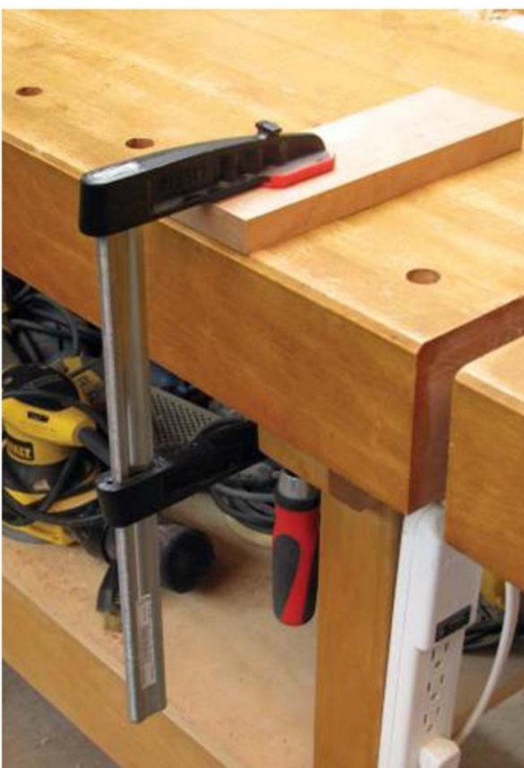
F-clamp handle too close to workbench leg to get a grip on it
