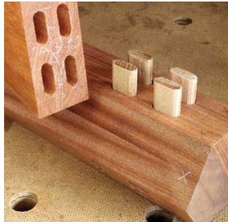
Twin double tenons give added strength to the joint. The rows of mortises were cut by referencing against the same registration face, but with different fence height settings
