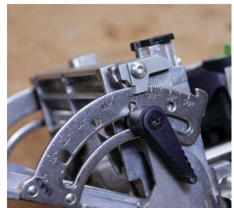
The fence is locked at 60°, the Domino angle for a hexagon
