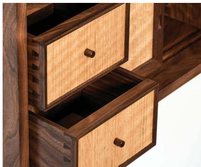
Hand-cut half-blind dovetails and inset drawer face
