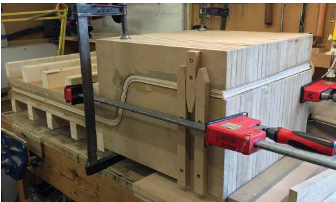
Cheaper and more dimensionally stable than solid timber MDF is perfect for making large formers
