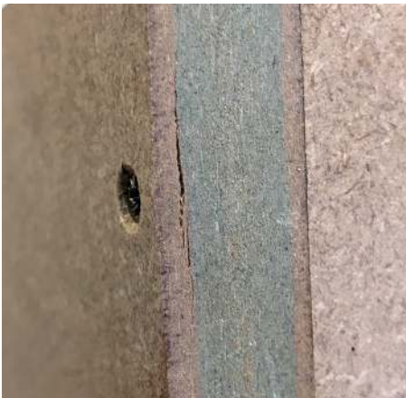
Sinking the screw too deep can pull the core fibres away from the outer skin
