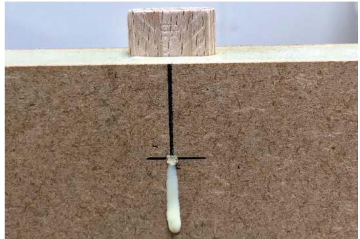
Place a hole at the base of the mortise to relieve the pressure and ease assembly. Tip, don't stand in front of the hole when you start hitting the Domino with a hammer
