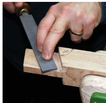
Used like a file, the float will ensure the tenon cheeks are smooth and flat
