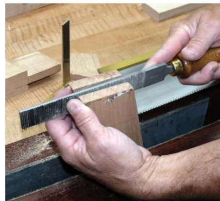
The long flat shape makes alignment easy to square up this bridle joint
