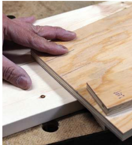
With the jig's edge on the pencil line, secure the jig to the rail with a holdfast or hold-down
