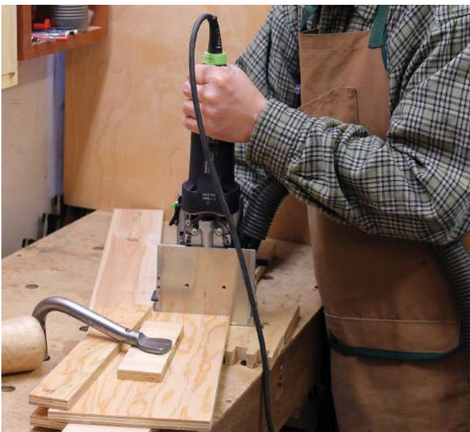
Hold the machine tight to the jig, and slowly plunge the joiner to make the cut
