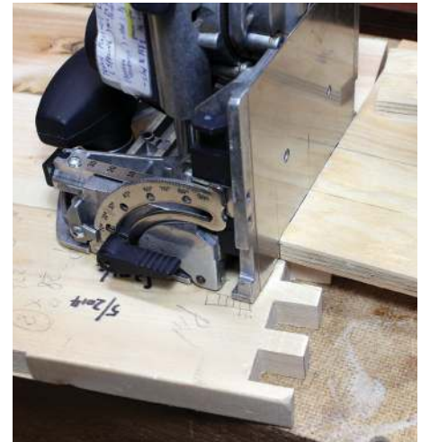
Position the machine with its baseplate's scribed line aligned with the pencil line on the jig
