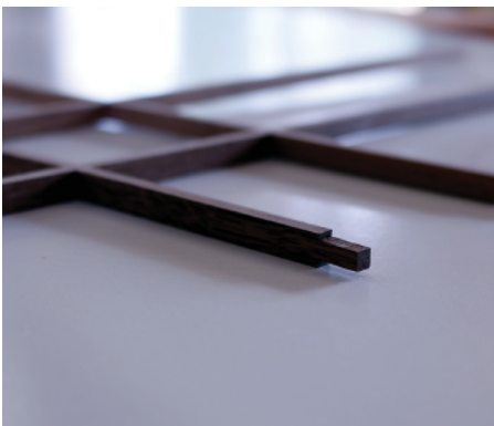
ABOVE: Hand-cut Kumiko tenon ABOVE RIGHT: Gluing the Kumiko, a drop of PVA using a dental syringe RIGHT: The Kumiko lattice assembled and waiting for the Tsukeko frame to be applied
