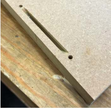
Position the biscuit away from the end of the board and with screw holes close to the slot
