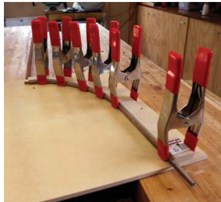
Steamed tapered stems clamped to curve jig
