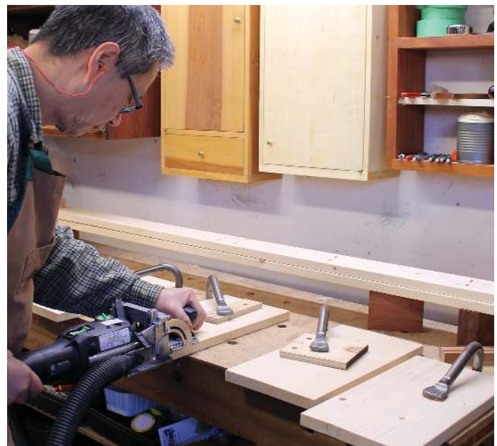
I cut all the front mortises with a standard width setting for precise alignment and the rear ones with a wider setting
