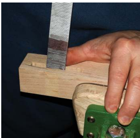
The float aligned vertically makes cleaning up the sides of the mortise a breeze
