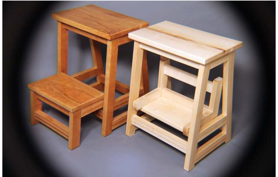
The different angular orientations of the parts to be joined and the narrow width of the stock present a registration challenge for the Domino joiner
