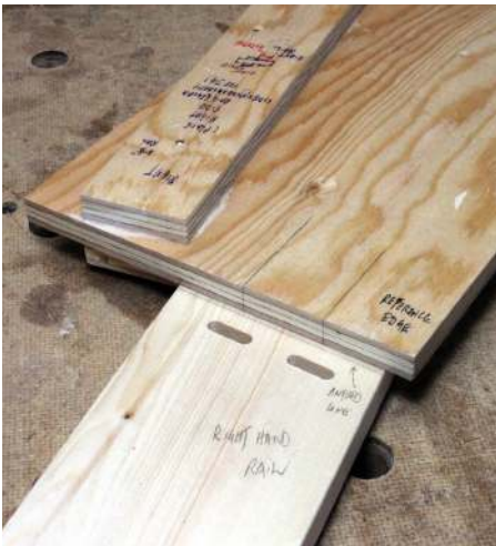
To mark out the shelf location, slide the jig's fence along the rail and hold the jig at the desired location to draw a pencil line
