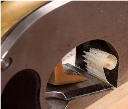
Narrow shavings are bad. A blade that's cutting square takes a shaving across its width. This blade is cutting too deep on the right
