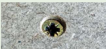
Bury a screw beneath the surface of the MDF without a countersink and...
