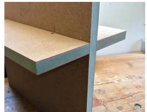
Another strong knock-down joint that doesn't require clamps
