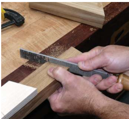
The flat surface of the float ensures your joint shoulders are flat and square, working well on surfaces too small for a shoulder plane
