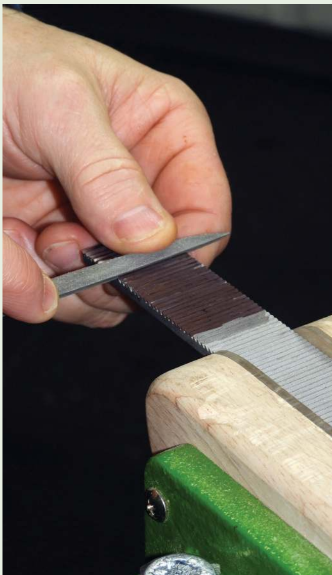
Using a file with a safe edge registered against the next tooth, light strokes are all that's required
