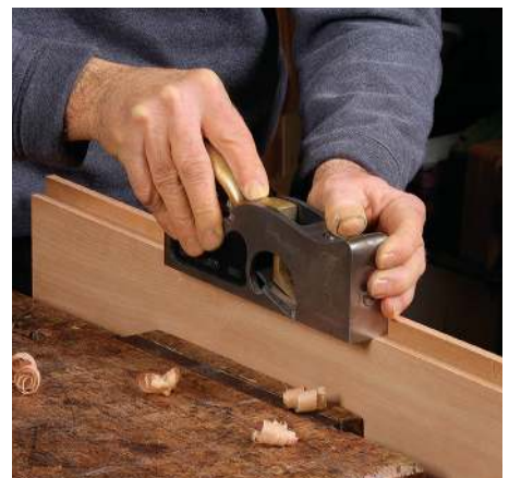
For rabbets, rotate the board (not the plane). For the wall parallel to the board's face (left), clamp the board between benchdogs and use your off hand to keep the plane tight against the rabbet's vertical wall. Use a vise for the other wall (right). With the board on edge, there's no need to lay the plane on its side.
