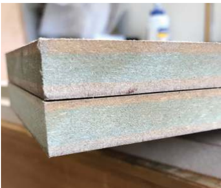
The screw may be tight but the swarf around the screw holes is enough to prevent the components from mating together neatly
