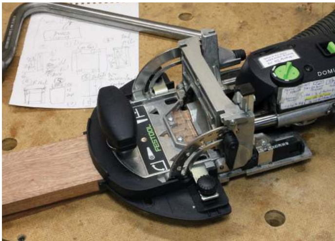
The author uses a trim stop with the joiner for precision and consistency whenever he cuts centred mortises on narrow stock
