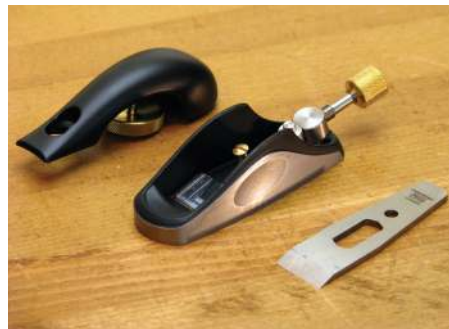
Dismantled, the plane consists of a lever cap, a body with a Norris-style adjuster and blade
