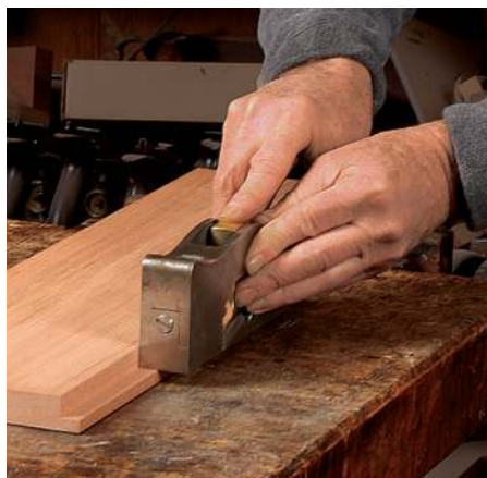
For rabbets, rotate the board (not the plane). For the wall parallel to the board's face (left), clamp the board between benchdogs and use your off hand to keep the plane tight against the rabbet's vertical wall. Use a vise for the other wall (right). With the board on edge, there's no need to lay the plane on its side.
