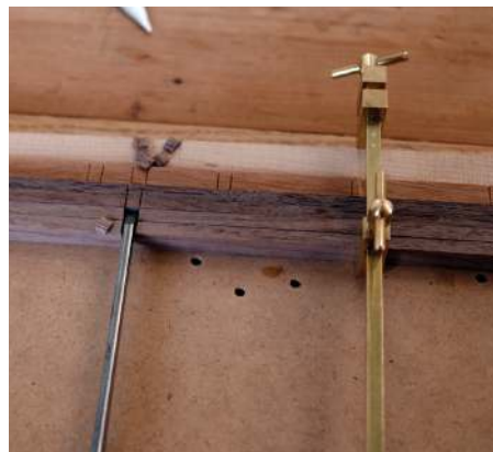
LEFT, ABOVE & RIGHT: Hand cutting the Kumiko half-lap joints
