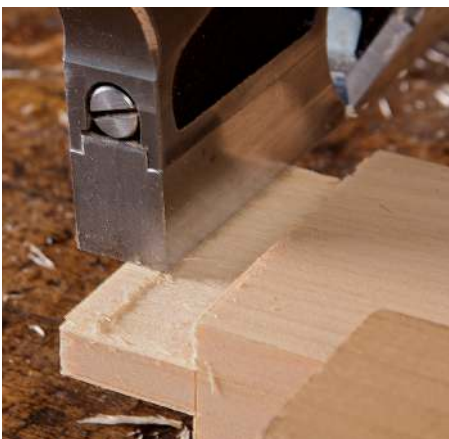
Start at the shoulder. And don't overlap cuts. Otherwise, you'll get cheeks that aren't parallel
