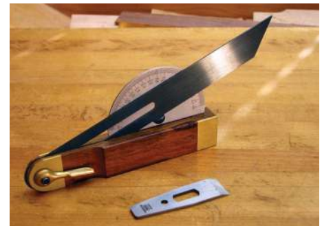
A 20° primary bevel onto a 15° bed makes this plane ideally suited to end grain work
