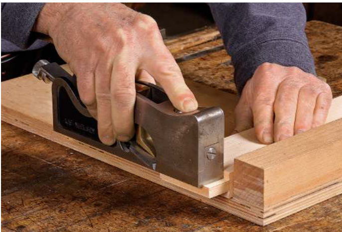
Keep the plane vertical in use. A simple bench hook holds workpieces on their side so you can hold the plane upright, where it is easier to control. For straight tenon cheeks, first place the toe of the plane on the tenon and slide it forward until the blade just touches. Then take a shaving, keeping even pressure on the plane throughout the cut
