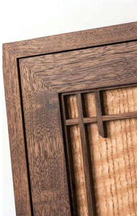
ABOVE: Mitred dovetails and door joinery for visual continuity ABOVE RIGHT: Feature posts provide additional joinery opportunities RIGHT: Detail of the decorative lattice in the door corner
