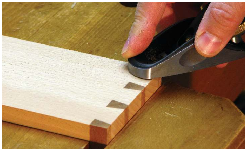
Use it to trim the ends of delicate through tenons or dovetail pins
