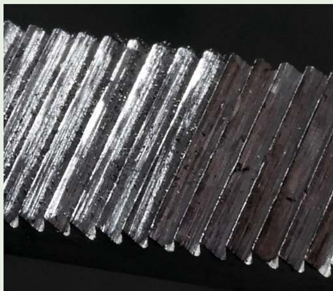
The black marker helps to ensure complete coverage and avoid going out of flat
