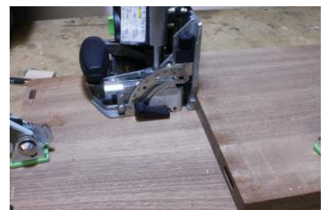
When mortising the vertical piece (side), the shelf is used as a reference edge with the baseplate held against the edge of the shelf
