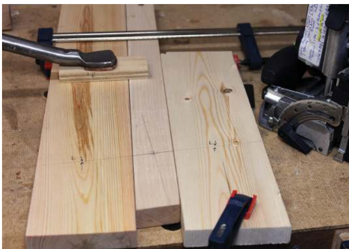
Cradle the leg between spacers and extend the shorter placement line to the enlarged registration surface
