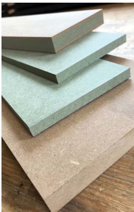
MDF comes in a multitude of grades and thicknesses each with a specific purpose
