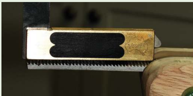
Checking for flatness before sharpening with a quality reference
