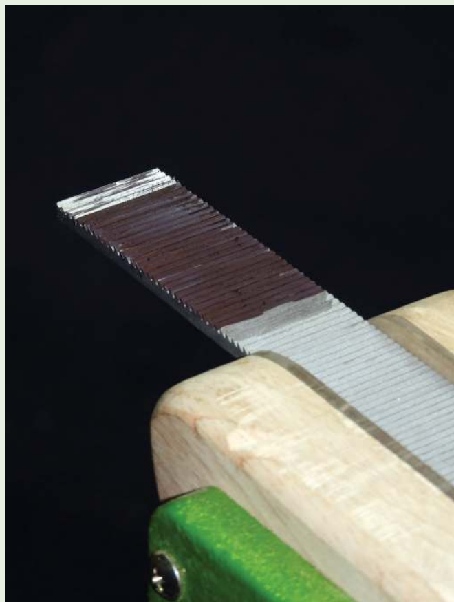
The end of the float showing the black marker removed from the first few teeth as feedback
