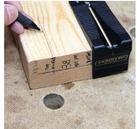
The mortise placement lines marked on the arm/foot will later be used to lay out the corresponding placement lines on the vertical post
