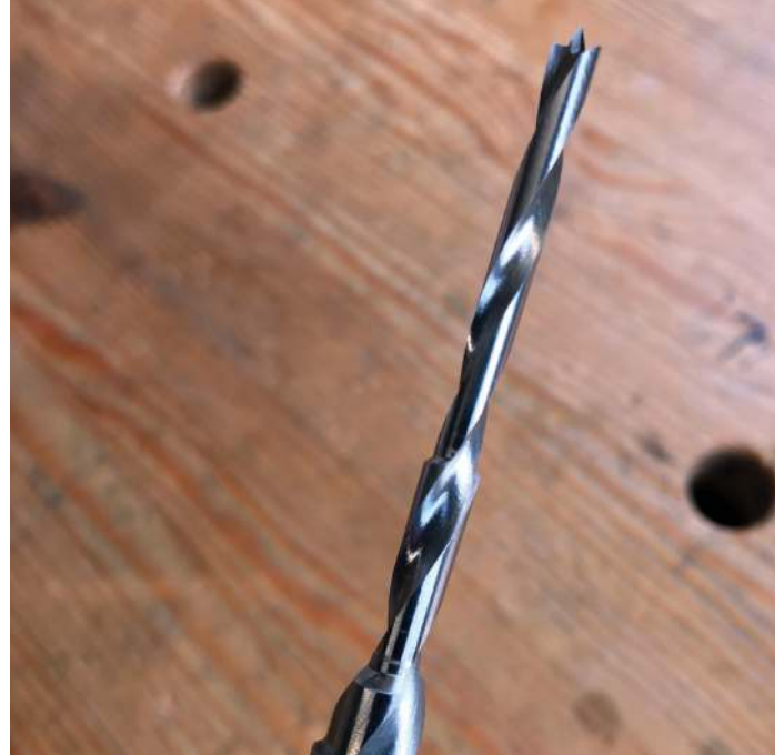
The all in one stepped drill from Hafele for use with dowel screws
