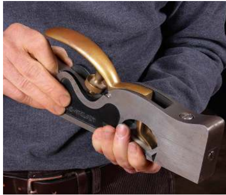
Here's how to fix the problem. Loosen the hold-down just enough to allow you to shift the blade's tang. Move it toward the side of the blade that wasn't cutting (left). When the blade is cutting square, it cuts a full-width shaving that has a uniform thickness (right)
