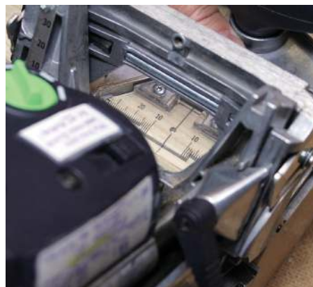
To position the machine, align the sight gauge centre line with one of the placement lines marked on the post's registration face
