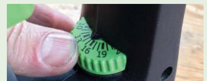
Minimise over tightening by setting the clutch on your cordless if it has one
