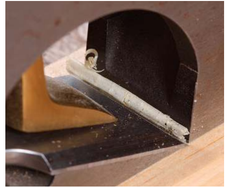
Here's how to fix the problem. Loosen the hold-down just enough to allow you to shift the blade's tang. Move it toward the side of the blade that wasn't cutting (left). When the blade is cutting square, it cuts a full-width shaving that has a uniform thickness (right)
