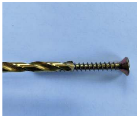
Create a clearance hole for the full thickness of the screw...
