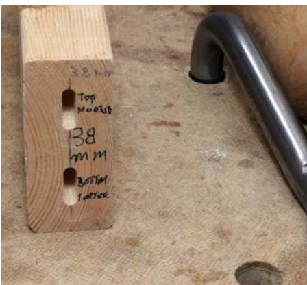
The double mortises can be cut in the centre, or off centre (as in the case of twin mortises), by adjusting the fence height
