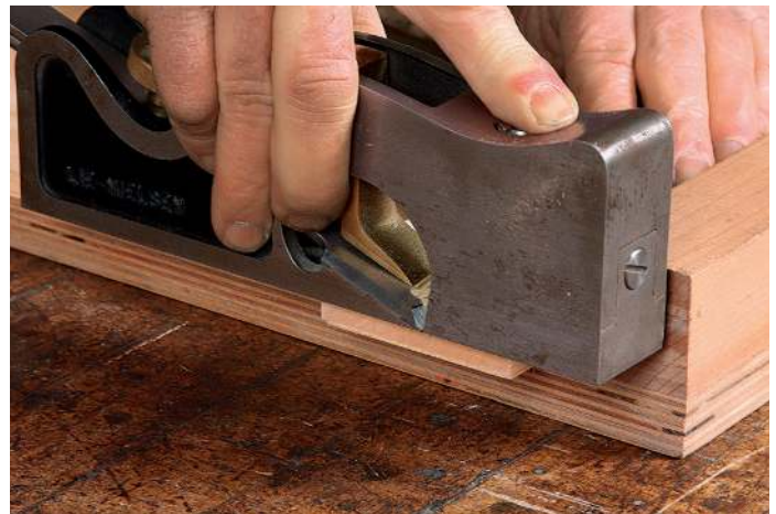
Keep the plane vertical in use. A simple bench hook holds workpieces on their side so you can hold the plane upright, where it is easier to control. For straight tenon cheeks, first place the toe of the plane on the tenon and slide it forward until the blade just touches. Then take a shaving, keeping even pressure on the plane throughout the cut
