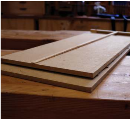
Taper jig for the drum sander
