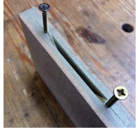
Failing to drill pilot holes can cause the material to delaminate and widen the biscuit slot
