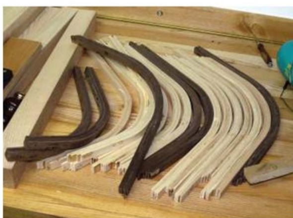
This selection of walnut and ash braces will make four chairs. The two walnut braces on the left are story sticks for drilling the attachment holes
