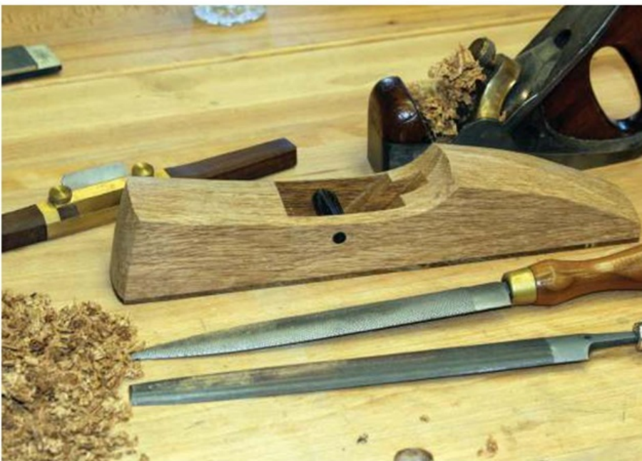
The chamfers are finished with a rasp and file
