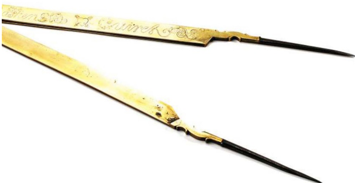
The Cupid's bows, quivers of arrows, garlands of leaves and pierced heart along one of the legs of this 27½in pair of compasses from the 18th century with brass legs and wrought-iron points are likely symbols belonging to the compagnonnage or French system of guilds of highly skilled craftsmen. The scroll-work makes this a handsome tool. On one leg is engraved the owner's name 'SeBastien Cuirel' [ sic ] and on the other his initials in monogram.
