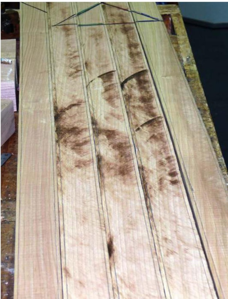
These cherry boards are prepped (left) and resawn (right) to make laminating strips for two Maloof-style rocking chairs. Witness marks allow the lams to be stacked back together for colour consistency
