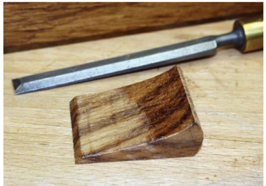
The wedge is cut on the bandsaw and then refined with a scraper chisel
