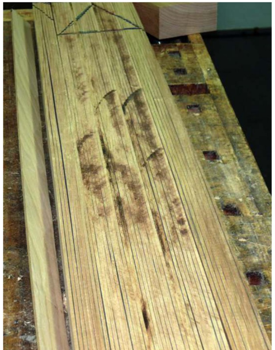
These cherry boards are prepped (left) and resawn (right) to make laminating strips for two Maloof-style rocking chairs. Witness marks allow the lams to be stacked back together for colour consistency
