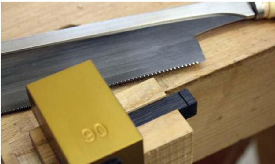
Cutting the shoulders on the cross pin
