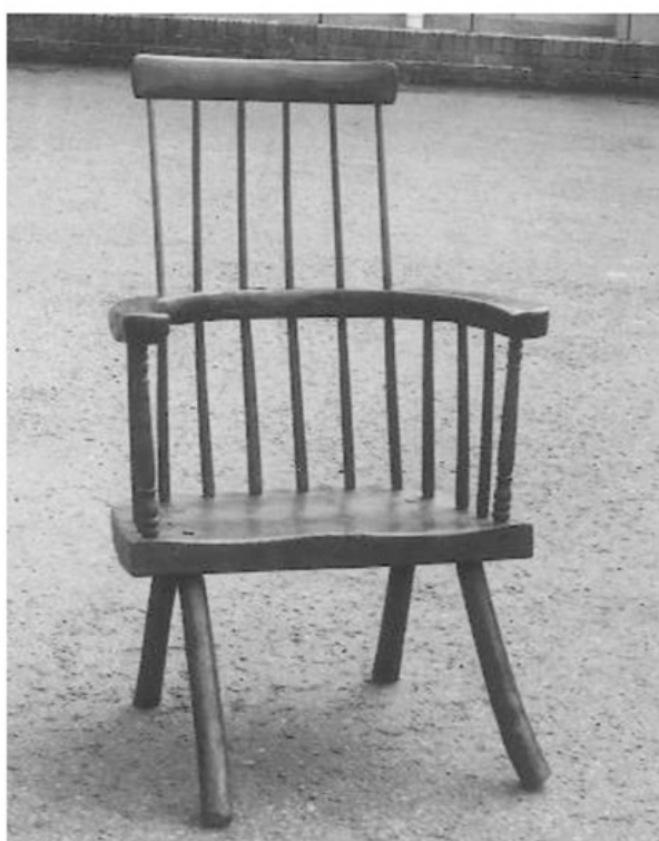
A four-square solid chair, obviously built to last. Some small attempt to scallop the seat, even a slight hollow, improves the comfort no end. Note the heavy arm and tapered sticks. The main arm posts are turned. The weak point is the legs; however, they are attractive, giving the chair its country appearance. A fine up-to-date undercarriage and this chair would be 'modernised' beyond recognition.
