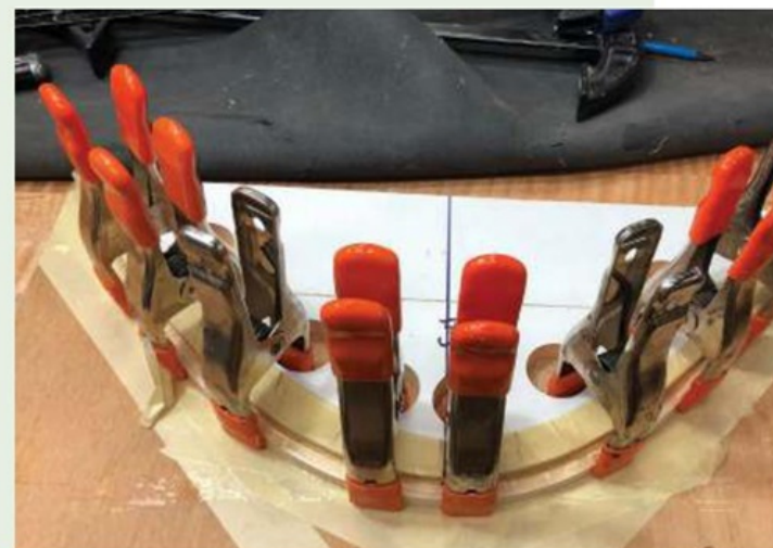
My quick form built from scraps, lined with masking tape holds these four strips of 3mm maple in place while curing
