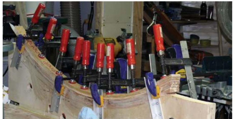
Using the backer strip and lots of clamps to hold the rocker lams in place to cure. Note the angle-iron strips and quick-grips to keep the lams aligned
