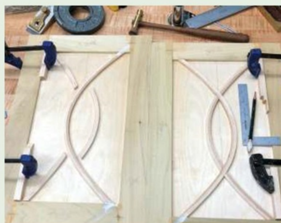
Cutting the pieces to install in the door face, after being thickened to 6mm to be flush to the front of the door frame. The offcuts are clamped in place to provide spacers for the bows
