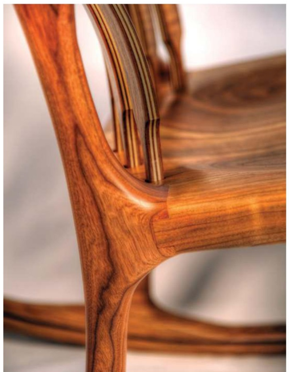
Laminations can be used structurally to create dramatic visual effects
