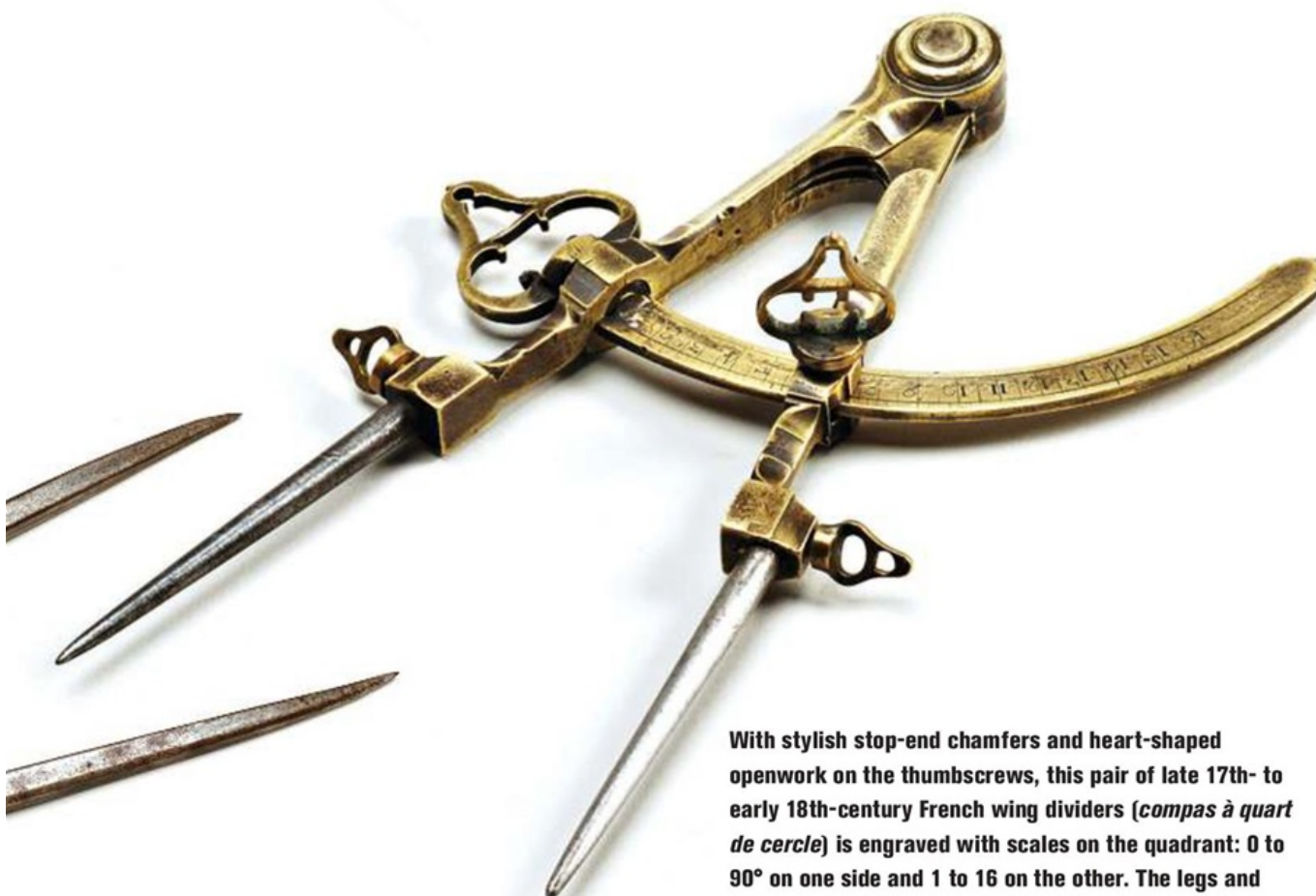
In patinated copper alloy, this pair of dividers is much akin to Gallo-Roman compasses, such as those at Vesunna, the Gallo-Roman museum in Périgueux, France. How little the design has altered between the Roman period and today.
