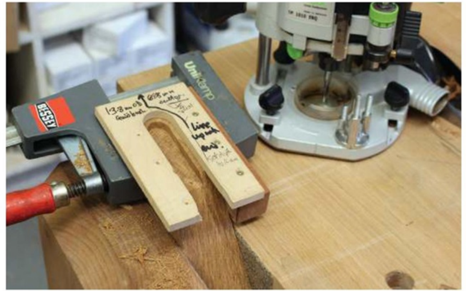
Routing the recess for the chip breaker screw
