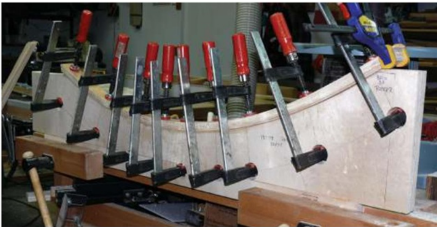
This rocker form is made from sturdy plywood, and a custom-built backer strip to ensure consistent pressure along the length
