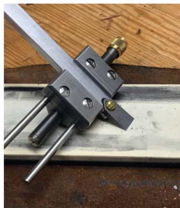
Set the bar into a honing guide for convenient and repeatable results
