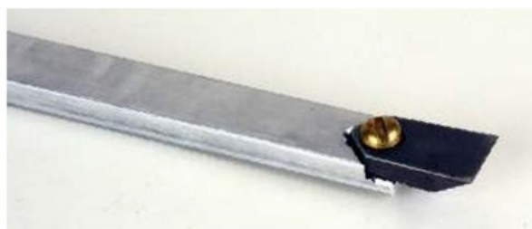
The cutter tip attaches to an extension bar for sharpening
