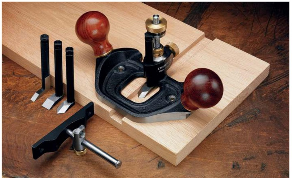
The Veritas Router Plane comes with a depth stop fine adjuster, a reversible tool post and two-piece cutter
