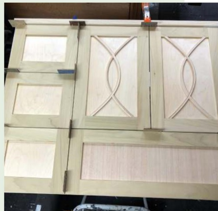
The final door arrangement for the vanity with inset curve detail, ready for painting
