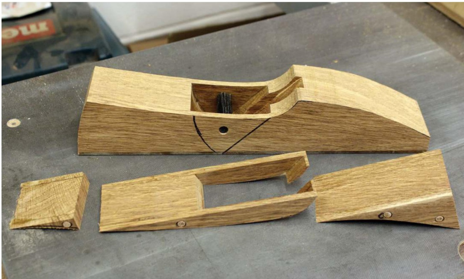
Three cuts on the bandsaw form the basic outline of the plane
