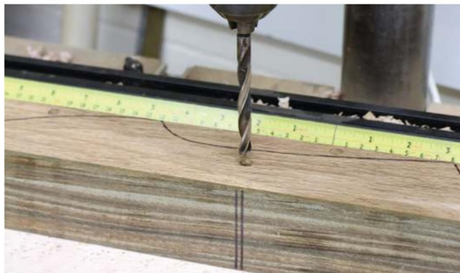
Drilling holes for the dowels and cross pin
