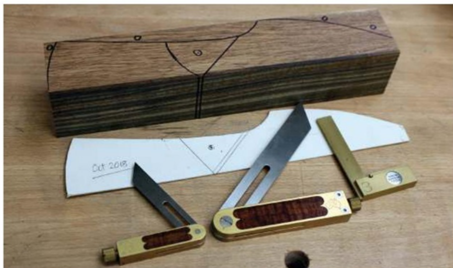
Marking out using a template, bevels and square
