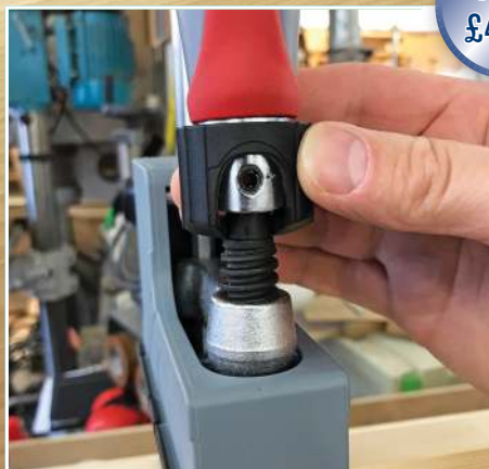
Rotate the collar at the base of the handle to unlock it
