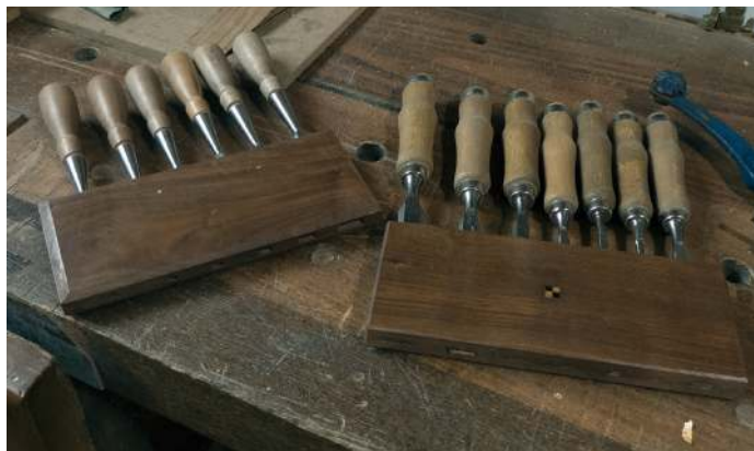
The racks also prevent the chisels from rolling around the bench
