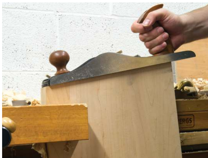
With a 25° bevel, the No. 62 is perfect for trimming end grain
