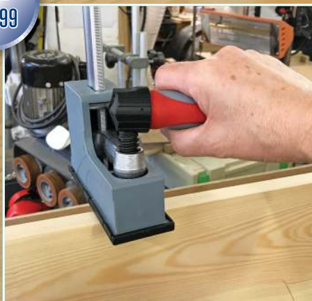
Flip the handle through 90° to gain more purchase and increase clamping pressure
