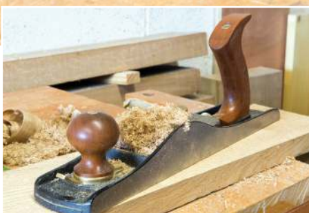
Processing oak for a chair crest rail using the toothed blade
