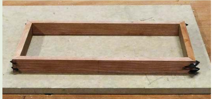
Splines are cut into the corners of the tray after the initial assembly
