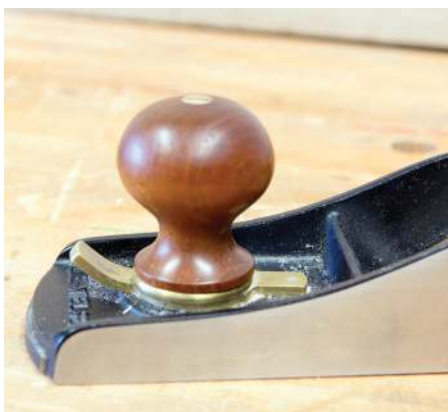
Twisting the front knob unlocks the mouth plate
