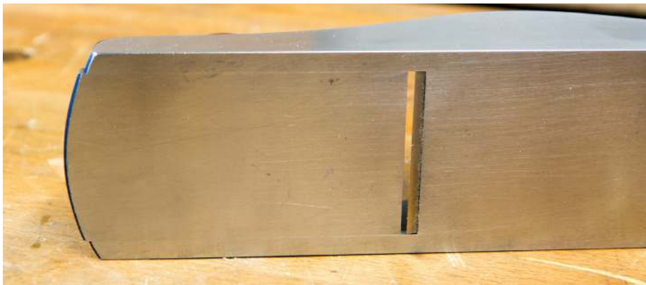
The mouth aperture can be adjusted by twisting the front knob and sliding the mouth plate
