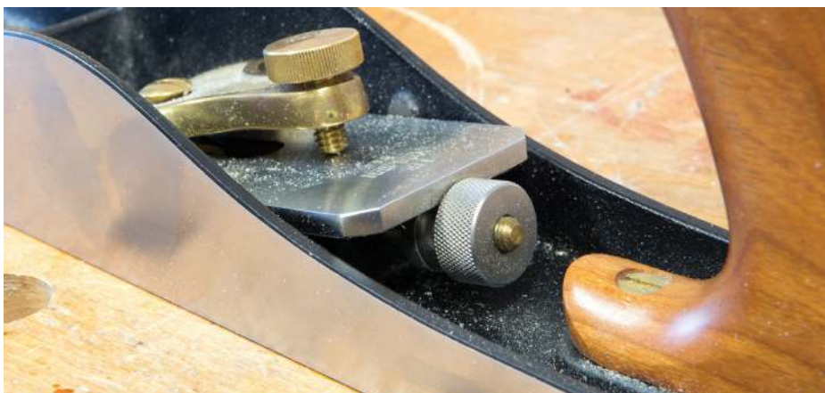
The knurled adjuster changes the depth of cut
