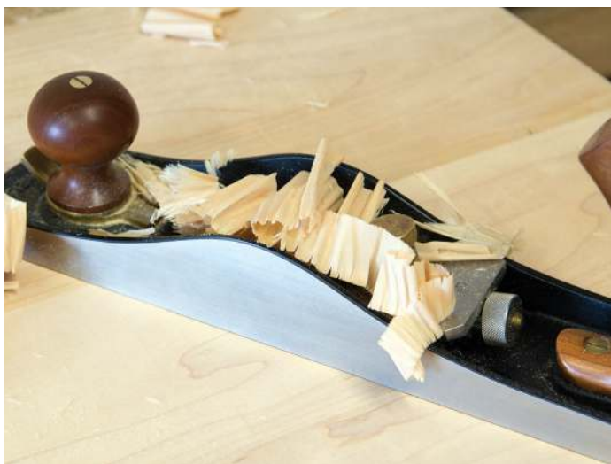
Flattening the seat blank
