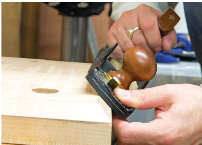
The low centre of gravity makes for a very comfortable experience when planing chamfers
