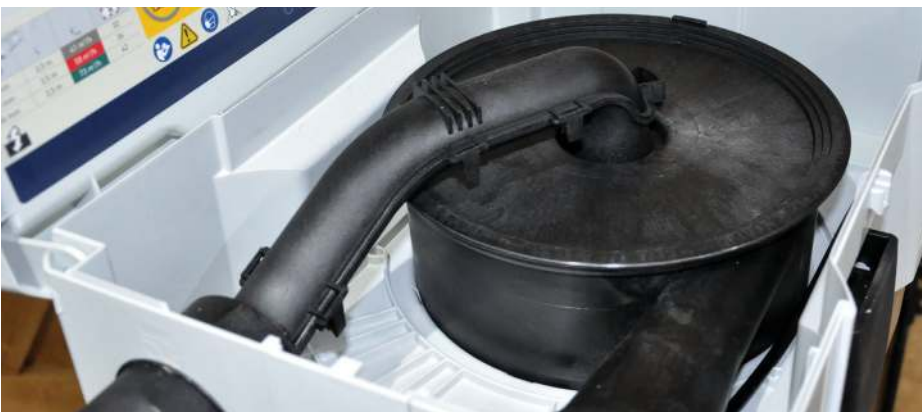
The separator cyclone components. Note on the end there is a removable panel between the two hose connections to allow fitting of a mains socket which plugs into the extractor outlet, purely for convenience of the height
