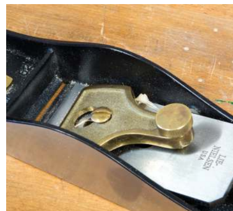
The iron is orientated with the bevel facing up, and held in place with a large cap iron
