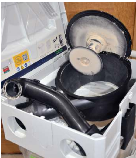
The disassembled cyclone, no tools required
