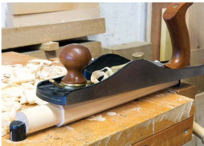
Shaping chair legs into tapered octagons
