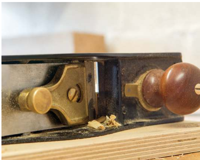
The No. 62 can be used as a very effective shooting board plane
