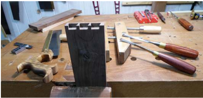
Making the pins on the drawer fronts
