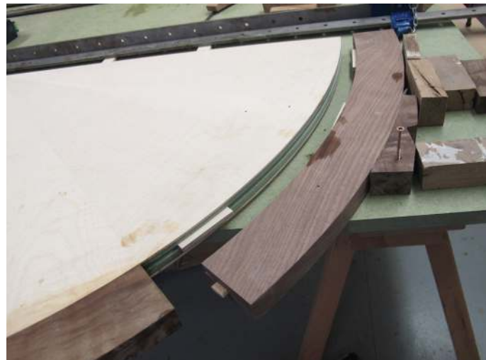
Splines and Dominoes used to attach the walnut lippings to the edge of the table
