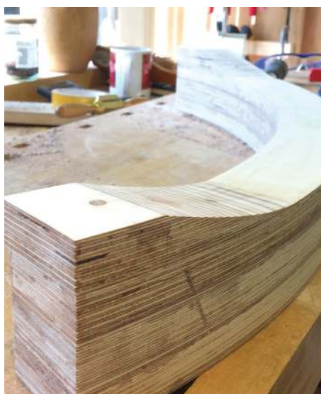
Apron core built from layers of ply
