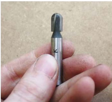
A core box cutter of the same diameter as the dowel cutter is also required
