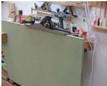
Planing a minute hollow on the edge lipping
