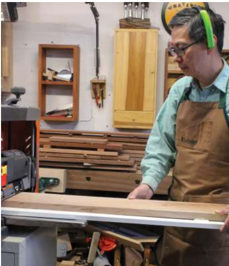
A planing sled and shims allow you to flatten rough stock with a thickness-planer alone
