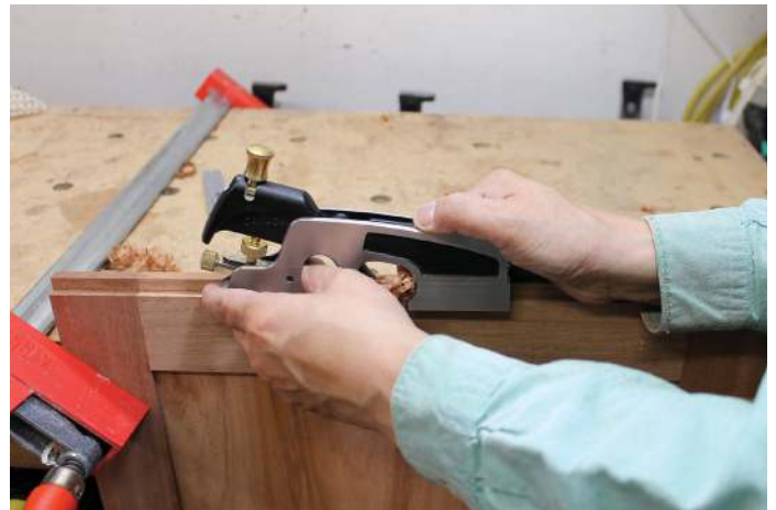
Chamfer the back edge of the cheek to allow the door to ease into the upper track
