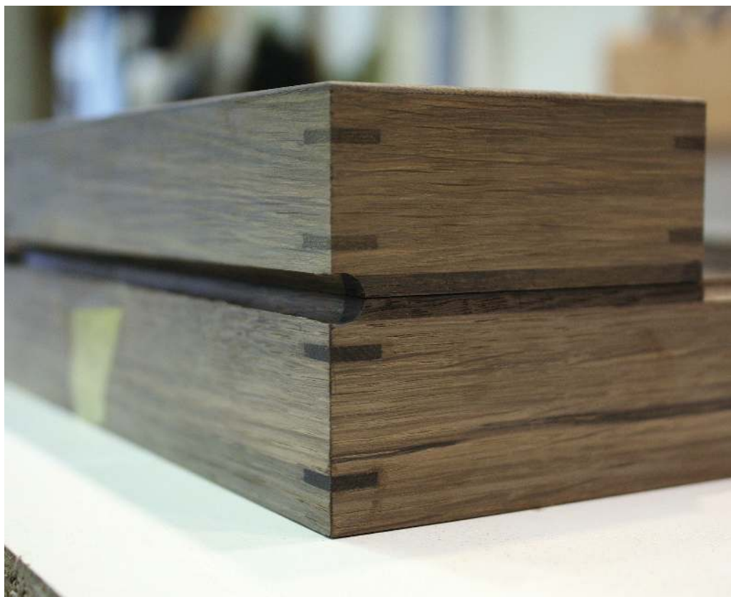
You need only machine one edge of the box for a single hinge design
