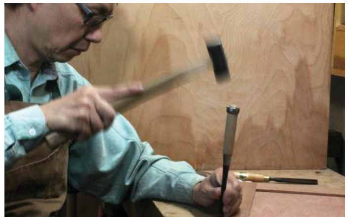
Hand tools offer better control and reduced risk in making cuts on a finished door
