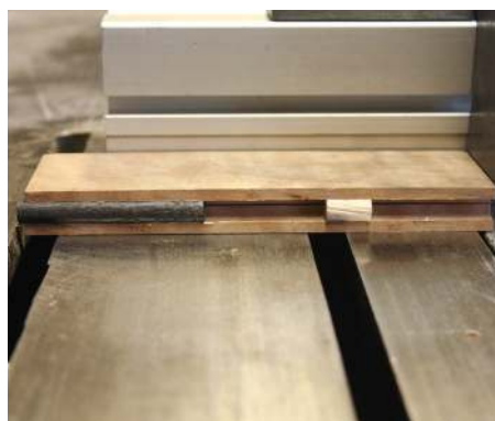
Use one end of the jig to clean cut one end of each of the dowels
