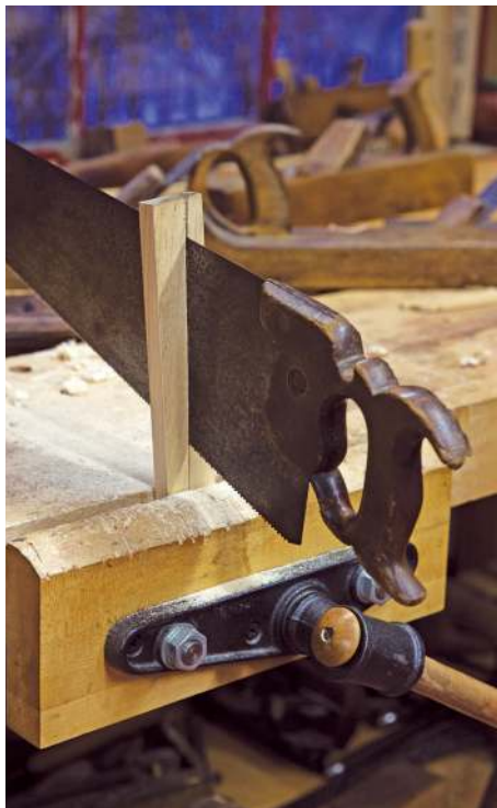
The lid's cleats were sawn out of one piece with no wasted wood and no further shaping
