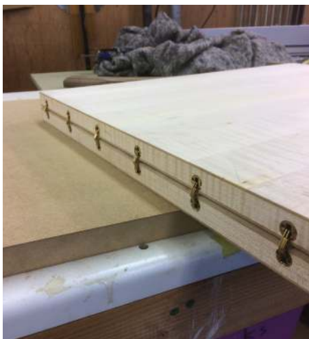
Barrel hinges installed
