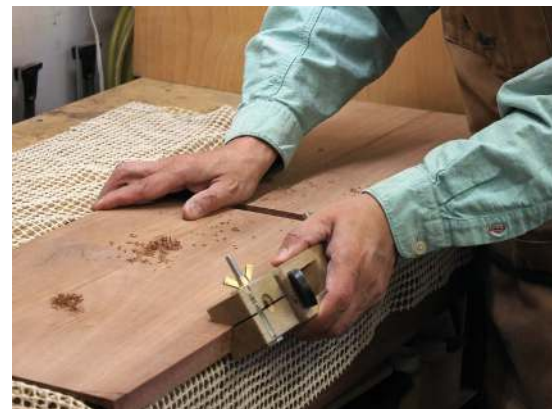
Ease the edges to remove the sharpness and add some edge protection
