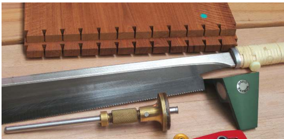
Cutting the carcass dovetails using a 1:5 magnetic guide
