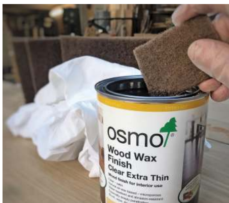
Using a Scotch pad to apply Osmo
