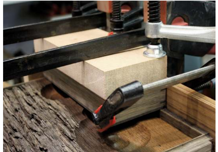
Clamping the hinge in place may require some hefty blocks and support boards to locate the parts accurately
