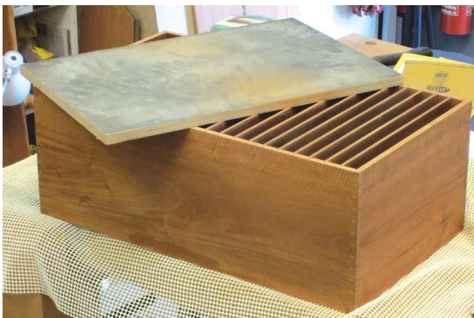
Using my large sanding board to get all the parts flush
