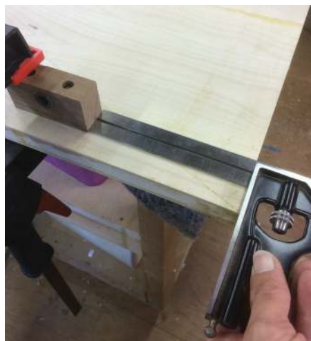
Determining the position of the pivot blocks on the underside of the table leaf
