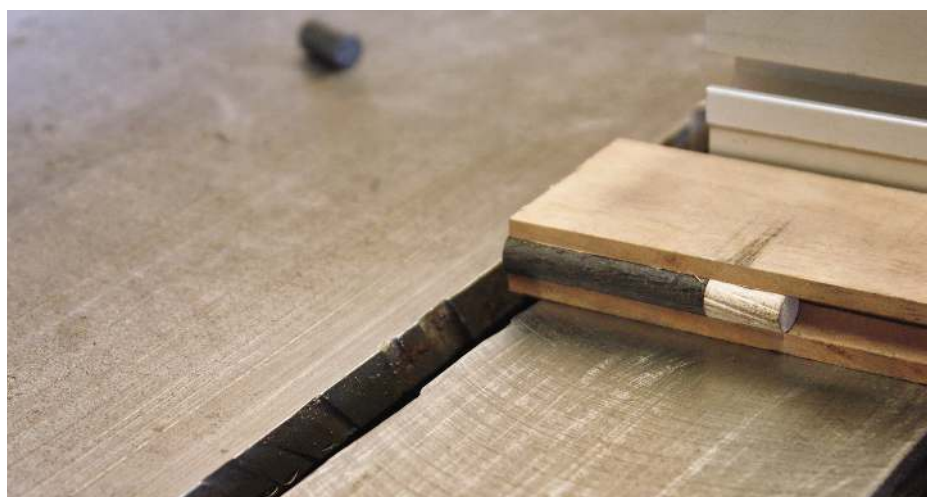
Use the 'stopped' end of the jig to finally cut the dowels to their finished dimension
