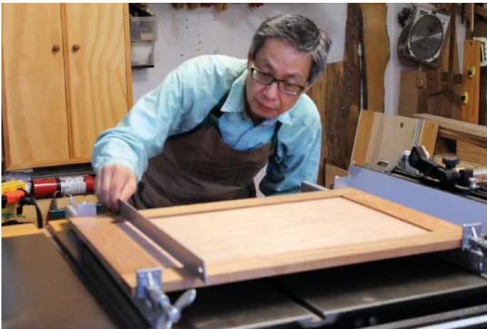
Check the door for flatness and then for wind (using a pair of winding sticks)
