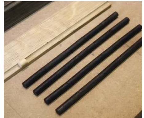
When assembled, lightly sand the hinge with a fine abrasive to key it up for gluing
