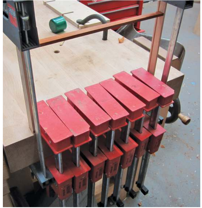
Gluing on one of the false fronts with plenty of clamps
