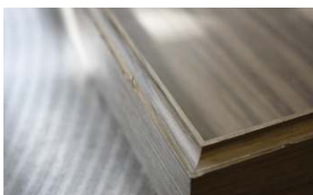
Resist the temptation to clean the channel after it has been machined as it may affect the fit later on
