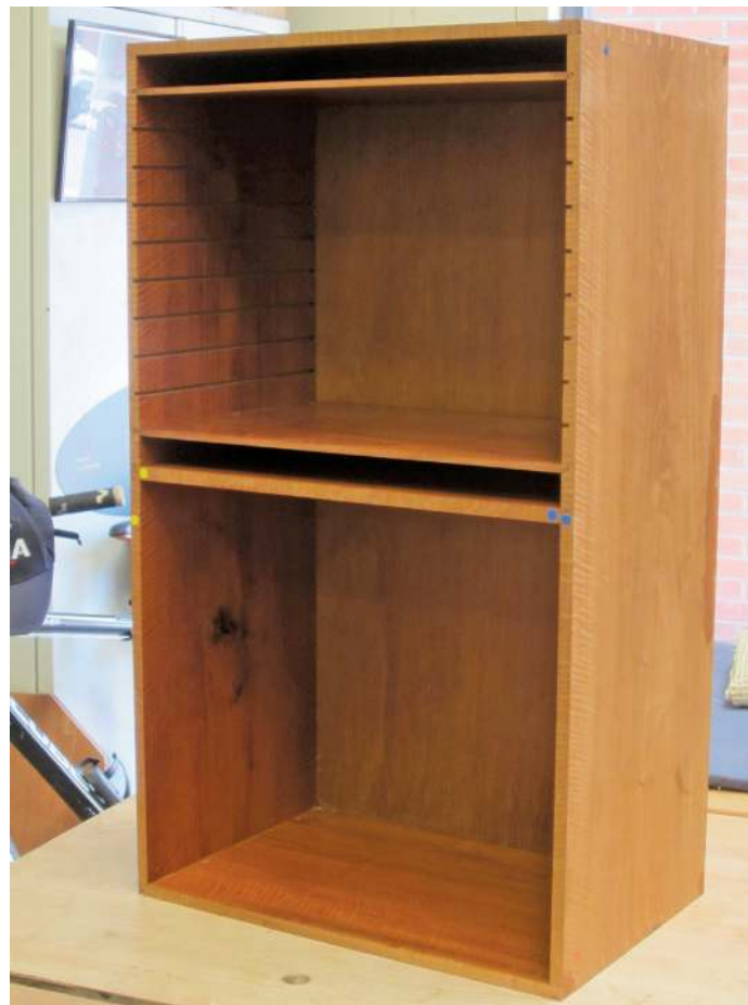
The carcass glued up, the shelf supports will be glued in later
