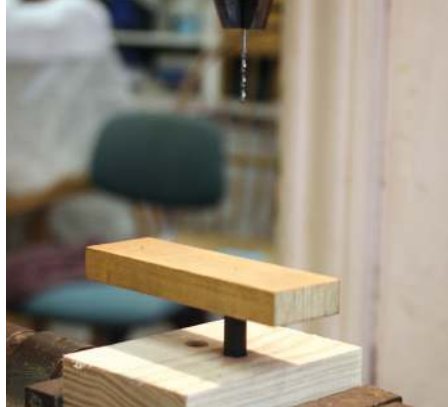
Place a dowel in the holder and position the guide block over the end of the dowel
