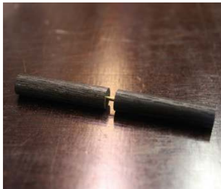
Cut the brass pins and assemble a set of components to make up a complete hinge
