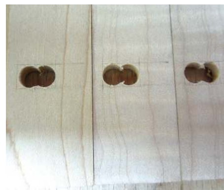
The bulk of the waste removed for the mortises in the sides
