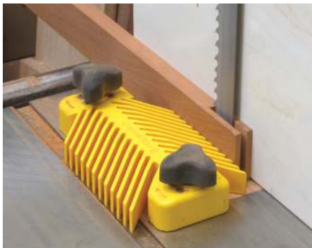
Cutting the mortises for the bridle joints on the bandsaw
