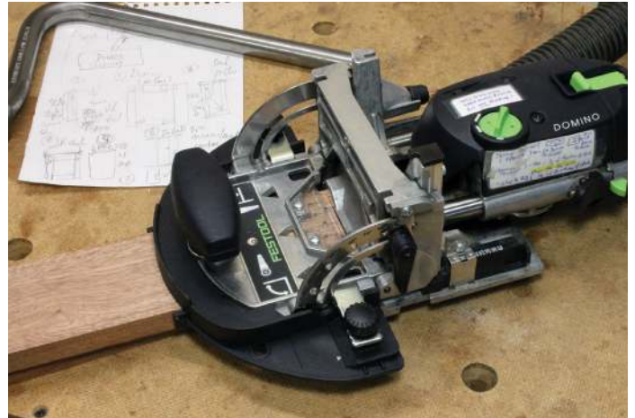
When mortising members on the endgrain, always use the narrow Domino setting
