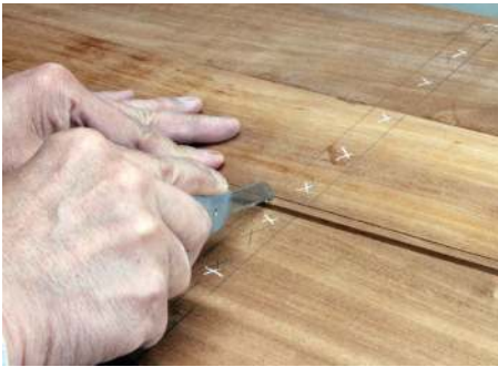
Mark the first dado, then transfer it to the other board with a knife and square for consistency
