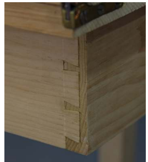
The half-blind dovetails were copied from rubbings of the original
