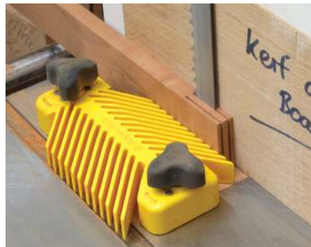
Cutting the tenons, with the same fence setting, using an offset board
