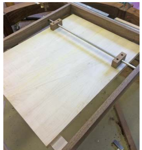
Leaf installed with steel rod threaded through the pivot block and apron cross stretchers
