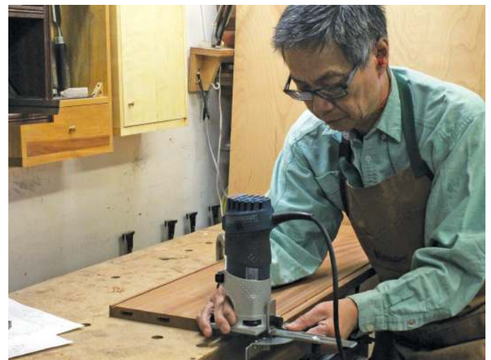
When routing a groove with a fence, rout left to right so the bit is pulling the router against the fence
