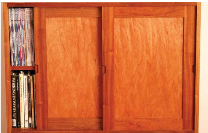
Use the cabinet opening (and not the door because of the uneven penetration into the grooves) to locate the centre point for the pulls
