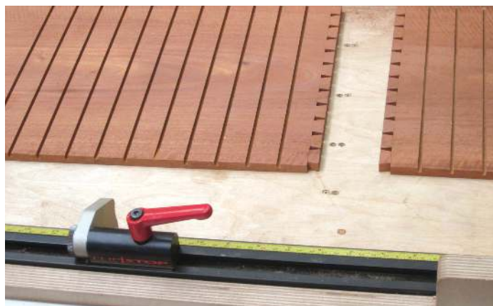
Grooves for the shelf supports being cut on the tablesaw
