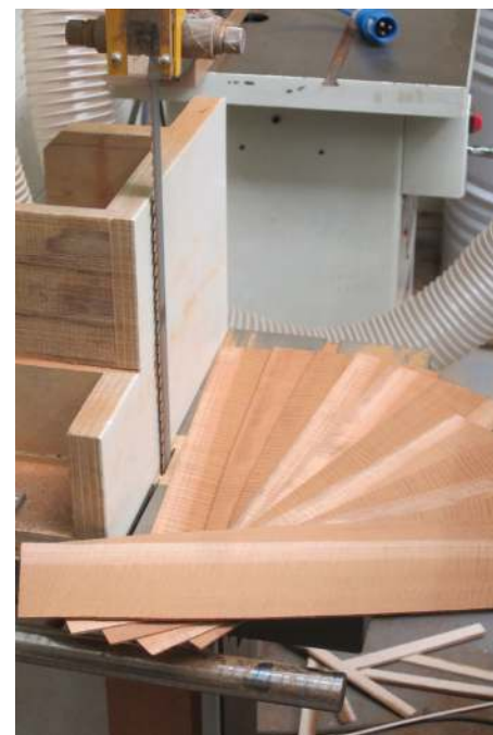
Bandsawing the drawer fronts from figured stock
