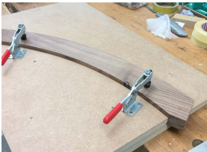
Jig used to cut the lippings at the correct angle
