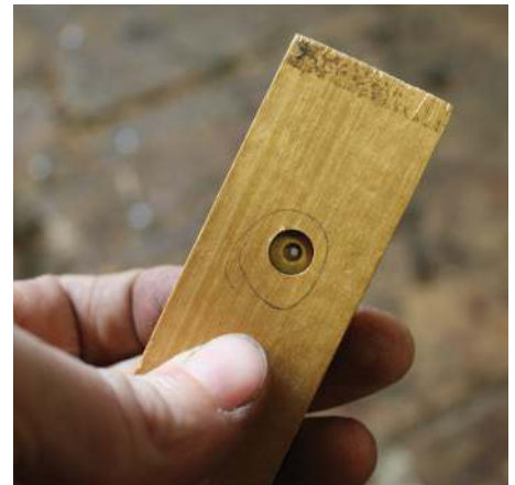
On the same centre, drill an 8mm hole partway through the hardwood guide block
