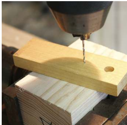
Drill a 2mm hole through a separate piece of dense close grain hardwood to make a guide block
