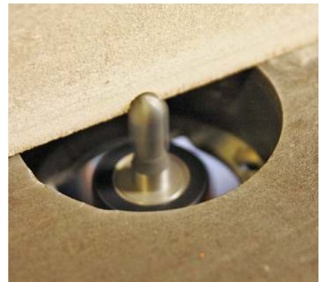
Fit a sacrificial fence to the router and slowly raise the core box cutter into it
