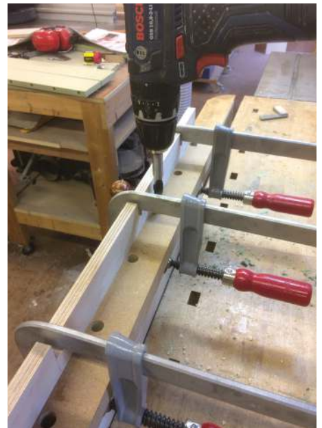
Drilling holes for the barrel hinges using an alignment jig
