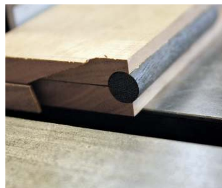
Cutting into the jig will help to prevent breakout and furring of the edges
