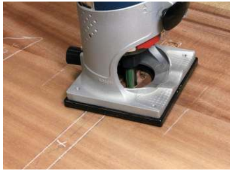
If you use a fixed router, pre-drill a blind hole on the board for the router bit to start freely
