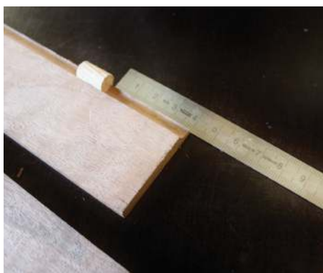
Calculate the number of dowels required for the hinge and make up a depth stop jig with one of the templates
