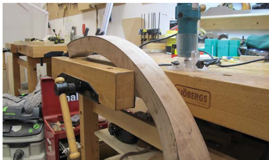
Trimming the apron walnut veneers with a router
