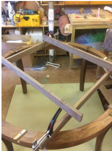
Constructing the internal frame for the extending runners and pivoting leaf
