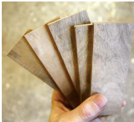
Prepare several blanks to use as test pieces and templates for holding the hinge components later
