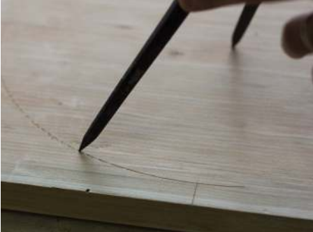
The ovolo corners were laid out with dividers and a square, just as was done with the original
