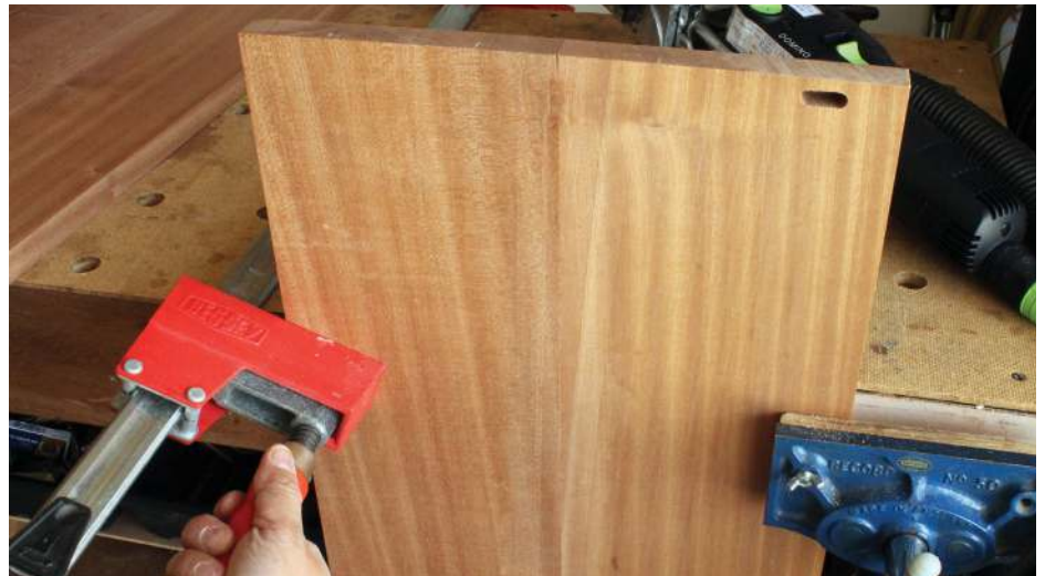
A long clamp is used cleverly with a vice to hold a wide board vertically to the bench
