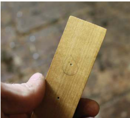
The guide holes can become worn so make more than one and mark them accordingly
