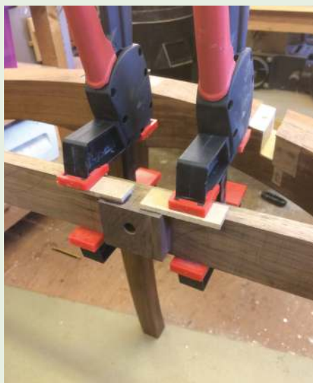
Drill guide block used to drill pivot holes in stretchers
