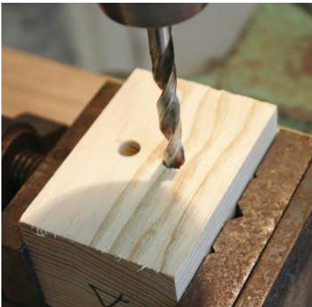
Drill an oversize hole in a block of hard wood to hold the dowel; 8.1mm dia in this case for an 8mm dowel
