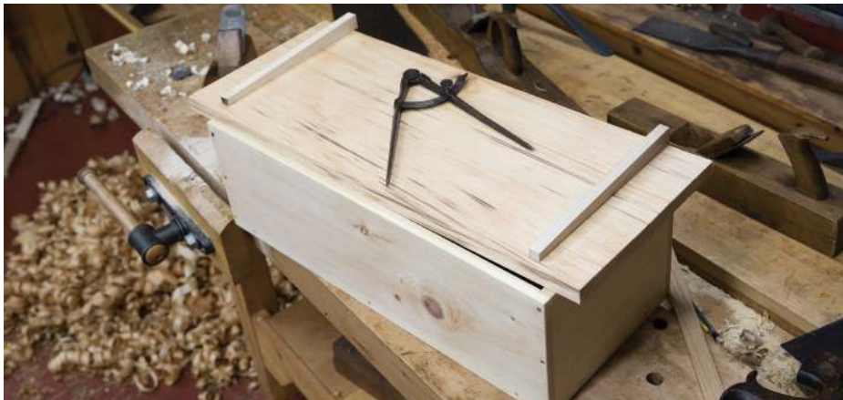
Dividers were used to design the box proportionally. Here, the cleats are ready to be installed onto the lid
