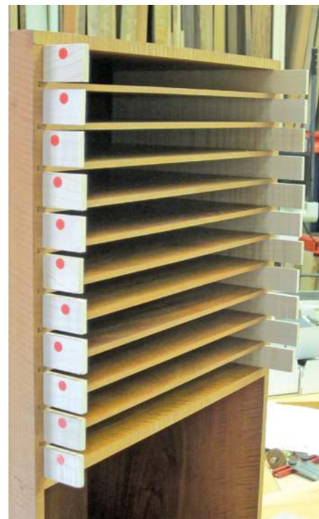
All the sides fitted in their openings and numbered
