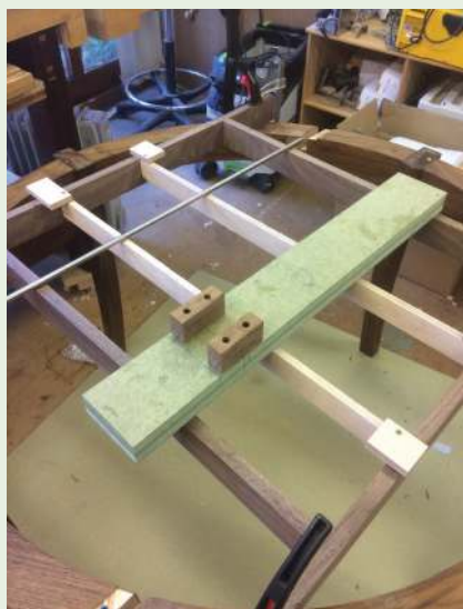
Leaf mock-up and temporary plywood stretchers
