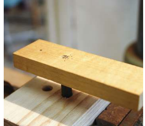
The guide block will now steer the drill bit onto the centre of the dowel
