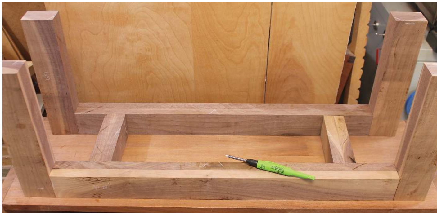
Prepare the components of the stand slightly overlength and place them on the cabinet to determine the stand's final size
