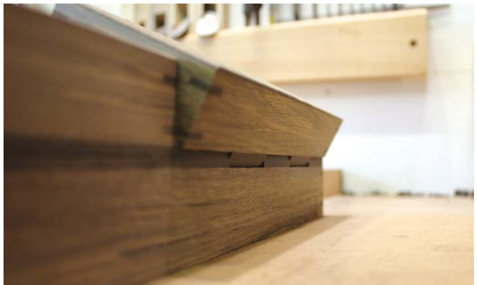
From the outside the hinges are hidden until the lid is opened
