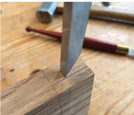
A mortise chisel determines the thickness of the tenon
