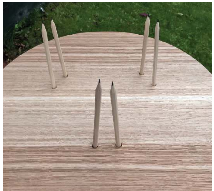
Adjacent pairs of pegs pinch the top to the base
