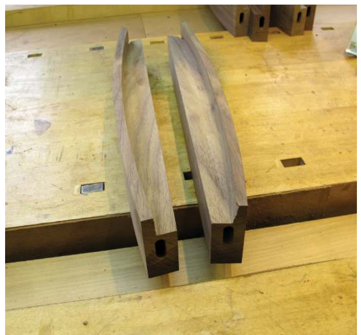
Completed side rails with rebates cut for drop-in seat
