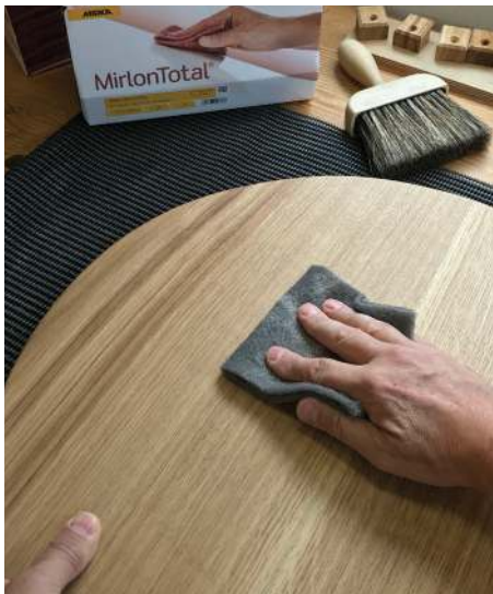
The Mirlon Total pads have many uses, they can be used to cut back in between coats of finish...
