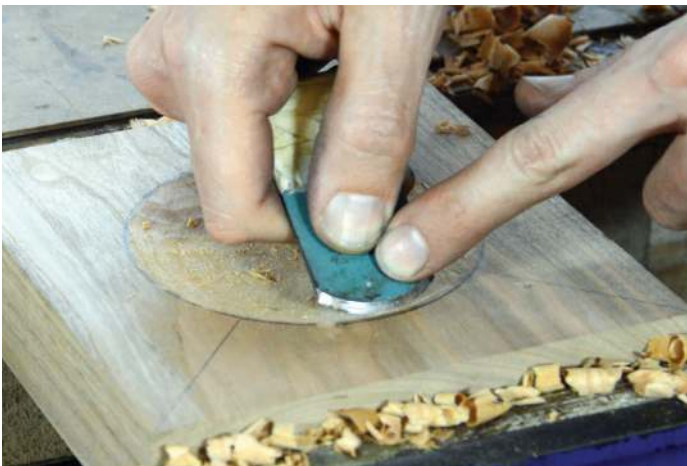
Use a cabinet scraper to smooth the edges
