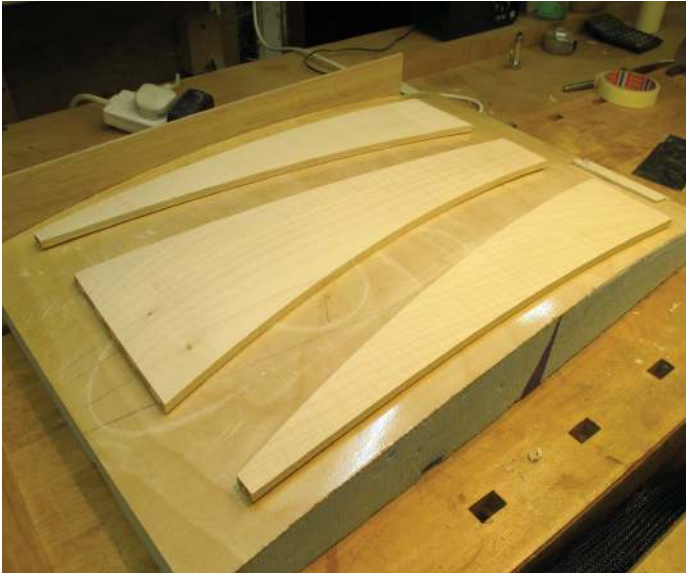
Finished back splats on the former used to produce them
