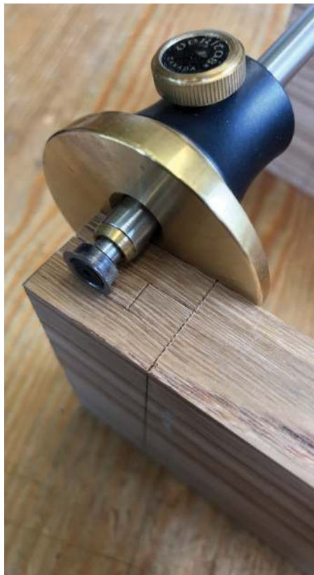
Capturing the second measurement to complete the joinery layout
