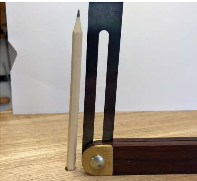
Drill holes through the top at the same splay angle for the pegs
