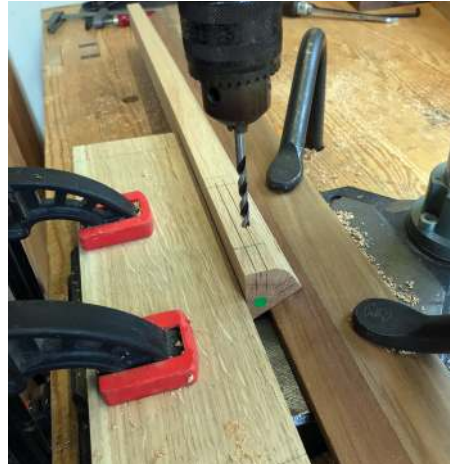
Drilling out the waste for the mortises using the 30° support board
