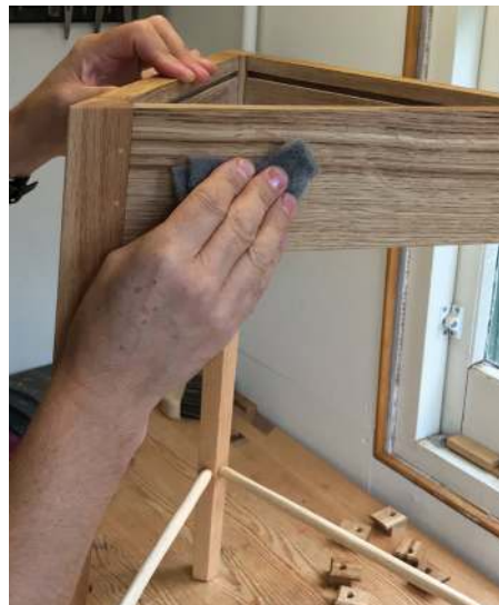
... and then used to apply an oil finish like Osmo and finally to apply a coat of beeswax
