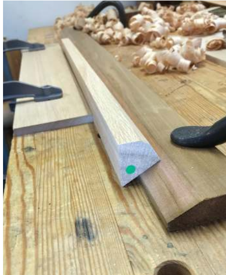
Boards placed either side of the leg for support while planing
