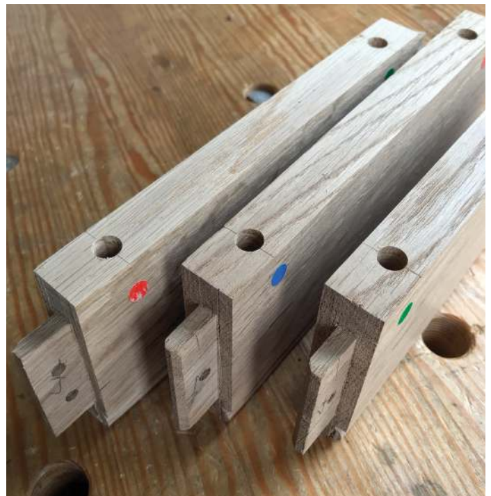
Aprons drilled for fox-wedged dowels before assembly
