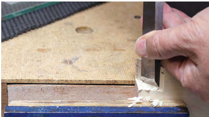
Pencil a line about 3mm away from the front edge and remove the waste up to the pencil line
