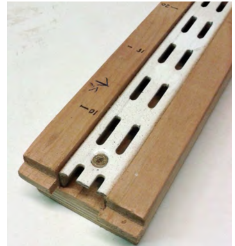
The matching tongue on the top of the upright
