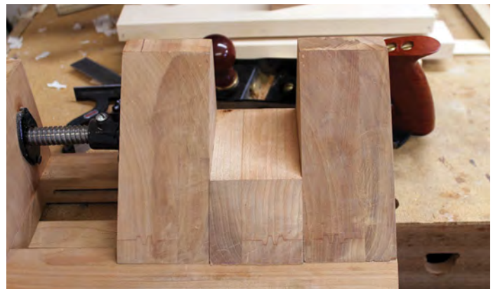
After sawing a block close to a mitre bevel, I held the block in the mitre jack and planed the block's face to a perfect mitre
