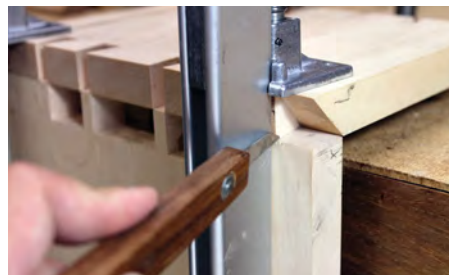
Transfer the outer tail line onto the pin's end grain, holding the knife tight to the tail face
