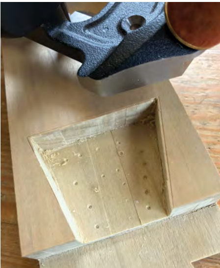
Go lightly with the grain to minimise the risk of tearout
