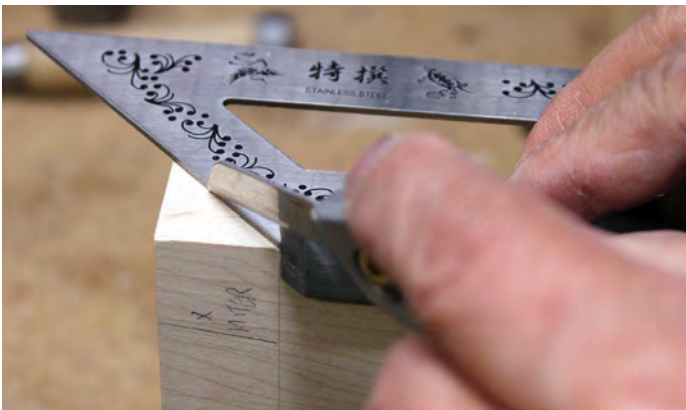
Scribe the mitre line on the edge in three strokes with progressive force
