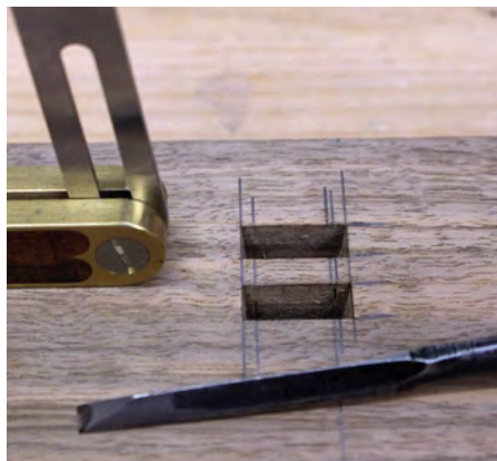
Angled mortise using a sliding bevel as a guide
