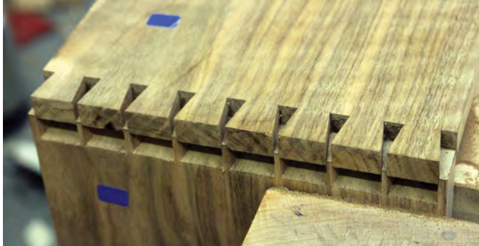
Testing the fit, a perfect result straight from the saw RIGHT: The sliding bevel setting used for the angled mortise was also used to make a simple jig for cutting the wedges on the tablesaw. A zero clearance sled is essential to do this safely
