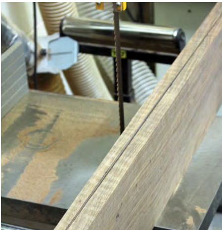
Carefully cutting the tapered sides on the bandsaw, from a single thick board
