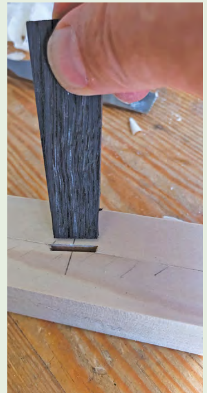
Cut a slot across the joint with a chisel to accommodate the locking pin
