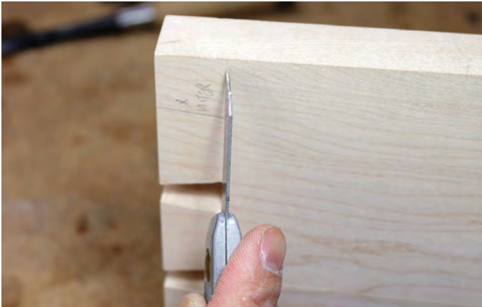
Register the knife tip in the shoulder line on the inside and near the edge
