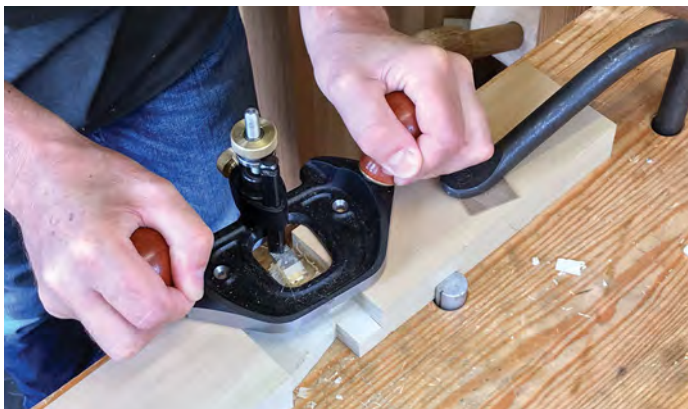
Level off the first pin with a router plane using the uncut components for support
