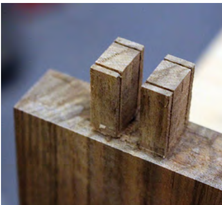
Tenons cut and waste cleaned back to the base line. Angled cuts have also been made for the wedges
