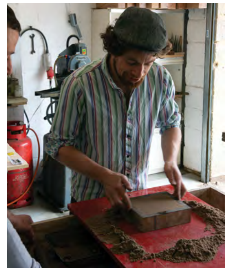
Ollie Sparks demonstrates metal casting
