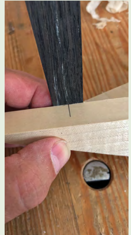
Pick a spot in the middle of the lap joint to locate a locking pin
