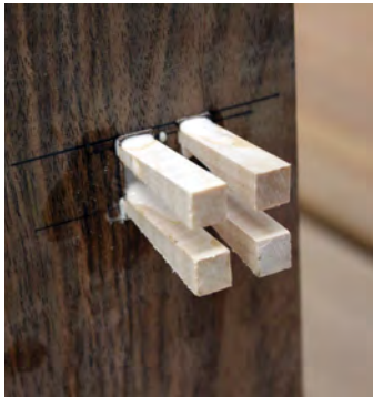
Identical wedges tapped in the same distance should give an even looking result
