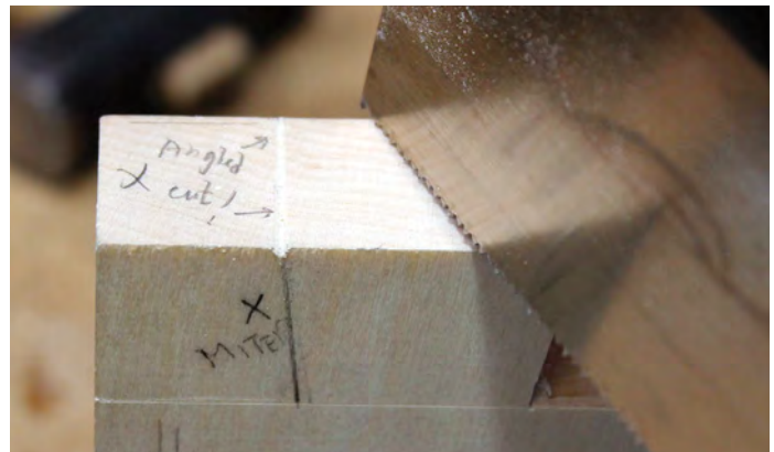
I labelled the waste to remind myself to not make the 45° cut right through the board
