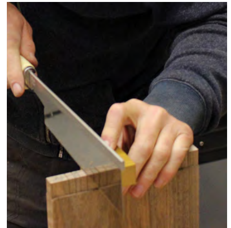
Cutting the tenons with my 90° magnetic guide
