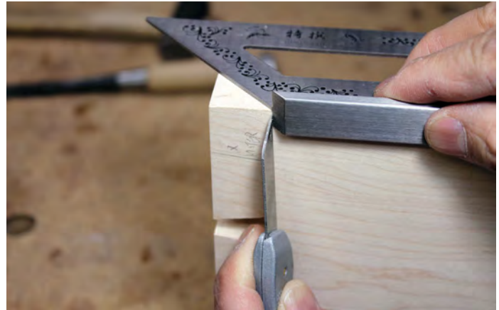
Butt the mitre square's base against the tip of the knife
