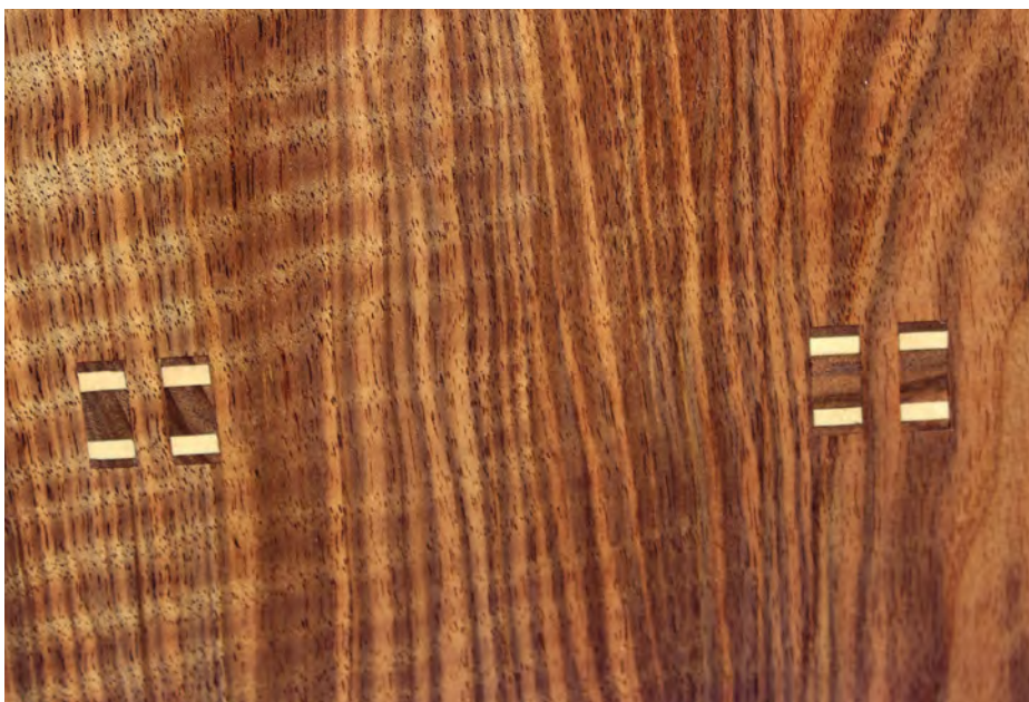
Wedged tenon detail
