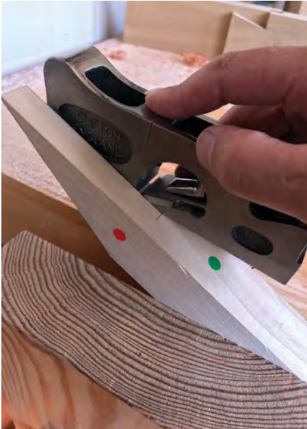
Trim the mating surfaces if required
