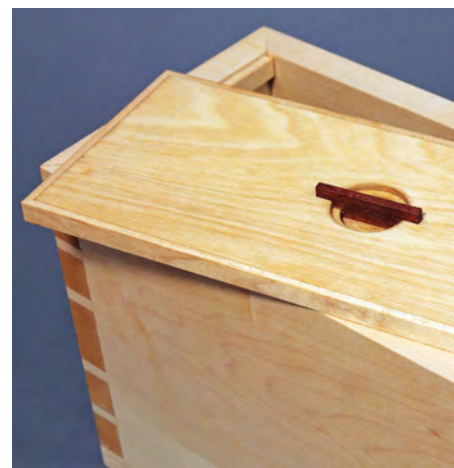
The lid's mitred corners line up nicely in harmony with the mitred shoulders
