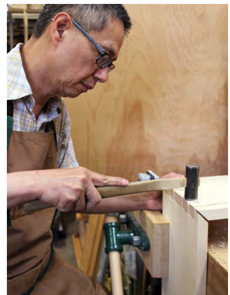
ABOVE: Trim off the excess as highlighted by the pencil mark left on the sides of the pins RIGHT: Use a hammer for dry-fitting, listening to the tap sound for resistance or seating
