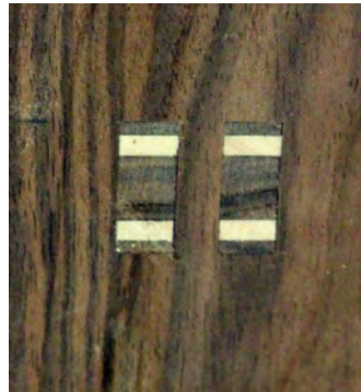
The result after cutting off and planing flush
