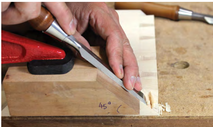
Clamp the mitre block at the shoulder line and pare with the chisel flat on the block. Take a thin cut each time if the waste is too much to remove in one paring
