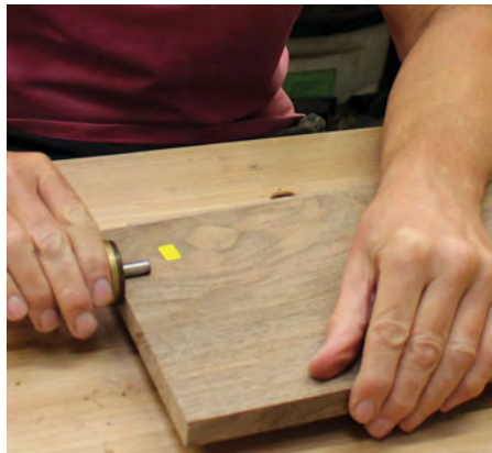
Marking out the base lines for the through tenons and dovetail pins. Although these boards will end up a different width, due to the tapering sides, I've cut them identically so that the base lines are a perfect match
