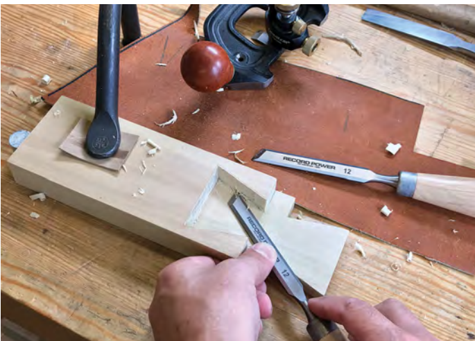
A pair of skew chisels are great for accessing those tight corners
