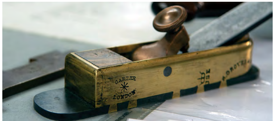
A mitre plane by Bill Carter, made from a brass saw back
