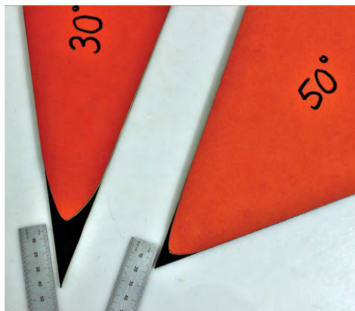
Blade bevels sharpened at 30° and 50°
