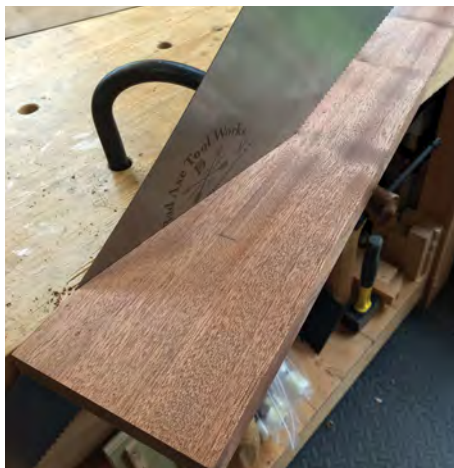
Split the board in two corner to corner
