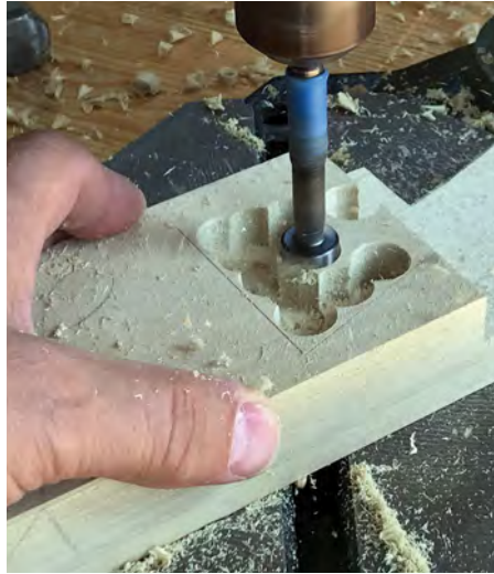
Remove as much waste as you can with a Forstner bit or similar
