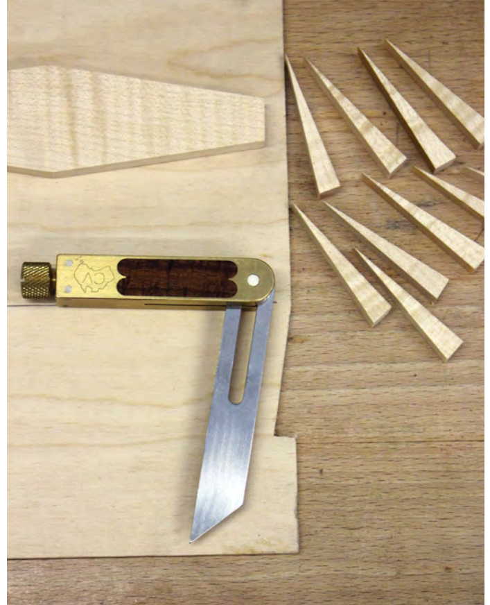
Testing the fit, a perfect result straight from the saw RIGHT: The sliding bevel setting used for the angled mortise was also used to make a simple jig for cutting the wedges on the tablesaw. A zero clearance sled is essential to do this safely
