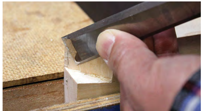
Register the chisel against the pared flat and trim off the last bit of waste in the final stroke
