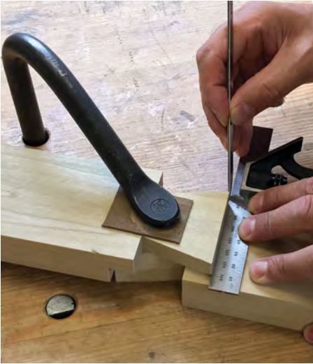
Use the first component to mark the shoulder on the second
