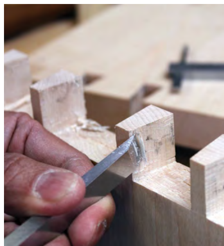
ABOVE: Trim off the excess as highlighted by the pencil mark left on the sides of the pins RIGHT: Use a hammer for dry-fitting, listening to the tap sound for resistance or seating
