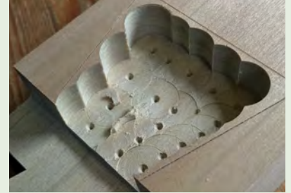
Leave enough material to accommodate the point of the Forstner bit
