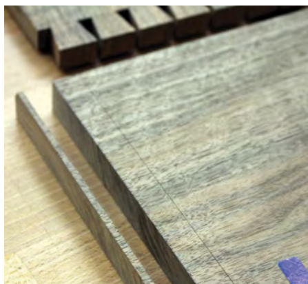
Before marking the pins on the top each end was reduced by 7.5mm to take account of the taper in the sides
