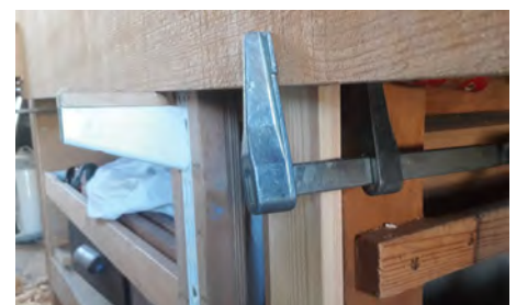
The extra upright to clamp the timber
