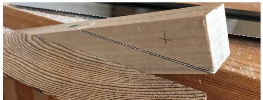
Angle the components in the vice for reference where you can
