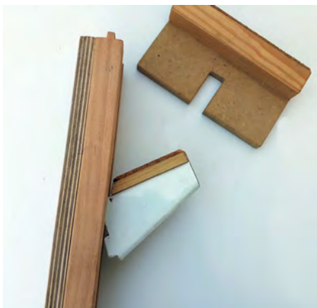
Remember to allow for the tilt required to fit the bracket
