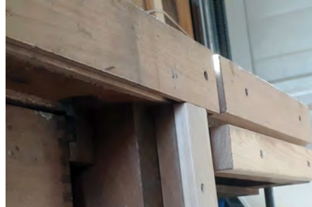
Groove the underside of the full-length bench cheek and add an extra piece or two to the end vice
