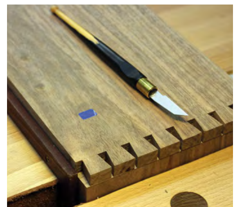
Marking the pins from the tails using my dovetail alignment board
