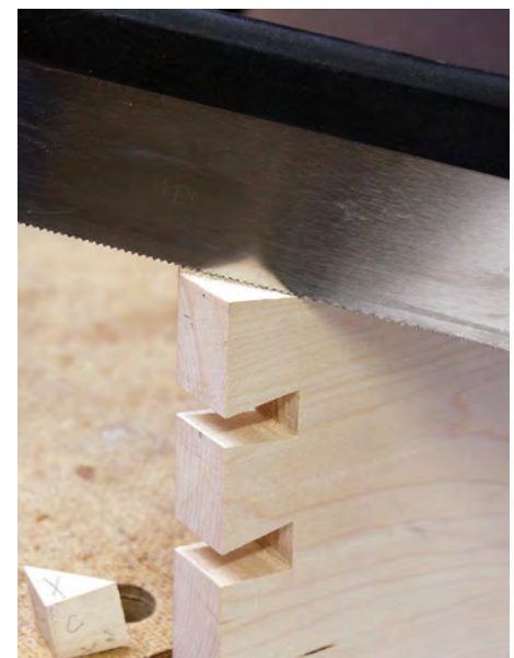
Saw on the waste side of the mitre line on the top edge until the waste falls away
