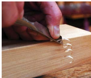
Chamfering bevel side down. With the bevel side down to the cut, the wedge tries to push the chisel up and out of the cut. It's easy then with slight hand pressure to keep it in the cut
