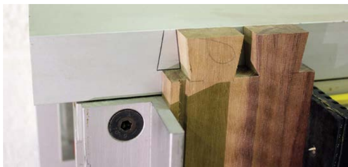
Aligning tailboard with cutter profile in the Marker Position
