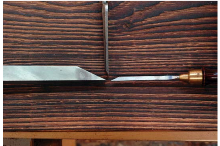
Firmer chisel (left) vs Blue Spruce bevel edge (centre) vs paring chisel (right)
