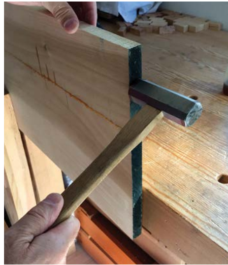
Secure the bottom board and tap the top one into position
