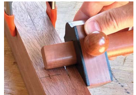
Clamp the boards back to back and set your gauge to half the thickness of the board
