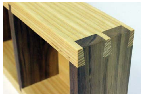
Completed through dovetail
