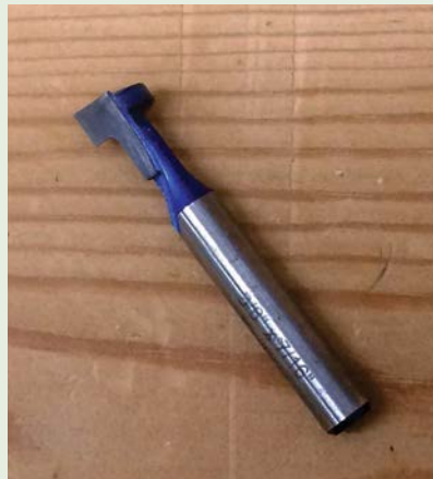
A typical keyhole cutter for use in a plunge router
