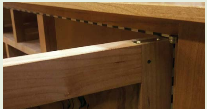
Knife hinge mounted on door and apron
