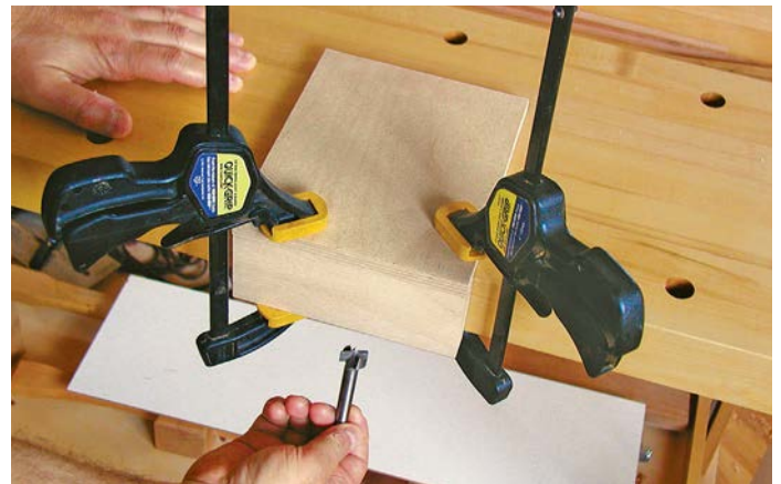
Locate the big dowel. Center the base over a dog hole. Use a ¾ in. Forstner bit to nick the underside of the base where you will drill
