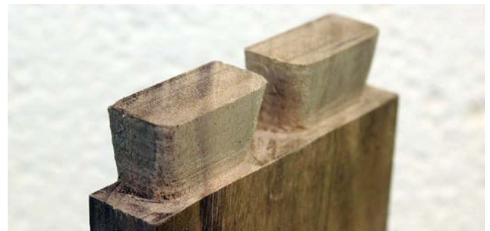
Finished tailboard after rounding over with a rasp
