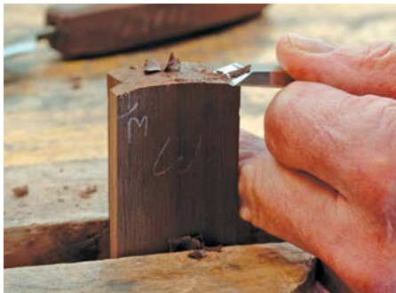
Paring long grain square plugs. Long grain plugs cannot be pared by carving up. This would result in tear-out. Pare across their edges but carefully so as not to nick the surrounding wood
