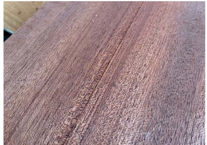
After cleaning up there's a faint glue line visible
