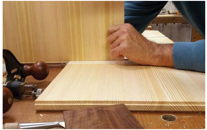
Testing the sliding dovetail
