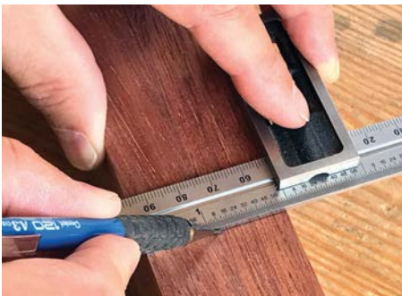
For convenience, position the square once and just mark both sides of the rule...
