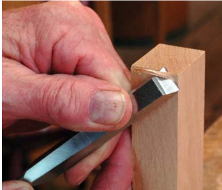
Paring off towards the supported fibres. Pare off towards the long supporting fibres or towards the end grain when paring off at the end of a board
