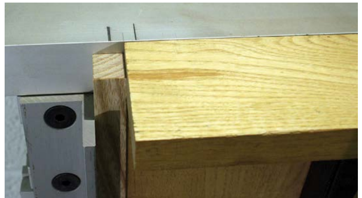
Alignment of measuring jig for cutting the half socket shoulders
