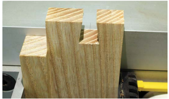
Set base of cutter profile flush with top surface of Rat body
