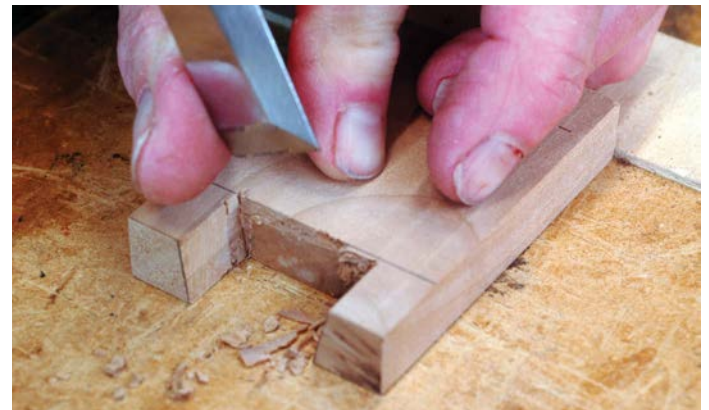
Chopping on the gauge line. After removing most of the waste the chisel can be placed right on the gauge line to finish up chopping at the gauge line
