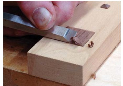
When shaping end grain, work towards the longer fibres to help support the cut
