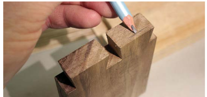
Transferring the difference to the tailboard with a pencil
