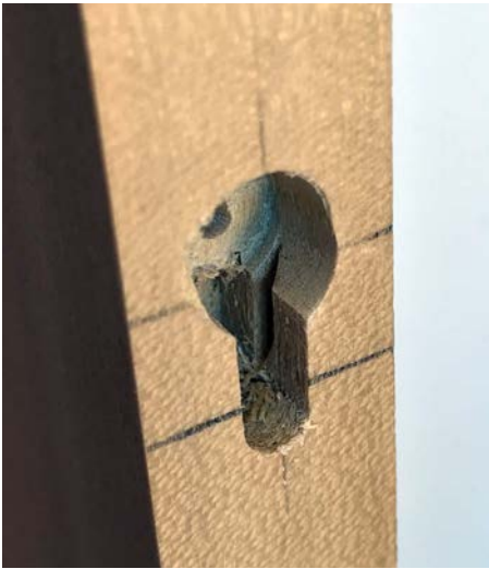
Notice where the screw head has gouged a path along the slot
