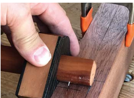
Both centre lines can be marked with a single setting from either side of the stack
