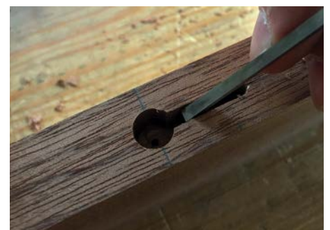
Use a thin chisel to clear the waste and create the slot
