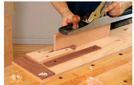
There's more. Once you've planed the face of the board, use the bird's-mouth attachment to plane the board's edge
