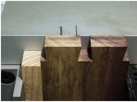
Aligning tailboard to cut pinboard waste
