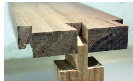
Final test pin with a good fit
