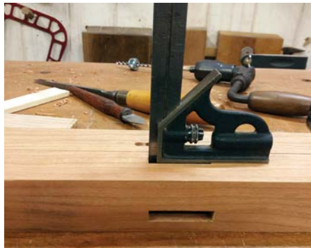
Checking the mortises with the combination square
