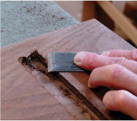
Cleaning the fibres out of a router cut
