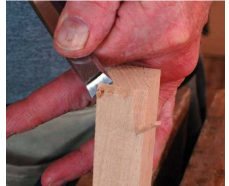
Paring off end grain. Paring off the end grain yields tear-out as the fibres being cut are unsupported
