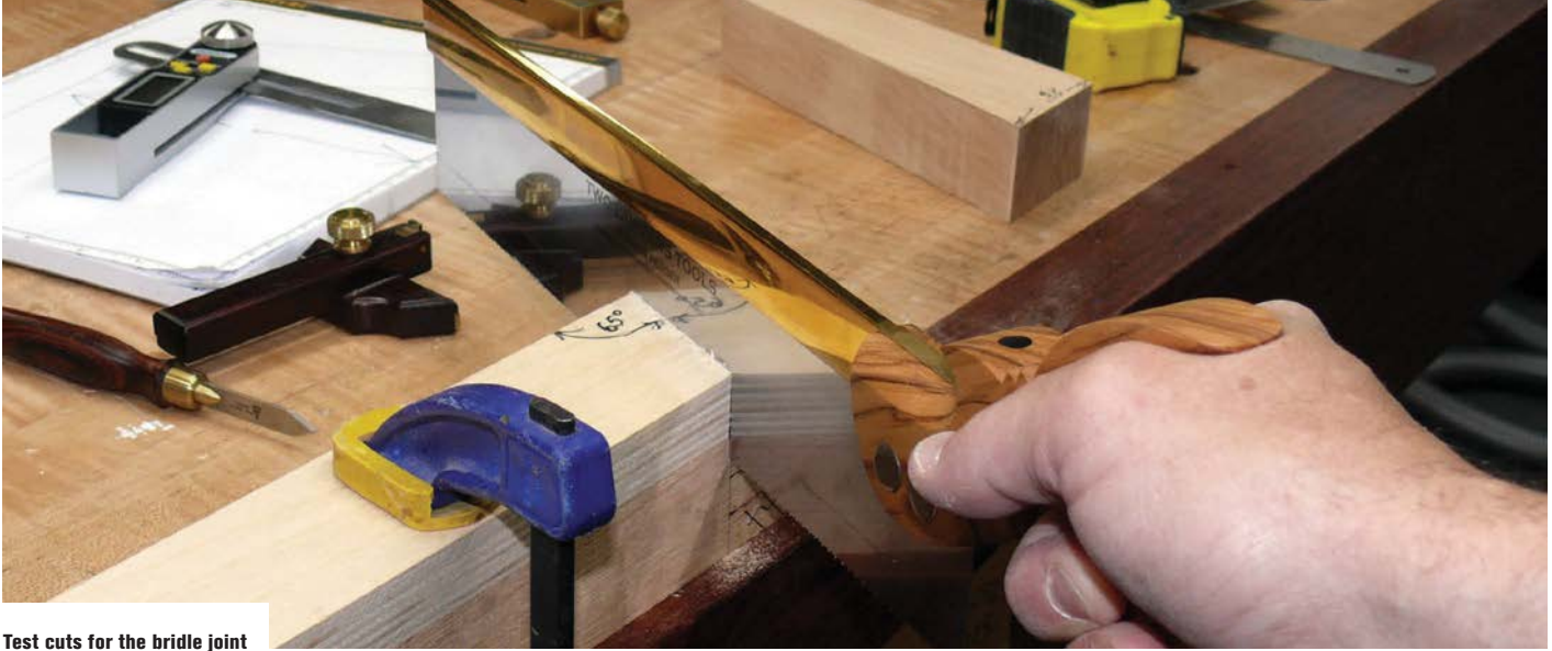
Test cuts for the bridle joint
