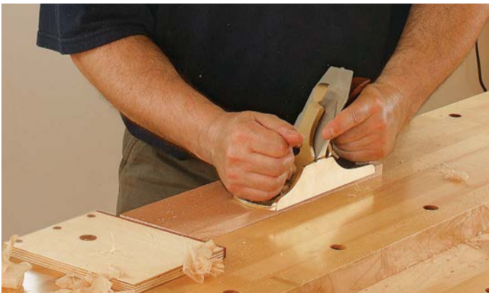
A simple stop is useful for face-planing boards
