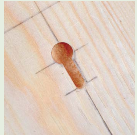
This cutter undercuts the slot so you must reverse back to the original point of entry
