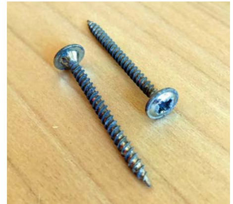
Screws with an integrated washer are a halfway house solution and work in soft timbers
