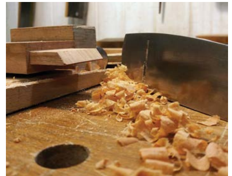
Making the mitre on the tenon using the small block plane
