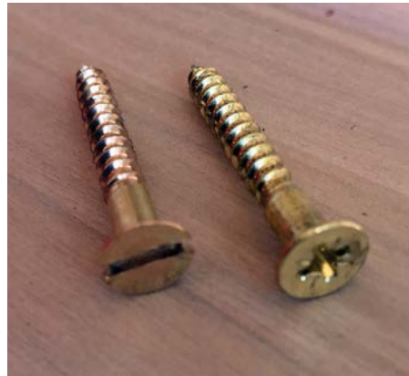
The thicker the shank above the thread the better
