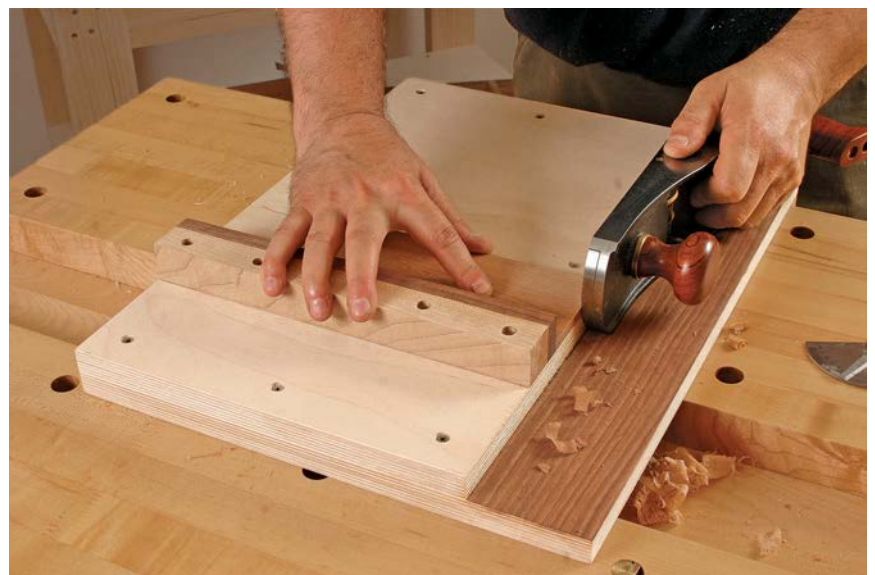
Square and true. Place the board against the fence with the end fractionally beyond the end of the fence. Slide the plane past it, taking thin shavings until the end of the board is clean and perfectly square
