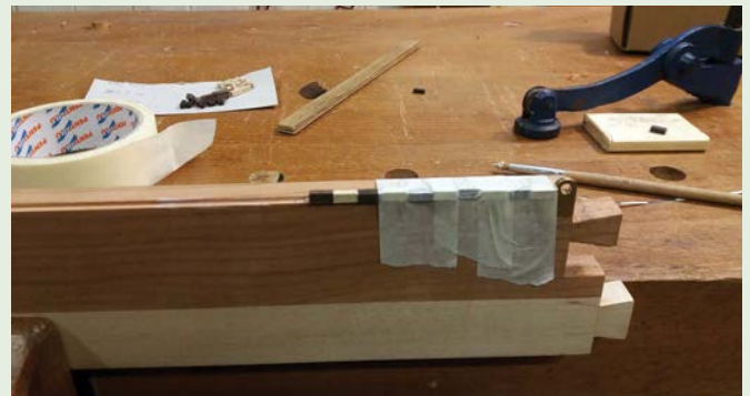
Gluing ebony and holly dots with the knife hinge fixed
