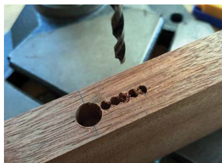
Create a slot with a series of holes along the centre line
