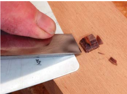
Paring end grain square plugs. I use an old credit card to protect the surface of the wood as I pare up and off towards the end grain of the plug
