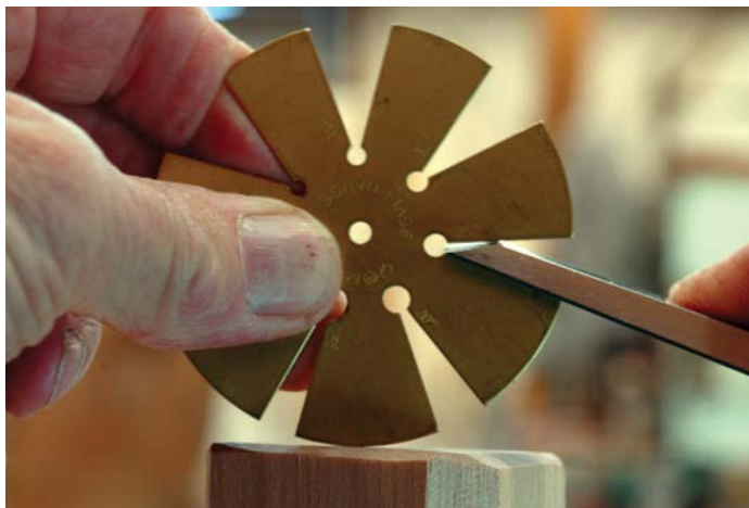
This angle gauge allows one to roughly see the angle of the bevel of a chisel
