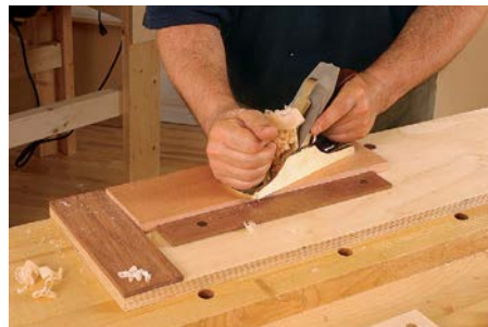
Side support. When you need to skew the plane or plane across the board, use the side stop to support the workpiece laterally
