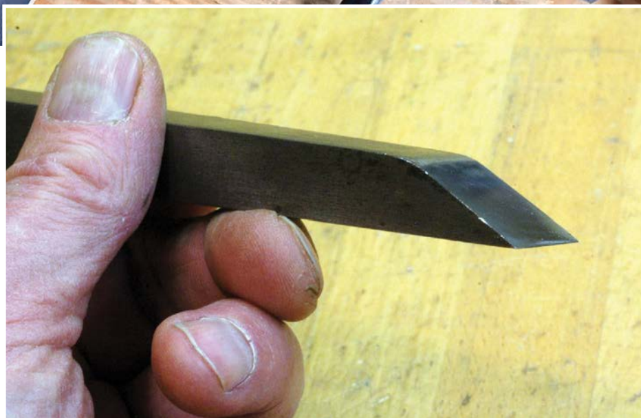
The wedge acts as a persuader in this ship carpenter's mortising chisel
