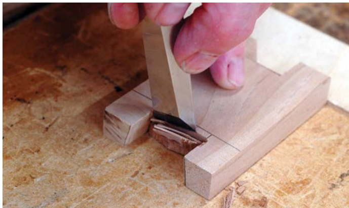
Chopping off from a gauge line. By starting well off the gauge line and close to the end of the wood, the wedge simply pushes away the waste
