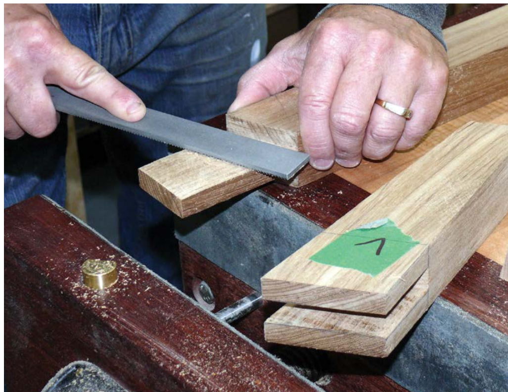
Final joint fitting
