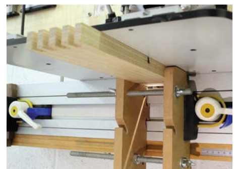
Ash board in mitre box for cutting the pins
