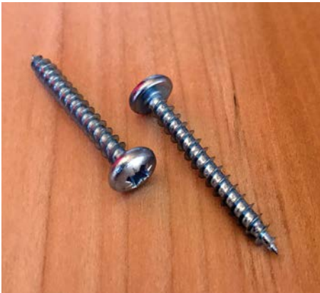
Pan head screws will require the use of the T-slot or keyhole cutter
