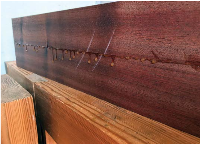
The squeeze-out indicates the pull from the screws is sufficient to pull the joint closed
