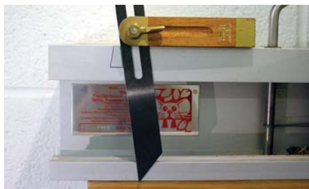
Setting sliding bevel to the dovetail angle
