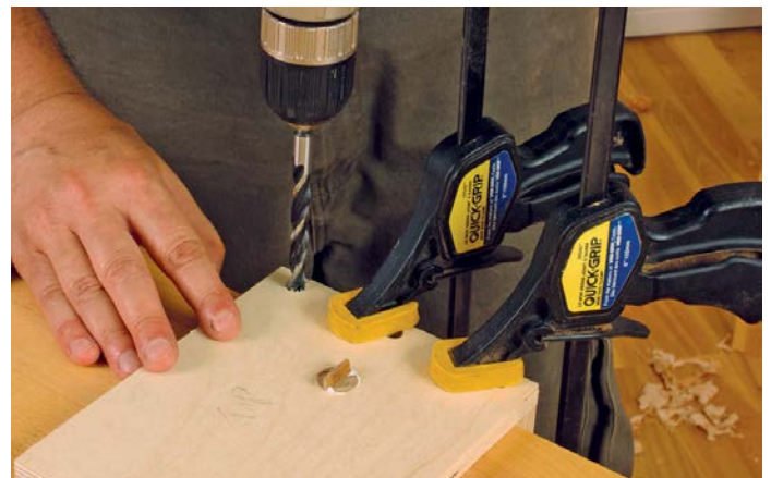
Attach the cleat. Insert the big dowel, ensure the base is square to the bench, then clamp on the cleat and extend the 3/8 in. dowel holes
