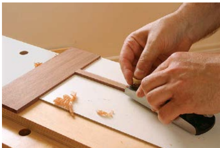
Thin stock, no problem. When planing stock less than 1/4 in. thick, add an auxiliary base of 1/8-in.-thick Masonite so the plane will clear the stop
