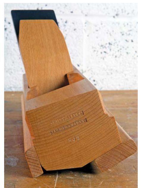
Viewed from the front you can see the two adjustable fences, the profiled sole and the skew of the iron
