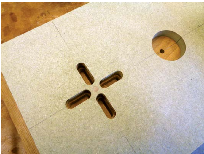
Finished cut showing the guidebush offset
