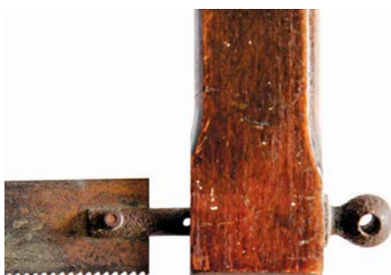
Detail of the round-headed shaft holding the blade that can be turned with a rod through the head
