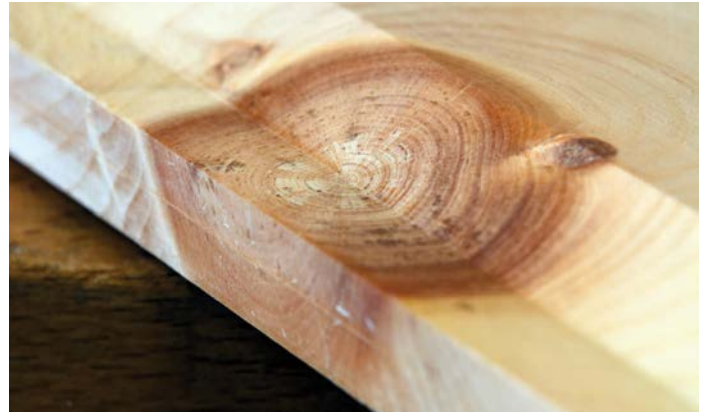
The torture test – the plane left a clean surface even on this large knot in position
