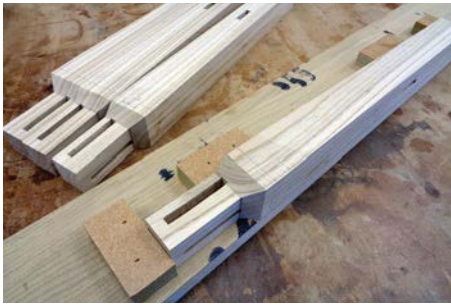
Using a parallel board to cut the tapers on the legs
