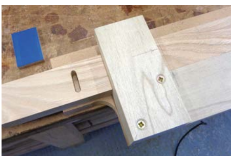
Domino spacing jig for attaching the stretcher rack to the rails
