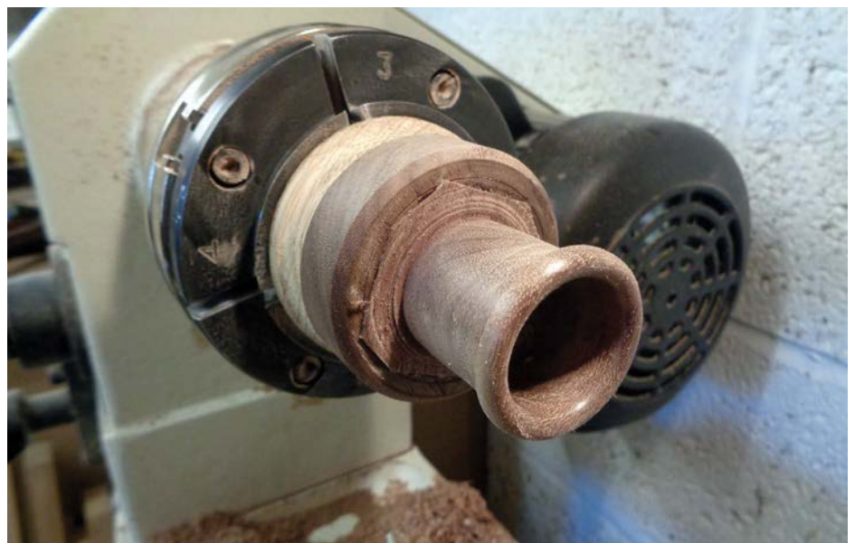
Leave enough material in the bottom of the hole to retain a good glue connection with the sacrificial blank
