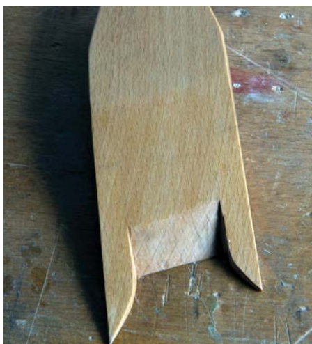
The wedge is well fitted and matches the skew of the iron
