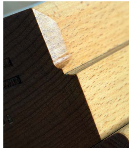
The body of the plane is decorated with perfectly executed chamfers
