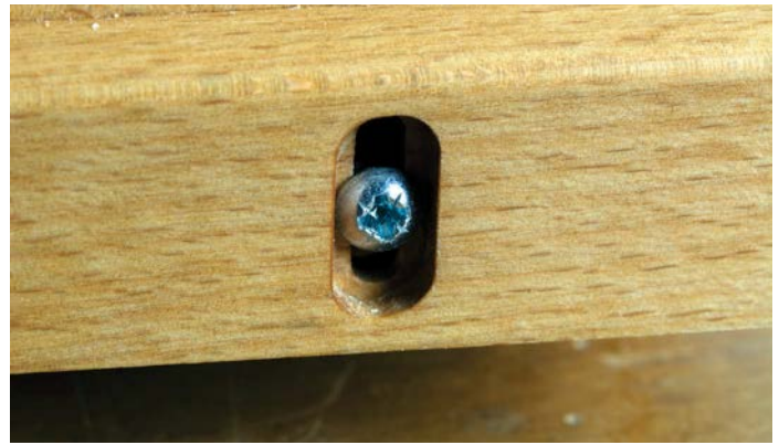
Steel screws hold the side fence in position
