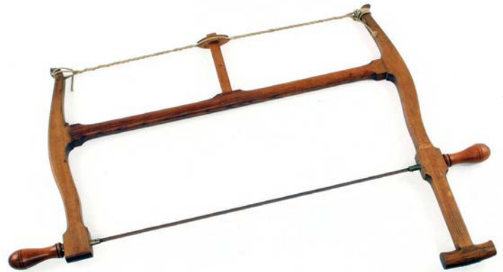
Like the woodcutter's saw, this bettye or chair-maker's saw has one cheek extended at its lower end to form a handle, but like the classic bow saw there are two boxwood handles in the axis of the blade that enable it to be turned. This kind of saw is used for cutting all manner of curved work from felloes in the wheelwright's shop to chair arms at the furniture maker's. The maker is unknown. There are also metal-framed versions of the bettye saw with tensioning device on the blade's axis not dissimilar to a metallic hacksaw
