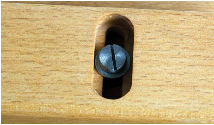
Steel bolts and washers hold the bottom fence in use
