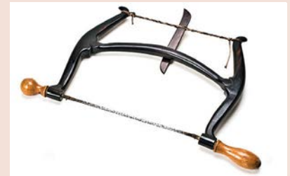
A late 19th- or early 20th-century bow saw from the late David Russell's collection, in rosewood with beechwood handles and a 12 1/2 in blade with 8 teeth per inch. The rounded-end design of the stretcher hints at the fulcral nature of the joints where it is loosely mortised into the cheeks. The maker is unknown
