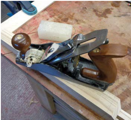
Removing the saw marks with a finely set No. 4
