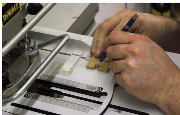
Marking out the cutter profile template onto the guiderail
