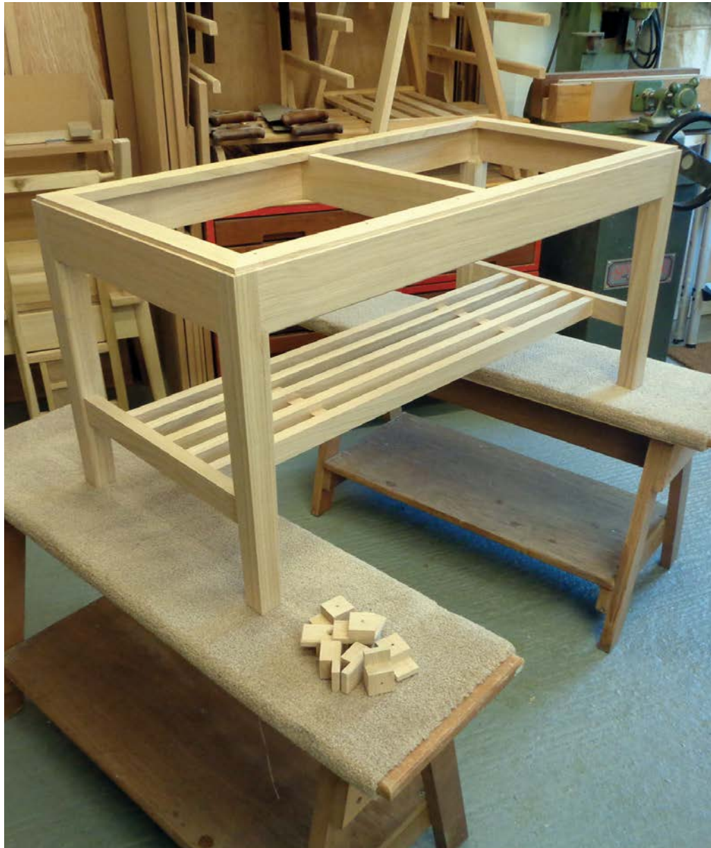
Assembled base with parallel centre rib and button rail
