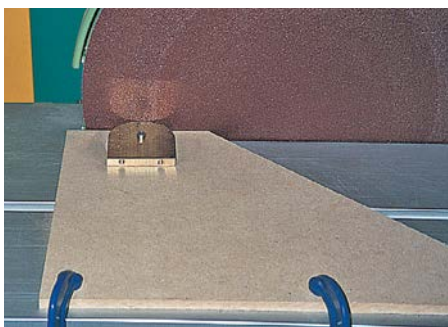
Shaping a half-round profile with a sliding jig mounted onto a disc sander
