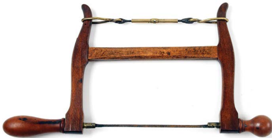
On this beechwood bow saw with boxwood handles the 6in web is held taut with a turn-buckle and stout brass wire. The stretcher is stop-chamfered. The maker is unknown
