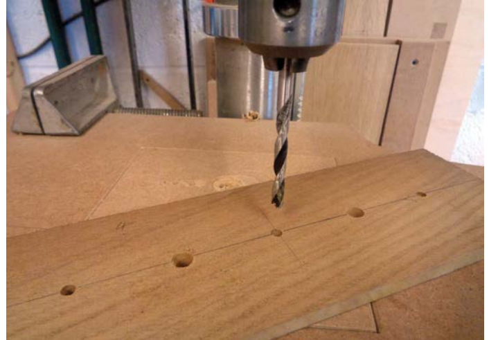
Boring the centre holes on the drill press
