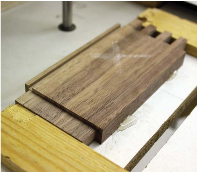
Short workpiece holding using horizontal table and fences
