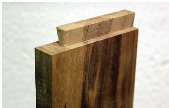
Completed sliding dovetail tenon
