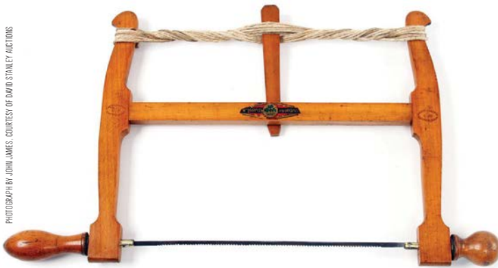
As the cheeks are brought closer together by twisting the twine on this classic English beechwood bow saw, the 12in blade (or web) is pulled tighter and held with a tongue, or in Sheffield terminology, with a 'clack'. The tightening process is done by leverage of the first kind, the slightly loose mortises on the cheeks receive the tenon fulcra at the ends of the stretcher. Both the colourful label on the stretcher and the maker's stamp on one of the cheeks show the shamrock trademark of William Marples & Sons of Sheffield first introduced in 1875
