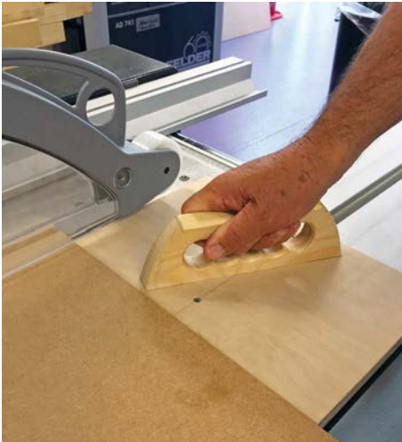
This shop made push jig rides in the T slot of the sliding carriage and is used to support smaller workpieces on the cross cut table
