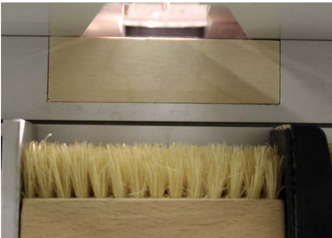
Blocked dust chute cavity using the ply block
