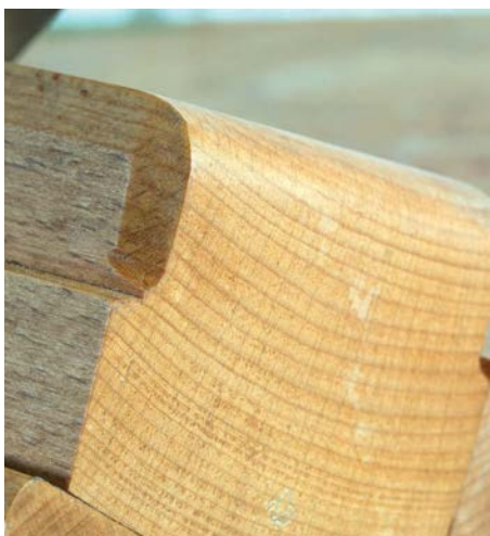
The rear chamfer makes for a comfortable grip in use
