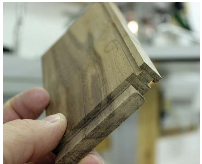
Both base grooves cut in the walnut divider
