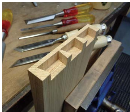
A good pair of skew chisels make light work of cleaning out the corners of pin sockets
