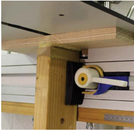
The brush is held in the camclamp to keep the workpiece pushed up against the underside of the base plate
