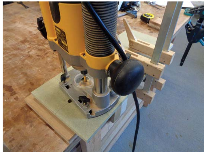
Routing the pattern with the Dewalt DW621 which has excellent extraction through the plunging column
