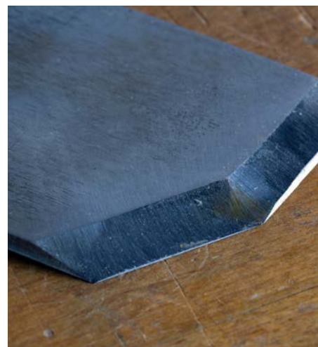
The hollow ground iron cuts two faces simultaneously
