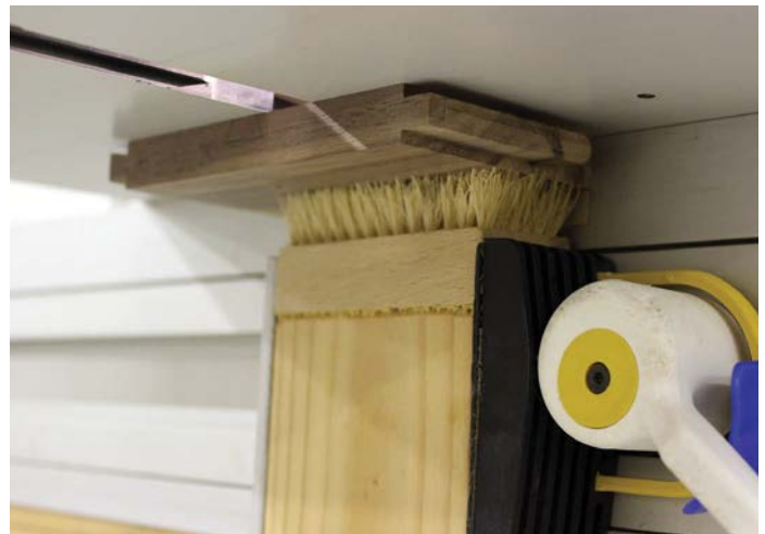
Brush support for workpiece while cutting the base grooves
