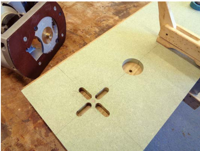
Lining up the jig on the centre line through the peep hole
