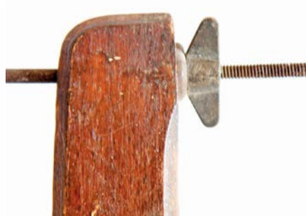
The wing nut on the threaded end of the tensioning rod provides simple and effective adjustment
