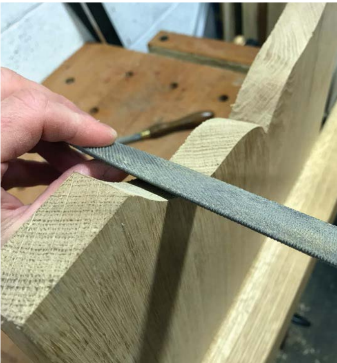
Shaping the concave portion of an ogee with the curved face of a cabinetmaker's rasp
