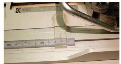
Pulling the router forward to 21.5mm on the rule
