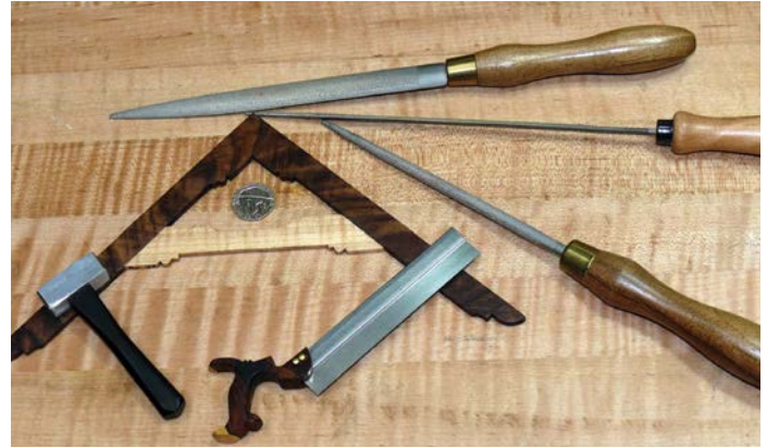
Small rasps are ideal for exceptionally fine work for miniatures or small details
