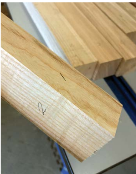
Use a number system that's clear and mark each face of the square blank
