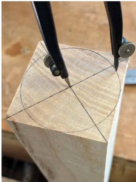
Draw or scribe a circle the full width of the blank
