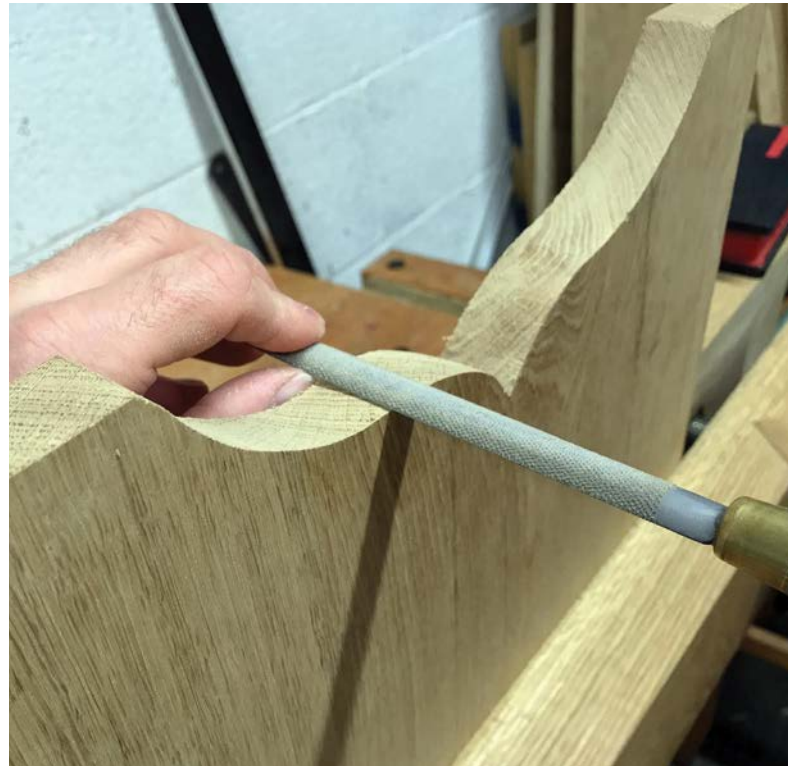
Shaping the convex portion of an ogee curve with the flat face of a cabinetmaker's rasp
