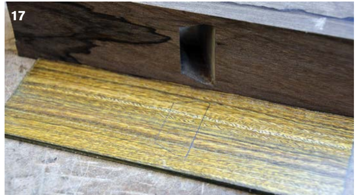
17 Place the plane on the sole and mark through the hole to show you where you need to cut the slot for the blade.
