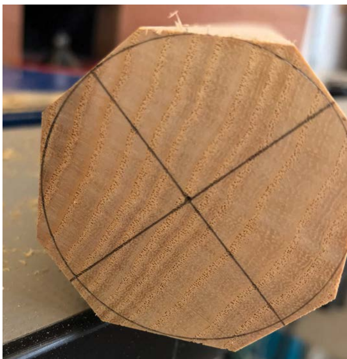
Leave a millimetre or less to remove on the last pass
