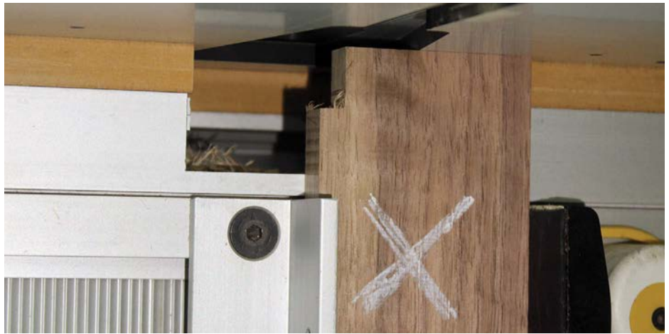
The walnut board with the first shoulder removed
