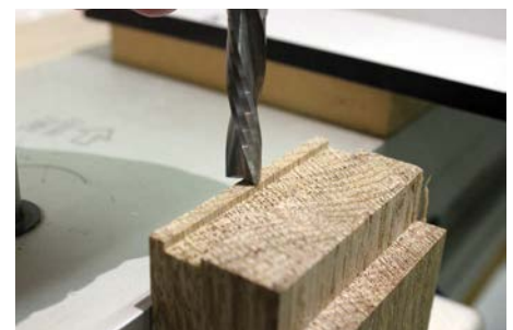
Router cutter removed and placed next to the rear wall of the slot to demonstrate the B/F alignment
