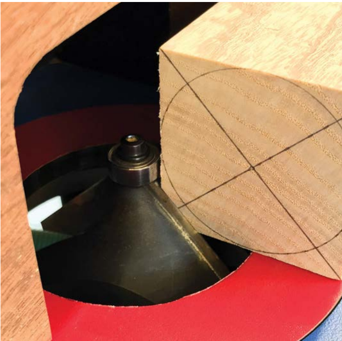
The first cut is most certainly not the deepest. A little bit shy of the edge of the circle is quite sufficient
