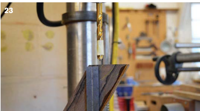
23 Select the drill bits you need and put a bit of tape on them as a depth gauge while drilling. Drill the 10 first, then 6.5, then 5. I would drill these holes using a pillar drill preferably. This could be done with a cordless drill but it needs to be quite accurate to avoid drilling through in the wrong place.
