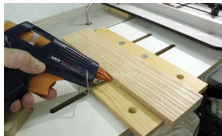
Hot melt glue secures the workpiece
