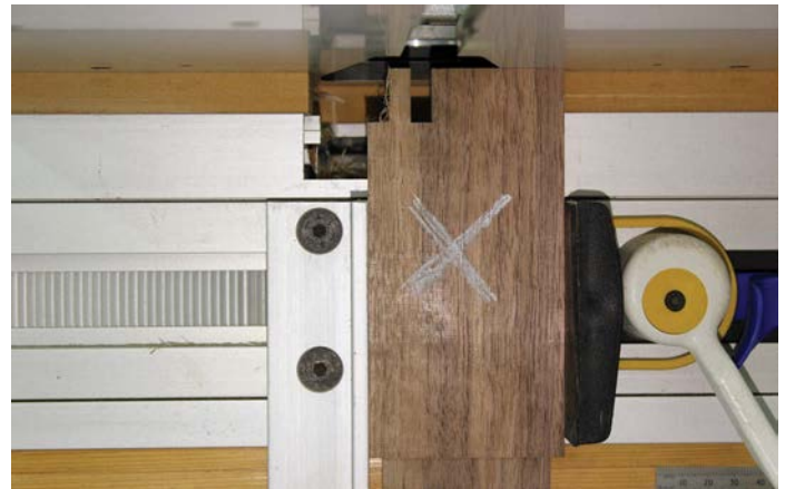
The walnut board with the first inner slot removed
