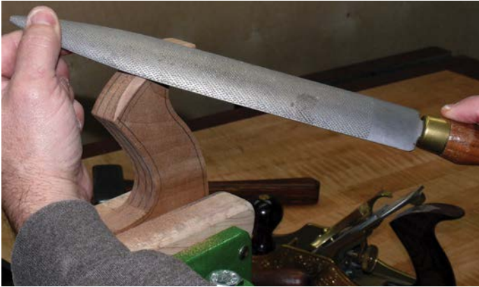
The cabinetmaker's rasp is the most useful rasp for many types of work
