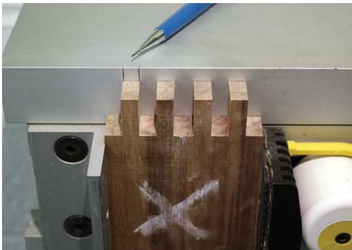
The final walnut board now in marker position to be used as a template
