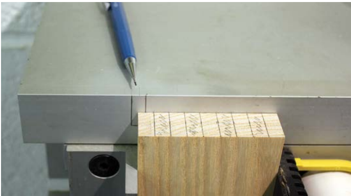
Ash template location to remove the first part of the 8.5mm shoulder
