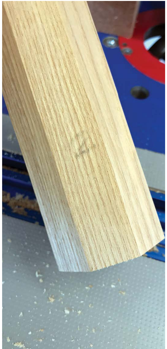
A zero cut should just remove the pencil marks and nothing else
