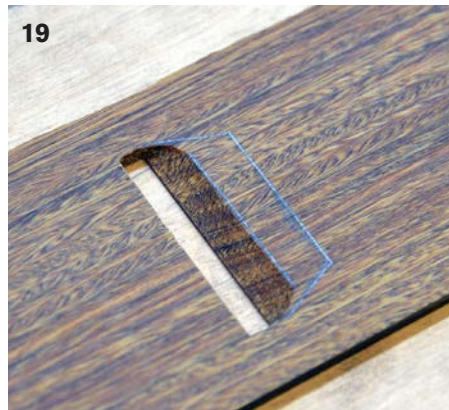
19 Chisel a slope on the inside of the sole. Again, this is to prevent the shavings from getting stuck. Clean the sole with acetone. This will help the glue stick to the oily wood.
