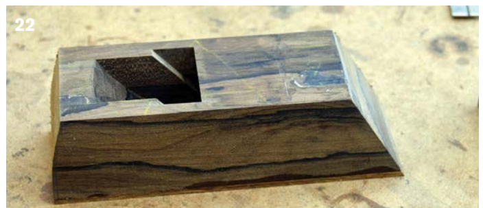
22 After you take the clamps off you should clean up the mouth in the sole. This can be done with a file and a bit of sanding. Then mark the 30° angle at the back of the plane and cut off the excess bit of wood. Then mark out exactly where you need to drill for the adjustment screw.
