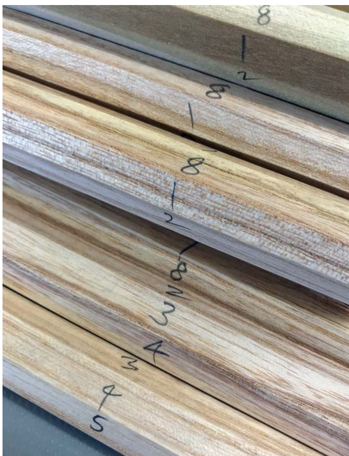
Number all eight sides before thicknessing
