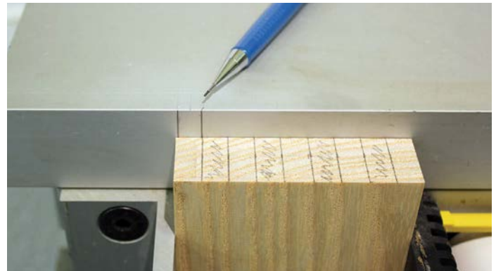
Ash template location to remove the second part of the 8.5mm shoulder
