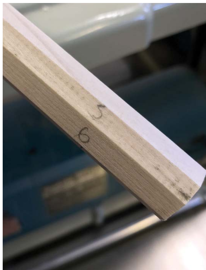
You're now at the halfway point and position No. 5. Time to set the thicknesser to the final dimension
