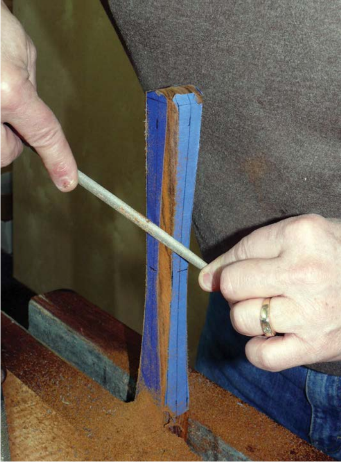
A fine thin rasp is perfect for refining the facets in this hammer handle
