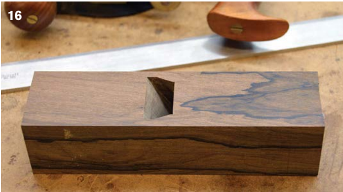
16 If you haven't done so already, cut the lignum for your sole. Cut the plane and the sole to the exact length. Also plane the sole to the exact width, this is a very important step to help with gluing the sole on. Plane the underside of the plane.
