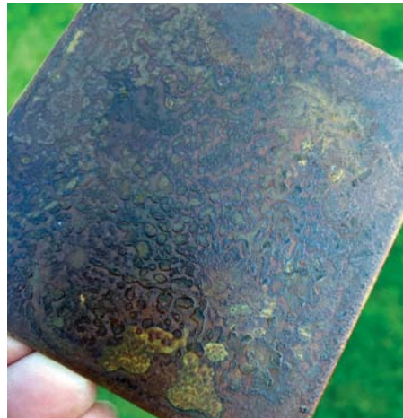
When sprayed onto a piece of mild steel plate the Japanese Brown patinating fluid was quite striking
