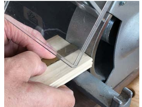
Grind a straight and square edge to the end of the blade
