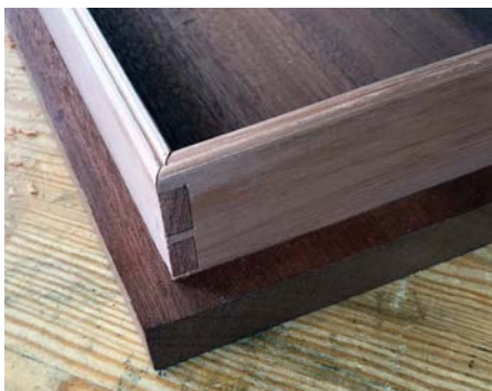
Glue the gallery together in the trench before finishing
