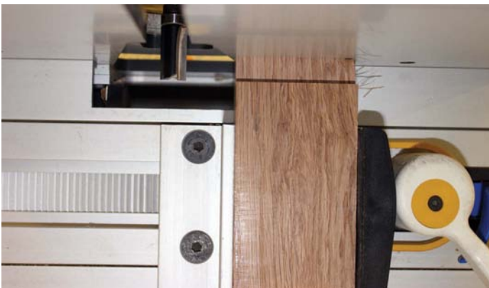
After climb cutting on the Rat
