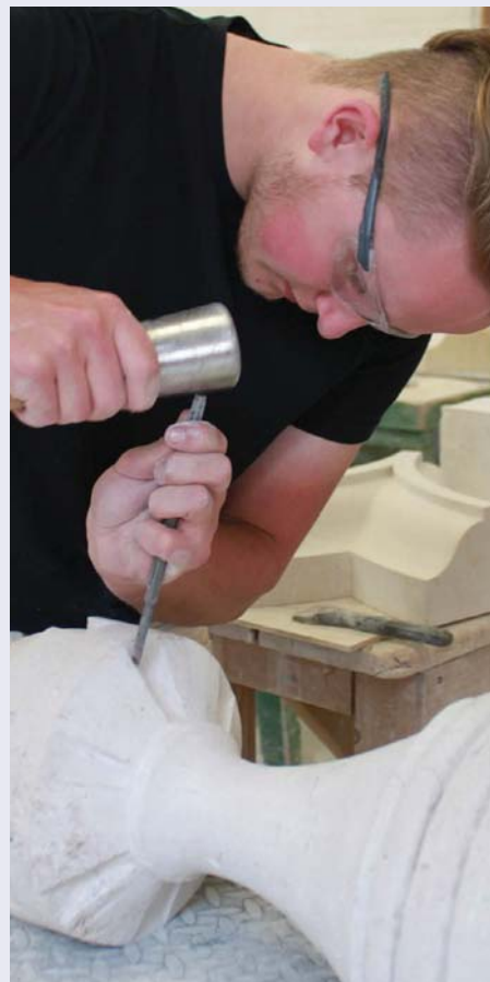
A masonry apprentice carves a stone finial
