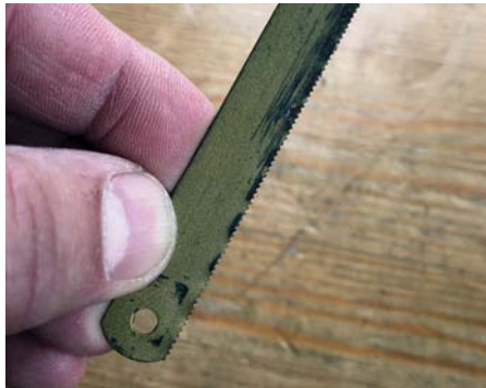
An old hacksaw blade is perfect scratch tool material
