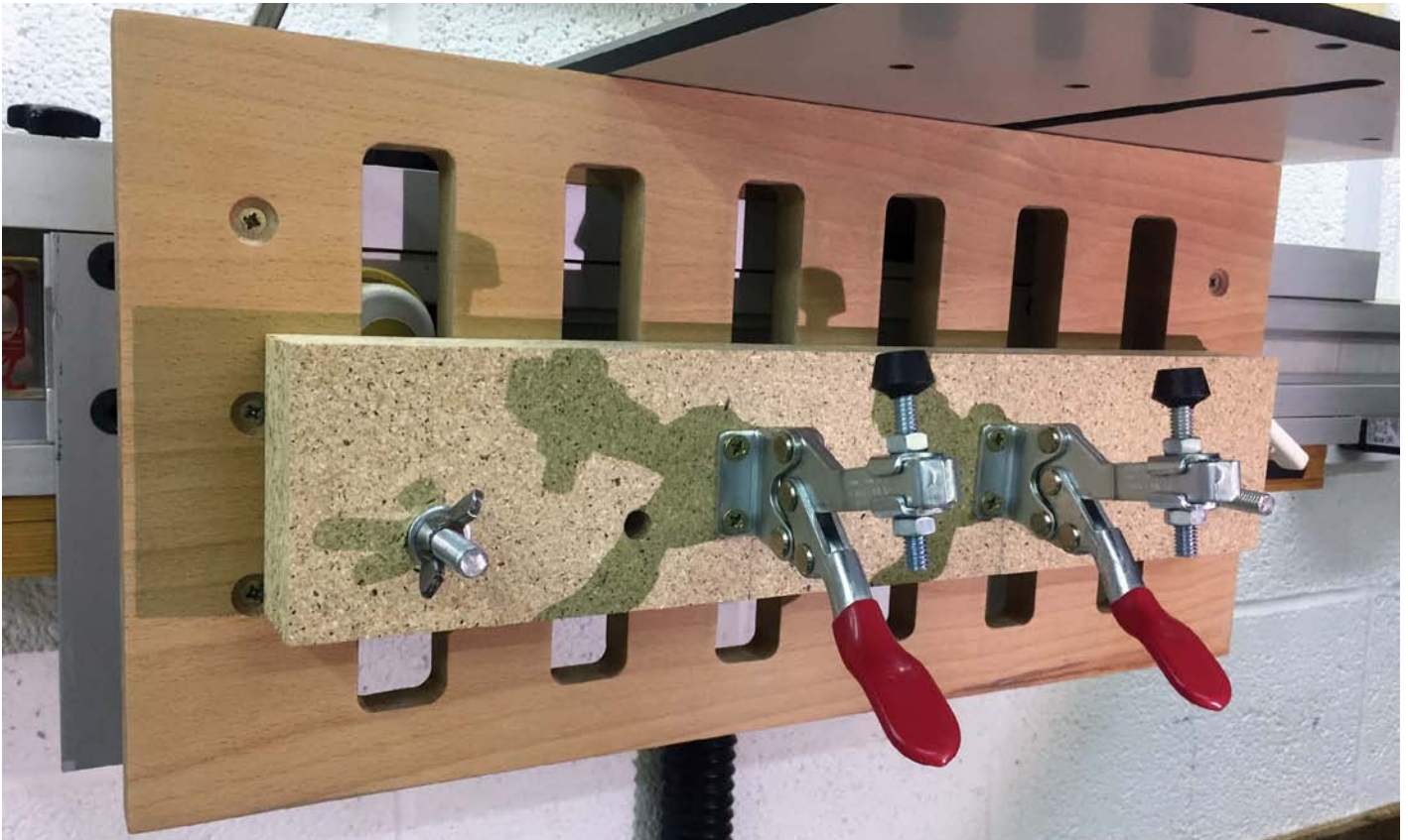
A homemade vertical table with adjustable support and clamps
