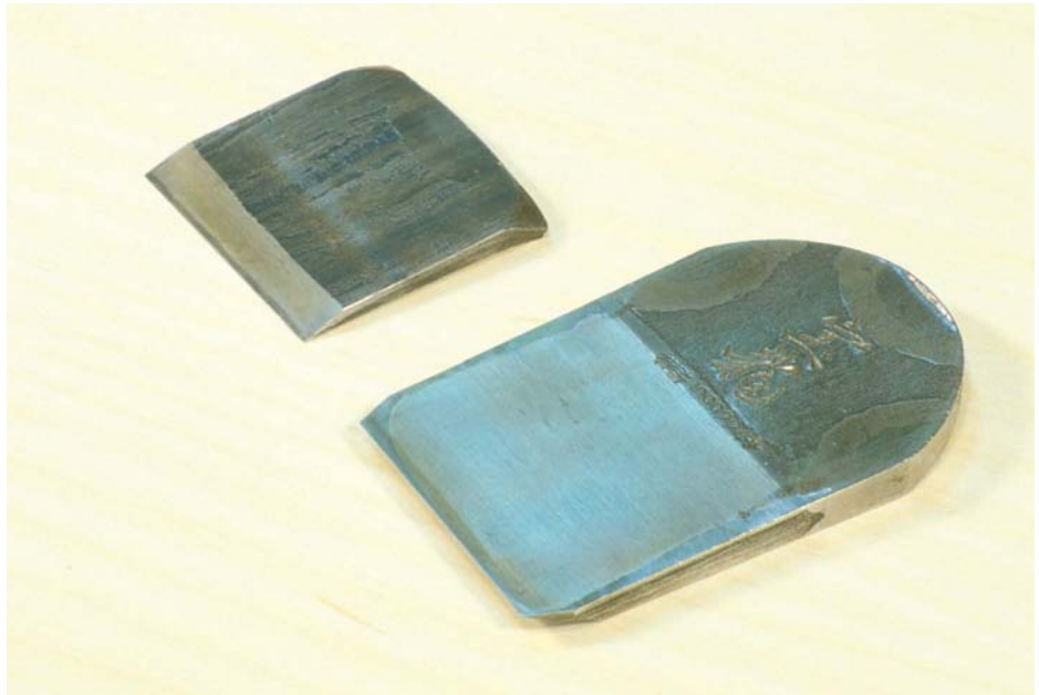
FINE JAPANESE BLADE AND CHIPBREAKER BY BLACKSMITH MIYAMOTO MASAO
