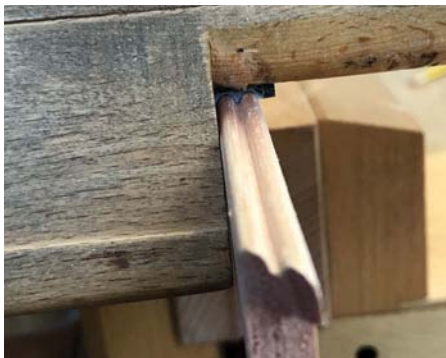
Angle the scratch tool towards the direction of the pass
