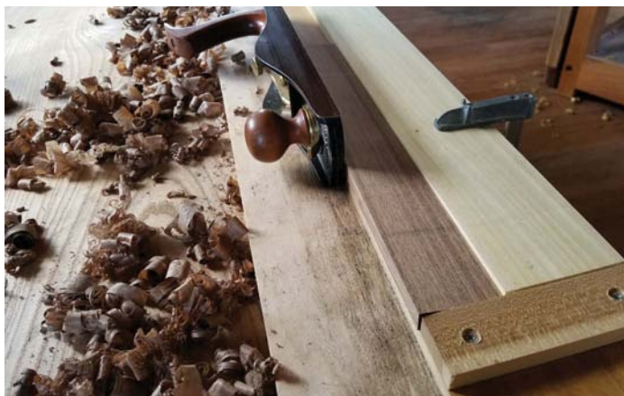
Dimension the sticks with a long grain shooting board
