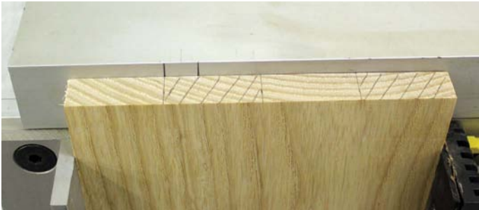
A marker position template showing that cutting here will remove the left-hand side of the hatched waste portion
