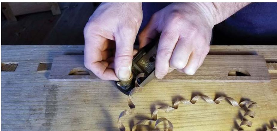
Remove the bulk of the waste with a block plane before flushing off with a jointer
