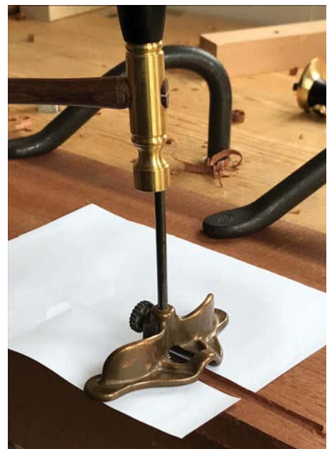
Make micro adjustments using a piece of paper as a spacer
