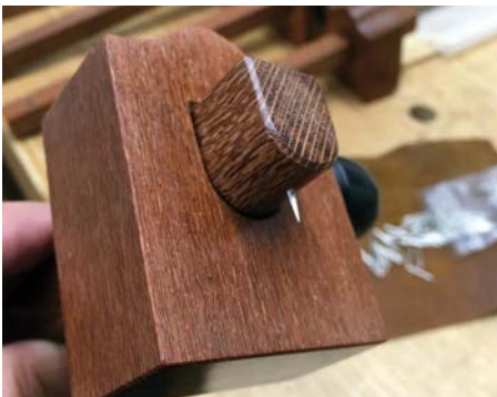
Use a pin-style marking gauge to establish the groove between the beads
