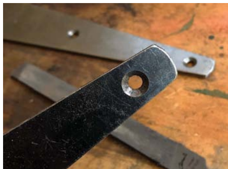
Remove any burrs around holes and countersinks
