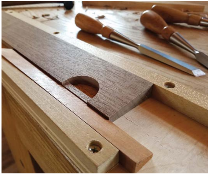
Create a ramp to guide your chisel to cut an even slope
