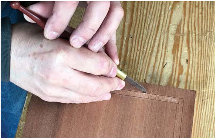
Two hands are better than one at guiding your knife in a straight line
