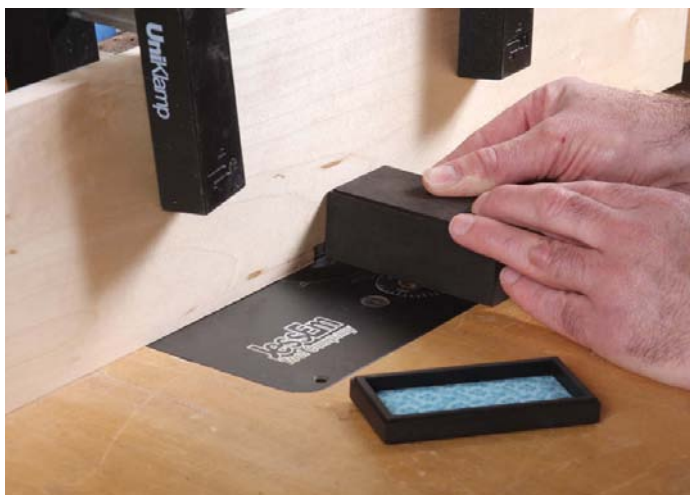
1 & 2. Rout a rabbet into the outside edge of the box and the lid
