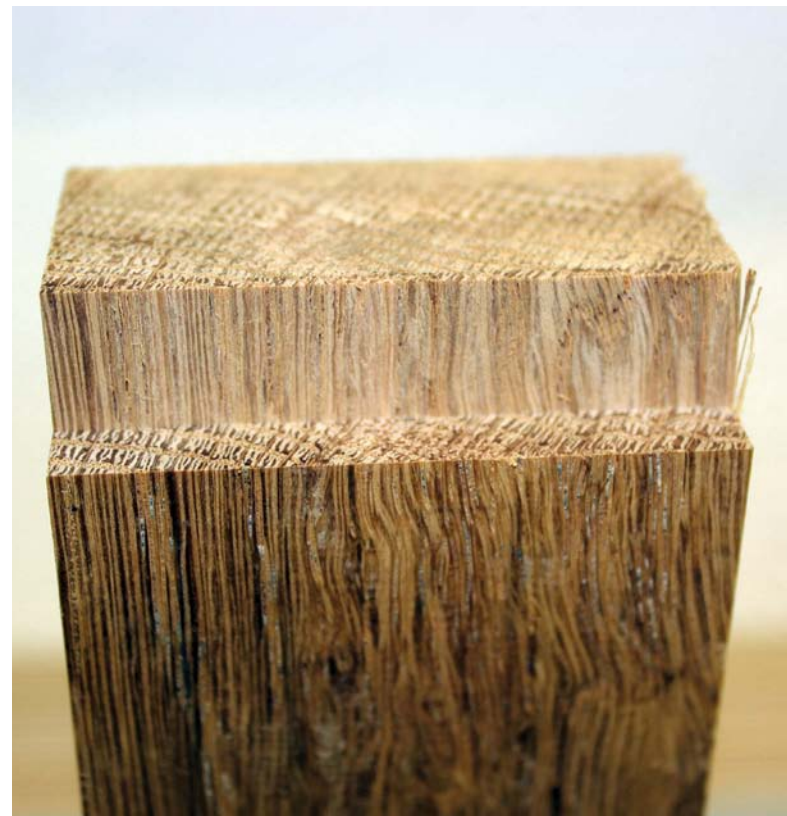
The clean shoulder cut by climb cutting
