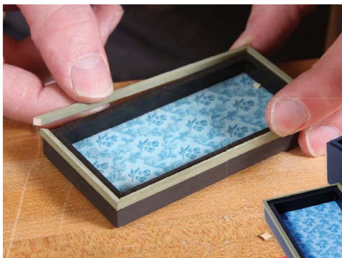
5. Fit the last strip into place
