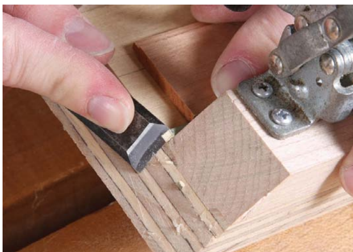
3. Cut strips of maple for the lid rabbet and miter the ends on a tiny miter shooting board
