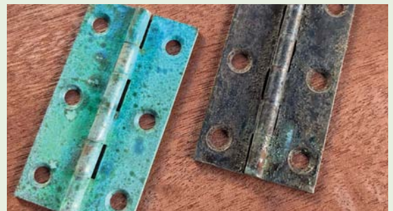
Build up layers of patina with more than one fluid for different effects
