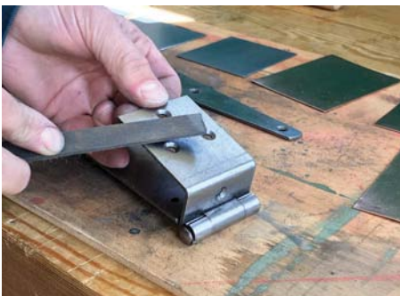
Soften any sharp edges with a file and finer abrasive for an aged appearance
