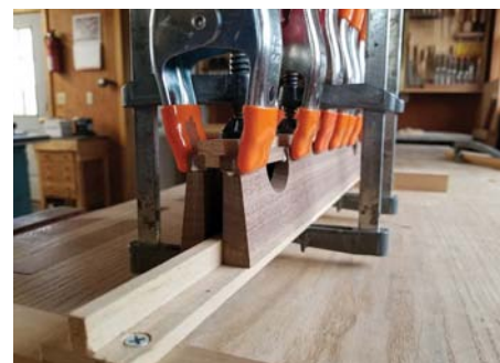
Two T section blocks are used to clamp the bridge section in place
