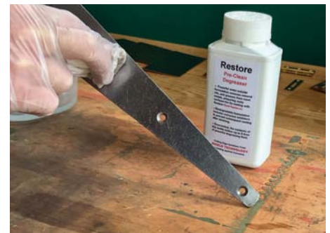
Use a degreaser to clean the items before patinating and then only handle them while wearing gloves
