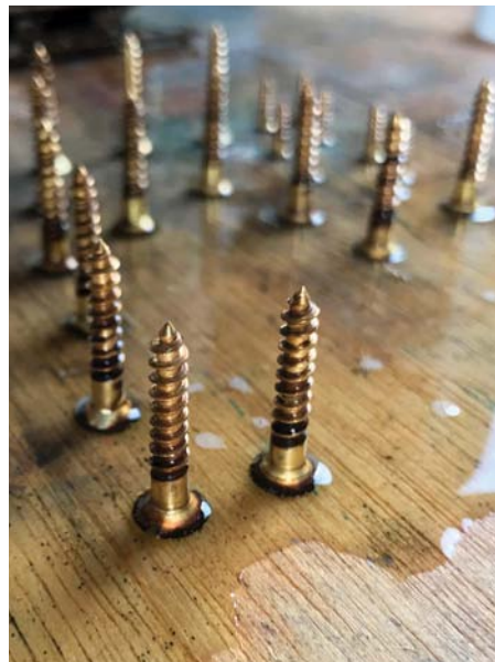
A shallow bath is perfect for colouring the heads of screws
