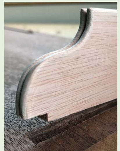
Angle the scratch tool towards the direction of the pass
