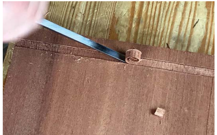
Rock an upturned chisel up and down on its bevel to find the optimum cutting angle
