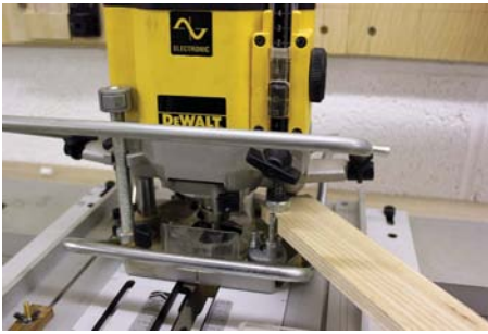
Depthing the cut to the thickness of the workpiece
