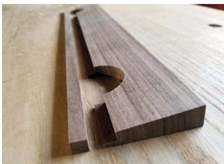
Prepare the bridge section slightly larger than the rebate
