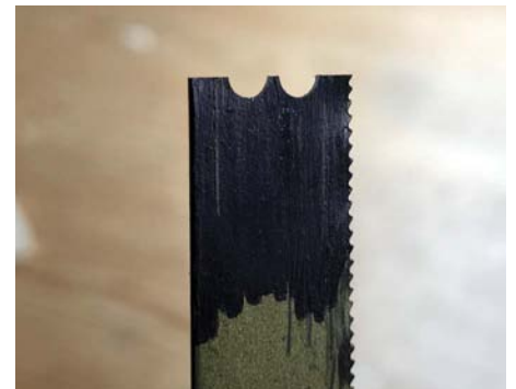
Leave sufficient material between the bead hollows for a more robust tool and to allow for a couple of sharpenings before the tool needs replacing
