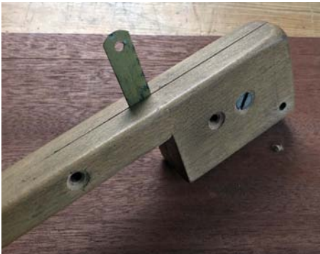
A homemade scratch stock might not be pretty but it will function every bit as well as a shop-bought one
