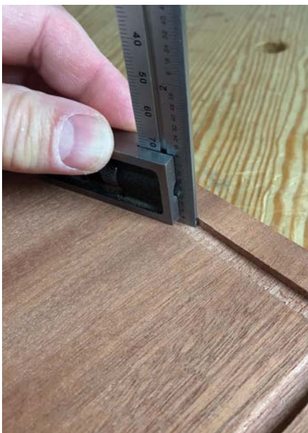
A small multi square will help you establish a consistent depth to your trench
