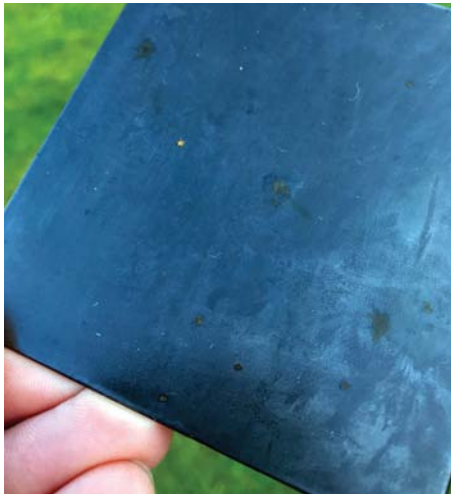
Light rust spots can form on ferrous metals after patination
