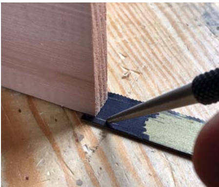
Transfer the thickness of the components onto the blade
