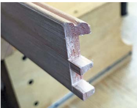
Leave a generous amount of material for the mitred pin to accommodate the depth of the moulding
