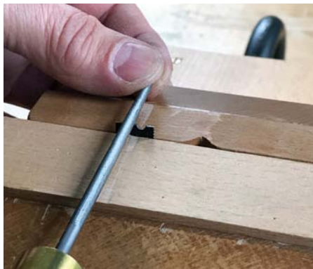
Use a tapered round file to create the head hollows
