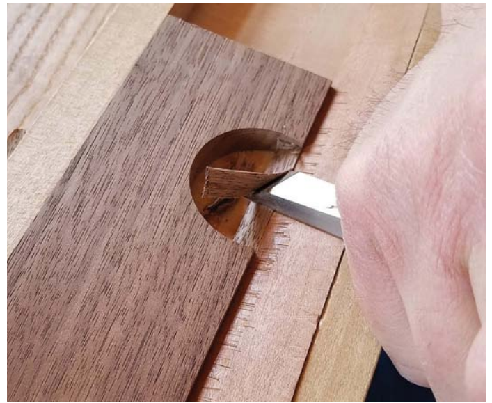
Pare away the inside face of the bridge
