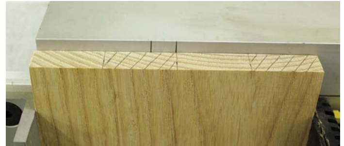
A marker position template showing that cutting here will remove the right-hand side of the hatched waste portion
