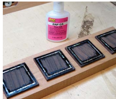
The shell inlay glued in place
