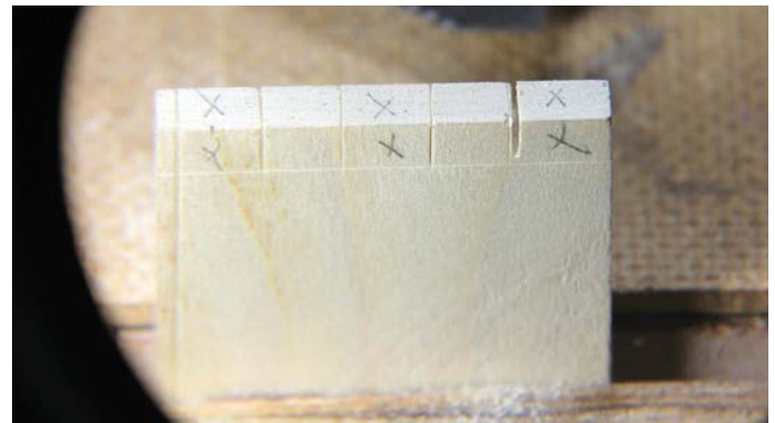
For thin stock, I use a saw of less aggressive cut, 20 tpi in this case
