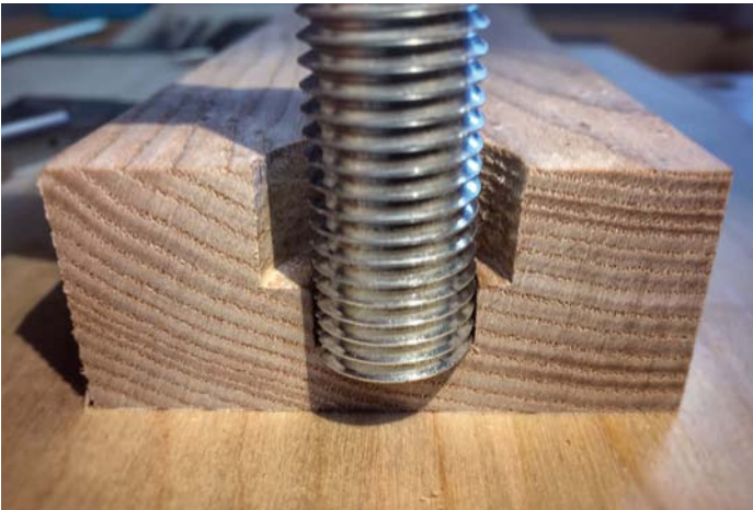
A cut-away section showing the pilot hole to support the bar
