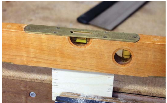
If you struggle with sawing perpendicularly, try starting with your workpiece held plumb
