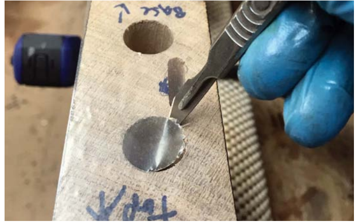
Protect the surrounding area of the first stage in a two-stage glue-up
