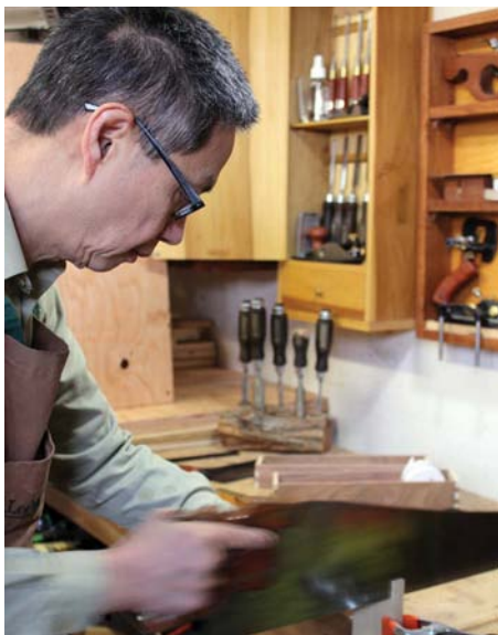
Notching out of the pad starts with gang sawing, followed by careful chisel work
