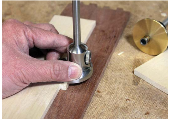
Use the wheel gauge like a depth gauge to set the depth of cut to the stock's thickness – with ease and precision
