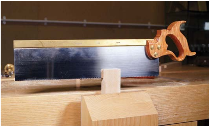
Removing the pyramid of material left over after sawing at 45°
