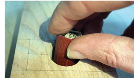
Drilling can burnish the inside of the hole so key it up with some coarse abrasive
