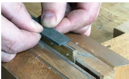
Filing along the edge and not across it will help to keep the leaves square
