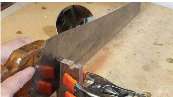
I used cramps to reduce vibrations when gang sawing the slope
