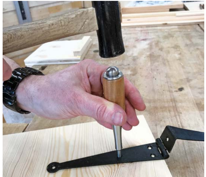
A light tap is all it takes to put a centre point in the middle
