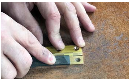
File the tops of the leaves to remove the machine marks
