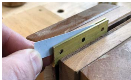
Place a piece of card between the leaves to limit the bevel on the back edge
