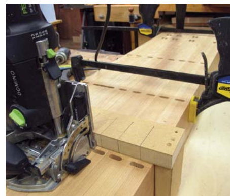
Dominoes being cut in the legs for the dust panels
