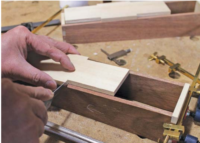
Hold the pad in position on the holder and scribe the knife lines on the edge
