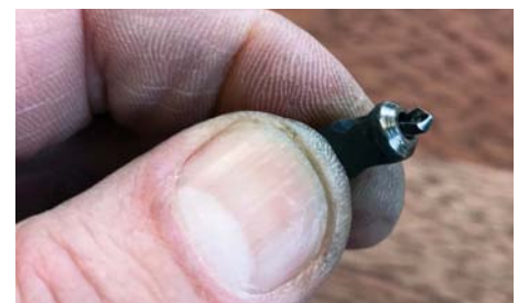
The drill bit tip on a centre should be ground to 90° and therefore more suited to drilling wood
