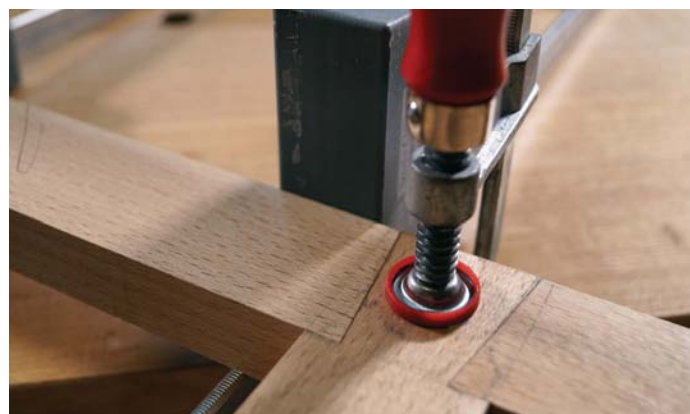
Seating the joints into their sockets
