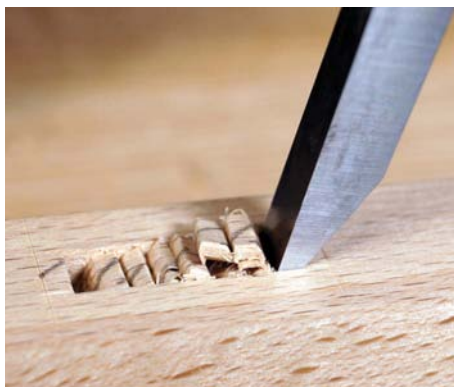
Leaving 5mm of material at the ends of the mortise to use as a cushion
