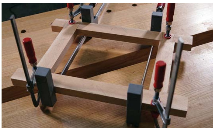
Clamping the frame together
