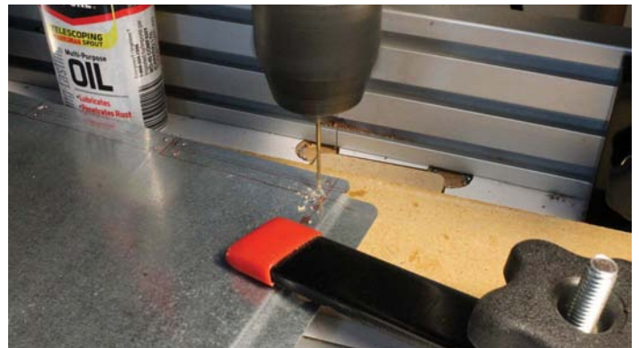
Drill the mounting holes before snipping the sleeves to size
