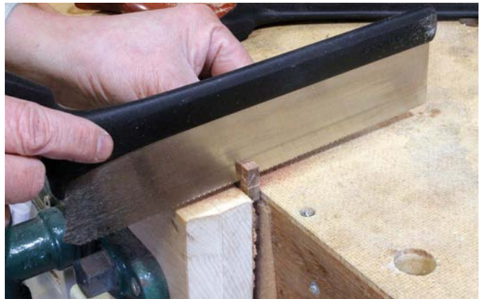
For shoulder cuts, I switched to a crosscut saw
