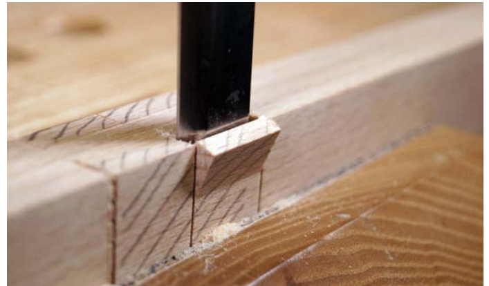
Splitting the waste material out of the bridle joint
