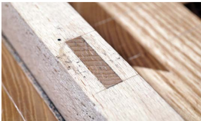
The through tenon before planing flush
