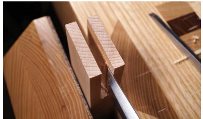
Removing the square lump in the bridle left over after establishing the edges
