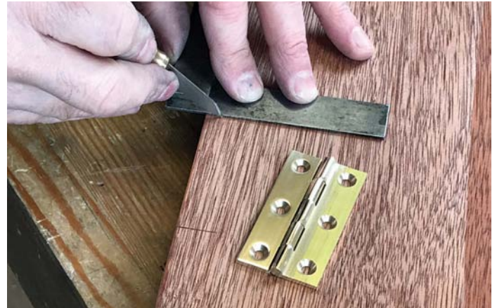
The second mark can be made directly off a square and requires no offset
