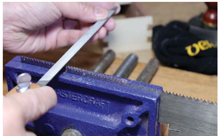
I used a discarded saw plate as a template when serrating the lower sleeves
