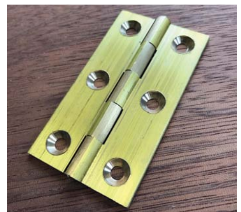
Good quality solid drawn brass hinge with drilled countersunk screw holes
