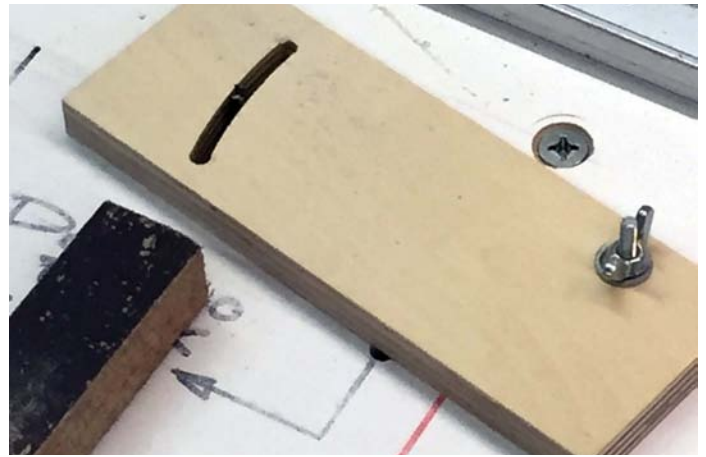
... and plunge up into the fence to cut the arced slot
