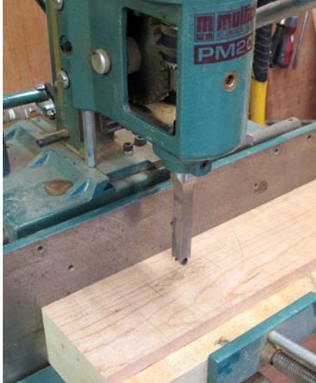
Leg mortises being cut
