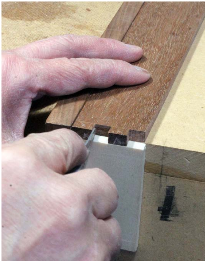
The finger transfer is made simple and easy by using a dovetail alignment jig
