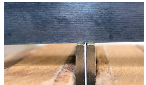
File past the rounded edge on the back of the leaves before setting the projection
