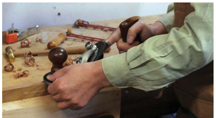
Plane the slope in pairs, which also gives more registration surface for the plane
