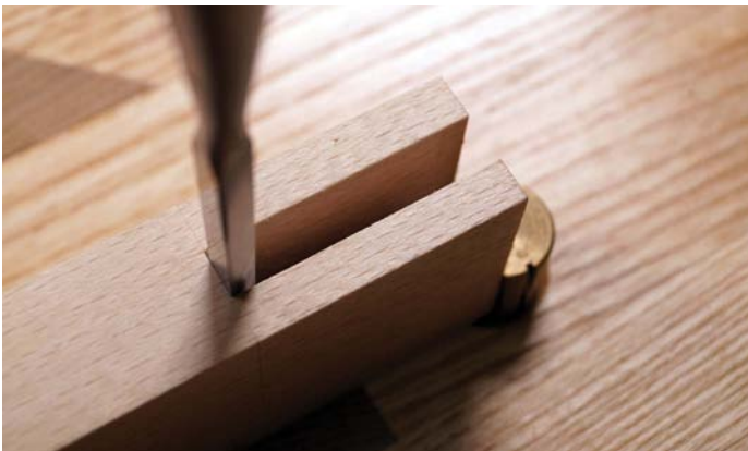
Chiselling down to the shoulder line
