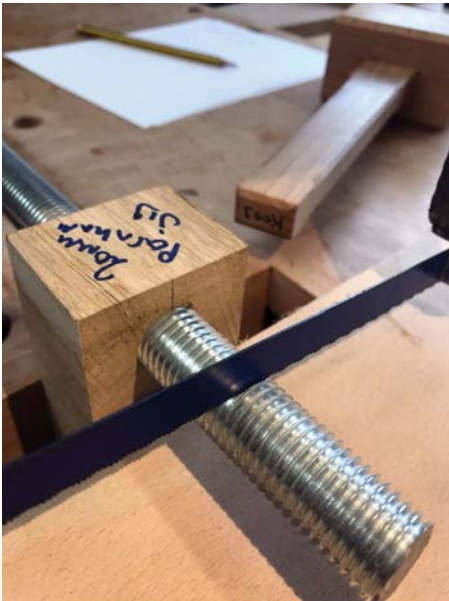
Prepare a block to hold the bar and protect the vice jaws
