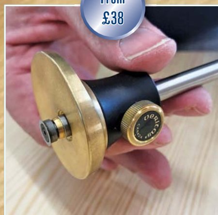
The main locking screw is larger than those found on some other makes and better for it
