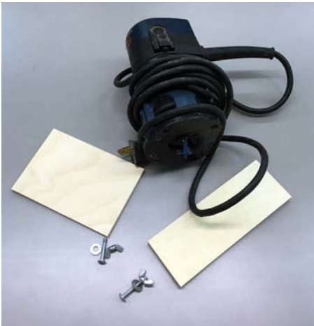
The only hardware you'll need is a couple of machine screws with wing nuts and washers
