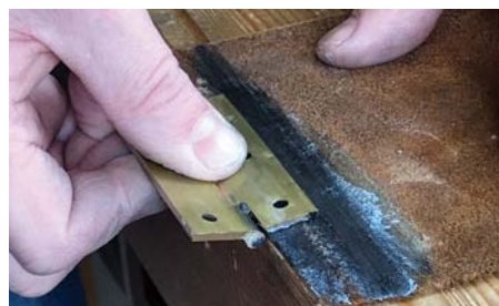
After working through the grits, finish with some metal polish and a leather pad
