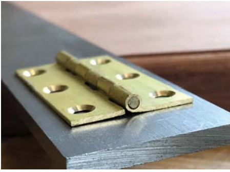
Not so good quality drawn hinge. Note the leaves don't sit flat
