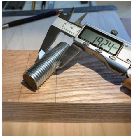
Threaded bar is not always exactly the size it's supposed to be
