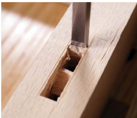
Using a narrower chisel to cut the exposed side of the mortise
