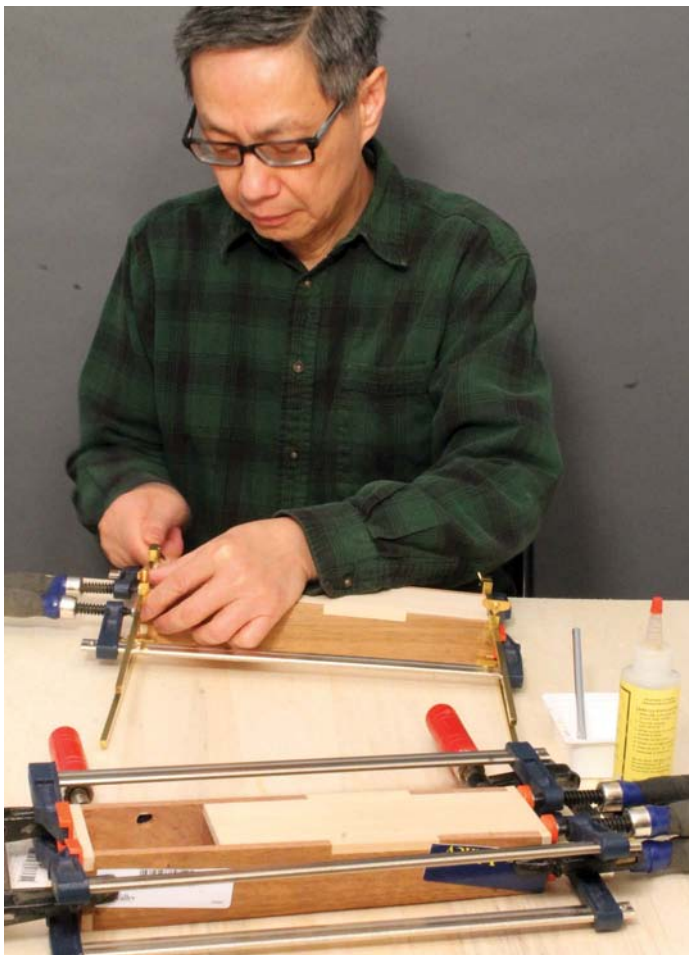
During gluing up, I used the notched pad (no glue) to help draw the assembly square
