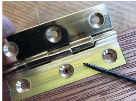
For just a couple of holes you can't beat a gimlet for speed and accuracy
