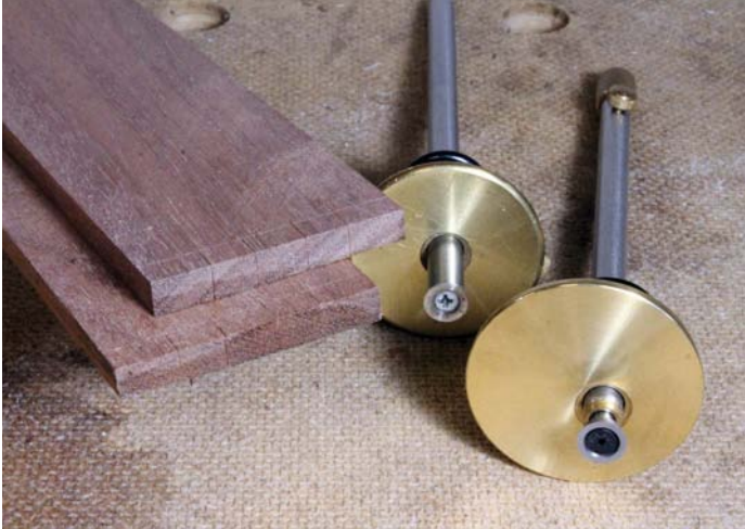
Two marking gauges are used to keep the resetting to a minimum
