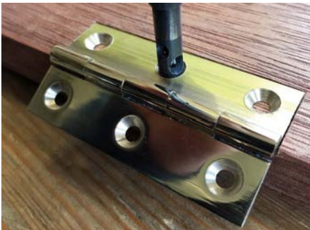
The sleeve centres the drill off the countersink
