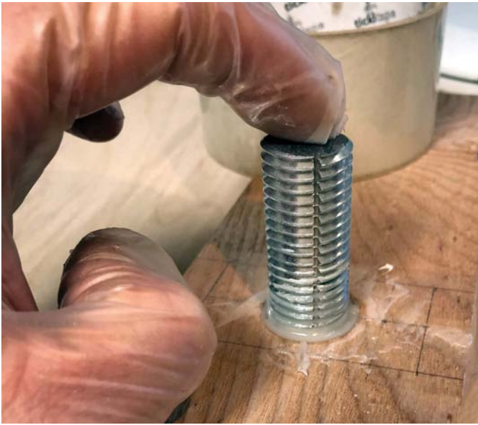
Press the bar home firmly to expel any air from the joint
