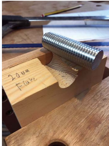
Make a cradle to hold the bar for fluting
