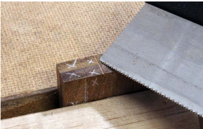
Mark out the wastes clearly and saw to the knife line so you have only a little to pare away
