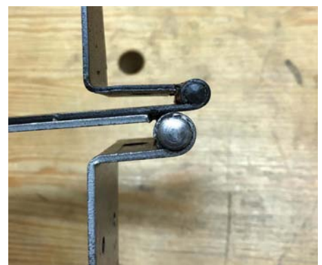
Waxed cranked hinge with penny rounds detail at the ends of the leaves INSET: Don't look for precision in strap hinges, you won't find it
