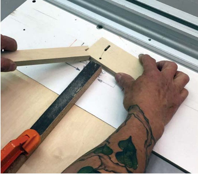
Attach the fence to your router table and fix stops either side of the cutter ...
