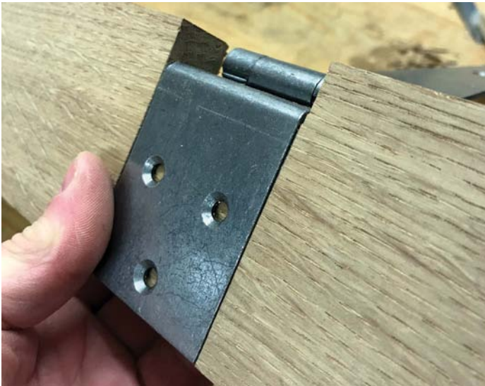
You can accommodate a shorter crank by letting the short leaf into the back of the chest
