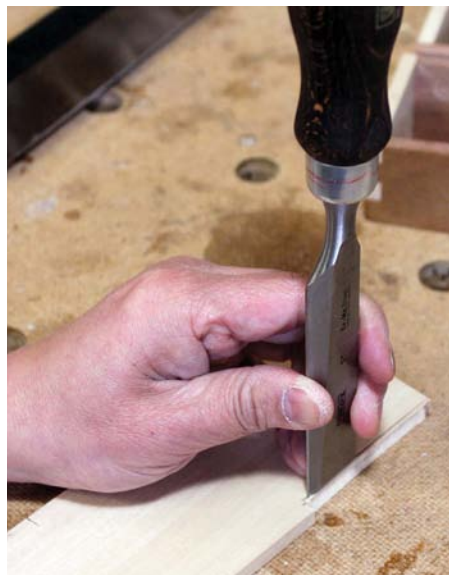
To prevent splitting, finish the cross-grain cut on the notch before working on the long edge
