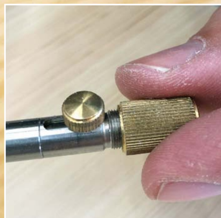
The micro adjustment screw has approximately 6.5mm of travel
