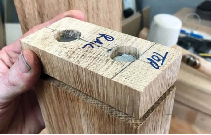
A simple jig may also be a viable option for accurate drilling
