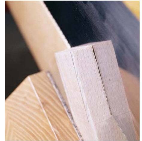
Tilting the material to 45° in the vice to help with sawing
