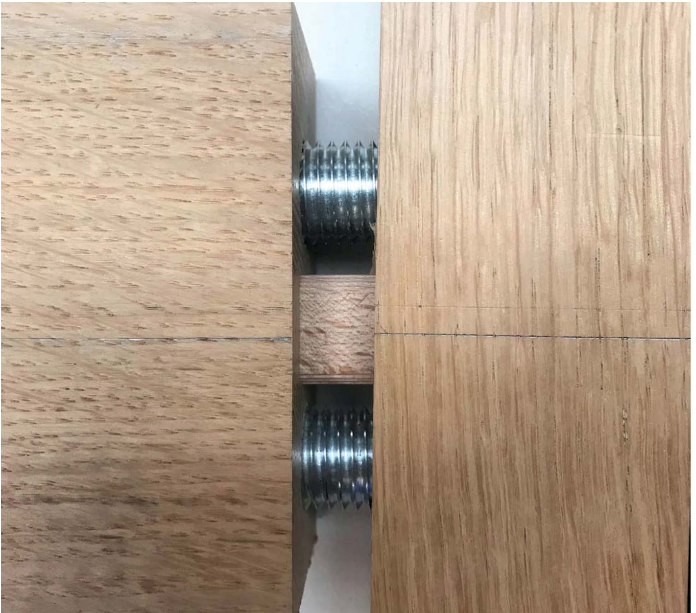
For a single-stage glue-up and easier alignment use a Domino
