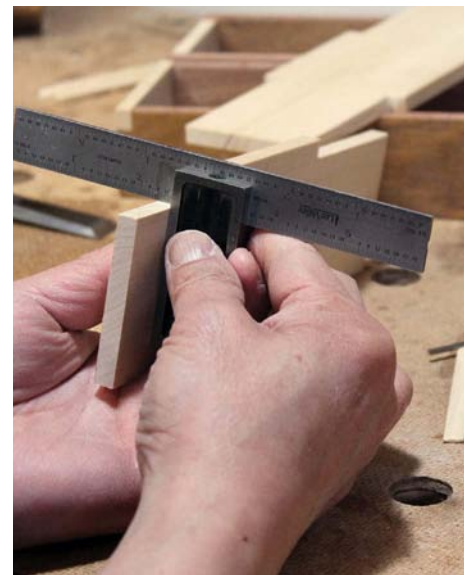
Check and remove any high spot on the notch, taking care to keep the edge square
