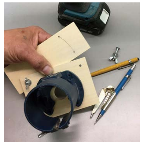
Attach the fence to the base and mark the arc through the pivot lock hole
