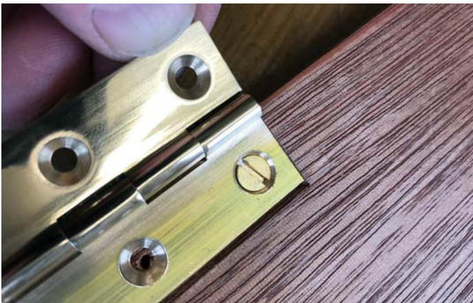
...your screw will pull the hinge out of the mortise
