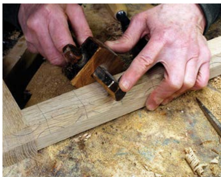
A marking gauge line is helpful to guide your paring chisel
