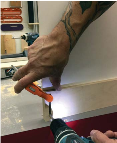
Drill through the arc to position the bolt
