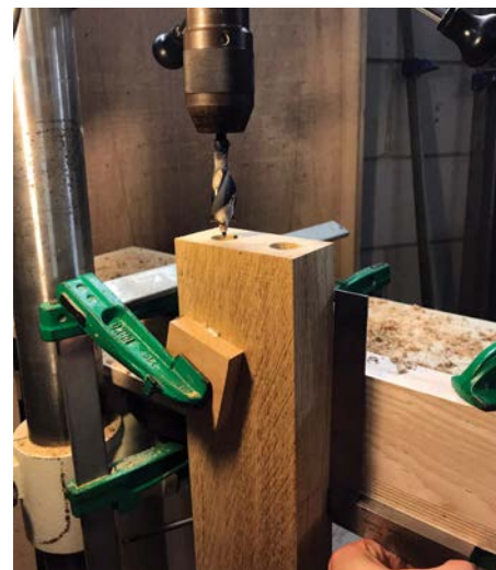
Drilling holes in end grain for the threaded metal bar
