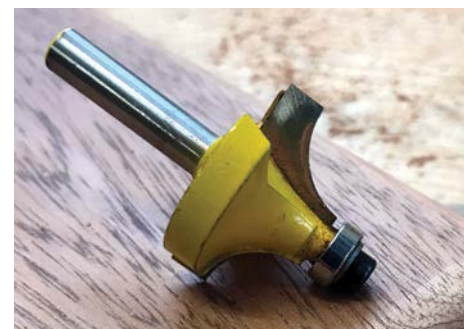
A 9.6mm radius cutter is on the limit but quite possible
