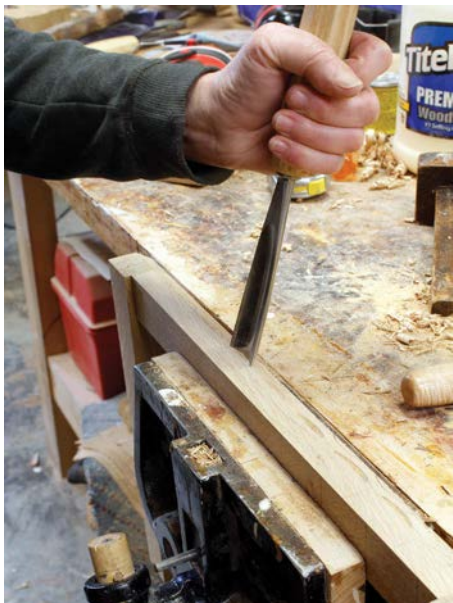
Hold your gouge at about 90° to the chamfer
