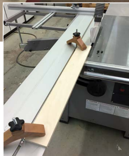
Straight lining one edge of the birch ply
