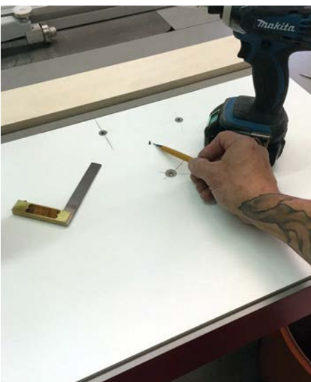
Fix down and pierce through with a small straight cutter
