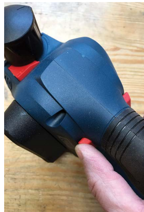
The trigger has a safety switch that can be operated from both sides of the machine
