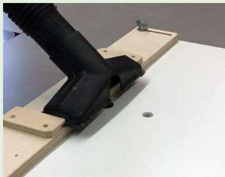
A standard vacuum accessory makes the perfect dust capture mechanism
