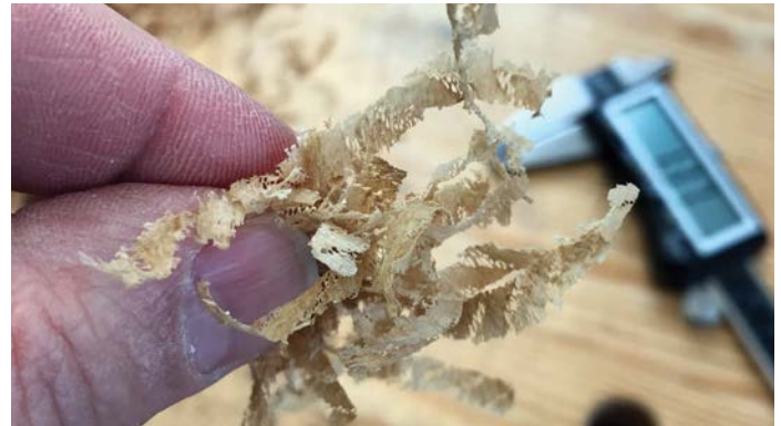
Thick, wide shavings could block the exhaust when used with the extraction bag
