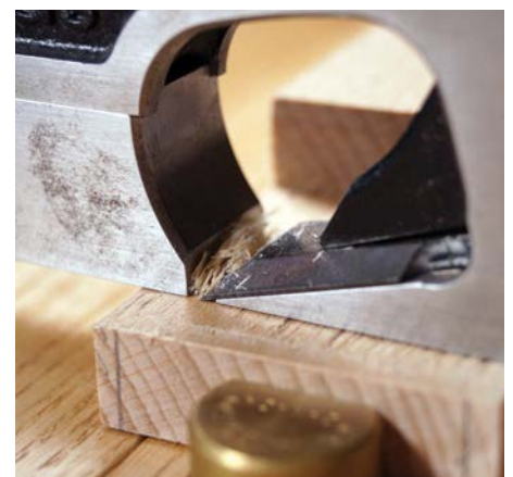
Fine-tune with a shoulder plane or chisel
