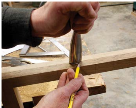
After marking out the basic spacing, trace the gouge pattern directly from the gouge
