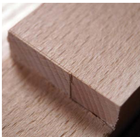
Chop back to the shoulder line in small increments
