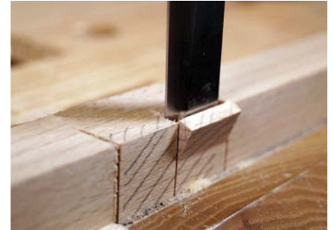
Work from both sides when removing the waste
