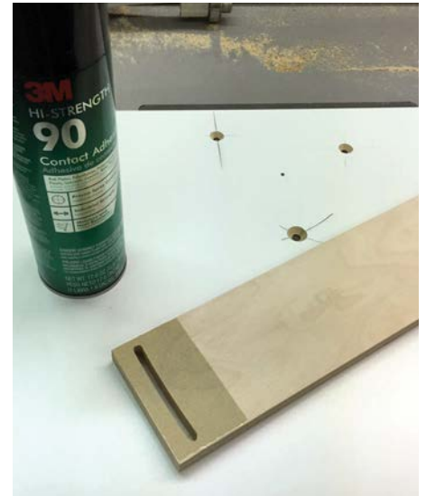
Glue a strip of abrasive paper to the underside of the fence
