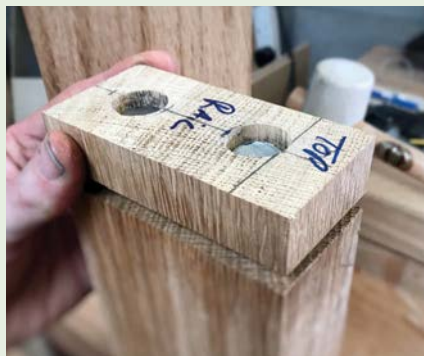
A jig is used to centre the dowels
