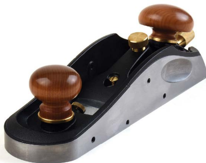
The latest incarnation of the mitre plane comes from Veritas in Canada, and among French speakers is called a rabot à onglet in the Félibien tradition. This 10 1/2 in ductile cast-iron plane brings back both the forward and rear knobs for ease of use. The low 12° bed angle of the bevel-up cutter with Norris-style adjuster makes this Veritas mitre plane work effectively across the grain
