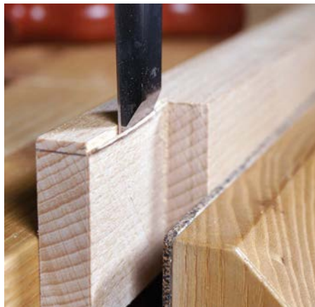
Use a sharp chisel to establish gauge lines
