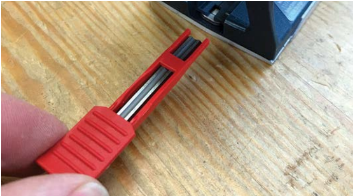
On-board storage for a spare blade
