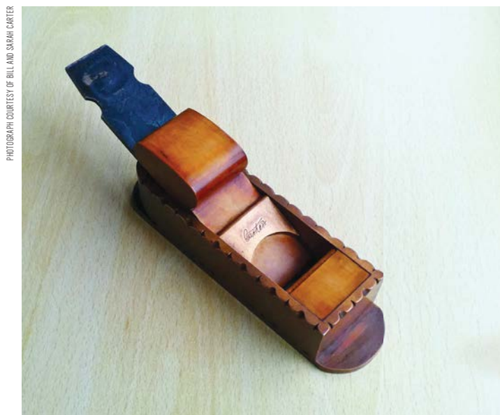
A bronze dovetailed 6 1/4 in mitre plane by Bill Carter shows exposed Cupid's bows along the bottom sides of the plane and also in the sole; there is also a Cupid's-bow decoration running around the top edge. The bridge is in bronze while the infill and wedge are in honey-coloured English boxwood. The cutter, made by Carter from an old iron by Aaron Hildick, is bedded at 20°
