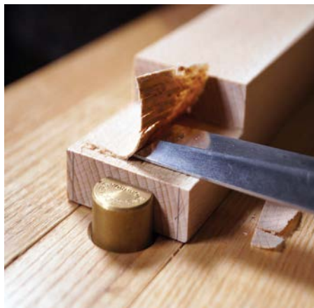
Remove the bump with a chisel
