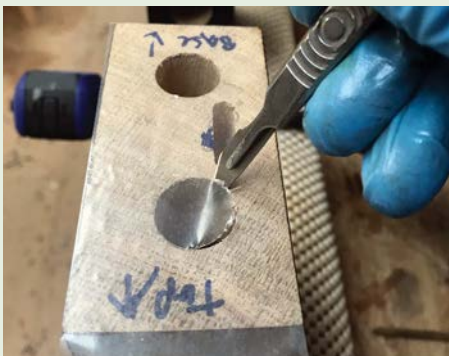
Masking the timber on the first stage of gluing up
