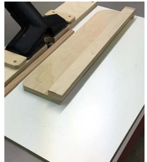
A captive push stick makes for safer routing of smaller stock
