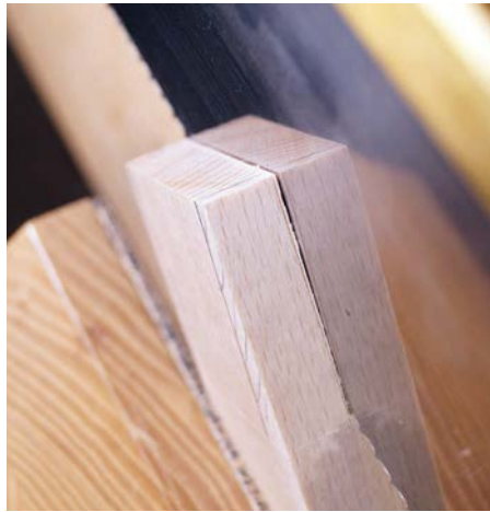
Saw 1mm away from the marking gauge line
