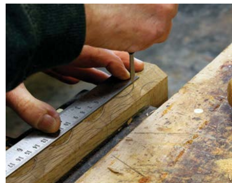
Use a marking knife and steel rule to define the edge of the chamfer wherever your gauge won't reach
