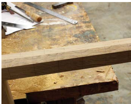
Square the ends of the gouge positions onto the flat area at each side of the chamfer to guide your marking gauge
