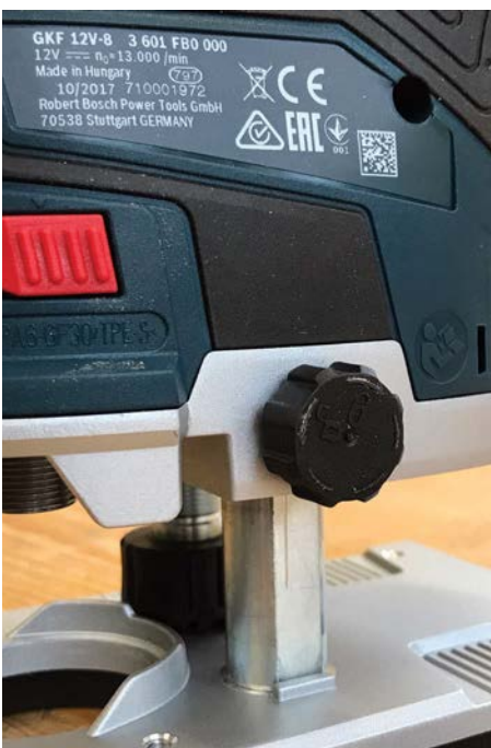
Depth lock allows to you save settings
