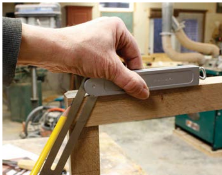
Mark the angle of the chamfer at each end of the table and extend with pencil lines, then plane the chamfers by hand, working from each leg towards the centre of the rail
