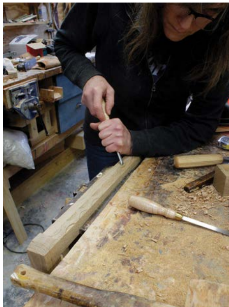
Pare the thumbnail from the gauge line at the edge of the corner down to the deepest part of the gouged curve
