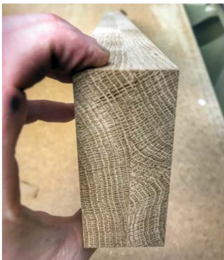
The seat rails are laminated for strength
