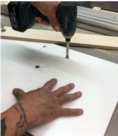
Fit the base in place using longer machine screws if necessary
