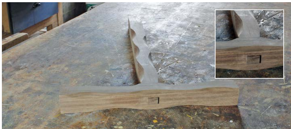
Where the end of a chamfer is near a shoulder, it's best to leave the last bit of paring until after you've glued up the piece, to avoid removing too much material
