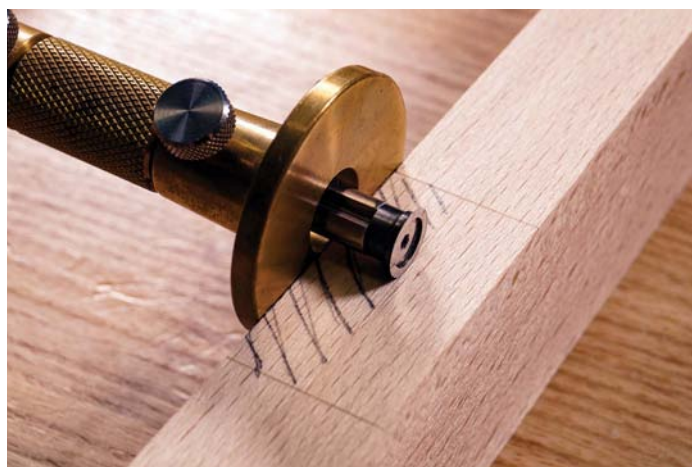
Gauge the waste material from the same face...
