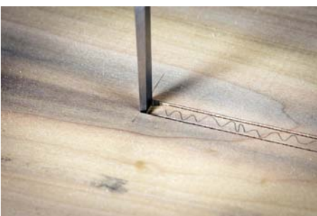
Come in from both sides with a chisel to remove the waste
