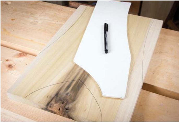
Make a half-pattern to help keep the form symmetrical
