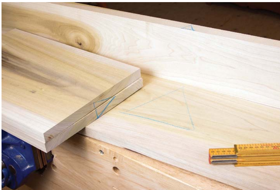
Keep the parts straight with the cabinetmaker's triangle
