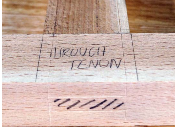
Project the mortise width from the tenon component
