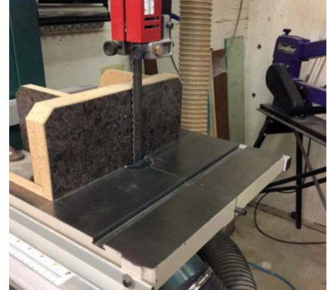
Lock down the fence or, if it's an auxiliary type, clamp it in place
