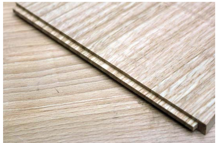
Tenons cut and cleaned up with a sharp chisel
