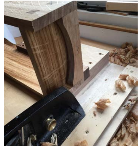
Flushing up with a shooting plane
