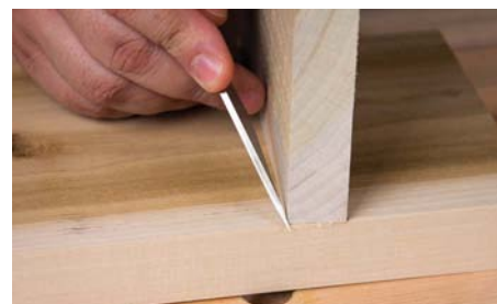
There's no need to measure: use the actual parts to ensure accuracy
