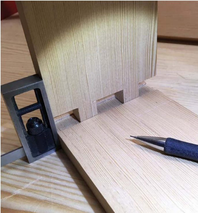
Use a dado to register the mortises from the tenons
