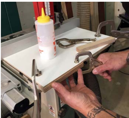
Using glue, clamp, then fasten a cleat ...
