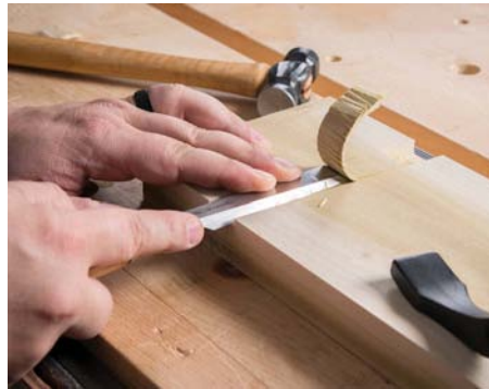
Be sure to keep both hands behind the chisel edge – safety first
