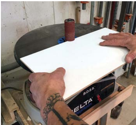
Start with clean, square cuts on some 1/4in material (with a notch for the blade) that is about the depth of your table. Allow a bit of overhang to the right for two cleats
