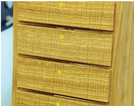
Fitting of the drawer fronts in their openings
