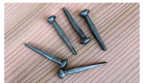
Traditional cut nails are quick and strong
