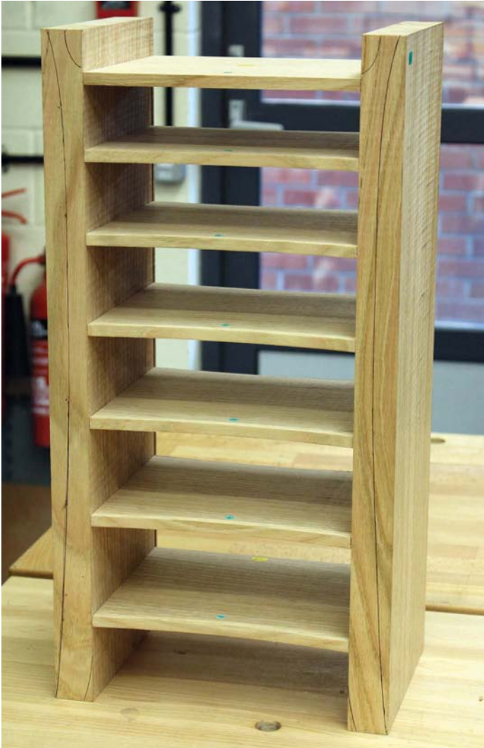
A dry fit to check everything
