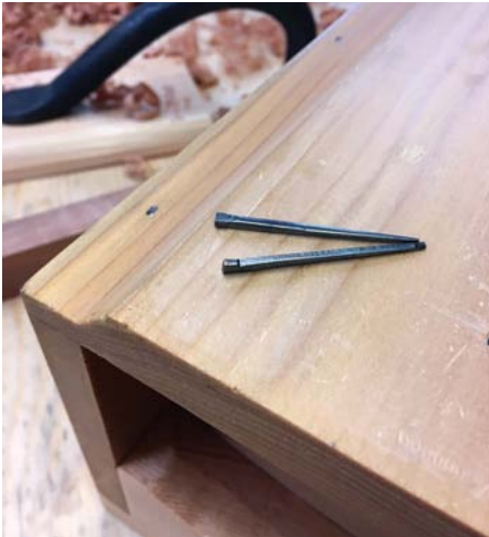
Run the nails in the rebate to keep a smooth bottom
