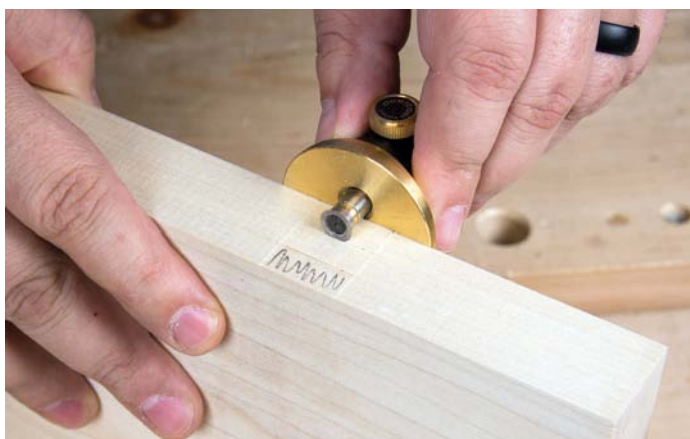
Set your marking gauge once you divide the thickness into thirds
