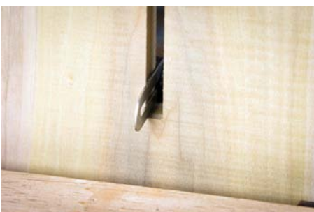
Use the sliding bevel to check the bottom of the slot
