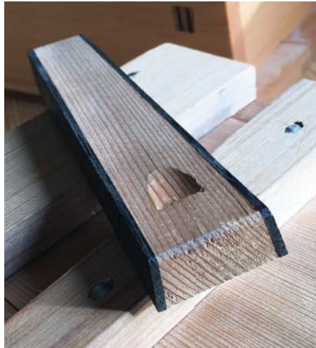
A retro fitted wedge with contrasting slithers on both sides
