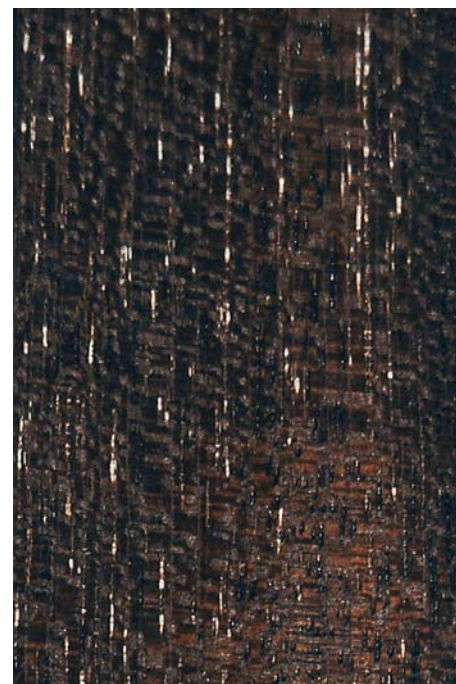
This unfinished true mahogany ( Swietenia spp.) was recycled from redundant 18th/19th-century table leaves. Note the very light-coloured silica deposits which cease to be visible when finish is applied ...
