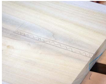
Mark the waste and make sure you don't saw on the wrong side of the line
