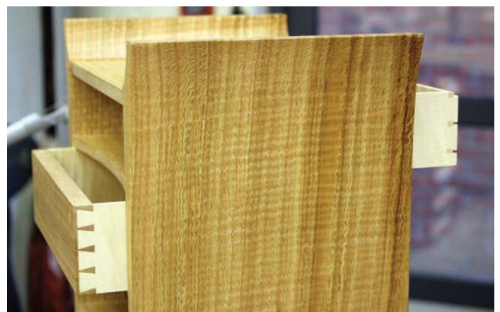
The drawers being fitted from the rear to ensure a smooth piston fit
