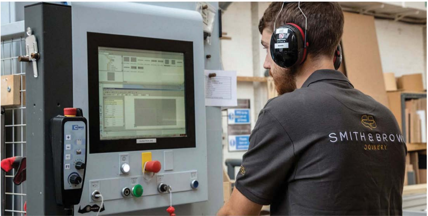
Programming a cutting list for optimal use of the board
