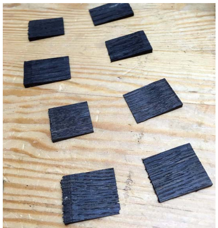
Keep your wedges short to avoid splitting the tenon
