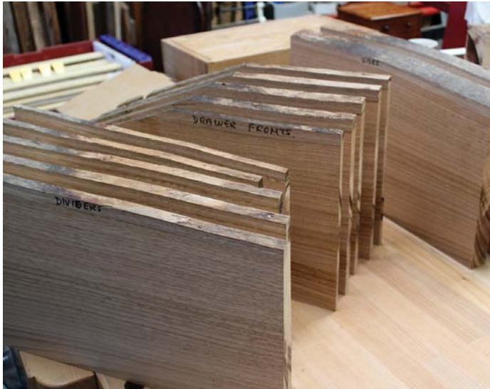
Parts cut on the bandsaw and being allowed to settle
