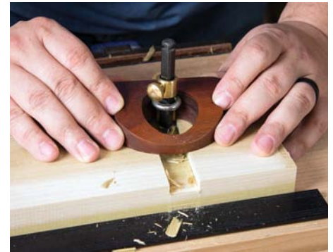
Router planes are perfectly suited for making a clean, flat surface
