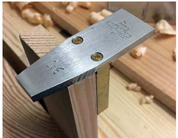
Use a dovetail marker to set the angle on the wedge
