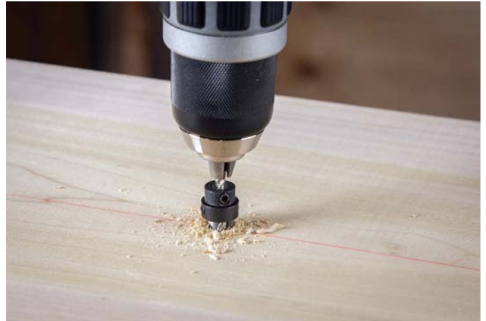
Always drill pilot holes for your screws to prevent cracking
