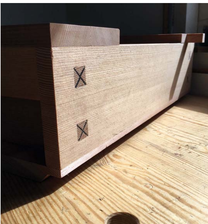
X wedges take a little more time but may help to close up any gaps in the joint
