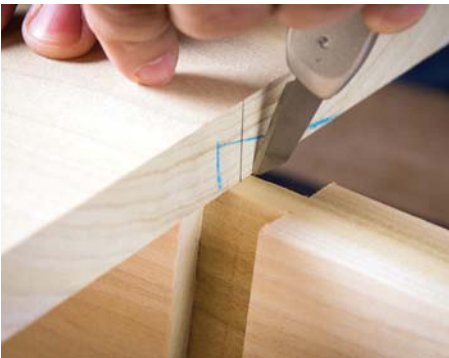
Transfer the thickness carefully with a marking knife
