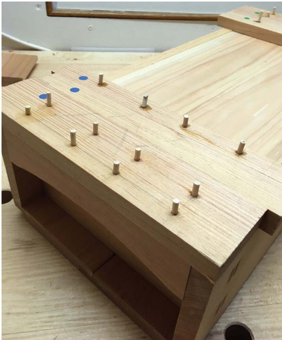
Tapered wooden nails are a neat way of securing the battens to the lid and box
