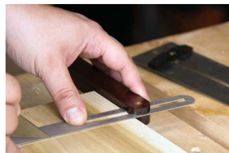
Make light strokes with the knife for accurate lines
