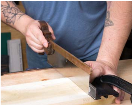
A jig can help you learn how to saw straight
