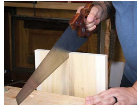
A panel saw is the best choice for deep cuts
