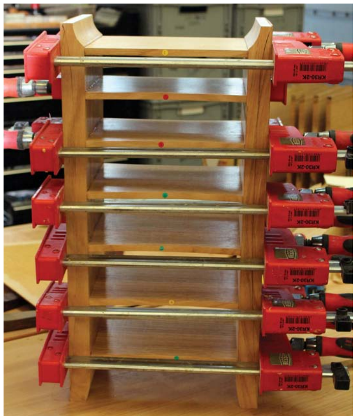
Gluing up the carcass using the offcuts to keep the clamps square
