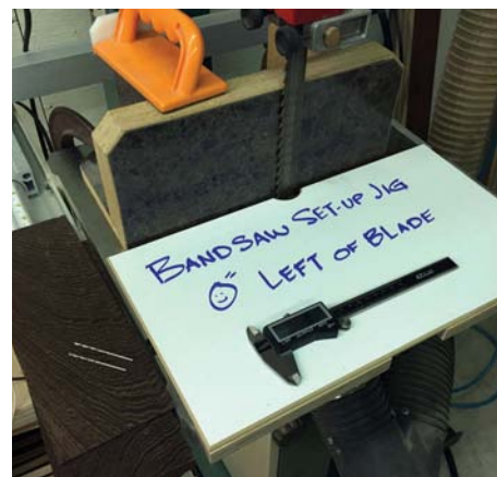
Once your jig is established and registers 0 distance left of the blade, you could use a matching pair of any size drill bits to make cuts quickly and accurately
