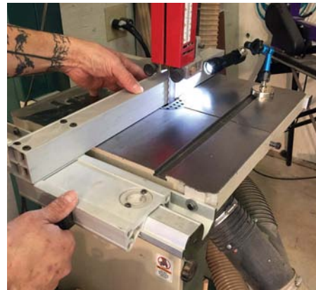
Use a strong light, and bring the factory fence just barely against the blade without actually quite touching it, and lock it down
