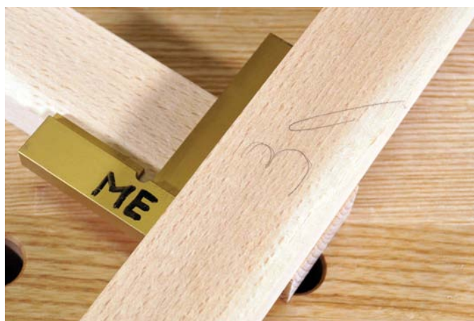
Use a square to line up the component...
