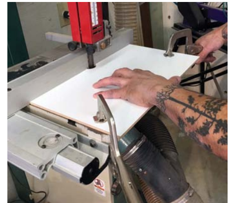
Place the 1/4in material against the fence, then clamp it secure
