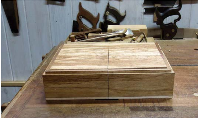
Checking the lids for alignment
