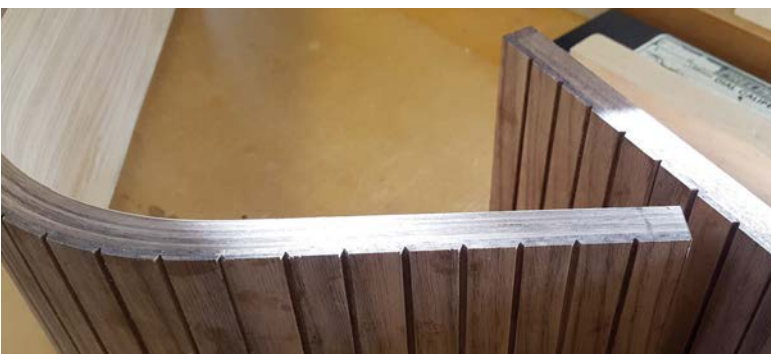
Tambour detail side with layers of constructional veneer
