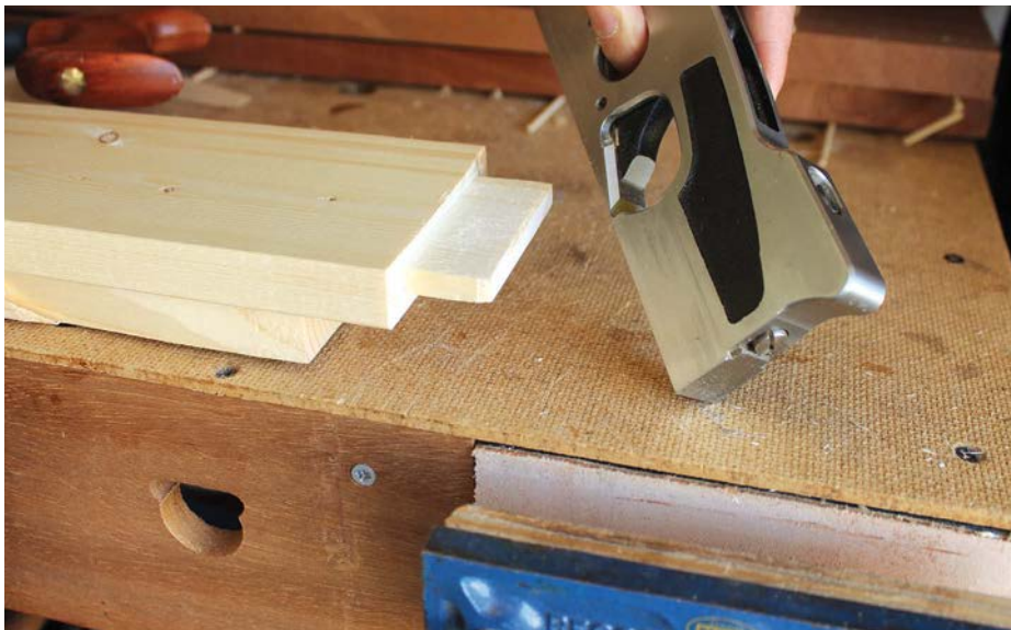
Reference the body of a shoulder plane against the cheeks to keep the shoulders square
