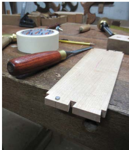
Rare earth magnets are buried into the tails of the sides before gluing the box together
