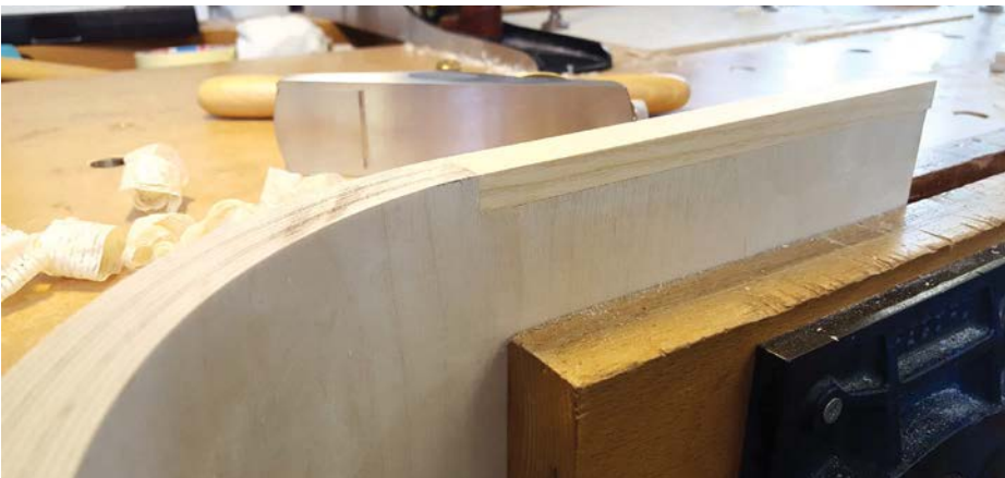
Solid wood blocks inset for handle seats
