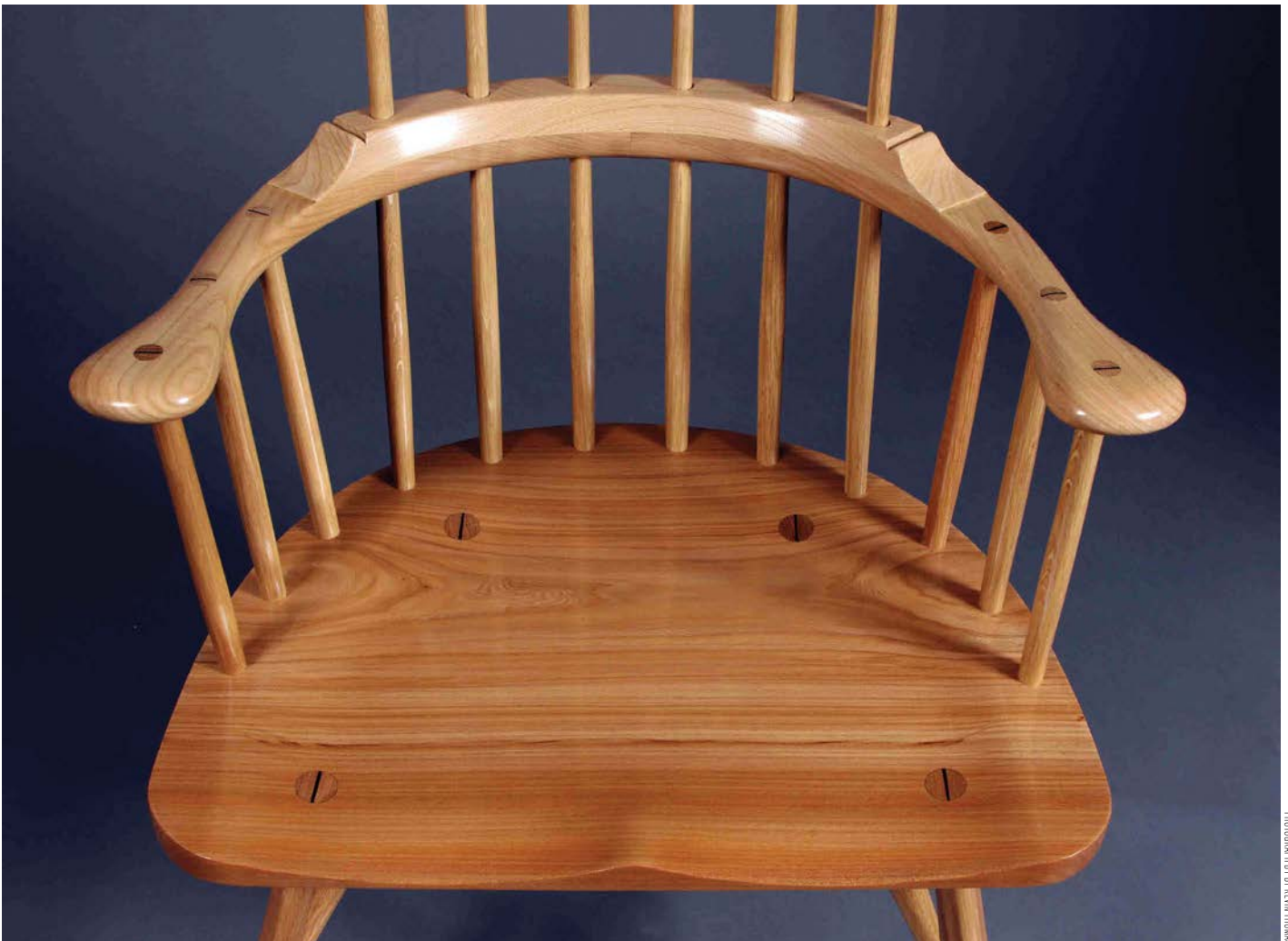
Here you can see the three-piece scarf joint in the arm
