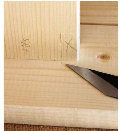
Position the stretcher in place and transfer the tenon lines to mark out the mortise ends on the upright
