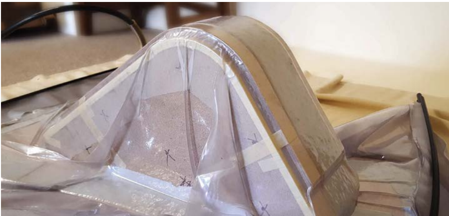
The flexiply layers of the apron side being formed
