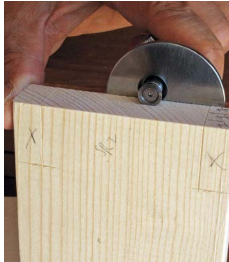
Use a wheel marking gauge, if you don't have a mortise gauge, to mark out the tenon cheek
