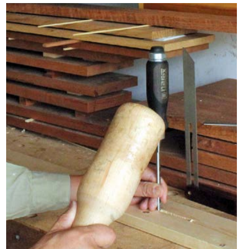
Sighting against a sliding T-bevel, taper the ends of the mortise to create the expansion slots
