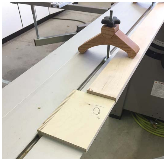
The 'Go-no-go' jig quickly ensures precise and repeatable alignment with the left side of the saw blade
