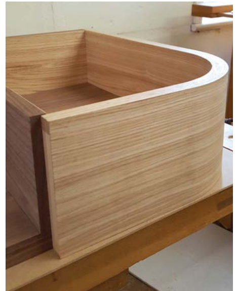
Completed apron sides dry fit to base
