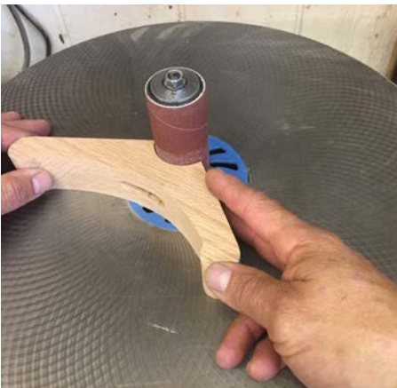
Smooth all cuts with an edge sander, bobbin sander, scraper, etc.
