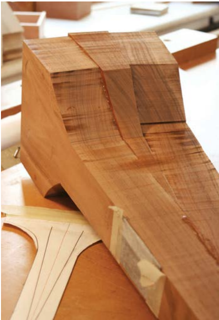
The wedged blank for turning the legs
