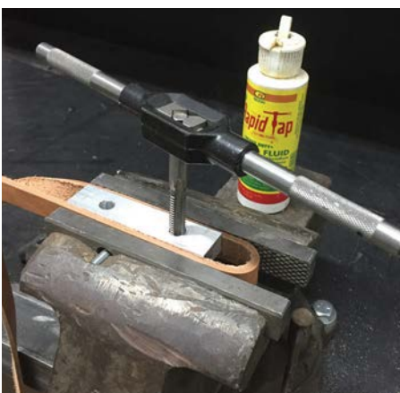
Drill and tap a couple of holes to suit your thread. I left mine long for easier clamping, then cut the aluminium into halves
