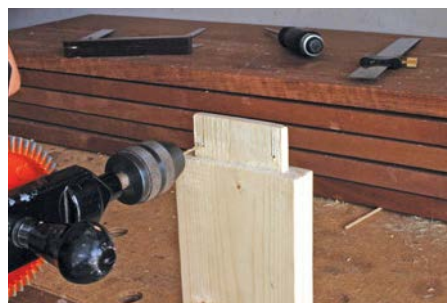
Drill the stress relief holes slightly off-centre towards the edges to prevent splitting
