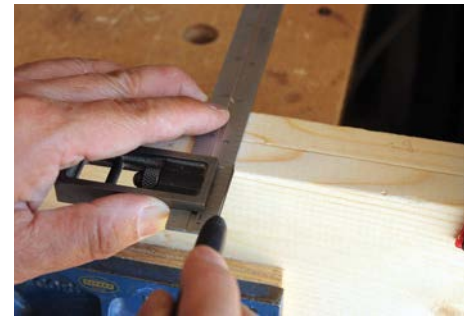
Lay out the ends of the blind mortises for both bases at the same time, ensuring consistency
