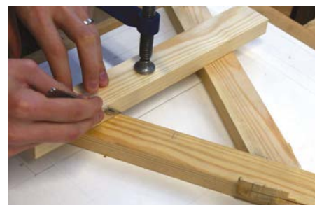
Clamping the crosspiece may require the use of a single deep throat clamp for better access and to aid accuracy
