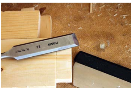
A knife wall is chiselled on the shoulder line to act as a saw guide for the cross-grain cuts
