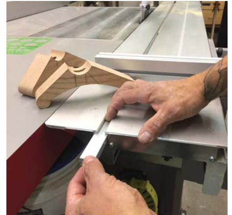
Select a piece of aluminium or steel bar to fit the slot
