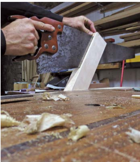
Ripping maple by hand to get the inner sides of the boxes from the same board (inside the box)
