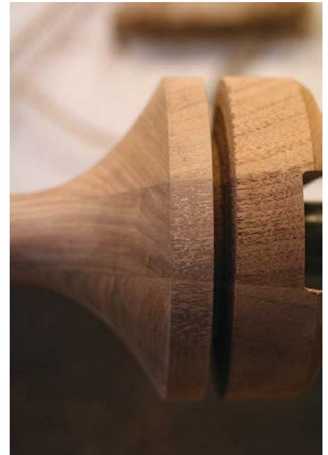
Turned walnut leg on the lathe, spigot and edge visible
