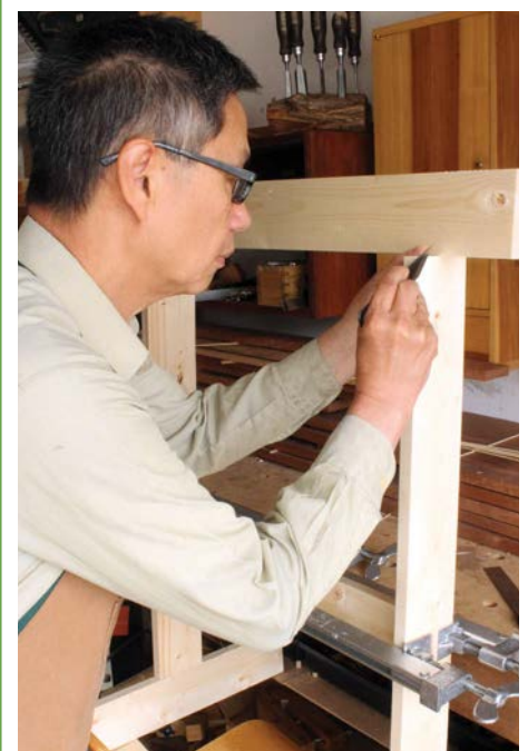
Dry-fit the frame and mark out the saddle joints maths-free
