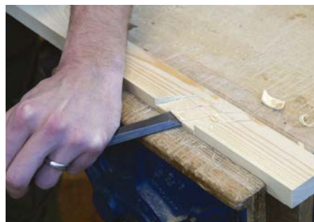
Removing the waste using a chisel and mallet
