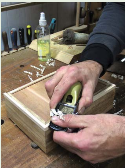
Levelling off the maple strips
