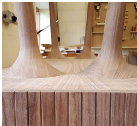
Legs dry fit in base after shaping
