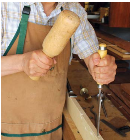
I prefer the layered approach, making shallow cuts and levering out small chips, rather than too much stock at one time
