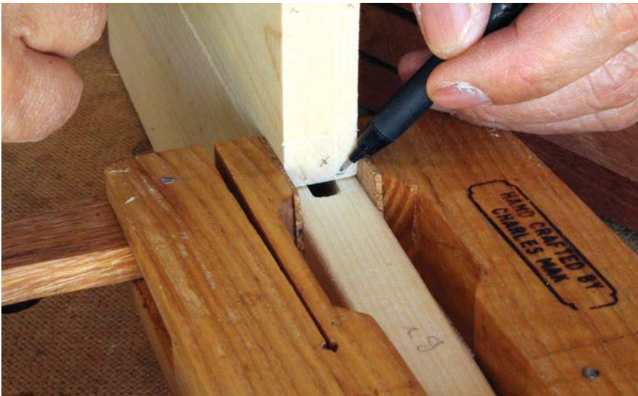
The precision secret: hold the tenon against the mortise to determine the tenon's saw lines
