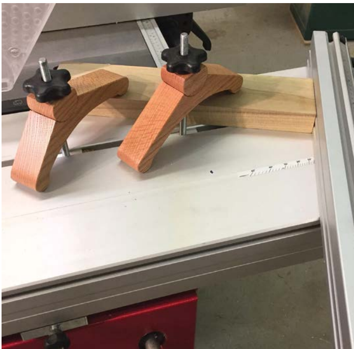
Use the clamps to securely hold small workpieces
