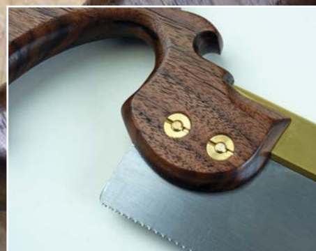
Split nuts enable disassembly for future maintenance
