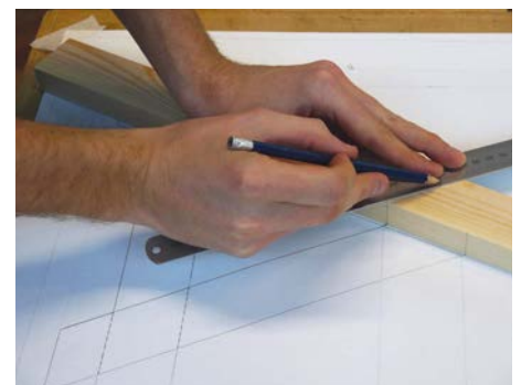
Marking out using the rod requires no calculations of angles or lengths
