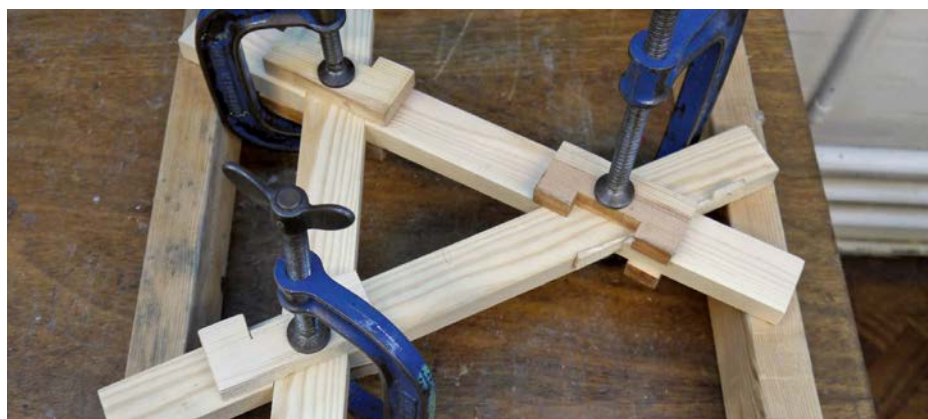
The setup used for gluing the frame
