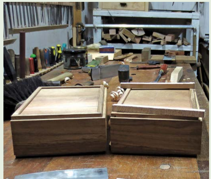
The maple strips are left proud and mitred at the corners
