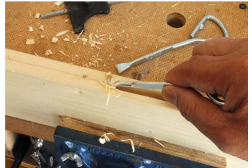
A paint can opener can be used instead of a bent chisel to excavate waste, a clever tip from Paul Sellers
