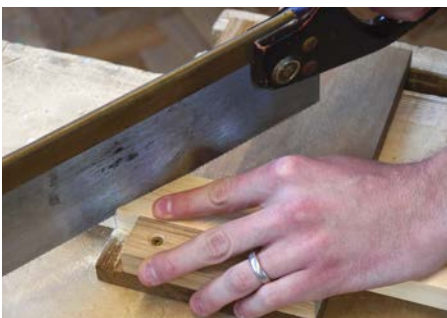
Cutting the angle of the joints is made easier by adjusting your positioning in line with the angle
