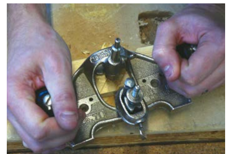
Using a router plane to tidy the base of the joints
