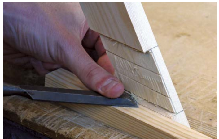
Any scrap timber will work to create the guide, as long as it is flat
