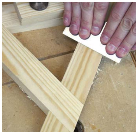
A freshly burnished scraper will give you the best results when tidying the frame up
