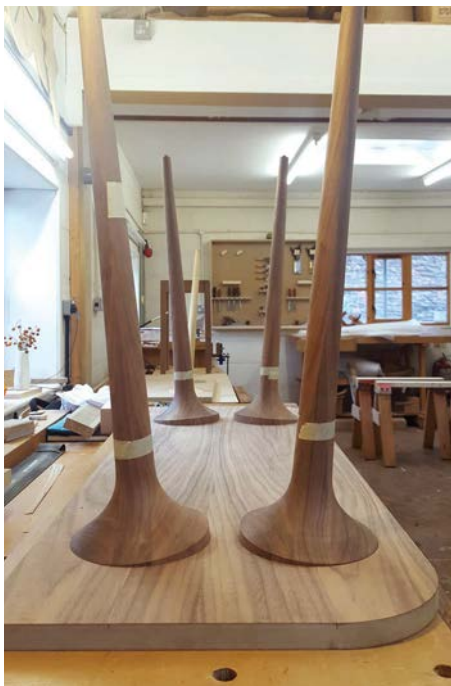
Legs dry fit in base prior to shaping
