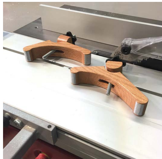
Small pieces of abrasive paper (sandpaper) will tremendously improve 'gription'
