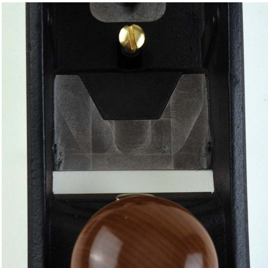
The bed is machined at 12° to achieve a cutting angle of 37°
