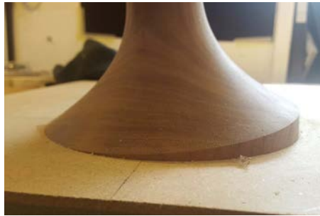
Leg placed into dummy base socket ready for shaping
