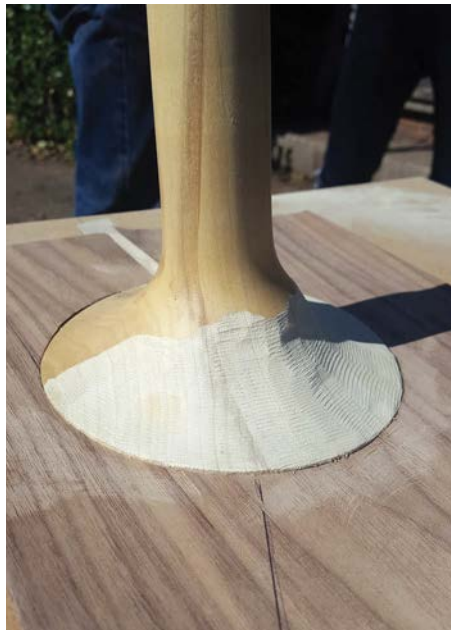
Rough shaping the practice leg with an angle grinder
