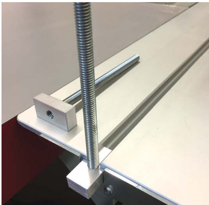
Ensure the blocks slide freely in the mitre slot
