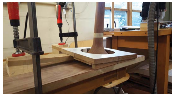
The leg socket routing template for the base – checking the fit of the leg
