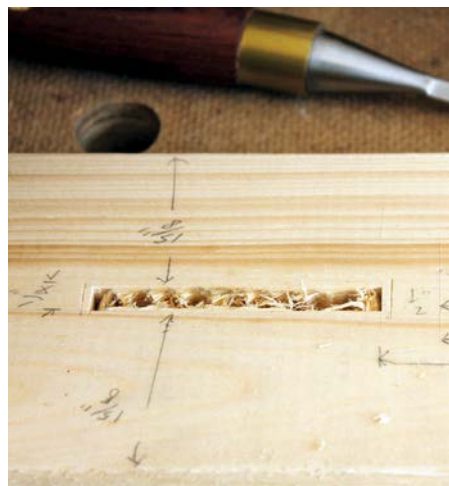
Use a smaller bit to bore inside the scribed lines, drilling from both faces of the workpiece
