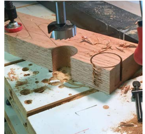
A Forstner bit will create an arc or 'saddle' for the pivot disc (circular section)
