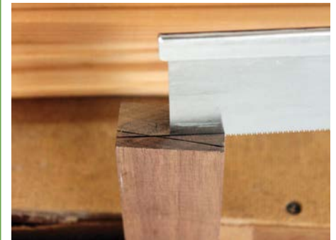
Make the wedges slightly longer and then blunt the tips to make them a hair thicker than the wedge slots
