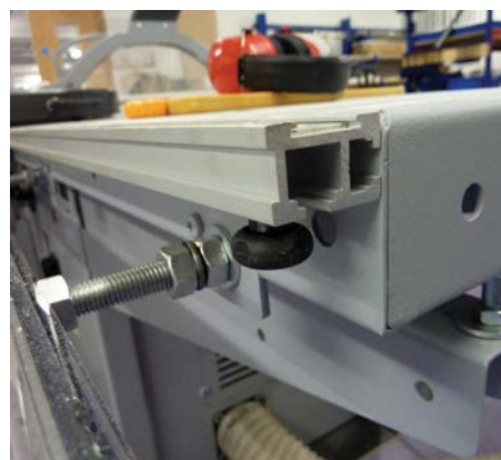
Loosen a thumb screw to recalibrate the fence scale
