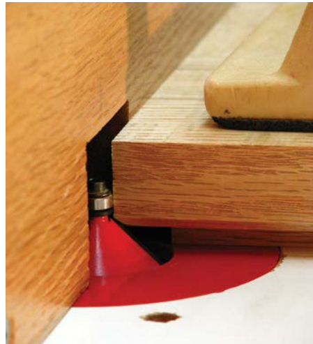
LEFT: Machine a small chamfer to the edge of the rebate
