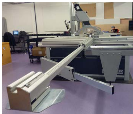
The standard outrigger will support a 2.6m long board
