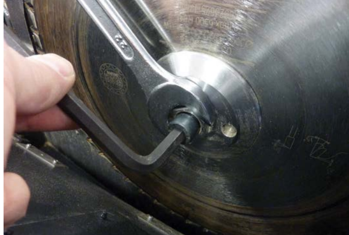
The small hex screw helps to avoid over tightening
