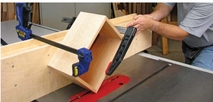
Cutting the spline grooves on the tablesaw
