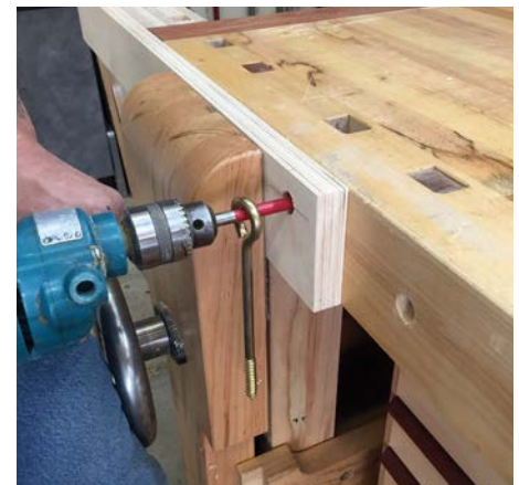
Drilling the location holes
