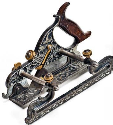
This skew-mouth fillister by Stanley Rule & Level Co. of New Britain, Connecticut, in jappaned and polished cast iron with rosewood handle, epitomises the short-lived passion among American plane-makers for elaborate foliate decoration in the late 19th century
