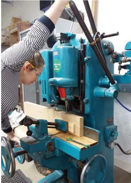
Drilling the mortises
