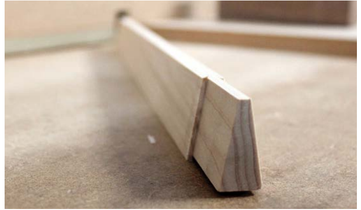
The shoulders are cut on three sides of the dovetail
