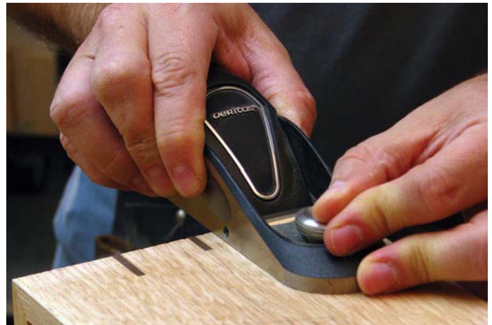
Plane smooth with a block plane in the direction of the grain
