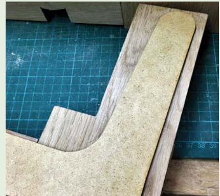
The extra waste made it easier to get identical curves
