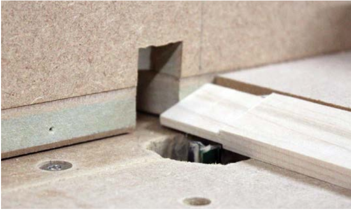
Cutting shoulders on the table router
