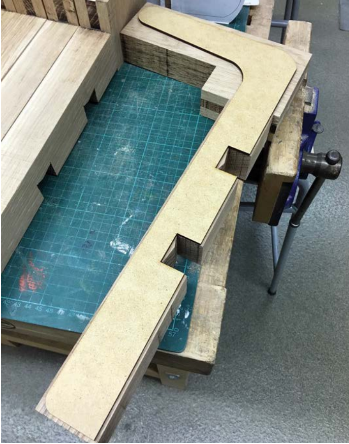
The MDF template was attached to each beam ...
