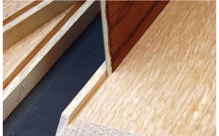
Mitred and grooved for the base panel
