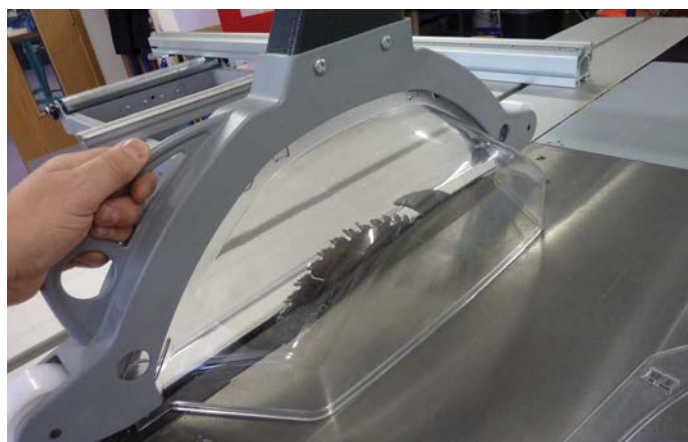
The guard can be lowered all the way down to the surface of the table
