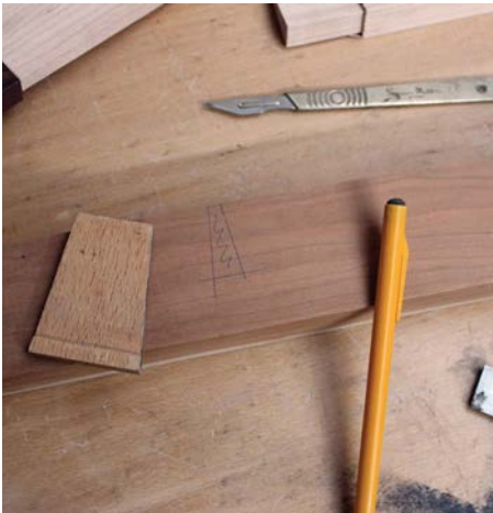
The layout lines from the scalpel are defined with a pencil and dovetail marker
