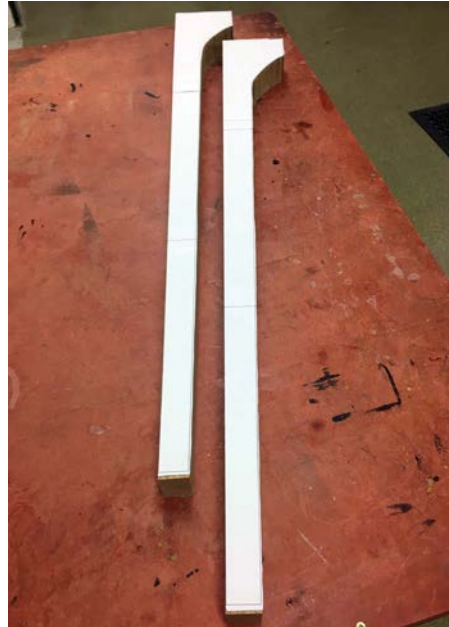
The legs were taped together to ensure they were identical
