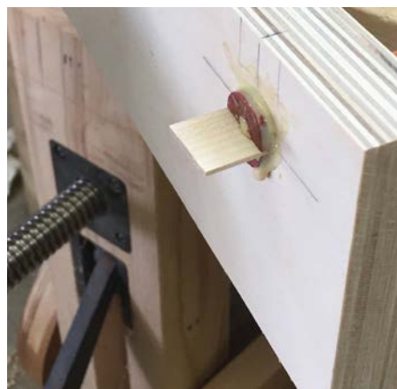
Dowels glued and wedged
