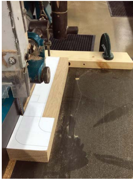
Setting up the guard and jig on the bandsaw
