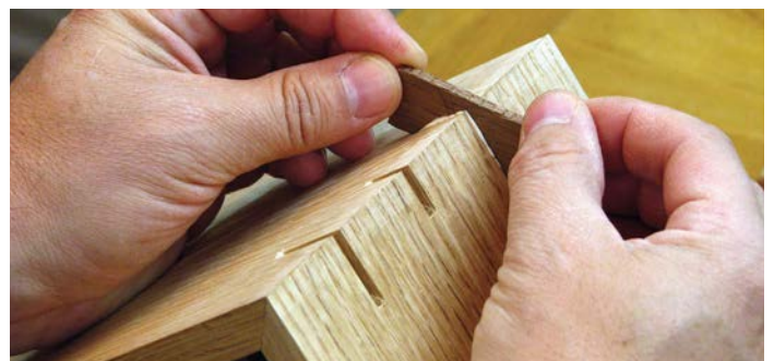
Slipfeathers help to strengthen the corners of the box
