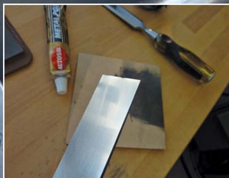
Metal polish and a block of MDF will put a good shine on the surface
