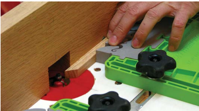
Featherboards apply firm pressure on small components
