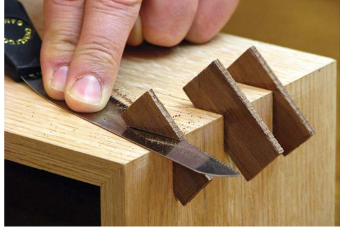
Trim the excess away with a flush cut saw
