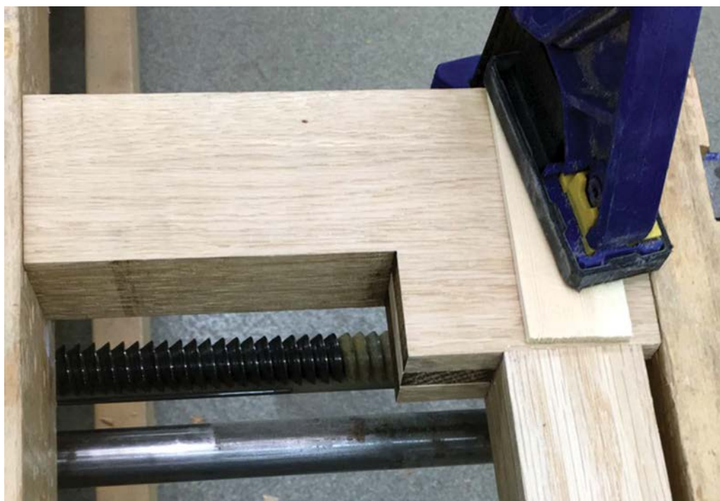
Extra clamps were used to apply pressure evenly
