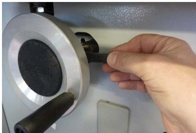
Height adjuster for the main blade and scoring blade
