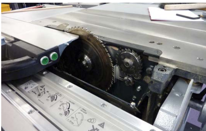
Slide the carriage forward to gain access to the scoring blade
