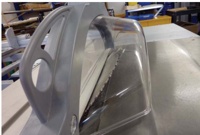
Tilt cuts are completely covered
