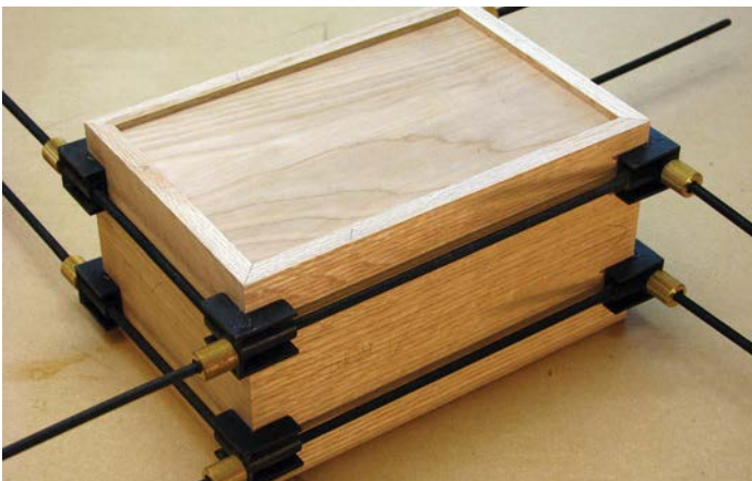
Veritas box clamps make gluing up easy
