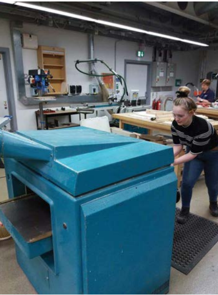
Planing and thickening the oak for the backrest
