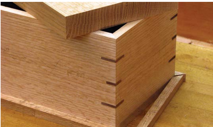
Account for the moulding when spacing the slipfeathers
