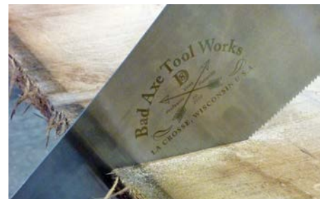
The 9tpi crosscut will charge through wide boards
