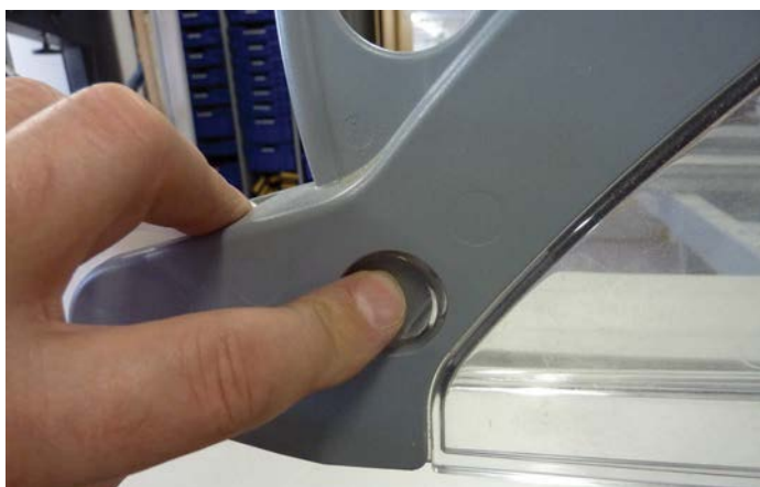
Push buttons hold the clear guards in place
