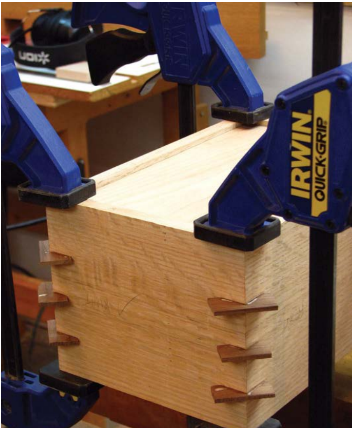
Clamping along the mitres helps to close any gaps
