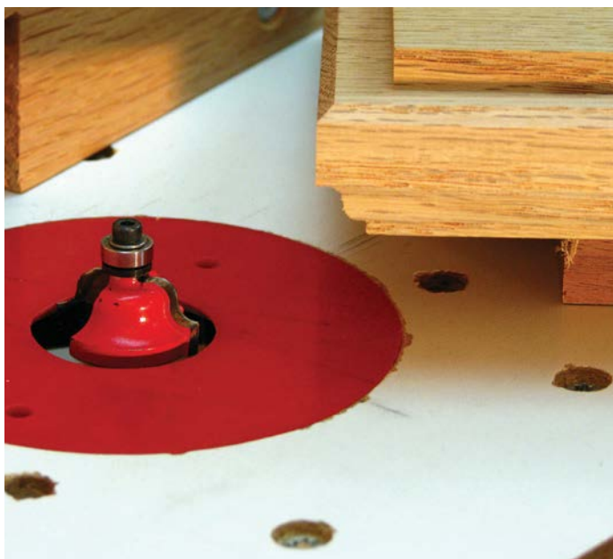
An ogee profile is routed into the top edge of the lid
