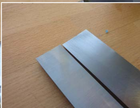
Machine marks are replaced by an acceptable scratch pattern
