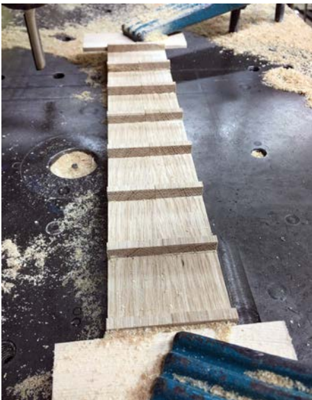
The beams are separated by spacers
