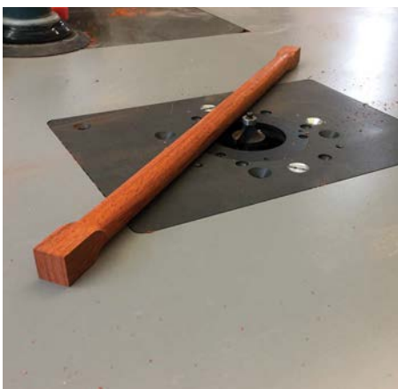
Machining dowel on the router table
