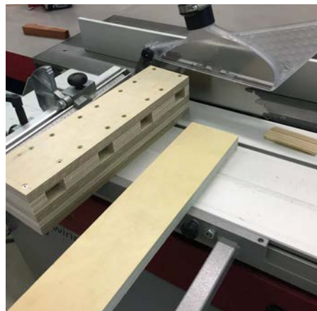
Extension trimmed to length on the tablesaw
