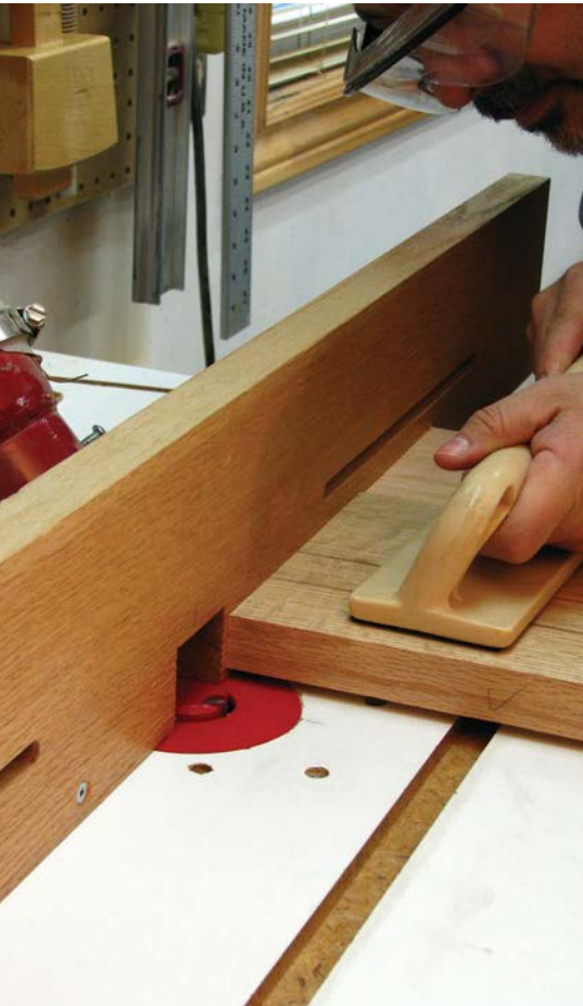
Cut the rebate on the underside of the lid starting with the ends
