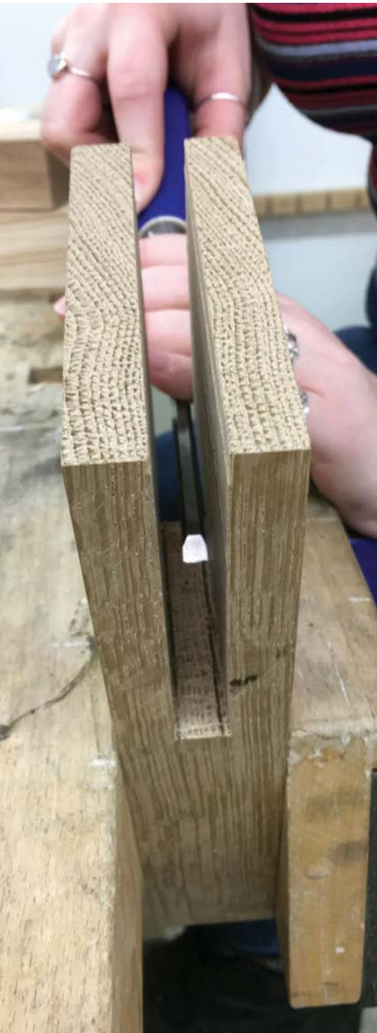
Chiselling to form a gap in a backrest piece
