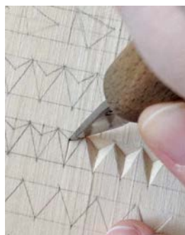
Rotate the board and complete the two remaining stop cuts
