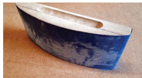
Custom-made sanding block, for final shaping of the inside curve
