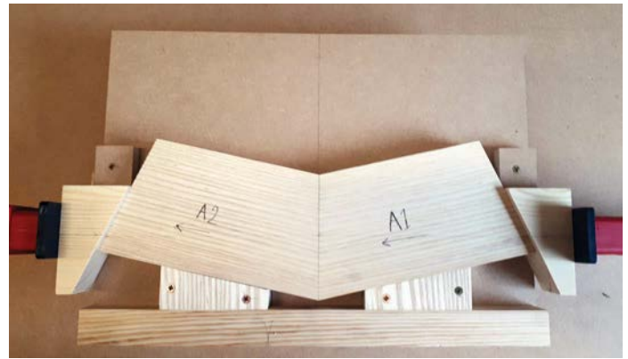
Glueing jig for the initial stage of the glue-up
