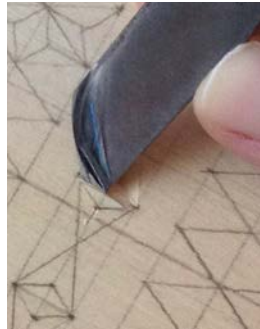
Remove the chip at the base with an angled cut of 45°
