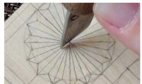
Avoid cutting the stop cuts right up to the centre of the pattern for now
