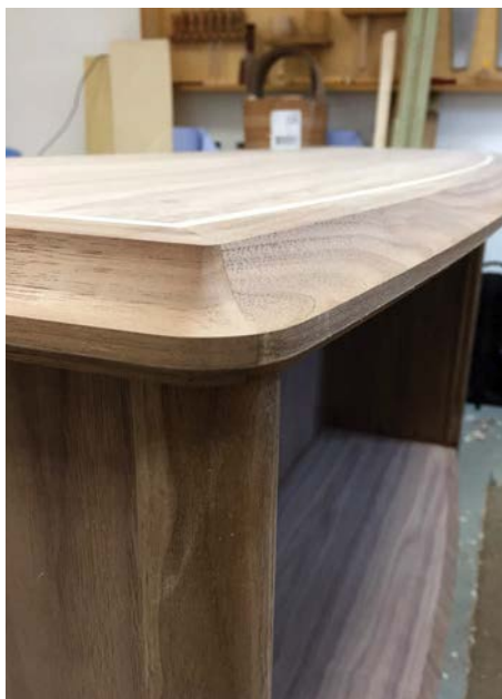
The edge moulding was applied after the inlay was cut and trimmed
