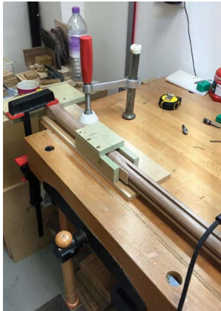
A stop jig was made to create a shoulder at the ends of the flat surfaces machined on the spindle moulder
