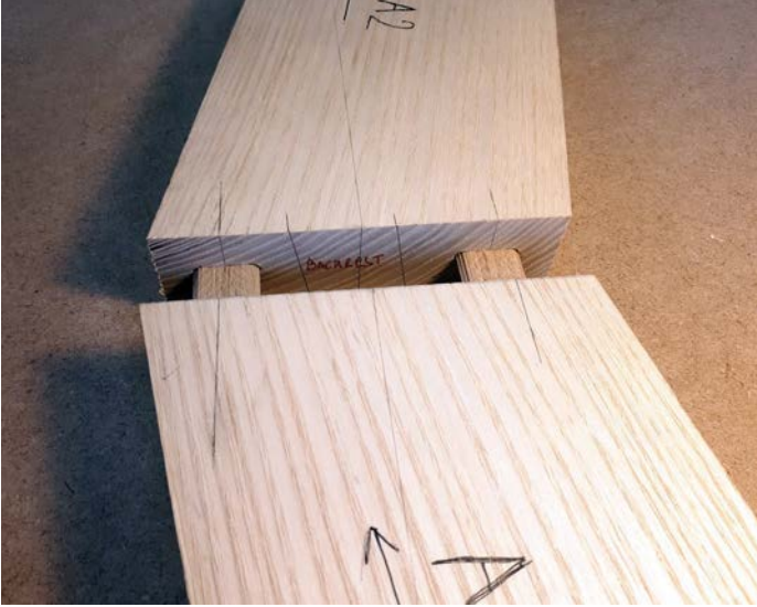
The first sections being glued together – showing the location of the sacrificial Dominoes
