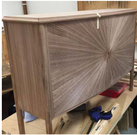
The doors are planed to achieve the smallest gap possible before fitting the SOSS hinges
