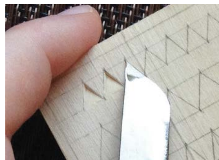
Push the knife towards the intersecting corner of the straight-wall sides to remove the chip
