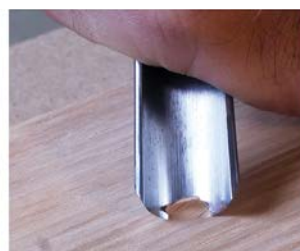
Rotating through the cut, using the full length of the blade. Slicing rather than forcing the cut ensures a cleaner finish
