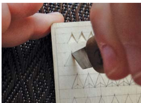
Hold the knife firmly at about 90° to the surface of the board. Then push the knife's tip deep into the wood...
