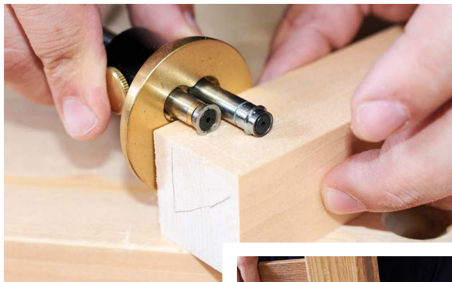
A marking gauge with two cutters makes easy work of marking this joint
