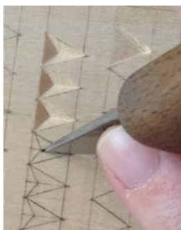
Place the heel of the blade at the top of the triangle and roll towards the centre
