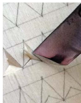
Place the knife at the edge of the triangle at 45° to undercut the first chip
