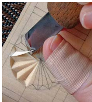
Cutting along the grain away from the centre of the pattern
