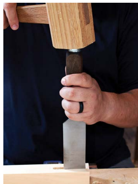
Go as wide as you can to make paring the mortise easier
