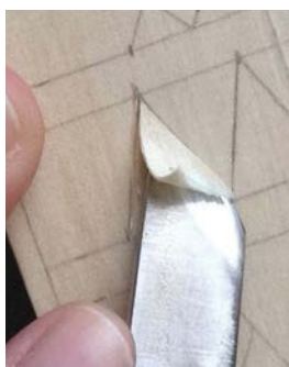
Make stop cuts and remove a regular straight-wall chip
