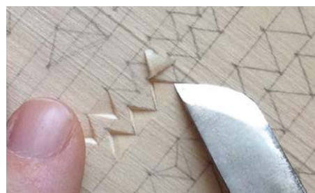
... removing a chip that meets at the top of the triangle
