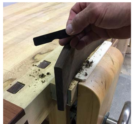
A 'shop-made' scraper removes the machine marks
