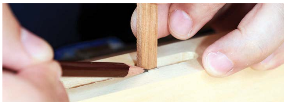
Forget the numbers and determine the depth of the mortise referentially
