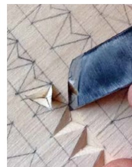
Rotate the board a second time and undercut the third side. The chip will pop out
