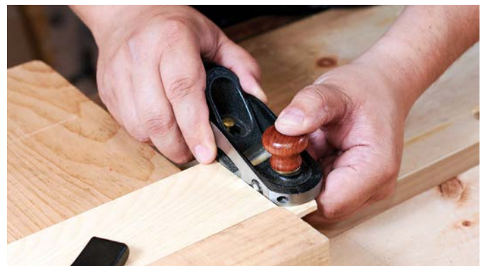
The width of this rebate block plane makes it ideal for thinning down tenons
