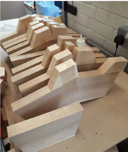
Once glued in pairs, wedges were glued on to give parallel pressure for the second stage of the glue-up
