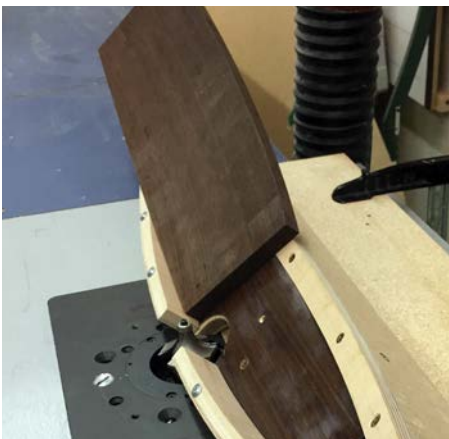
The jig needs plenty of lead-in and out-feed
