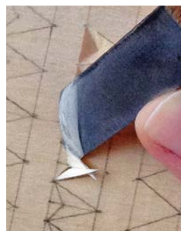
Rotate the board and undercut the second chip
