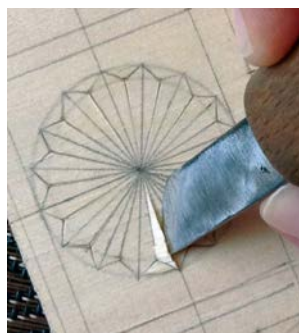
Push the knife deep into the centre of the chip...
