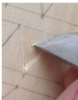
Make two stop cuts from the centre to the base of the triangle
