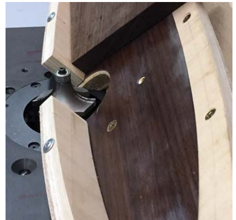
Create an opening in the fence for the router cutter
