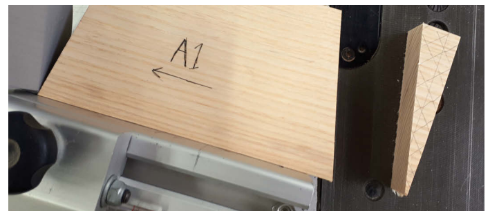
Keeping offcuts from the trapezoidal sections meant I didn't have to remake angled wedges for the glueing jig
