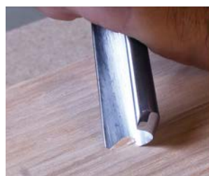
Rotating through the cut, using the full length of the blade. Slicing rather than forcing the cut ensures a cleaner finish
