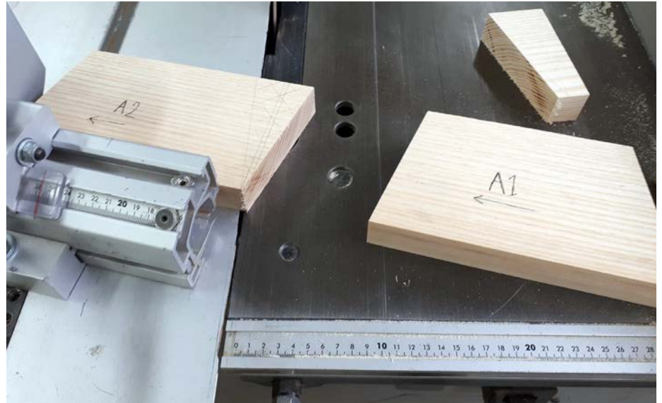
Cutting the angles on the dimension saw, coding each piece as it comes off the saw
