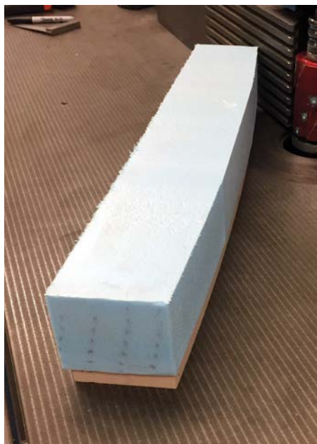
Sections of medium density foam were shaped from templates cut on the CNC using the spindle moulder
