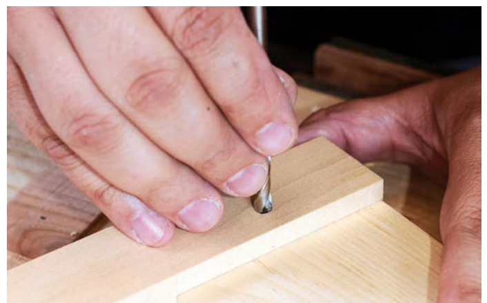
Prick the location of the hole using the drill
