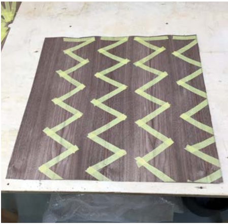
Taping across the joints helps to keep the veneer panel flat before pressing
