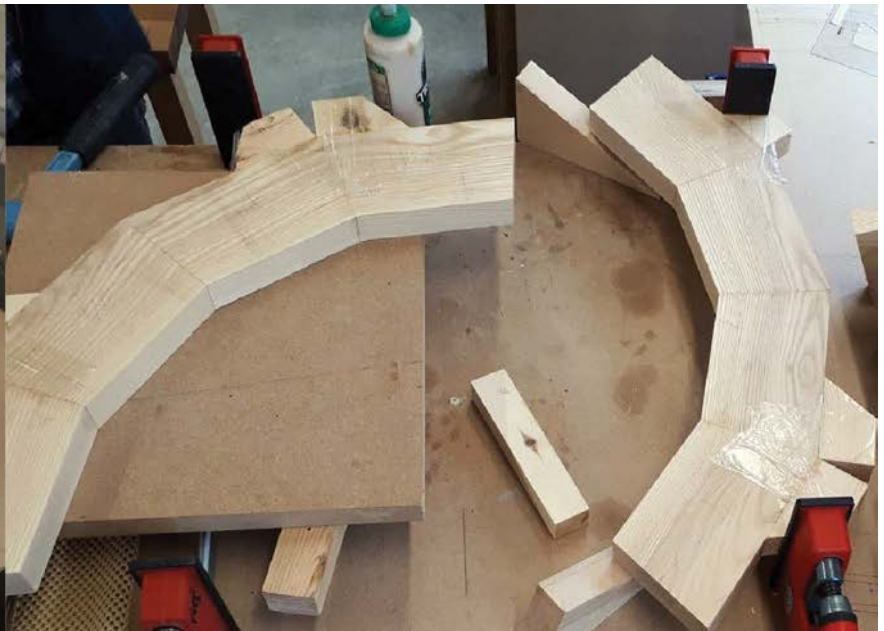
Once glued in pairs, wedges were glued on to give parallel pressure for the second stage of the glue-up
