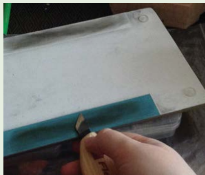
Abrasive strips stuck onto a piece of float glass
