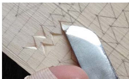
Insert the blade to cut along a straight line...
