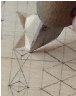
Now complete the two shorter stop cuts
