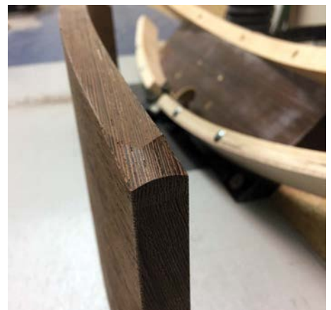
Test cuts on a spare crest rail
