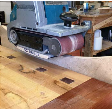
Fairing the curve with the appropriate platen
