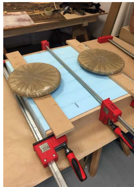
The foam was glued together to make the former for the doors
