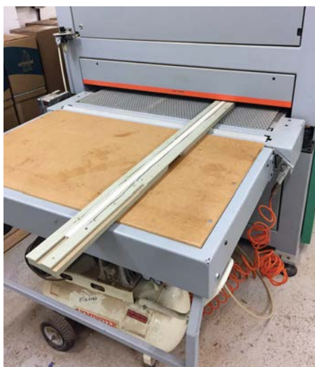
A carrier was used to hold the maple strips of inlay as they were passed through the calibrating sander
