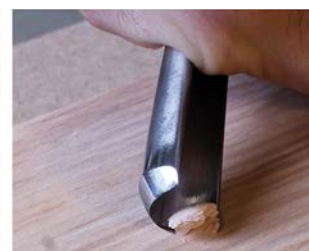
Rotating through the cut, using the full length of the blade. Slicing rather than forcing the cut ensures a cleaner finish
