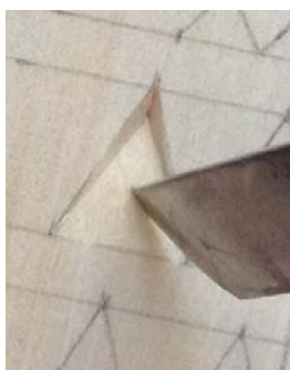
Place the tip of the knife in the centre of the big chip area
