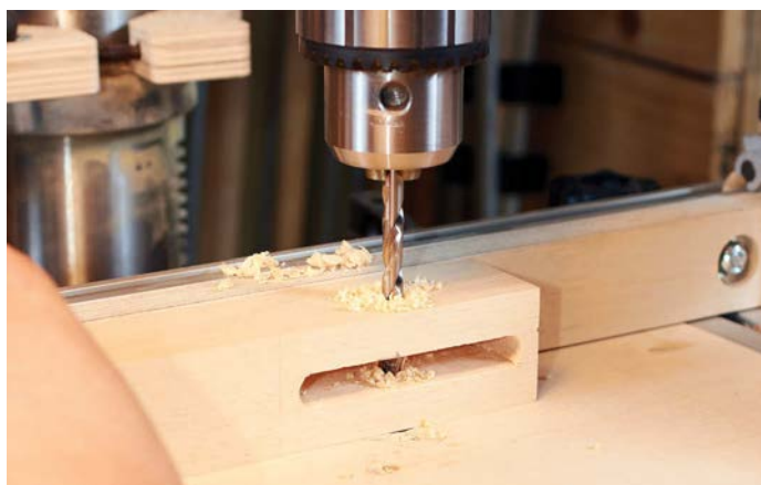
The drill press allows you to not worry about whether the holes are plumb
