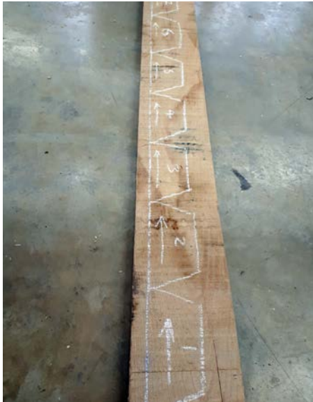
Marking out the trapezoidal sections on each board for grain continuity around the backrest
