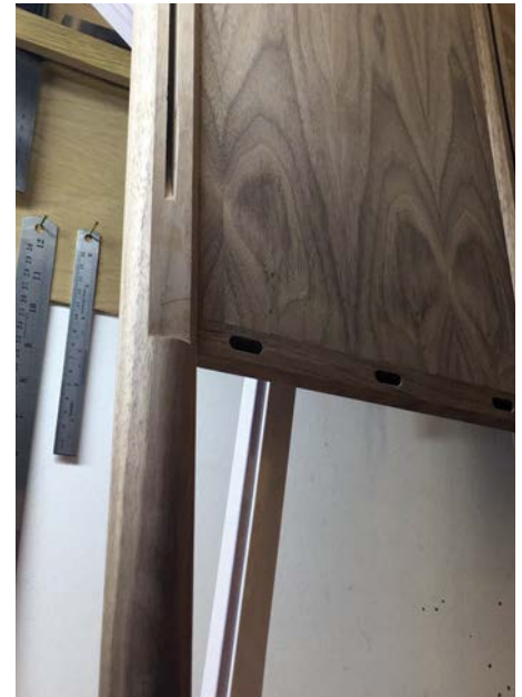
The shoulders line up with the bottom of the sides and back
