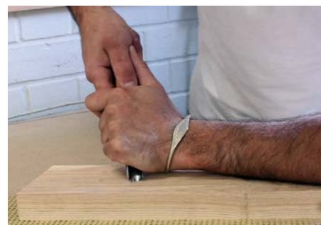
Carving grip, where the left (weaker) hand acts as a brake ensuring control in the cut when carving
