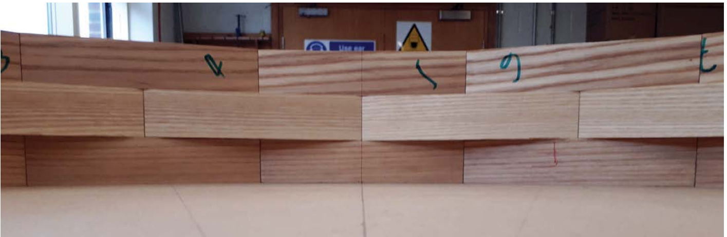
Carefully aligning the glue lines of each layer
