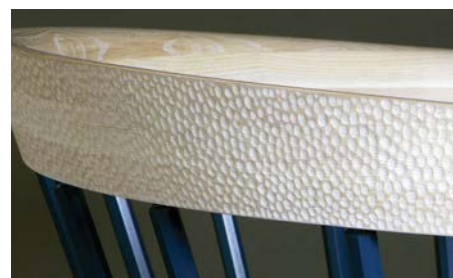
INSET: Approaching each cut at the correct angle, using the bevel to burnish the cut LEFT: The finished carved surface of the seat RIGHT: The completed stack laminated, coopered backrest with hand-carved dimpled texture
