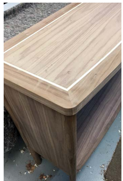
The inlay was placed where the lippings attach to the top
