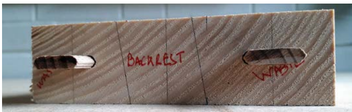
Location of Dominoes, staying well clear of where the backrest will be after shaping
