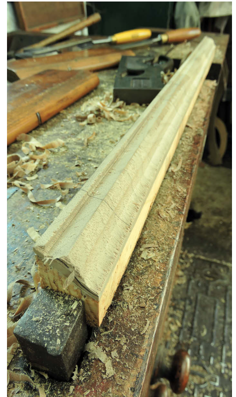
A shoulder plane is used to define the square edges
