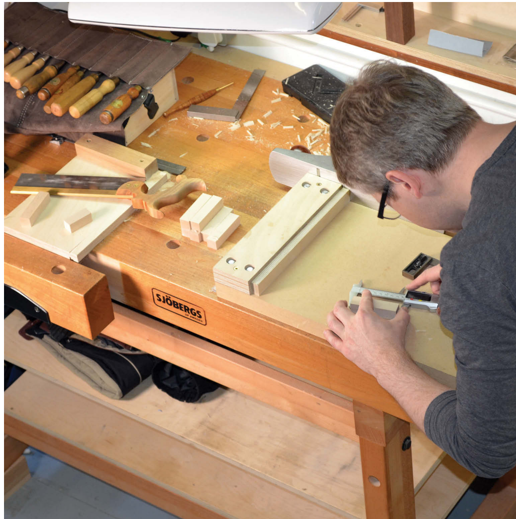
Shooting board in use squaring end of 20mm component
