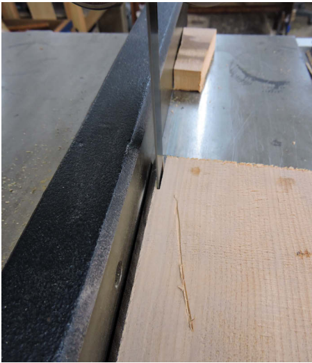
The moulding is cut from the mother board with a small amount of substrate for support
