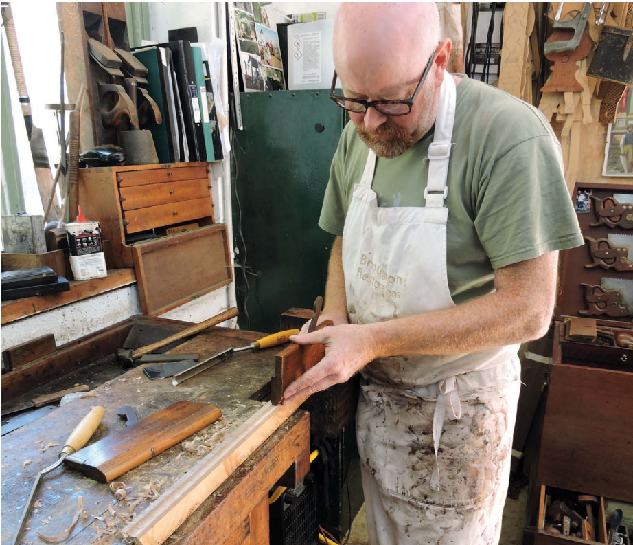
Moulding planes are used to create the profile
