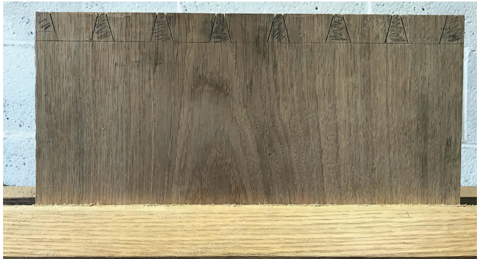
Cutting the dovetails – you can see the half pin on the far left
