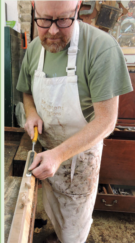
Pattern maker's gouges are perfect for shaping without tear-out
