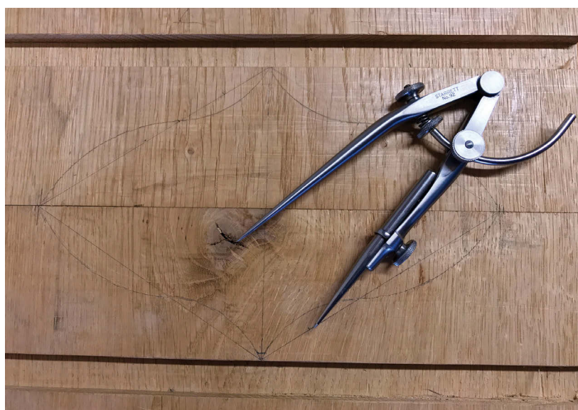
Laying out the foot detail – here you can see the triangular layout lines as well as the cyma reversa
