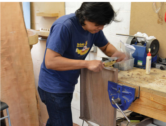
Shaving the handle to fit the frame
