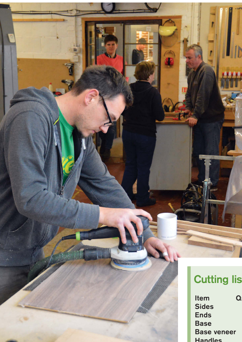
Working through the grits with a random orbital sander
