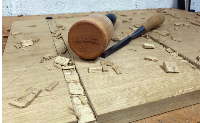
Once the dados are cut, knock out the waste with a chisel and mallet before cleaning up with a router plane
