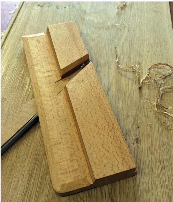
A beading plane adds subtle but effective decoration to the tongue-and-groove joints on the backboards
