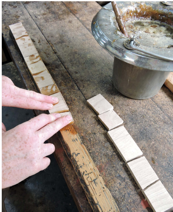
The show wood is glued to the substrate
