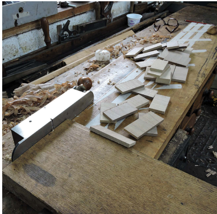
The blanks may be trimmed to length with a mitre plane on a shooting board...
