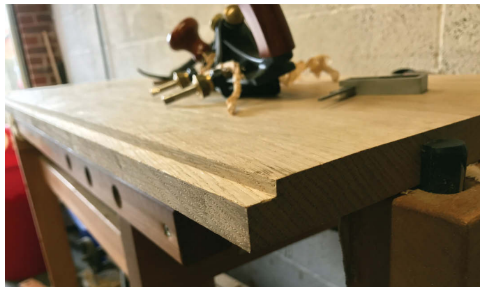
The rebate along the inner rear edge of the top. A moving fillister plane makes easy work of this
