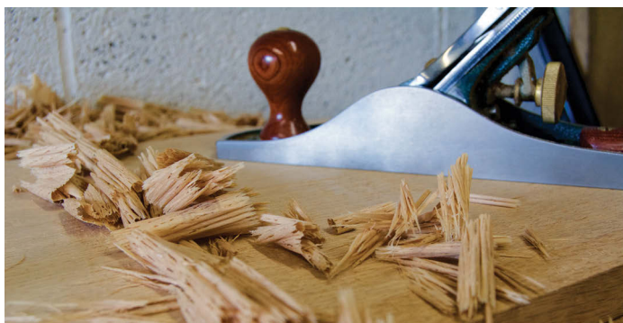
Processing the rough boards with a No.5 plane – traversing the board allows you to take a heavier cut for quicker stock removal
