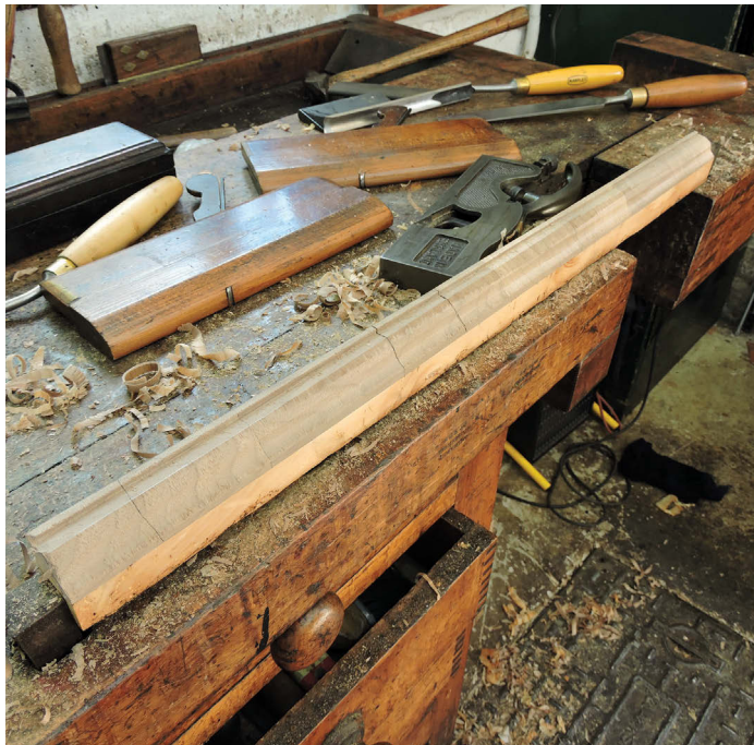
Traditional hand tools are the best way to create authentic cross-grain moulding
