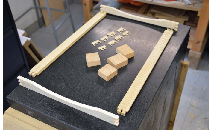
Glue blocks and spacers are cut in advance to ensure the glue-up runs smoothly
