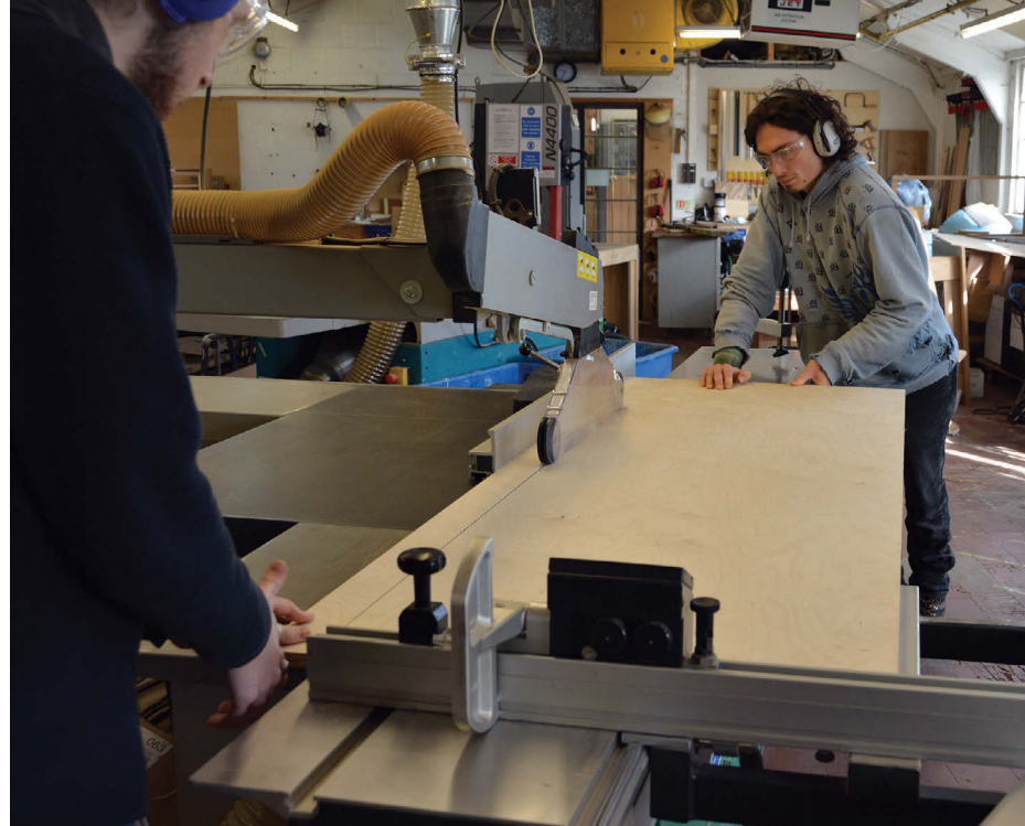
Ripping up a plywood sheet to make the tray base
