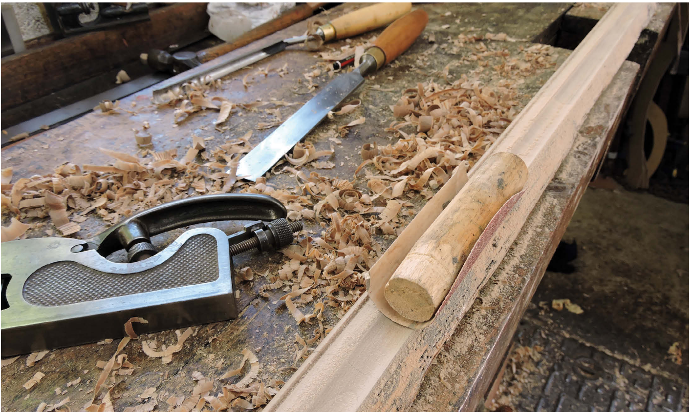
Varying diameters of dowl wrapped with abrasive help to blend the curves
