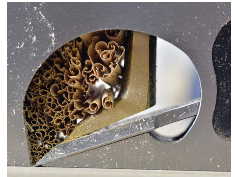
A small shoulder plane is useful for fine tuning the fit of the shelves to the dados
