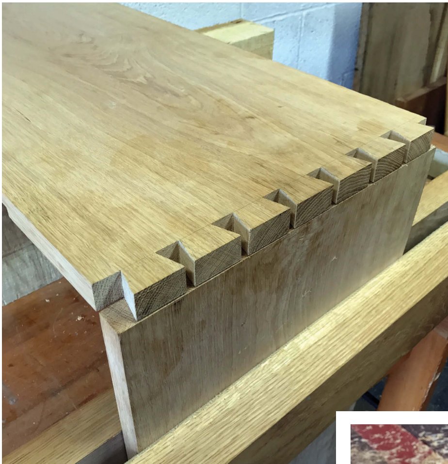
With the tails cut, it is time to lay out the pin board
