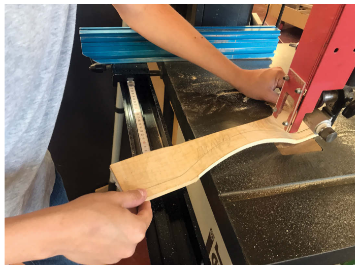
Roughing out the shape of the handle on the bandsaw
