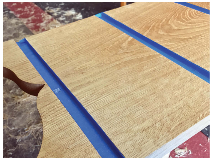
A small shoulder plane is useful for fine tuning the fit of the shelves to the dados
