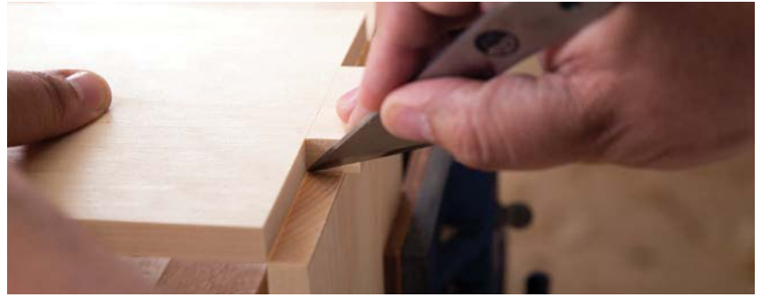
Use a sharp knife like this blacksmith-made kiridashi to transfer the first half of the joint to the mating board
