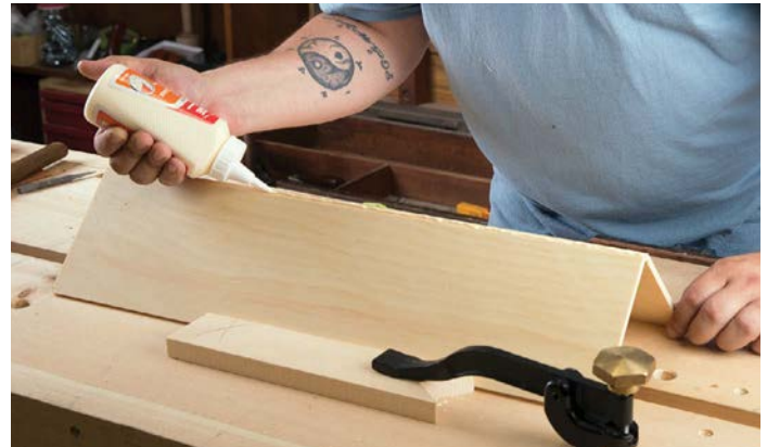
A narrow bead of glue is all you need to create a seamless top joint
