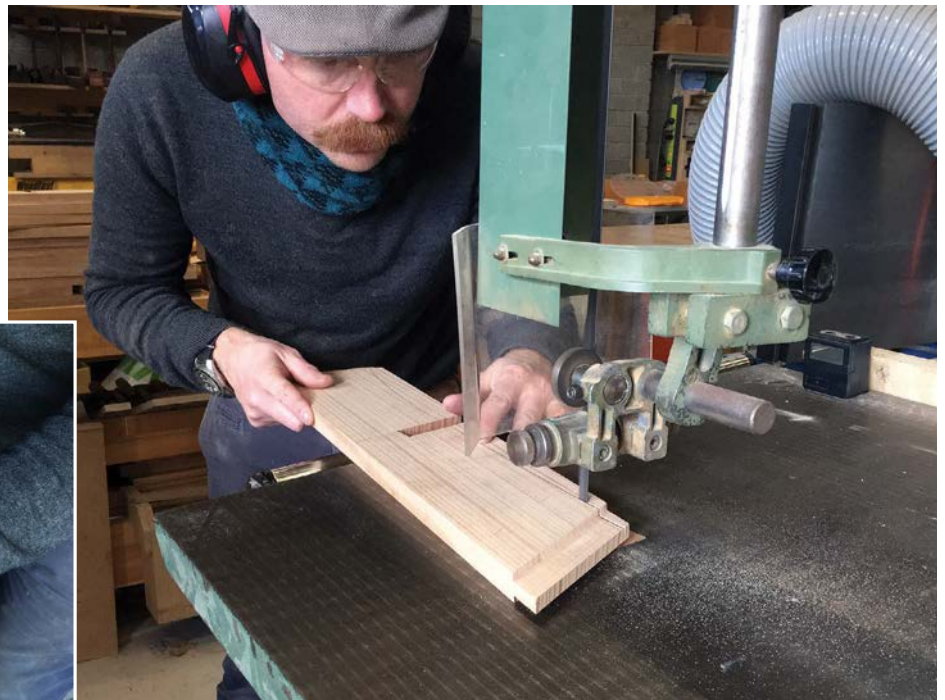
ABOVE: The bandsaw table angled to match the half-lap LEFT: Cleaning up bandsaw marks with spokeshaves
