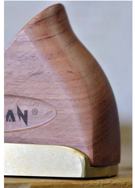
The rear infill is plagued with sharp corners and hard transitions, which make it uncomfortable when using the plane in an upright position
