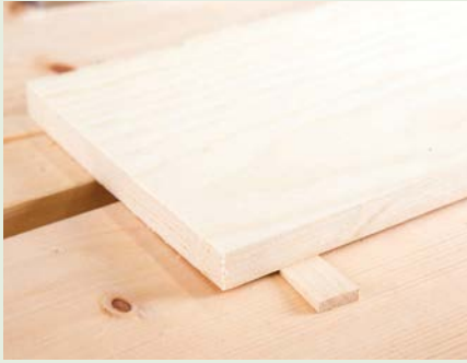
Wedges will keep the boards from rocking as you work
