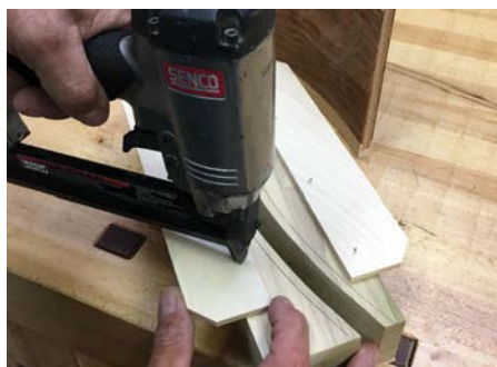
5. Attach some support wings
