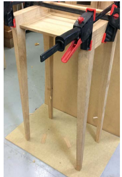
Tapered legs and dust panel dry clamped and awaiting the fitting of the stretcher
