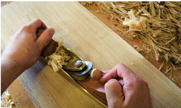
The rear infill creates an awkward grip when using the plane upright. The front bun is much more comfortable in this position
