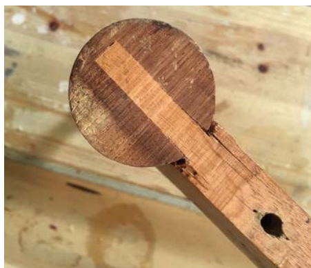
Not much material left at the end of the tenon
