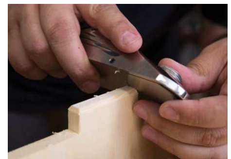
Keep it between the lines to create those delicate chamfers
