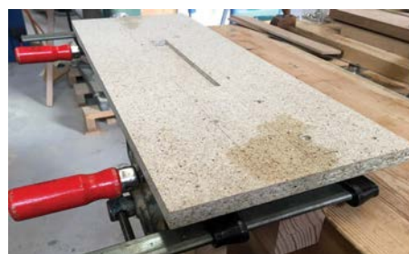
Jig fences clamped in position
