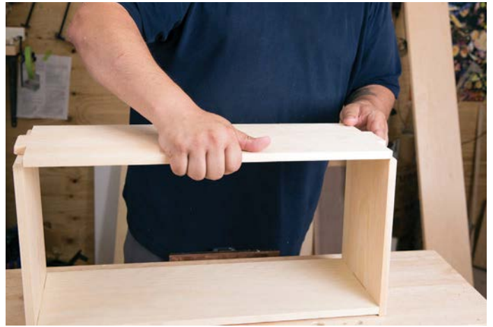
The last board to go in will slide into the two end pieces
