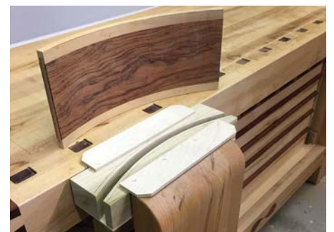
6. Drop the jig into the vice and you're ready to clamp
