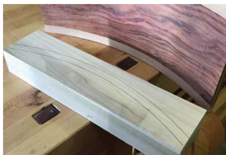
2. Trace the shape onto the block
