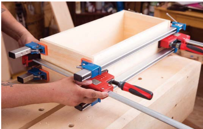
Put a clamp across each set of fingers for a solid glue-up
