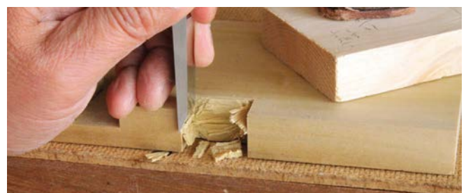
Work on the two cross-grain walls first, chopping from both faces
