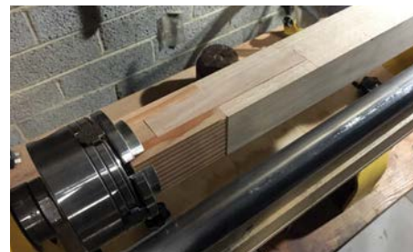
Lathe jig with leg in position
