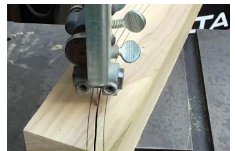
3. Cut between the lines
