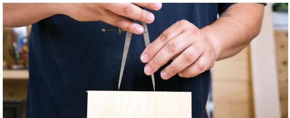
The humble divider once again takes the maths out of woodworking
