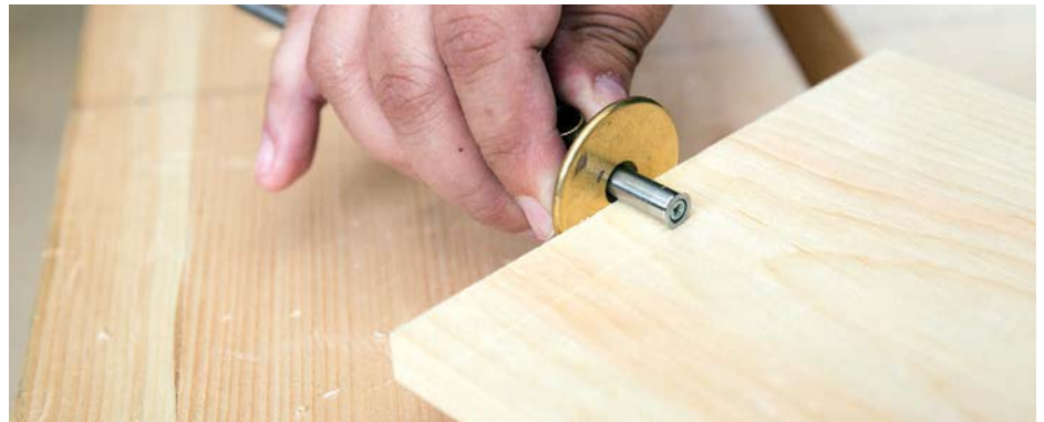
Mark the depth of your fingers using a wheel marking gauge
