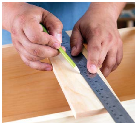
With careful layout, taking the wedge and the locking batten out of one board will almost guarantee a great fit
