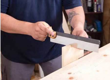
Saw as straight as you can because this half of the joint becomes the pattern for the other half
