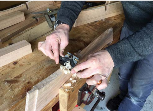
ABOVE: The bandsaw table angled to match the half-lap LEFT: Cleaning up bandsaw marks with spokeshaves
