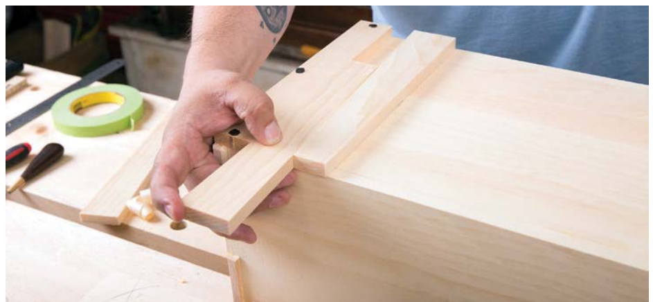
With careful layout, taking the wedge and the locking batten out of one board will almost guarantee a great fit
