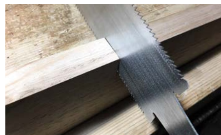
Ryoba saw cutting almost to the line
