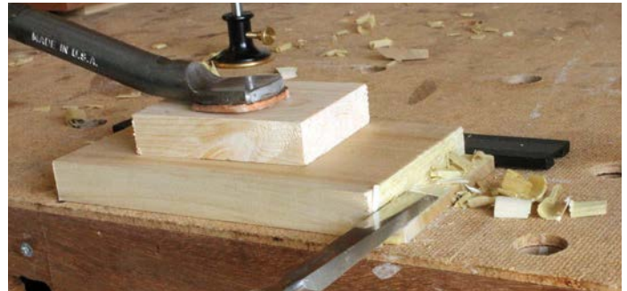
Trim the depth of a rebate freehand, or use a block that matches the rebate lip as a guide
