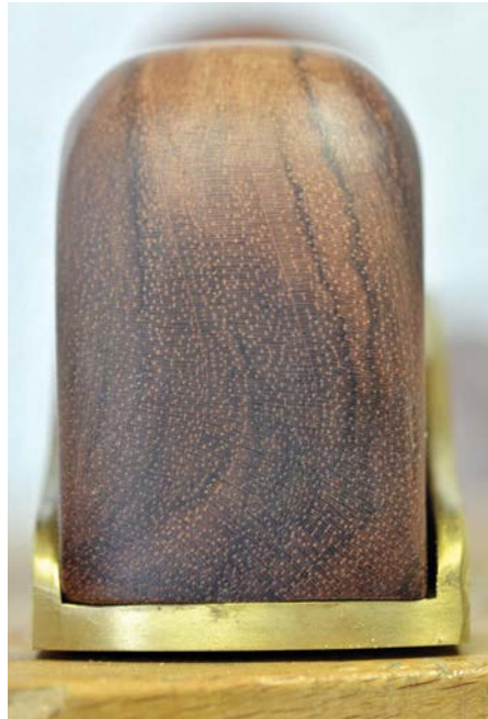
Both infills are fitted to just one side of the plane body, with a small expansion gap on the other side
