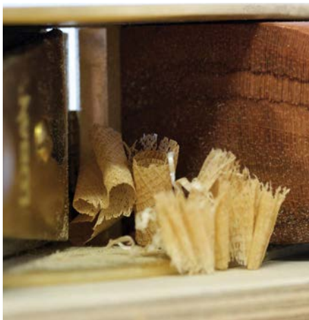
The No.22 takes fine end grain shavings, leaving a clean surface
