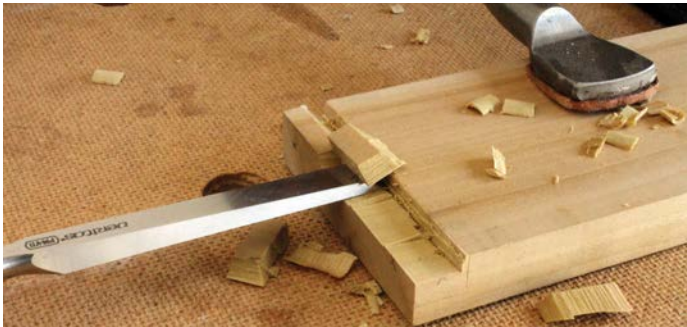
Watch the grain when paring at the end to avoid removing wood beyond the baseline
