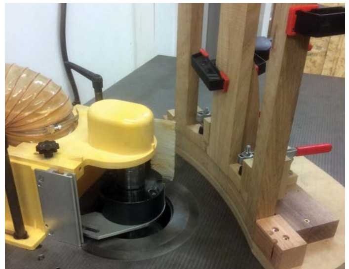
Jig holding doors ready to be shaped on the spindle moulder with rebate block and ring fence
