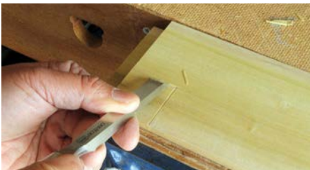
To prevent lifting up the fibre, cut the knife walls across the grain first
