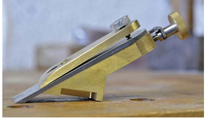
Together the thick cap iron and frog clamp the iron tight and prevent chatter
