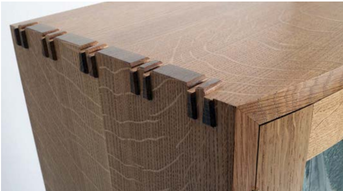
Hand-cut protruding through dovetails with chamfered edges: a key feature of the cabinet's design
