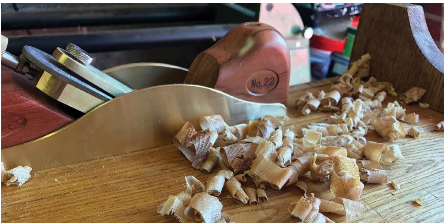
Trimming the end grain of backboards on a large carcass
