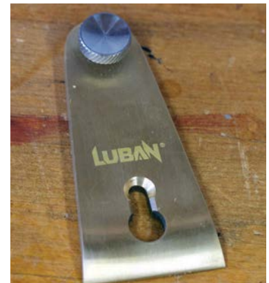
The cap iron is a substantial block of bronze which works well to minimise chatter
