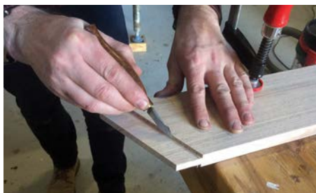
Knife run along the shoulder
