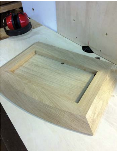
Curved and chamfered plinth with recess for the LED lights' electrical junction box and transformer
