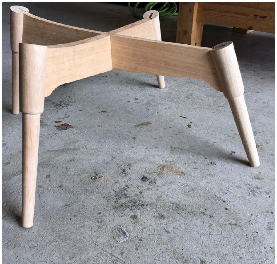
Rail curves after being cut and tidied
