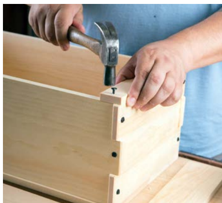
These fixed battens are what keep the top captured, securing your tools
