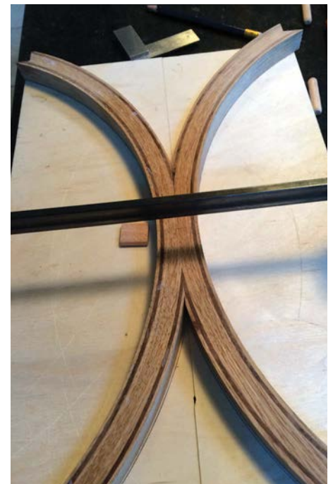
Completed curved stretcher in laminated oak and walnut on top of the plywood template
