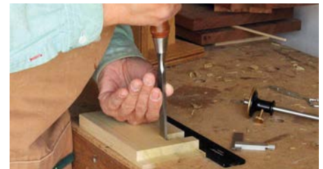
Pare down on the scribed line to remove the last bit of waste
