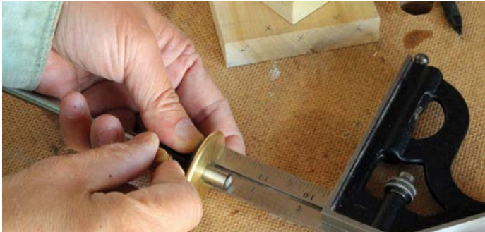
Using a trick attributed to woodworker Chris Schwarz, I set the marking gauge by placing its cutter into the engraved line on a ruler
