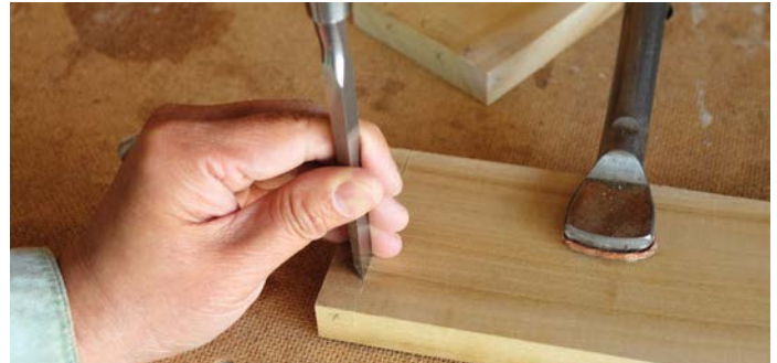
You may also scribe a second line on the waste side from the shoulder line to guide your initial chopping
