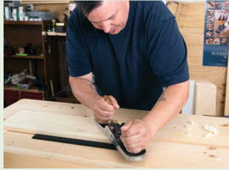
Start by working across the grain to get boards flattened by hand
