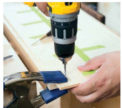
Go easy when you are driving in these small screws. One slip of the trigger finger and you'll sink them in too deep
