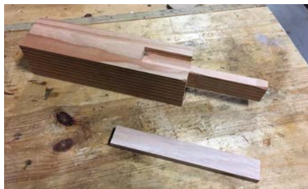
Lathe work-holding jig with sacrificial insert
