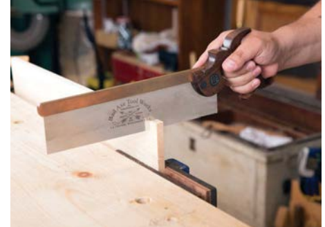
The shoulders need to be right on the line. If necessary, pare to the line after sawing
