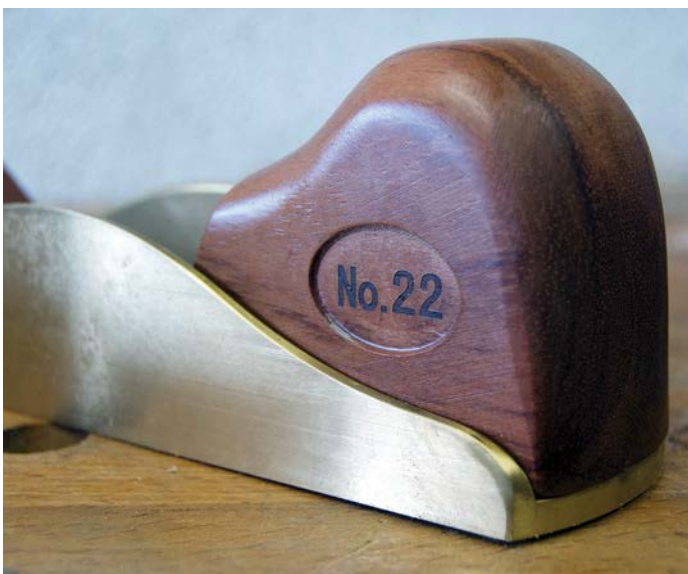
The front infill is nicely fitted, and curved to support the hand
