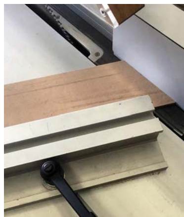
The angled tenon shoulders cut on the saw
