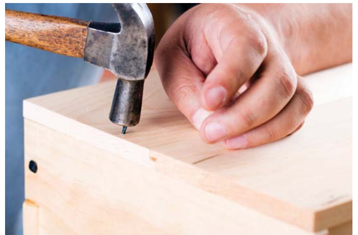
Angle the nails in to give them more holding power
