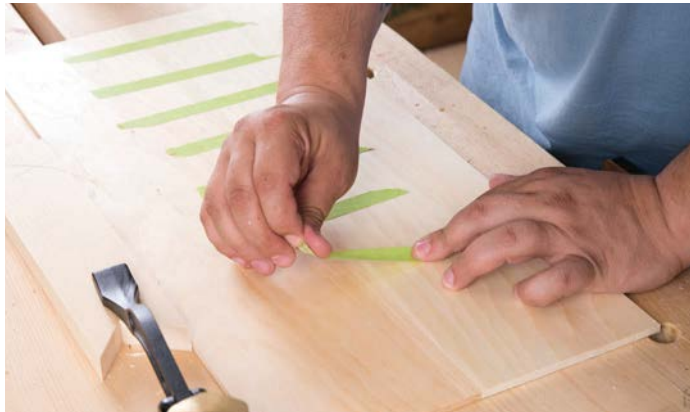
Binding tape is used extensively by guitar makers and there is lots of use for it when making furniture
