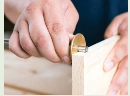
If you are thicknessing by hand, strike a line for your final depth and work towards that line
