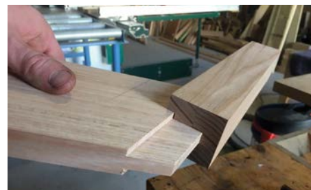
Test fit of housing and mortise
