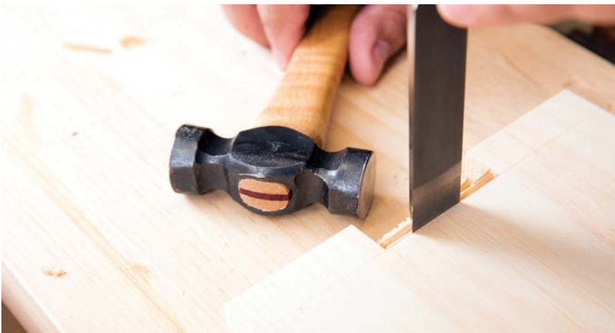
Remove the waste slowly. Rushing this step could lead to blowing past your knife line
