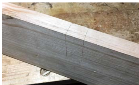
Half-lap knife lines marked out
