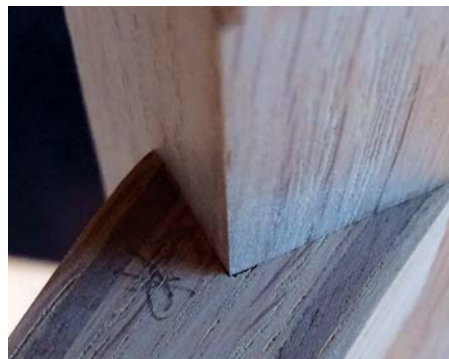
Bird's mouth joint between stretcher and tapered leg
