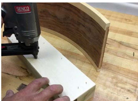
4. Fix the cauls to a flexible base board
