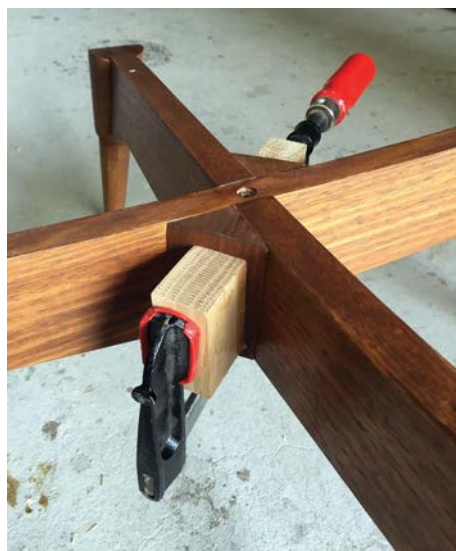
Corner blocks glued and clamped
