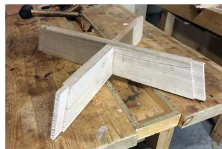
The half-lap joint cut, pared and test fitted
