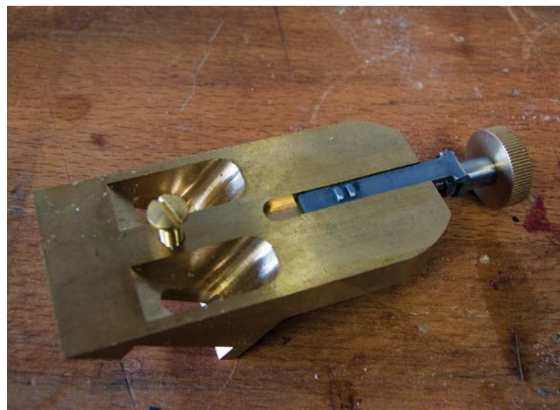
The frog is also very solidly made, supporting the blade even in heavy cuts
