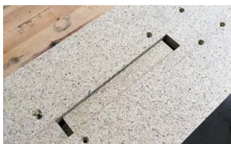
The centring jig locating in the router jig slot
