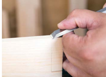
Making a knife wall is a great way to ensure you are sawing in the right spot
