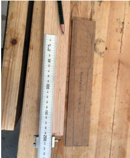
LEFT: Marking out the legs ABOVE: Leg blanks, mortises drilled out RIGHT: Routing the rail shoulder housing
