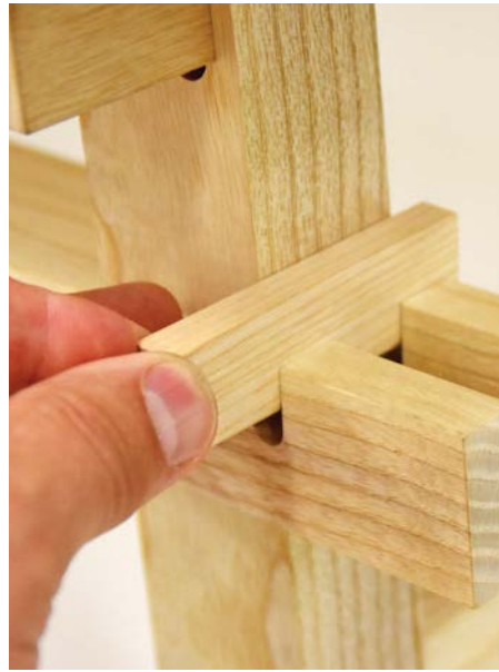
Avian Evans-White's Work Space range is designed for disassembly and eliminates the use of non-recyclable consumables by incorporating wedges and sliding dovetail joinery
