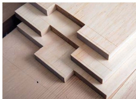
Mark out the small chamfers that will adorn the protruding fingers
