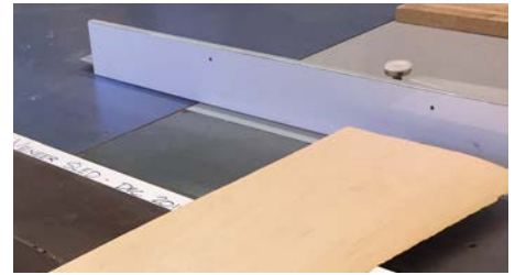
5. Move your fence so it does not interfere with the path of the veneer when cross cutting
