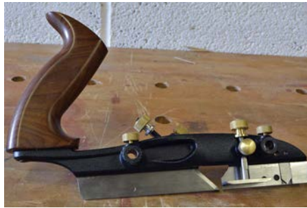
The main body holds the plane irons, and is fitted with a roasted maple tote, depth stop and cutting spurs
