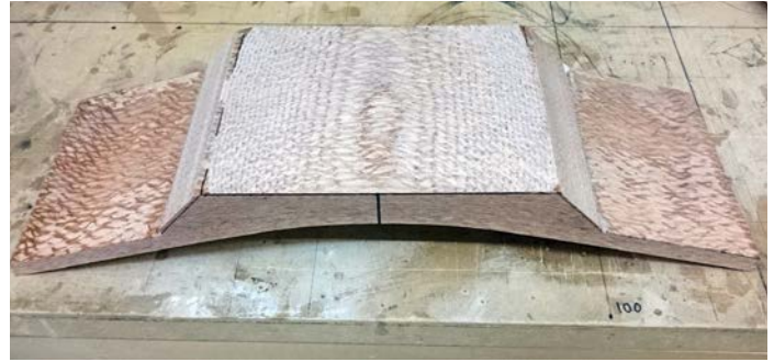
Creating a perfectly flat area at the crown of the laminated piece was essential to ensure a clean joint
