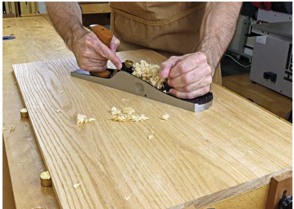
Start flattening the panel by planing diagonally across the grain
