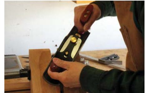
With the stock pinched in the mitre jig, I trimmed the mitre with a precise finish cut
