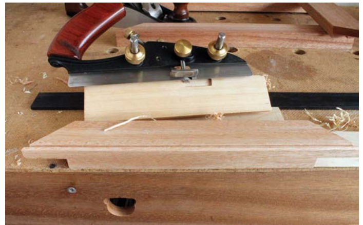
I used a back-bevelled cutter so I could bead against the grain without tear-out concerns
