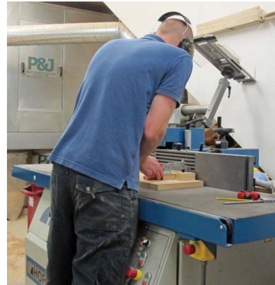
Head tutor Graham Loveridge using the spindle moulder to apply the taper to the legs of the occasional table
