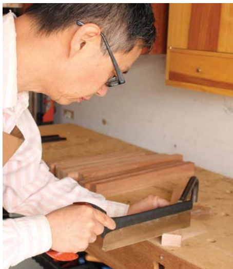
Butt the sawblade against the chiselled groove and saw down to the centreline
