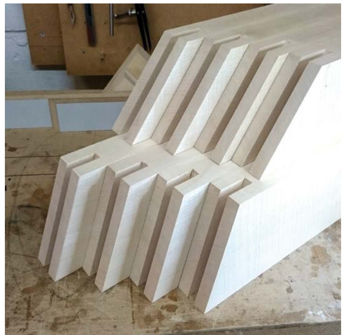
The router approach created clean, parallel and square-bottomed slots
