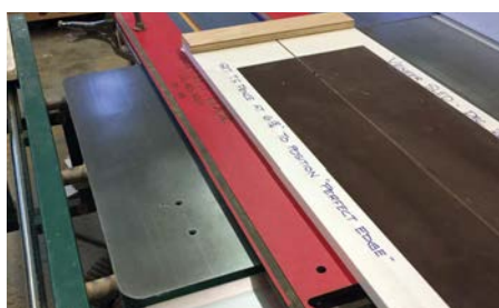
3. Ensure you have sufficient length in the sled to accommodate a wide range of veneers
