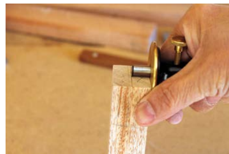
Use the 'thickness gauge' to scribe the centreline around the end and both edges
