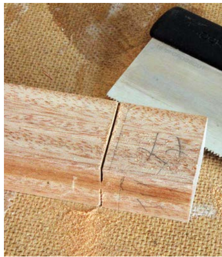
Chisel a sloping groove on the shoulder line as a saw guide and saw down the line
