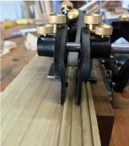
ABOVE: When cutting reeding, the sliding section is positioned so that its skate runs in the groove of the reed RIGHT: Mirror image – fluting and a bead, both cut with the Combination Plane
