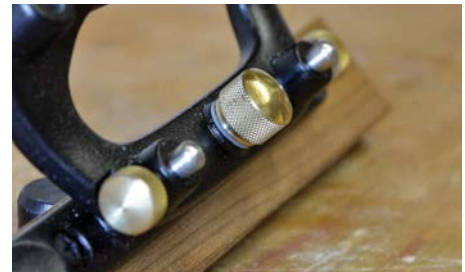
The micro-adjust mechanism allows the fence to be set with real precision
