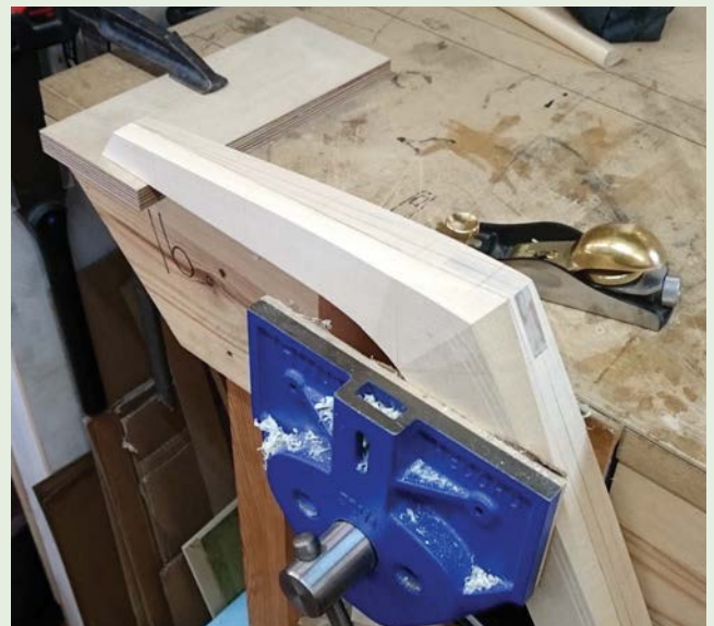
Extra support for the odd-shaped workpiece helped a great deal in keeping it stable while shaping
