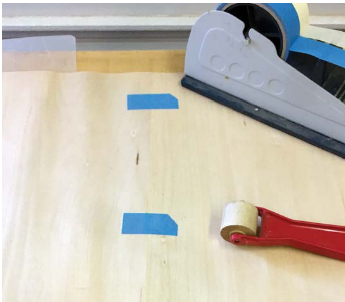
9. Roll the tape to ensure good contact
