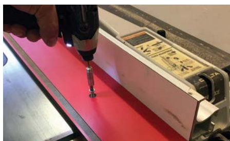
1. Fix a suitable straightedge in place with a machine screw directly into the saw table-top
