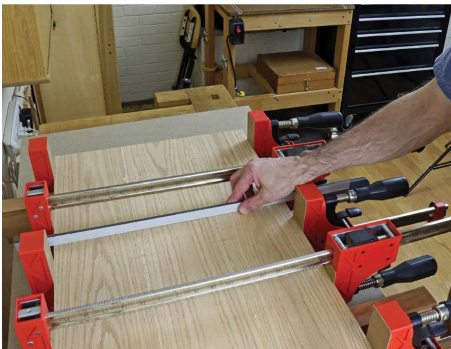
Check with a straightedge to ensure balanced clamping forces
