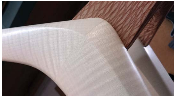
The smoothed-out form of the finished joint
