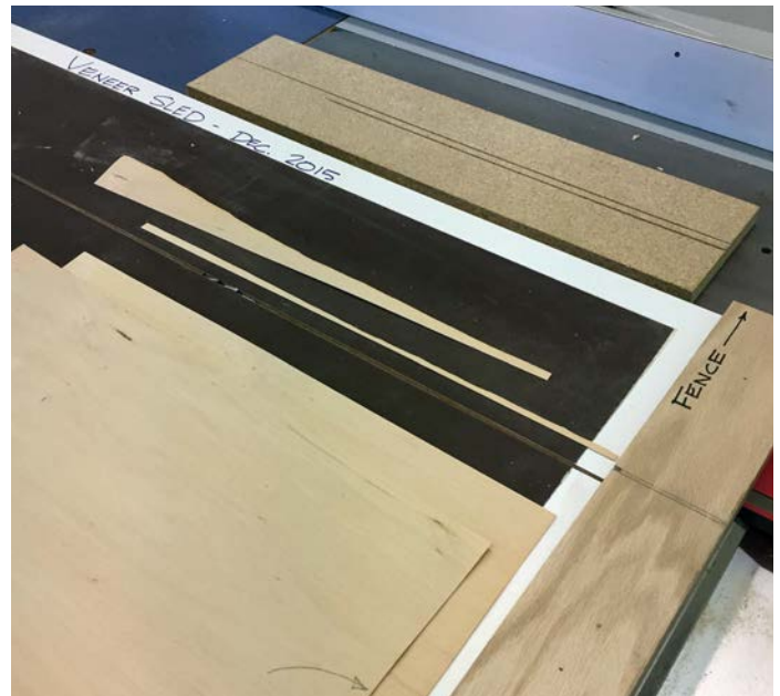
8. Adjust the height of the blade to accommodate a thicker stack of veneer
