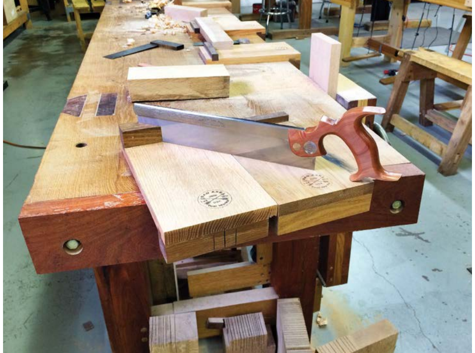
A dovetail saw is often the first back saw in a collection but it doesn't have to be that way
