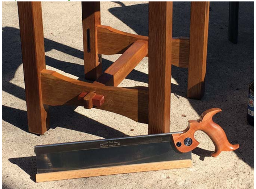
Hybrid tooth geometry will handle everything from cross cutting shoulders to ripping tenon cheeks
