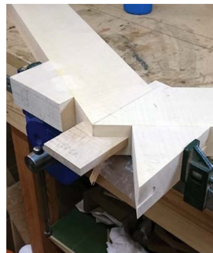
Offcuts from the earlier mitres were glued on to provide clamping locations for glue-up. Sacrificial dummy tenons were also used for alignment and mechanical support
