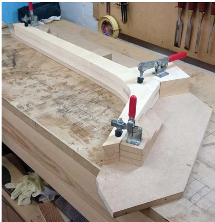
A template jig was used to rout the internal curves on the legs
