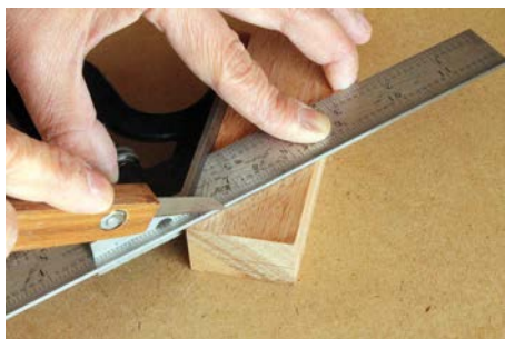
Start with a light stroke, then two heavier strokes, to avoid the first cut following the grain line
