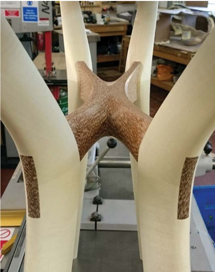
The tenon ends were blended in with the legs
