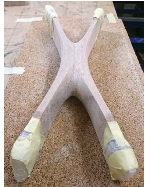
The curves of the cross-brace were hand-shaped with a spokeshave, rasps, files and sanding blocks
