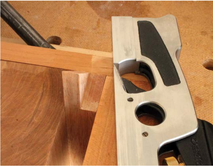
The mitre shooting block is also ideal for trimming or squaring the shoulders
