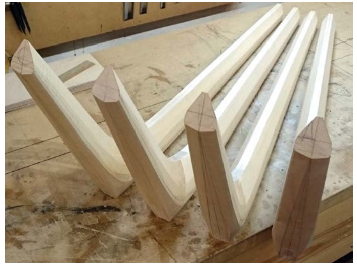
The smooth curve of the inside of the leg was initially formed of several flat facets, later blended together
