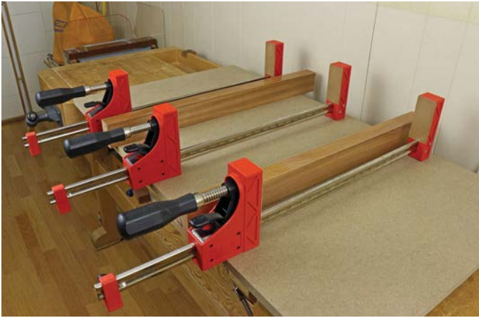
Supports and lower gang of clamps ready to accept the boards
