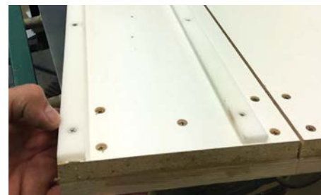
2. Use UHMW strips to guide the sled between the rails
