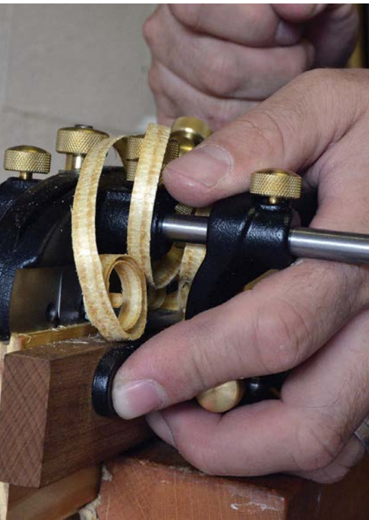
The dominant hand pushes the plane, while the off-hand holds the fence against the workpiece. The fence can be moved to the other side of the plane for left-handed users
