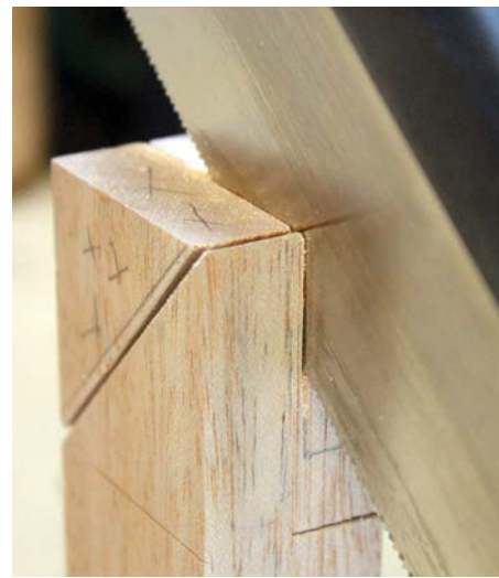
After sawing from corner to corner, I finished the cut with horizontal strokes
