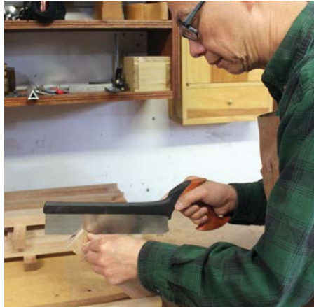
Avoid sawing down two scribed lines at a time or sawing to a line that is out of sight
