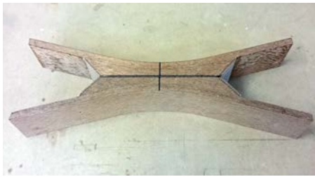
The laminated piece was split in half lengthways and bookmatched to form the 'x' shape of the cross-brace
