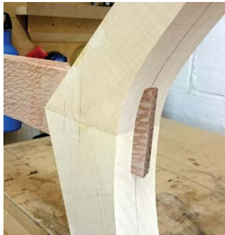
Ensuring the tenon sections of the cross-brace were flat and parallel was key to getting clean join lines
