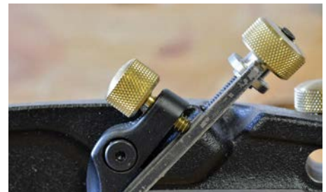
The blade clamping mechanism holds plane irons firmly and allows for precise adjustments to the depth of cut
