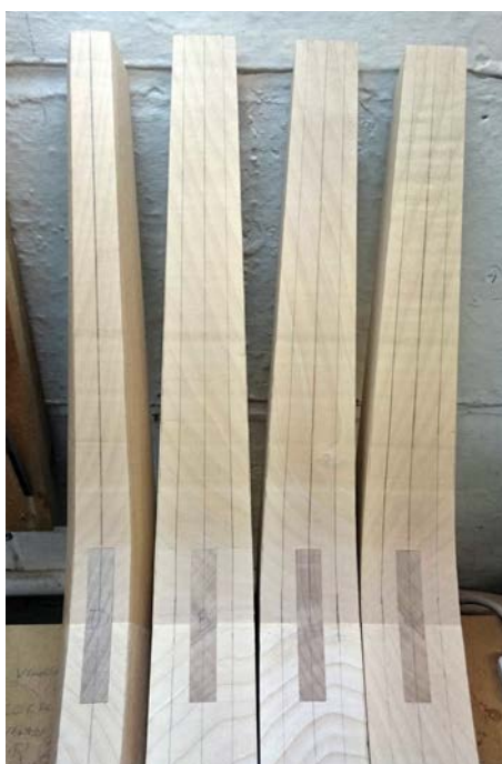
Areas to be shaped were marked out step-by-step, with each step being completed on each leg before moving on
