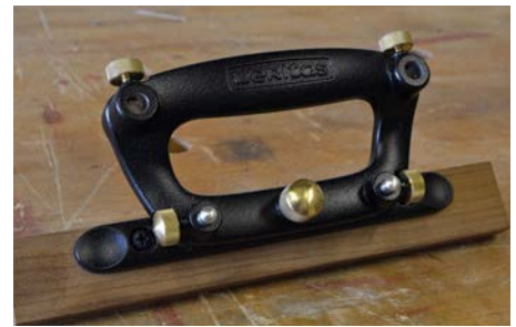
The fence comes fitted with a roasted maple auxiliary fence as standard, which provides a large surface area to register against the workpiece
