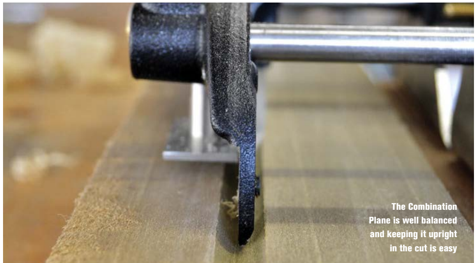
When cutting flutes the sliding section is moved away from the plane iron
