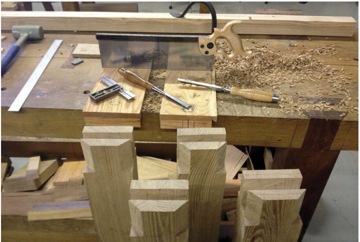
Select a tenon saw for the largest joints you expect to cut
