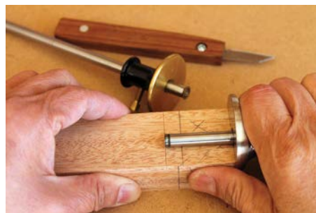
Hold the 'width gauge' tight against the end to scribe the shoulder line
