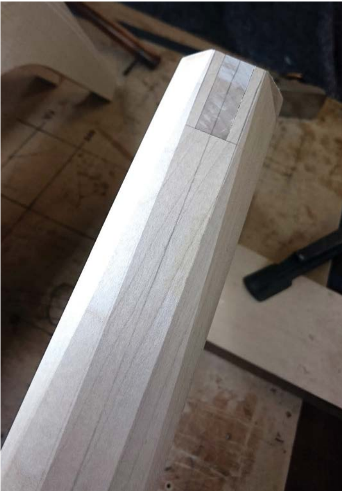
Using a block plane wherever possible allowed for close control over the facets and edges being shaped
