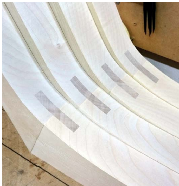
The dummy tenons remained in place throughout the shaping process to provide structural support and minimise risk of damage to the mortise edges
