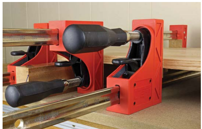
Note that the top face of the panel is about the same distance from the bar of the upper clamp as the bottom face is from the bar of the lower clamp
