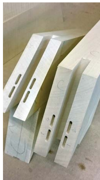
Small Dominoes were used to bolster the end grain joint
