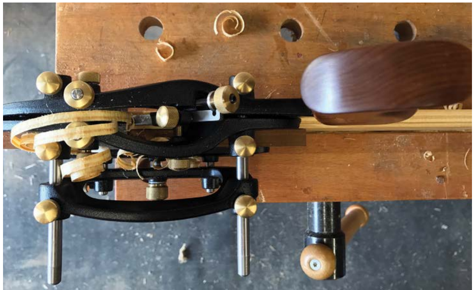
When cutting flutes the sliding section is moved away from the plane iron
