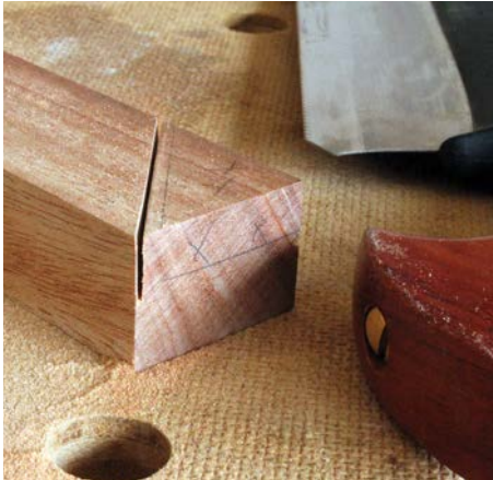
If you need some sawing warm-up, start with the half lap, which is simpler than the tongue to cut
