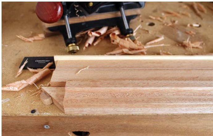
A through rebate was planed on the rails, while a stopped rebate was cut on the stiles
