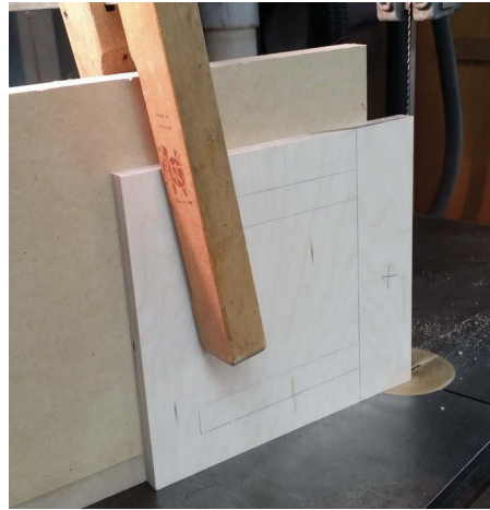
Sawing close to the bevel line
