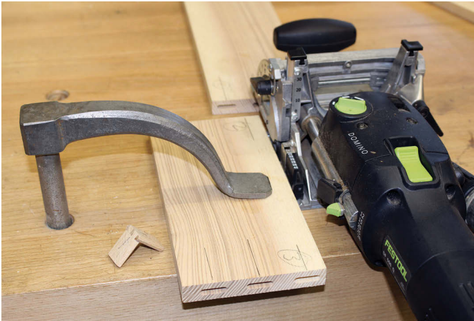
Domino slots being cut before mitring the corners
