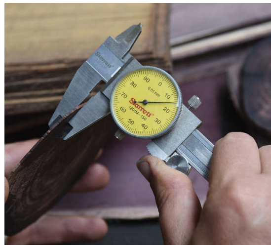
A uniform thickness in excess of 1mm means you can approach finishing in the same way as working with solid timber
