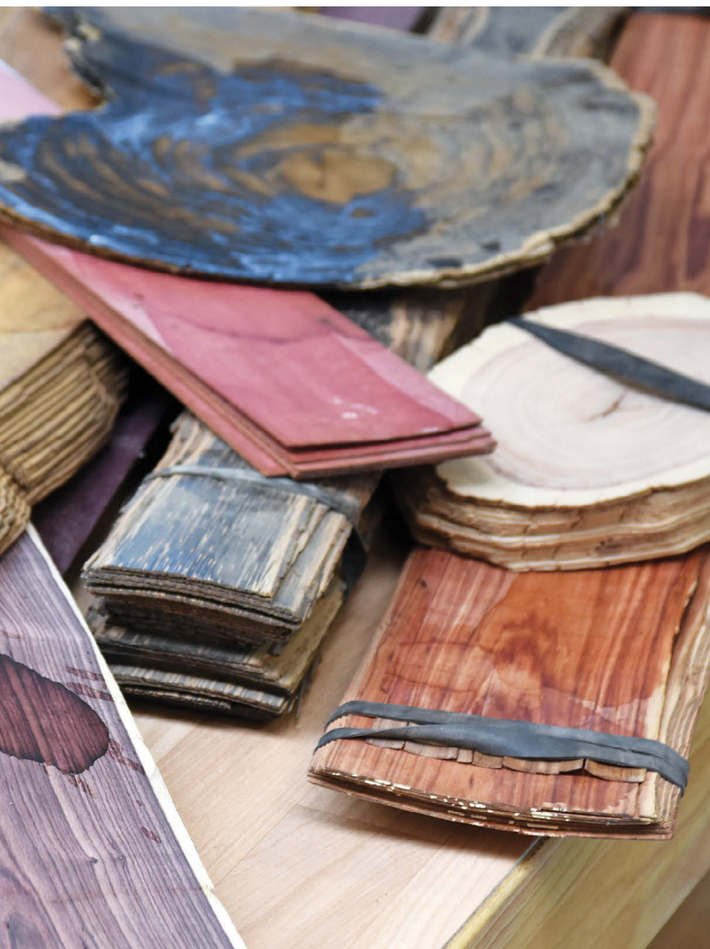
Sawing timber into veneer preserves the natural colour of the wood
