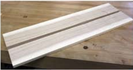
50mm-thick board of olive ash resawn on the bandsaw
