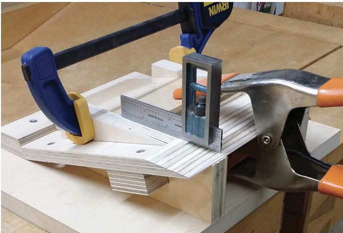
Checking that the sides and bevel are co-planar
