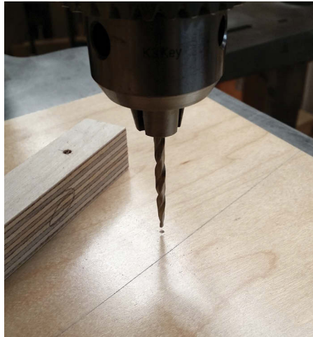
Drilling into dimple with tapered bit
