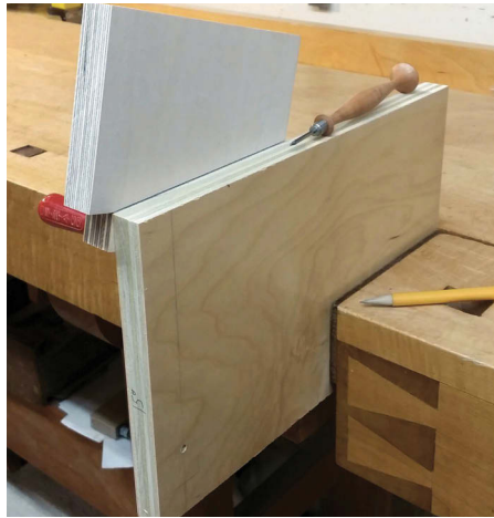
Marking side pieces to be bandsawn
