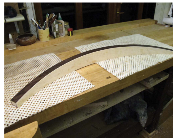
Apron half lipped in rosewood and ripple sycamore
