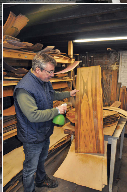
Frederic George wets the surface of the veneer to reveal the true colour
