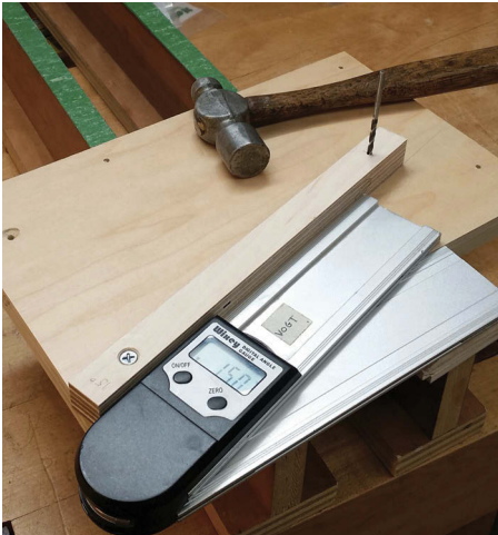
Setting the precise angle
