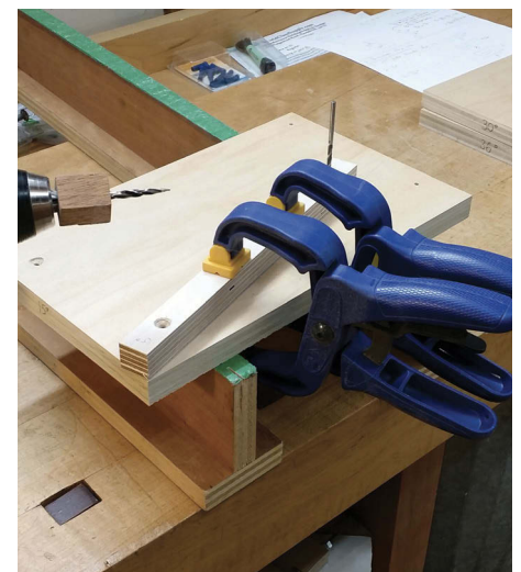
Fence secured while tapping transfer punch
