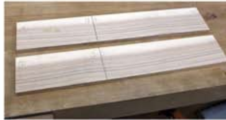
The chosen sections cut to length and marked out
