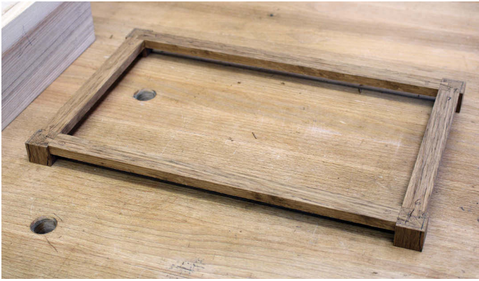
Dry fitting the dovetailed base
