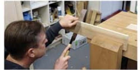
Making the cross cuts with a fine Japanese saw
