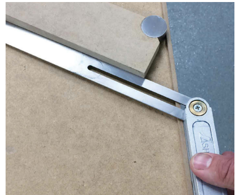
Obtuse angle for sliding bevel
