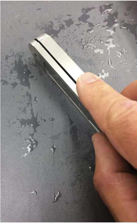
Truing the sides of the sliding bevel blade
