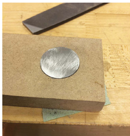
Filing the cylinders flush with the MDF holder
