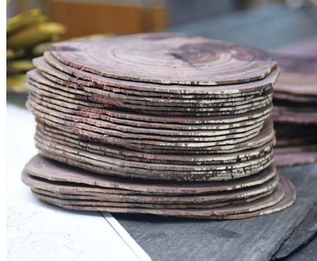
End grain veneers (oysters) provide some of the most vibrant and unusual patterns
