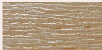
A typical sliced maple veneer showing cracks, tears and open grain caused by boiling and slicing
