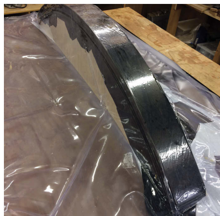
Rosewood apron veneers being applied using a bag press
