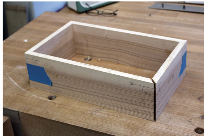
Checking the mitre fit using masking tape
