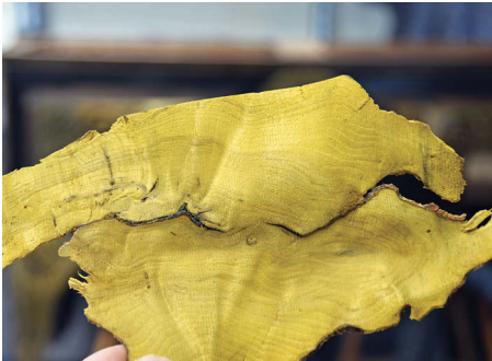
If boiled in readiness for splitting, these berberis and tulip veneers would lose all their natural colour
