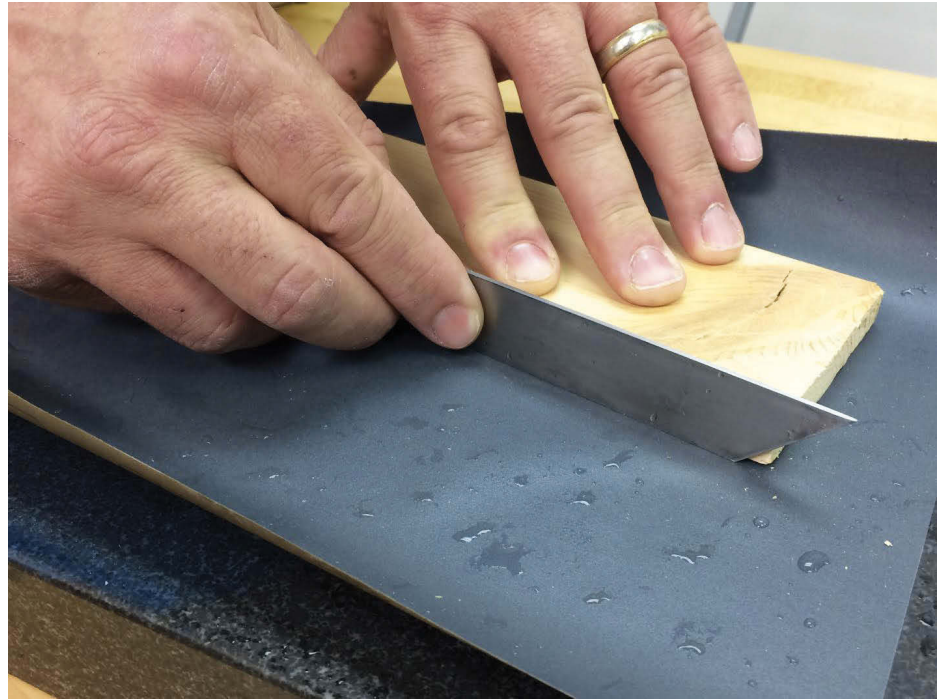
Truing the sides of the sliding bevel blade
