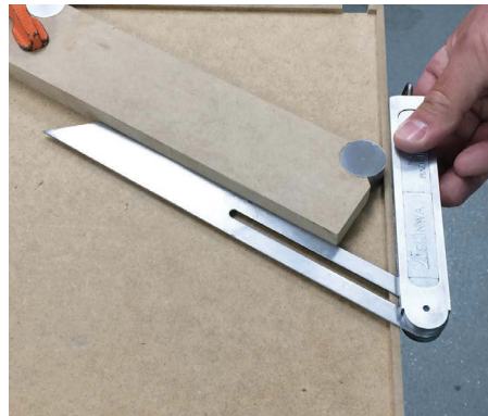
Acute angle for sliding bevel
