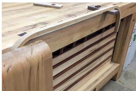
The bench dog block offers extra support for small but longish pieces
