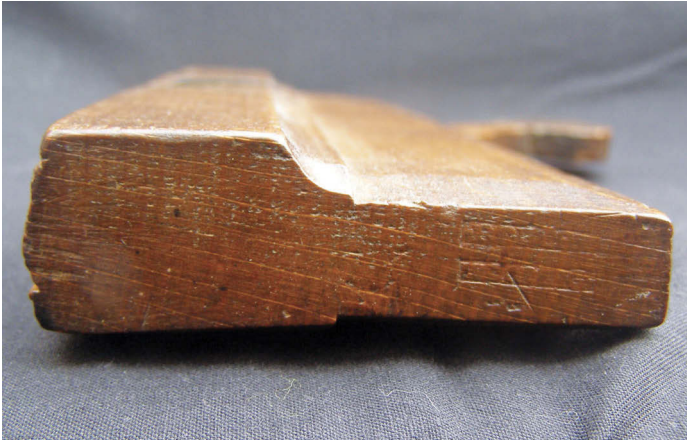
Robert Wooding moulding plane with steeply dropped shoulder
