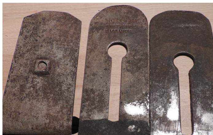
Round-topped irons with a back iron on the left
