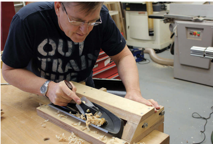
Mitres being finished on the shooting board
