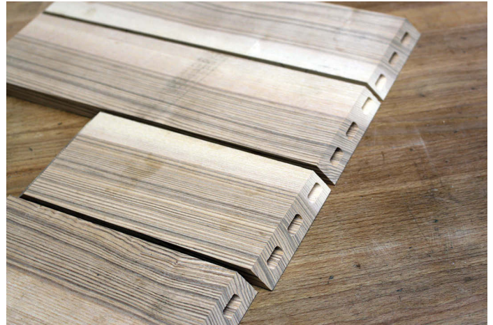
Mitres after rough cutting on the tablesaw
