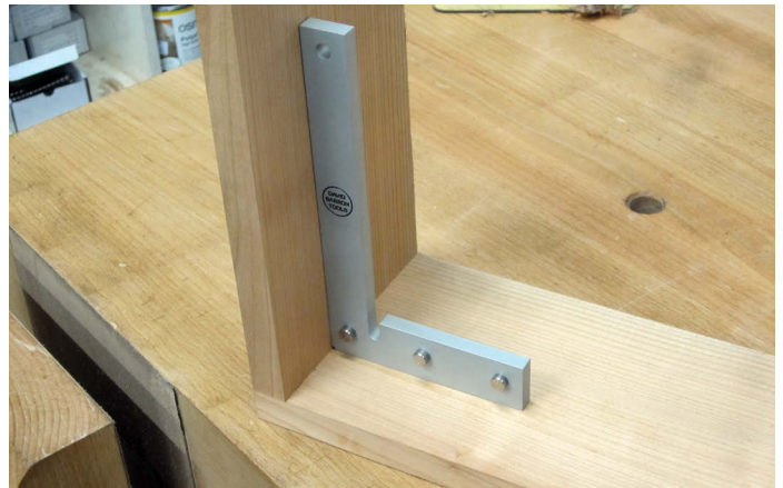
Making sure the glued up boards are at 90°
