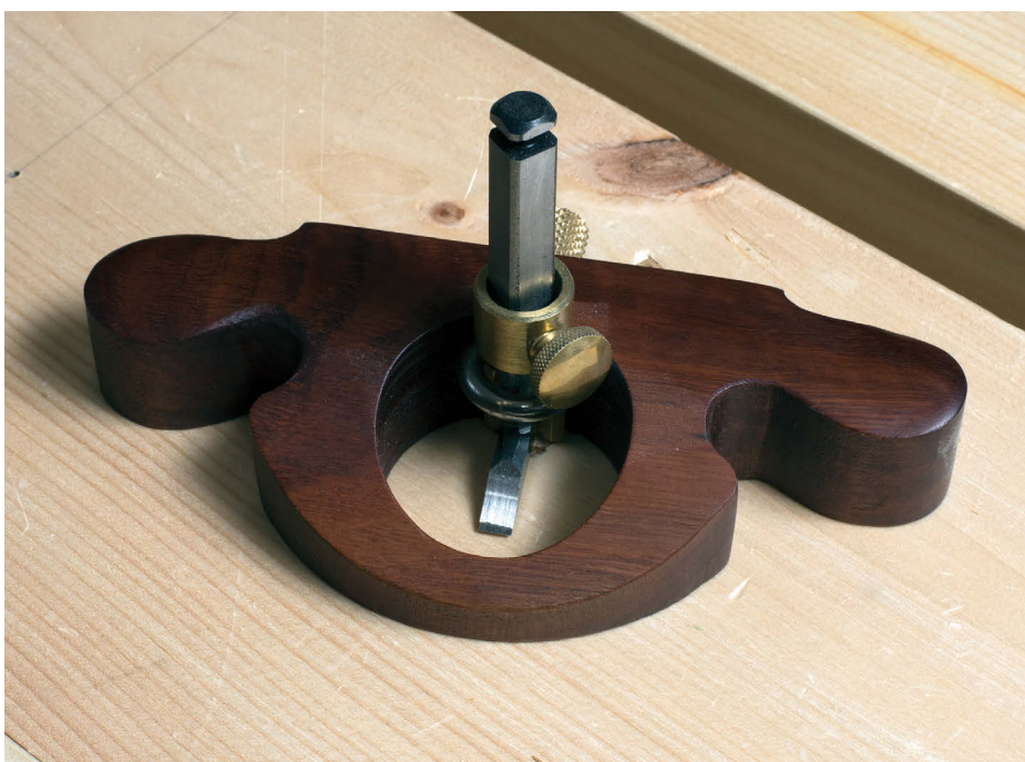
This handmade router made by Derek Cohen in Australia is perfect for those flat-bottomed details in your work
