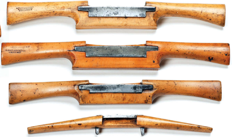
View of the undersides of three boxwood spokeshaves and the back of one
