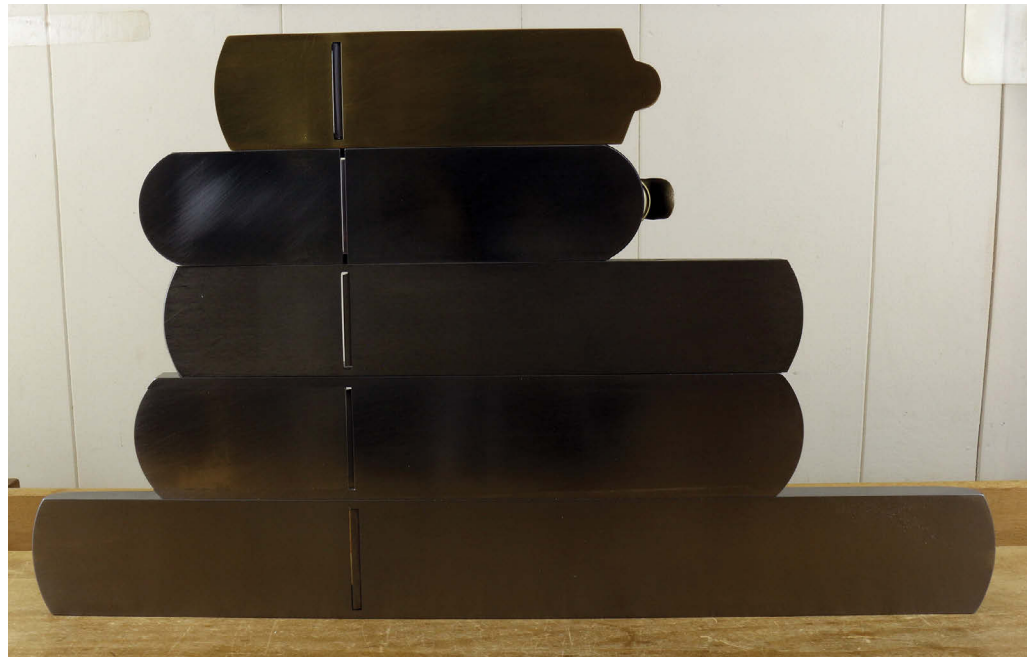
Plane soles for comparison, from top to bottom: #4 smoother, 11in #9 shooter, 14in #5 bevel-down jack, 15in bevel-up jack, 22in #7 jointer
