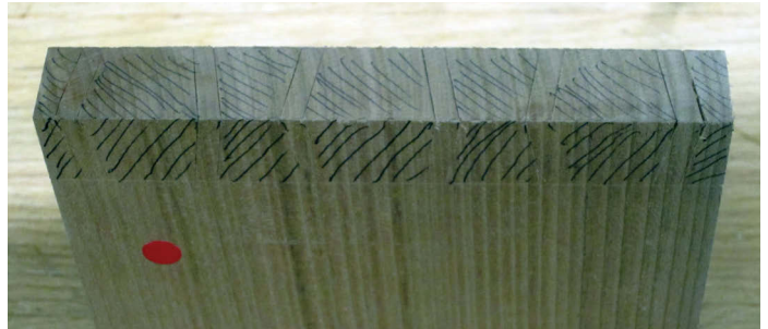
The waste area for the pins marked out
