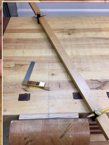
Laying out a 23in radius on the edge of the Baltic birch ply
