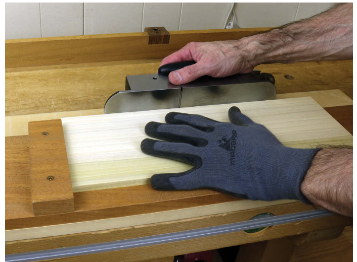
The grippy glove, along with the front stop, makes it easy to control the workpiece
