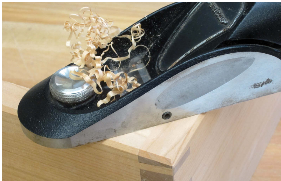
Plane a chamfer on the inside edges
