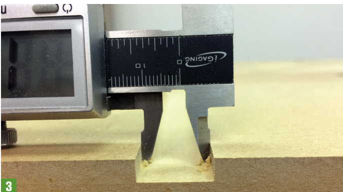
Determine the exact cutter width by measuring the width of the cut
