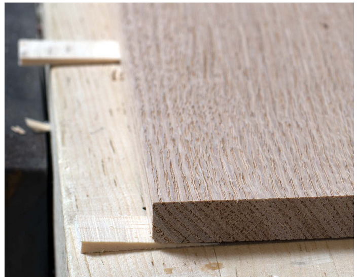
Wedges are the simplest tools and are handy all over the shop. Here we are shimming the board to prevent rocking
