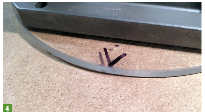
The indexing point is marked on the edge of the router base
