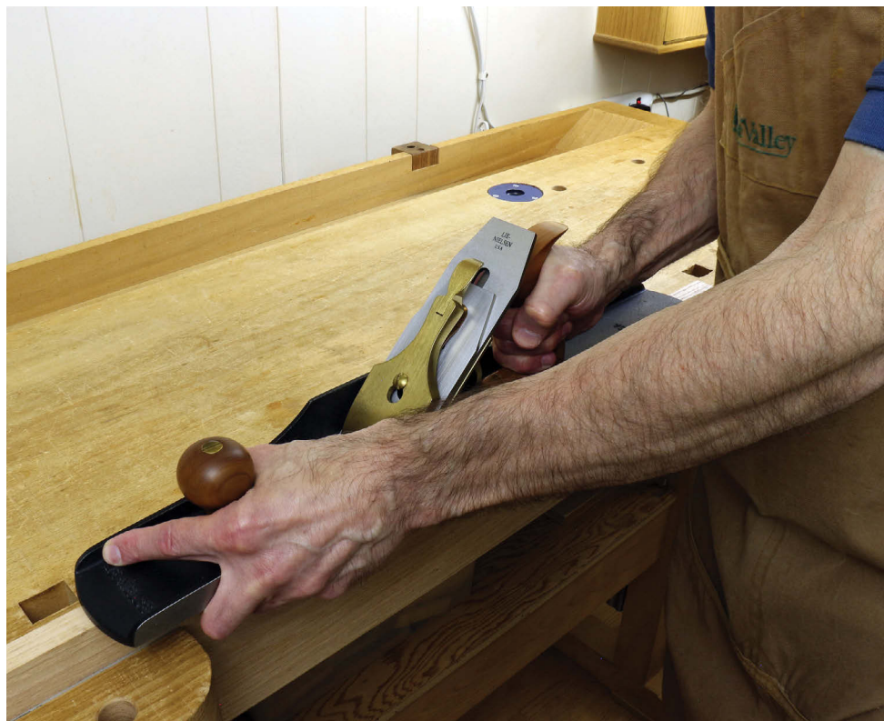
The front hand helps to sense flat and guides the lateral position of the plane, as it applies variable downward pressure during the pass
