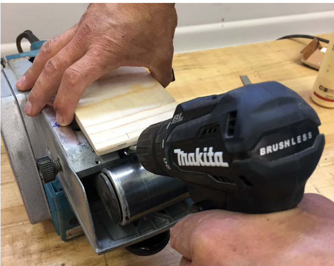
Then attach the assembly to the belt sander with the original factory machine screws
