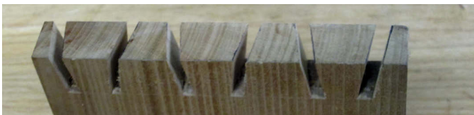
Rear view of tails cut and cleaned out
