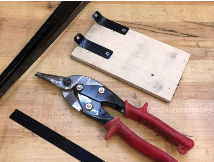
Ordinary metal banding works fantastically well. Attach to the platen with wood screws
