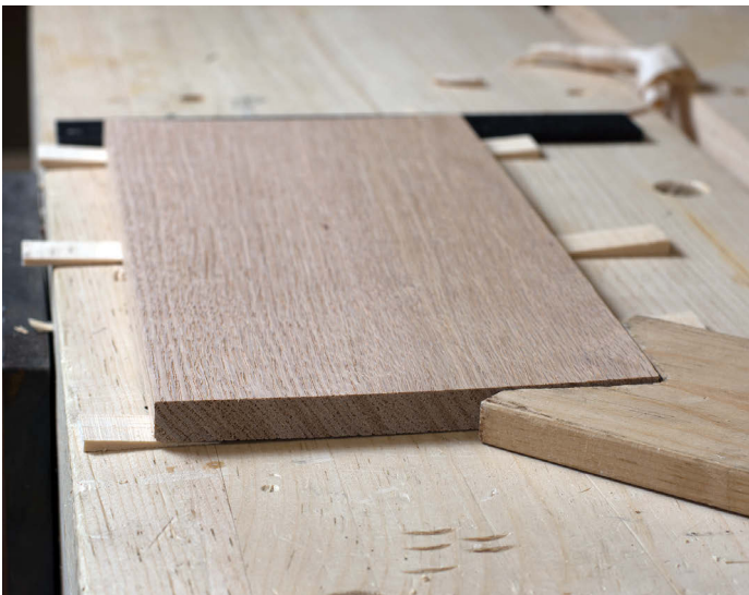
Secure the board to your bench using stops or a vice of some type
