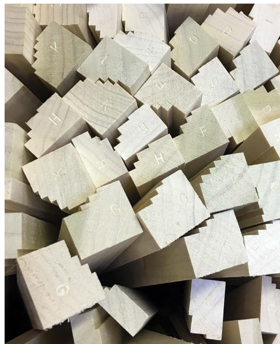
Rabbets cut in preparation for planing moulding profiles – this is the cornerstone of Matthew's moulding technique
