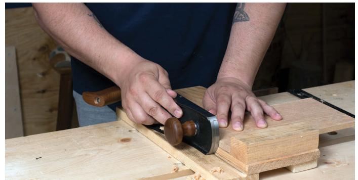
A shooting board is a must-have bench appliance
