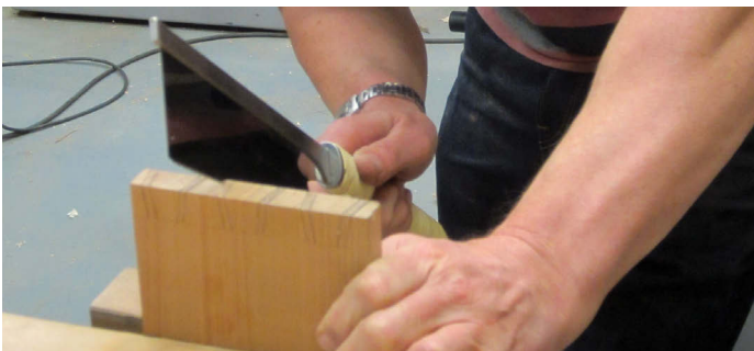
Tails being cut at 45° following both lines simultaneously
