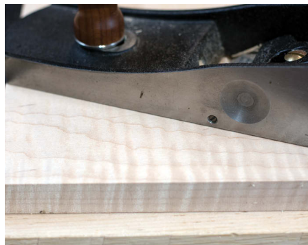
A well-honed and polished high-angle blade makes easy work of high figure
