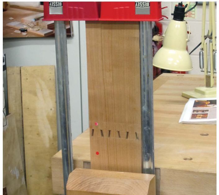
Set up for marking the pins from the tails
