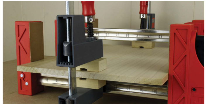
These easily made clamping blocks keep this thin panel aligned
