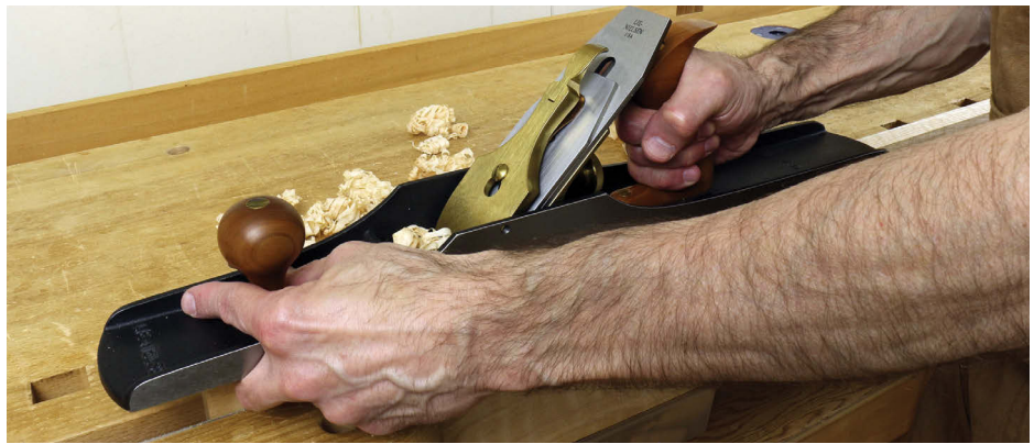
With practice, you will sense when you have produced a good camber, even before you test it
