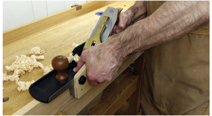
The front hand maintains pressure on the fence against the side of the board, as it applies variable downward pressure during the pass
