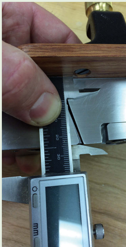
Using the calliper/stack for setting hand tools
