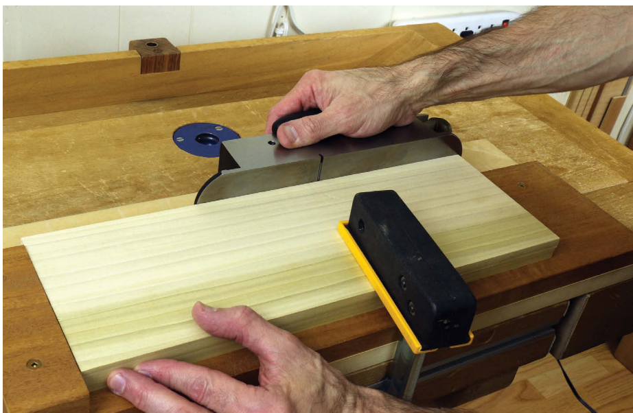
The grippy glove, along with the front stop, makes it easy to control the workpiece
