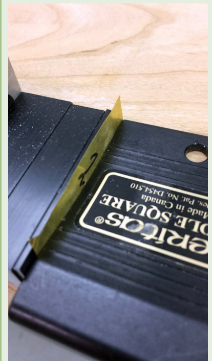
A shim is used to adjust for glue
