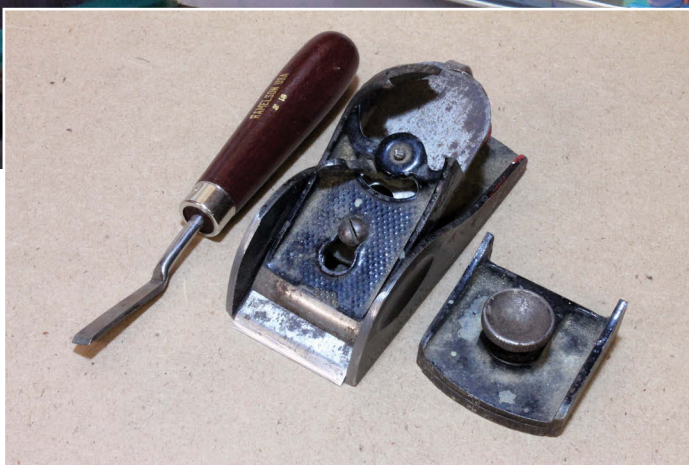
RIGHT: I cut the toe off a broken-down block plane to use it for glue clean-up, a tip from American woodworker Brian Koppert
