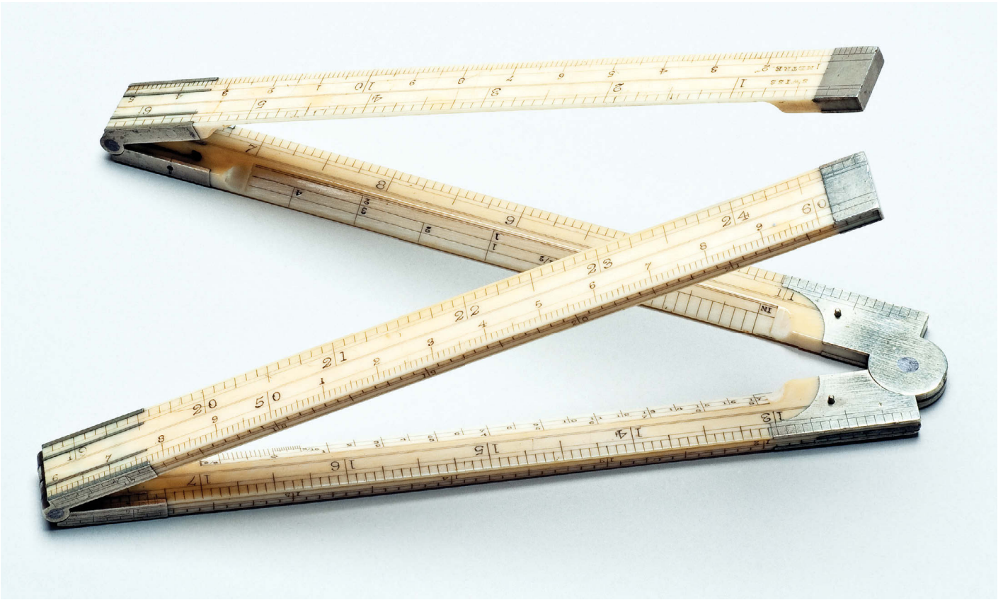
Four-fold rule in ivory and German silver. This mid-19th-century rule has the maker's mark of Holtzapffel & Co., Charing Cross, London
