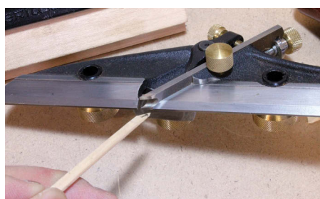
The plough's skate is ground slightly thinner than the outer cutting edges are wide
