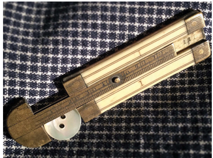
A brass and ivory button gauge. Its sliding calliper is graduated in fortieths of an inch, the standard typically used for button sizing
