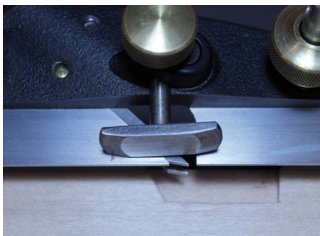
This is a fine-cut setting. Coarse cuts are harder to control and more prone to tearing the wood fibres
