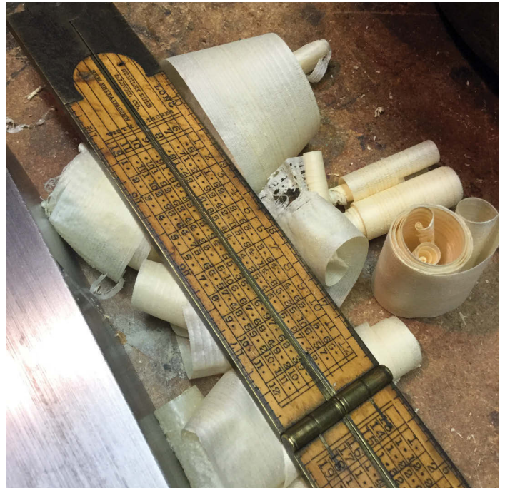
Stanley Rule & Level No. 82 2ft, four-fold rule. This rule features, on its interior faces, board tables that reference the number of board feet in sawn lumber of varying lengths and widths. This rule is not overly common and when found, is often in a fairly abused state due to a rough work environment
