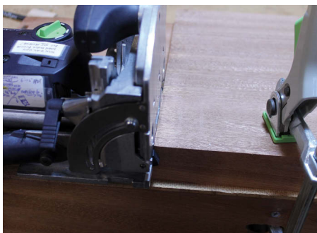
With its baseplate resting on the side piece, I registered the stop latch against the shelf to make the cut
