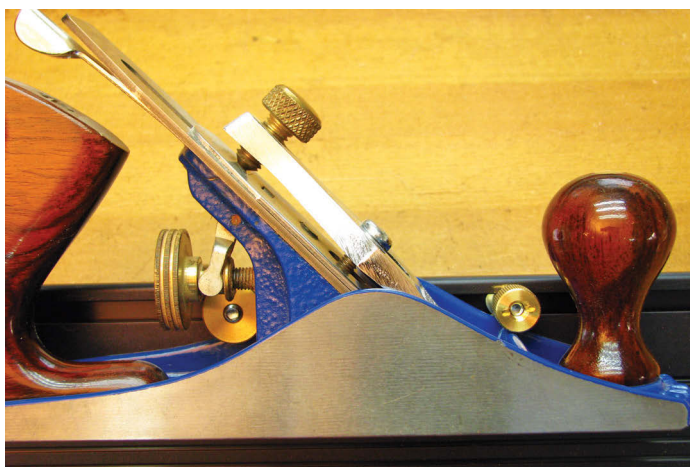
The two brass nuts can be adjusted to locate either side of the frog
