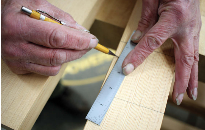
Marking out the dovetailed edge of the tenon
