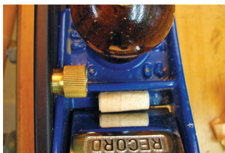
For best results grind your blade straight and set it parallel to the sole of the plane
