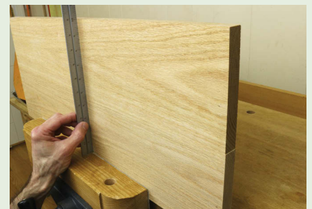
This is a direct and accurate check to prove the panel wants to go together flat
