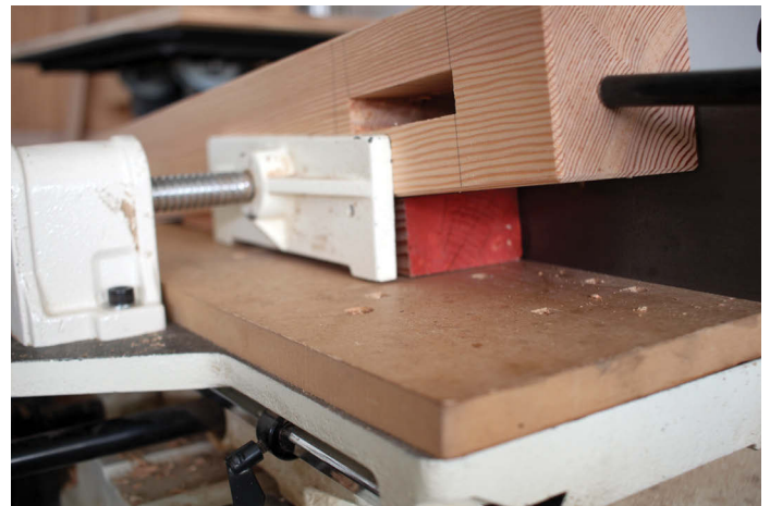
Place a shim beneath the leg to cut angled mortises
