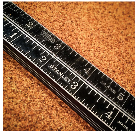
Two Stanley No. 423 aluminium zigzag rules. These 3ft folding rules were the smallest of four different sizes of cast aluminium zigzags made by Stanley from 1919 to 1935
