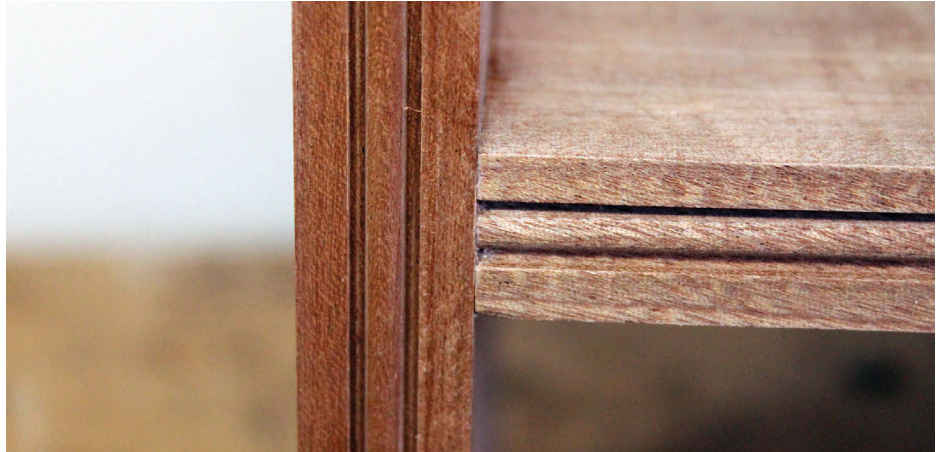
Beading comes before joinery if you want a second chance to recut a profile gone awry
