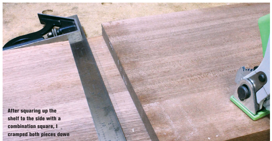
Stand the shelf in position and mark out the shelf location with double lines
