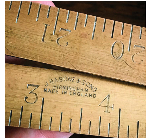
A No. 1243 brass blacksmith's rule made by John Rabone & Sons of Birmingham. This 24in, two-fold rule is made of brass to avoid scorching in a highly heat-infused workspace
