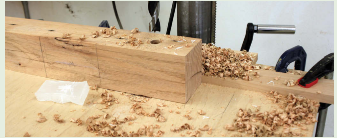
Using stop blocks streamlines the mortising process
