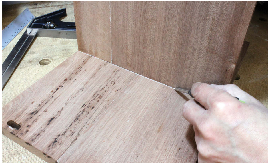
Stand the shelf in position and mark out the shelf location with double lines
