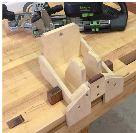
Above and right: a 'shop-made cradle designed to hold the DF700
