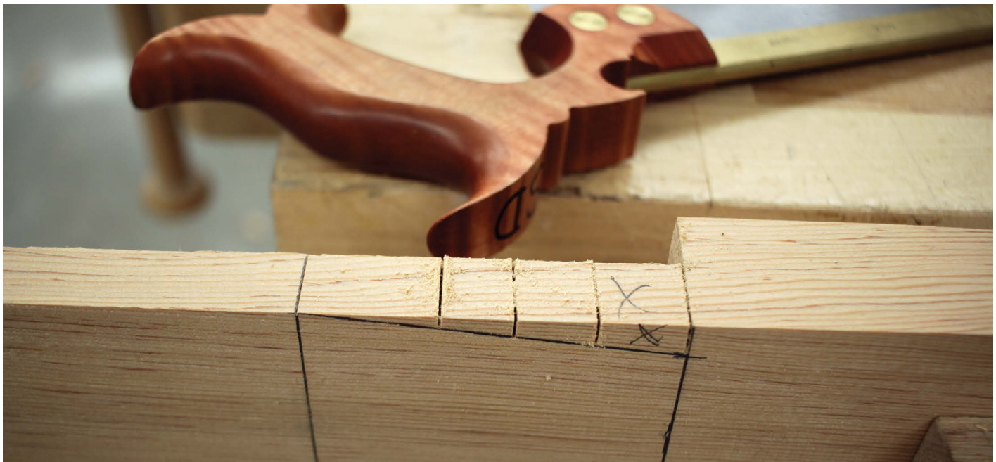
Saw cuts down to the line help to prevent the waste from breaking beyond the line
