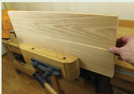
Here, the joint surfaces are grabbing only at the ends – good
