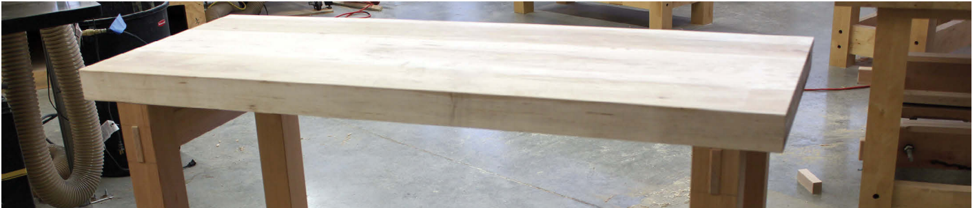
Position the benchtop onto the base to mark out for the dowels
