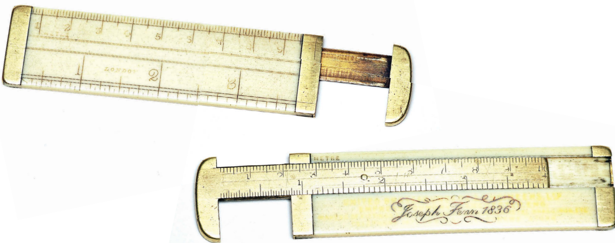
Rule and gauge made from brass and ivory or bone, shown here with both sides to view. It is dated 1836 with the maker's mark is of Joseph Fenn, London
