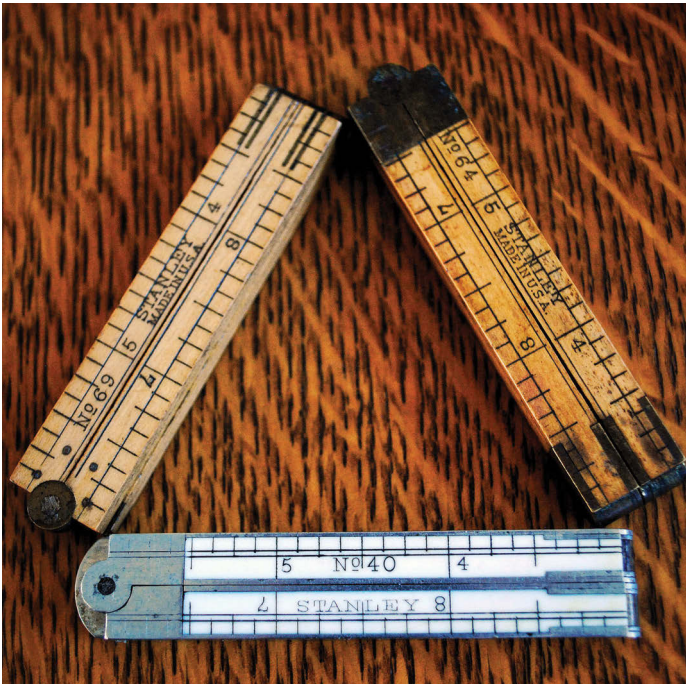
Trio of 1ft, four-fold rules from the Stanley Rule & Level Company. Left: a fairly basic No. 69 in boxwood and brass, with a simple round joint, but in exquisite condition. Middle: an ivory No. 40 caliper rule with main square joint and edges fully bound in German silver. Right: a harder-to-find No. 64, which has a square main joint in brass, and edge plates on the knuckle joints, which are a stronger design than the middle plate on the knuckle joints of the No. 69
