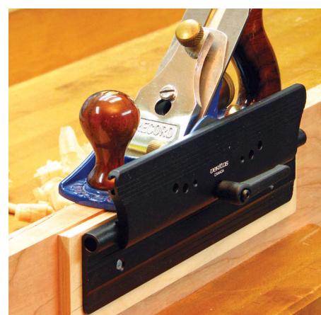
For cambered blades use an off-set packer to position the plane in the middle of the stock
