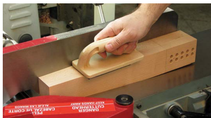
Check the grain direction on each component to avoid tear-out
