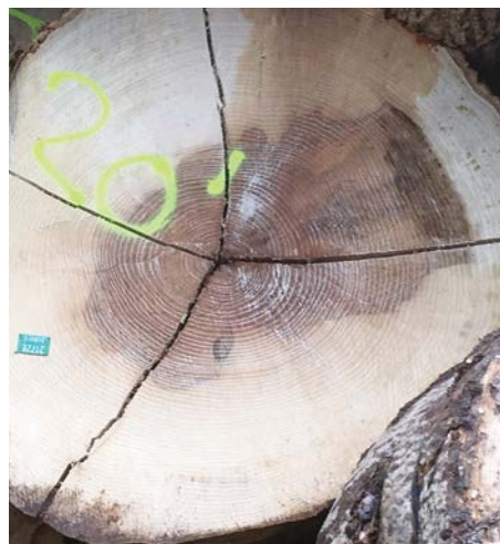
This ash log may have star shakes but the dark colouring at the centre indicates 'olive' ash inside
