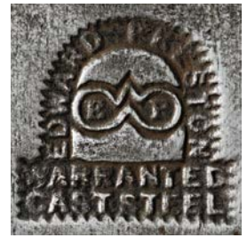
Maker's stamp on the cast-steel plane iron of the cast-iron smoother
