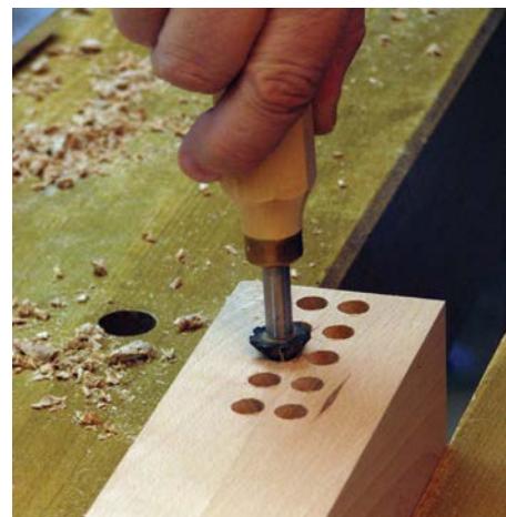
Removing the sharp edge from the top of the dowel hole will aid assembly
