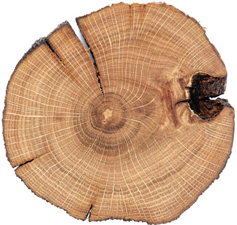
A small fissure on the outside could be hiding something more sinister on the inside
