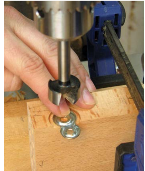
Allow sufficient clearance for the fixing to rotate
