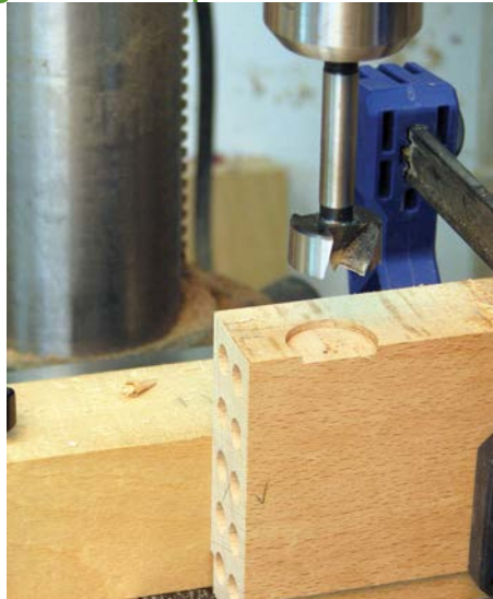
Use a Forstner bit to create the rebate for the fixing
