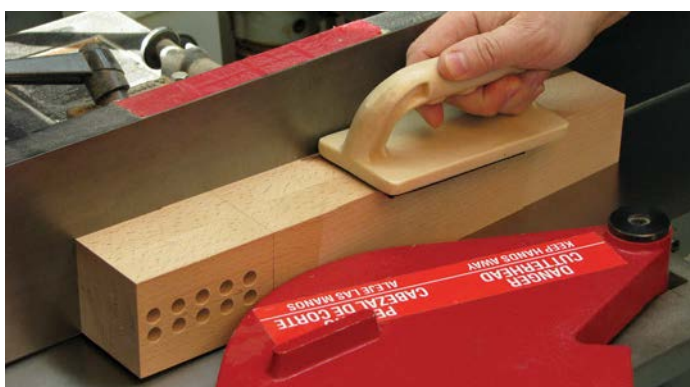
Use pressure pad as well as a push stick to smooth the tapers on the jointer
