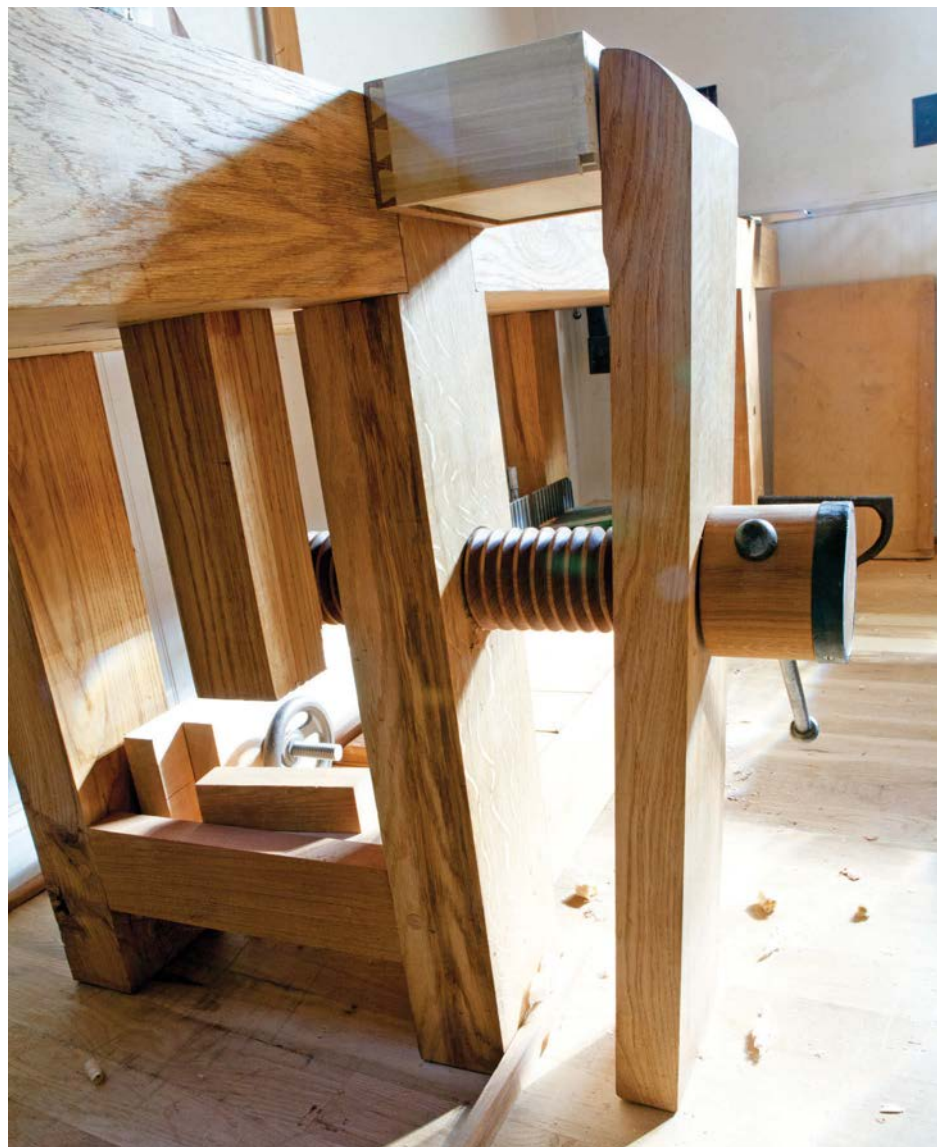
For the translated edition of L'Art du Menuisier , several woodworkers put Roubo's writing into practice. Here, a leg vice without a parallel guide holds a drawer
