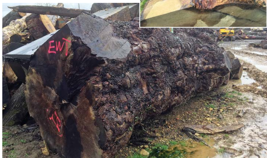
ABOVE: This long plane burr may contain boards with the most outrageous figuring INSET: A series of little growths or burrs on the outside is a good indicator for pippy oak
