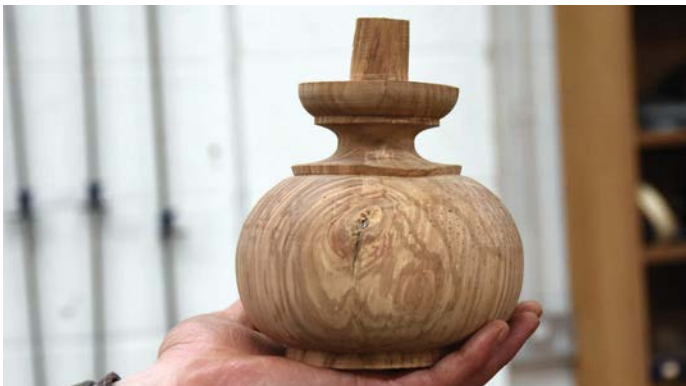
Replacement bun foot turned from wet olive ash
