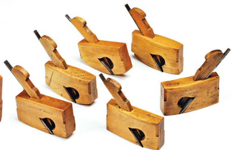
A set of late 19th- or early 20th-century boxwood 3½in compass and flat-sole rebate planes with maker's mark of E. Preston & Sons, Birmingham
