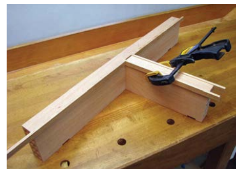
The inlays were glued into place before assembling the T joint
