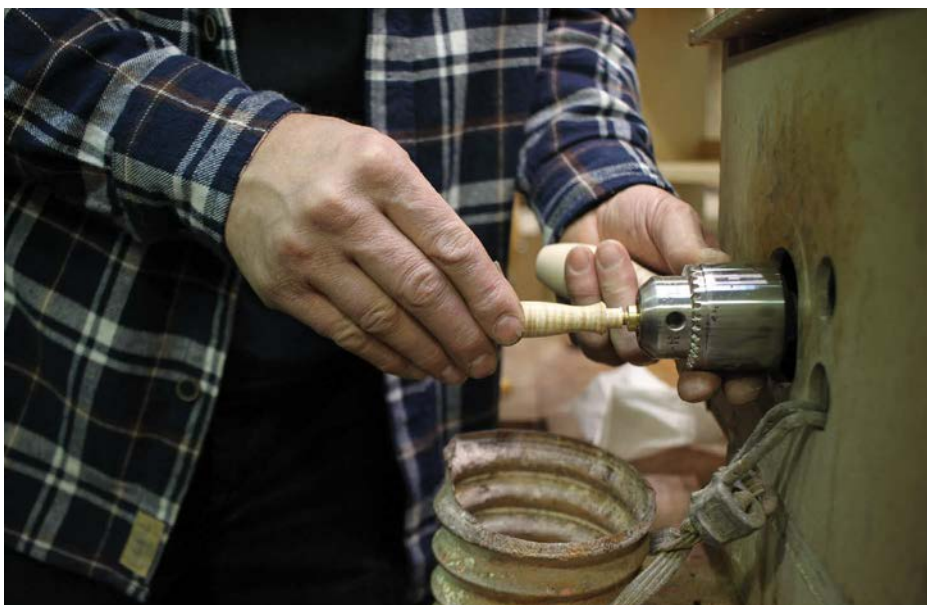
Securing the handle to a marking knife in the chuck of the Sand-o-Matic 3000
