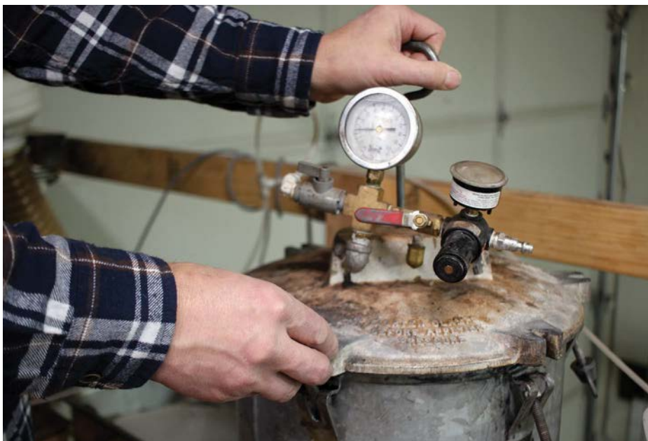
The vacuum chamber on the unique Blue Spruce infusion process
