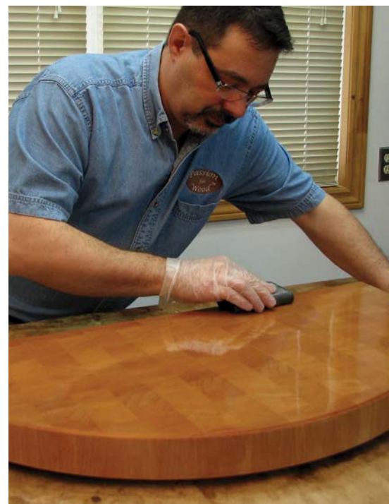
Final surface finishing the top
