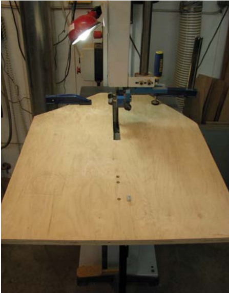
A simple plywood jig with pivot point cuts perfect circles
