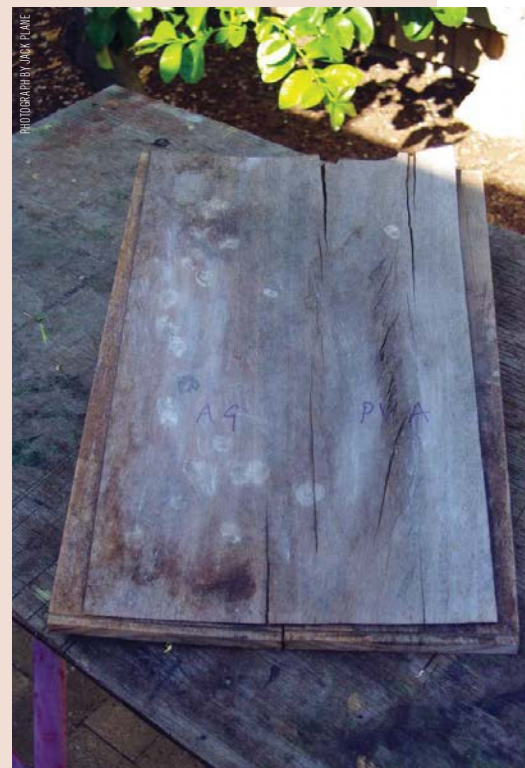
Weathered test board; animal glue on the left and PVA on the right
