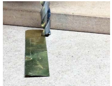
Setting the hole depth for through-holes
