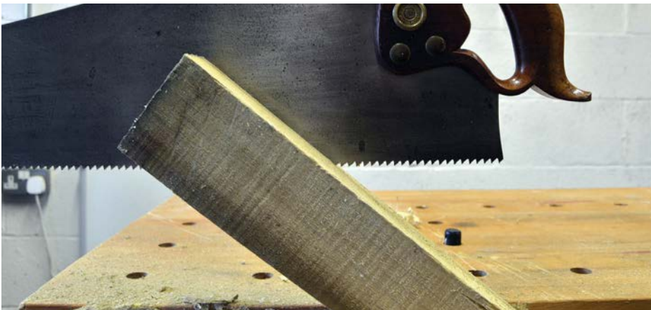
The Quangsheng plane's kerfing blade leaves the ideal kerf to drop in a handsaw for resawing thick boards
