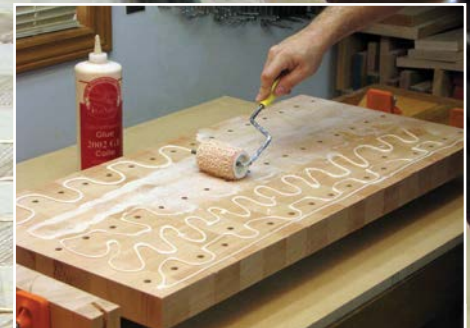
Glue is applied to the other side of all strips at once. A heavy nap paint roller coats the surface without depositing glue in the dowel holes
