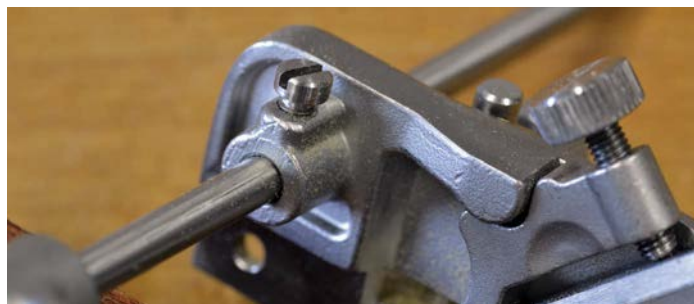
Set screws secure the fence posts at the body of the Quangsheng plough
