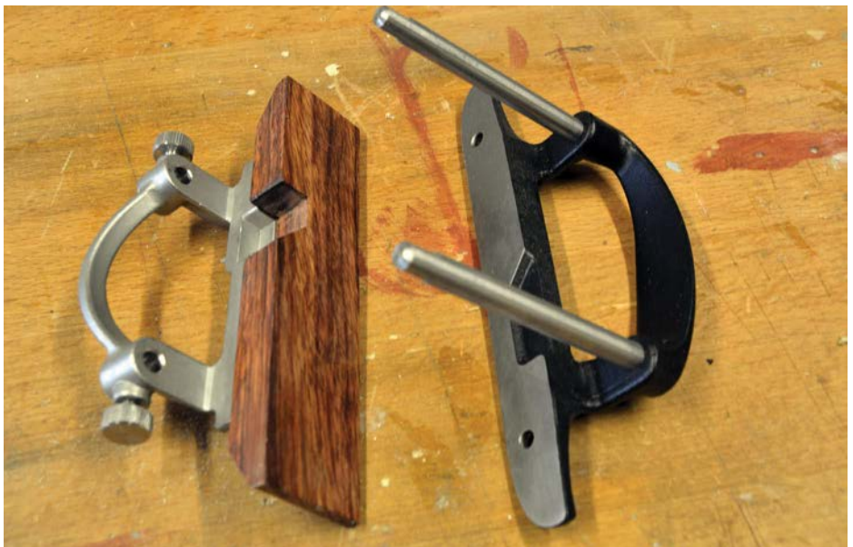
Comparing fence surface area – the Quangsheng auxiliary fence (left) is shorter but deeper compared to the Veritas fence (right)
