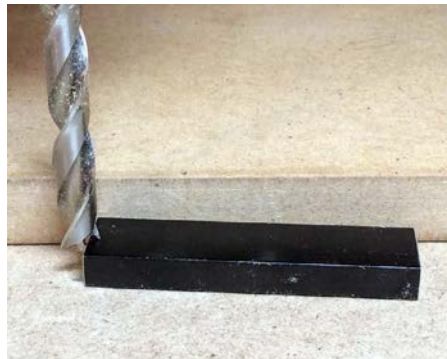
Setting the hole depth with a 'stack'
