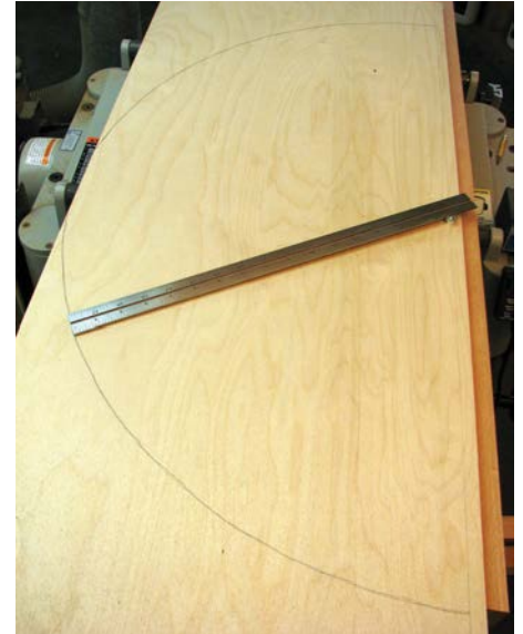
A hole drilled in the template stock provides the pivot point. Then cut out the shape, which is slightly larger than a half circle
