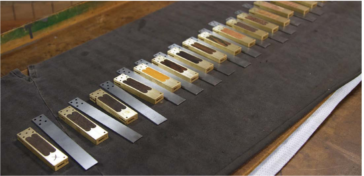
The next batch of infill Try Squares awaiting inspection prior to final assembly
