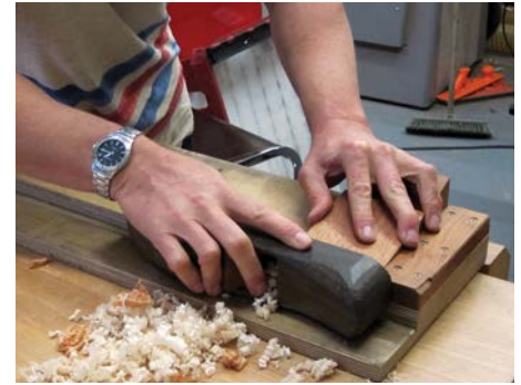
The top and bottom of each piece are angled at 9° (using the vertical support) on the shooting board. Check and double check here as it's easy to plane the angle the wrong way!
