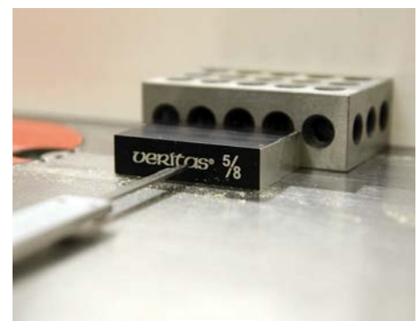
Using the 'stack' to set the rip fence
