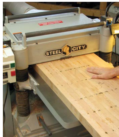
A wide thickness planer levels both sides of the long grain slab, saving me a lot of hand planing time
