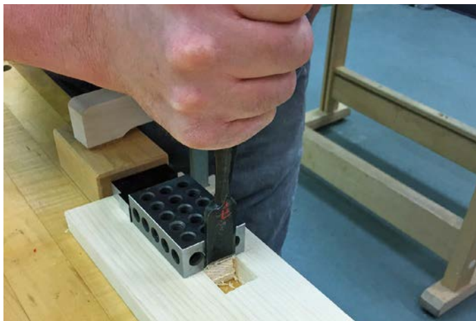
Precision paring along the workpiece
