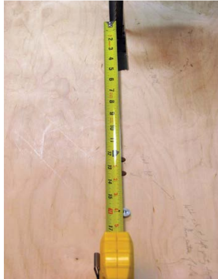
Position the jig on the bandsaw table with the centre of the pivot point the correct distance from the right side of a right-pointing tooth. This sets the radius of the circle
