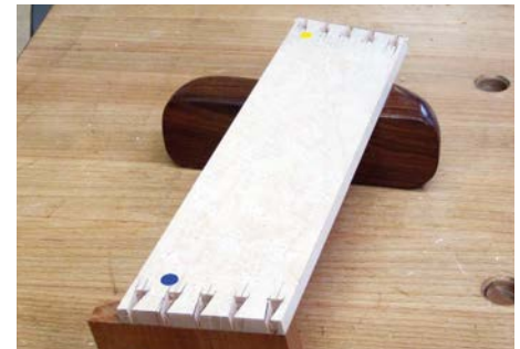
With the tails all cut and cleaned out it's time to mark the pins. Although it's a compound angle, the two boards are actually at right angles to each other so the setup in the vice is quite straightforward. The only thing to take care with, is aligning the bottom two edges exactly, so that when the grooves for the bottom are cut (using the same edge), they all line up
