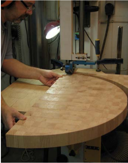
Semi-circles are cut out of the end grain slabs freehand, leaving about 1.5mm to trim later with a router
