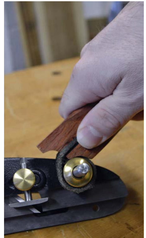
Locking the Veritas fence in place using a Nut Saver by Bern Billsberry
