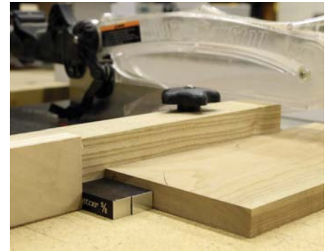
Partial 'stack' being used on the tablesaw
