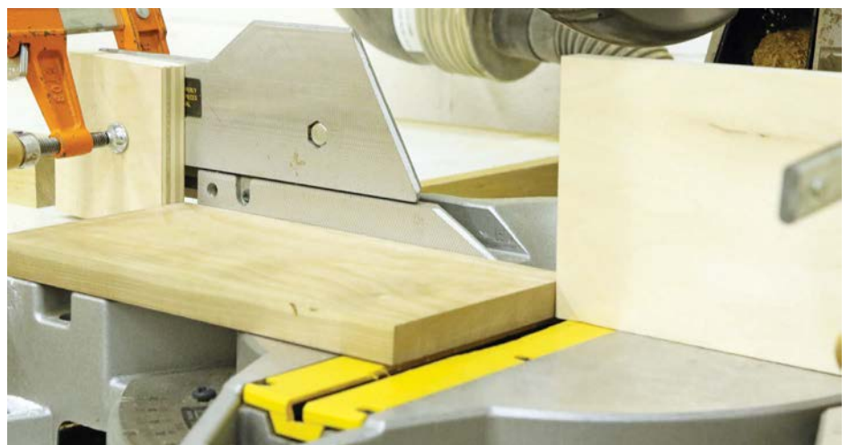
Original stop to the left of the blade and temporary stop set to the right of blade
