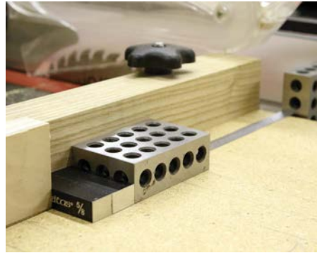
Final stop position with 'stack'
