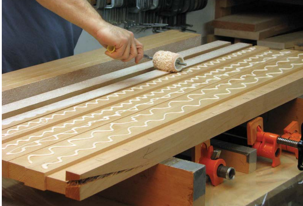
A thick nap paint roller makes quick work of spreading glue on the strips of wood
