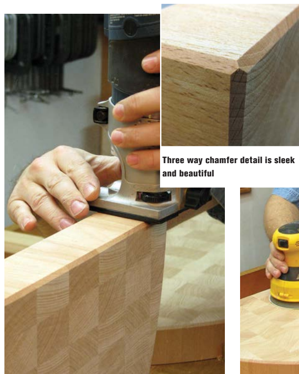
A palm router adds the chamfer detail to the vertical corners at the rear of the table tops
