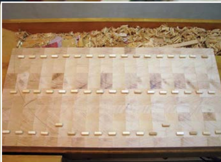
Short dowels between the strips keep them aligned during glue-up, but they must be carefully placed around the cut-line of the semi-circle
