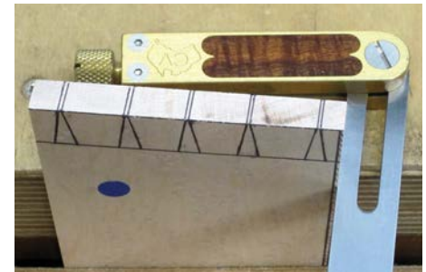
The end grain saw cuts are marked at 9° parallel with the bevelled edges. Setting a bevel gauge using the vertical support board is the easiest way to translate these lines. The base lines are scribed in the normal way using a cutting gauge or wheel marker
