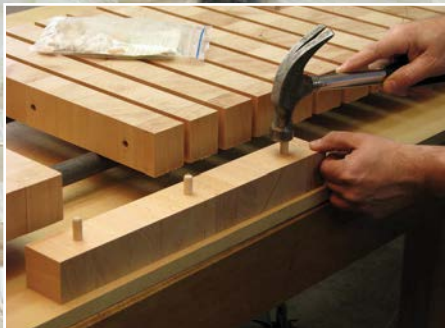
Dowels are hammered all the way home into one half of every joint. The dowels are used for location only and do not require glue
