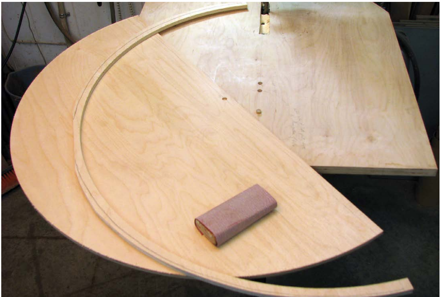
A short dowel provides the pivot, resulting in a perfect circle requiring only minor sanding
