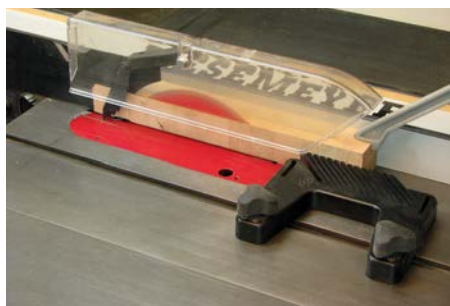
Each strip is ripped to ensure consistent width and defect-free surfaces
