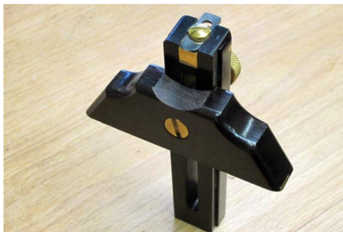
My adapted cutting gauge to handle curves
