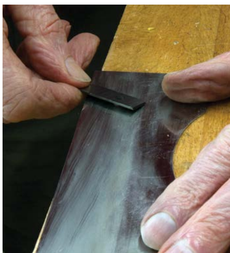
The blade is held at a small angle to the edge and moved outwards over the length of the stroke. Firm pressure combined with this diagonal action draws the metal out from the edge
