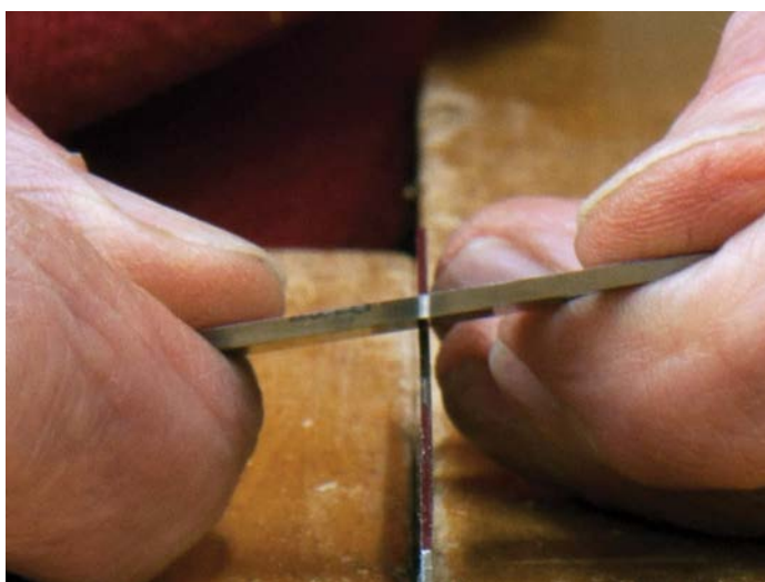
Finally, tilting the tool at about 5° towards the worked face creates the finished hook
