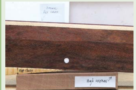
The gap on the wedge shows how much material is to be removed at the diagonal high corners
