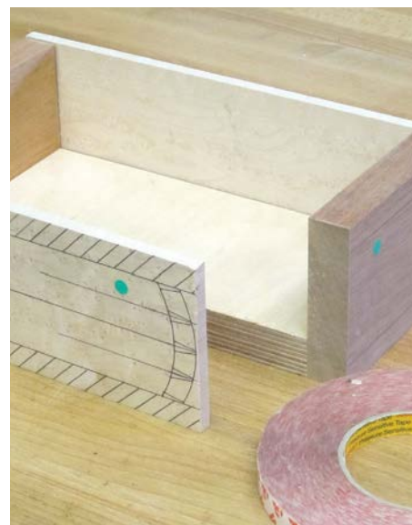
Assembling the box using double-sided tape and an accurate spacer block
