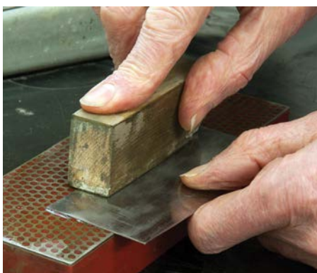
Applying pressure with a wooden block helps to achieve a flat, even face adjacent to the scraper's edge
