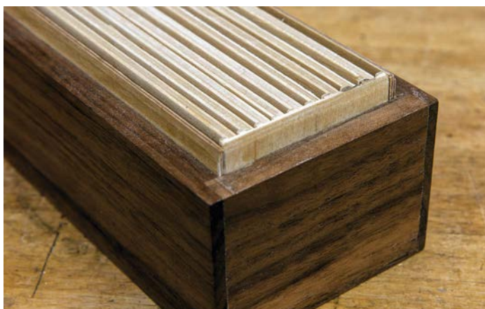
Thin ply liners project to provide location for the lid. Spacers are only 2mm apart to maximise capacity
