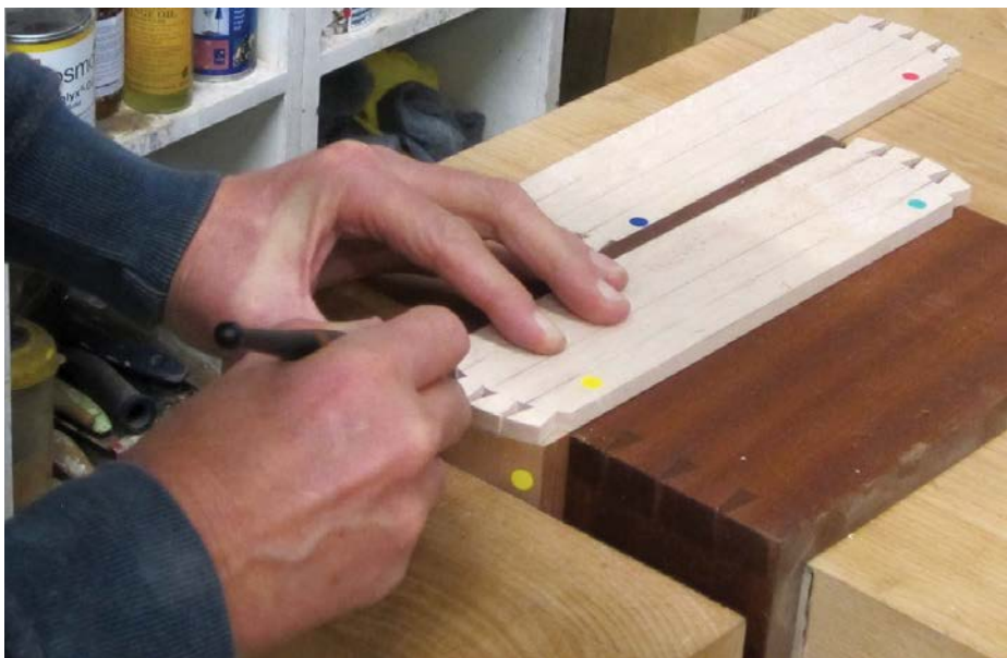
Marking the pins using my alignment board
