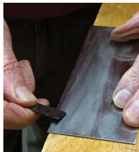
The blade is held at a small angle to the edge and moved outwards over the length of the stroke. Firm pressure combined with this diagonal action draws the metal out from the edge
