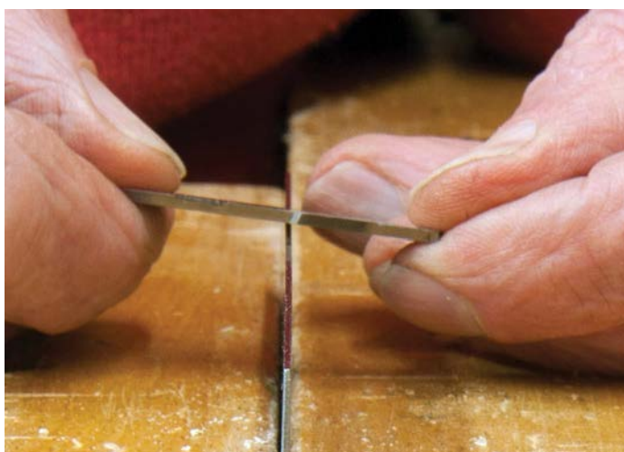
Stage 2 turns the metal raised in stage 1 so that it projects at almost 90° to the face
