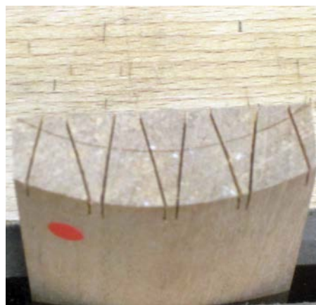
Saw cuts made on the pin board
