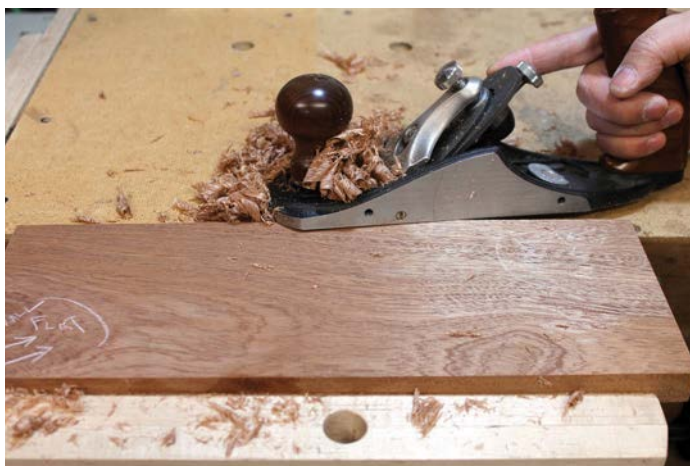
Plane down the two high diagonal spots and check the work often to avoid taking too much material from one spot
