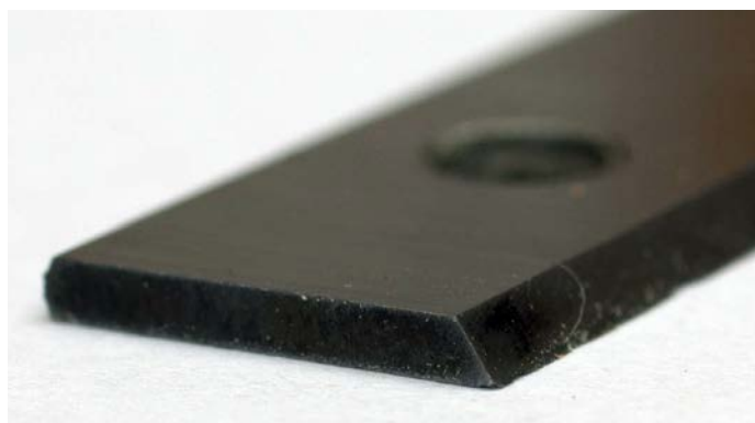
Only the obtuse angle between the bevel and the front of the blade is used, so blunt the cutting edges for safety
