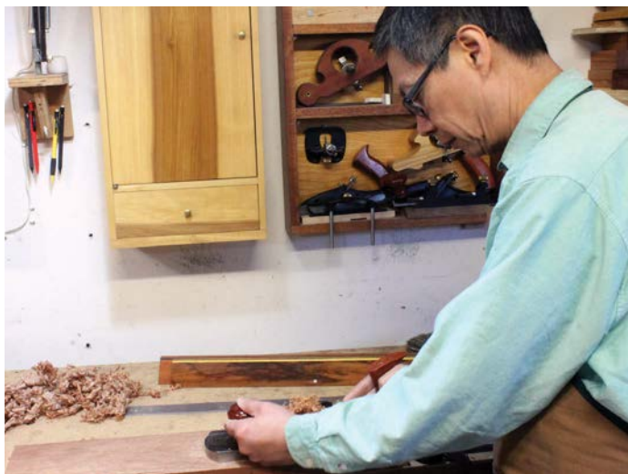
In finish-planing, loosen up the grip and make the final, long strokes with the grain
