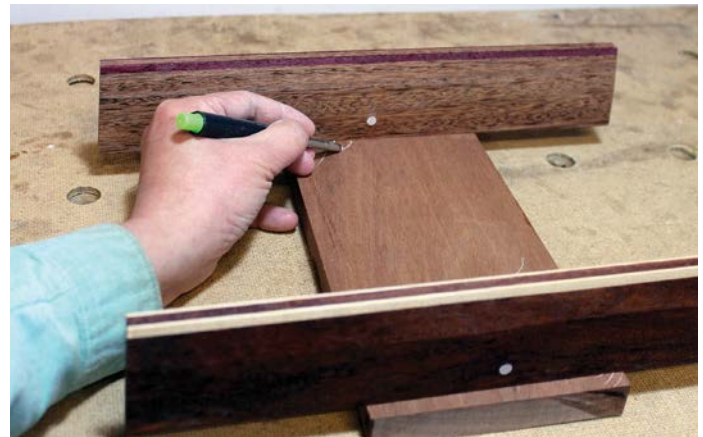
Keeping one of the sticks constant, run the second stick back and forth to find other high areas
