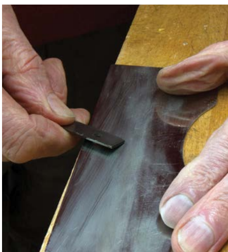
The blade is held at a small angle to the edge and moved outwards over the length of the stroke. Firm pressure combined with this diagonal action draws the metal out from the edge
