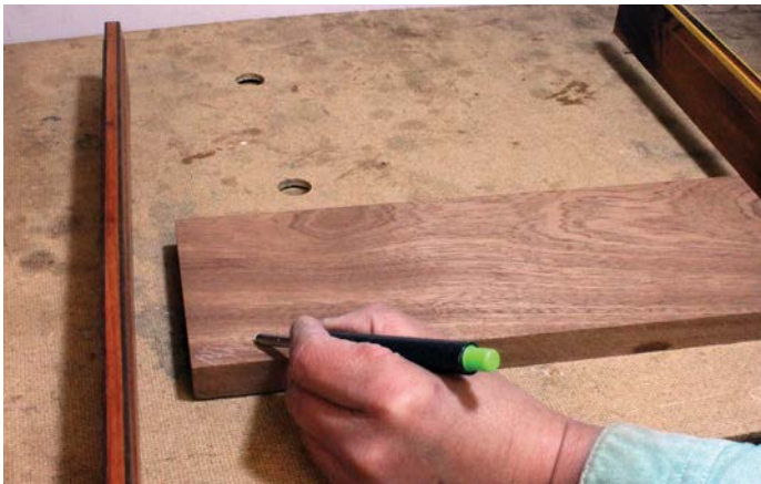
Mark the first high corner and then the diagonal corner which is also a high spot
