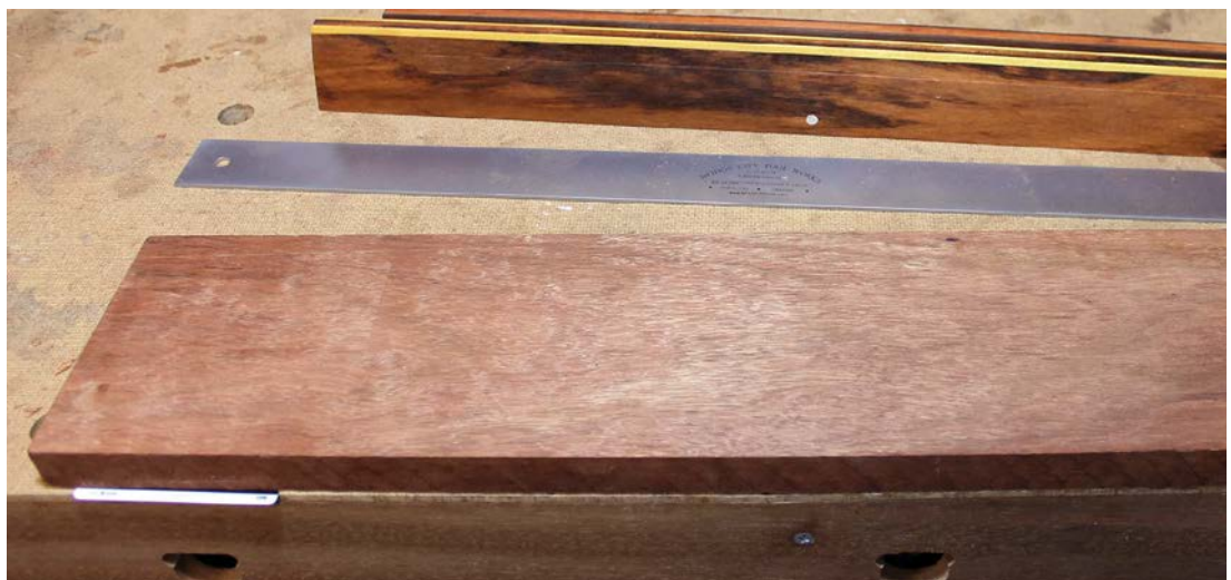
For a board too big for the vice, I clamp it to a bench with shims placed underneath the high corners
