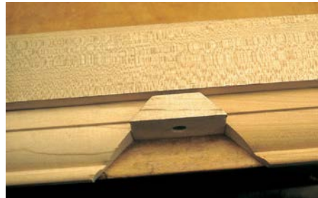
Fig 15: The jig for holding multiple pieces with mitred ends
