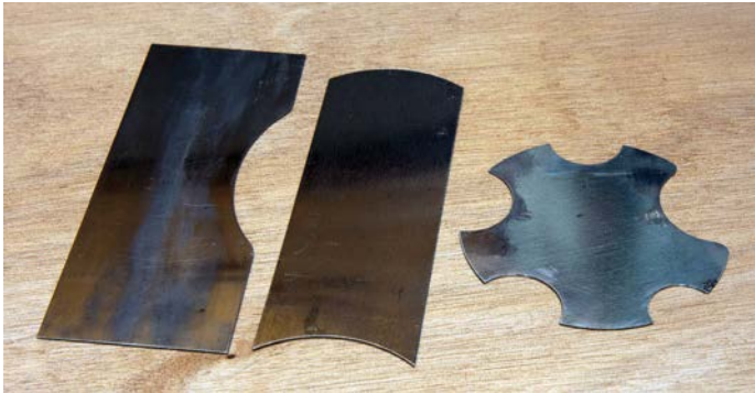
A workshop-made profiled scraper on the left with two commercial examples. Note that some of the transitions between curved and straight edges have been rounded to prevent them scoring the workpiece
