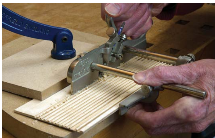
A Record 044 plough plane proved ideal for cutting the closely grooved end linings – in a quietly satisfying way too
