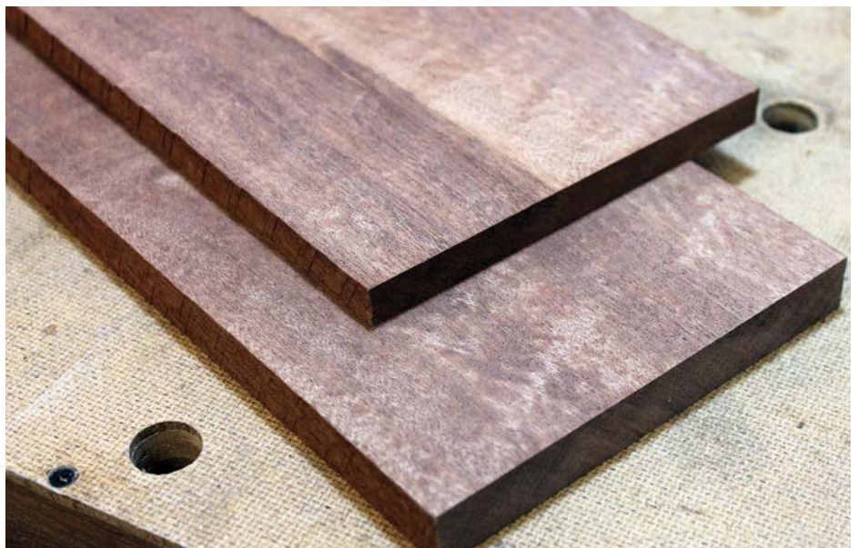
After being flattened, a twisted board can become too thin for your particular project
