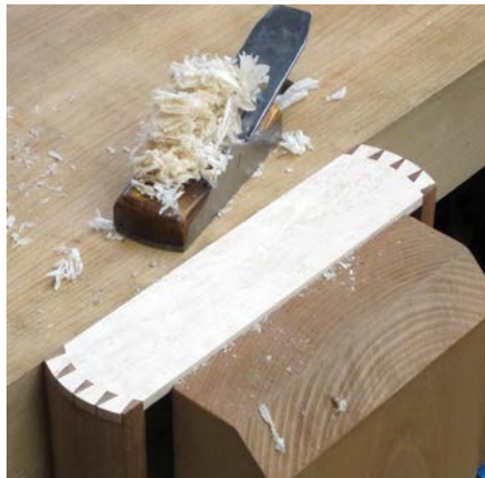
Cleaning up the sides including removing all trace of the base lines
