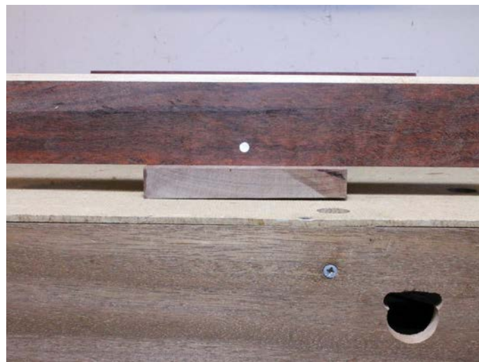
Sighting a dark edge against a light background allows easier reading
