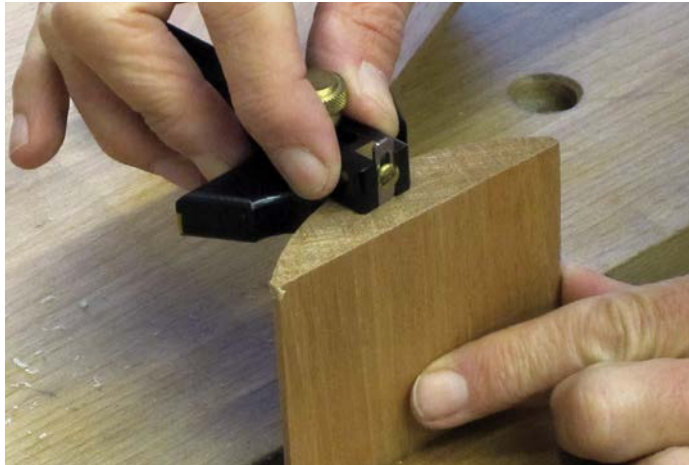
Marking out the end grain of the pins
