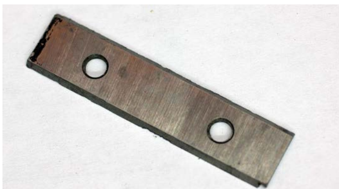
The perfect burnisher – a 50mm tungsten carbide blade used in spindle moulders and decorators' scrapers
