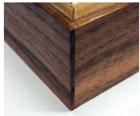
A simple rebated construction with glued-in top and bottom ply panels is perfectly adequate for a small box
