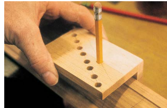
Fig 11: The gauge block in use. The multiple holes allow more than one pencil to be used at a time if necessary
