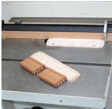
Cutting the grooves on the router table
