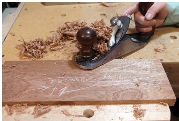
Enlarge the flats by making alternating diagonal cross strokes and inward from the edge to avoid break-out
