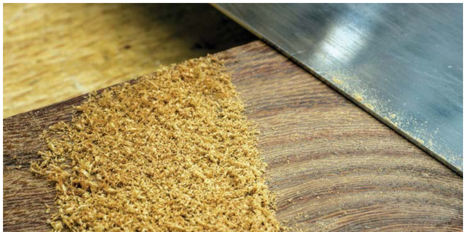
Not quite dust but the scraper edge was definitely past its best
