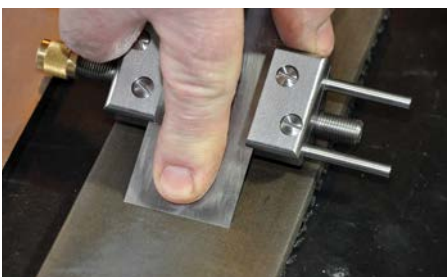
This one-finger technique is how I avoid uneven bevels on narrower blades although at 38mm wide this would normally require a two-fingered grip
