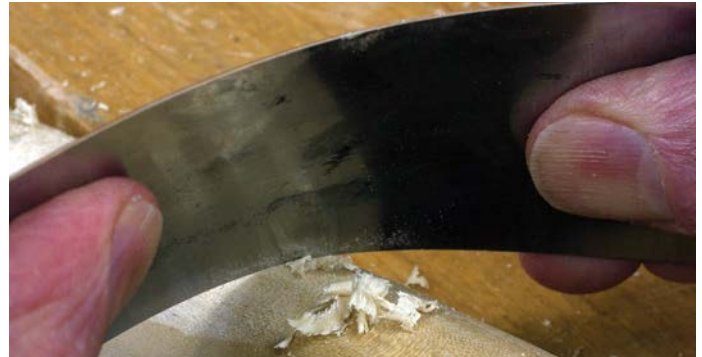
A thin, flexible scraper can be a good alternative to a profiled one if the curve to be scraped is gentle
