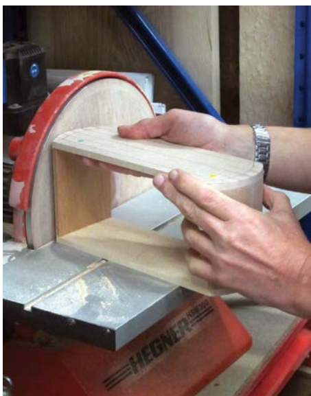
Sanding the convex curves on a disc sander
