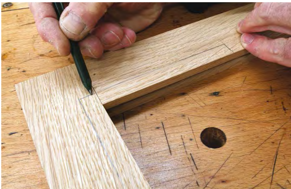
Marking out the position of the mason's mitre shows where to stop the moulding
