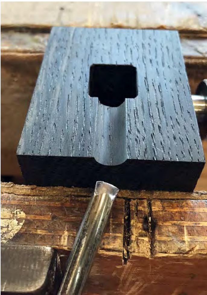
Use a gouge to create a hollow for the pencil...
