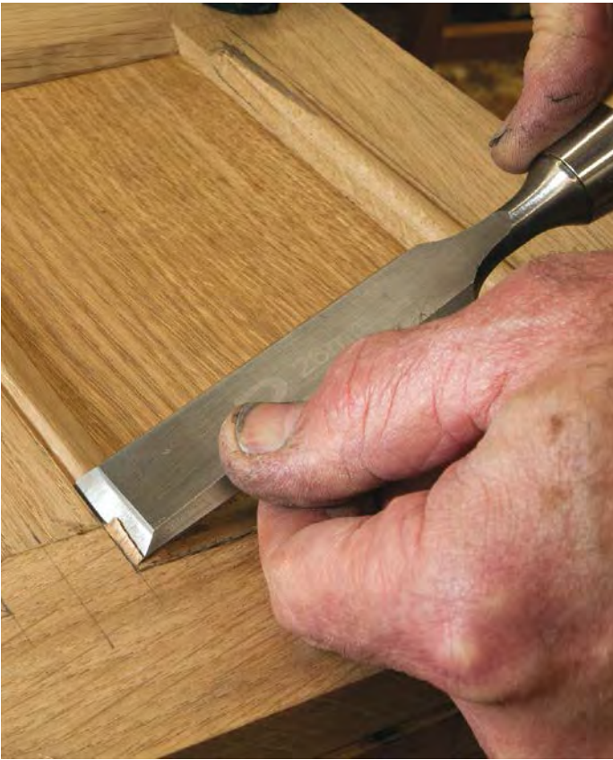
A wide chisel can be a useful tool to extend the moulding shape into the mason's mitre
