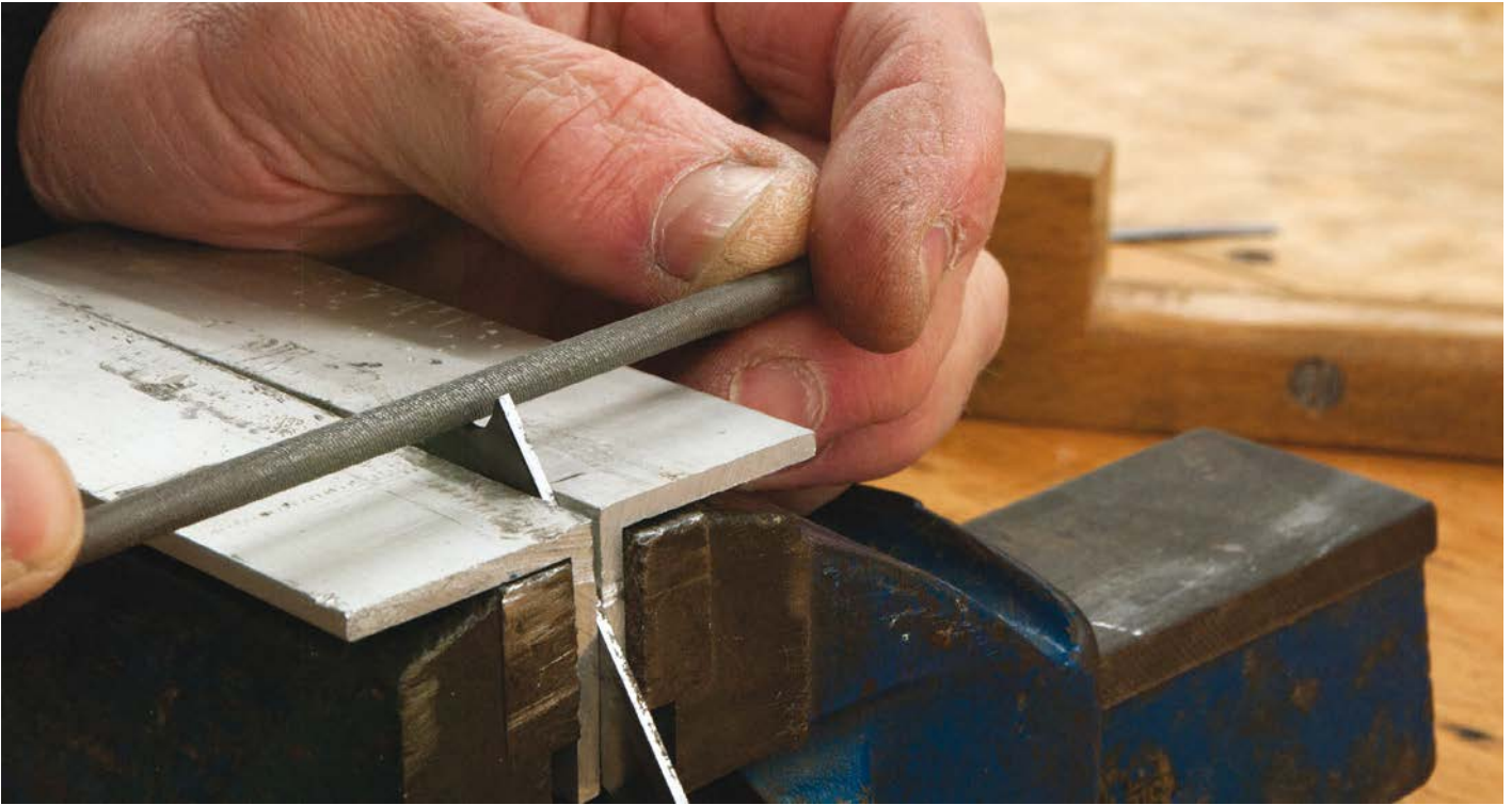
Scratch stock cutters are easily shaped with files
