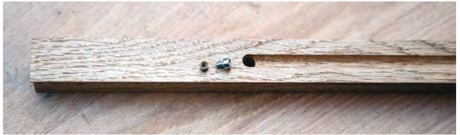
Machine screws are located in the slides to act as either a stop or a hook
