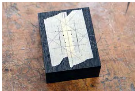
Centre mark the holes before drilling to avoid drilling outside the gauge lines
