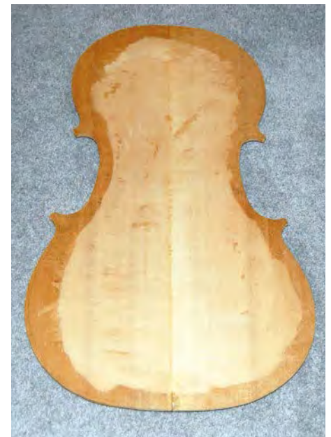
The central join on the cello after it had been cut from the wedge-shaped piece of wood
