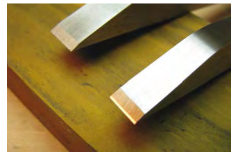
Super sharp 8000 grit microbevel helps
