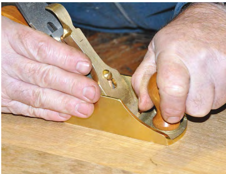
Using the No. 2. Unlike Goldilocks' porridge, this is too small for a proper grip, too big to use like a block plane – certainly not 'just right'
