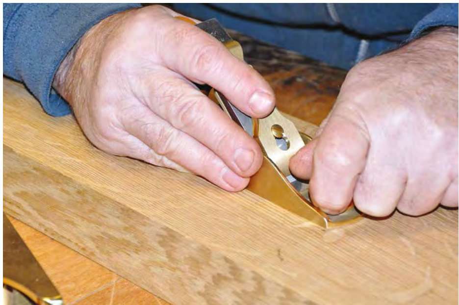
Using the No. 1 as a smoothing plane, which is more comfortable than it looks
