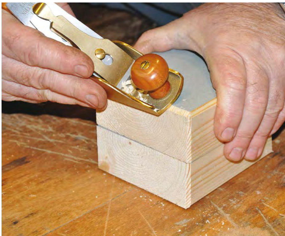
The No. 1 is nice to use one-handed like this. It's more comfortable than a block plane
