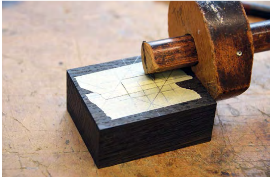
Use a cutting gauge to establish clear parameters
