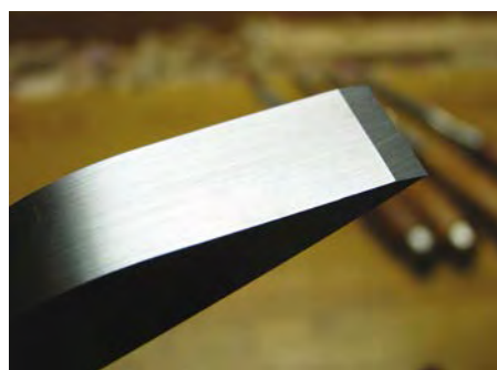
The curved top of the bevel makes levering out waste easy
