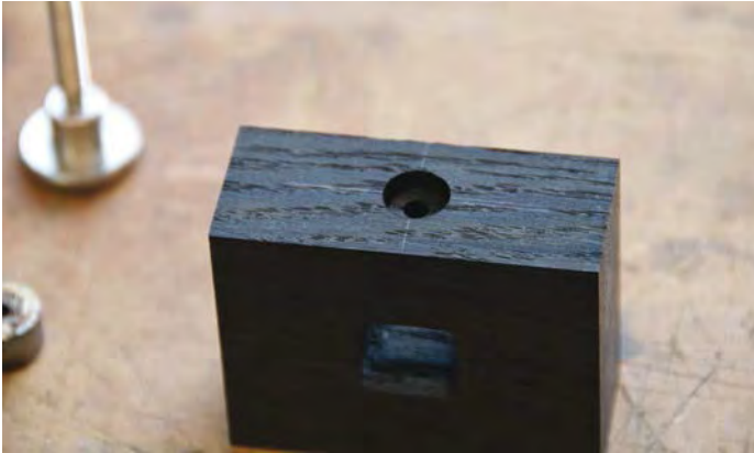
Through hole and thumbscrew sleeve clearance
