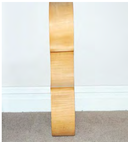
The sides or 'ribs' fitted to the mould
