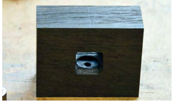
Create a recess to accommodate the washer
