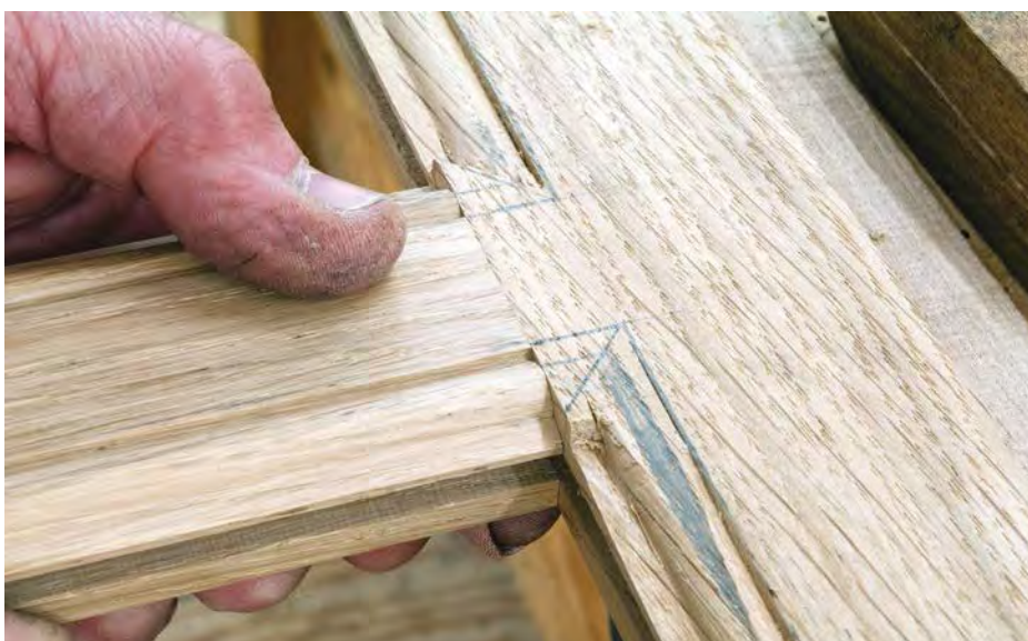
Mouldings cut and ready for the Mason's Mitre
