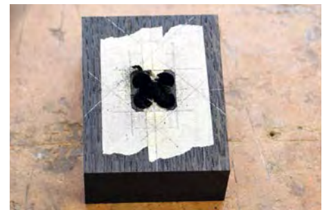
Leave enough material to fine tune the hole with a sharp chisel
