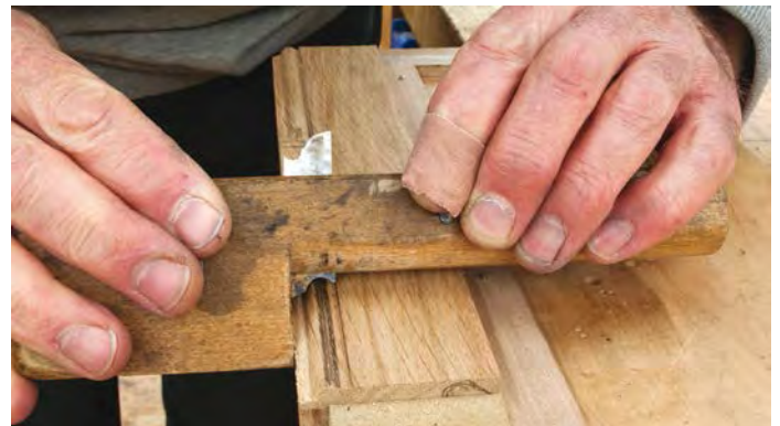
With a sharp cutter even cutting mouldings in oak is relatively quick
