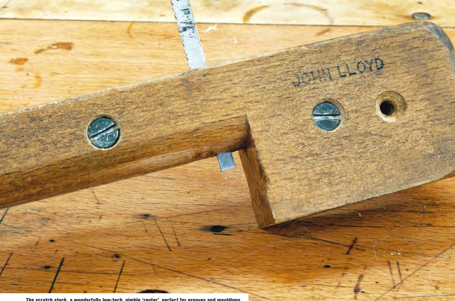
The scratch stock, a wonderfully low-tech, nimble 'router', perfect for grooves and mouldings
