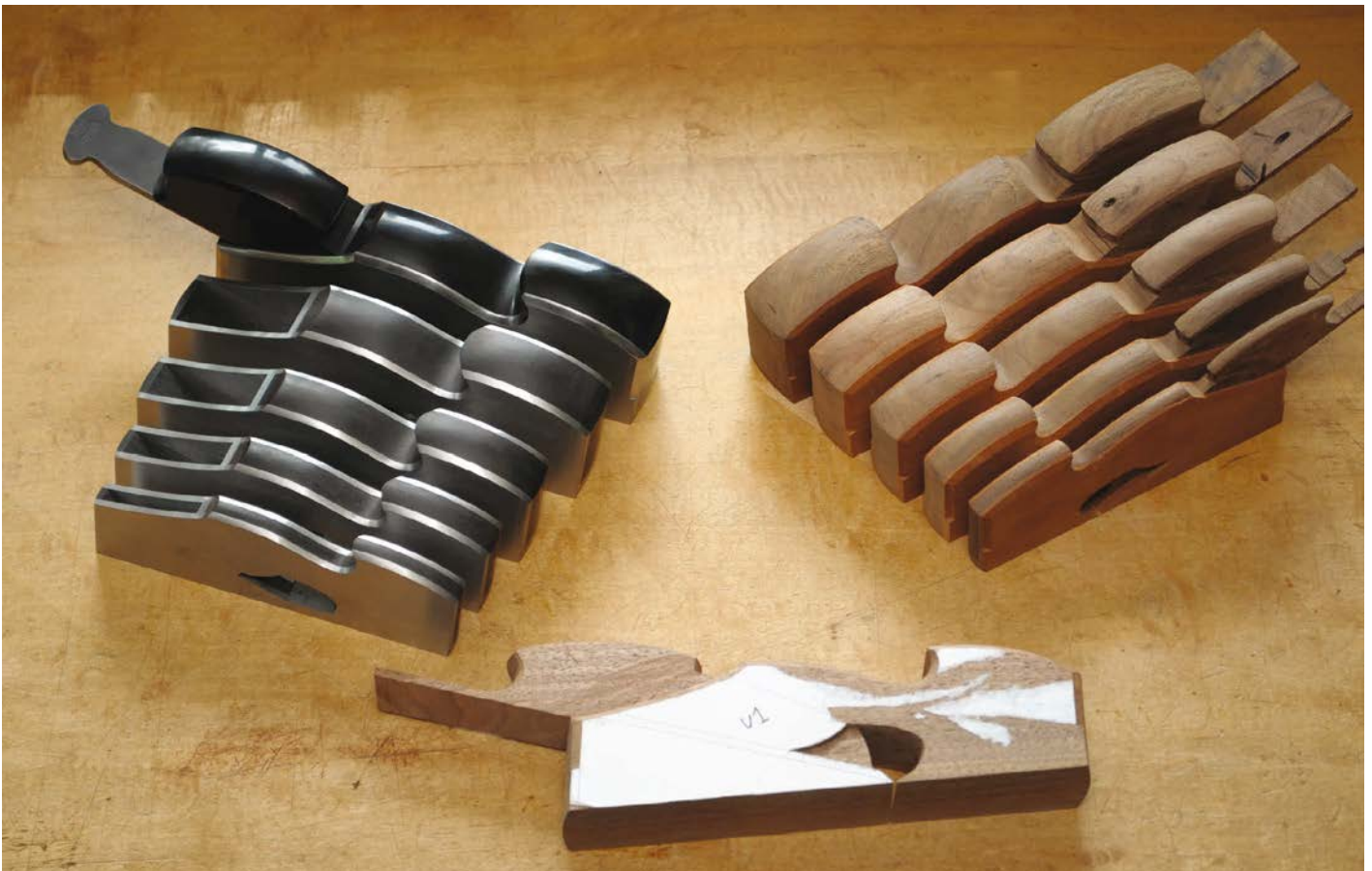
The new KS shoulder plane series. The original wood mock-up in the front; scaled wood mock-ups; the nearly finished prototypes
