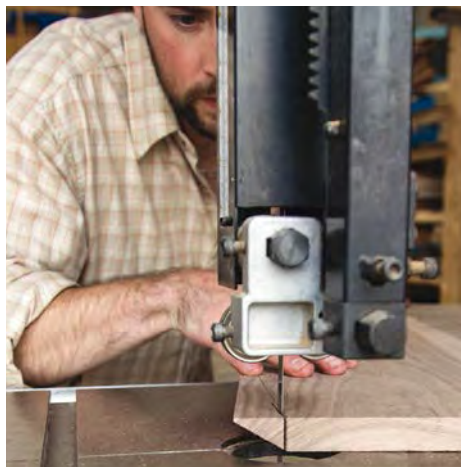
Roughing out the curve
