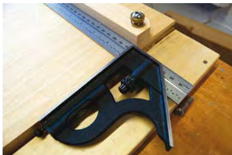
An accurate square helps adjust the position of the fence before tightening the thumbscrews
