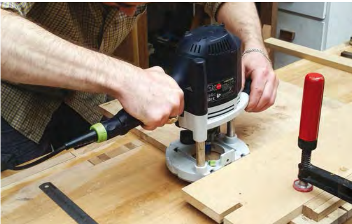
Routing the grooves for the dovetail strips
