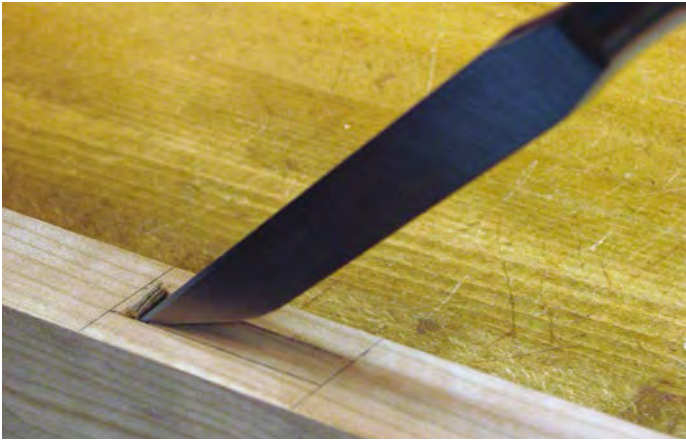
Levering out the first bit of waste
