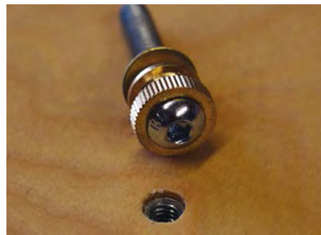
The thumbscrews fit into threaded inserts that have been fixed with epoxy into the deck of the shooting board
