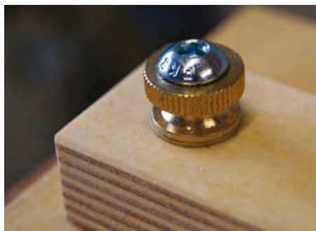
The fence is held in place with a pair of these knurled thumbscrews
