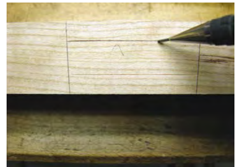
Tracing over marking gauge lines with 0.5mm pencil lead
