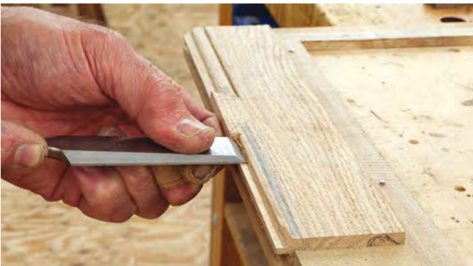
A rebate can be used to remove waste, leaving less work for the scratch stock
