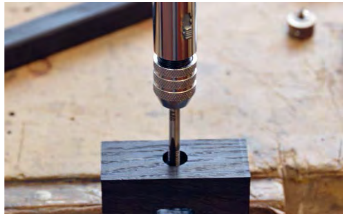
Cut your thread straight into the wood with a metal tap
