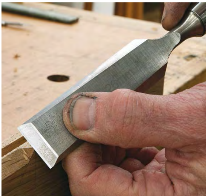
Cut the 45° stop to the chamfer with a chisel
