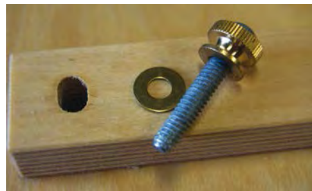
Evenfall Studios use oval holes in the fence and substantial thumbscrews to allow fine adjustment for seasonal movement while locking the fence down tight in use
