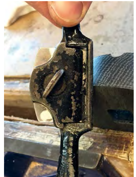
Soften all the edges with a chamfer
