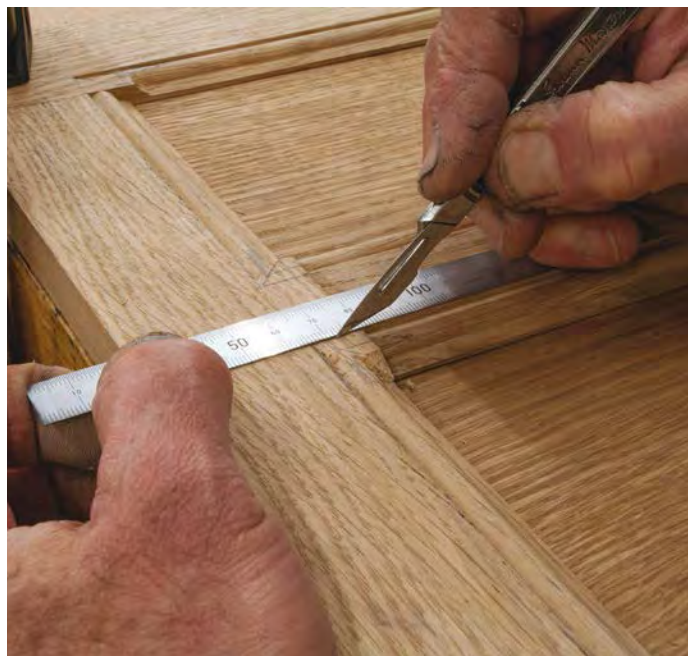
To start the mason's mitre, cut in the outside edge with a scalpel
