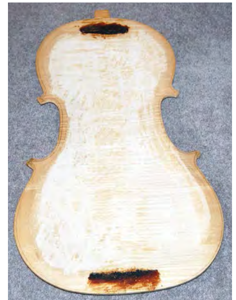
A foul-smelling animal glue was used to tack the front and back onto the mould to check for alignment
