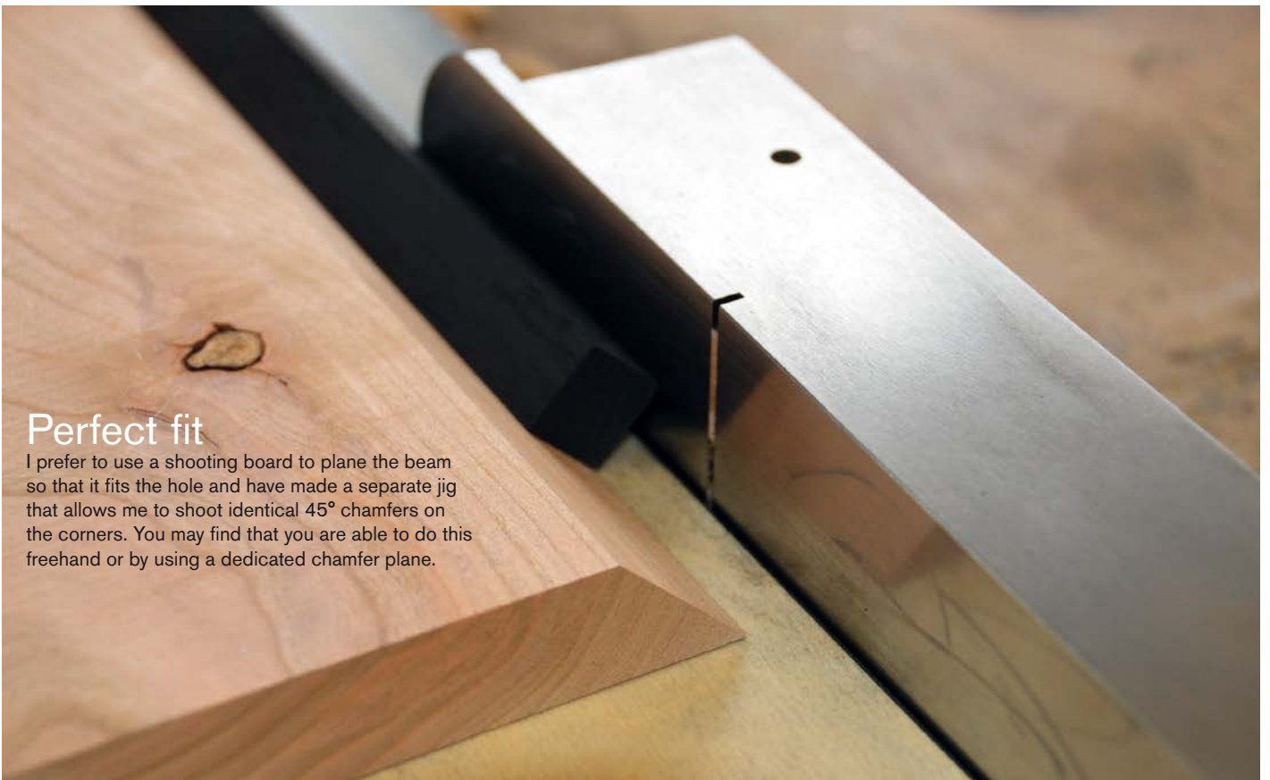
Convert your shooter to plane 45° with a simple jig
