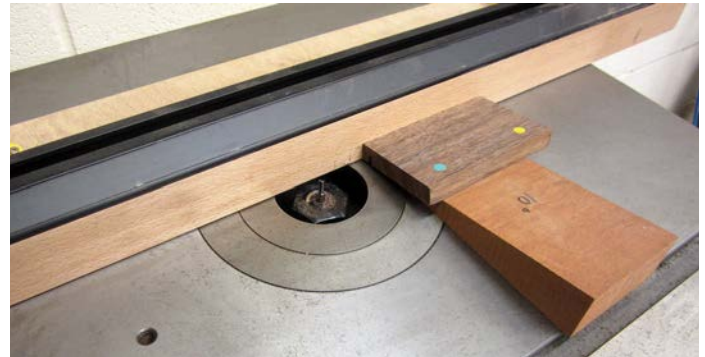
Slots for the base being carefully routed with a 10° block
