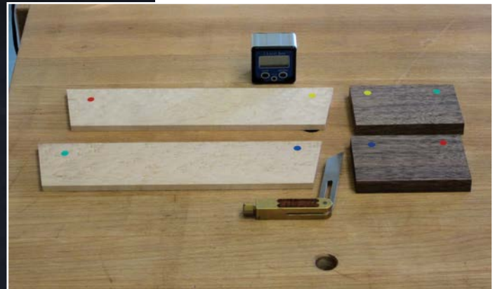
The sides cut to size, note the coloured dots which help you keep track of the pieces
