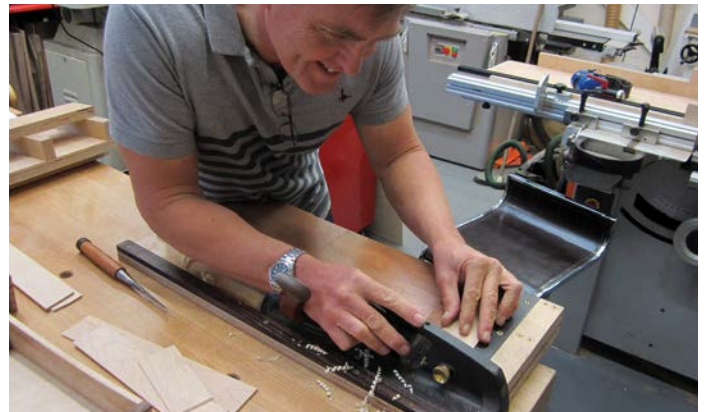
Trimming the lining on the shooting board
