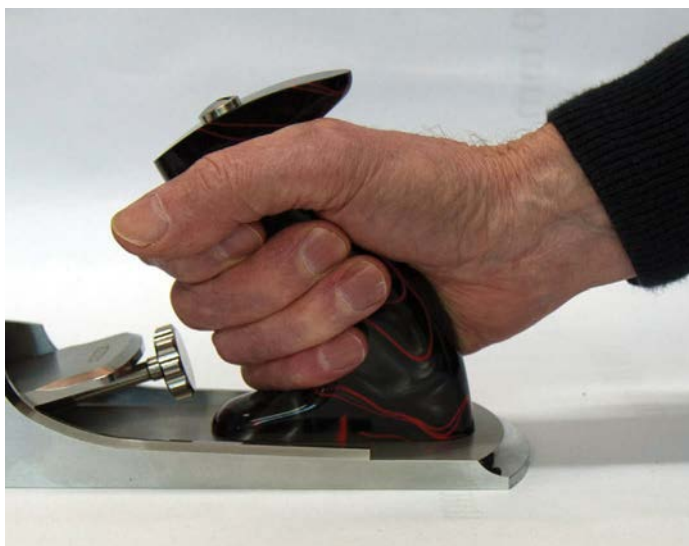
... but, in a normal planing stance the arm adds an even larger angle, so plane handles need to slope forward significantly for efficient and comfortable planing
