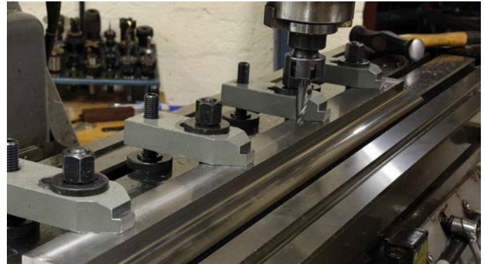
Lever caps are partly machined as a strip and then cut up before final machining to shape and hand polishing. There is still a lot of metal to be removed here...
