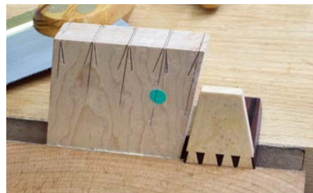
Angling the boards so that the cut is vertical
