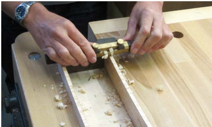
Cleaning up the curves with a spoke shave
