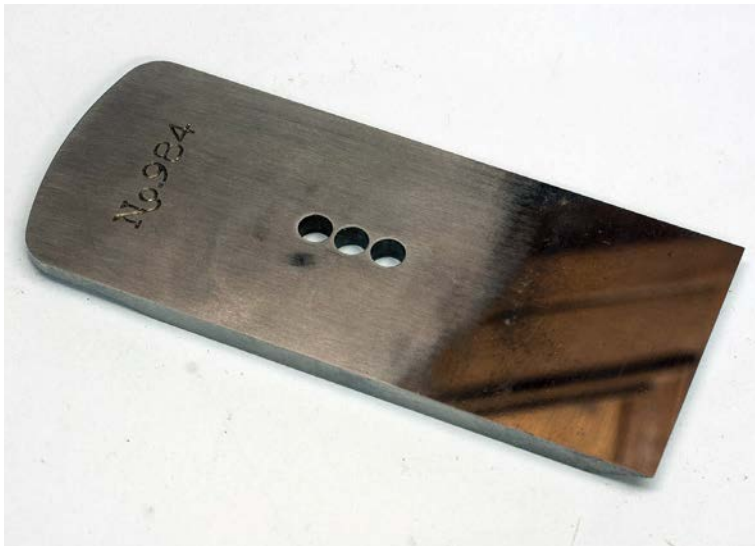
Full surface grinding makes polishing the back a doddle
