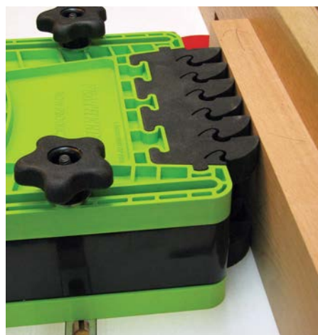
Stacking the Featherboard on thick stock gives even pressure across the face of the board
