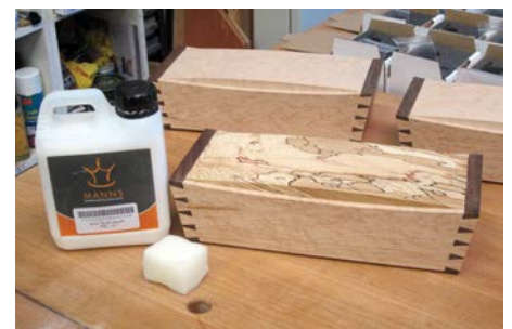
Finishing with a matte water-based varnish
