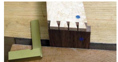
Marking the pins, ensuring the bottom edges are in line
