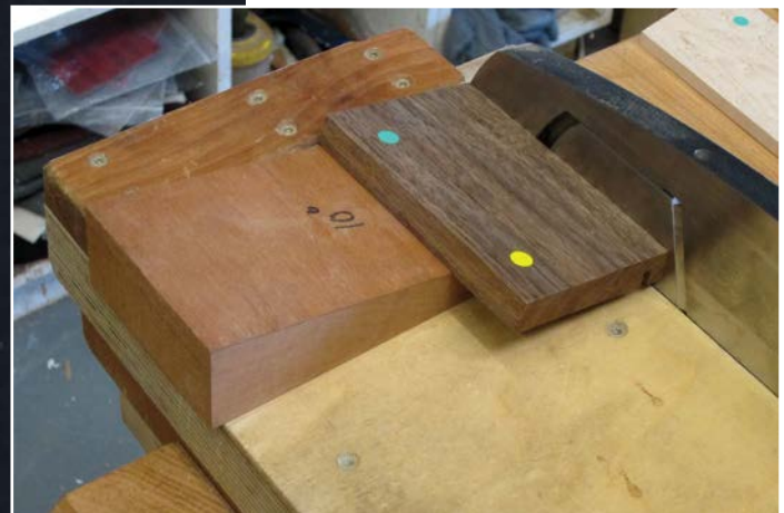
A 10° bevel being shot on the underside of the walnut ends
