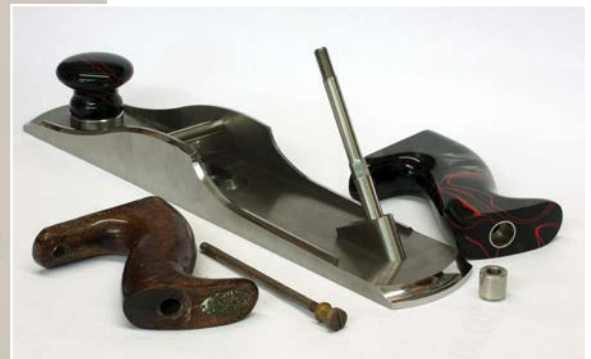
The rear handle fixing is much more substantial than that of the pre-war Record No. 5 shown alongside. Note the inset sleeve in the top of the handle into which the cylindrical fixing nut fits
