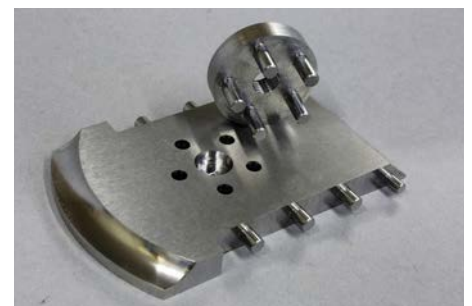
The front part of the 984's sole showing the integral rivets used to fix it to the sides. Also shown is the boss to which the front knob attaches
