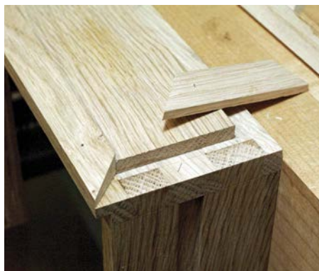
Mitred chamfered cushions hide the through dovetails
