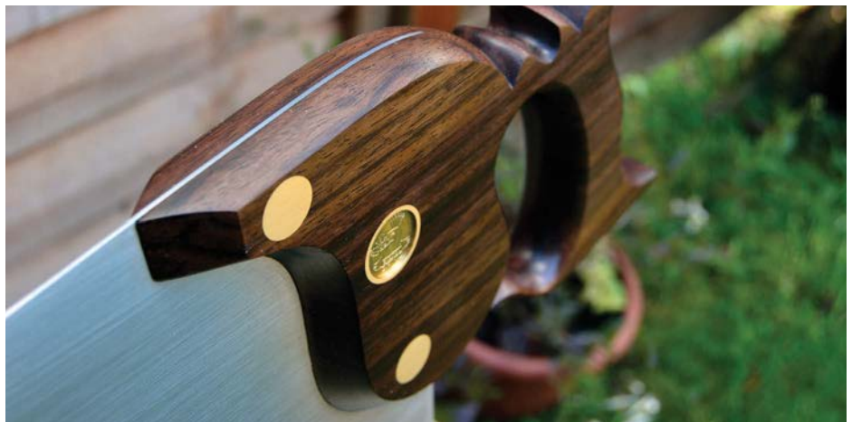
The curved top of the tote is incredibly elegant, particularly given that the saw plate is also curved to match the handle
