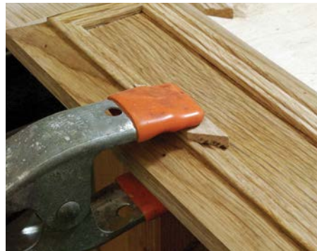
An upside-down offcut of moulding helps if you want to use a clamp
