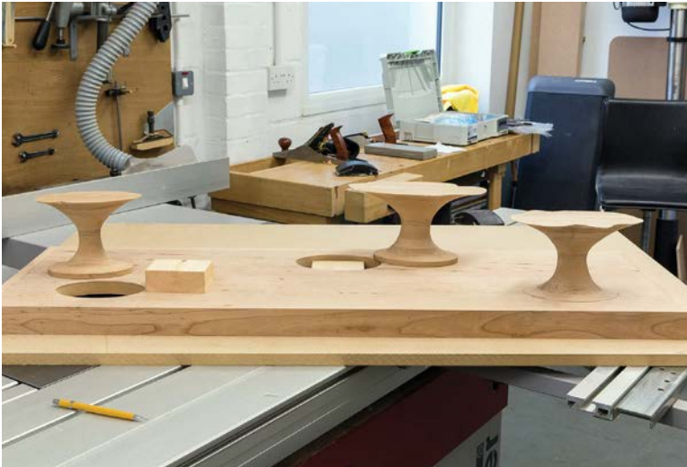
Assembling the islands to the table top
