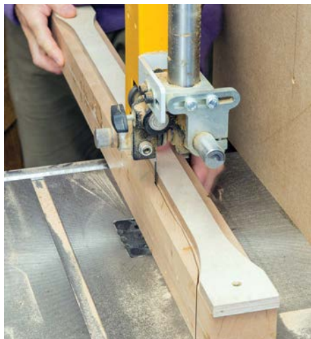
Bandsawing the table legs to rough profile
