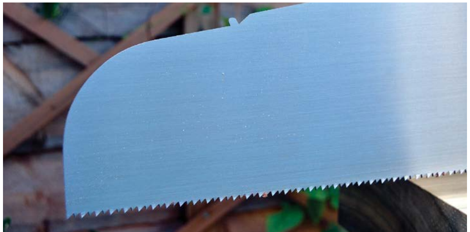
The Panel Saw has the same distinctive shape as the saw plate of the Kenyon saw, including the nib
