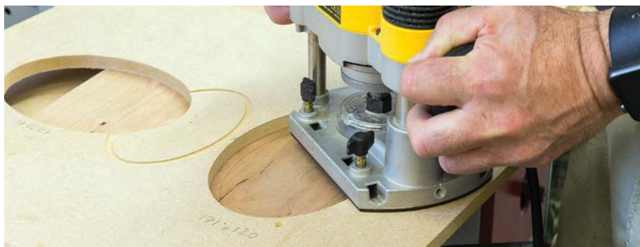
Hole for the island being routed out
