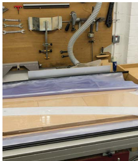
Vacuum pressing the veneers to the MDF substrate
