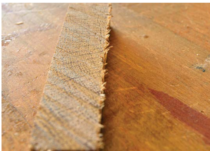
Even on this splintery oak, the Panel Saw cut smoothly and minimised blowing out splinters on the exit side of the workpiece
