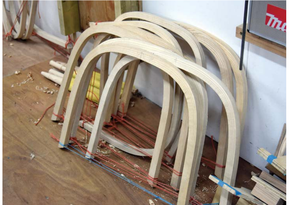
Back rails held in tension before fitting
