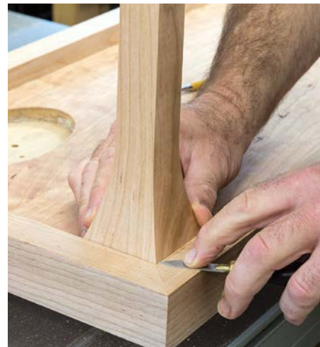
Scribing the top of the leg to the table frame
