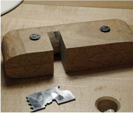
Moulding the scratch-stock and finished sharpened cutter
