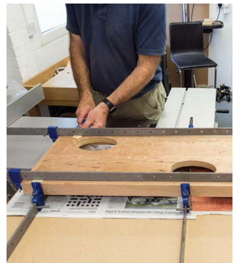
Assembling the table top frame and veneered panel
