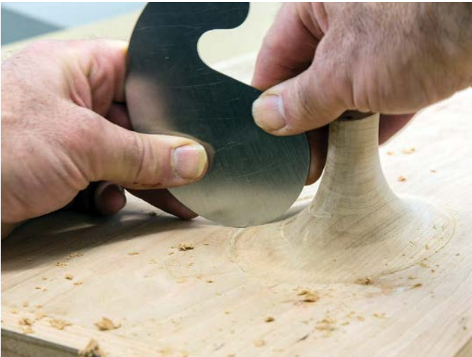
Finishing the interface of an island to table top with a curved scraper
