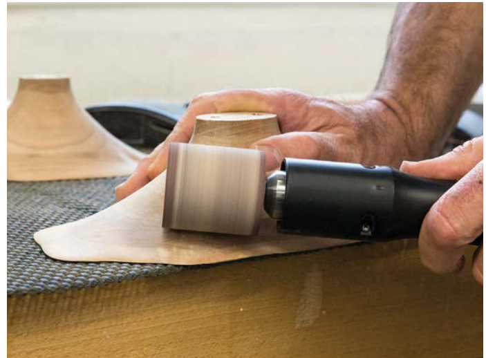
Finish sanding an island top with Kirjes sanding drum
