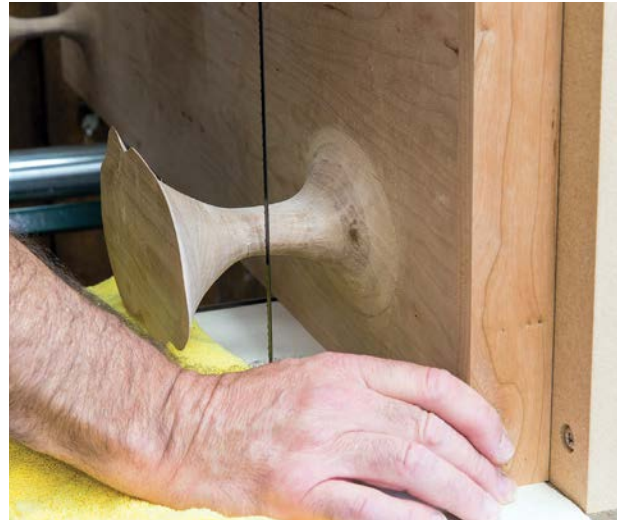
Parting the island tops at glass level
