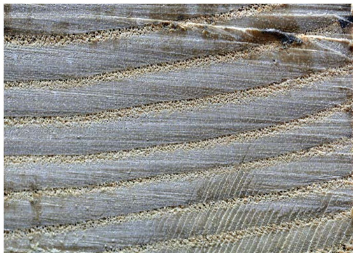
Despite being a coarse tooth profile, the Panel Saw leaves behind a good surface that won't take too much effort to clean up
