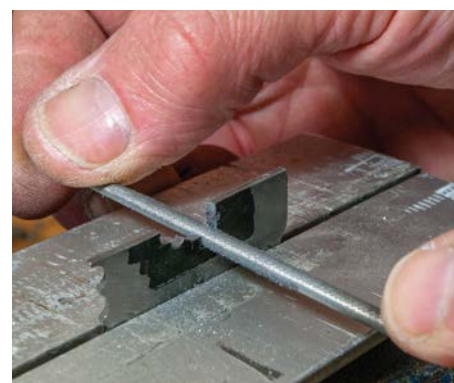
File the scratch-stock cutter to your chosen profile
