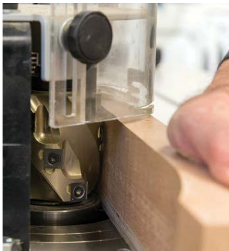
Spindle moulding the table legs to finished profile
