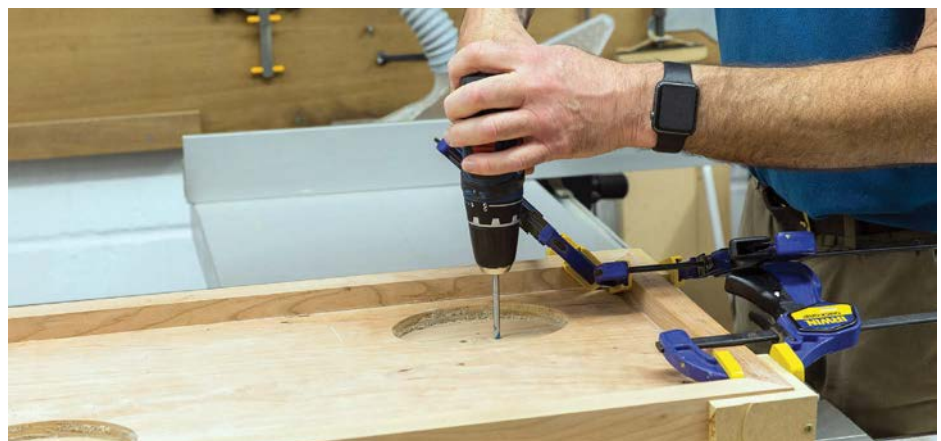
Drilling the glass template through the island reference holes
