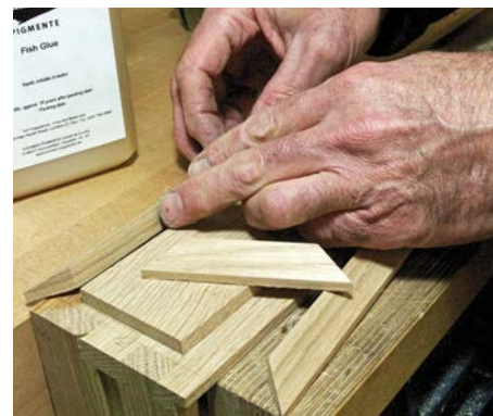
The cushion mouldings are glued and pinned
