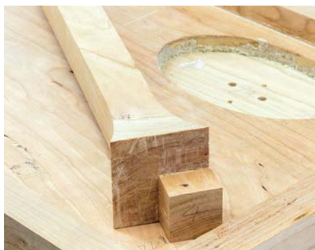
Finished leg joint ready for glueing up
