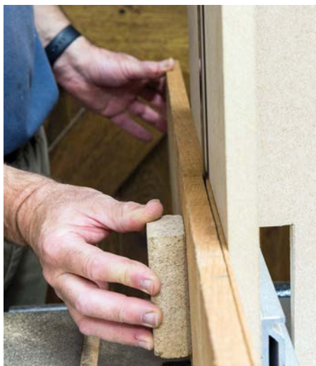
Bandsawing the veneers for the table top
