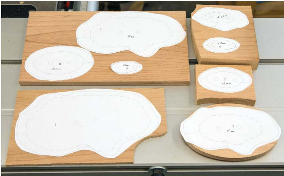
Templates on the cherry blanks ready for bandsawing
