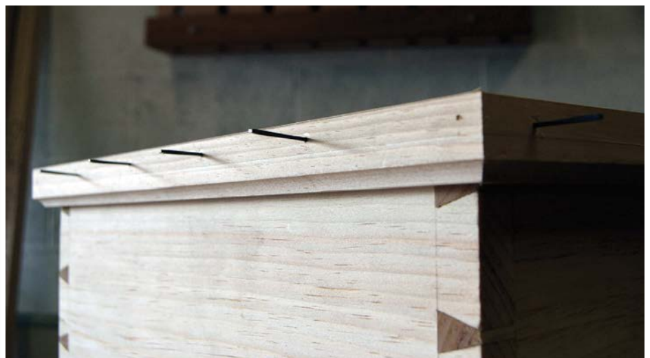
Cut nails hold moulding in place and allow for seasonal movement of the lid
