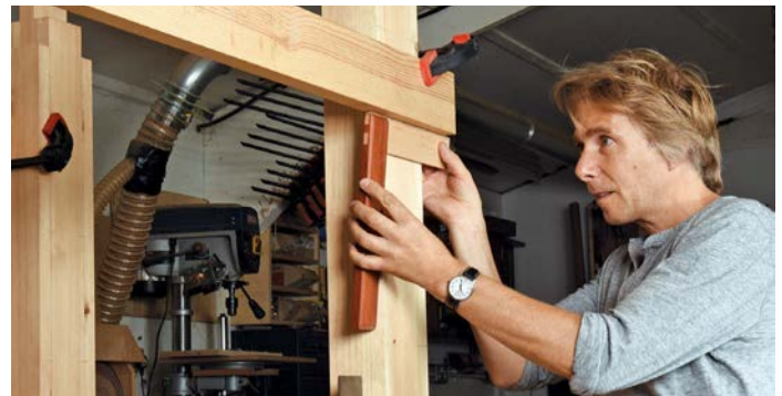
Clamp the rails in place to hold the legs in position
