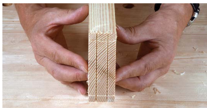
Use the bandsaw to create a kerf for a hand saw
