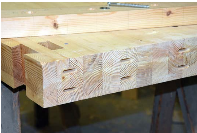
Loose tenons on quartersawn stock is the most stable solution
