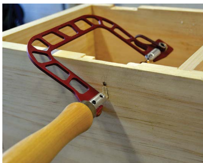
Cutting the keyhole for the School Box lock
