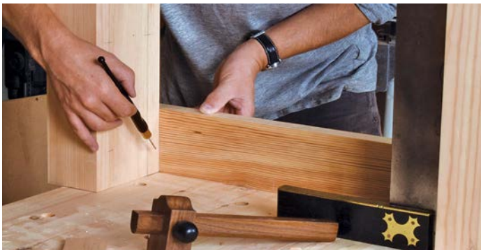
Mark the shoulder lines close to the work top
