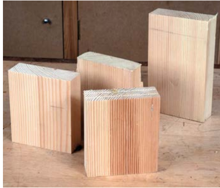
Look for a quartersawn pattern with pin straight grain on all four sides
