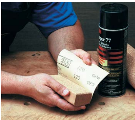
The author's favorite sanding block is lined with ¼-in.-thick cork and is sized to fit his hand comfortably.
