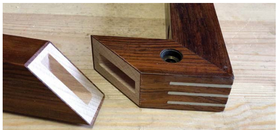
Rosewood legs cut and mortised
