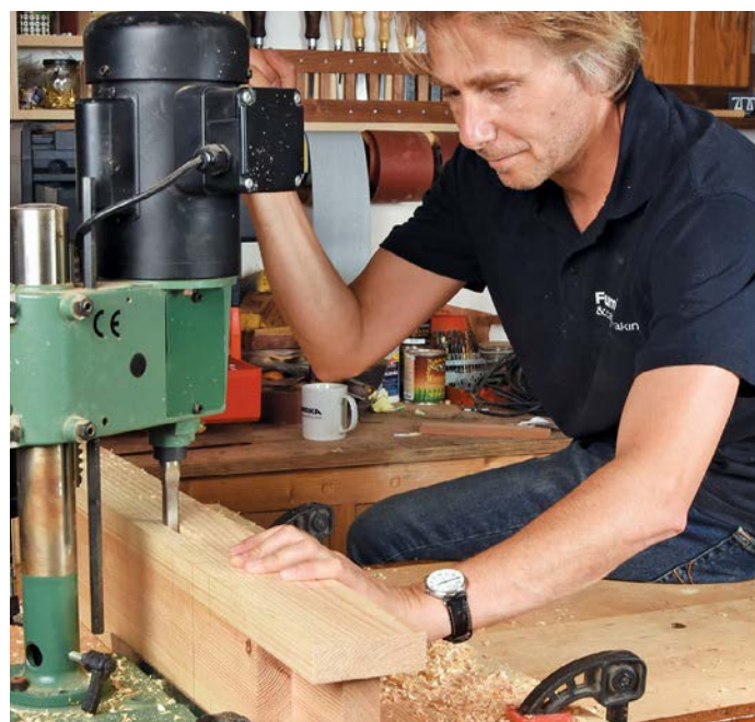
Gain extra height on your bench top mortiser by rotating the body to work away from the base
