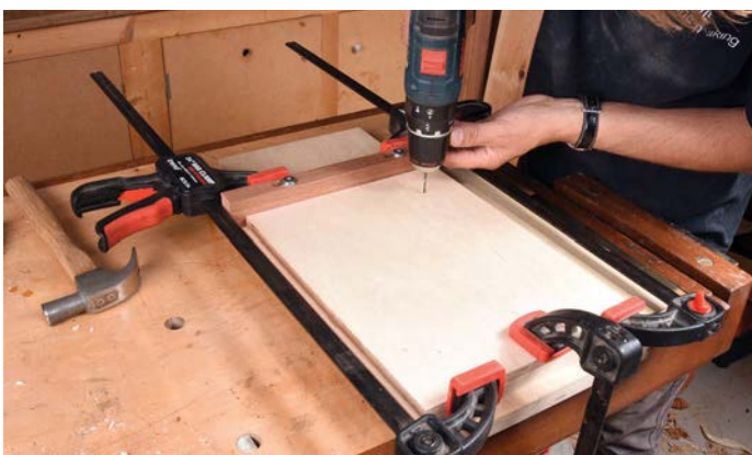
Clamp the components tight in registration if you drill the pilot holes by hand
