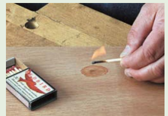
2. Touch the drop with the tip of a lit match. The alcohol will burn with an almost imperceptible blue flame. It will expand rapidly as it burns, causing the crushed wood in the dent to swell.
