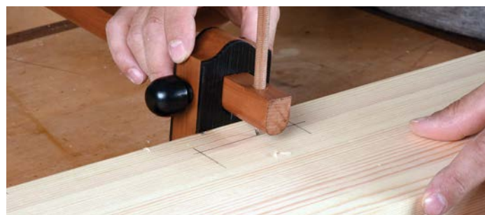
For big mortises a pencil line is adequate and there's no need to mark every boundary
