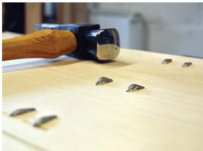
Nail clinching is an often overlooked, but very valuable joinery technique
