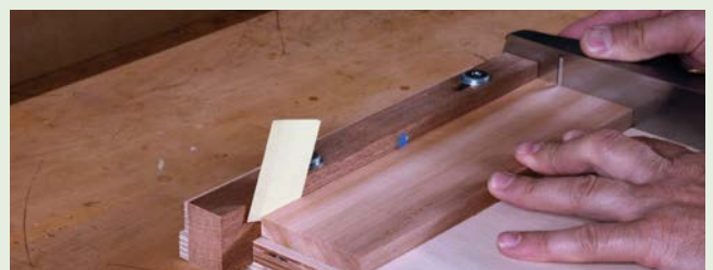
Make micro adjustments to the 90° angle by inserting a spacer between the workpiece and the back stop
