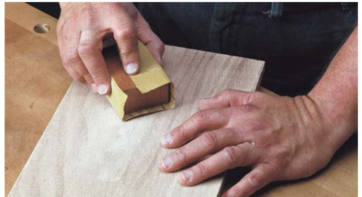
Sand until the original shape of the gouge is clearly outlined.
