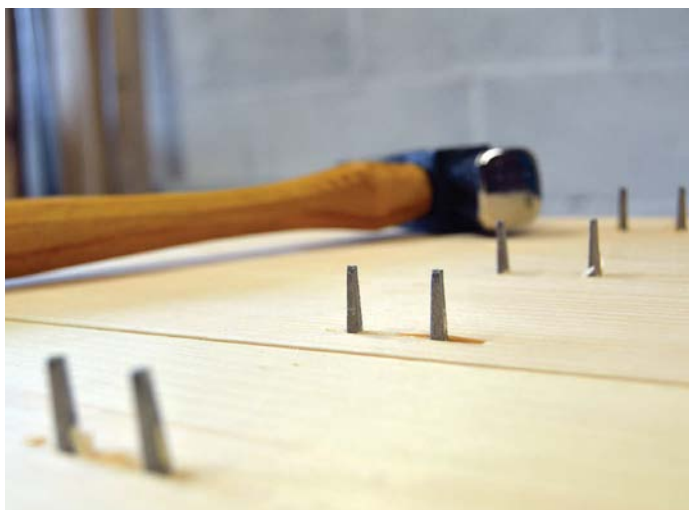
Cut nails waiting to be clinched
