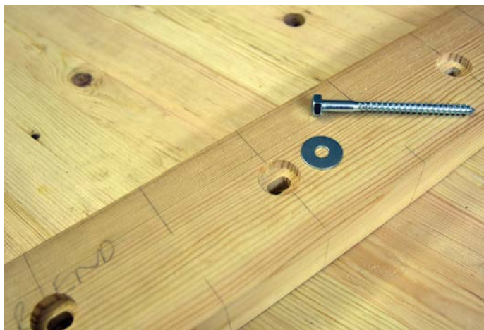
Cut slots for the bolts and use washers to avoid compression around the holes
