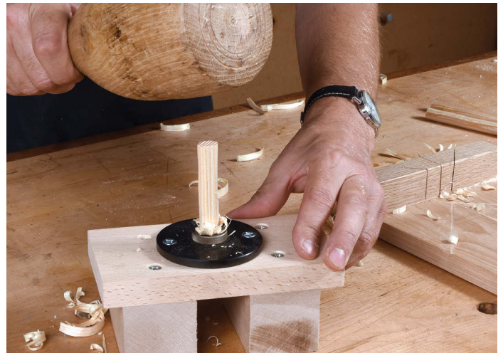
Use a dowel plate in decreasing sizes to knock off the corners
