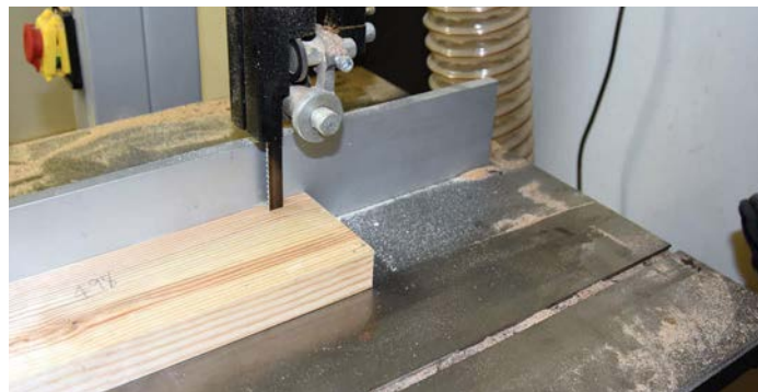
Shallow cuts can be made on the bandsaw without deflection
