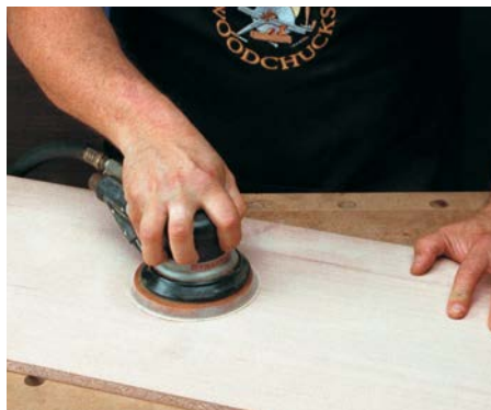
Pressing down on a random-orbit sander will slow its progress and will leave scratches in the wood. Let the weight of the sander alone do the work.
