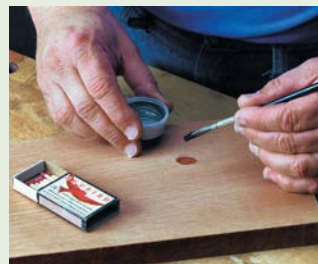
1. To raise a dent with alcohol instead of water, place one drop of denatured alcohol into the depression with a fine touch-up brush or toothpick.
