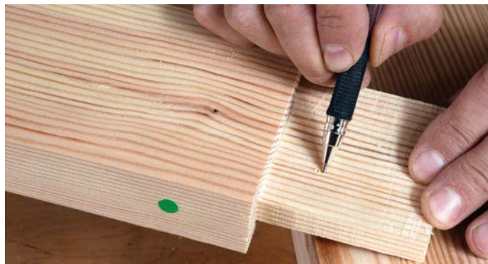
Re-mark the hole position a few millimetres back towards the shoulder for final drilling
