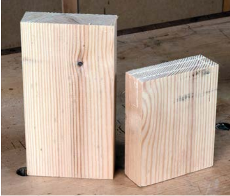
Reject offcuts that have even the slightest defect or deviation in grain direction
