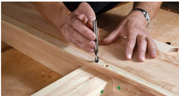
Use a spurred drill bit to make an initial mark on the tenon
