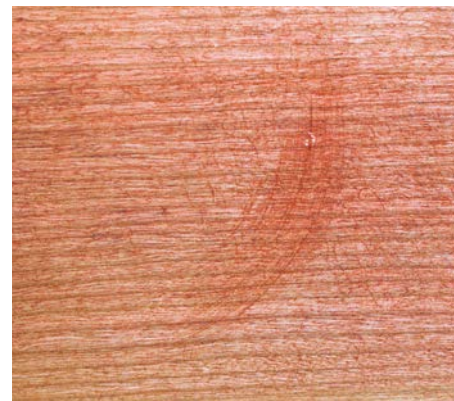
Swirls in the wood are caused by pushing down on the sander.
