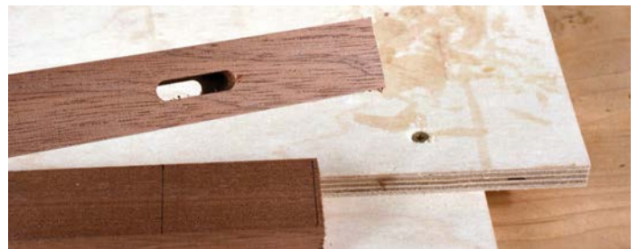
The Festool mortise can easily become a through slot
