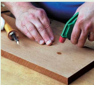
1. With the wood horizontal, place several drops of water into the dent.
