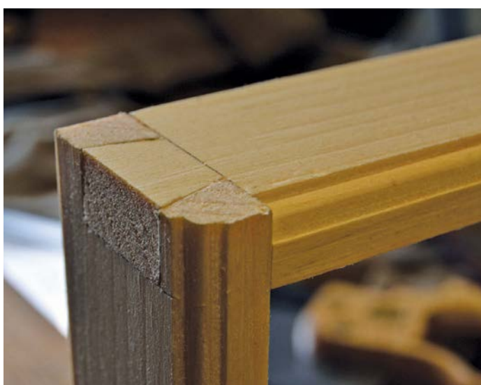
Dovetailed base moulding for the School Box – as well as dovetailing this project introduces the reader to making short runs of moulding
