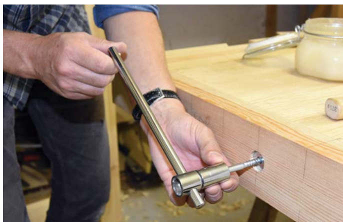
Push the washers into the clearance hole for the bolt head before tightening
