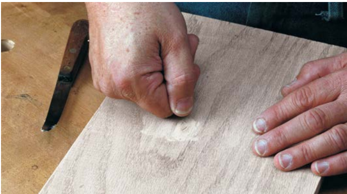
Putty will shrink as it hardens, so let it protrude slightly above the surrounding surface. The putty is ready to sand when it will not take an impression from your thumbnail.
