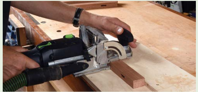
Use a bench hook to mortise thin components
