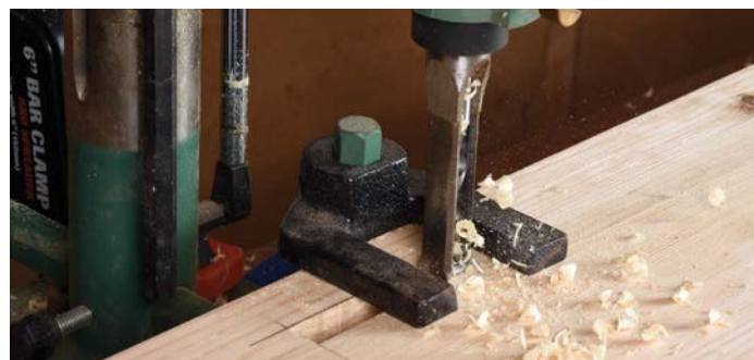
Opt for a mortise that can be cut in a single row
