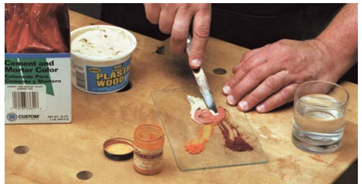
If you can’t find a putty that matches the wood, mix a custom color from “natural” putty and cement colors from your local hardware or home store, touch-up powders from wood specialty stores, or artist’s fresco powders. If the putty starts to get too thick, add a few drops of the thinning solvent listed on the container.
