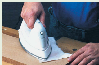
2. Cover the spot with a slightly damp cloth and place a hot knife or iron directly over the drop. Hold it there, checking frequently, until the spot is dry. If the dent is not completely out, repeat the process.
