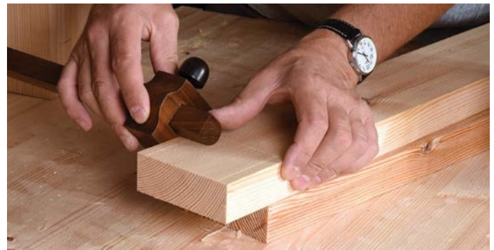
Mark the tenons with a pin gauge
