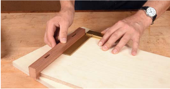
The back stop must have parallel sides to maintain 90°
