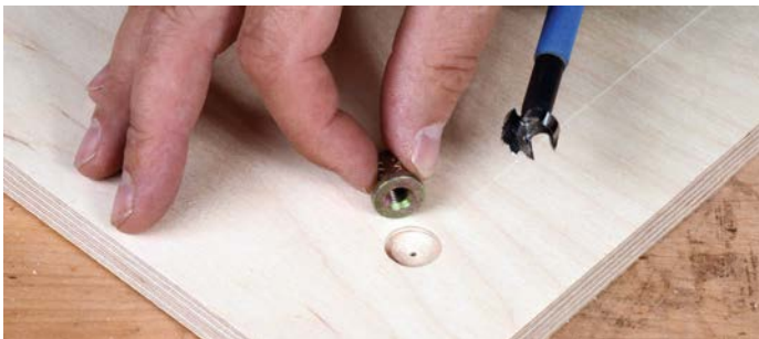
Use a Forstner bit centred on a pilot hole to recess the fixings
