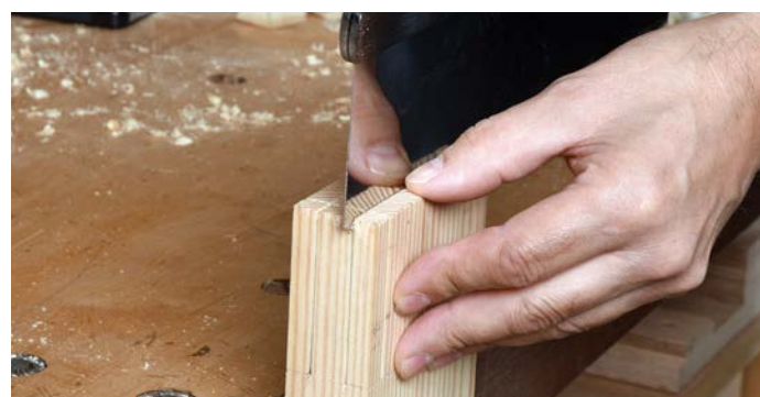
Push the saw plate over to the inside of the kerf
