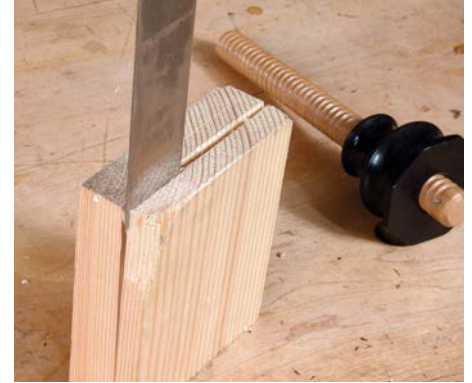
Split the blanks and resist the temptation to saw
