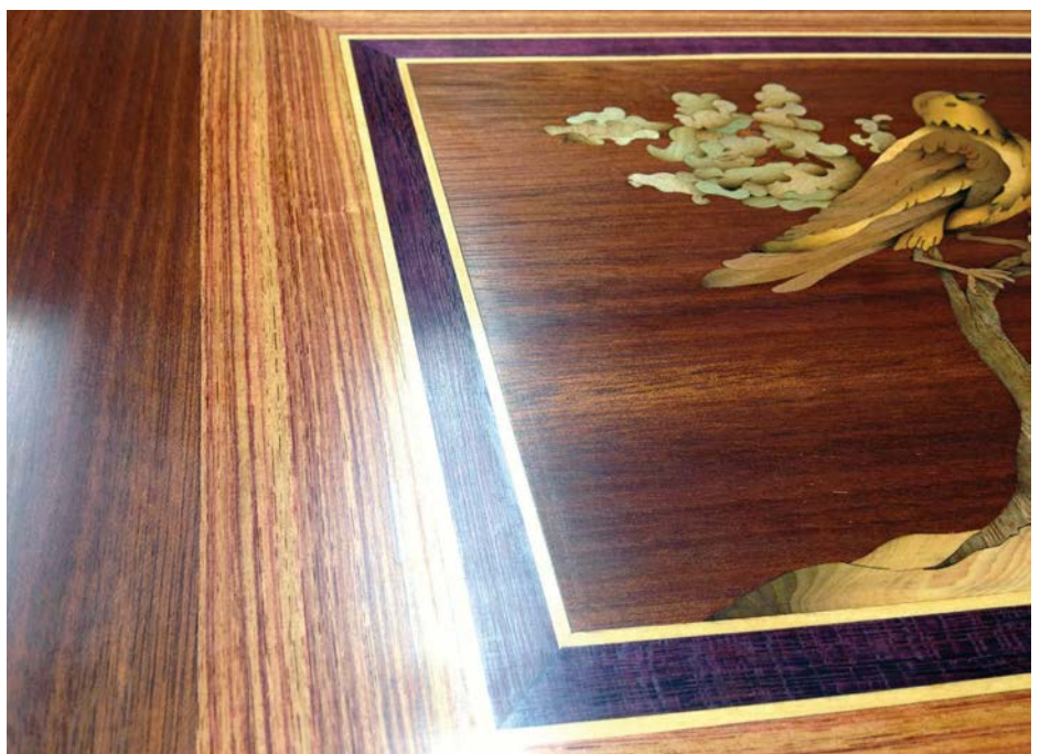
A perfectly pore filled surface. Notice the satin sheen and even appearance
