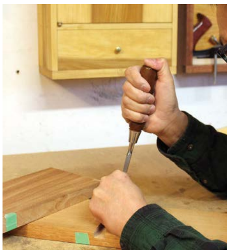
Secure the work piece to your bench and use a chisel to adjust the walls of the housing
