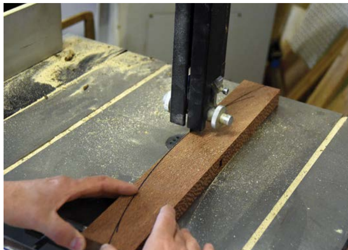
Leave as much material in tact as you can while shaping
