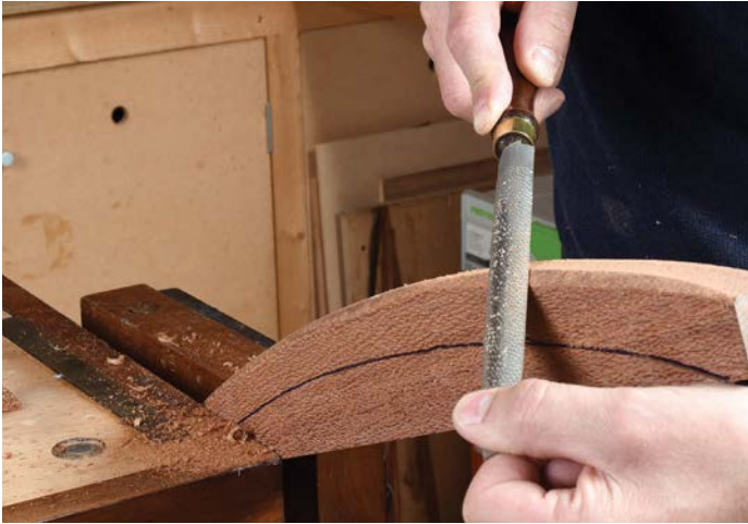
A coarse rasp removes material quickly and doesn't need sharpening
