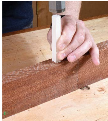
Drive the wedge in to complete the joint
