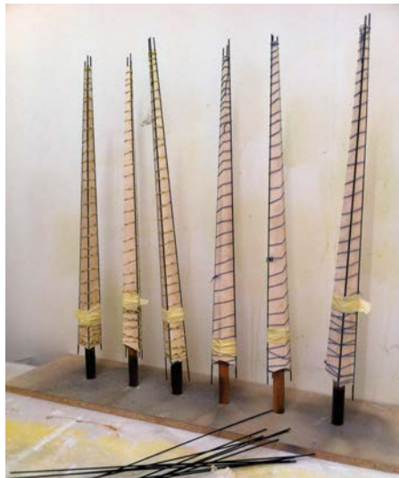
Gluing in the stringing lines on three of the four corners of each leg using 1mm plastic coated wire
