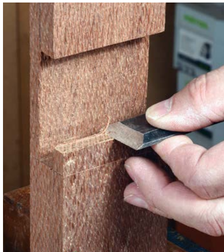
Remove the waste with a chisel
