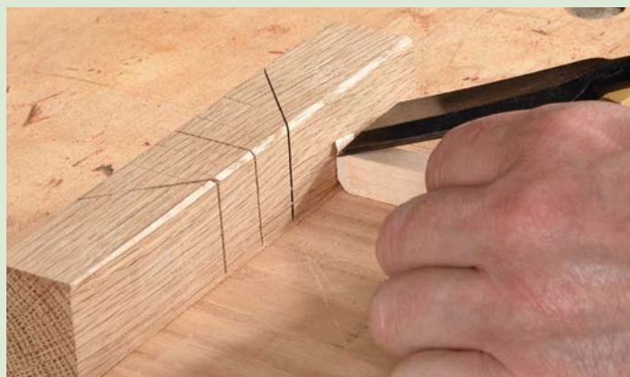
Chamfer the tip of the wedge to keep it on track
