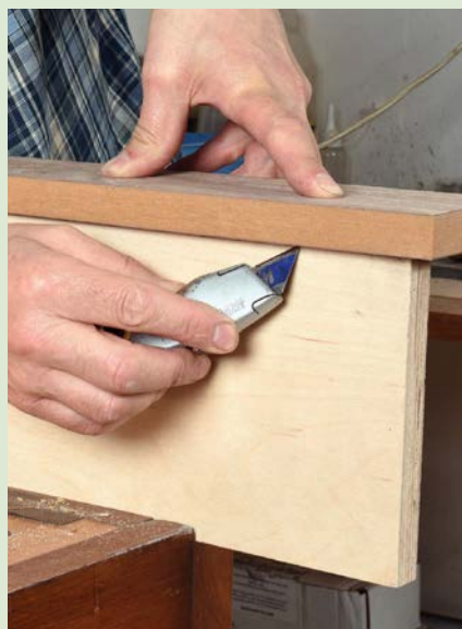
Make a series of light scores to remove excess rather than one heavy cut
