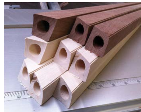
The legs shaped, jointed and rebated ready to take the stringing
