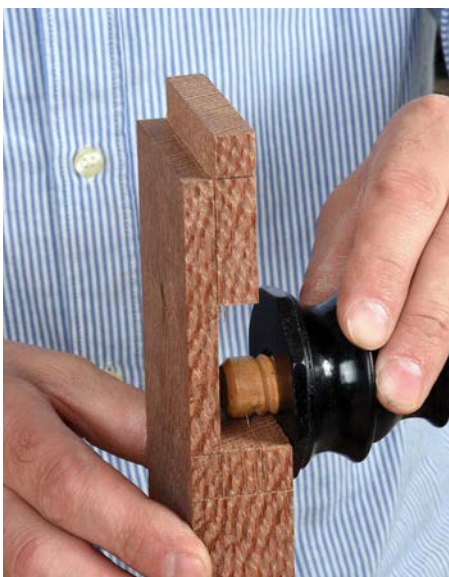
You'll have to gauge up twice so make sure you have a gauge that can get into tight spaces
