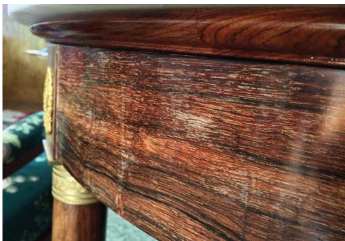
White pores appear over time as a result of improper poor filling
