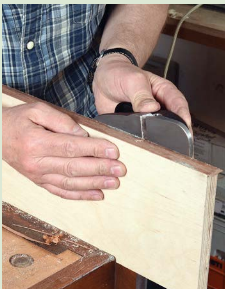
A scraper plane can level and square the corners of the veneer with less risk of tear-out
