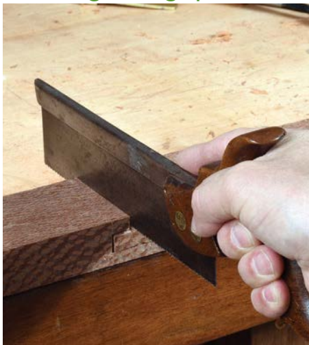
Cut partway through the joint line
