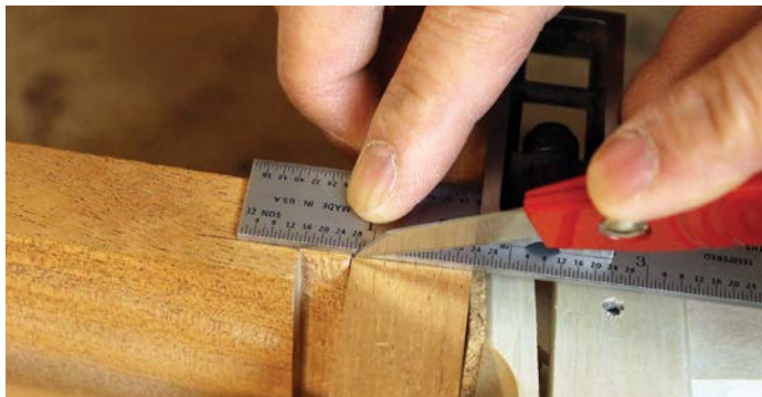
Position the dovetail against the adjacent board and transfer the narrow tongue base to the edge of the board
