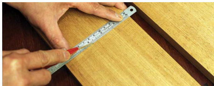
Scribe the taper lines and make knife walls to guide the sawing
