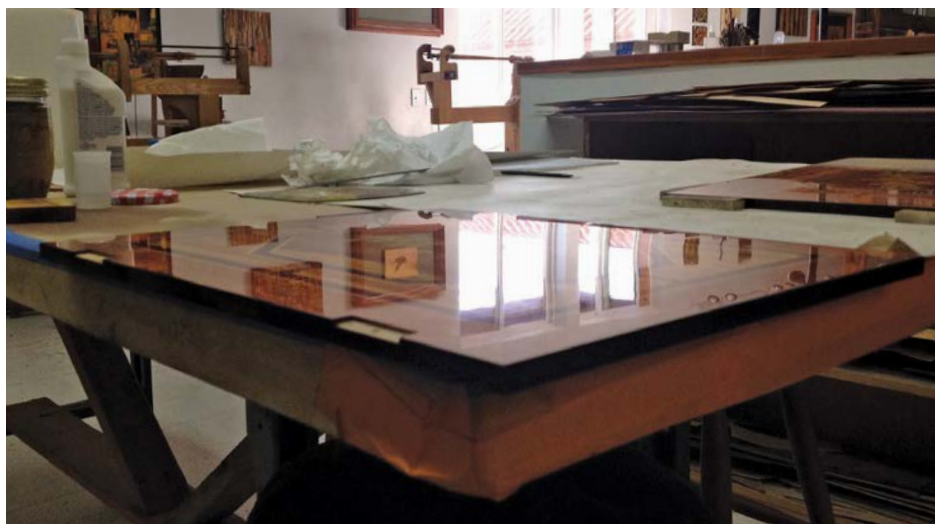
Using raking light to check a nicely polished surface
