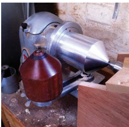
Turned cones for shaping the shoulder of the legs. The wooden one is showing signs of degradation from friction
