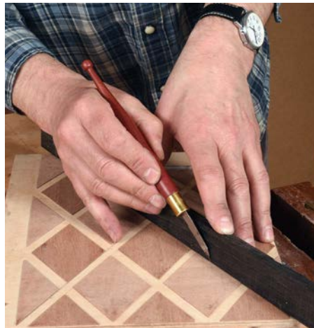
Use a second template or the inlay material to mark up the opposite edge of the groove
