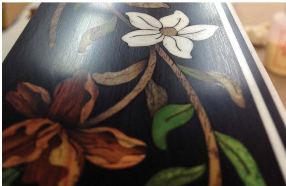
An example of ebony dust being transferred to the pores around it. Some transfer is unavoidable but careful attention can reduce the amount greatly
