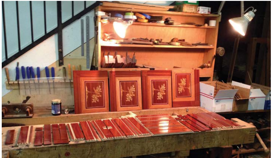
Using an overhead light to check the surfaces of the panels
