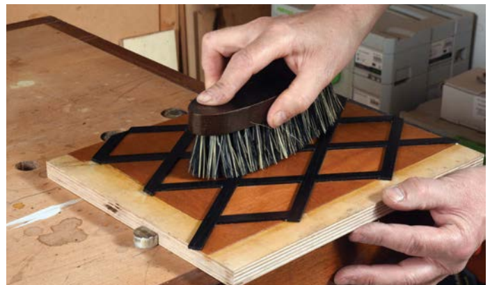
Use a brush when the wax has dried and buff to a shine
