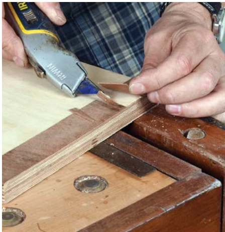
Peel away the offcut from beneath and iron the two edges down
