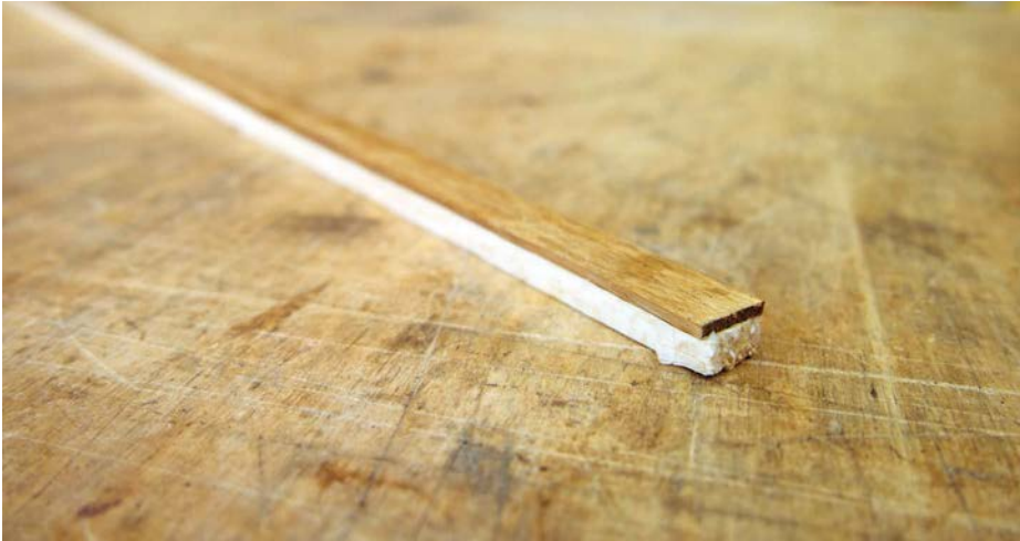
Sliver made of balsa veneered with oak
