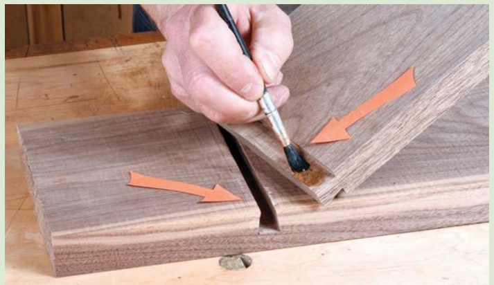
A tight joint will hold the parts together, glue keeps them aligned at one end
