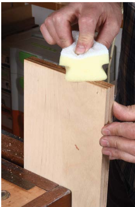
A light application of water from a damp sponge is sufficient
