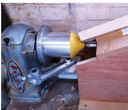
The modified sanding disc stuck neatly onto the cone. The leg is mounted in a cradle over the lathe ready for shaping the shoulder
