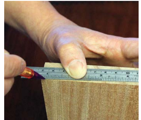
Connect the tail points on the top edges to lay out the taper lines on the endgrain
