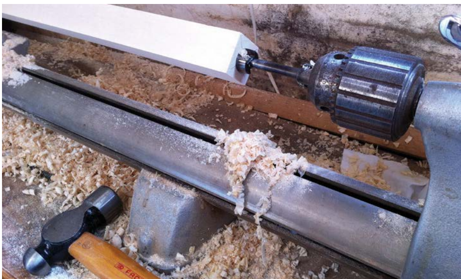
Using the lathe to bore a hole in the end of a leg with a Forstner bit
