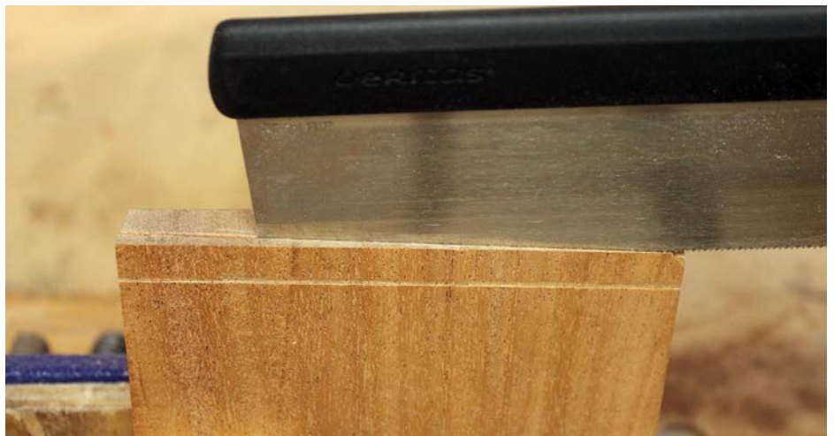
Given the tendency to arc the bottom of the kerf, I made a few more saw strokes in the middle part to remove that high bit
