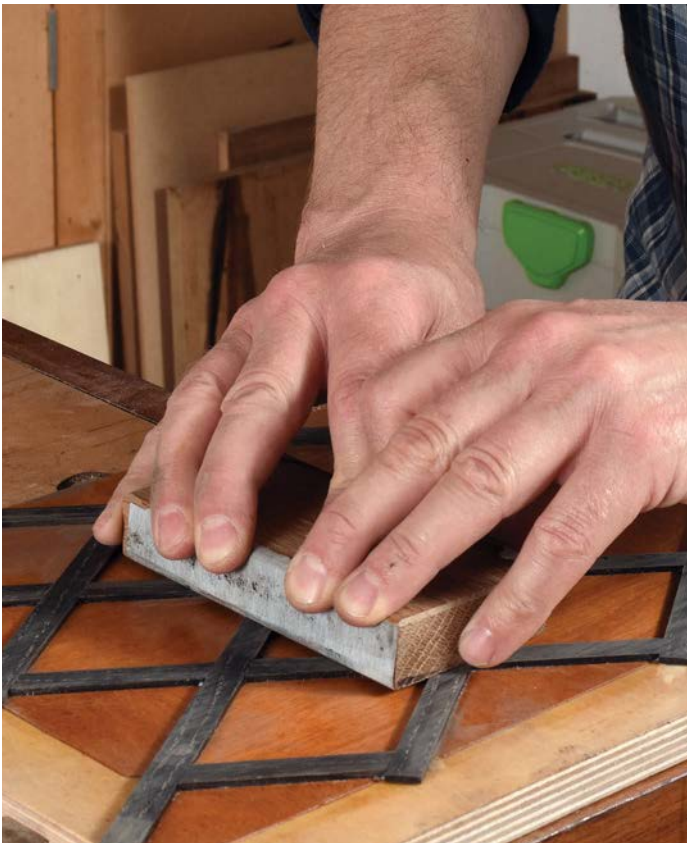
Use a wide block to sand the raised infills so you don't damage the polished background
