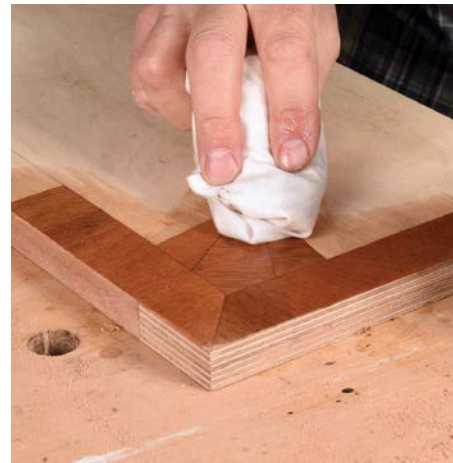
Test with meths to gauge the strength of your glue layer
