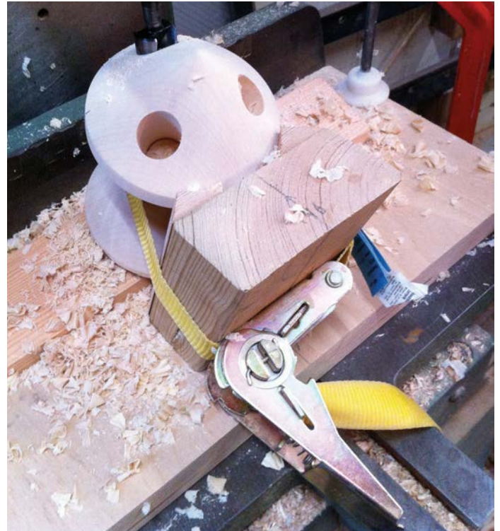
The boss is securely mounted in a pillar drill and held fast with a band clamp
