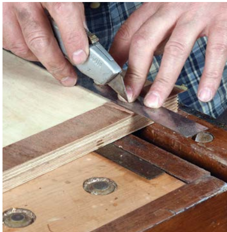
Lay the second piece directly over the first piece and cut through them at the same time to make the joint
