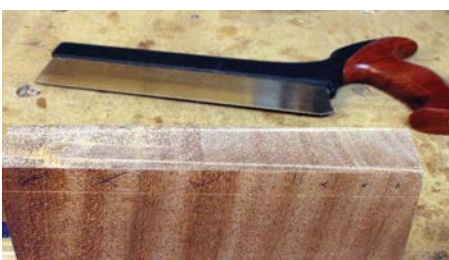
The shallow guide kerfs are no deeper than the saw teeth
