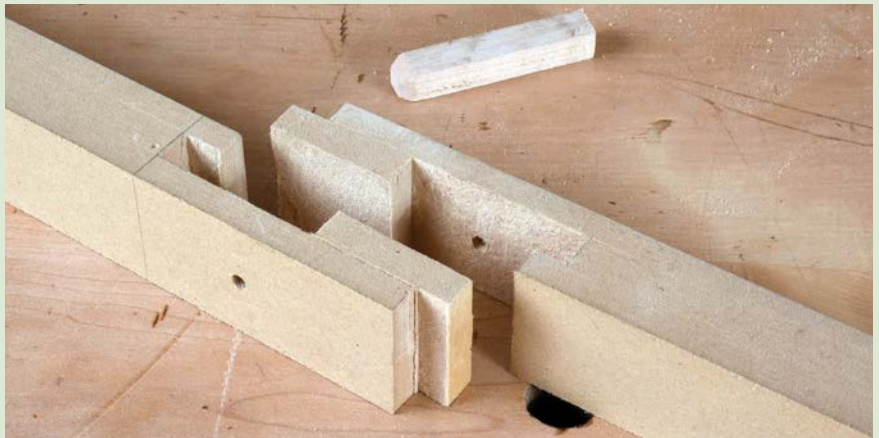
An MDF test piece shows all the major parts of the joint and how the voids are to be filled
