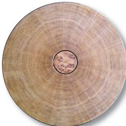
Horizontal slice of oak veneer showing medullary rays with burr oak roundel
