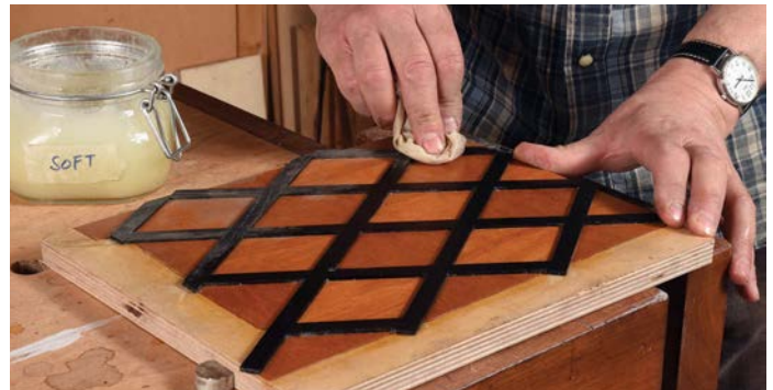
A soft beeswax polish combined with a little black sawdust from sanding is a no-nonsense finish for dark timbers like bog oak
