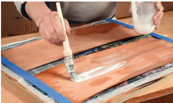
Apply the first thinned coat of glue to the back side of the veneer
