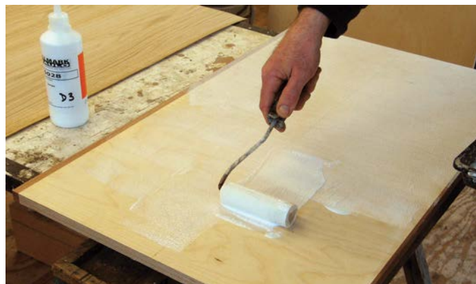
Gloss paint rollers work well once they are full of glue
