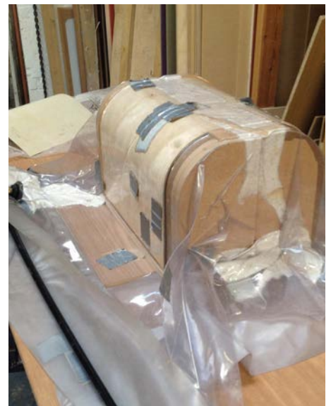
Door former in vacuum bag
