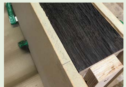
Removing the damaged veneer from the front leg
