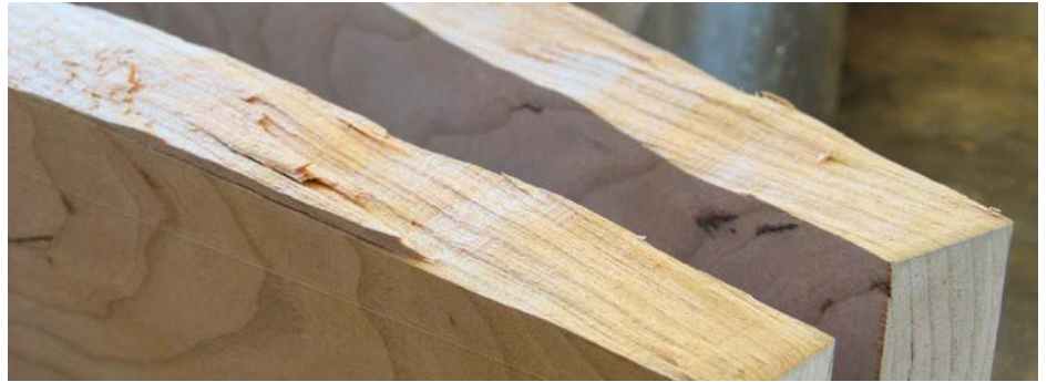
A nasty ragged break shows that the glue is still 'stronger than the wood itself'
