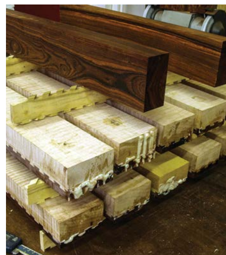
A stack of T21 bodies with sole and body bonded with polyurethane glue
