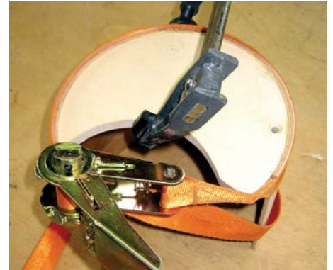
A strap clamp works nicely when gluing the round backs in place
