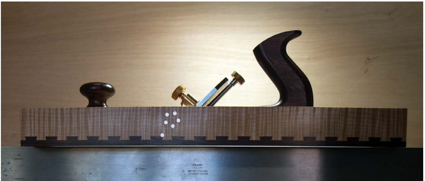
Here the sole shows longitudinal concavity of the sole of about .0020in due to wood movement caused by changes in environmental humidity
