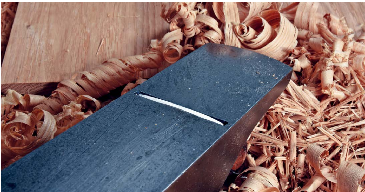
A new plane from old steel. Giving a cranky old No. 5 a new lease of life
