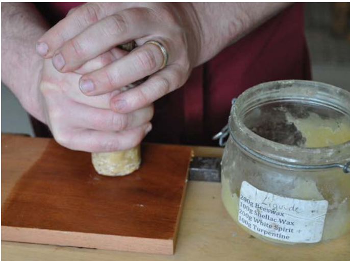
Rubbing the polissoir hard on the surface will polish the wood (fine sanding), fill the grain and lay a coat of melted wax all at the same time
