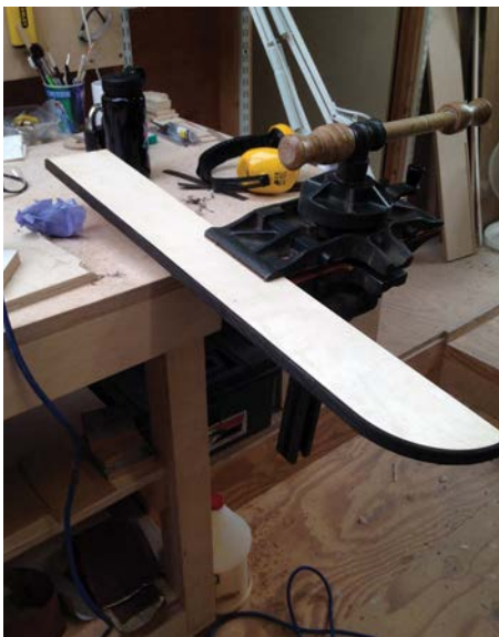
Leg panel is held in the pattern maker's vice while the lipping is flushed off
