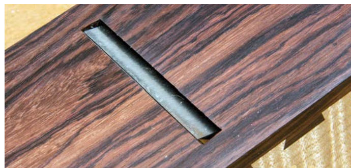
The mouth is fine but not superfine as befits a jointer that may be used to take quite thick shavings
