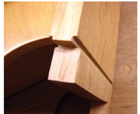
Grooves in the drawer support are used to locate the drawer housing
