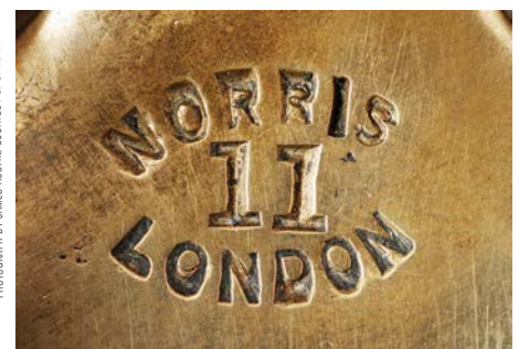
The maker's mark and model number in an ellipse on the lever cap
