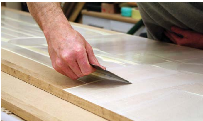
A notched spreader is great for fast, even spreading over a large area
