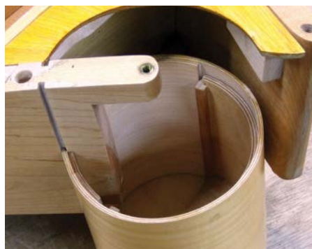
Test fit the housing on the mounting arm and assess the need for any adjustments to the drawer and components
