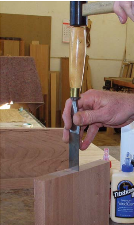
Glue can be checked for strength by using a chisel to try to split the wood along the glue line
