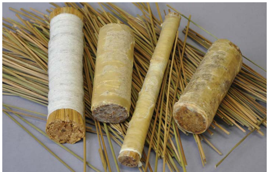
Modern polissoirs. The polissoir on the left has not yet been filled with beeswax. The others have been soaked in molten wax
