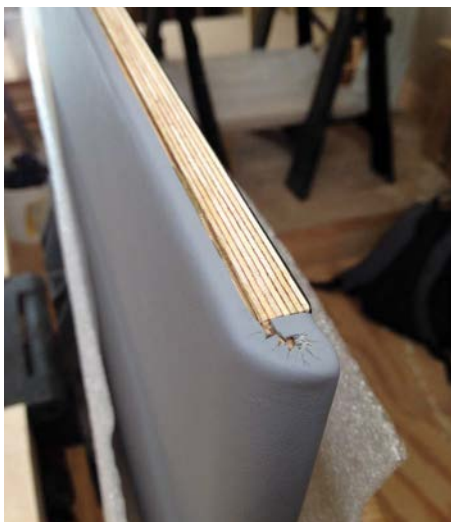
Edges of leather are carefully wrapped and glued into rebates with contact adhesive
