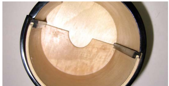
Use off-cuts from the drawer to locate the position of the drawer box within the housing
