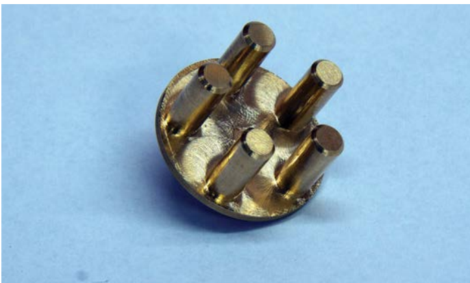
The 'spider' is a real challenge to make but an elegant way of transferring the clamping stresses of the lever cap into the plane's wooden sides
