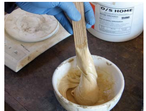
The 'custard technique' of adding only half the water for the initial mix avoids embarrassing lumps
