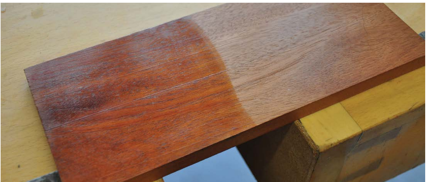
This sample of plantation mahogany came straight out of the planer/thicknesser with an open grain and was finished with the polissoir. Unfinished surfaces like the one in the photo are, of course, not recommended for fine cabinet manufacture but this picture illustrates that, even on very poorly finished timber, a wax polissoir will work its miracle. The waxing and polishing happens almost immediately, no oil or grain filling being necessary
