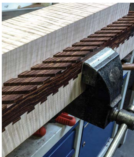
Both the sole and body have machined dovetail slots at 45° allowing the two to be slid diagonally together
