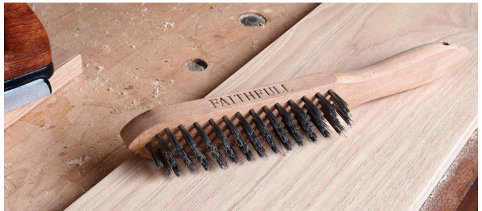
A heavy-duty wire brush will remove all the dust and pith from the grain
