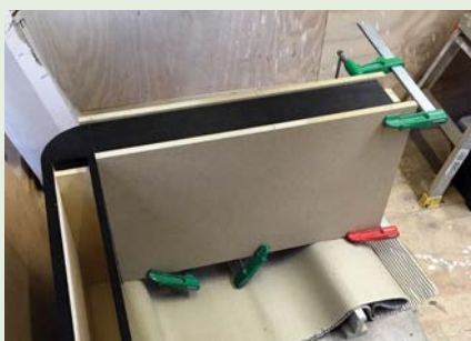
MDF panels clamped to leg
