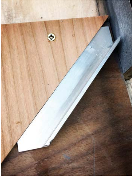
The metalwork shooting jig is used to produce crisp and flat polished surfaces
