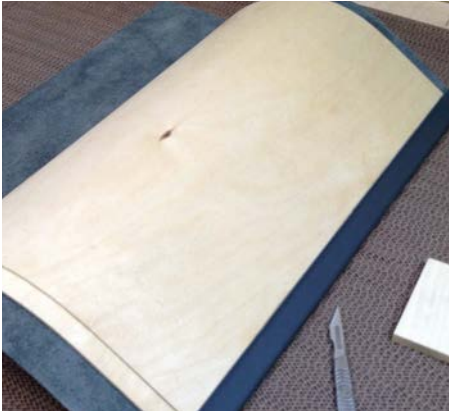
Interior curved door component being clad with leather
