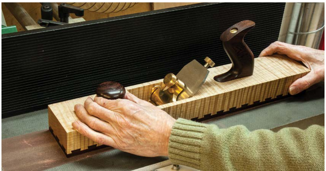
When abrading the sole of a plane to remove longitudinal concavity it is important to avoid downward pressure in the centre which might distort the body
