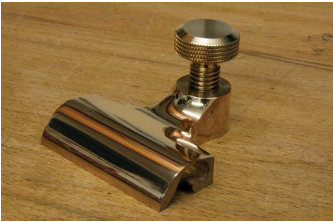
The lever cap has scroll recesses that locate over pegs on the gunmetal 'spider' bonded into the plane sides. The cap screw has finely machined knurling and square thread for long life
