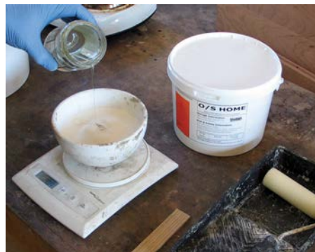
Powdered UF glues must have the powder and water measured accurately to ensure success
