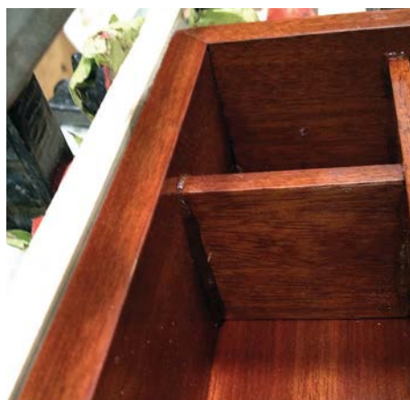
Excess squeeze out can be cleaned with cold water and a cloth
