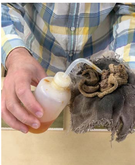
Squirt the alcohol or shellac onto the core
