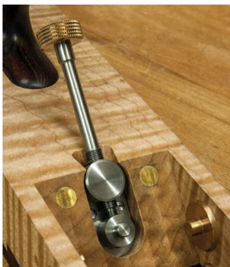
The Norris type adjuster is beautifully made. Brass pads are in fact rods bonded into the base of the body to minimise the effect of wood movement on blade bed angle
