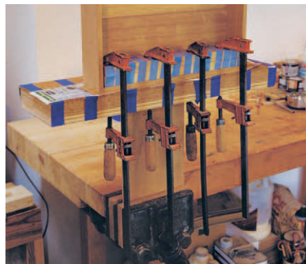
A new face. Thick, shopsawn veneers are glued to the front and back, tidying up and strengthening the joint.
