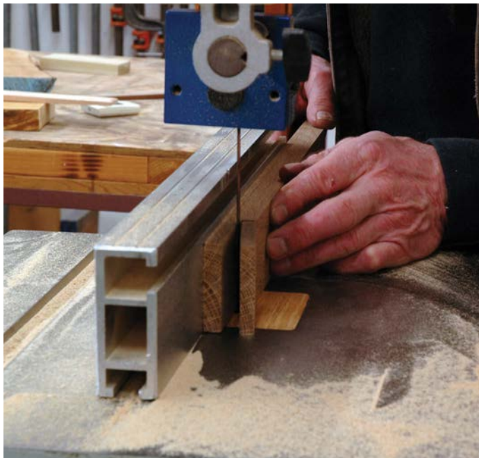
Rough out the cheek on the bandsaw down to the gauge line
