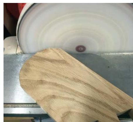
Refining the curve on the disc sander – the guard is removed from the right-hand side to allow the full arc to be faired in, but all the contact is on the left where the disc is descending into the table. The guard goes back on when the operation is completed
