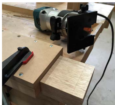
New angled fence jig for the router to run against
