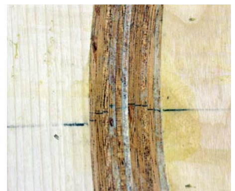
Close-up of the 3mm layers clamped between the formers. The broken pencil line shows a slight but acceptable deviation in alignment of the strips
