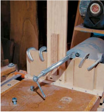
Minimortises. Using a horizontal mortiser and a 1/8-in.-dia. end mill bit, the author cuts through mortises in the drawer sides.
