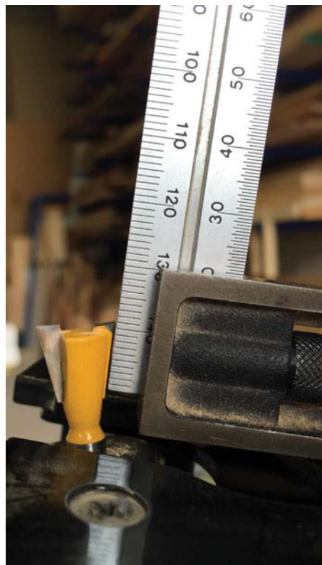
The quick and easy way to set up the tilting base angle is to use a square
