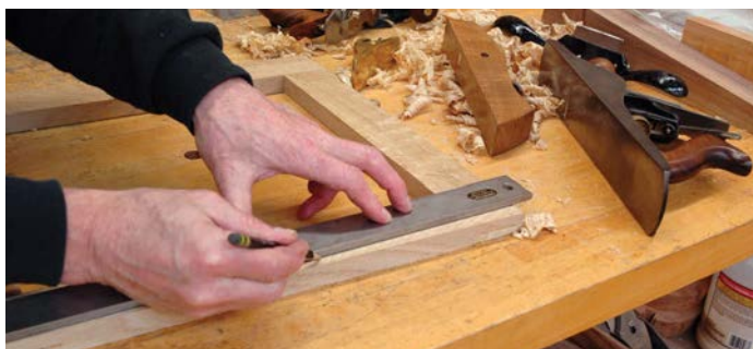
Mark out the frame tapers on the stiles with a straight edge
