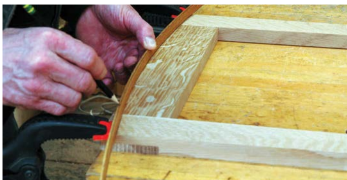
A thin piece of red oak works well as my template to mark out the shape of the rails
