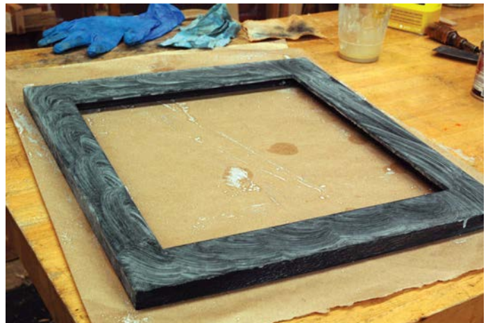
Give the filler paste time to glaze over
