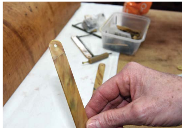
A handle reformed using pieces that have been cut and then glued together
