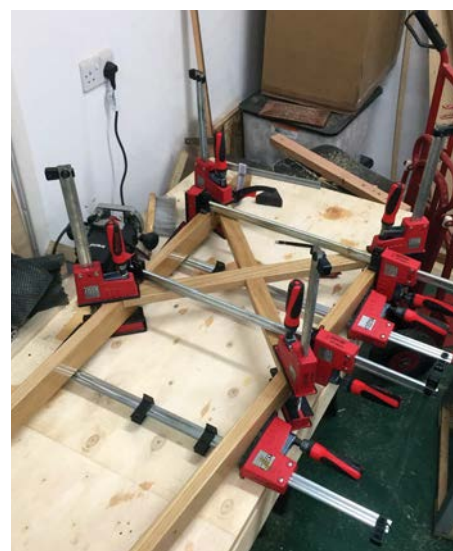
Dovetailed back brace being glued up
