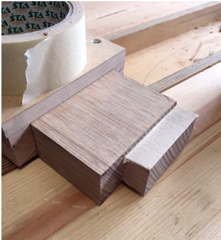
Using layers of masking tape can help with fine adjustment of cutter depth
