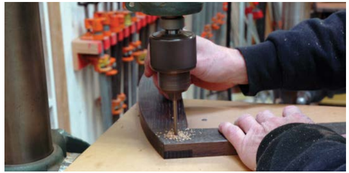
Drill with a 5mm bit for the pin hole
