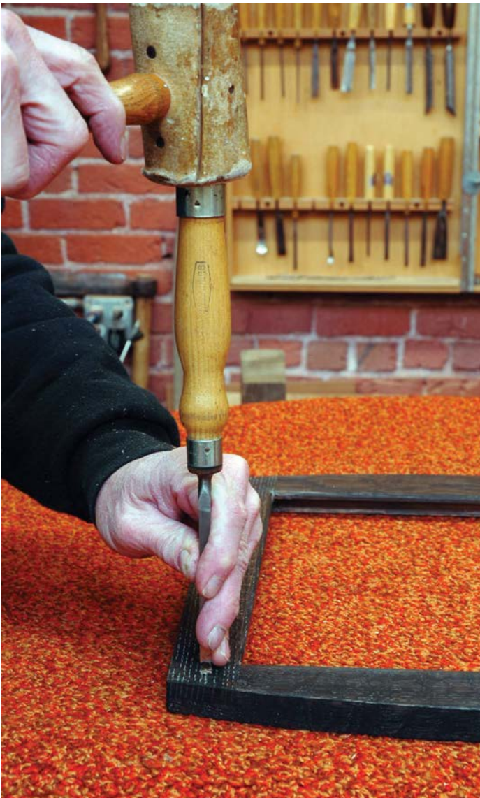
Chop straight down around the hole to create a 6mm square hole
