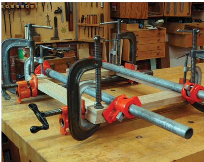
Get your clamps together first and practise the assembly process before any glue goes on
