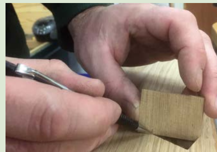
Showing the wedge to the mortise and marking the length
