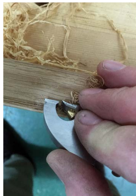
Easing the sharp edge of the quirk on the bead with a miniature shoulder plane
