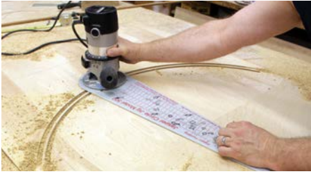
Cutting the radius with a small circle
