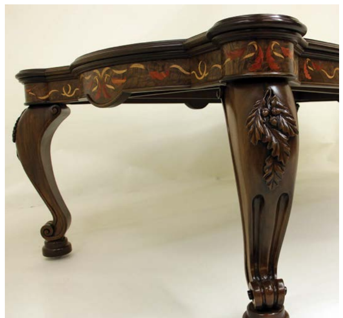
The finished apron
