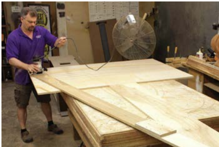
Routing out the large radius clamping jig
