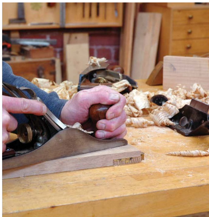
Use a hand plane to clean up the frame surface
