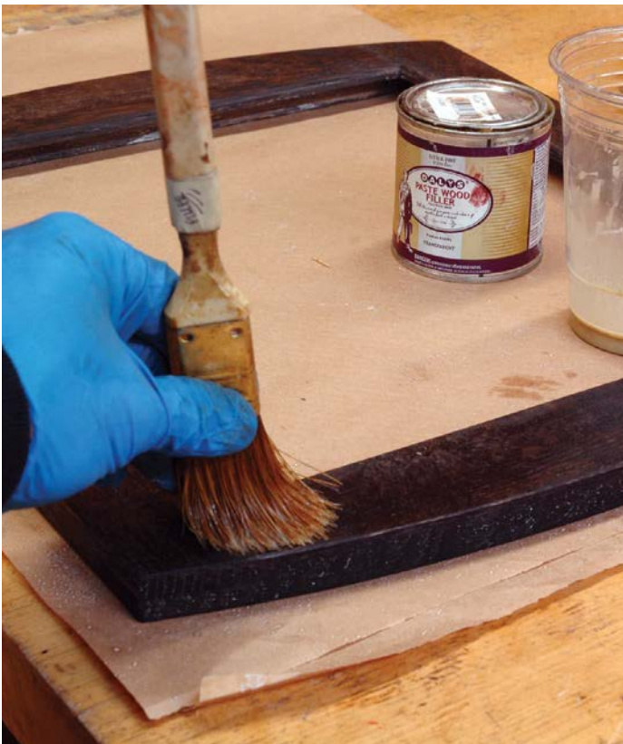
Use an old brush to push the filler down into the pores of the ebonised frame
