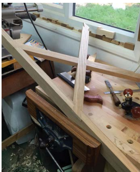
Dry fitting a pair of dovetails together changed the fit of the joint slightly and tightened everything up
