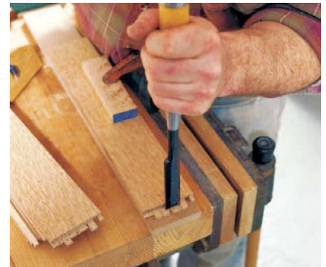
Chisel out the middle. Between the tenons where the handsaw won't reach, the author chops out the waste with a bench chisel. The waste can also be removed with the part held upright on a tablesaw crosscut sled.
