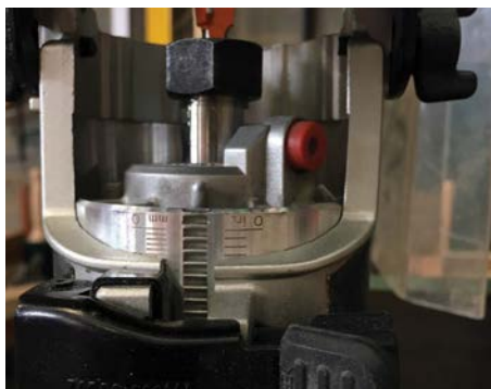
Depth adjustment on the router is simple with some patience
