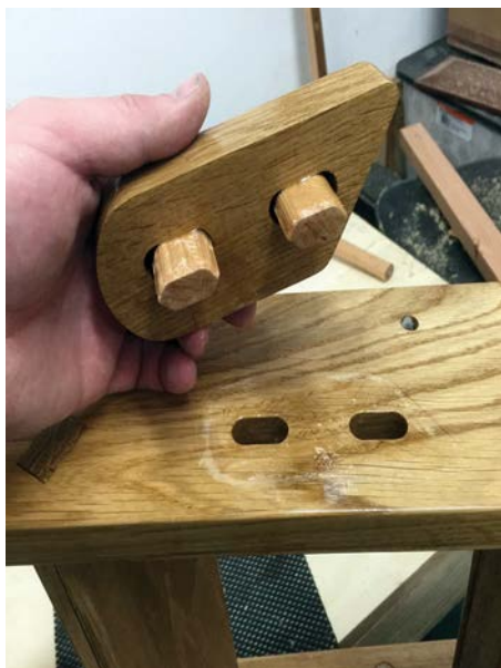
Fitting the stops with Dominoes and hide glue
