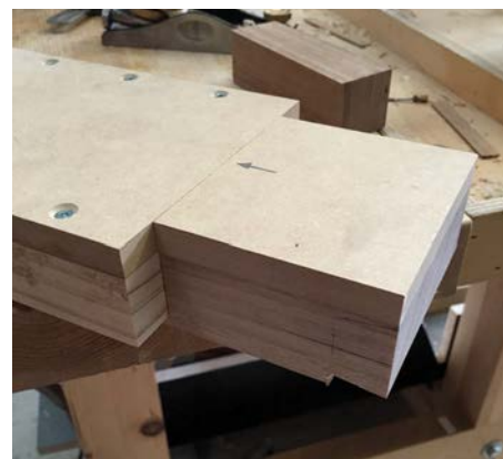
MDF spacer, with 2° angled sides...
