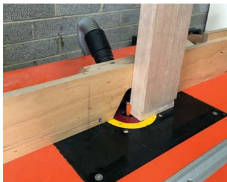
One option was to cut the sliding dovetail vertically on the router table
