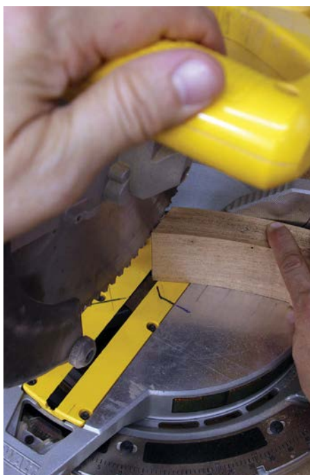
Cut the mitres with a mitre saw
