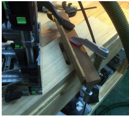
Inserting the shim to space the Domino off an additional 12.5mm and widen the mortise to 25mm – positively locating against stops and this shim is more repeatable, accurate and quicker than measuring
