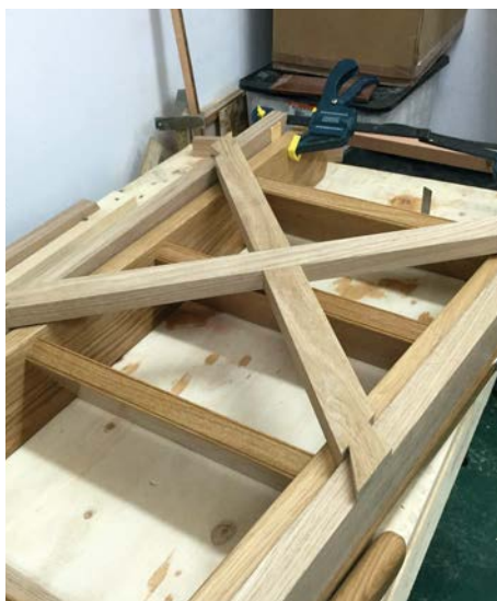
Marking the dovetail sockets with the rear section clamped to the ladder section over 2mm spacers for clearance in the final assembly
