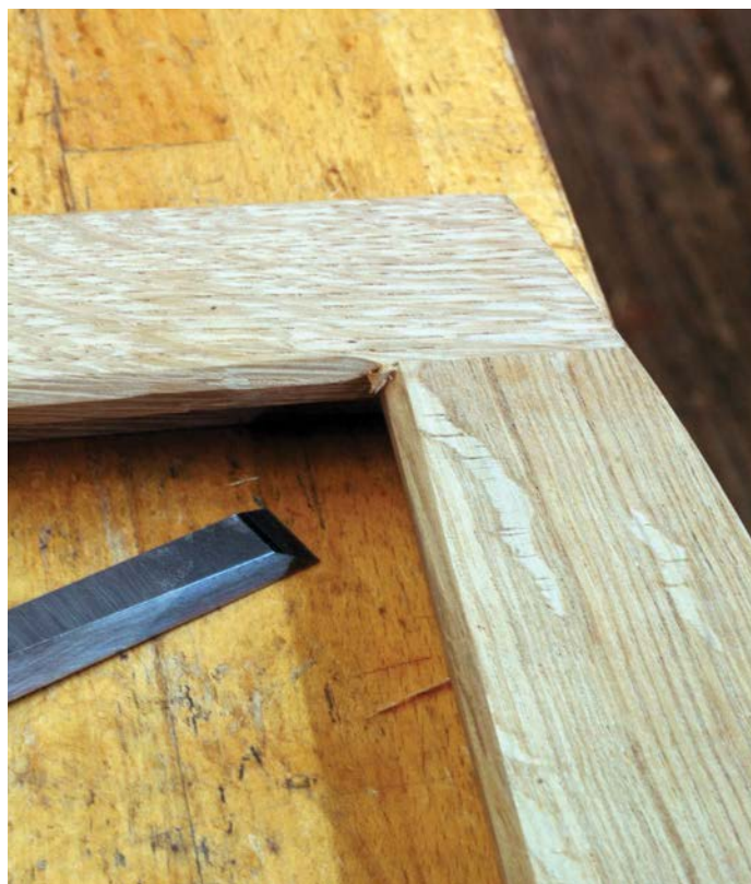
The corner left by the chamfering bit has to be cleaned up by hand with a mason's mitre
