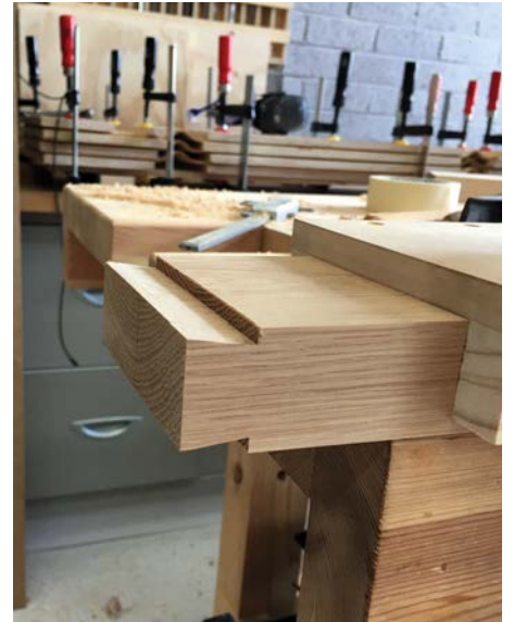
The fence is flipped over and spacer used to align the second cut
