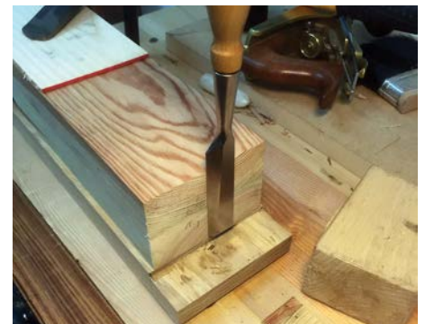
Paring the 3° shoulder line using a guide block secured to the piece and the bench with a holdfast
