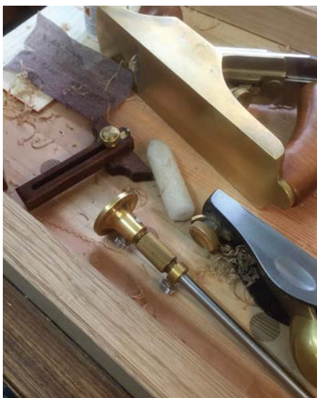
Tear-out reduction strategy for beading – define the extents of the quirk with cutting gauges, round with a block plane with the grain, use lots of wax on the beading plane and blend it all at the end with some Abranet
