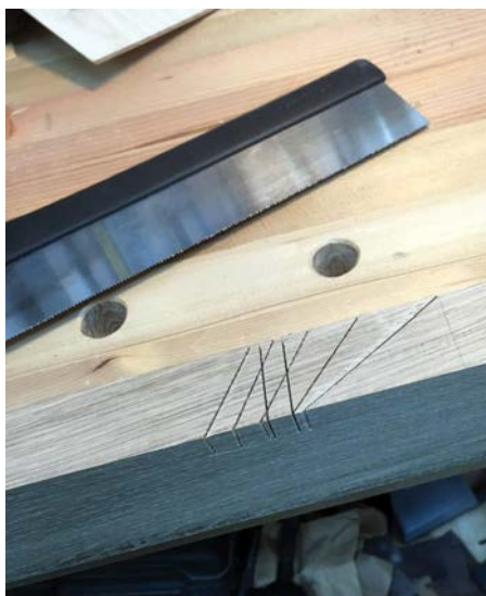
Cutting the sockets and kerfing the waste prior to chopping out
