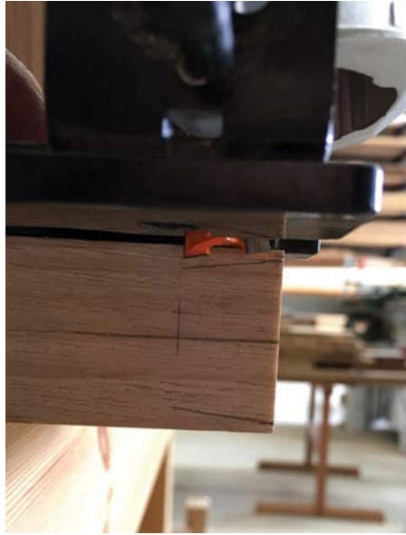
Marking out the joint can help with depth and fence alignment
