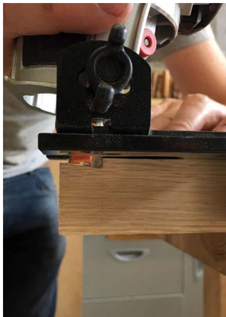
Tilting base angled to that over the dovetail cutter
