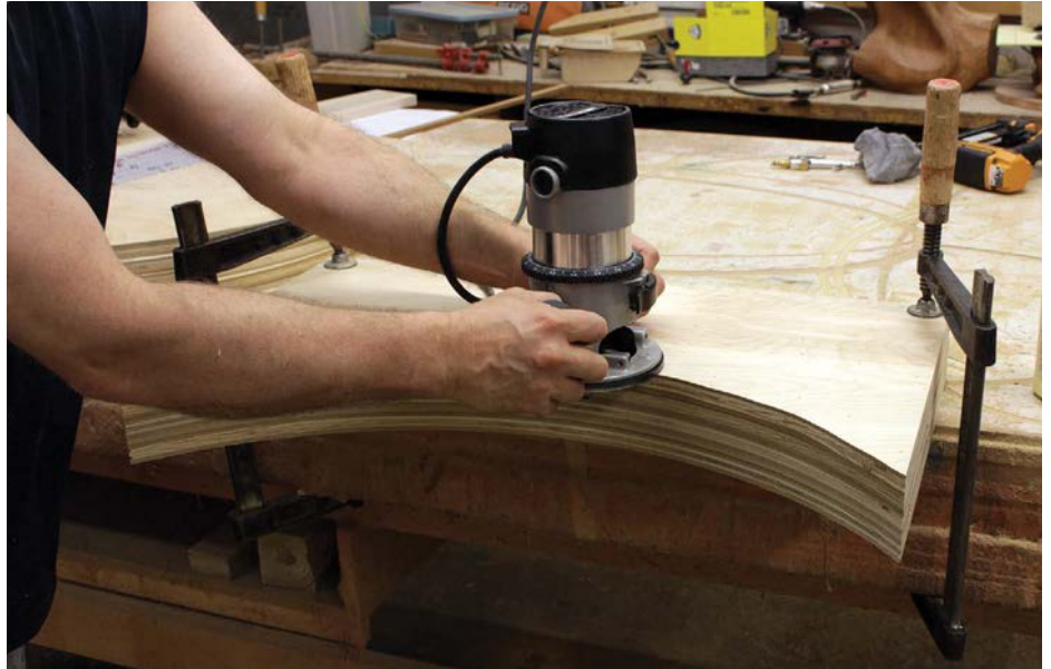
Building up layers of plywood to make the clamping jigs
