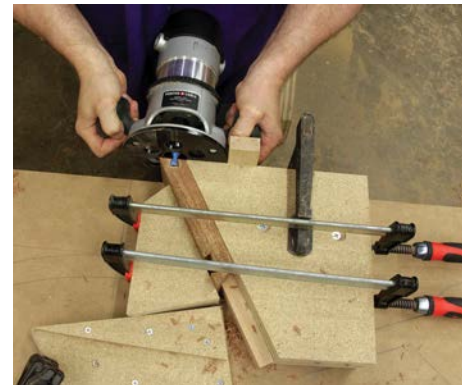
Routing the dovetail dado into the ends of the straight aprons
