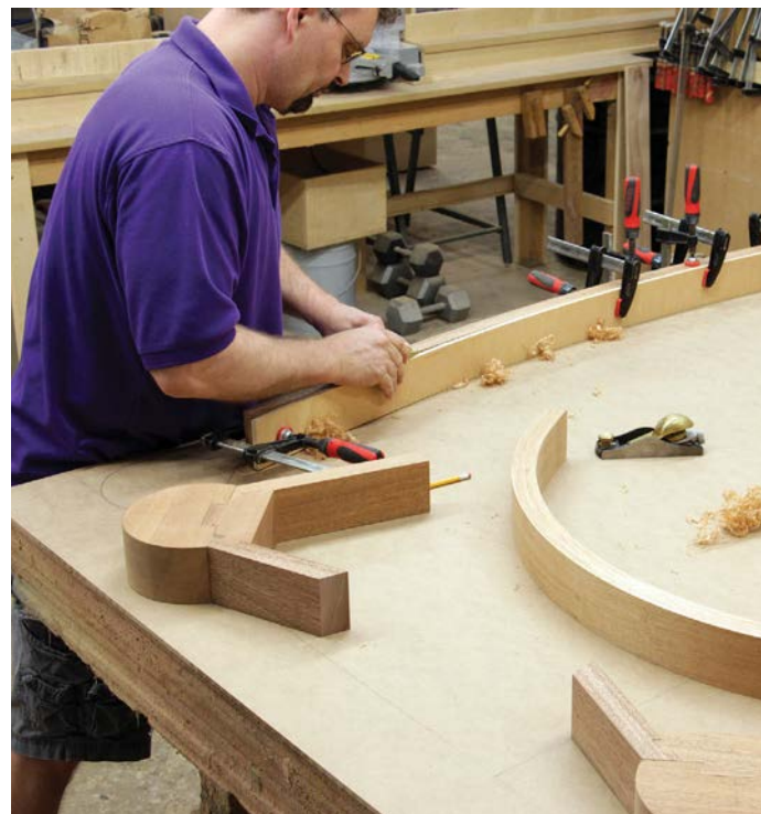
Hand plane the aprons square and flush to the template
