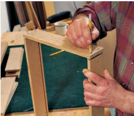
Mark through the mortises. To mark out the tenons, the author pushes the tongues into the grooves. Then he traces the mortises with a sharp pencil.
