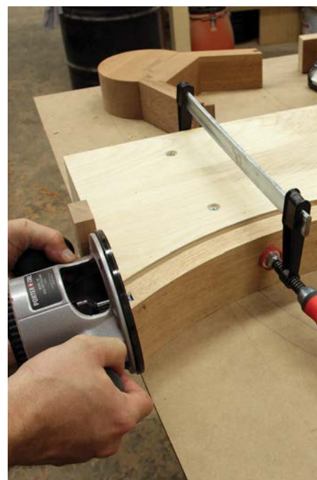
Routing in the dovetail dado into the radius aprons
