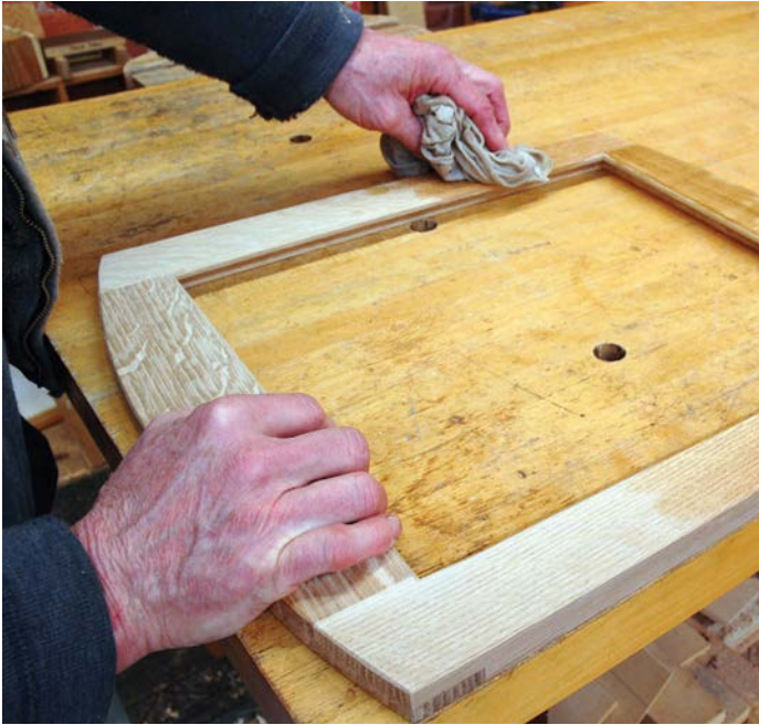
Raise the grain with a damp rag before the finishing work begins
