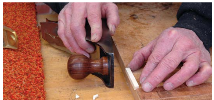
Shoot the edges of the holly on a bench hook using a sharp bench plane
