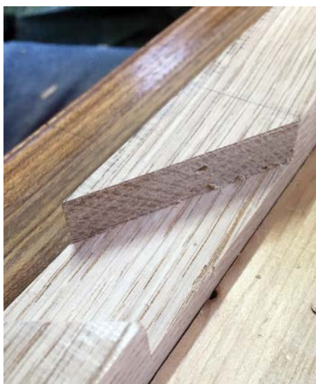
Dovetail socket cleaned out ready for dry fitting
