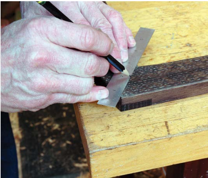
Measure across the diagonal of each joint and find centre on that line. Use a pencil or scratch awl to mark the point to drill
