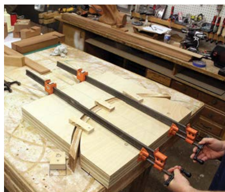
Clamping the layers of the apron together with the clamping jig
