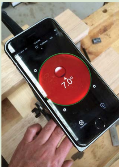
Clinometer app showing the router tilt base angle
