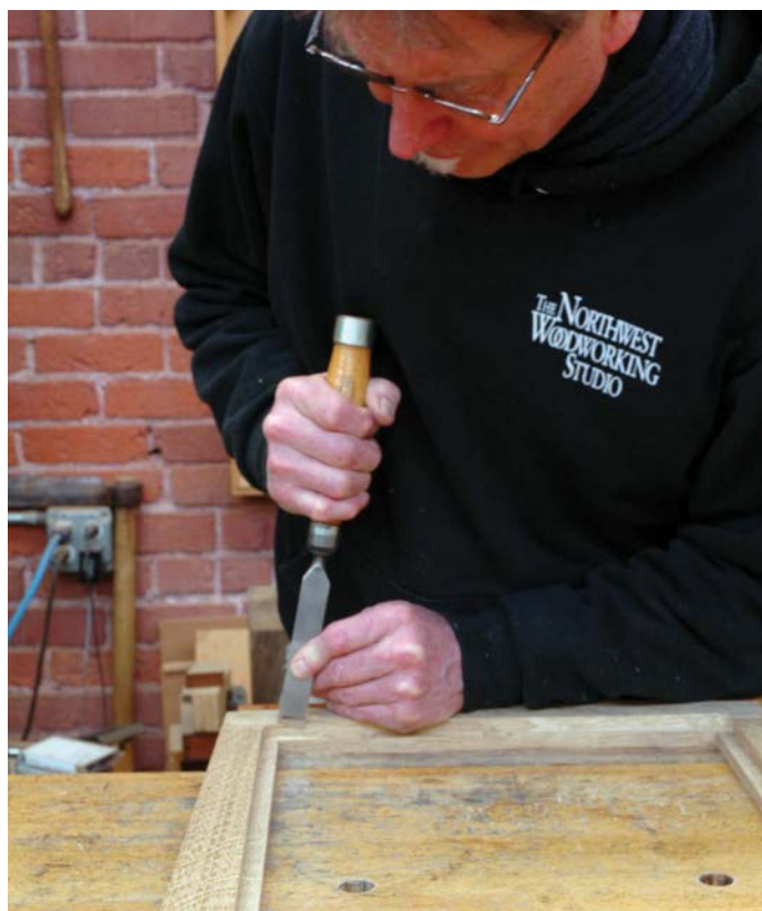
Clean up the corners of the rabbet cuts with a sharp chisel
