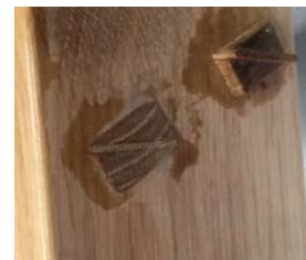
Trimming the tenons flush with a flushcut saw before smooth planing the outsides of the ladder section
