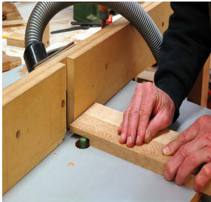
Clean up the cheeks and cut the shoulders of the half-lap
