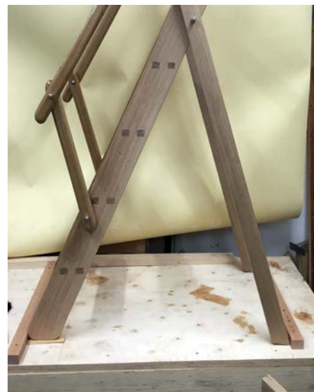
The ladder section shimmed up by 6mm to allow the angle and length of the rear section to be scribed to exact length and angle with a 6mm block
