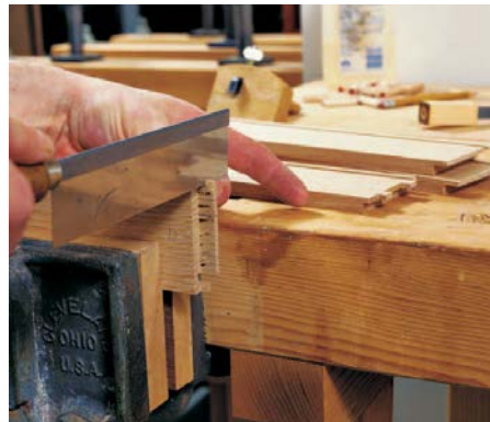
Quick saw. A thin saw makes quick work of cutting the tenons.
