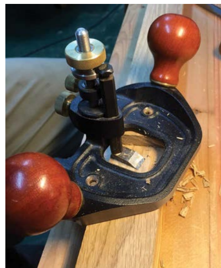
Cleaning the base of the dovetail sockets with a router plane to final depth
