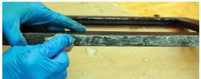
Rub off the excess dried filler with a piece of burlap first. It is soft but easily picks up a load of debris from the surface. Then finish off wiping with a piece of brown paper
