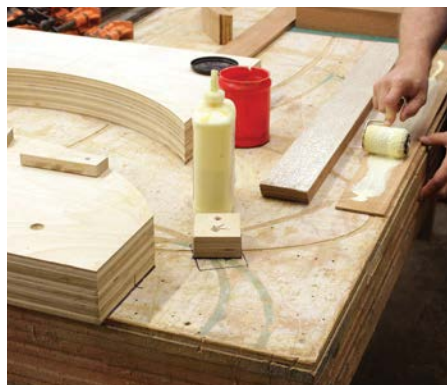
Rolling yellow glue onto the layers of hardwood
