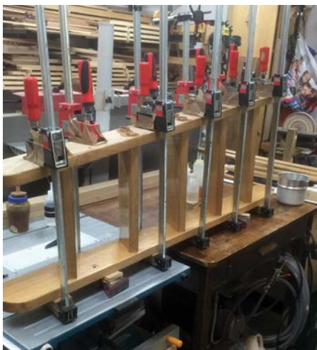
Glue-up with angled clamp head packers to allow clamping without bruising the timber
