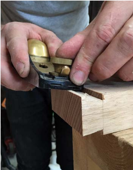
... which was easily cleaned up with a block plane
