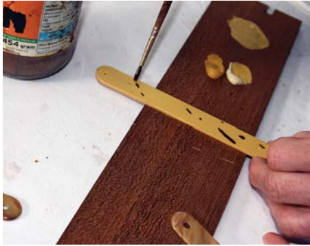
Applying the spots and streaks of each colour to match the original handle
