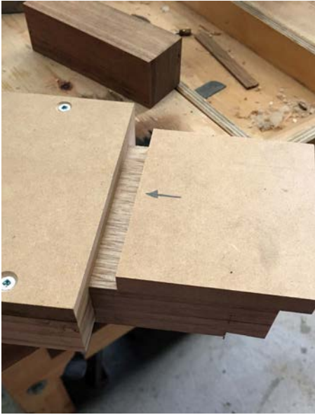
... used to set the fence spacing on the workpiece
