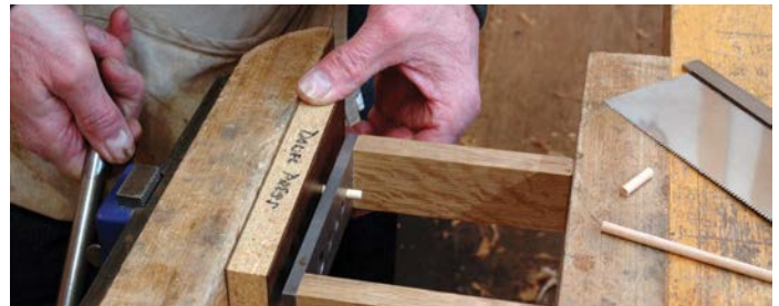
Press the dowel through the dowel plate rather than hammering, unless your therapist recommends the exercise
