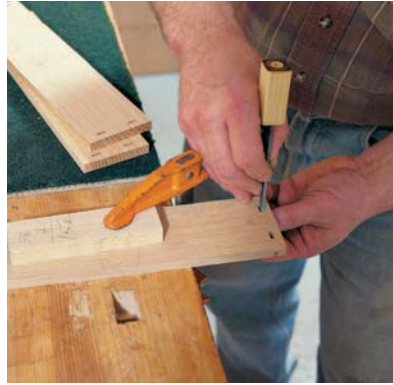
File it away. A file is used to square up the round corners left by the mortiser. This takes time, so be sure to use a sharp file small enough to maneuver easily.
