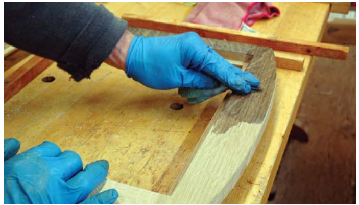
Wet down the frame with the ebonising solution
