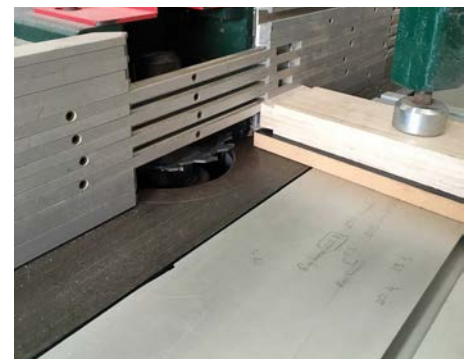
Another was to cut the dovetail using the sliding table spindle moulder
