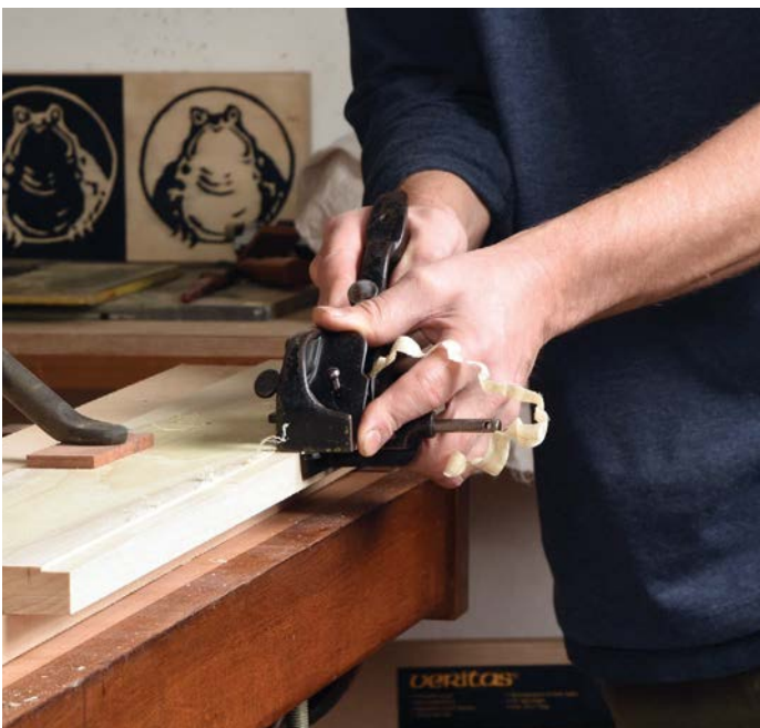
Set up and go with a dedicated rebate plane
