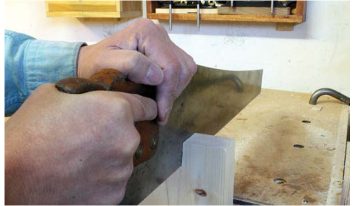
I drew two parallel lines instead of one line for each of the V-lines to guide the sawing
