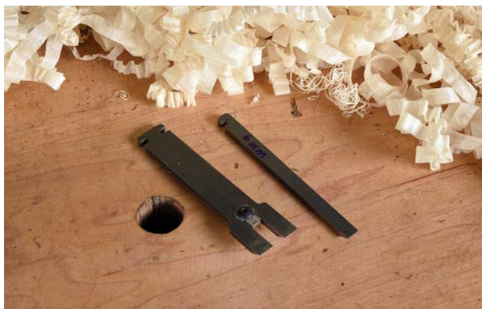
Matched sets of irons can create tongues for your grooves
