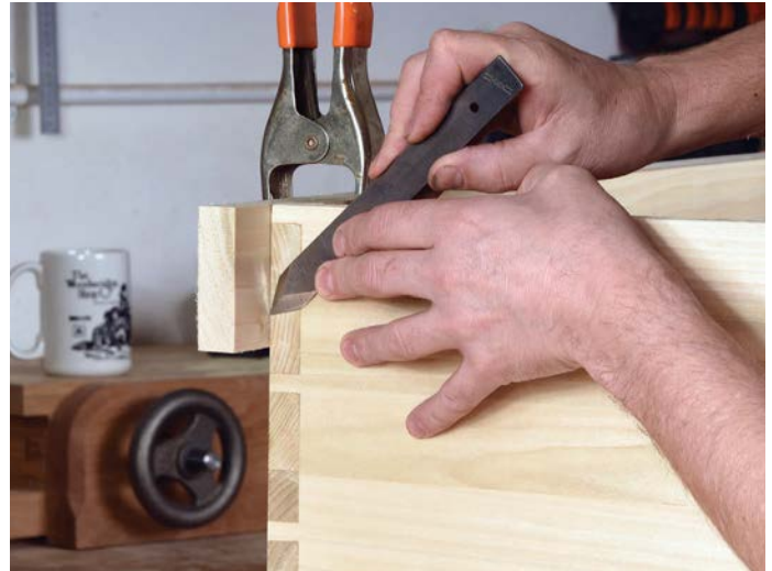
Use the workpiece as the template
