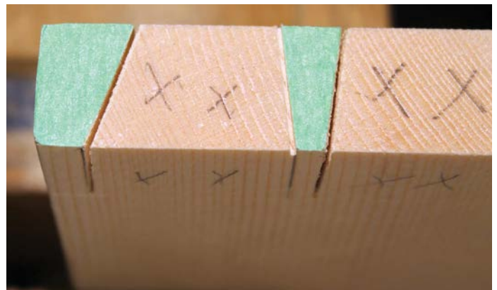
'Splitting the line' can be quite hard. Cutting against the tape edge is much easier
