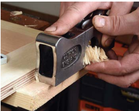
A shoulder plane cuts rebates as well...
