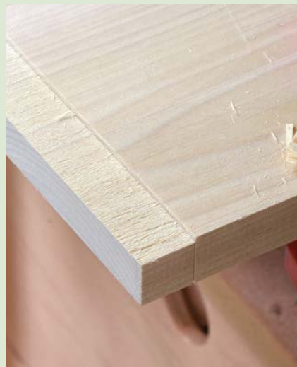
Rebate the inside of the tailboards to a depth of a couple of millimetres
