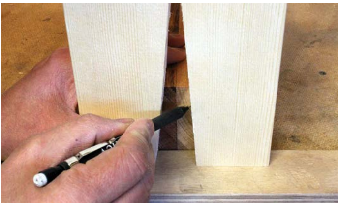
Centre the battens with the V-notch and trace the bevel lines on the ends for a perfect match
