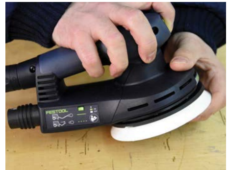
A green warning LED and audible signal indicate the machine is set to disable mode and cannot be used unless attached to an extractor
