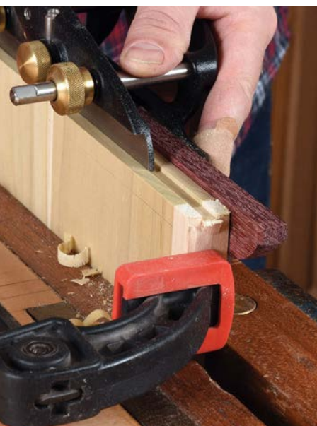
Set the panel grooves in line with the mortises
