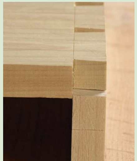
2mm is enough of a ledge to register the tailboard in place and help transfer knife marks for pins
