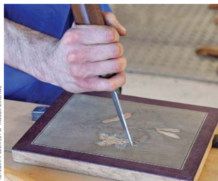
This method of marquetry is done using a long-handled shoulder knife
