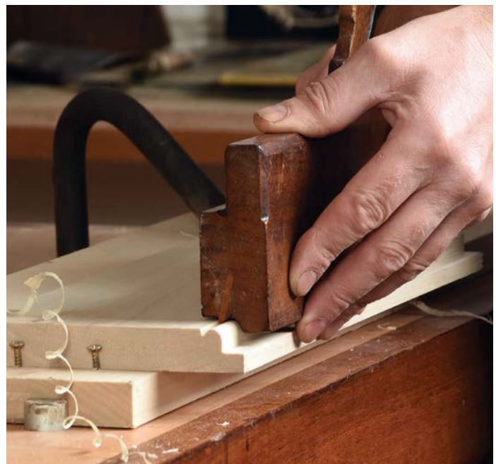
Shape up with a moulding plane
