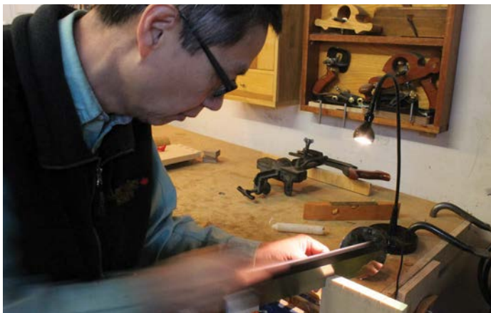
The mirror helped me know when to slow down to avoid overcutting
