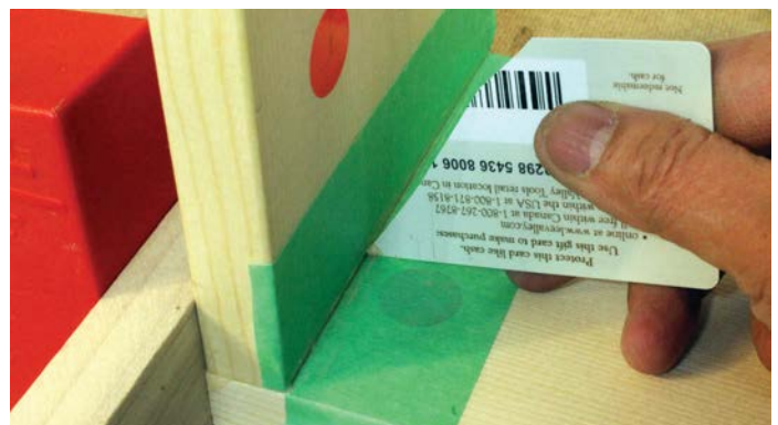
Tape and a sharp angle point cut on this expired gift card were my secret weapons to handling the glue squeeze out
