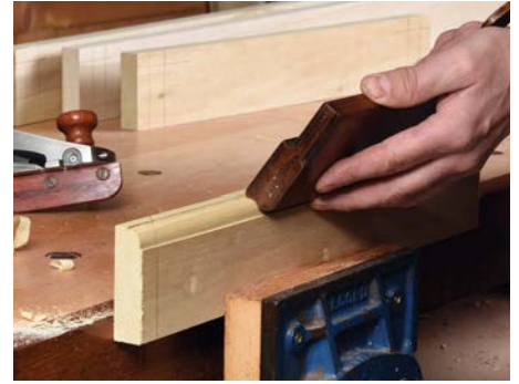
One setting on the skew block plane equals two matching rebates and a custom ovolo
