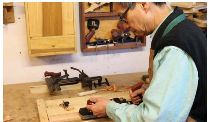
I planed with heavy cuts to remove bulk waste at the start and then switched to fine cuts near the end
