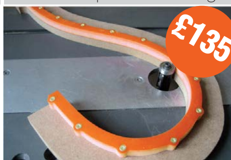
Flexible Template for Routing
