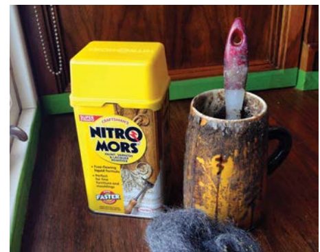
A typical clean-up operation with paint stripper and steel wool
