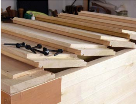
You can hide a lot in a rebate, including nail heads
