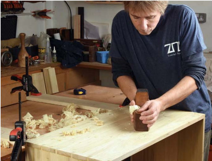
Outside faces are sometimes reference faces as well so be careful with that smoother
