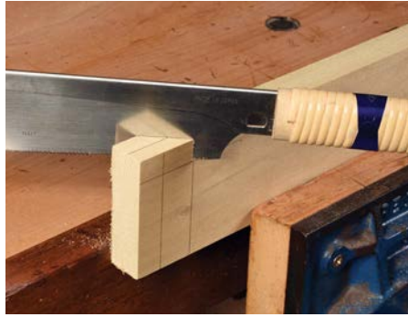
Shiny surfaces are also very functional. If it looks square in the 'mirror' it is square
