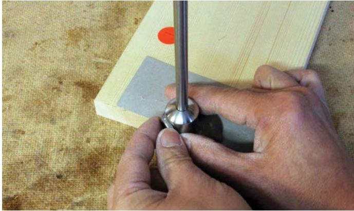
I used a paper shim to set the marking gauge just shy of the board's thickness. The orange dot shows the inside face
