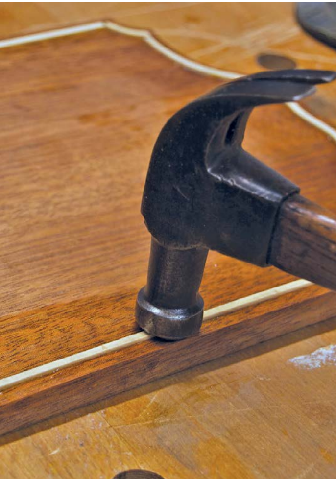
Gentle taps with a small hammer will seat the purfling within the channel
