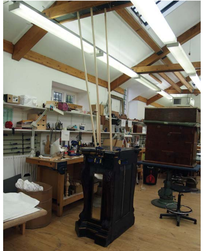
The battens were stretched between the ceiling and the surface to push down lifting veneers
