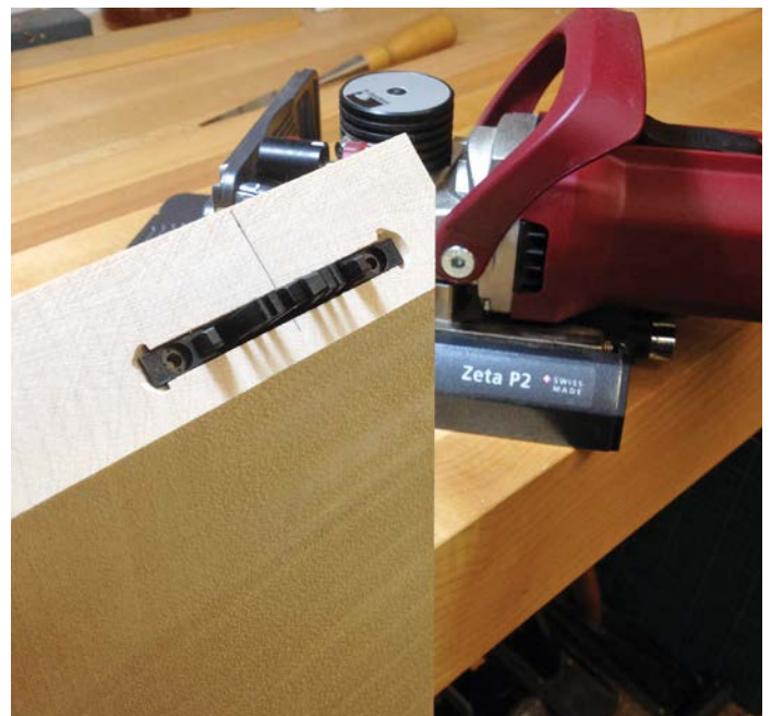
Lamello have some cunning solutions that can do away with cramps altogether
