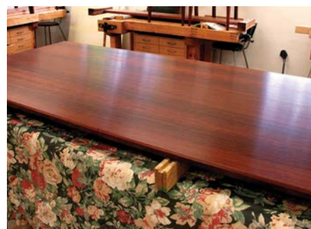
Burnishing is hard work but produces excellent results
