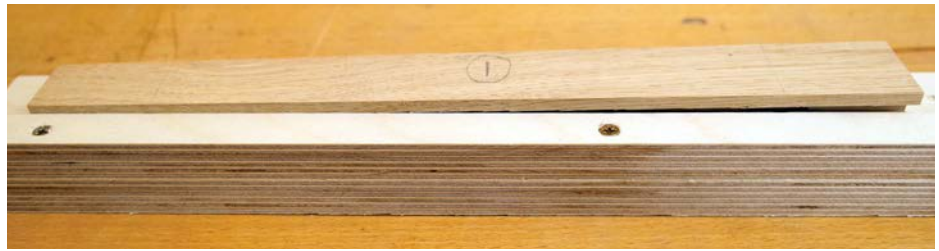
The stave is then shaped in its thickness using a second sled jig
