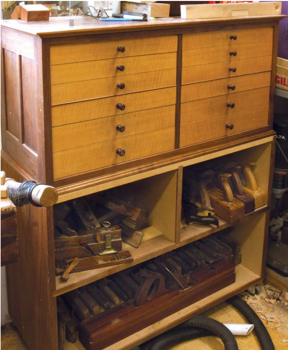
Like many woodworkers, Phil couldn't resist the temptation to make this piece of workshop furniture look nice. Despite appearances, this tool cabinet is at least 90% MDF
