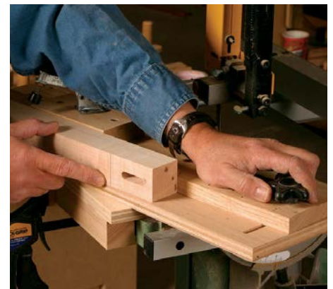
Locate the taper's start. Align the beginning of the taper with the edge of the jig and tighten the infeed knob.
