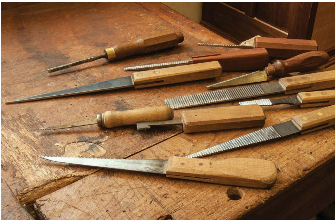
Phil's collection of floats, used for forming mouths and throats, plus a homemade specialised scraper
