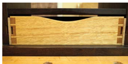
The drawer is fitted to the opening with packer pieces to allow for the runners
