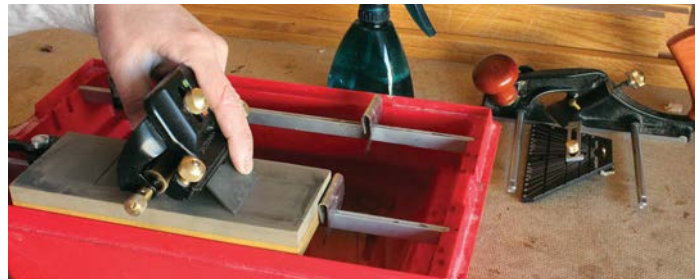
The registration accessory sets the blade at the precise bevel and skew angles in the honing jig
