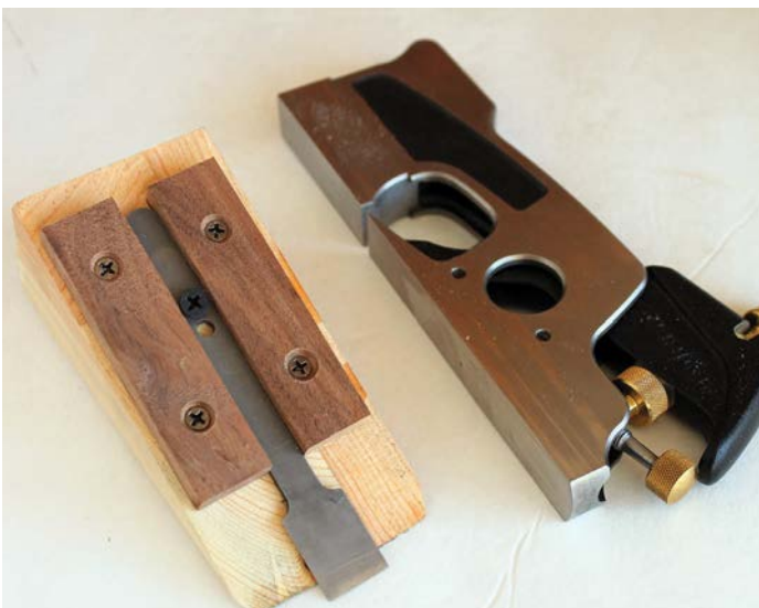
The strips and screw keep the blade in the proper honing position
