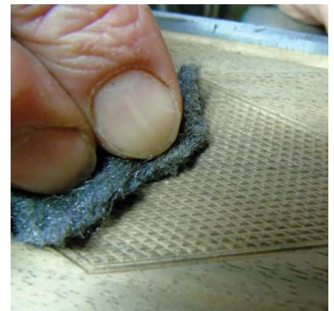
Using wire wool to deburr and polish
