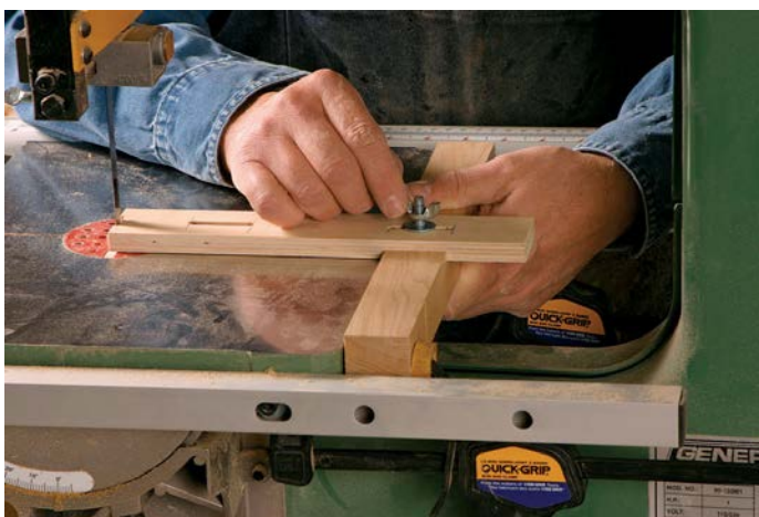
The notched finger jig surrounds the blade. For simple curves, the finger rests on the tables and a short bolt holds it in the dado of the clamping block.
