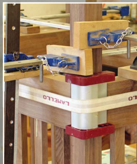
Gluing up in manageable chunks could result in a simpler cramping solution
