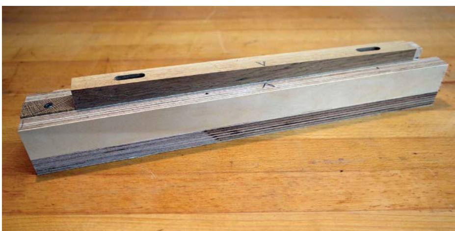
The jig holds the stave at the appropriate angle for the taper
