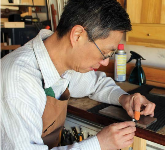
In a sitting position and with my elbow resting on the bench, I move my arms back and forth to hone the bevel face
