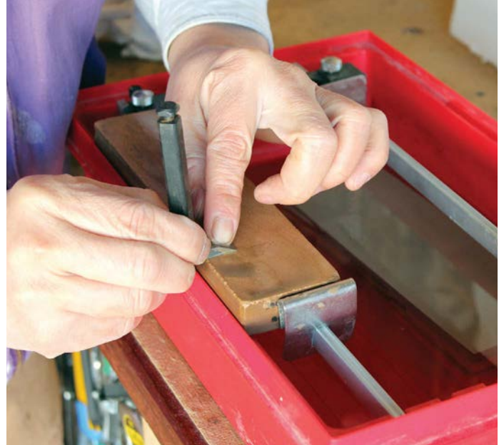
Polish the flat side to remove the wire edge
