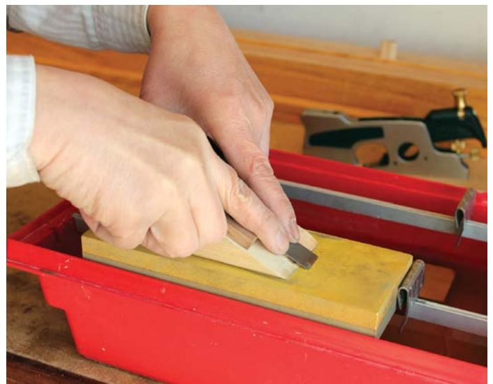
Hold the jig in both hands and keep your index fingers near the front as you push with even pressure
