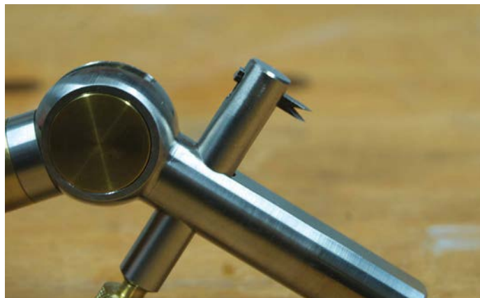
Using the two blades together cuts a channel 2.5mm wide, which can be expanded up to 4.8mm wide using shims
