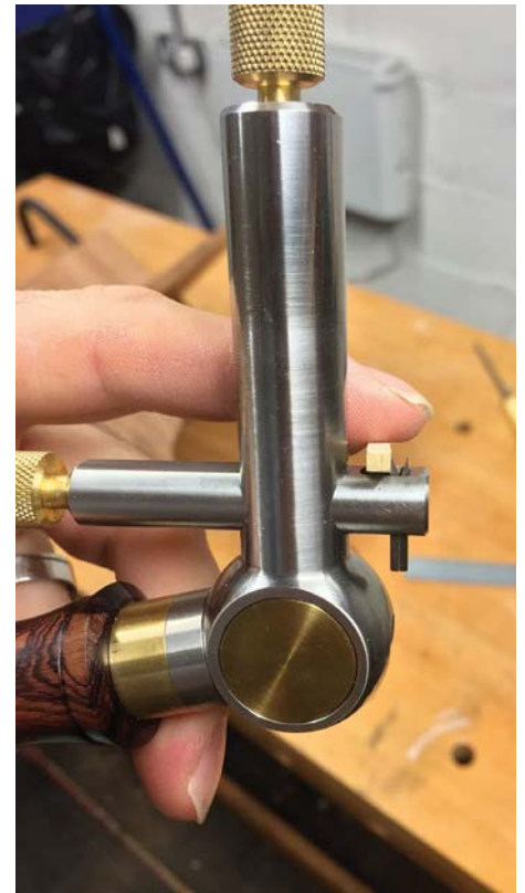
Set the depth of cut by referencing the blades against the purfling material
