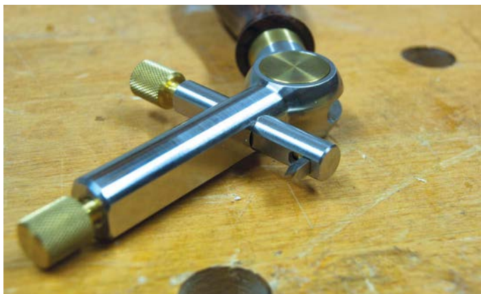
Here you can clearly see the flat face of the fence, as well as two blades
