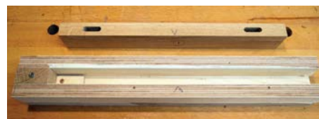
The stave is shaped in its width using a sled jig
