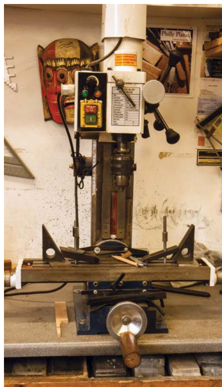
The small milling machine used for forming recesses in Philly planes. Being lightweight it is more suited to working in wood than metal
