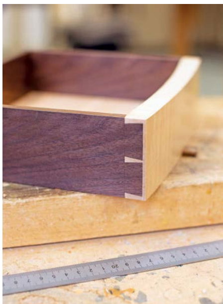
The lack of 'tells' on the joint is a mark of Simon's skill
