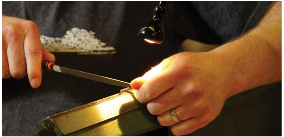
Check your stance is correct before you begin sharpening
