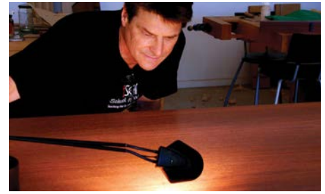
Working with a raking light helps to expose scratches
