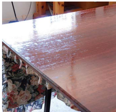
Dry spots will appear where the oil has been absorbed into the wood
