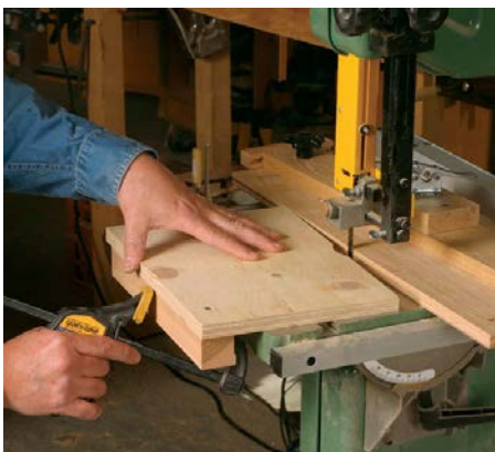
Jig setup. Adjust the rip fence so that the jig is almost touching the blade. Then clamp down the plywood guide, which should just allow the jig to slide.
