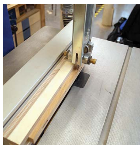
First the taper is roughly cut on the bandsaw
