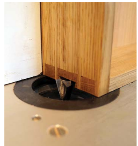
The housing is routed into the drawer side
