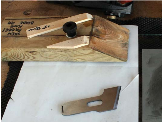
With the blade mounted on the jig and the jig clamped in a vice, stroke a diamond stone on the bevel face
