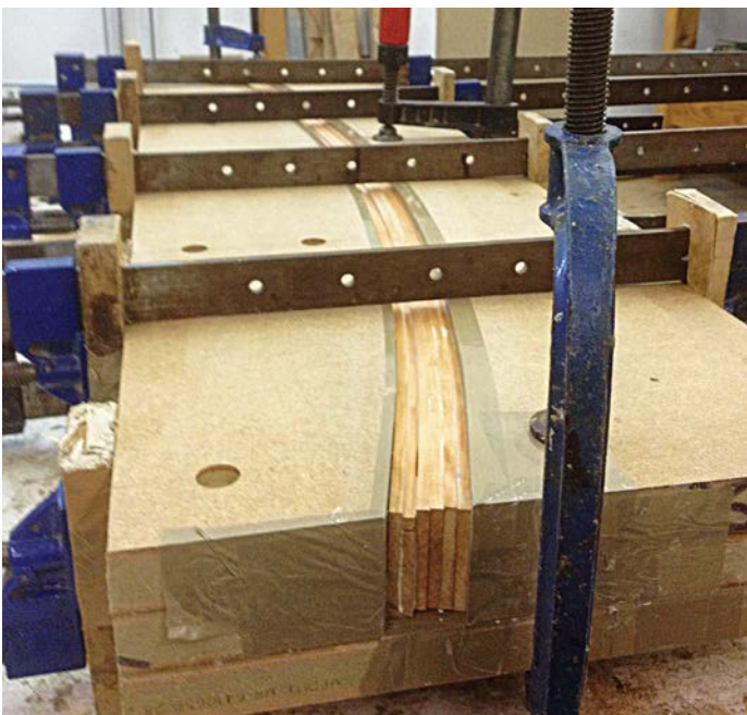
A well-thought-out former design will make for stress-free laminating
