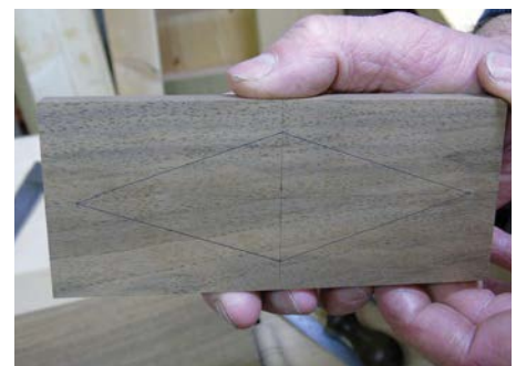
Fully marked out diamond ready for cutting
