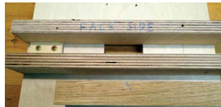
The underside of the jig contains a number of stops to accurately locate the stave
