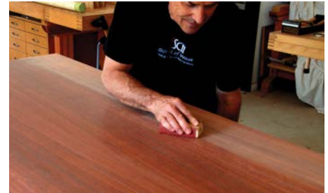
Hand sand to finish, working with the grain using long, even strokes
