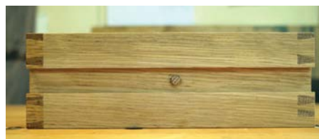
Dovetail layout to accommodate runner housing in drawer side
