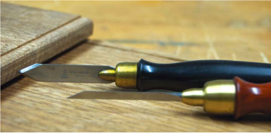
A fine bladed marking knife and a mini chisel are useful for cleaning up the transitions between sections of the purfling channel
