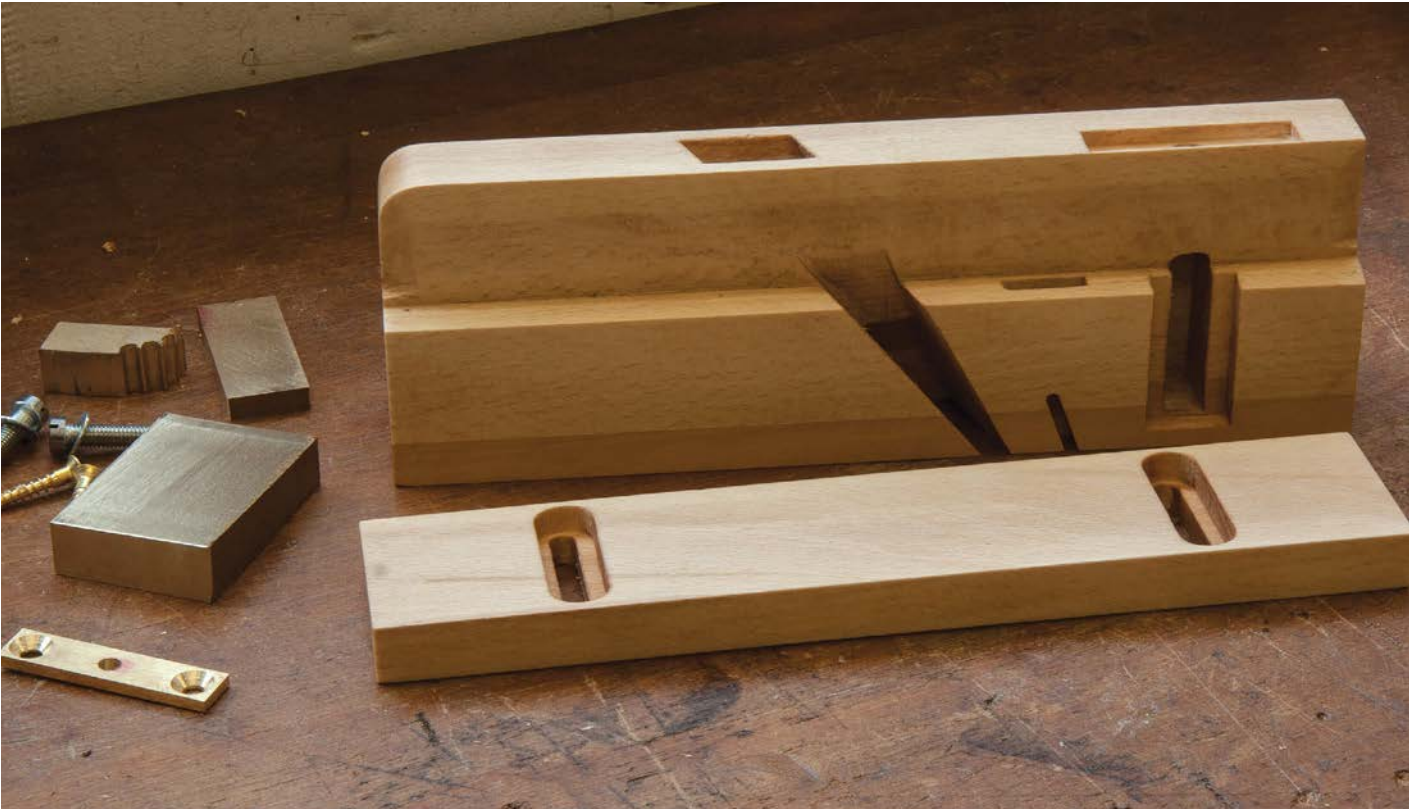
The completed wood parts for a moving fillister. The large brass block will be milled to form the adjustable depth stop
