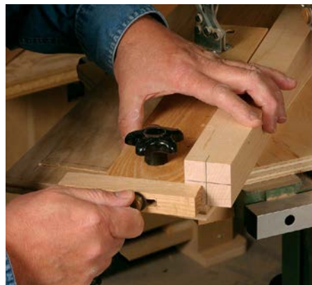
Locate the taper's end. Marks on the stock align with the edge of the jig, which is the cut line. After fixing the outfeed knob, adjust the stop to clear the base.
