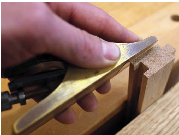
Prior to glue-up the stave ends are finished
