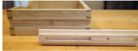
The stops prevent the drawer overextending ...
