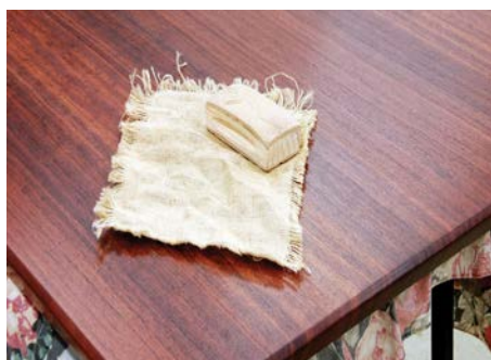
The hessian wad can be wrapped around a sanding block
