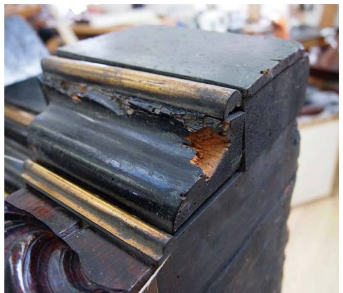
Substrate losses caused by furniture beetle
