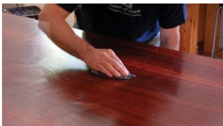
Rub across the grain first, then rub along the grain in a figure of eight
