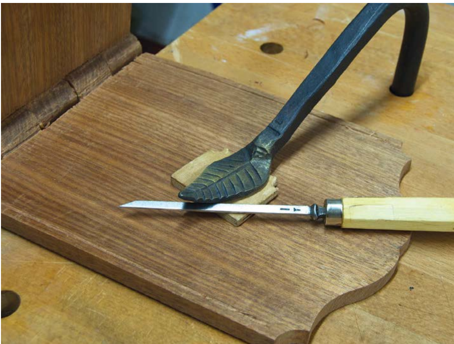
A holdfast is perfect for securing the work, while a fine chisel removes the waste
