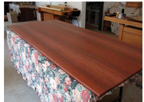
The first coat of oil can be applied after planing, sanding and dust removal
