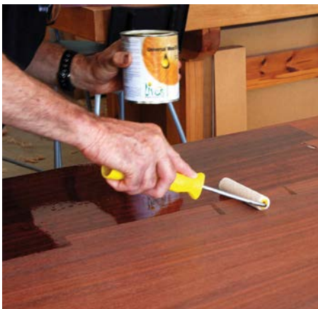
Use a paint roller to apply the first coat quickly and heavily
