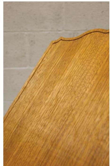
The purfling channels have been cut and cleaned out
