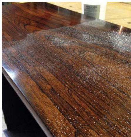
Lightly dust French chalk onto new shellac with a thin film of oil to prevent it from sticking
