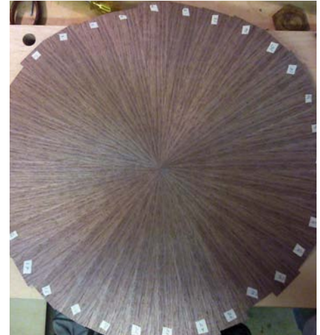
This sunburst has been laid up with all the leaves in position. The numbers can be clearly seen marked onto each piece of veneer
