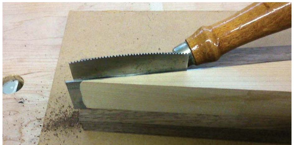
The tip of the triangular template with a 1mm thick metal ruler held between the template and veneer saw. The ruler increases the triangle size by 1mm each side, meaning the whole bundle can be cut consistently oversize in one go
