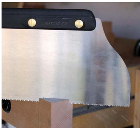
I saw out the waste, close to the ogee profile line before shaping the ogee with assorted rasps
