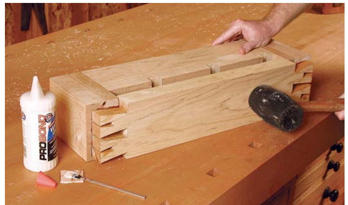
Add the front piece. Apply glue to the tails on the front piece and the pins on the end jaws, then use a mallet to tap the front into place
