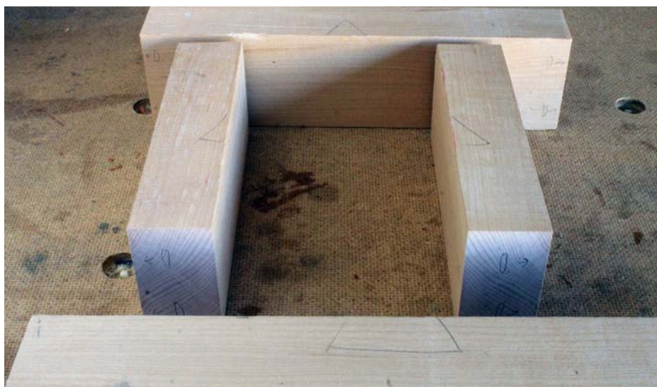
To avoid cutting errors, I marked out the parts and mortises before mortising the stock with a Domino joiner
