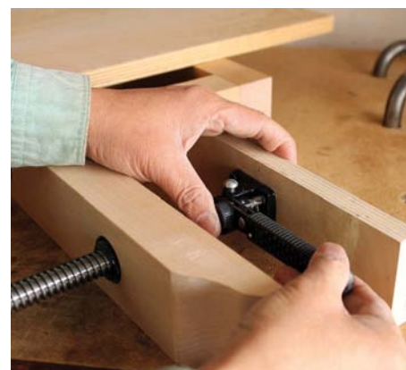
I predrilled before attaching the vice jaw to the swivel head
