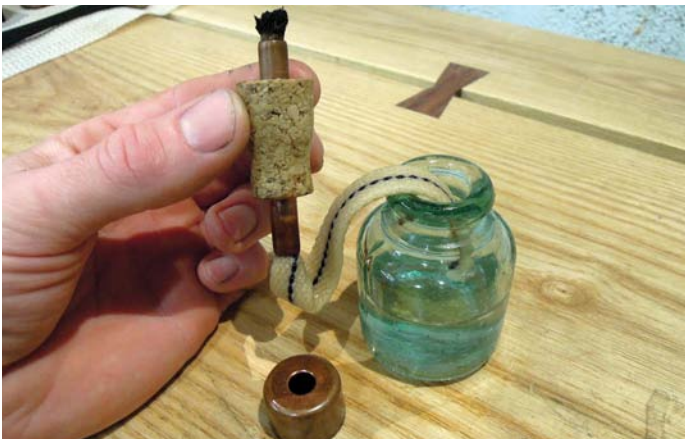
The smoke lamp consists of an oil reservoir, wick and burner
