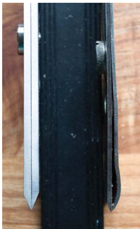
Modern vs vintage blade and chipbreaker thickness
