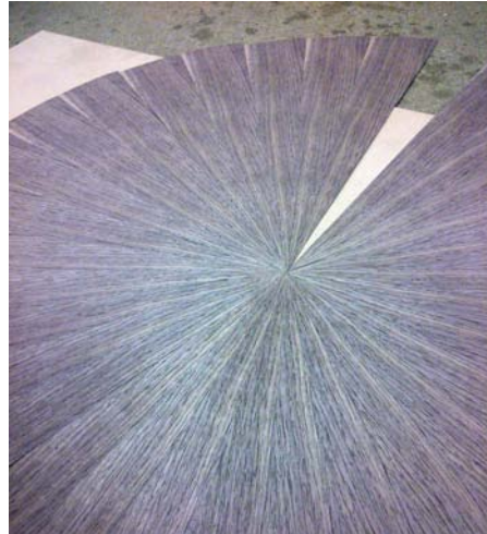
This sunburst has been laid up and held together with sticky tape, it has then been turned over to check each joint is perfect. One leaf has been left out to allow for expansion during gluing
