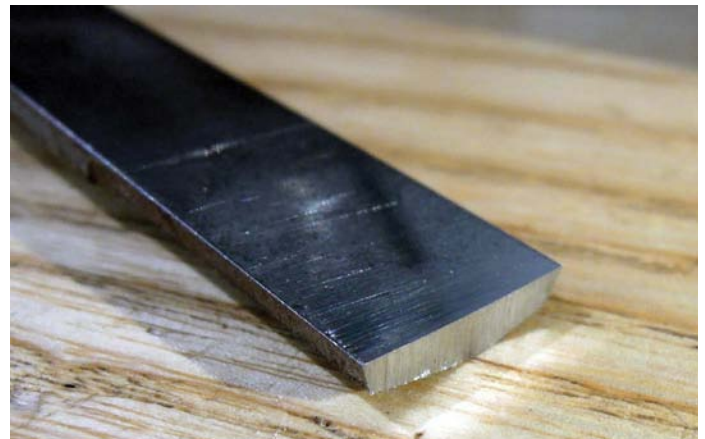
Grinding the cutting face of a bench chisel at 90° turns it into a flat scraper
