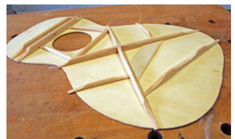
The soundboard bracing on this parlour guitar will in large part determine the sound of the guitar
