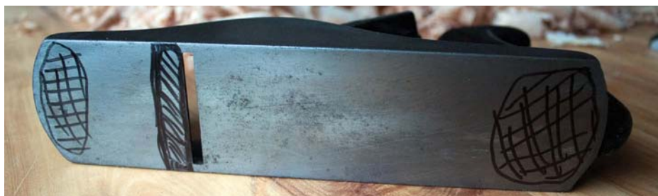
Essential flat spots on the sole of the plane
