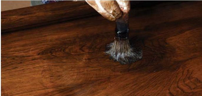
A dirty wash or stipple builds up patina on new parts
