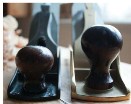
Much thicker castings are used on modern planes
