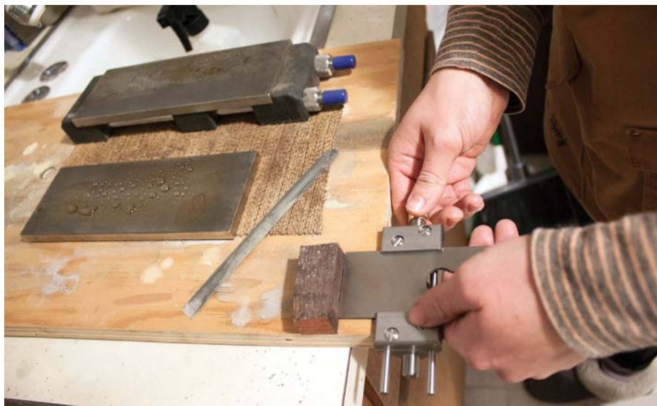
Stop blocks save time and increase repeatability
