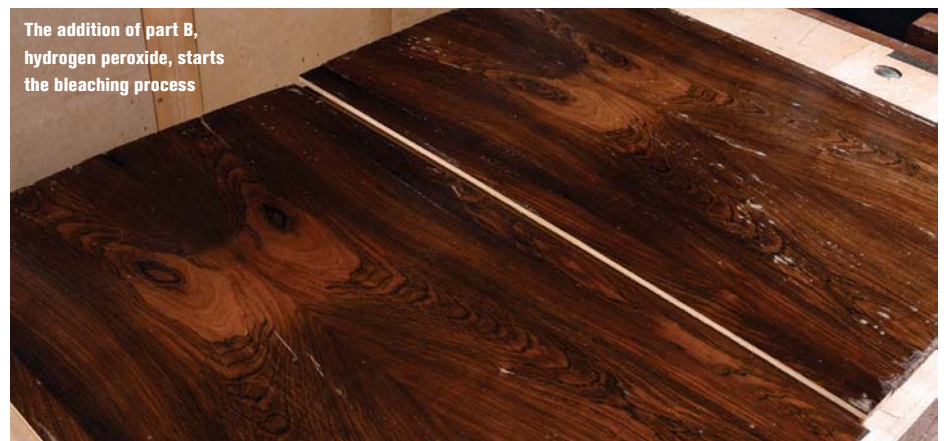
Part A, caustic soda, turns the timber almost black
