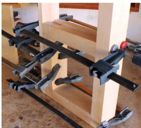
I completed the frame first and then glued the fixed jaw to the assembly
