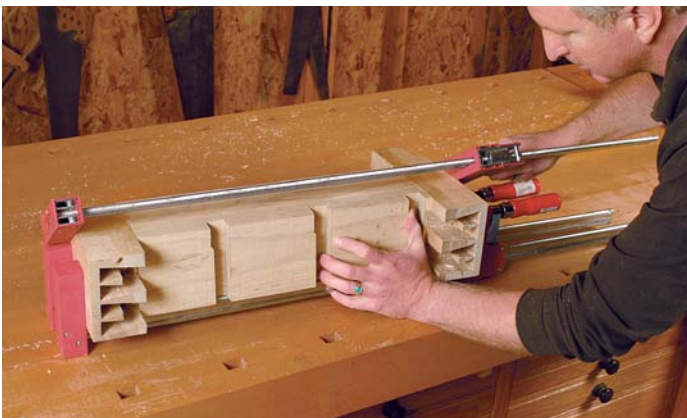
Begin gluing the vise parts. Glue the end, the jaw, the dog-hole block and the top. You'll need several clamps to squeeze the four parts together
