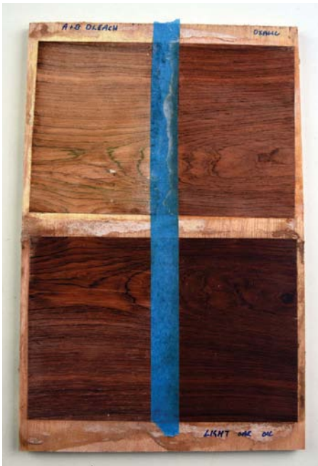
Oxalic acid has little effect on dark timber but will often remove ink and iron stains
