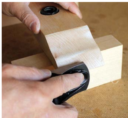
I varied the planing angles, locked my arm and fine-tuned the convex part of the profile with an apron plane
