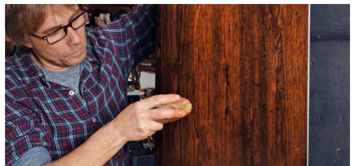
Seal the camouflage in place with some clear shellac to a much wider area
