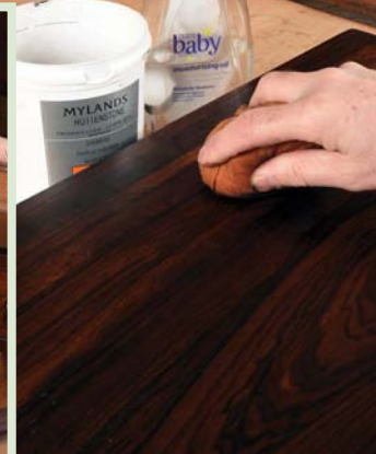
Cut back with baby oil and Rottenstone
