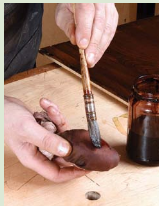
Red tinted shellac, use sparingly
