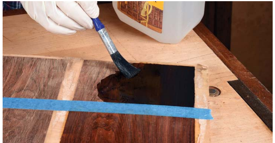
Part A, caustic soda, turns the timber almost black
