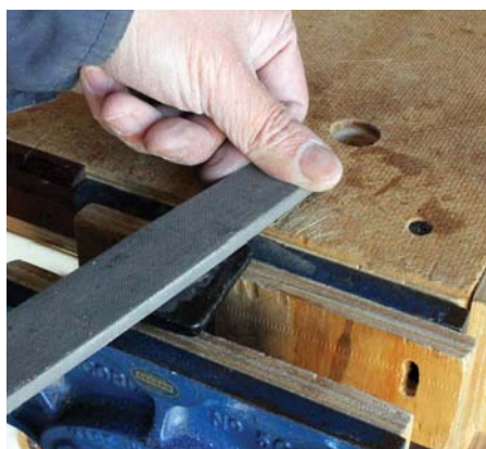
Drill the corner holes on the base and file the whole bottom flat
