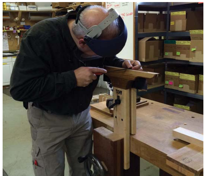
Your body position in relation to the saw plate is important
