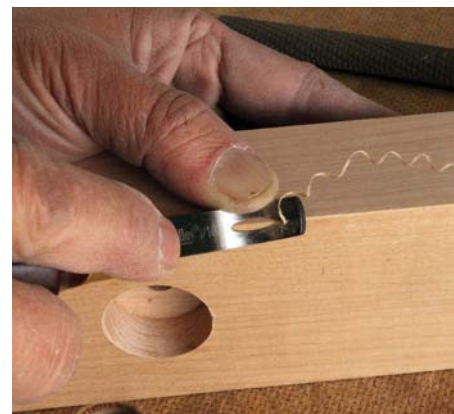
Depending on the grain direction, use push or pull strokes to relieve edges with a cornering tool
