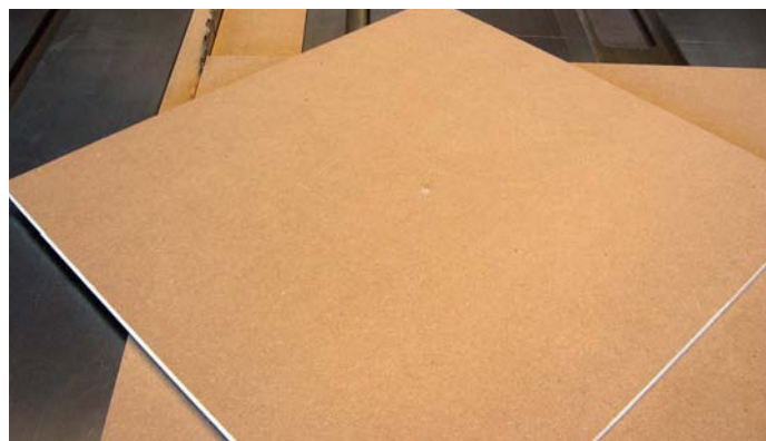
Attach a runner to the underside of a slightly oversize board and trim the jig flush with the blade
