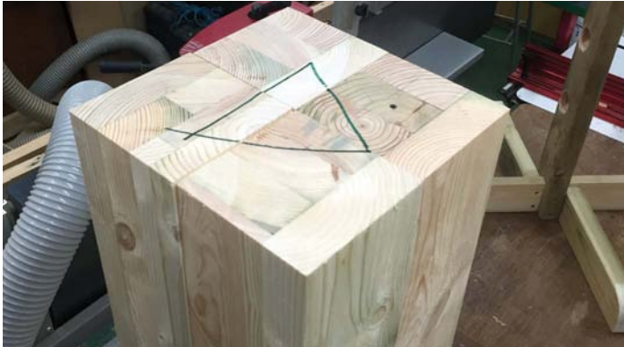
All four legs together marked with the marriage mark
