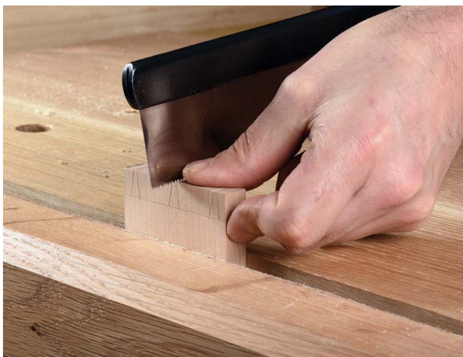
The .015 gauge 300mm-long Bad Axe Stiletto dovetail saw has relaxed tooth geometry at the toe to assist with the start of the cut
