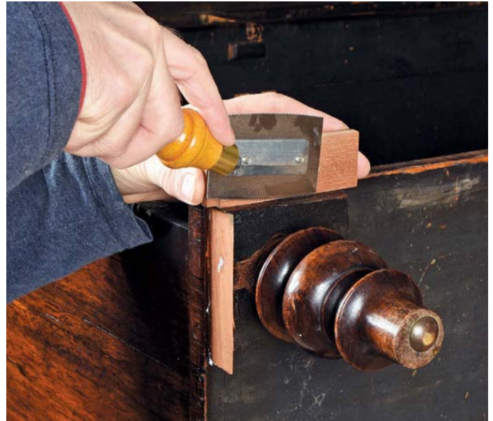
A veneer saw is better than a knife for cutting thick veneer patch repairs
