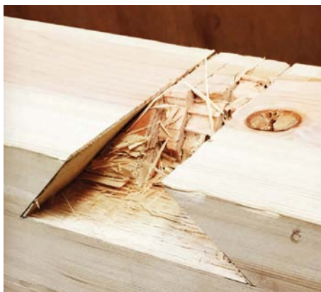
Breaking out the waste from the sliding dovetail socket with a chisel
