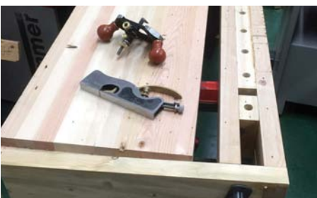
Fettling the fit of the breadboard endcap and tongue
