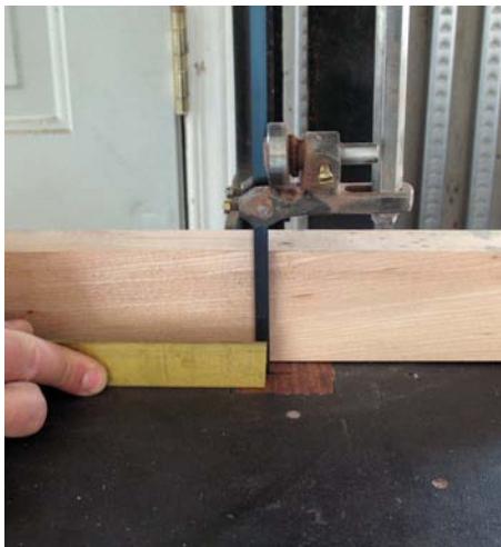
Cutting brass on the bandsaw is noisy, but easy
