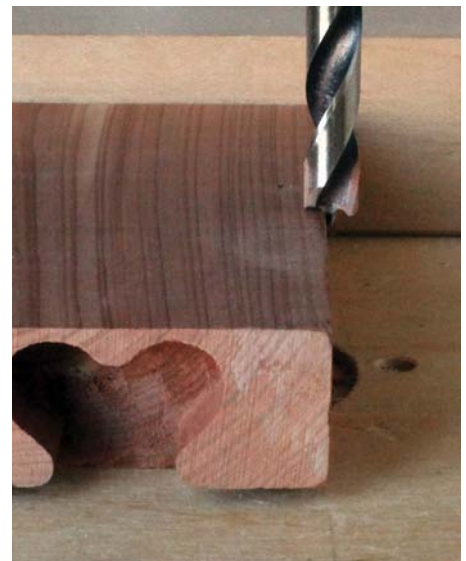
When setting the zero mark, make sure the cutting edge of the bit, not the spur, touches the surface of the stock
