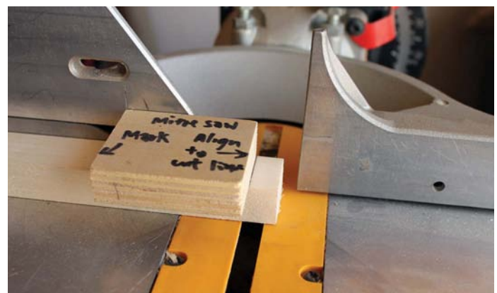
Align one end of the block with the cut line on the stock and the other end with the scored line
