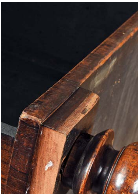
Cut with the grain to achieve a seamless joint
