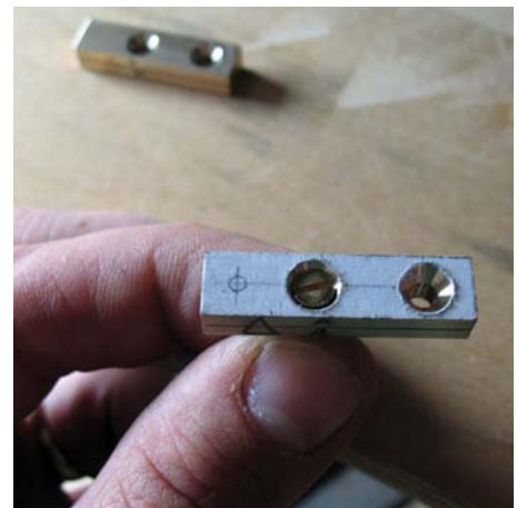
Use the depth stop on your drill press to guarantee consistent countersinks
