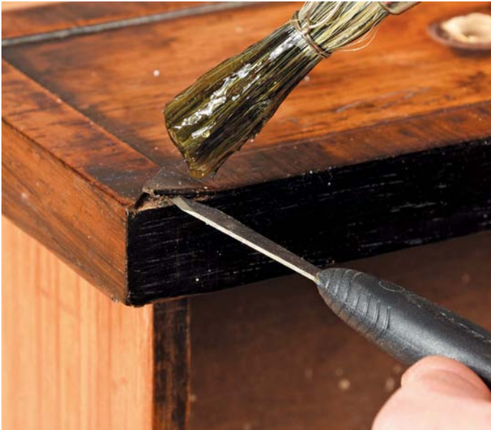
Take care of any loose veneer before carrying out any cleaning
