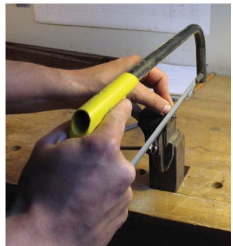
Definitely hold on to the drill rod when cutting the often short-and-hard-to-find-once-on-the-floor pins
