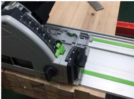
Trimming the slab to length
