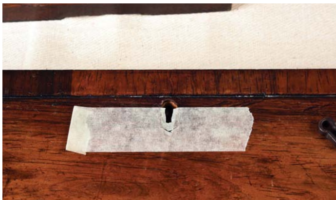
Use tape to transfer the shape of the new brassware
