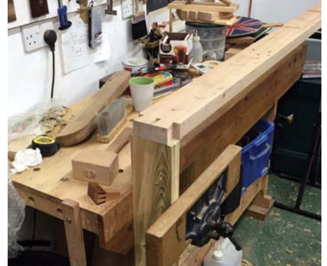
Marking the dovetails for the end cap
