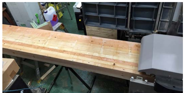
Keeping the slab under 410mm wide allowed rapid planing of the top
