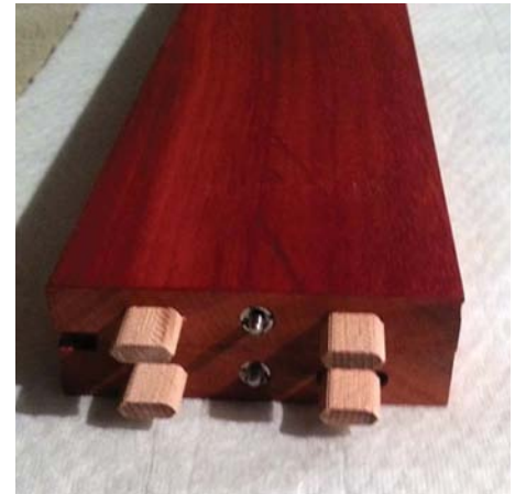
The lateral rail joints were drilled as standard and supported with Dominos
