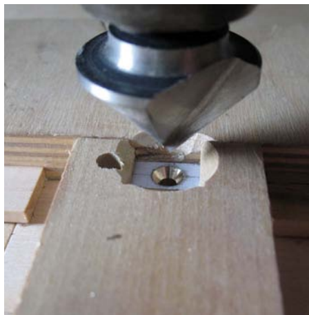
Ensure that your hold down has sufficient clearance for the countersink
