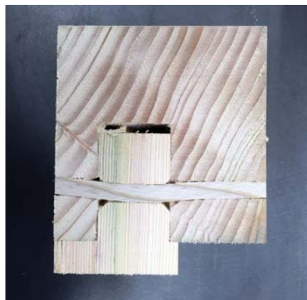
Successful trial drawbore joint with curve to 1/2in ash peg
