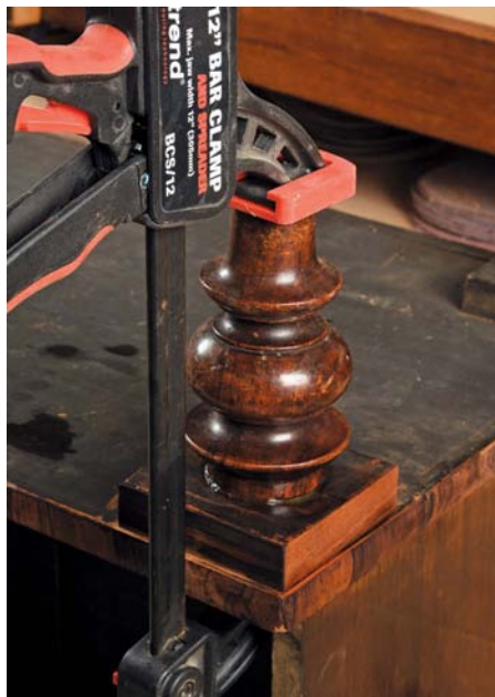
No need to completely disassemble. Just add hide glue and clamp
