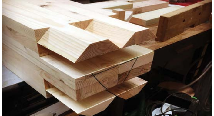
Legs after cutting the joints on the bandsaw
