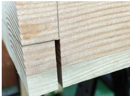
Shoulder cut with tracksaw
