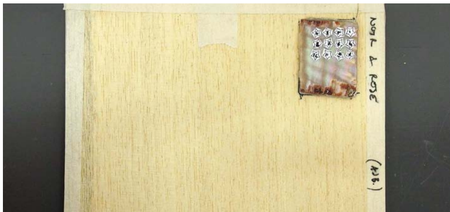
It may seem wasteful to create a large packet for cutting mother-of-pearl, however, the larger the waste material, the easier and safer it is to manipulate
