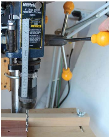
With the rule in place, lower the drill until the bit touches the stock and align the zero mark on the rule with the depth pointer
