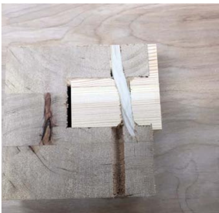
Failed trial drawbore joint with too much offset
