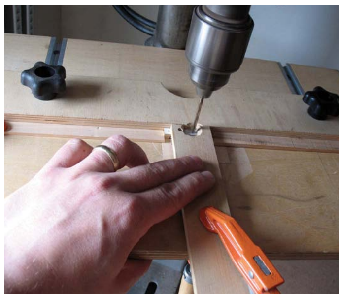
Carefully set up your drill press taking into account the different lengths of bits that are to be used. You do not want to have to move the table once you have started
