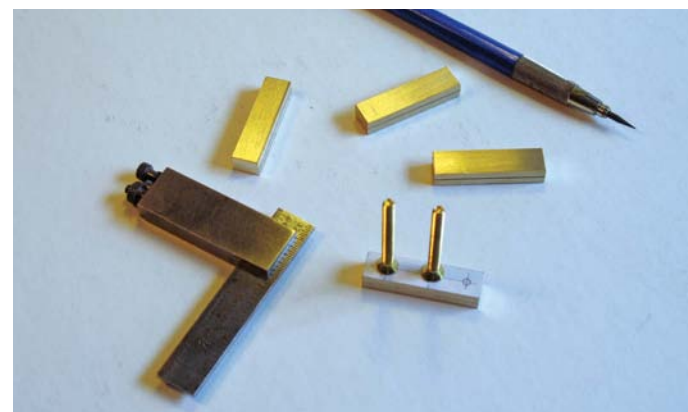
Generate layout lines on only one set of hinge leaves to reduce the chance of errors and maintain consistency
