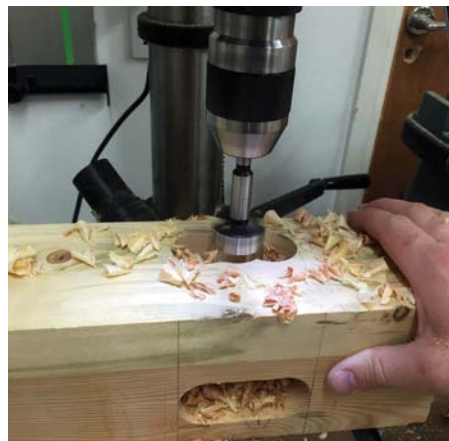
Drilling the waste with a 40mm Forstner bit
