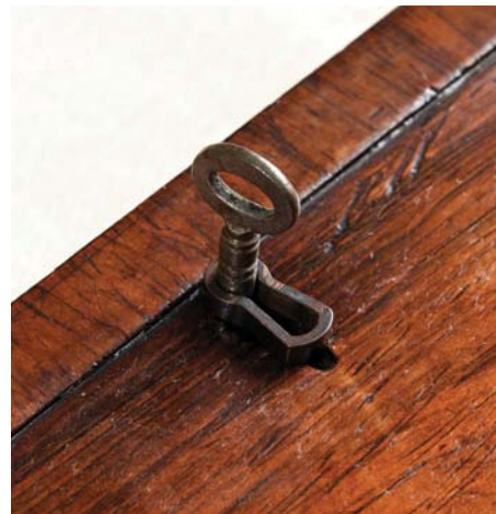
Test fit the escutcheon with the key to make sure it works
