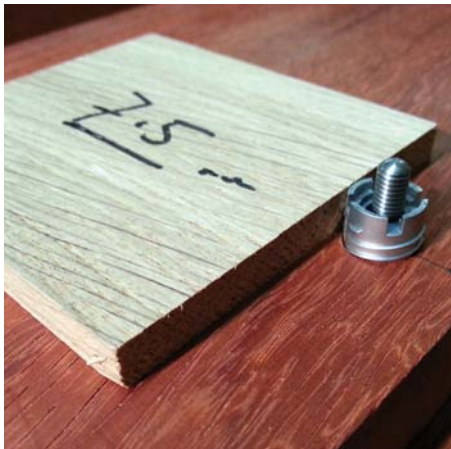
The male component fitted at the correct length, 7.5mm higher than the standard setting
