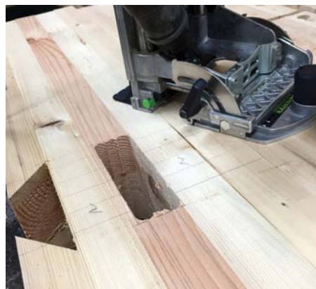
Roughing out the through mortise with a Festool Domino
