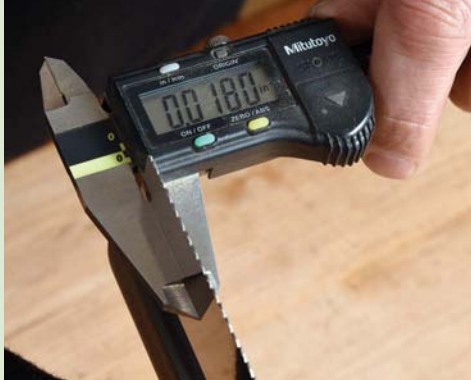
018 gauge dovetail saw typically for use on stock up to 30mm
