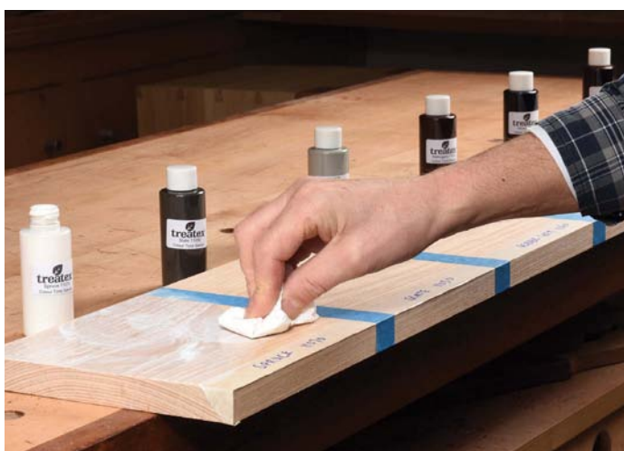
The base tones are a wipe-on wipe-off product
