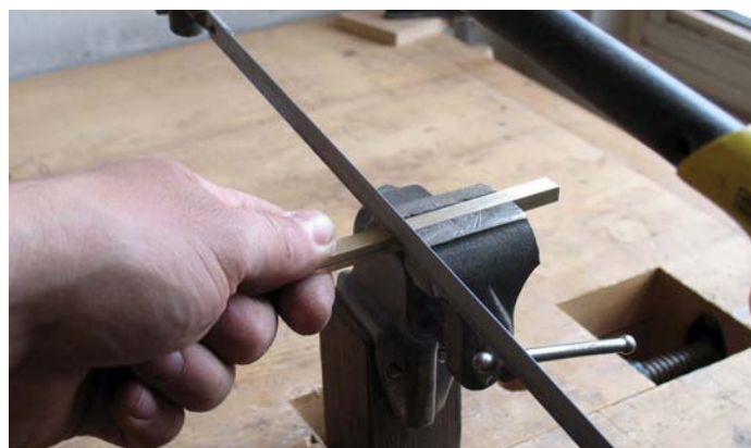
When using a hacksaw to separate the lengths of hinges, hold on. After the cut, true up the ends to make sure all the sets are the same length
