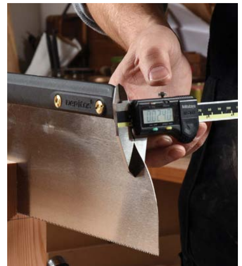
024 is a typical gauge for 410mm long and over tenon saws
