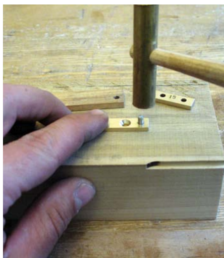
Gently persuade the pin into the press fit leaf. It's critical that the pin goes in square
