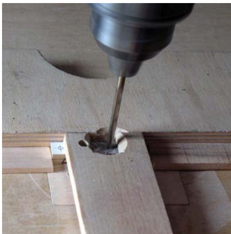
With the brass firmly clamped to the table, drill your screw holes
