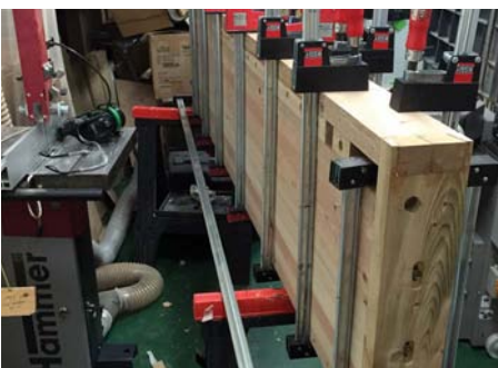
Laminating the final section to the main slab top
