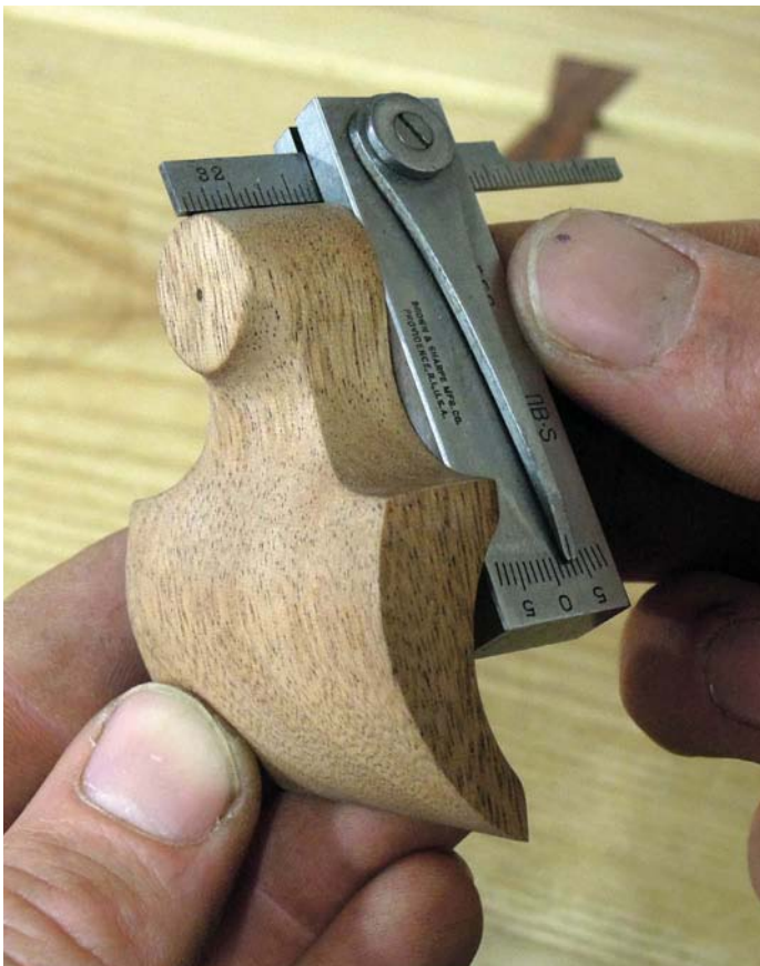
Checking the draft angle on a lever cap pattern
