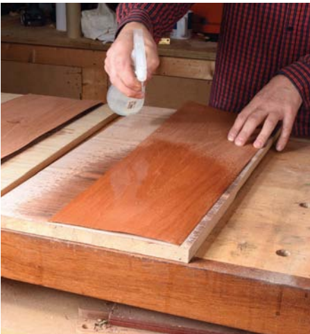
Dampen the veneer with a light spritz of water
