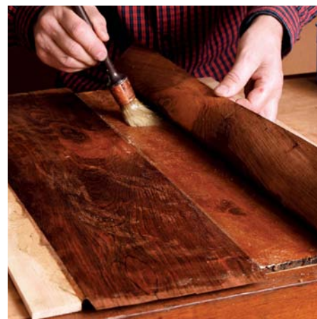
Apply glue to the rest of the groundwork...
