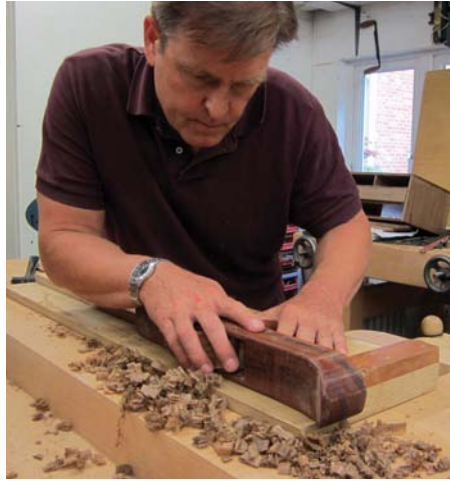
The walnut drawer fronts were marked from the backs and trimmed to fit with a slight outward taper on the shooting board
