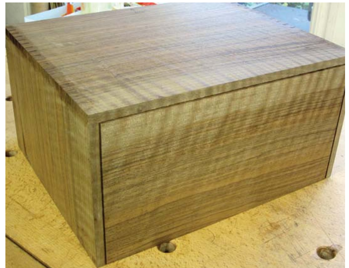
The back was fitted enabling the drawer sides to be cut to length
