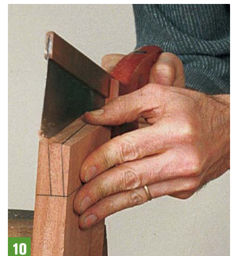
10 After knife-marking the shoulder lines, cut the tenon and shoulders with a backsaw, then trim to fit.
