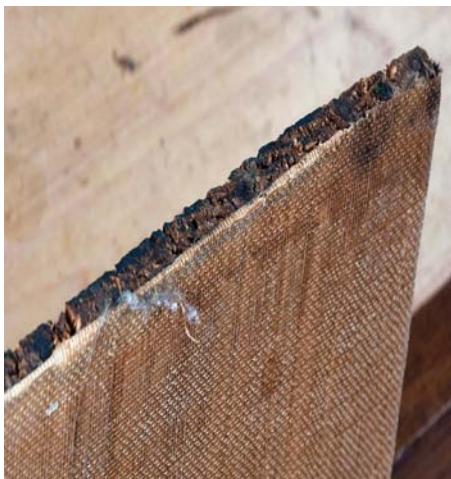
The top edges of our panels were riddled with pin holes
