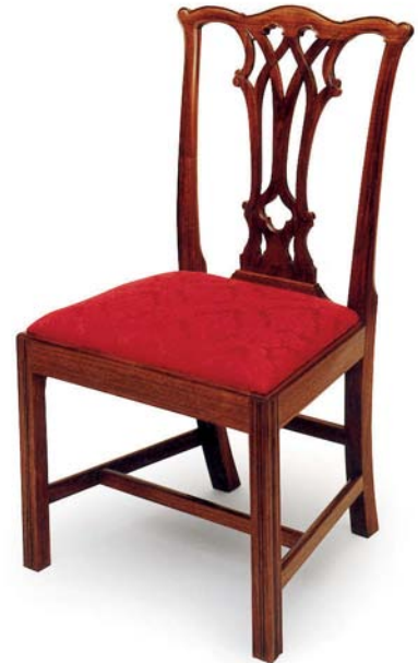
Chippendale – one joint, many chairs: No matter what chair you're building, if your back legs are canted and your seat is trapezoidal, you'll need to use compound-angle tenons to join them, as was done with this Chippendale chair by Rich Heflin
