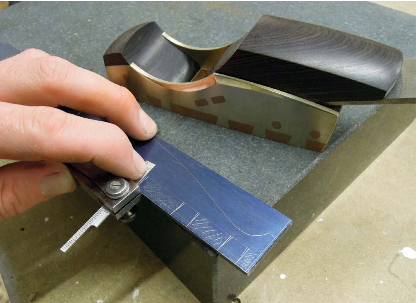
Laying out dovetails onto steel
