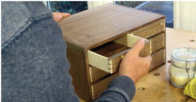
Lightly sand and then wax the drawer sides. Pushing the drawer in and out of its slot creates shiny spots which can be trimmed until a perfect fit is achieved
