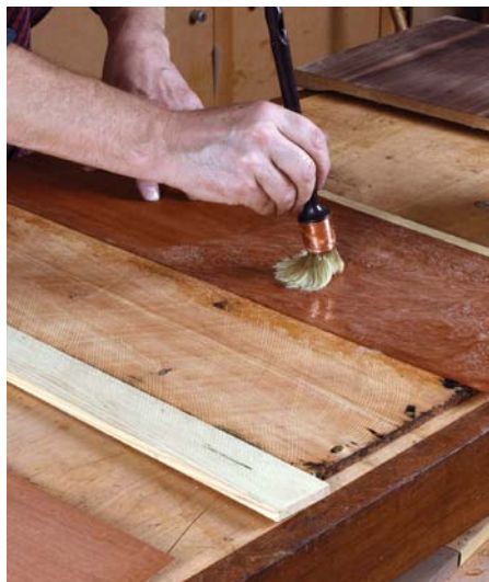
Apply a second coat of glue to the top face of the veneer after it's been laid
