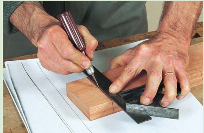
Knife marks are more exact. Once the tenon shoulder has been correctly marked, knife-mark the lines on all sides of the rail. The knife marks provide a specific line to pare or shoulder-plane to
