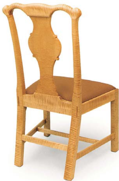
Country Chippendale in any style: Made of curly maple, Mary Conlan's Chippendale chair of simple form is built using the same leg-to-rail joinery as a more flashy, high-style chair
