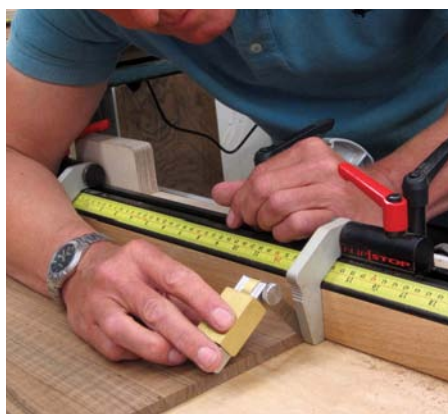
Verifying the taper between two fixed stops
