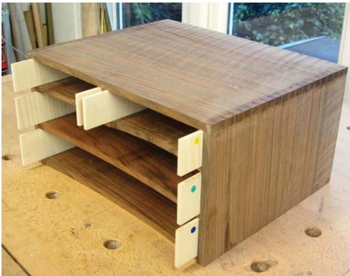
With the carcass glued up each drawer side could be shot into its opening and marked with a coloured dot
