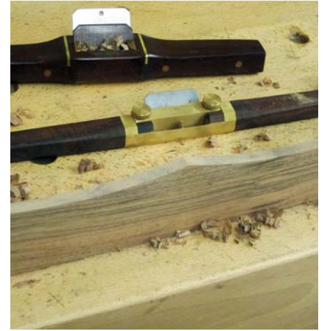
The curved fronts to the rails were shaped with flat and curved HNT Gordon spokeshaves
