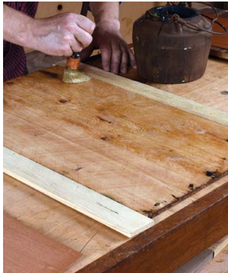
Apply glue to enough of the groundwork for the first leaf
