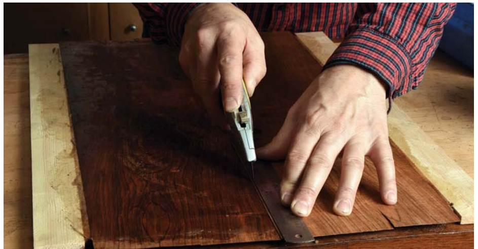
Cut the two veneer edges at the same time
