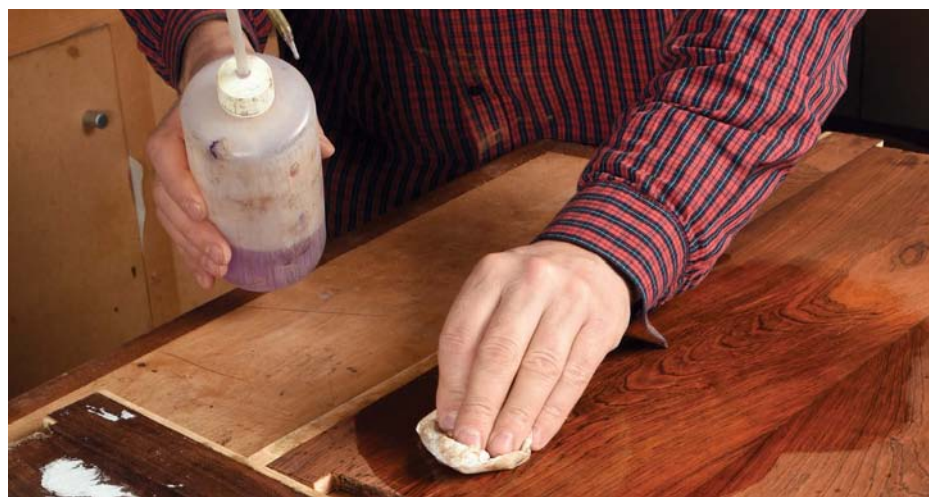
Expel the excess glue via the joint line
