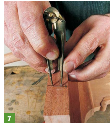
7 With the dividers still set to the mortise width, measure from point y to mark the tenon width at the top of the rail.
