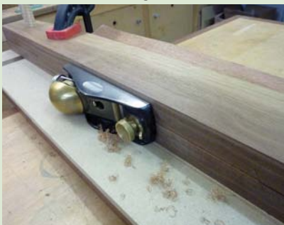
The jig doubles up as a shooting board for veneer as well
