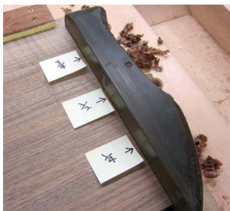
Progressive shavings being taken from each side on the shooting board to create a minute taper
