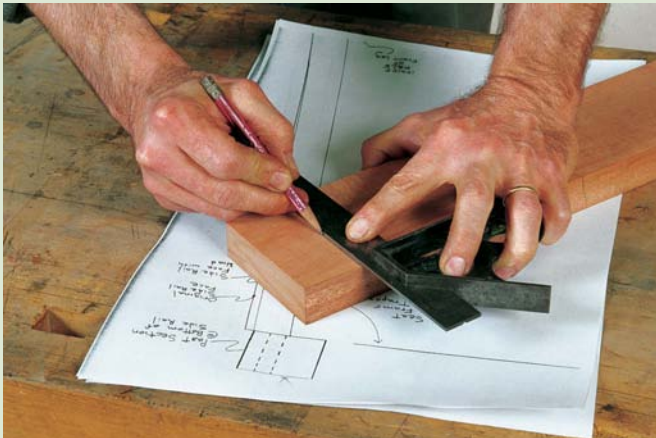
Marking the first face. Set the side rail into place over the drawing – make sure there's enough stock for the full tenon. Make a tick mark on the bottom inside corner of the side rail, and pencil in the shoulder line on the inside face
