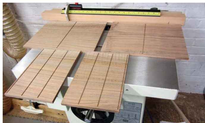
The stopped grooves being cut on the shaper with a 3.25mm bit
