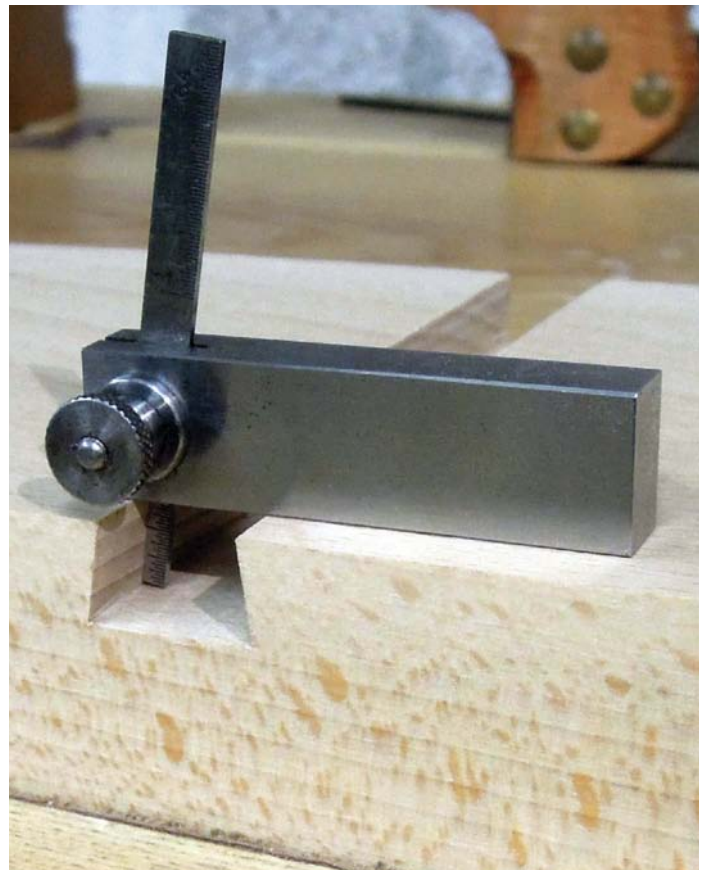
Checking the angle on a sliding dovetail
