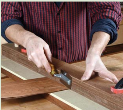
Trimming veneer oversize with a veneer saw on the 'shop made jig
