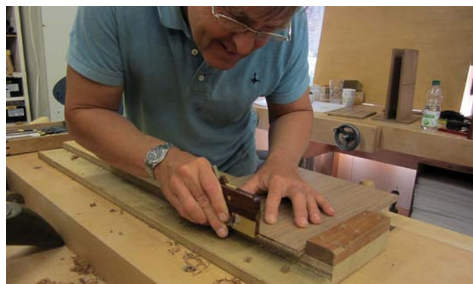
The stub tenons were trimmed to a tight fit in the grooves
