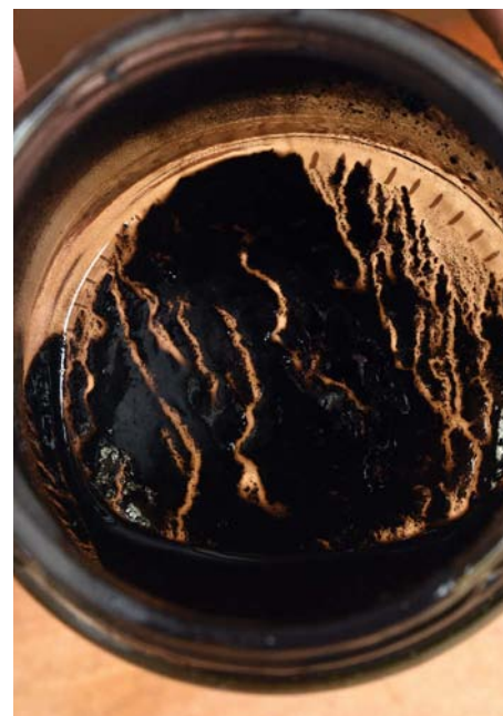
When the shellac has dissolved what's left at the bottom of the jar is a slurry of various earth pigments
