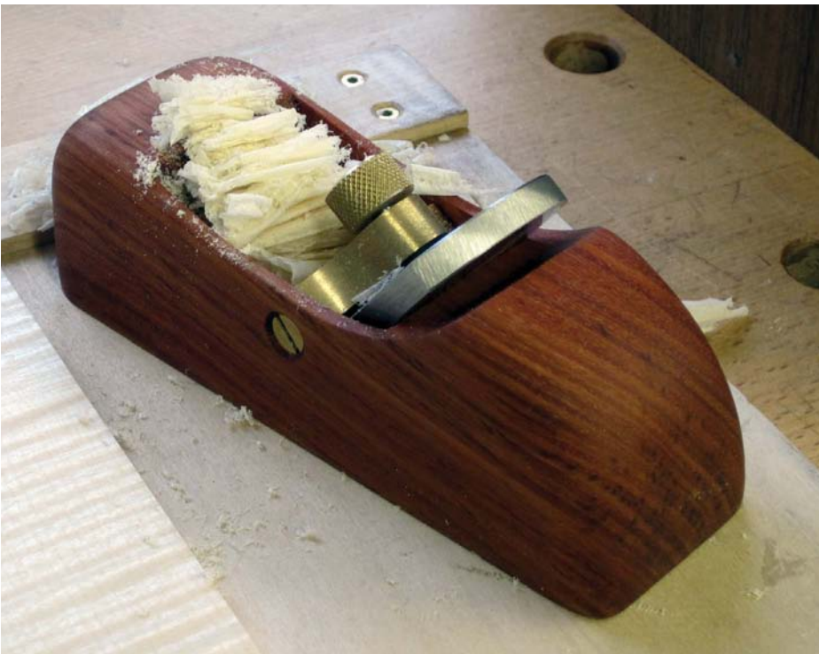
Bringing the inside of the drawer parts to a finish with a high angle smoother
