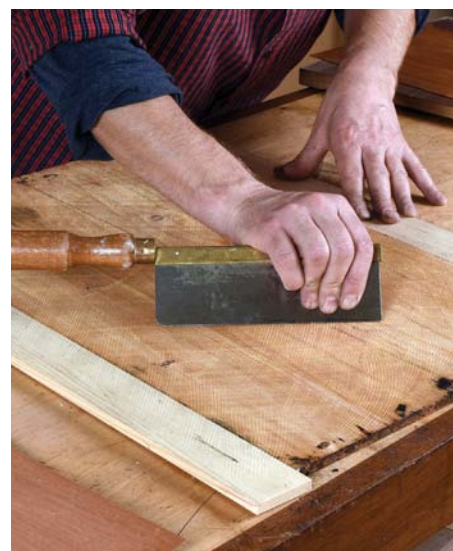
Score the surface of the groundwork to help with adhesion
