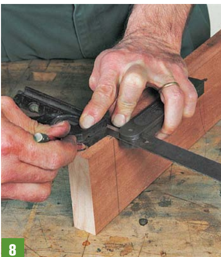
8 Tenon cheeks are marked perpendicular to the shoulder line by registering a square against the bevel gauge – which is still set to the trapezoidal seat angle.
