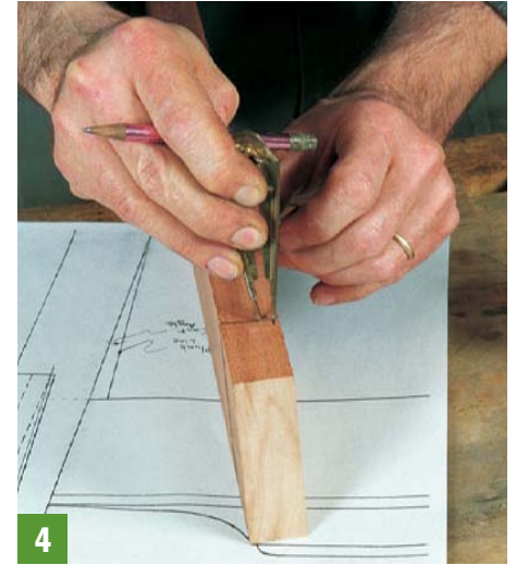
4 Use the divider setting from step 3 to locate point y on the top edge of the rail, measuring from point x .
