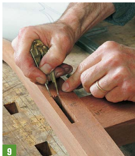
9 After the top and bottom of the tenon have been marked, use a straightedge to connect the points and complete the layout.
