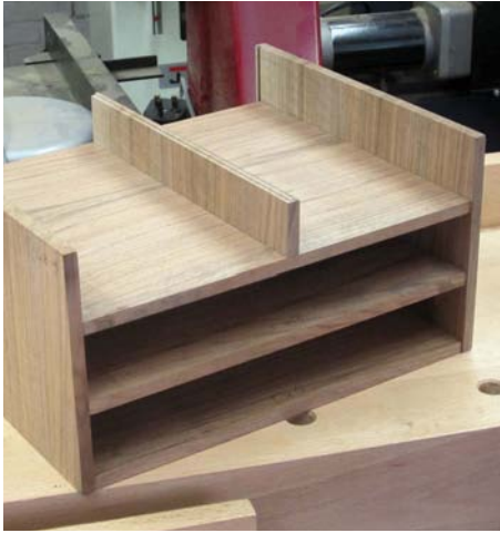
Dry fitting the carcass parts, tapers can be checked at this stage
