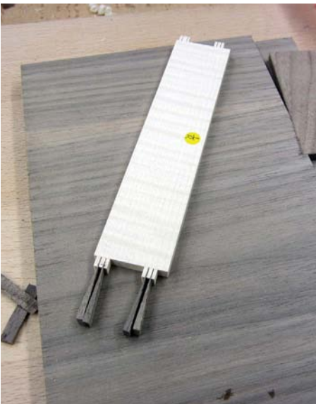
Identical tapering wedges cut for the through tenons
