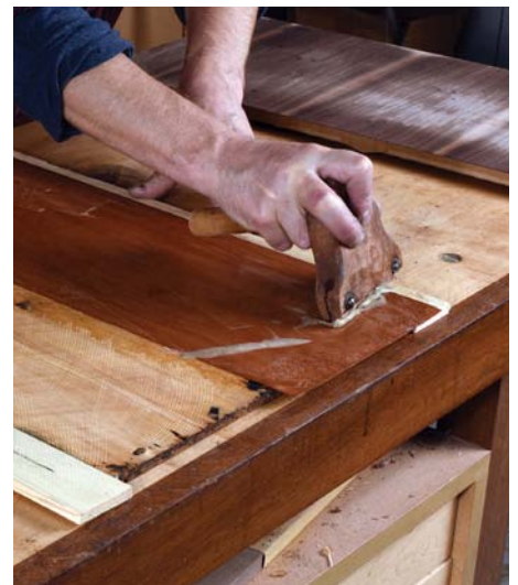
Use more force with the veneer hammer to expel the excess glue from under the veneer
