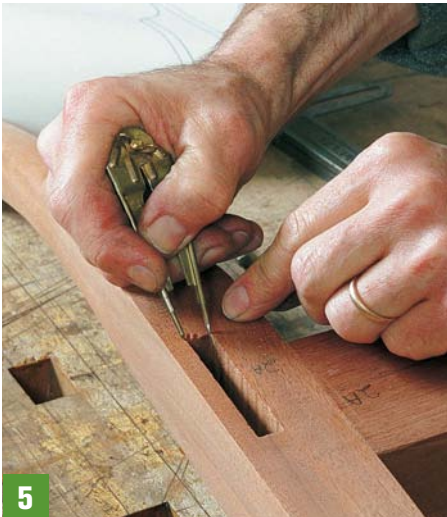
5 Set the dividers to match the mortise width on the rear leg of the chair itself.
