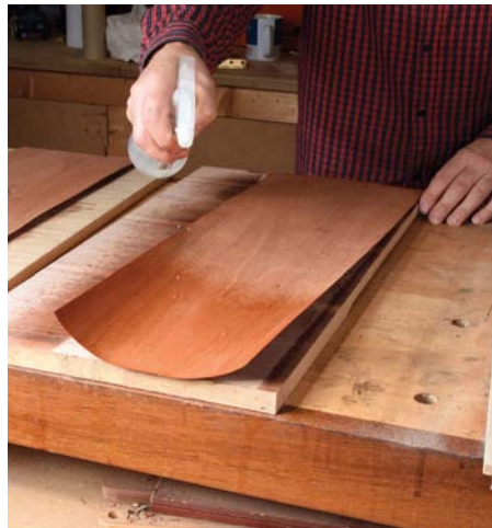
Treat both sides the same to equal out any cupping
