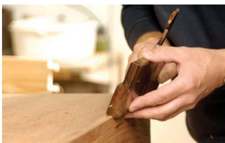
Break out the moulding planes to put an authentic round-over along all the edges
