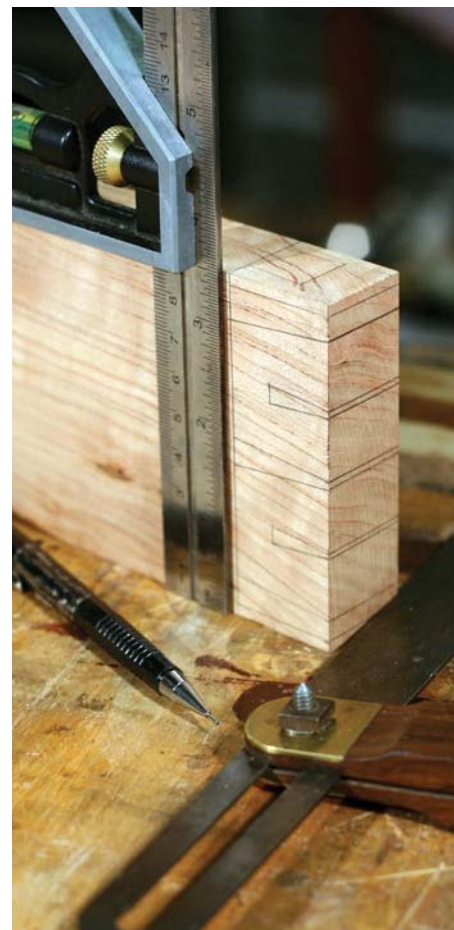
Lay out in fine pencil rather than scoring with a knife
