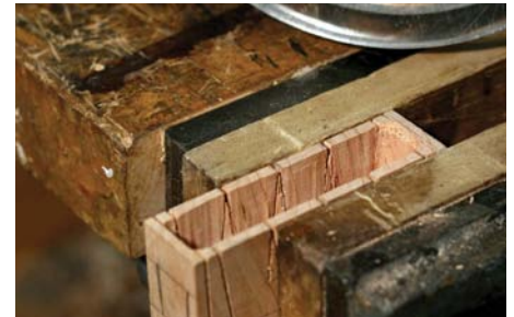
Rout out the waste from the middle of the board, stopping right below the tail line
