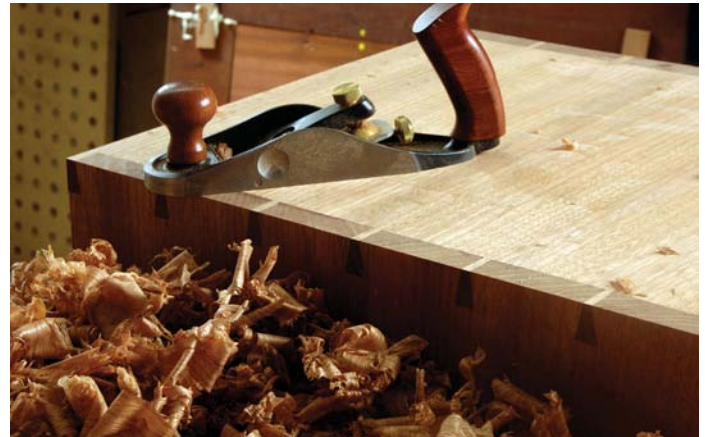
Level off the box and trim the top to match its shape
