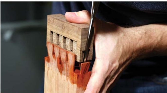
Gently prising out the top and bottom tails while the wood is still pliable
