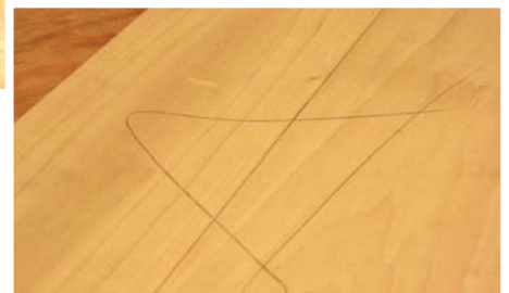
The edges were planed straight and square relative to the board's reference face
