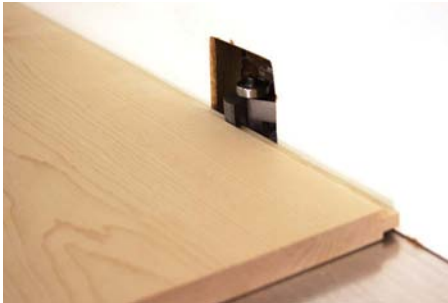
The tongue bit removes waste from both sides of the joint in a single pass
