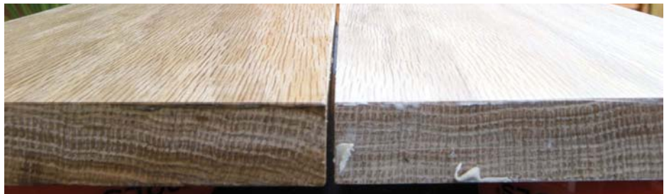
When the weather is good nothing beats finishing in the open air. Here you can clearly see how the panel filled with Aqua Coat (left) has a darker finish and greater contrast than the panel filled with my usual brand of filler. This is before any lacquer has been applied
