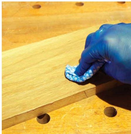
Aqua Coat is easily applied with a cloth, simply rubbing in small circles across the grain
