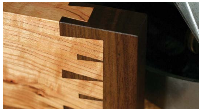
After a few clean-up passes with a hand plane the joint is finished
