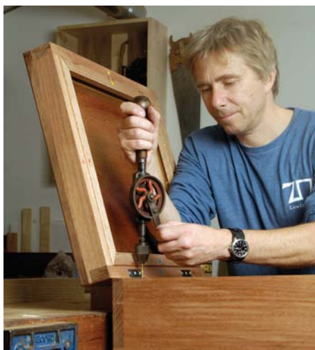
Re-drill the holes carefully
