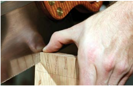
I clamp my tail board to where my angled lines are vertical so I can make more consistent cuts each time
