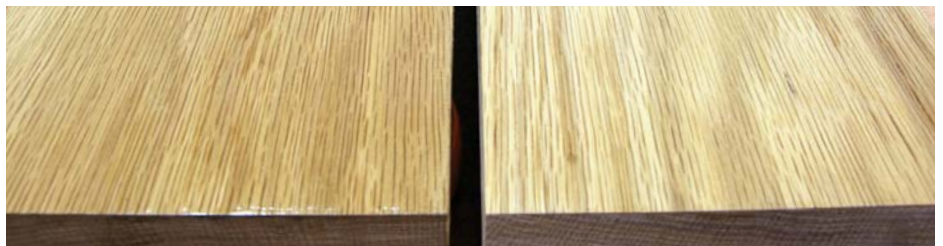
After two coats of lacquer, the effect of the different grain fillers remains very noticeable. The Aqua Coat (left) still has a higher level of gloss and a warmer colour than my usual filler
