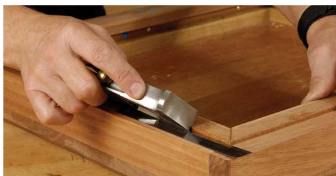
Put a slight chamfer on the leading edge
