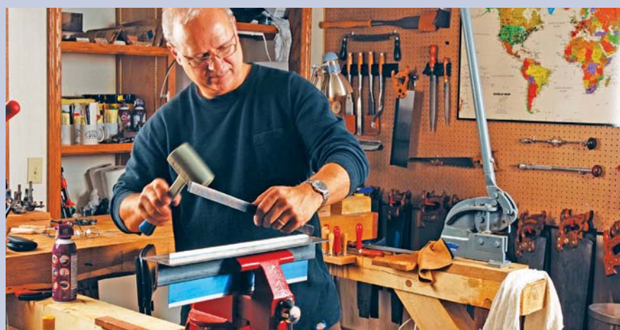
Mark Harrell, from Bad Axe saws, applying a traditional folded sawback with the aid of a dead blow mallet
