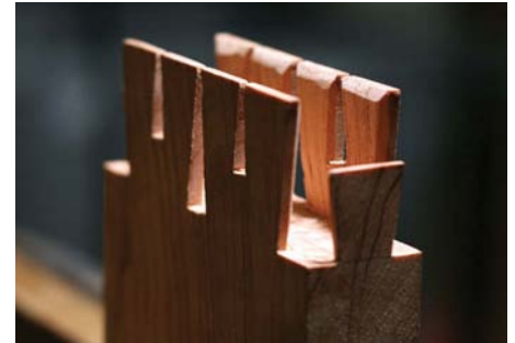
The sides and tops of the tails all have bevels on the inside edges
