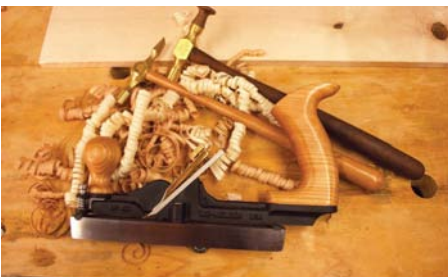
A light tap to the back of the blade will increase the depth of cut
