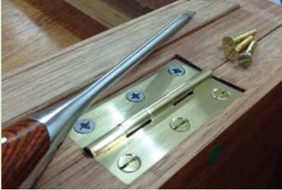
Aim to fit the brass screws just the once
