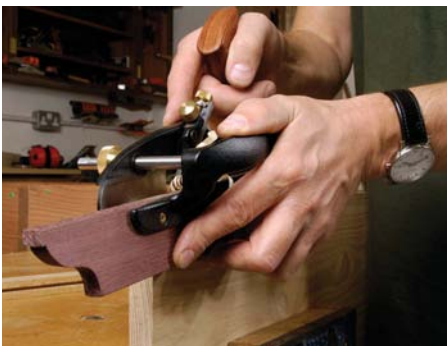
Tip the nose of the plough plane towards the ground at the far end of the board to establish the cut when cutting with the grain
