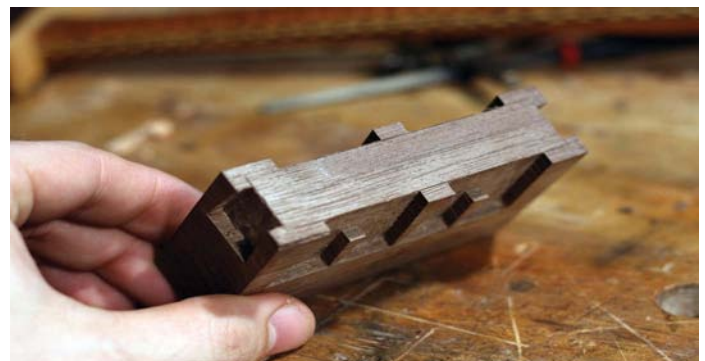
The finished socket board with shallow pins
