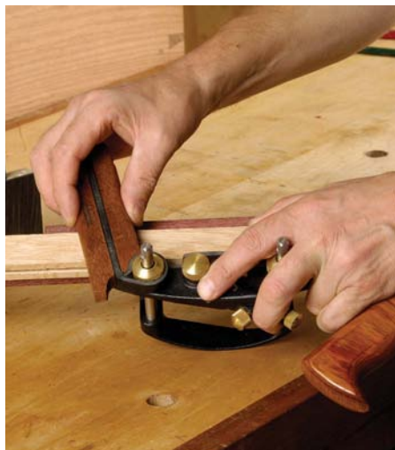
The Nut Saver from Bernard Bilsberry is the perfect tool for fixing the fence on your plough plane so it won't budge
