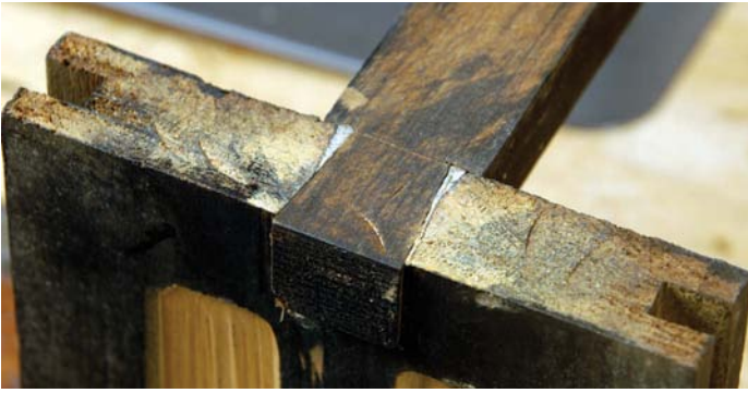
The support strut is now holding the central runner upside down. Note the two arrow-head shaped wedges of new material
