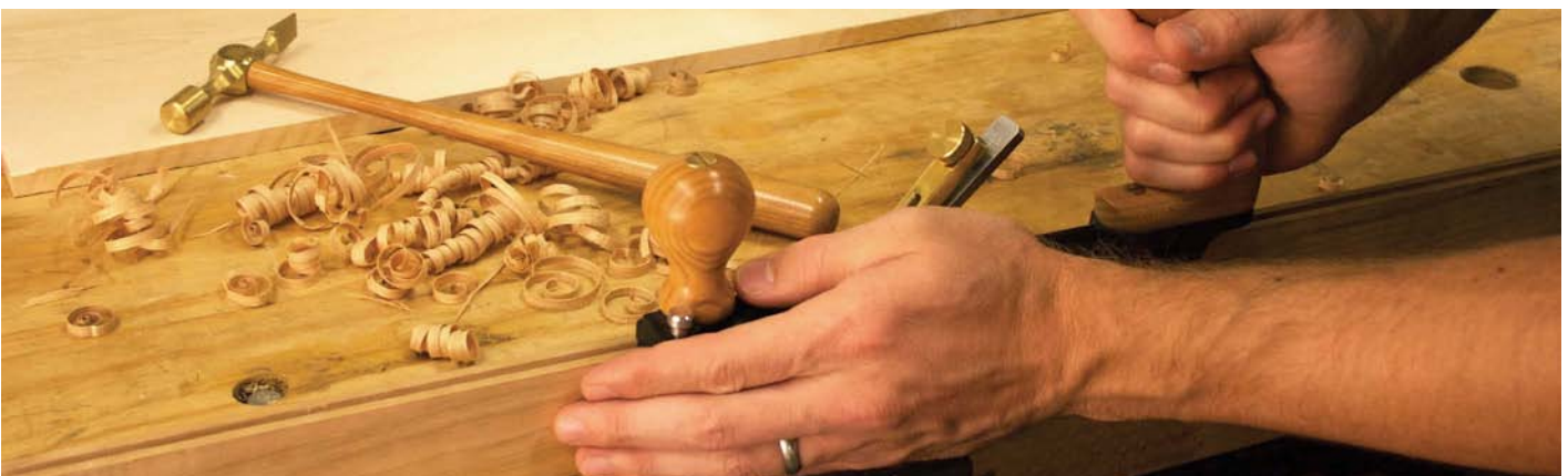
Press the fence firmly against the reference face with one hand and push forward with your other hand
