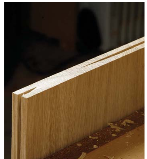
Point the nose of your plough plane skywards at the front of the board to establish the cut when cutting end grain
