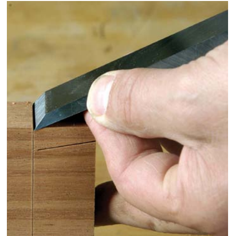
Protect the shoulders from saw drift by creating a trough for the saw to sit in
