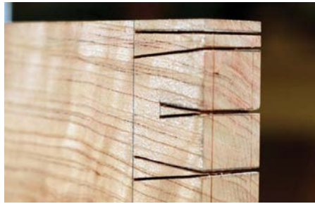
All lines cut, including the top and bottom tail walls. It looks wrong but trust me
