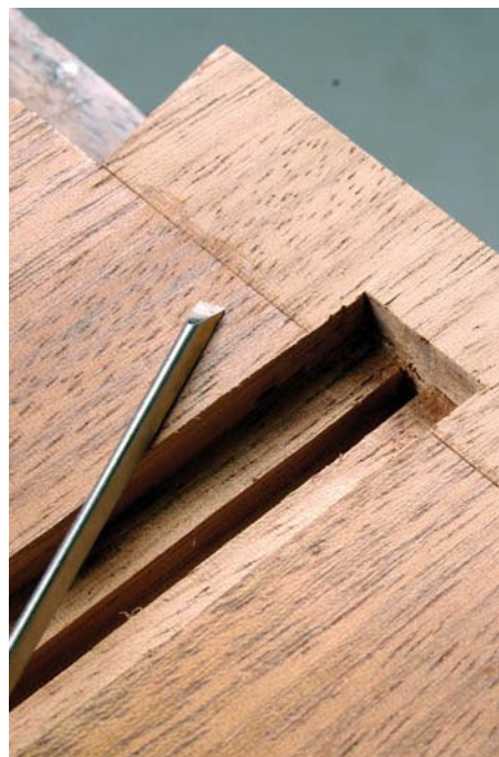
Overshoot the groove and clean out the round corners
