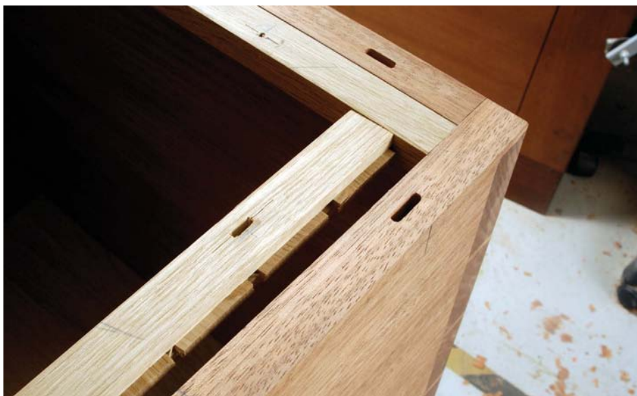
Cut slot holes in the buttons that will register with the sides and back edge of the top
