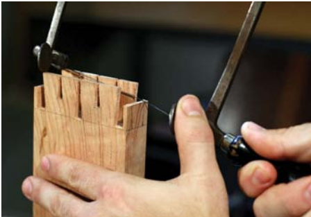
Cut the top and bottom tails with a fret saw. Use some packing material if you need to
