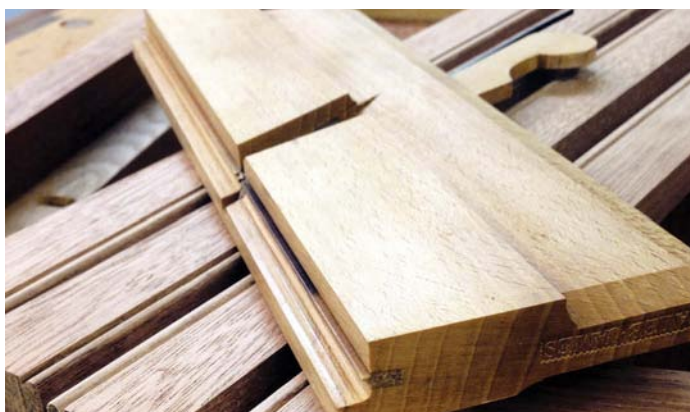
Add a little edge bead detail to the dust seal
