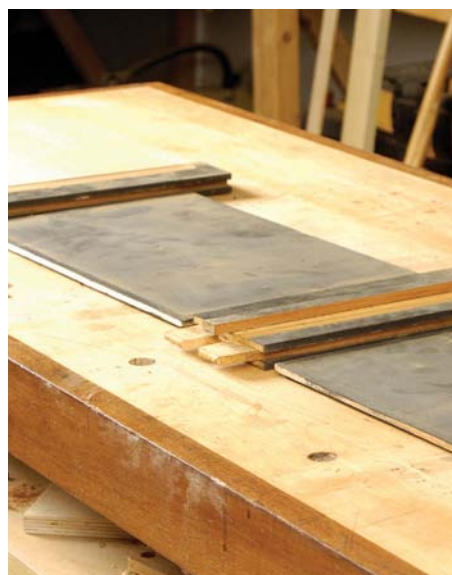
A combination of full-length and stub tenons locate the runners into the front rail
