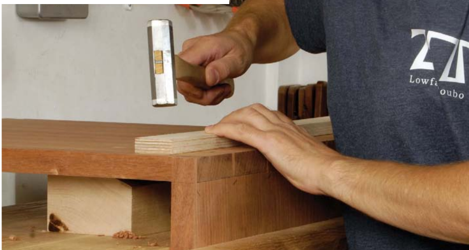
Protect the edges of your joints with support blocks above and below when dry fitting large components
