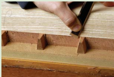
Keep your paring square and in line by using a reliable straight edge to guide the chisel. Cut at an angle away from the pins when working from the face of the board to avoid damaging them at the back side.
