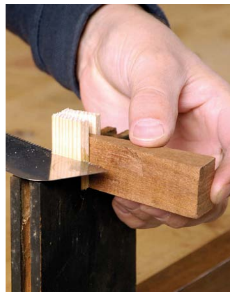
Keep the wedge in place after the glue has dried while you trim the bulk of the waste
