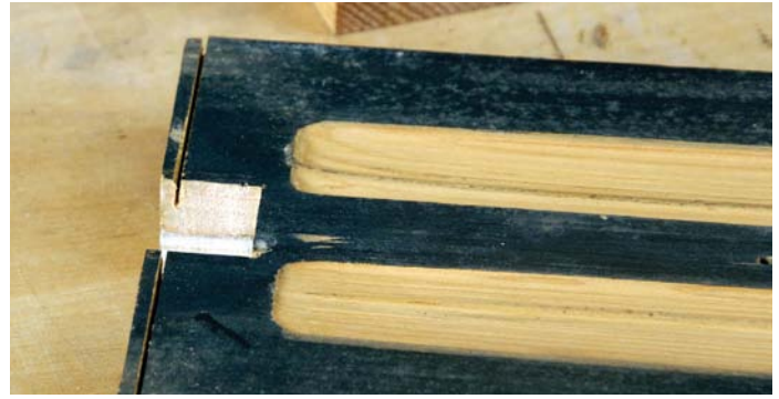
The central runner needs trimming to length to match the width of the carcass sides. The dovetail socket was increased to suit
