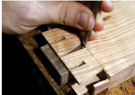
Cleaning up the tails with a support block placed beneath within the void
