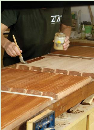
Carry out as much of the finishing on the inside faces as you can before assembly
