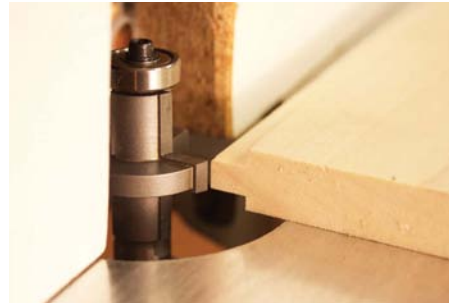
The groove bit can be setup initially by eye from the edge of the tongue profile
