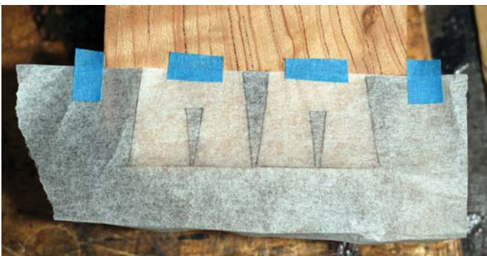
Tracing paper for transferring tails. I use the two side pieces of tape as a way of registering the position of the tails
