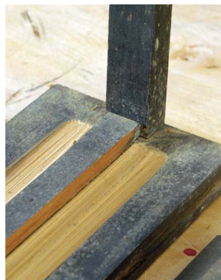
The runners are well worn with channels wider than the combined thickness of the original drawer sides and slips
