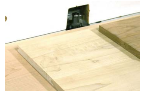
After all the grooves are cut, the boards are ready to assemble
