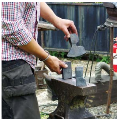
Nic Westermann demonstrating the stages in forging an axe head from a blank piece of steel
