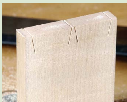
A 20 tpi dovetail saw cuts smoothly on thin stock with a clean face edge kerf on sycamore
