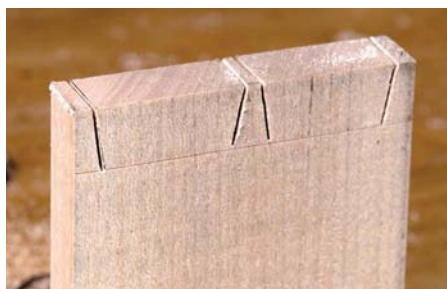
Timbers behave differently. The same 14tpi dovetail saw has a clean kerf on the face side of the board...
