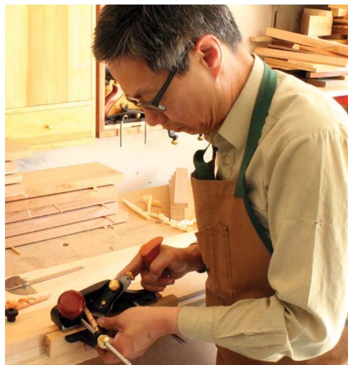
I made a 5° angle fence and made a few test cuts to verify the bevel angle on the scrap
