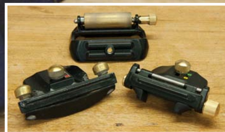
The neat new narrow blade carrier on the right alongside the standard carrier with the roller assembly above. Note the curvature of this much used standard clamping bar, the result of the clamping pressure necessary for a secure hold
