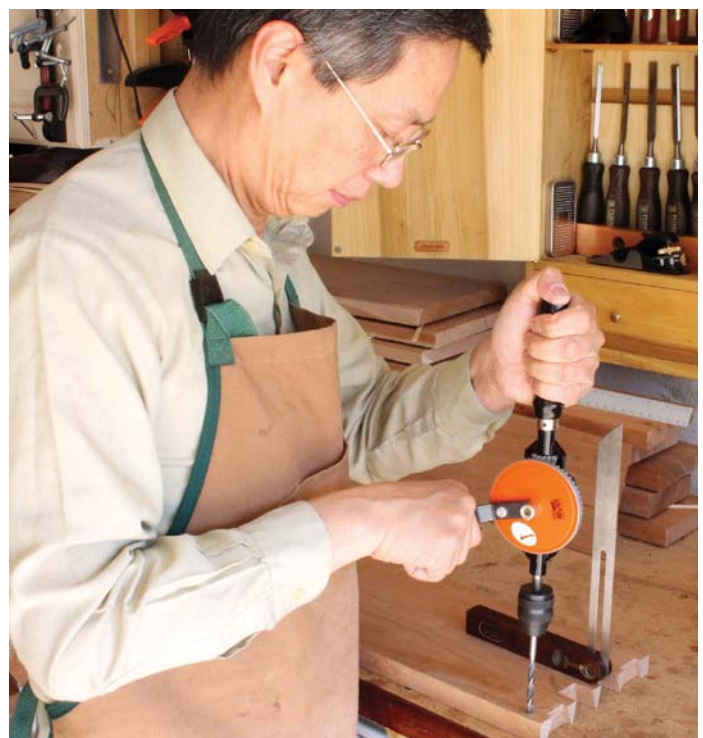
I drilled two stopped holes for the groove to guide the chiselling work
