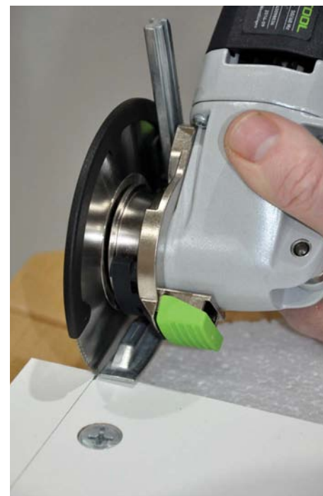
Using the sliding shoe guide at maximum depth of cut is not easy if starting at an edge – it really does need to be longer
