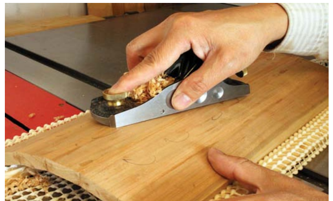
I placed spacers under the board before I shaped the top with circular slicing cuts
