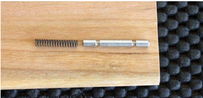
The spring-loaded pin hinges make a strong and invisible pivot for the lid
