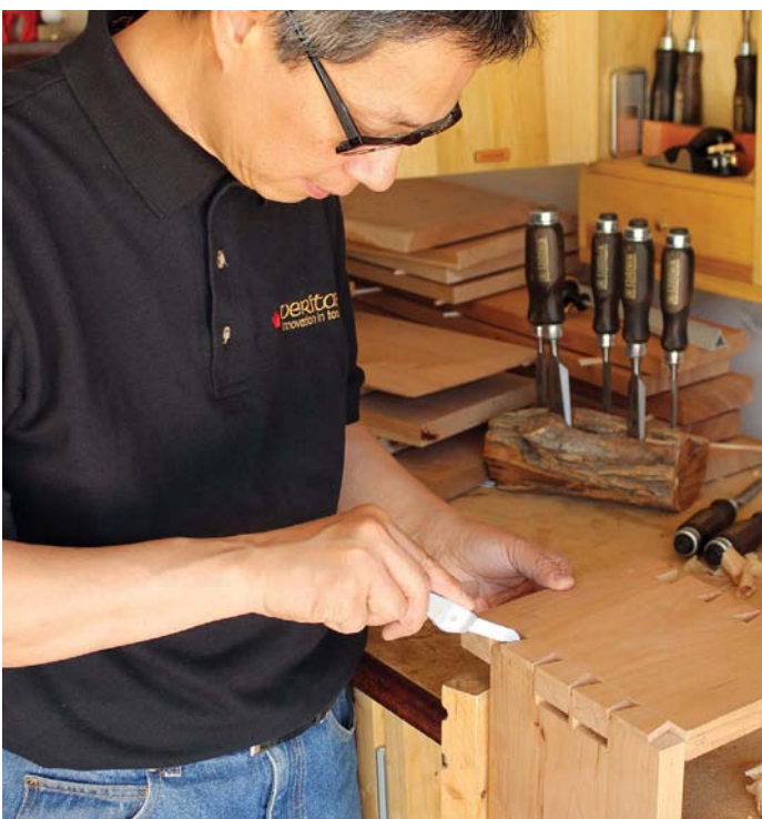
With the tail and pin boards partially assembled, I marked out the pins for the thin tails
