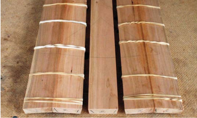
Rubber bands work well as coopering clamps for staves that are not too wide
