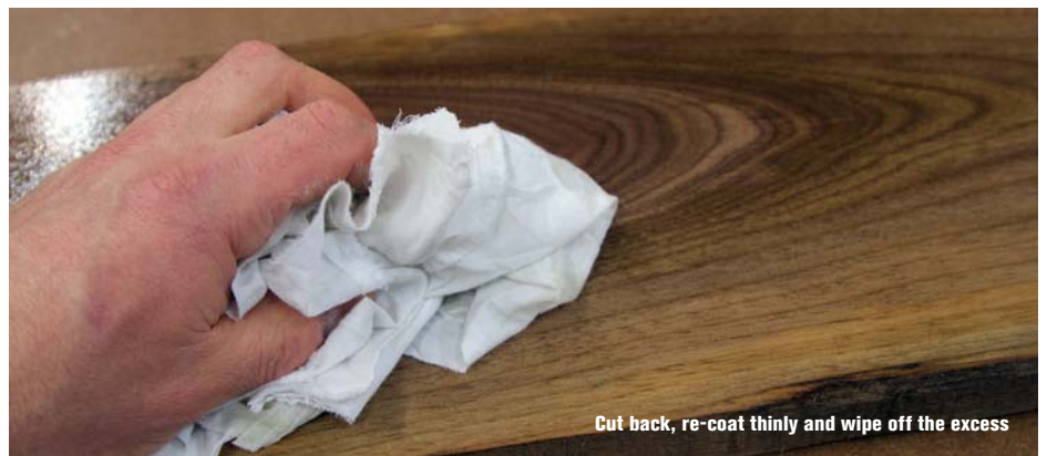
Scratch pattern eliminated and an even sheen
