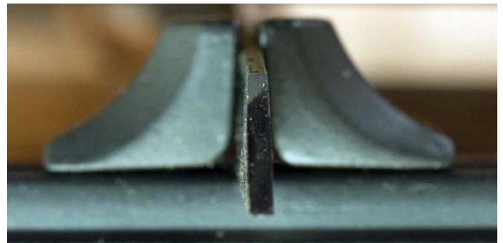
... while the almost parallel upper section is good for rectangular section blades like this 1.5mm Japanese chisel. With a chisel this narrow care must be taken to ensure it is clamped square in the guide
