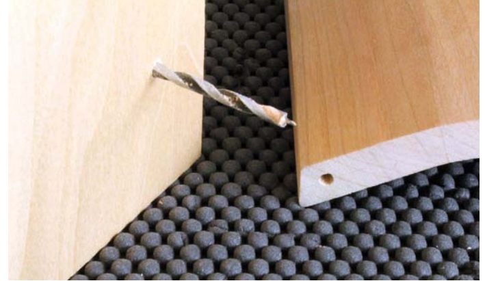
A scrap board with a predrilled hole acted as a guide for precision drilling
