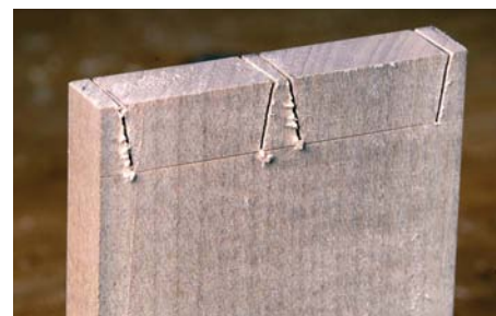
...but a ragged edge on the exit side of this board of sycamore suggesting it's less suitable for gang cutting pairs of drawer sides
