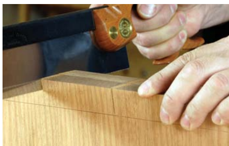
This 14tpi dovetail saw leaves a clean kerf on the exit side of this stack of mahogany making it suitable for gang cutting
