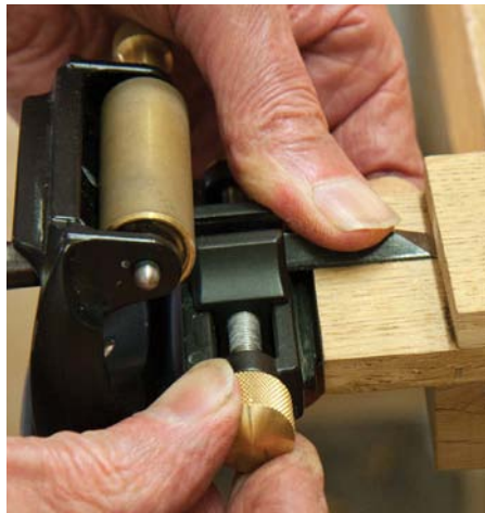
This simple blade projection setting jig can be made from oddments in about 20 minutes ...
