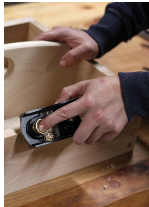
The wide sole makes it an excellent chamfering tool ➤
