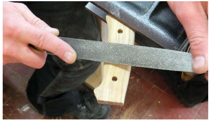
Use a rasp to shape the timber
