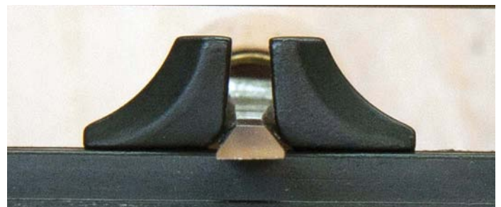
The rounded bottom corners of the jaws effectively clamp bevel edge or triangular section chisels ...
