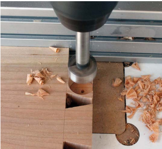
I drilled out the waste in several passes to avoid splintering
