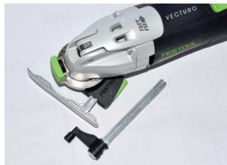
The sliding shoe and depth stop accessories. The orientation of all three attachments is easily changed by depressing the large green button on the gearbox, allowing the attachment to rotate. Depth adjustment is also very easy
