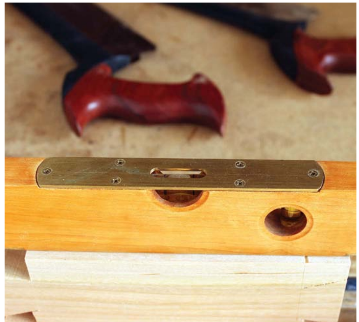
The shop-made torpedo level with a plumb vial is an essential part of my dovetailing kit
