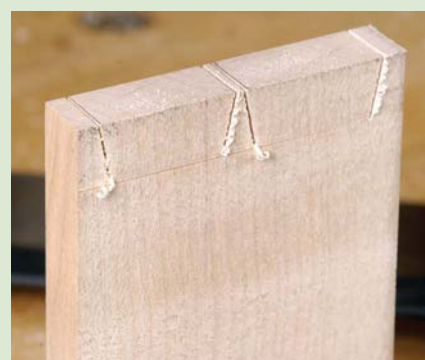
The exit kerf, however, is far from perfect with the threads concealing the lines
