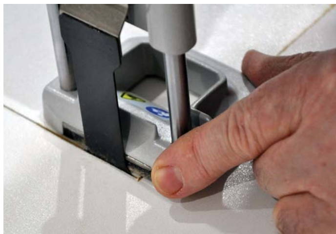
Plunge cutting into thin material was easy and I was able to cut a quite accurate straight line. A strobe light to 'stop' the blade would have made the end of the cut more accurate
