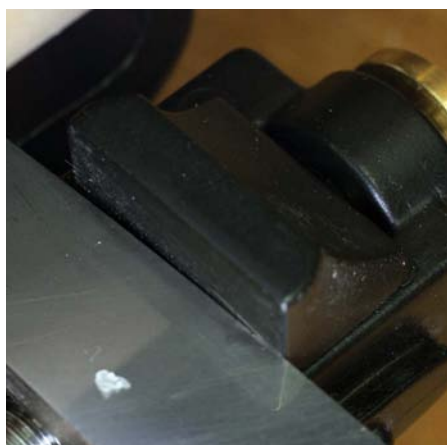
A Veritas DX/NX block plane blade automatically clamps square at 30° because there is sufficient length of parallel blade but at 25° the blade all too often ends up out of square because the extra blade projection needed throws the jaws almost completely onto the non-parallel part of the blade sides
