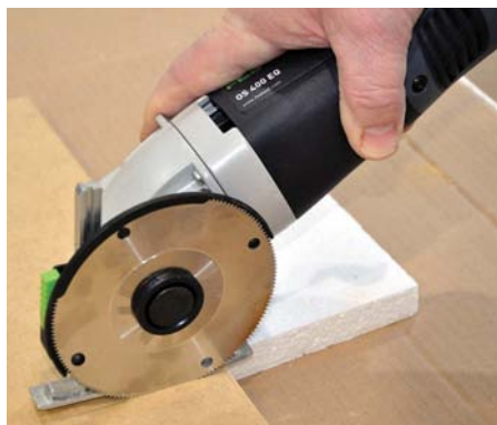
Using the same guide on thin material shows it can work well – it just needs to be longer
