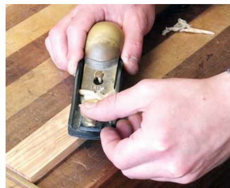
Use a block plane to flatten and square the blanks
