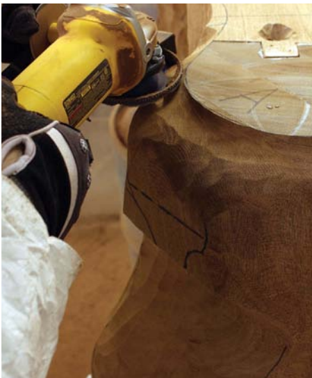
17 Grinding the bottom of the legs to reach the radius shape
