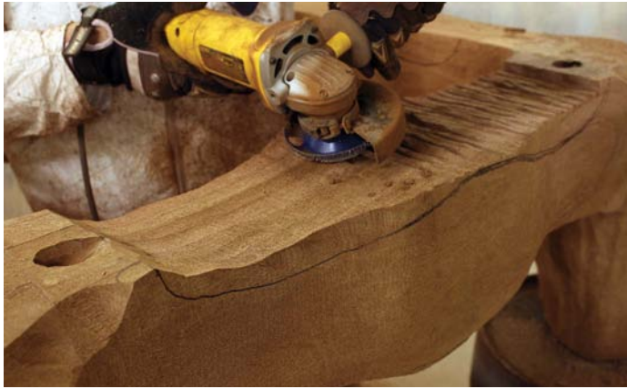
19 Using the coarse grinding wheel to remove the bulk of the wood
