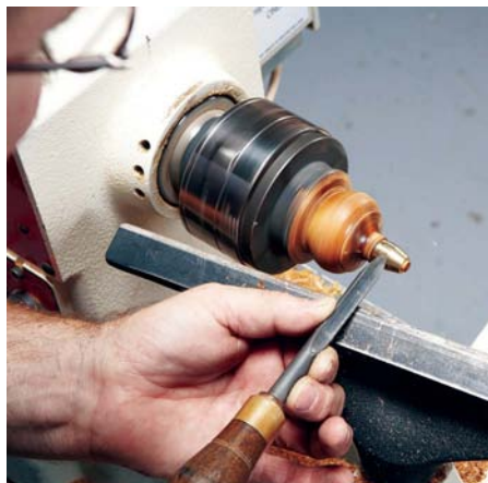
3 Turn away the flats of the nut and shape the ferrule with a detailing gouge. Cutting brass and copper on the lathe is similar to cutting wood. However, take light cuts
