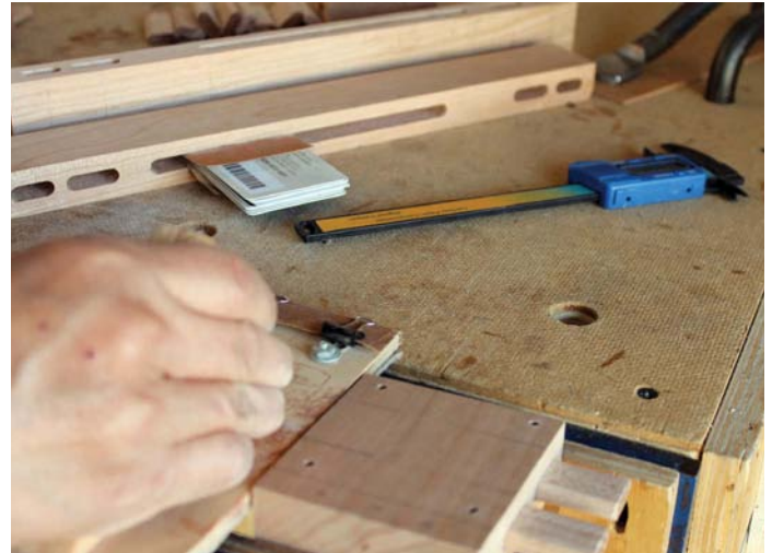
Sand or plane down the tenons on the sliding spacer plate for a snug fit
