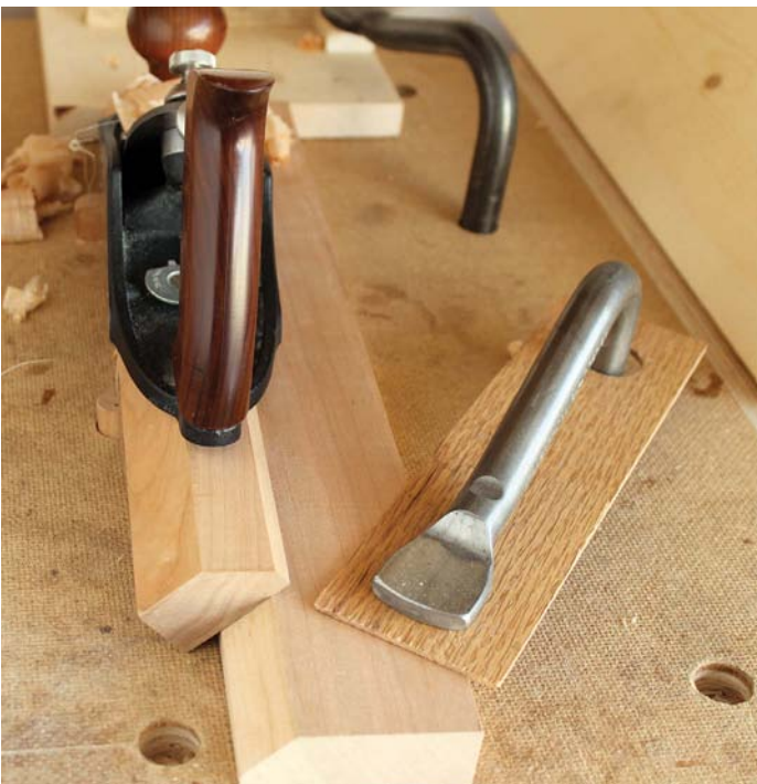
I orientated the bevel face up with an offcut so I could plane off the saw marks on the bevel
