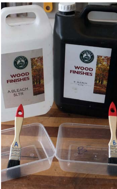
A and B bleach – as you can see here, containers and brushes are labelled accordingly
