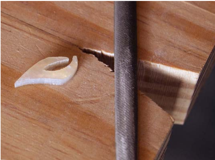
Refining the shape of the mother-of-pearl leaf with a needle file. Here you can also see the birdsmouth support I use for cutting the shell
