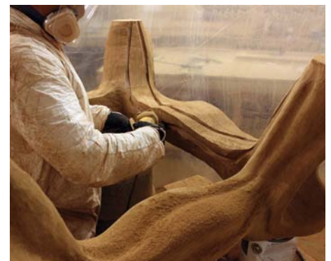
23 Using the side of the grinding wheel to cut into the hardwood
