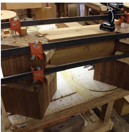
12 Using bar clamps screwed to areas where wood will be ground away
