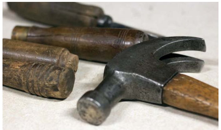
Steel-headed hammers damage chisels
