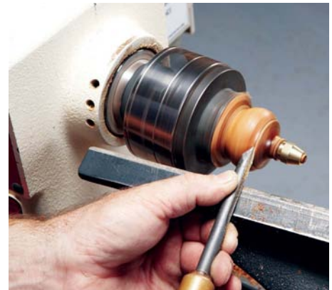
2 Rough in the basic shape of the handle with the detailing gouge. The shape and size of the handle is up to you
