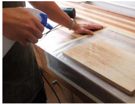
Spray with water to raise the wood fibres
