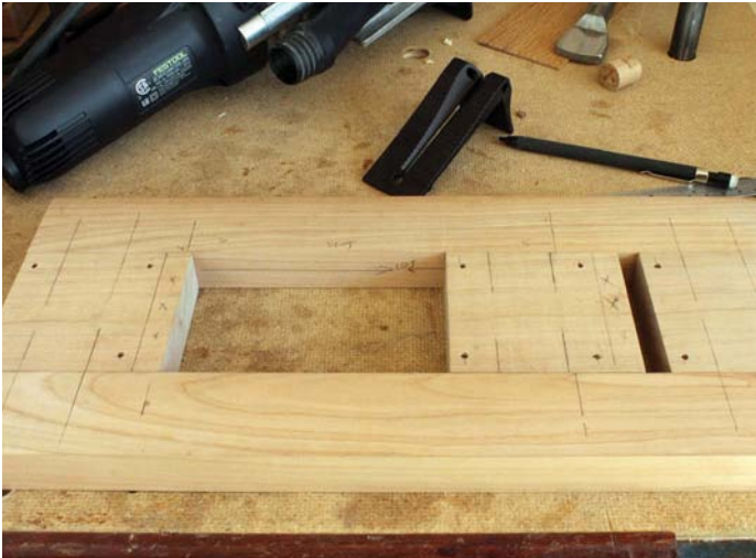
I started with oversized spacer plates and after mortising, cut them to final size
