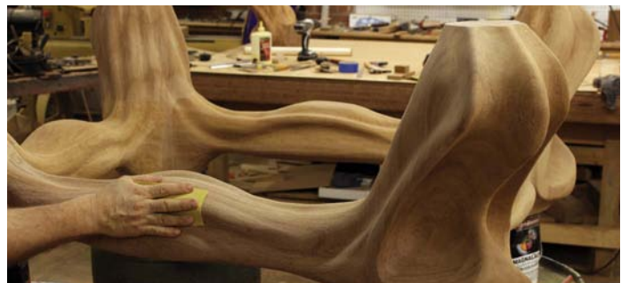
25 Hand-sanding the entire base system
