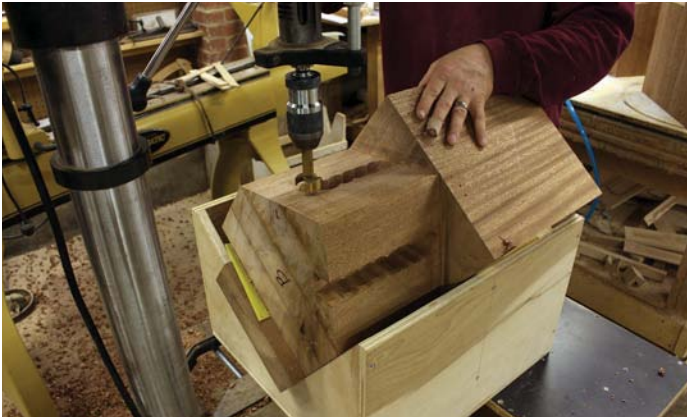
8 Drilling into the side of each leg using a 38mm diameter Forstner bit
