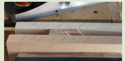
Cramp a scrap between two boards and scribble some pencil marks across the surfaces to practise the glide-to-shave technique
