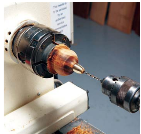
4 Drill the hole to accept the steel drill rod. Use bits 0.4mm larger in diameter than the drill rod to allow room for the epoxy
