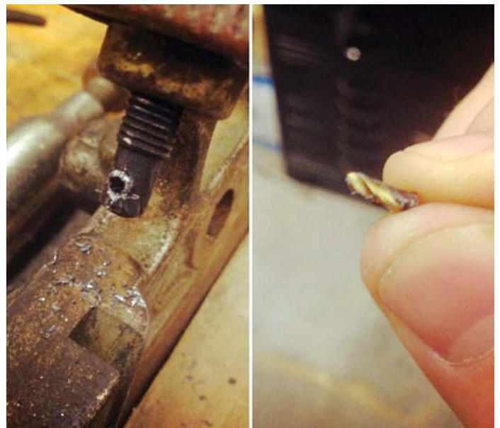
The fight to remove the iron advancement pin and broken drill bit
