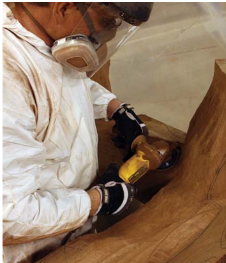
16 Grinding one leg at a time to remove the back side of the leg
