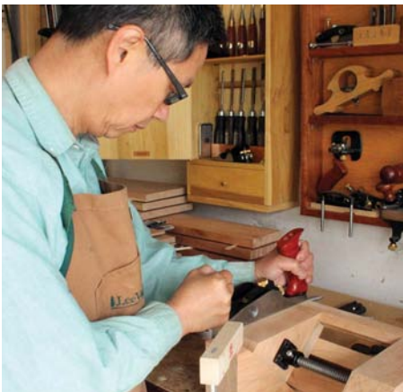
I rested the back side on the spare ramp block as I planed the bevel faces flush
