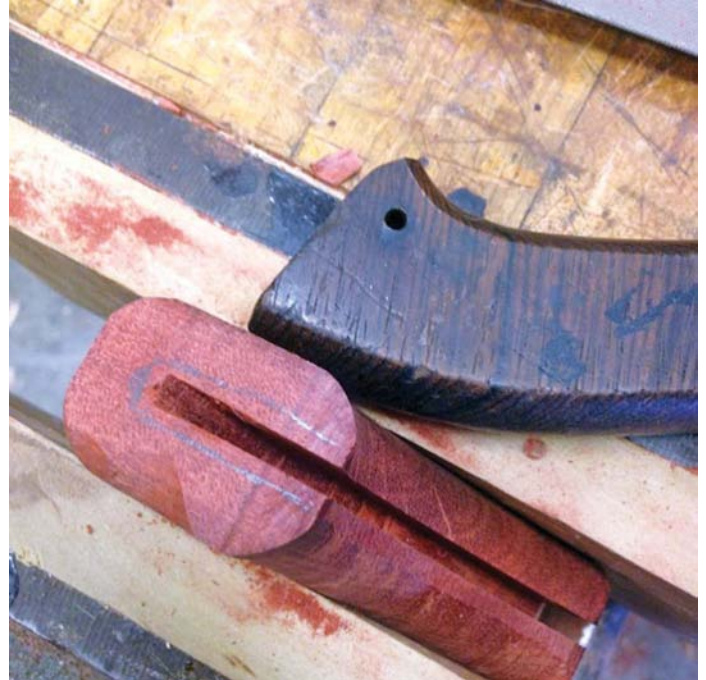
The process of fitting the new handle
