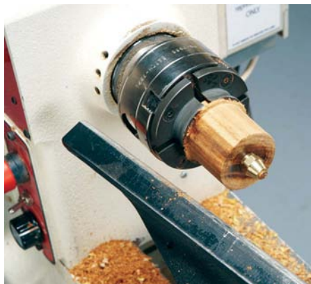
1 Round the handle blank and fit the ferrule on the end. You can use different materials for a ferrule; this one is a solid brass nut with a tapered end section
