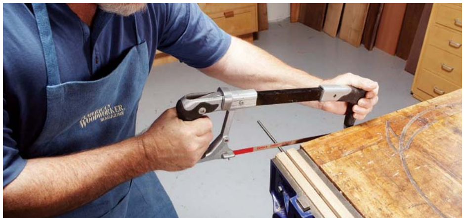
5 Make the awl's steel shaft from a piece of drill rod. Cut it to length using a hacksaw
