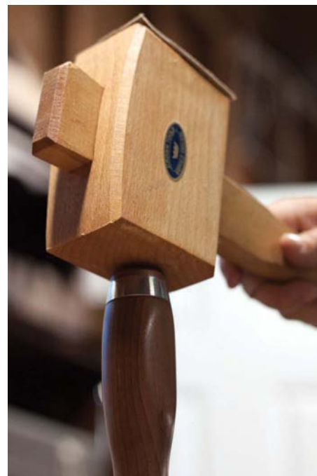
Using a joiner's mallet
