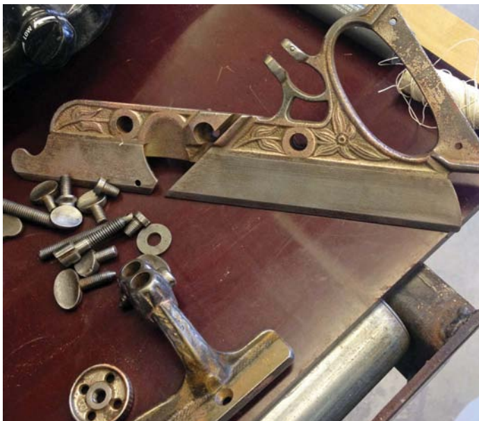
Parts sanded and ready for degreasing
