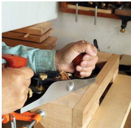
The spare ramp block was used to support the jig when I worked on truing the jaws flush and square
