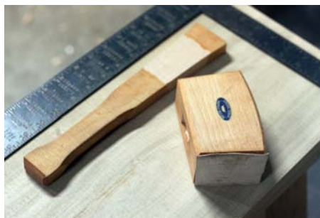
The mallet head is held on by friction
