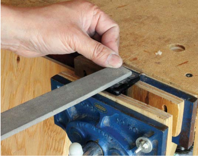
I filed the bottom of the swivel head flat and then drilled a small screw hole on each corner
