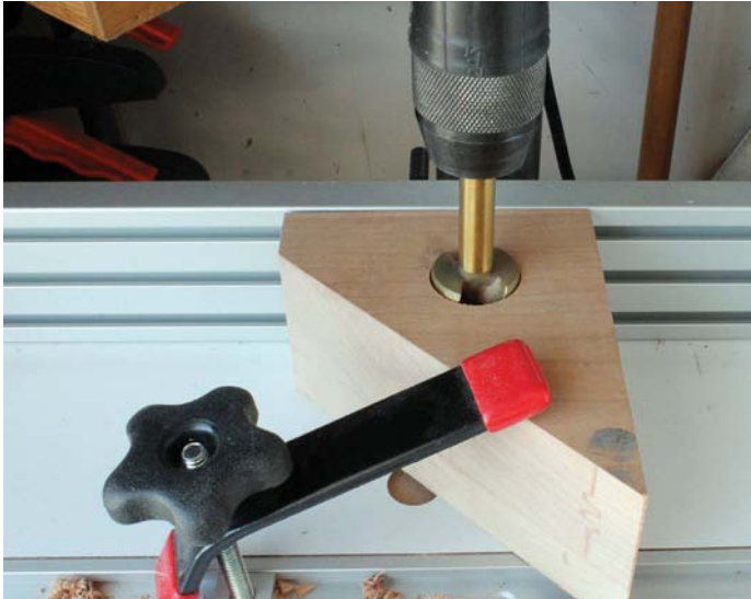
Drill the larger clearance hole for the screw collar first while the centre point is there
