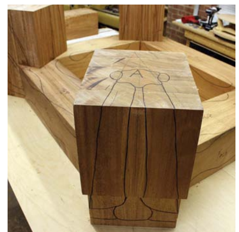
14 Using a marker pen to go over all the pencil lines drawn on the base system
