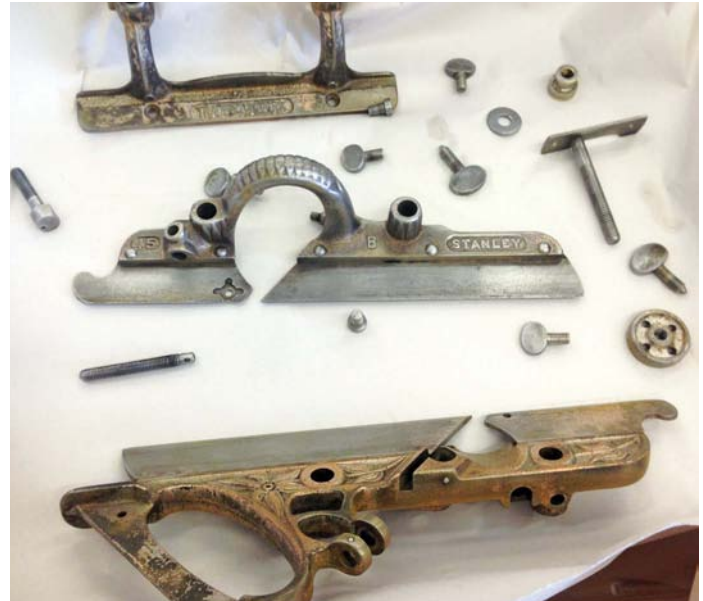
Parts degreased and ready for the nickel bath
