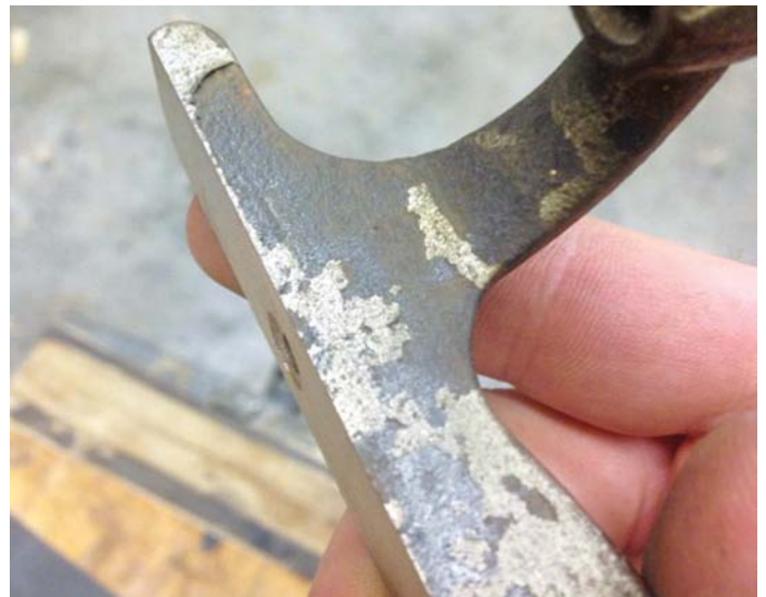
Original condition of nickel plating
