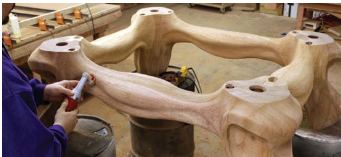
24 Smoothing out the curves and twists using a smaller grinder with a medium 50mm diameter grinding wheel
