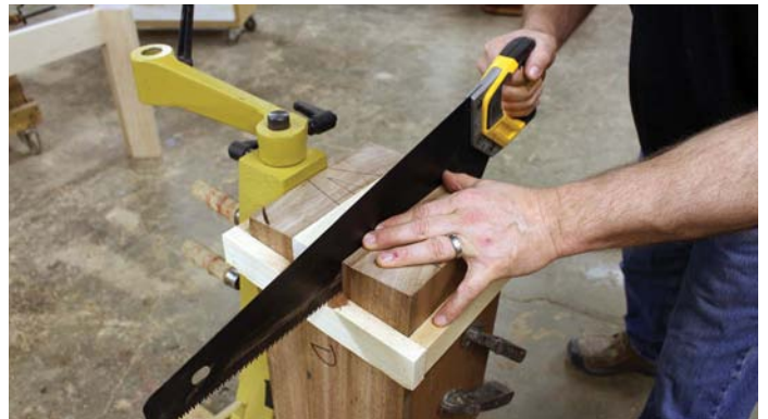
11 Cutting out each tenon into the ends of the runners
