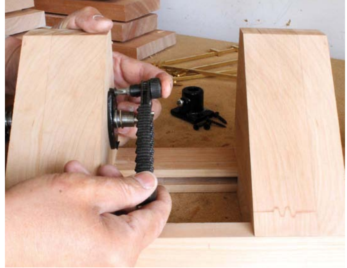
After installing the screw collar, I added the swivel head and attached it to the sliding jaw
