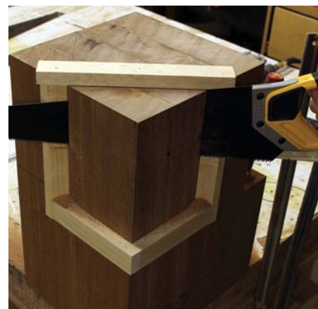
7 Cutting a 45° angle on both lower back sides of all four legs
