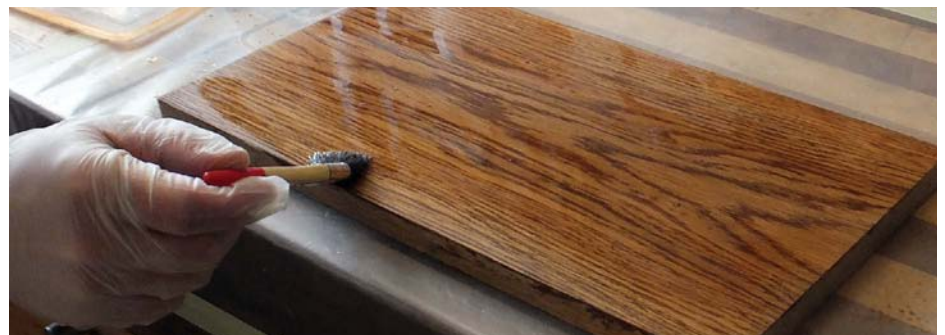
Oak will go darker than other timbers when you apply the bleach
