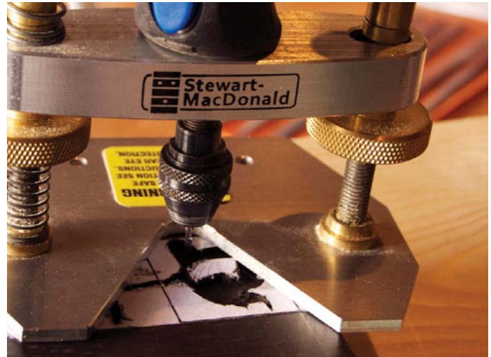
Cutting the recesses for the shell using a fine cutter in a Dremel
