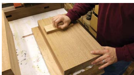
4 Sanding the blocks for the legs with a sanding block
