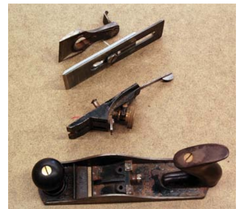
Bench plane disassembled: lever cap, chipbreaker and iron, frog and plane body
