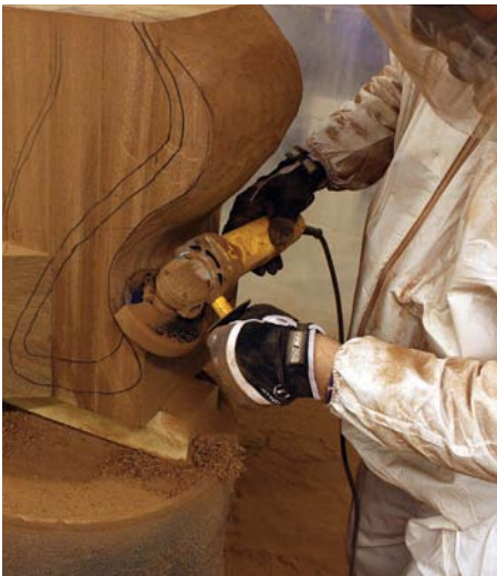
15 Using a grinding wheel with durable tungsten carbide with my hands in a safe position
