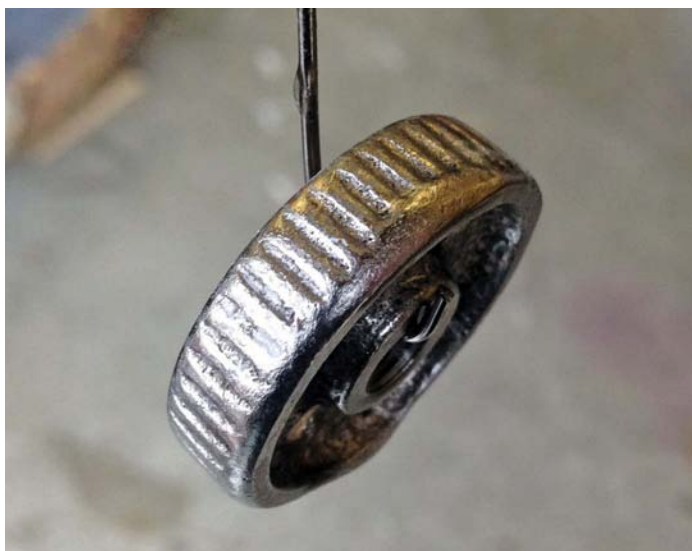
The iron advancement after 10 minutes in the nickel bath
