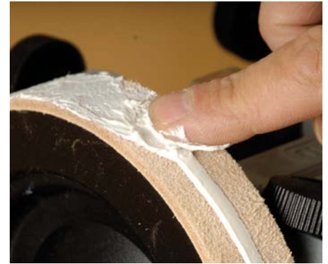
Load up a new honing wheel with paste before turning the machine on
