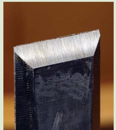
Re-grading the wheel before grinding a secondary bevel results in a finer wire edge
