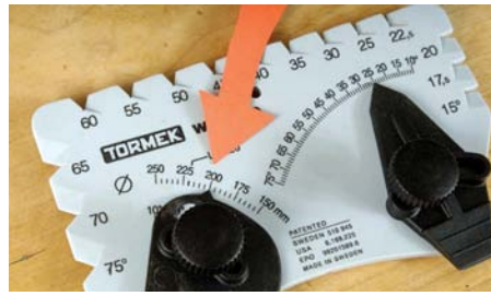
Set the first dial on the WM-200 to the diameter of the grinding wheel
