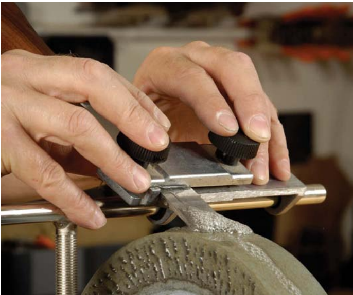
Placing a lot of weight behind the guiderail can cause it to flex. Levering the tool up to increase pressure on the wheel will have the same effect
