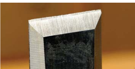
Re-grading the wheel before grinding a secondary bevel results in a finer wire edge
