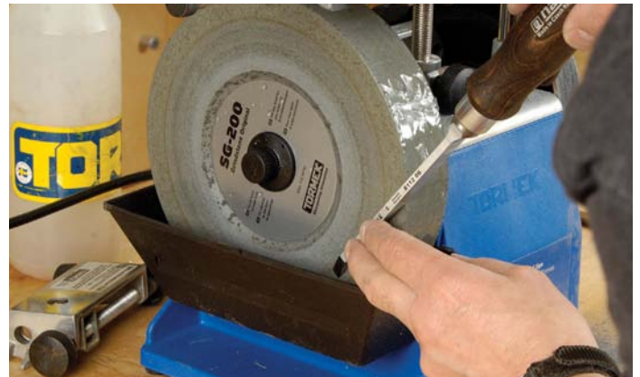
Use as much of the surface as possible to avoid making indents
