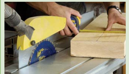
The Irwin Marples 48-tooth General Purpose blade will tackle 70mm maple with no problems
