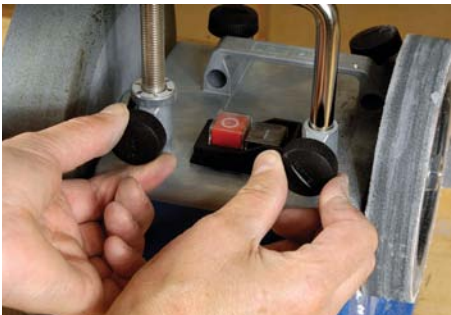
Tighten both screws to set the guiderail in place
