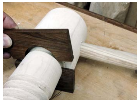
A two-piece garter is used to fix the screw thread to the vice jaw
