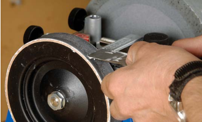
Only hone the blade from the front of the machine with the wheel rotating away from the tool edge
