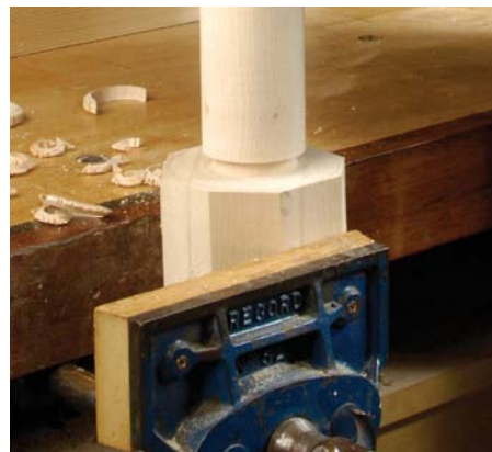
Use the flats to secure the column in your vice
