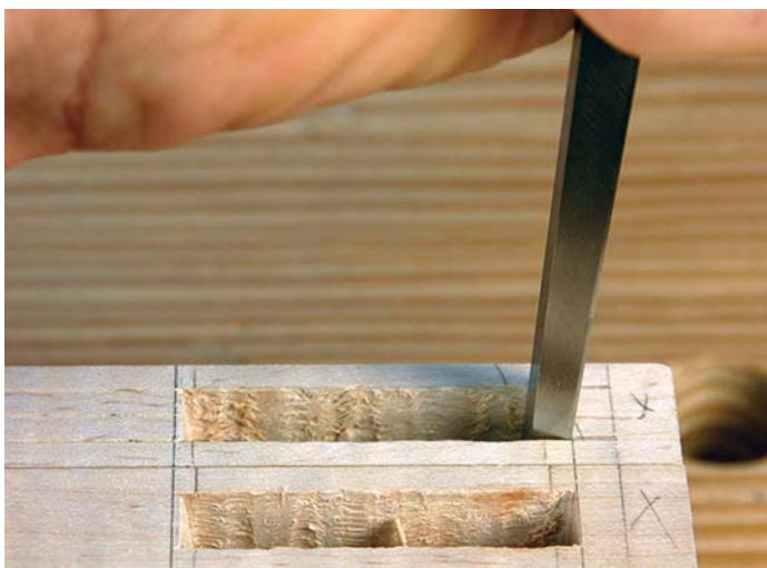
5 Tip the chisel a few degrees as shown and drive it into the work. You want to stop the taper somewhere in the middle of the mortise. Don't go all the way to the bottom
