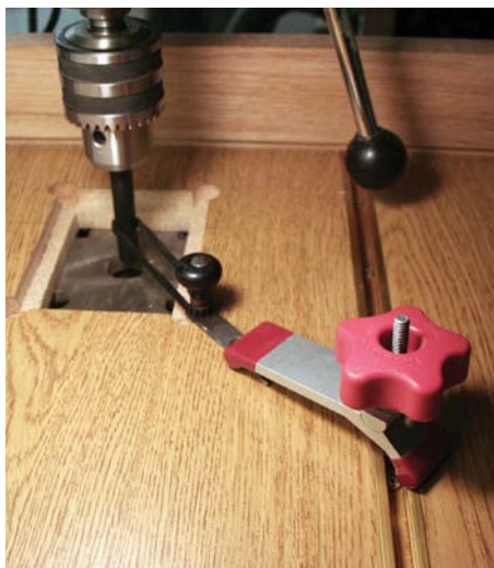
Clamp a post in the drill press and run a belt from the post to the ferrule on the crank knob. With a little tension, the knob should spin quite easily for sanding and finishing
