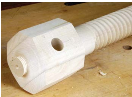
Drill through the widest part of the column
