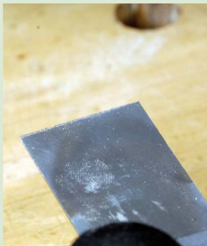
Grinding away from the tool edge leaves a long bur or wire edge
