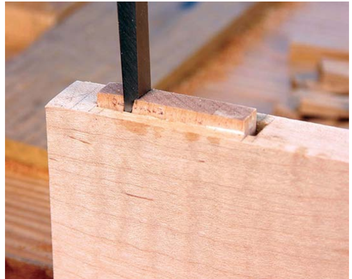
10 Drive a chisel into the end of the tenon to split it. I positioned the chisel 8mm from the end of the tenon and drove it straight down until the gap closed up
