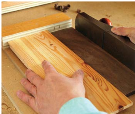
The rebate acts as both a fence and a hold-down for the long edge of the workpiece
