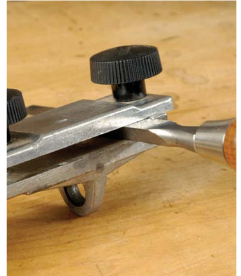
Keep the jaws of the clamping bar parallel with each other and flat across the back of the tool
