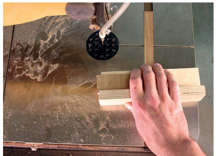
6 This jig makes wedges better than anything I know. I picked up the idea for it from Lee Valley's website – www.leevalley.com . It essentially is a sled that is skewed 4° and runs in the saw's mitre slot
