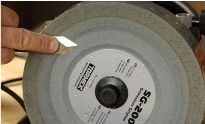
Use the side of the wheel sparingly as there is no easy way of flattening it if it becomes misshapen
