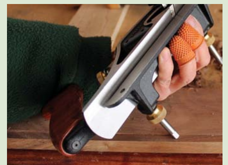
Rubber fingers offer a better grip of the metal fence as well as preventing finger cuts
