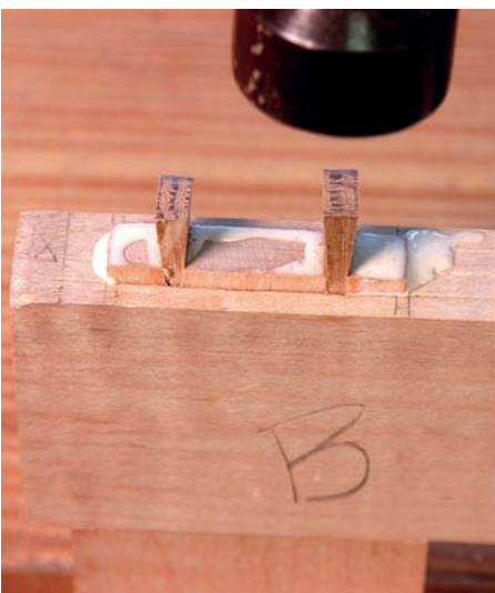
11 Add your adhesive, yellow glue or hide glue and drive your wedges into the joint. Tap them in evenly, alternating one wedge to another. The sound of the hammer hitting the wedge will change when the wedge hits bottom
