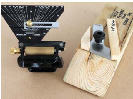
A skew jig offers repeatability and simplifies the work of setting both skew and bevel angles accurately
