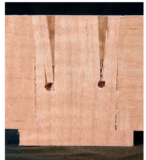
Here you can see the joint with a hole drilled tangent to the kerf – left – and centred on the kerf. In all the samples, the joints with a hole that was tangent to the kerf split back up the tenon as shown – this one filled with glue after the split
