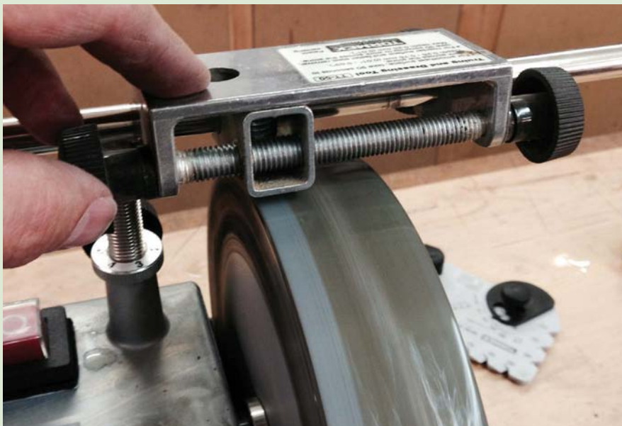
Refresh the grinding surface of the wheel at the end of each sharpening session
