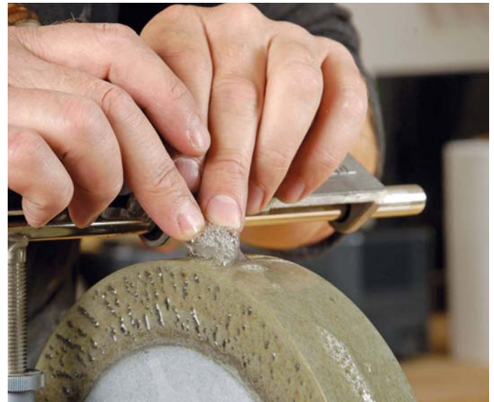
A light touch in front of the guiderail will give the best results. Use the guiderail to assist with lateral motion and not for leverage
