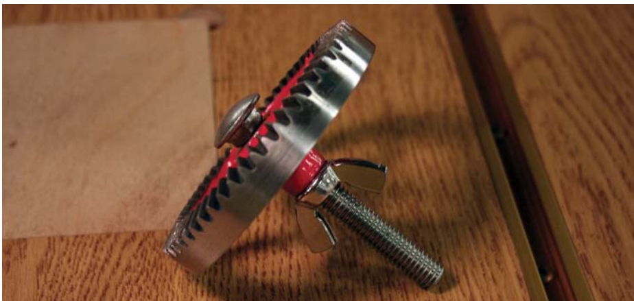
Place a snug-fitting bolt through the gear, lock it down with a nut, then chuck the entire assembly into the drill press
