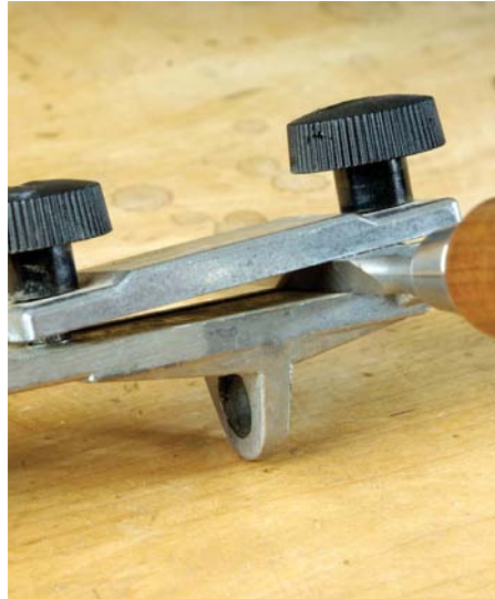
Overtightening the screws can distort the clamp and pull the tool over to one side
