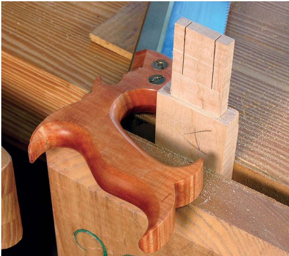
Because this tenon has a loose fit – about 3mm on either side – I used a backsaw to make the kerfs in the tenon. Note that the kerfs don't extend all the way down to the tenon's shoulder. There's no need – the wedges will only travel so far
