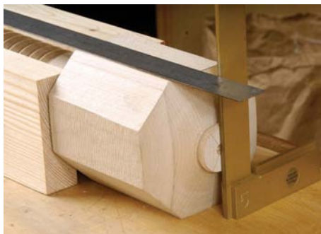
Extend the line to the centre point on the end to locate the hole for the handle
