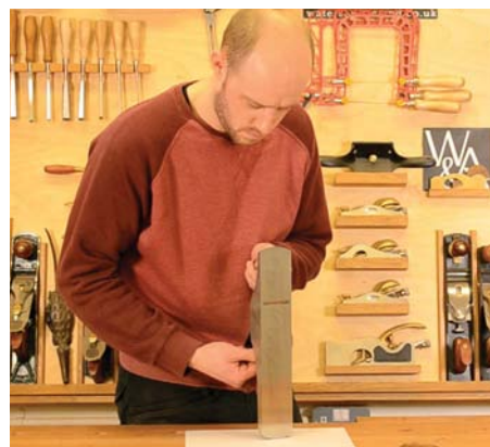
Hold the plane upside down to examine the amount of blade projection
