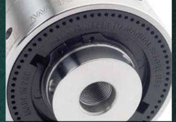
Sealed Backing Plate with Full Indexing The SC4 features a strong backing plate to protect the gear mechanism from dust and 72-point indexing around the full circumference.
