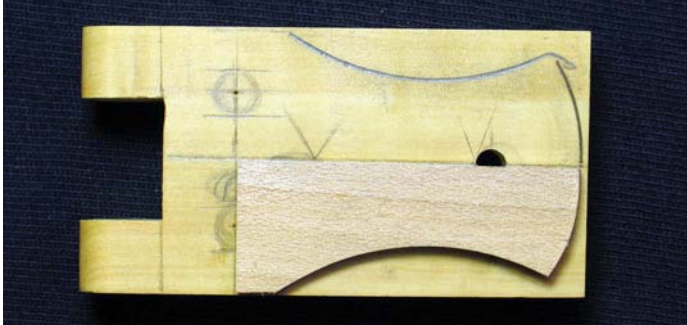
A template of half of the hinge drawn around then flipped over for the other half, ensuring symmetry
