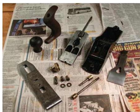
A bench plane disassembled can easily total twenty items
