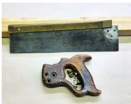
A disassembled saw will typically consist of nine items
