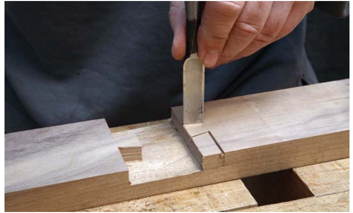
Rebated areas on either side of the dovetail pin are chopped with a vertical chisel
