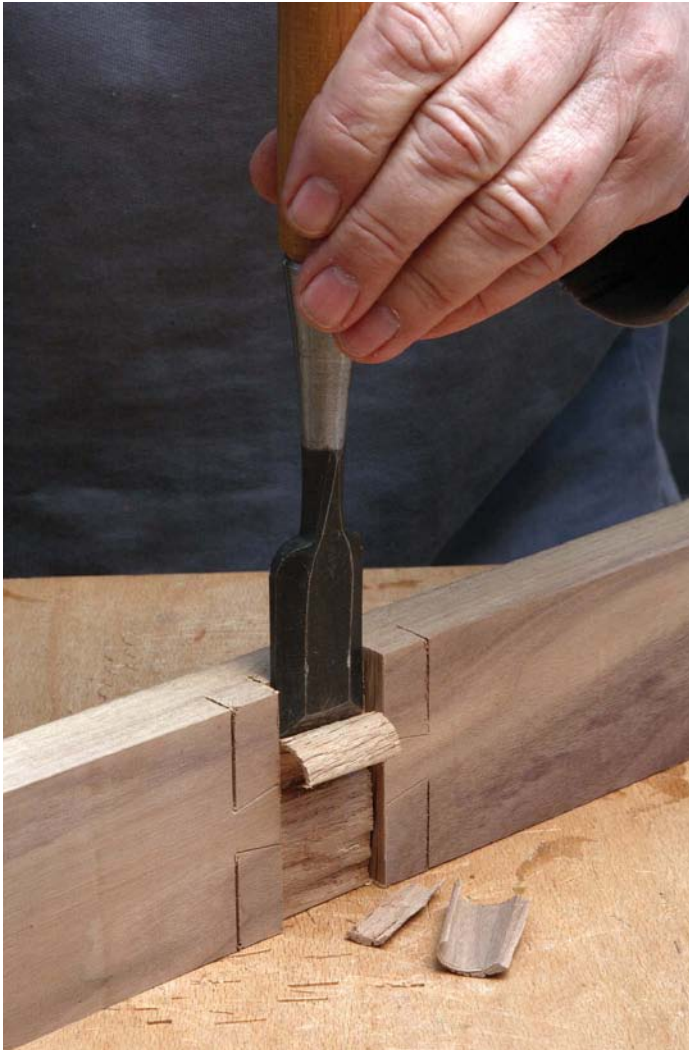
Central channel between the two opposite tail pins is pared out with a wide chisel
