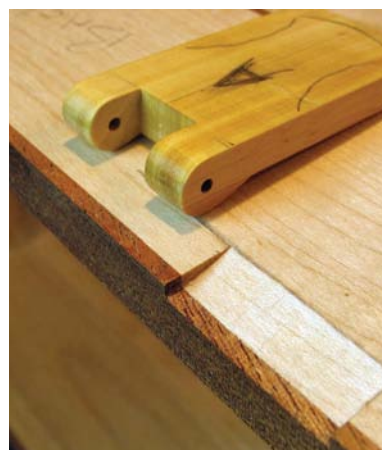
Wedge-shaped recesses cut to accept the knuckle of the hinge
