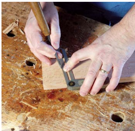
Adjustable bevels are often small enough that you can grip the handle and blade in one hand, pinching the whole tool against the rail's top edge. However you hold the tool, be sure it has not lost its setting and keep it steady while scribing the shoulders
