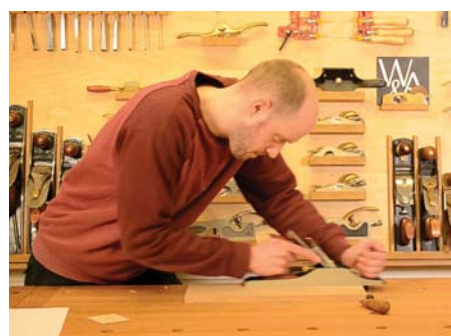
Transfer the balance of pressure to the rear tote as you complete the pass
