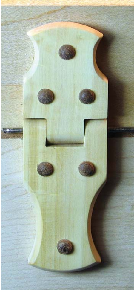
Glued and pegged with the pin in place, ready for a test opening
