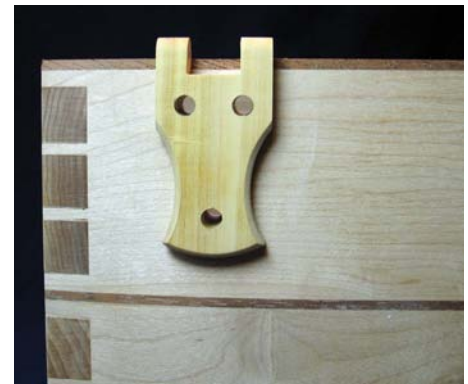
The 5mm holes ready for the pegs
