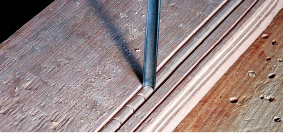
Carving is a study by itself, but this is the simplest shape to get the hang of – one tool, two moves. This form of carved work is utilised in most 17th-century carved oak
