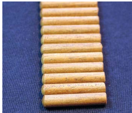
Utile pegs ready to go with one end rounded and a 'lead in' the other
