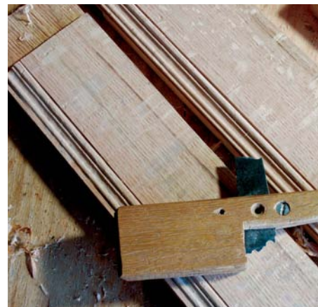
The most common form of scratch stock, this time it's made from an offcut of riven oak. You can cut a shape on each end of the blade, then switch it around for a different moulding. Make these as you need them. The price is right, as is its effectiveness and ease of use
