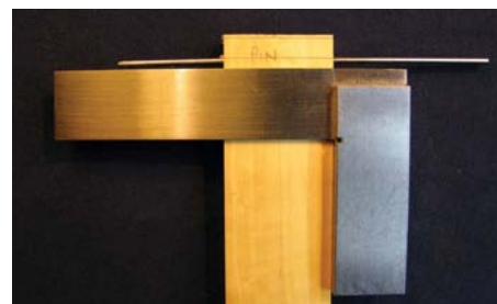
With the pin in the hole, the squareness can be checked
