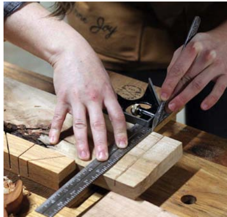
Mark the sides with a combination square and knife
