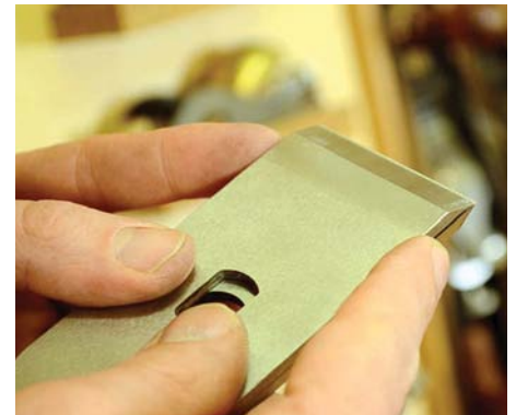
Align the sides of the blade with the chipbreaker
