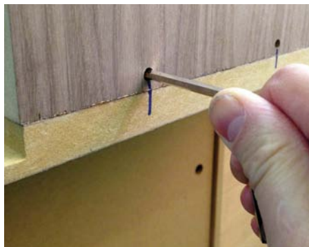
Align the components and lock into place with a hex key
