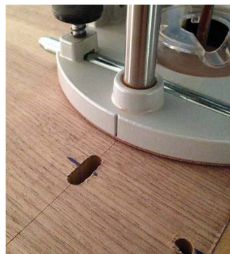
Rout slots in the carcass top so the bolts can move freely if so required
