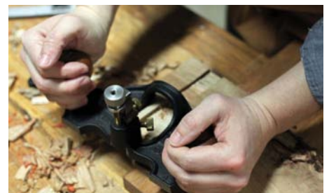
Meet in the middle to avoid blowout
