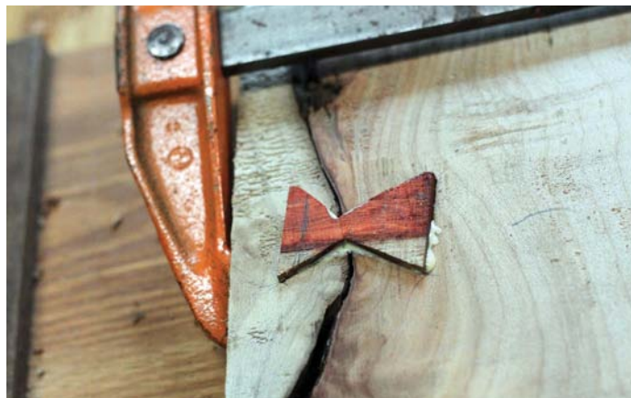
Clamp the joint tightly
