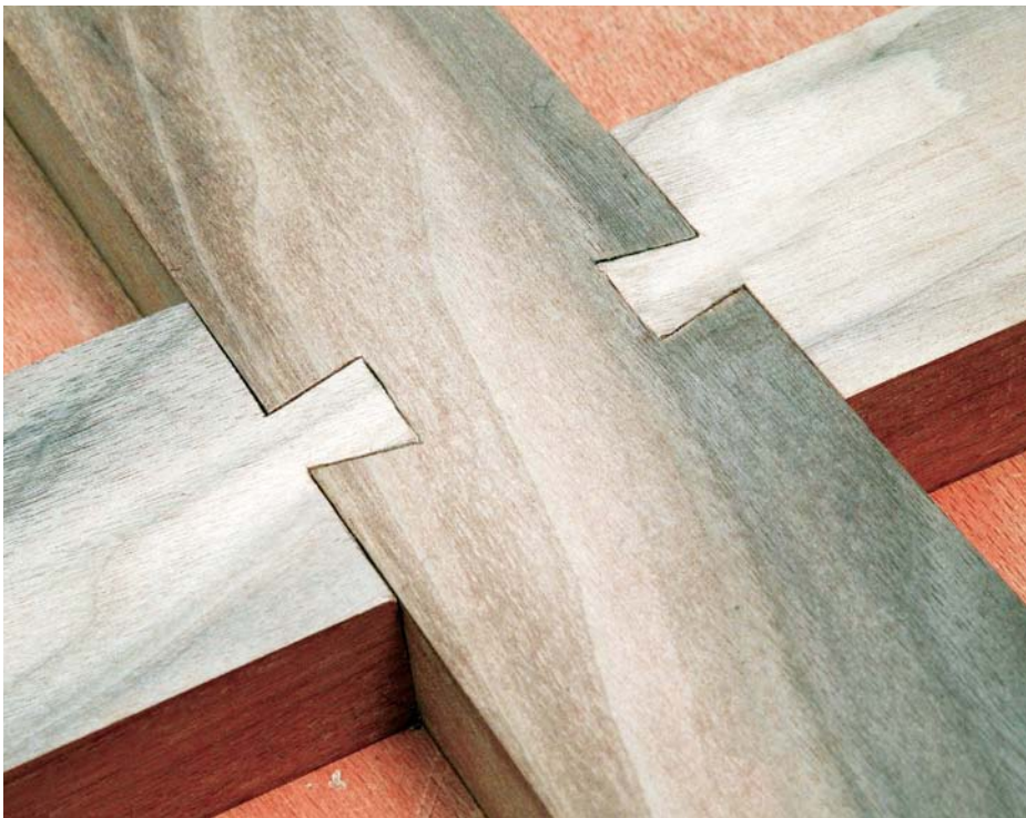
The Shi-ho-ari-kumi-te dovetailed cross lap joint is trial fitted ready for gluing
