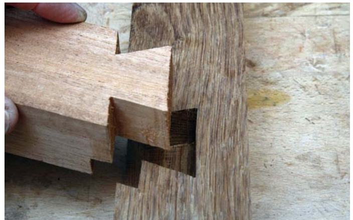
Two halves of the Hiuchi-ari-otoshi are fitted together, leaving the dovetail pattern visible on one side of the joint only
