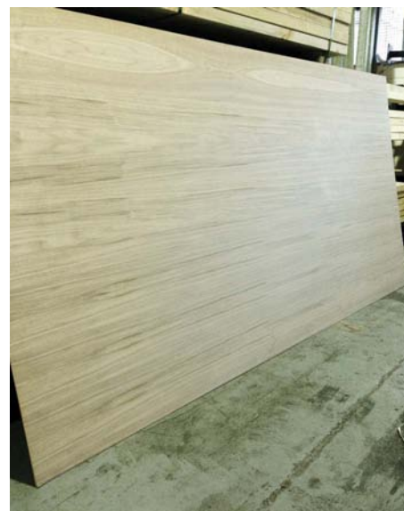
A quartersawn face. Note the slight pattern at the top of the board
