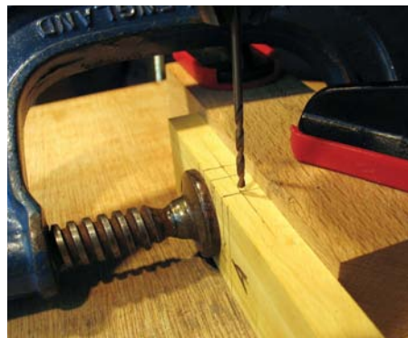
The pin holes drilled while the hinge was cramped to a right angle block. Slightly oversize wood ready to make the inevitable corrections
