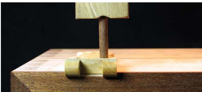
The pegs tapped in until the flat of the notched 'punch' reached the hinge, leaving them standing uniformly proud
