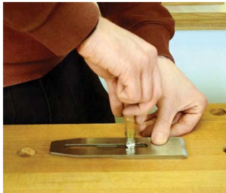
Rest your blade and chipbreaker on a hard surface
