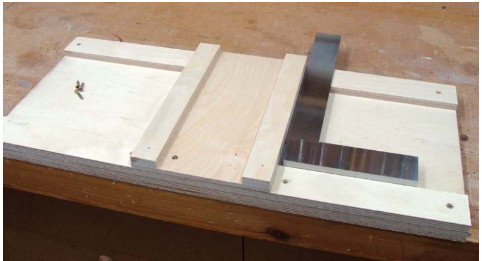
The rebate jig is very simple to make and the only thing requiring particular attention is that the router guide must be mounted square to the longitudinal fences. The jig took less than half an hour to make from offcuts
