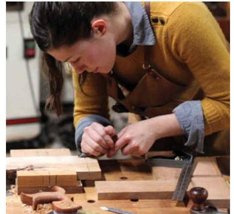
Create a 'V' groove for the saw
