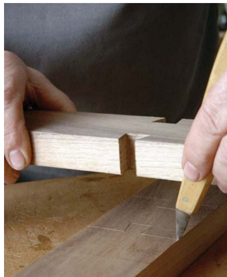
The full-depth socket pattern on one rail is used as a template to knife-mark to other rail
